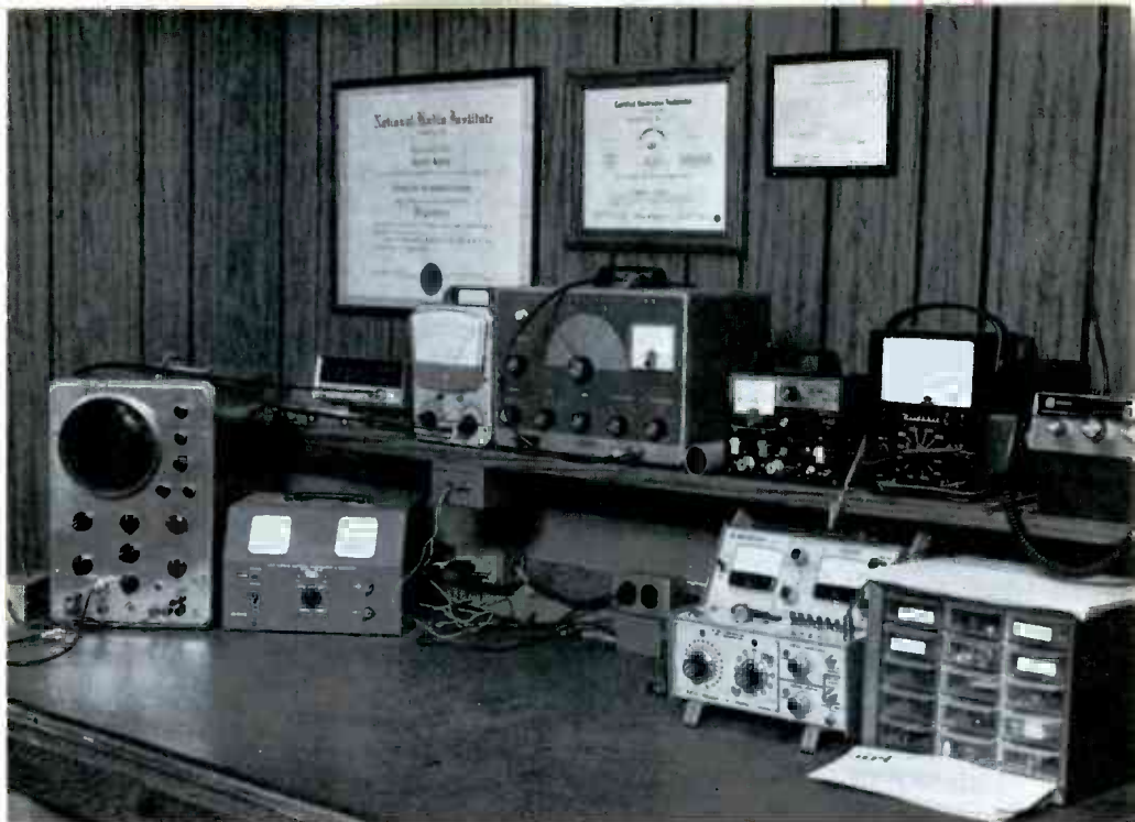
FIGURE 3. (L. TO R. ON SHELF) HEATHKIT IB1100 FREQUENCY COUNTER, CONAR MODEL 211 VTVM, HEATHKIT IG42 SIGNAL GENERATOR, JOHNSON TRANSCEIVER TESTER, HEATHKIT MODEL MM1 MULTIMETER, AND JOHNSON 123A CB TRANSCEIVER. (L. TO R. ON BENCH TOP) CONAR MODEL 250 OSCILLOSCOPE, EICO MODEL 1060S BATTERY ELIMINATOR, AND NIKOLTRONIX CB ANALYZER.
