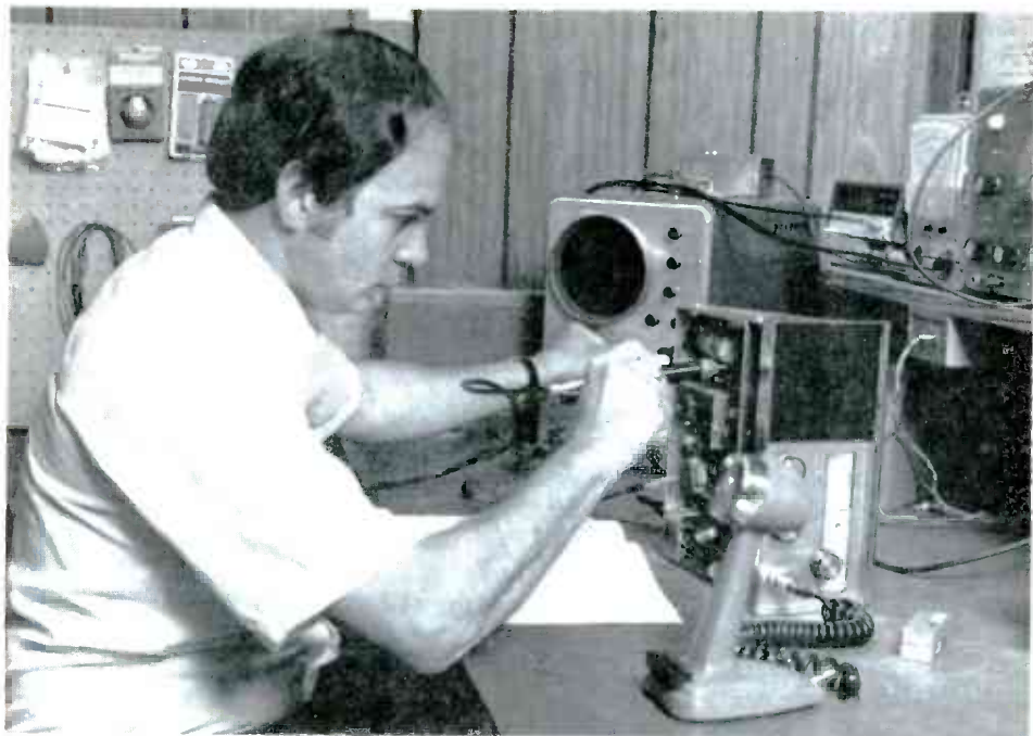
FIGURE 5. CHECKING POWER SUPPLY RIPPLE IN JOHNSON 223 TRANSCEIVER USING OSCILLOSCOPE.
