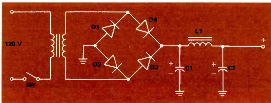
FIGURE 3. DIODE BRIDGE RECTIFIER.
