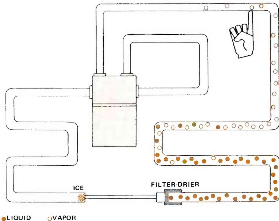
FIGURE 4. MOISTURE IN THE SYSTEM WILL CAUSE ICE TO FORM AND BLOCK THE REFRIGERANT FLOW AT THE CAPILLARY TUBE. THE CONDENSER WILL FEEL COOL.
