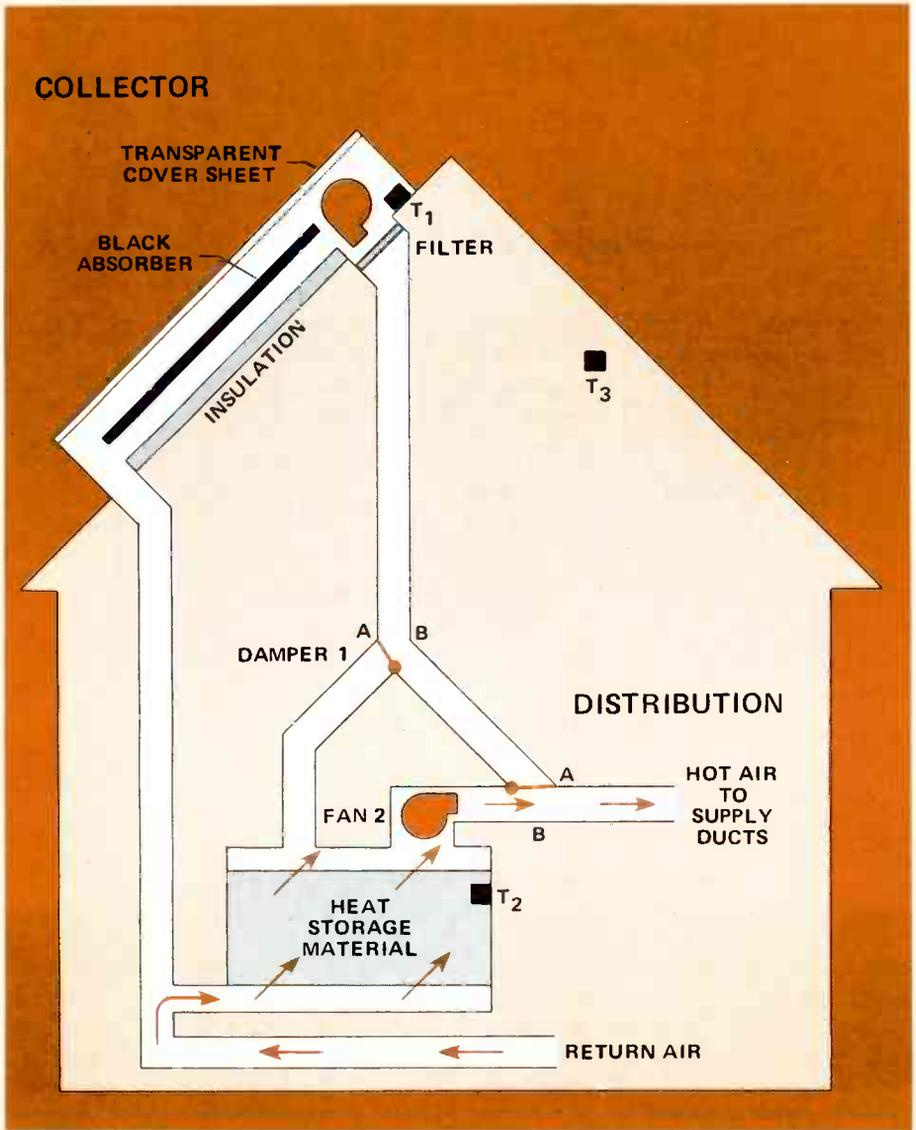
FIGURE 3. HEATING FROM THE STORAGE.
