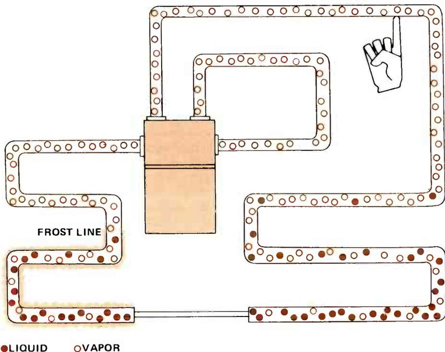
FIGURE 2. A PARTIAL LOSS OF REFRIGERANT. THE CONDENSER TEMPERATURE WILL FEEL ABOUT NORMAL.
