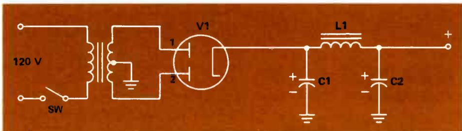
FIGURE 1. FULL-WAVE RECTIFIER.
