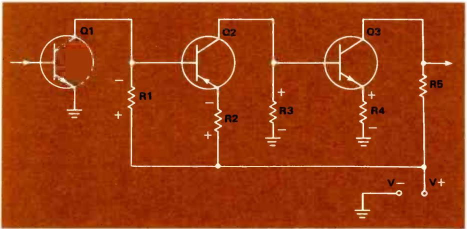
FIGURE 7. THREE-STAGE TRANSISTOR AMPLIFIER.
