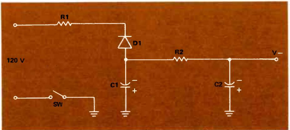
FIGURE 8. A HALF-WAVE RECTIFIER PRODUCING A NEGATIVE VOLTAGE.
