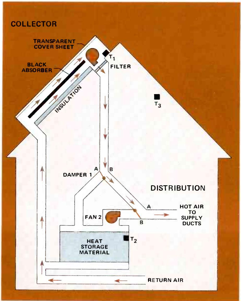
FIGURE 1. HEATING DIRECTLY FROM THE COLLECTOR.
