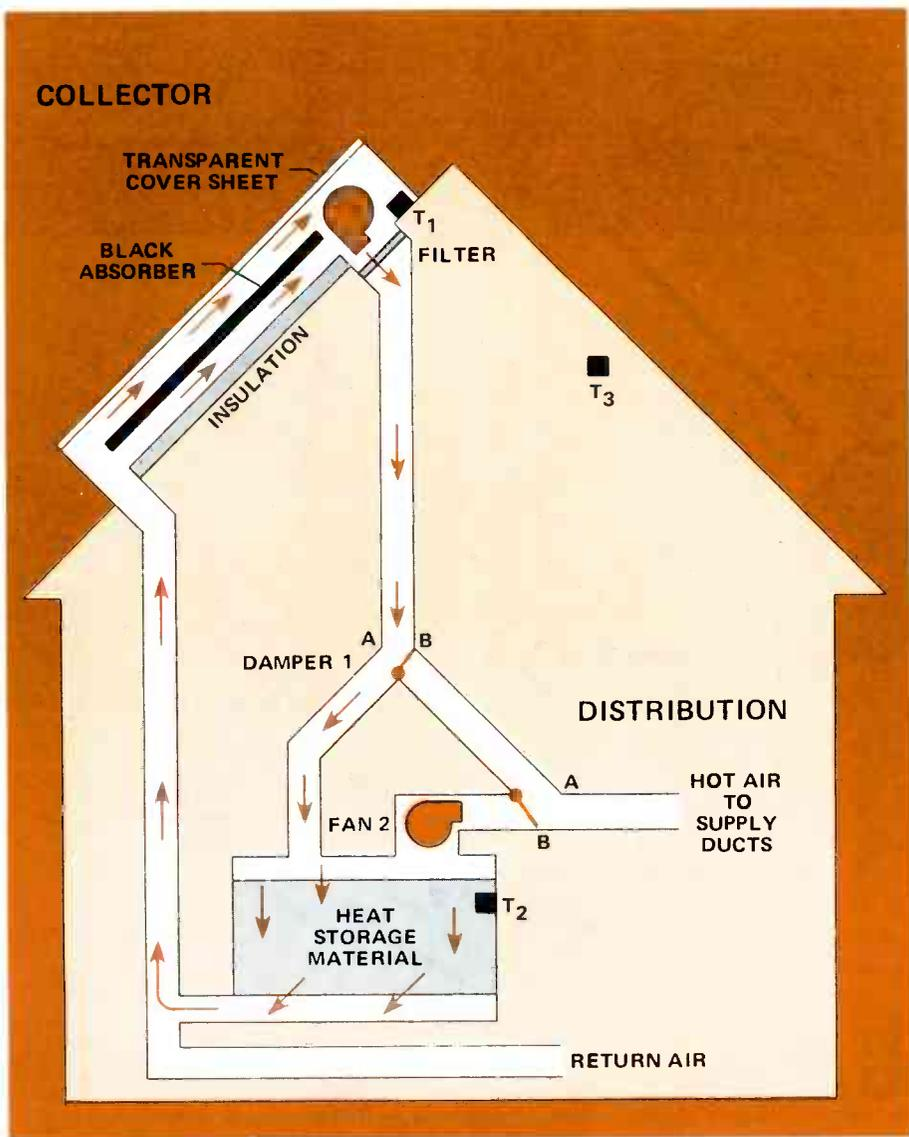
FIGURE 2. STORING HEAT FROM THE COLLECTOR.
