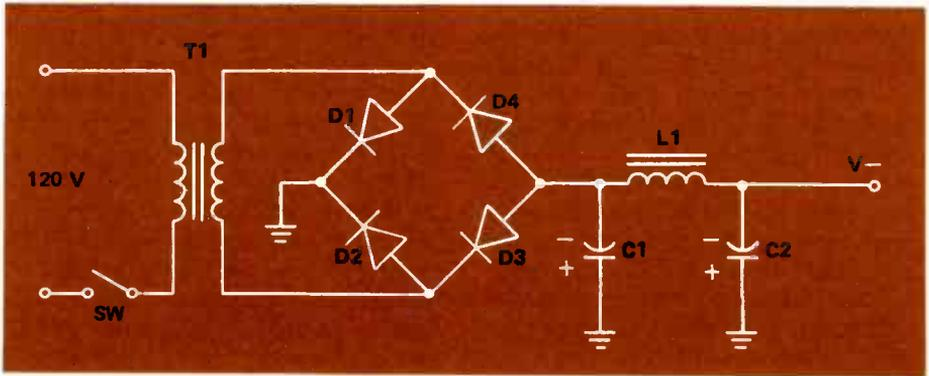
FIGURE 9. A FULL-WAVE RECTIFIER PRODUCING A NEGATIVE VOLTAGE.
