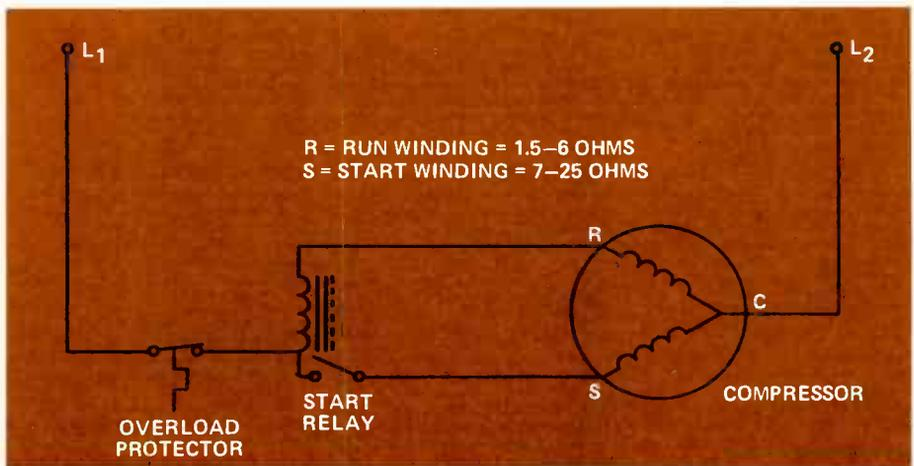
FIGURE 5. THE ELECTRICAL DIAGRAM FOR THE COMPRESSOR.
