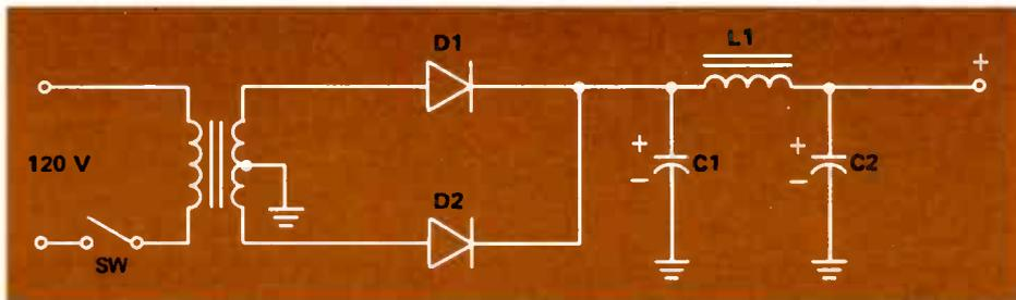
FIGURE 2. DIODE FULL-WAVE RECTIFIER.
