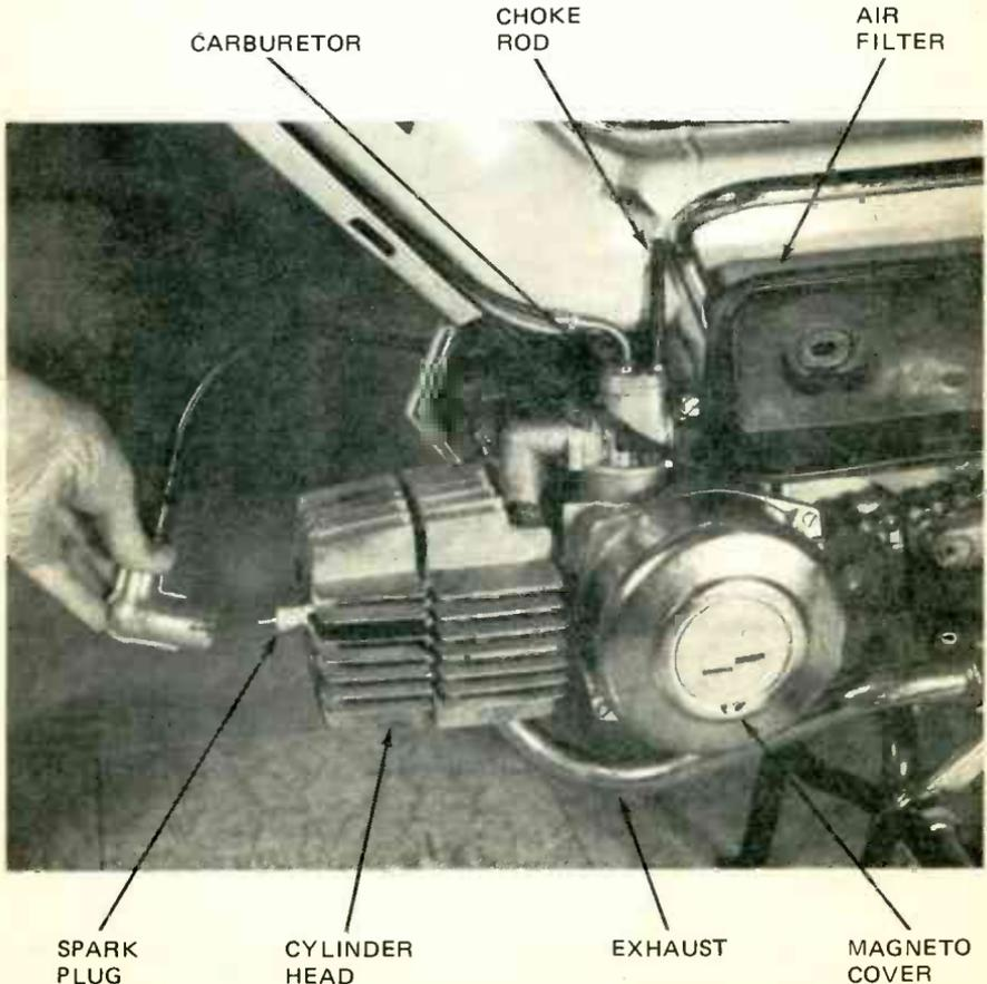
FIGURE 3. VIEW OF THE MOPED ENGINE AND CARBURETOR.
