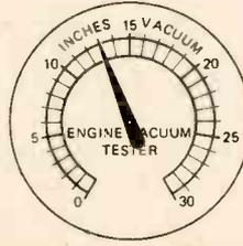
An intake manifold gasket air leak will lower the reading from 3" to 9" Hg.
