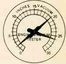
Piston ring defects can be determined by a low reading on the gauge when the throttle is closed rapidly after speeding up the engine.
