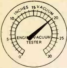
A normal engine will show a gauge reading of 18-22" Hg, with the needle remaining quite steady.
