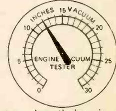
Late valve timing is evidenced by a low, steady reading, but lower than late ignition timing.
