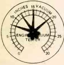
A blown cylinder head gasket will cause sharp drops of the needle.
