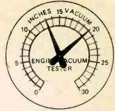
A burned valve will cause the needle to drop sharply each time the valve tries to close.
