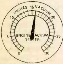
Late ignition timing is evidenced by a low but steady reading.
