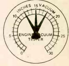
A rich air-fuel mixture on idle will cause the needle to drift back and forth.
