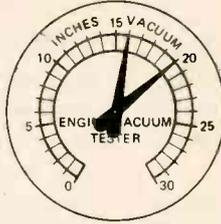
A sticky valve will cause the needle to drop sharply each time the valve tries to close, but not as much as the burned valve.
