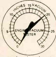
A restricted exhaust will cause a momentary stop to the return of the needle when the throttle is closed quickly.
