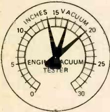
Worn valve guides admit air, which upsets carburetion. The needle will fluctuate slowly.
