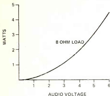
**FIGURE 3.** AUDIO VOLTAGE VS AUDIO POWER FOR AN 8 OHM LOAD.
