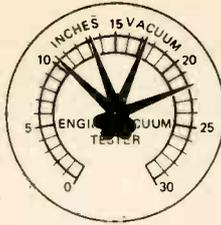
Weak valve springs will cause wide fluctuations of the needle.
