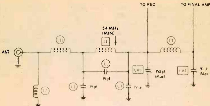
FIGURE 4. RF OUTPUT NETWORK OF GTX2300.
