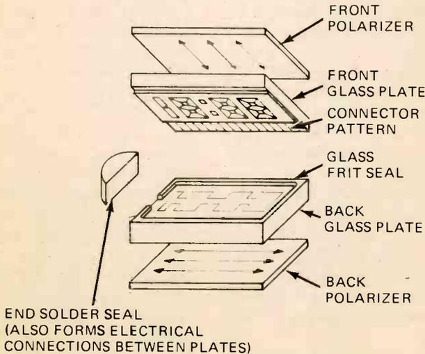
FIGURE 1. LIQUID CRYSTAL CELL STRUCTURE.
