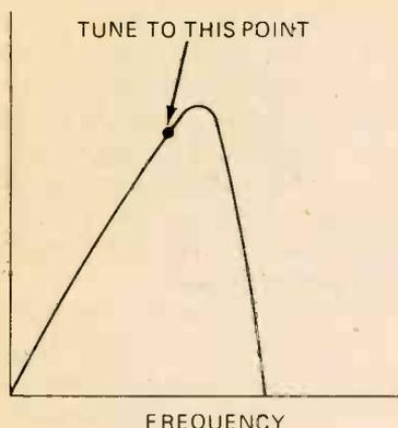
FIGURE 1. PROPER POINT FOR TUNING THE SYNTHESIS OSCILLATOR COIL IN GEMTRONICS GTX-36.
