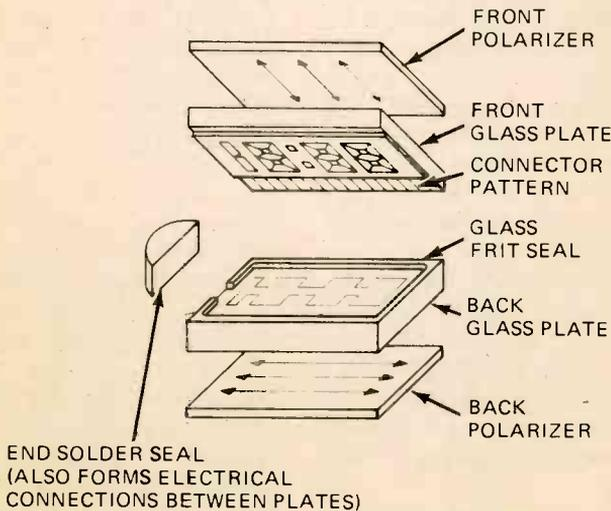
FIGURE 1. LIQUID CRYSTAL CELL STRUCTURE.
