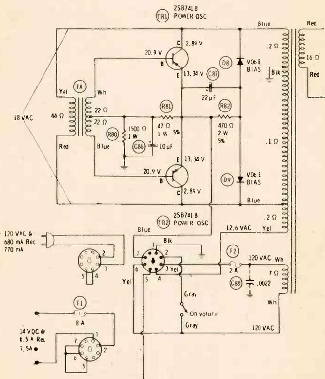
FIGURE 2. GTX-2300 POWER SUPPLY.
