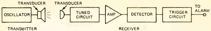
FIGURE 6. A BLOCK DIAGRAM OF AN ULTRASONIC TRANSMITTER AND RECEIVER.
