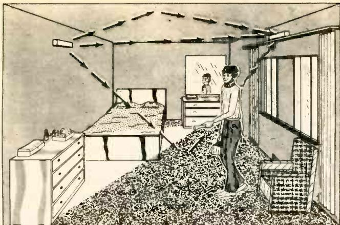
**FIGURE 4.** DIRECT AND REFLECTED SOUND WAVES COMBINE TO FORM A CONSTANT FREQUENCY AT THE RECEIVER. ANY MOVEMENT CAUSES A CHANGE IN THAT CONSTANT FREQUENCY.
