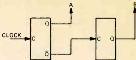
FIGURE 1. A 2-BIT BINARY COUNTER USING JK-TYPE FLIP-FLOPS.
