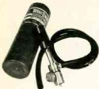
Compact and lightweight, this halide gas leak detector has an accuracy of almost 100 parts per million of any chlorinated refrigerants, such as Freon, Carrene, methyl chloride, and ethyl chloride. One valve for positive flame control. Lights instantly, with brilliant color changes. Valve and burner parts are all brass.
