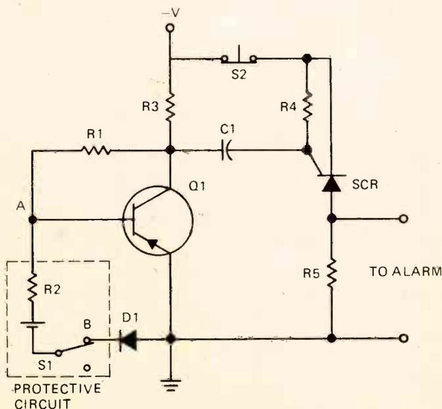
FIGURE 1. A TYPICAL ELECTROMECHANICAL ALARM CIRCUIT.
