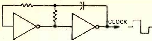
FIGURE 2. AN ASTABLE MULTIVIBRATOR SQUARE WAVE OSCILLATOR.
