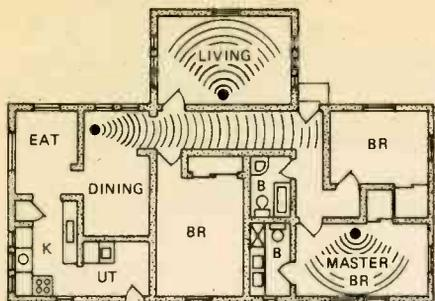
**FIGURE 7. AN EXAMPLE OF ULTRASONIC DETECTOR PLACEMENT. THE CONTROL DETECTOR IS PLACED IN THE CENTRAL HALLWAY AND TWO "SLAVE" DETECTORS ARE SET UP IN ROOMS WHERE VALUABLES ARE KEPT.**
