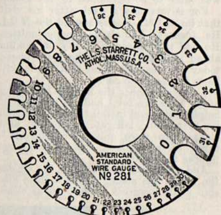
Fig. 1.—A Pocket Wire Gauge which can be purchased from any hardware store handling copper wire.
