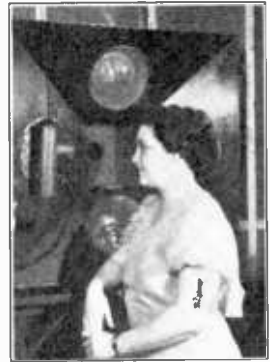
Matilda Biglow Russ, Radio soprano, before Television Camera. Circular openings in camera frame contain photo-electric tubes which convert light into electrical impulses.
