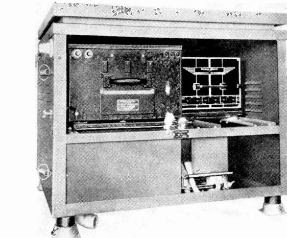
Cabinet assembly of Marine Radiotelephone equipment, housing the transmitter, (upper left), the receiver, (upper right), and below, the junction box and selector set. (Photo Western Electric)
