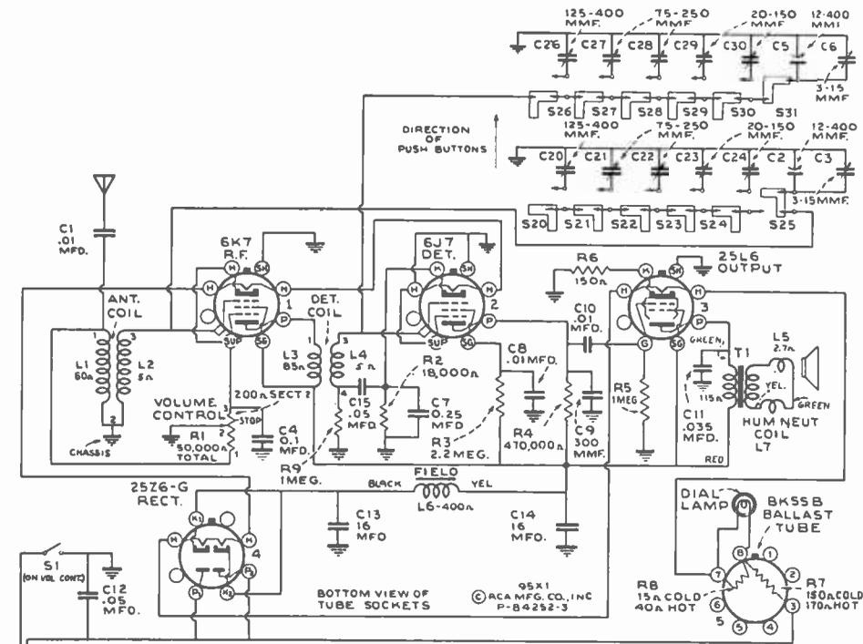
⚡ Schematic Circuit Diagram. The line by-pass, C12, is changed to .25 mfd. (Stock No. 12484) in some sets.
