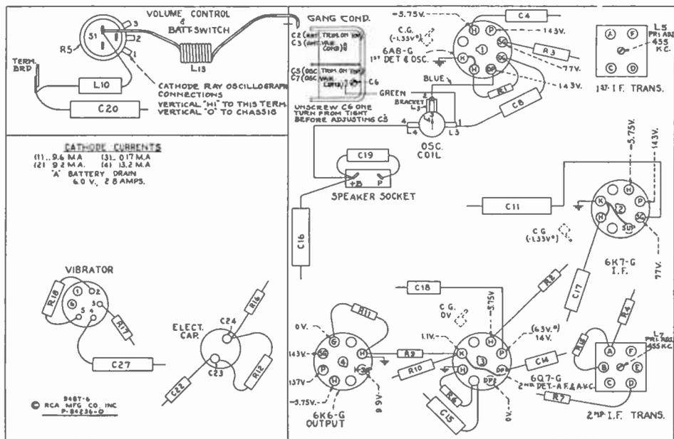
\*Note: Values with star (\*) are operating voltages. Values not starred are actual measured voltages. Measurements made to chassis unless
