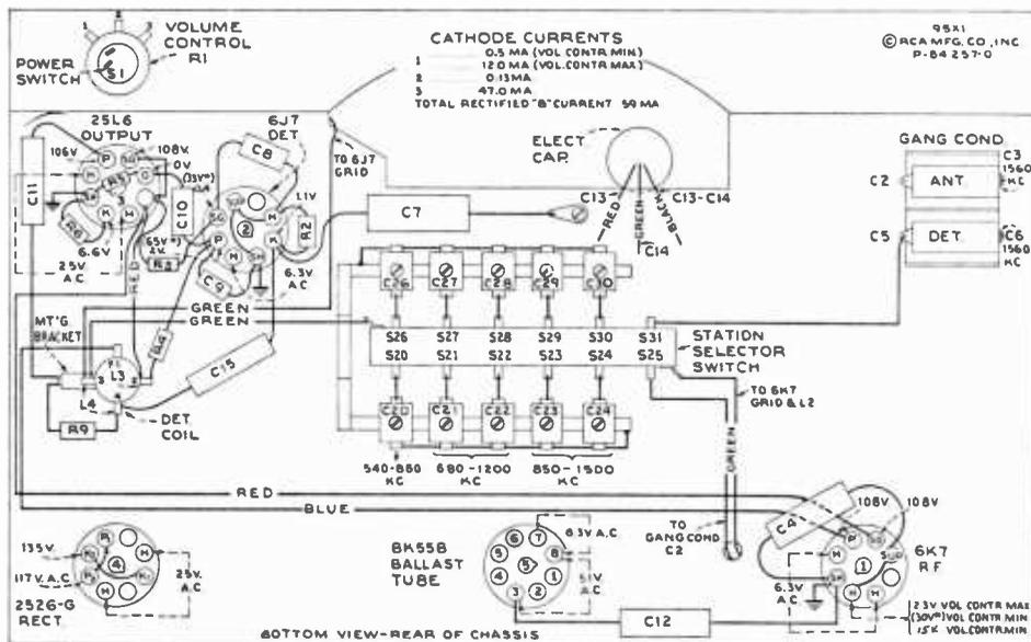
**RADIOTRON SOCKET VOLTAGES, AND LOCATION OF PARTS**
