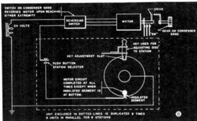
FIG. 7. RCA electro-mechanical automatic tuning system. Shaft coupling units are designated as BB.
