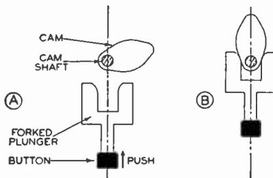
FIG. 4. Egg-shaped cam and plunger mechanism used in the mechanical automatic tuning systems of some Philco receivers.
