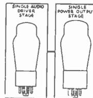
11. *One Driver Stage and Single Power Output Stage.* This combination is the simplest audio amplifier that can be incorporated in a radio receiver providing loudspeaker reception. The undistorted volume that can be secured is low, which means that overloading and blasting occurs if the volume control is advanced beyond low volume levels.
