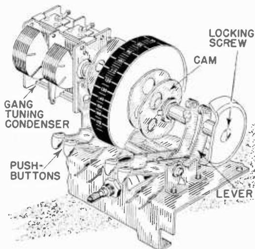
FIG. 4. Typical cam-and-lever mechanism employed in mechanical automatic tuning systems.
