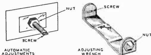
FIG. 2A. Example of coaxial adjustments sometimes used for electrical automatic tuning systems, with special adjusting wrench. On Zenith sets, the center or screw adjustment controls the oscillator, while the nut controls the antenna or input tuned circuit.
