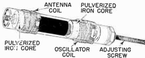
FIG. 2B. Example of dual permeability tuned coil, which requires only a single screwdriver adjustment of the center screw when setting up a push-button. Parts of the coil are cut away or shown in phantom view for clearness. Rotation of the adjusting screw makes the pulverized iron cores slide in or out of the coils, thus changing the inductance of each coil. One coil like this is provided for each station-selecting button.
