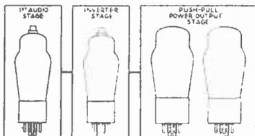
13. *One Audio Stage, Inverter Stage and Push-Pull Output Stage.* This combination, with a distortionless phase inverter stage, provides much cleaner reproduction at all degrees of volume, especially from fine recordings which are recorded at low level, and are therefore difficult to reproduce perfectly on any but a very good audio amplifier.
