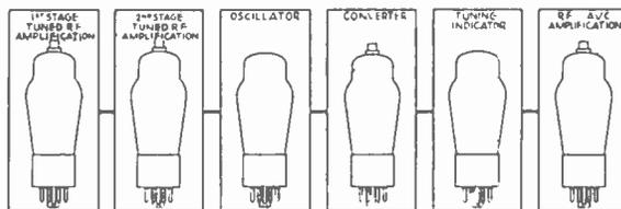
6. *Two Tuned R.F. Stages, With Separate Converter Tubes for Oscillator, Mixer-First Detector, Tuning Indicator, and A.V.C. Amplification.* The additional r.f. stage makes this combination the most efficient and highly developed antenna and r.f. section it is possible to incorporate in a radio receiver for entertainment purposes. It provides extremely quiet reception from all stations (when used with two or more i.f. stages) with a minimum of station interference.
