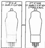
8. *Two Stages of I.F. Amplification, With Second Detector and A.V.C. System.* This combination provides better selectivity (ability to separate interfering stations) than a receiver using only one i.f. stage. The increased sensitivity will give greater distance-getting ability and better a.v.c. action than a receiver with only one i.f. stage.
