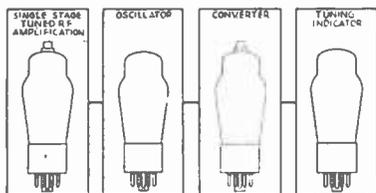
4. *One Tuned R.F. Stage, With Separate Tubes for Mixer-First Detector and for Oscillator, and With Tuning Indicator.* By using a separate tube
