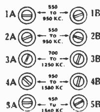
FIG. 1. Typical arrangement of adjusting screws for electrical automatic tuning systems. The left-hand (A) screws are for oscillator trimmers, and the right-hand (B) screws are for antenna trimmers. This diagram is for an auto radio receiver in which the buttons are arranged vertically; in home radios, however, the buttons are usually arranged horizontally.
