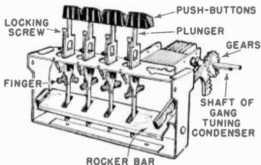
FIG. 3. Typical rocker bar mechanism employed in mechanical automatic tuning systems.
