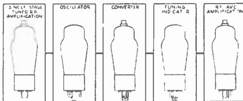
5. *One Tuned R.F. Stage, With Separate Tubes for Oscillator, Mixer-First Detector, Tuning Indicator and A.V.C. Amplification.* This combination provides a very good signal, giving quieter and clearer reception from all stations, because full sensitivity is available for weak signals and overloading is prevented on strong signals by the amplified a.v.c. action.
