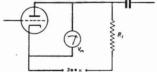
Fig. 3. A practical voltage-measuring problem. The meter reading depends on the ohms-per-volt sensitivity of the meter.
