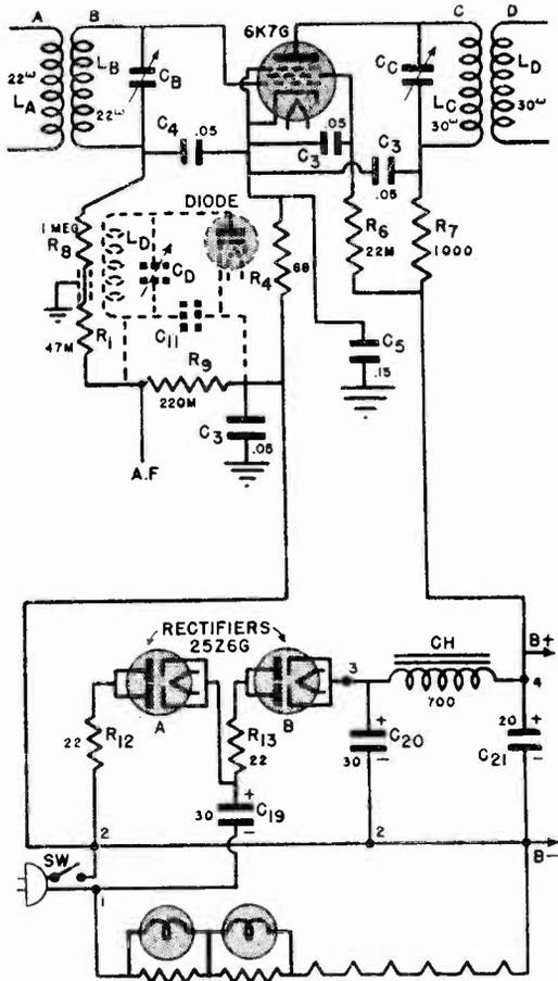
Fig. 8. Power supply and i.f. stage used in the Zenith model 5719. The diode detector circuit has been drawn in dotted lines to show its relationship to the grid return circuit of this i.f. stage. Note that the manufacturer has identified parts having the same electrical value with the same code number. This is the reason for the three .05-mfd. condensers being identified as  $C_3$ .
