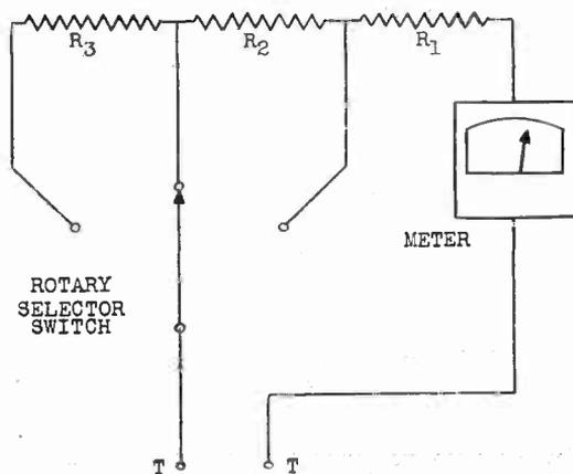
Fig. 1. Schematic of multirange voltmeter using rotary range selector switch.
