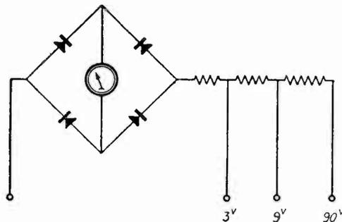
Fig. 6. A d.c. meter, properly connected to a copper-oxide rectifier and series resistors make a multi-range a.c. voltmeter.
