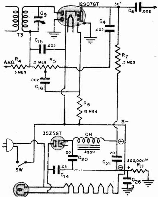
Fig. 10. Power supply and detector-first a.f. stages of the Emerson FC-400 universal a.c.-d.c. receiver.
