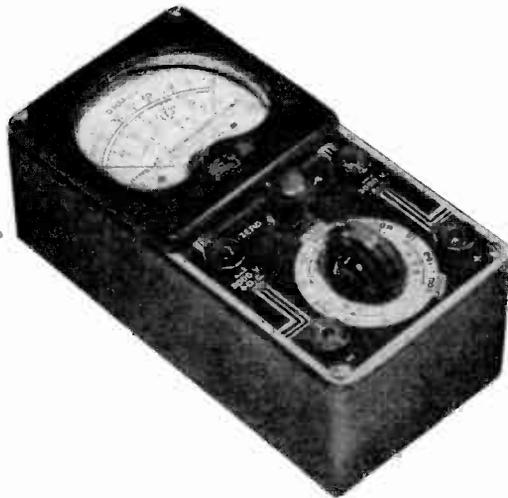
Fig. 2. Typical pocket type commercial multi-meter.
