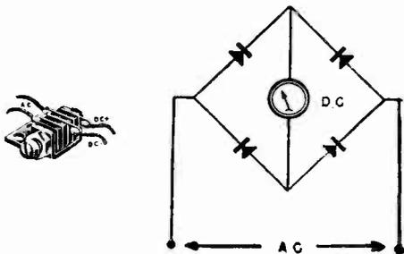
Fig. 5. Instrument type of copper-oxide rectifier and schematic of the connections by which it may be used with a d.c. meter to measure a.c. voltages.
