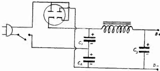
Fig. 9. This full-wave voltage doubler does not have the same reference points as the half-wave type shown in Fig. 8.
