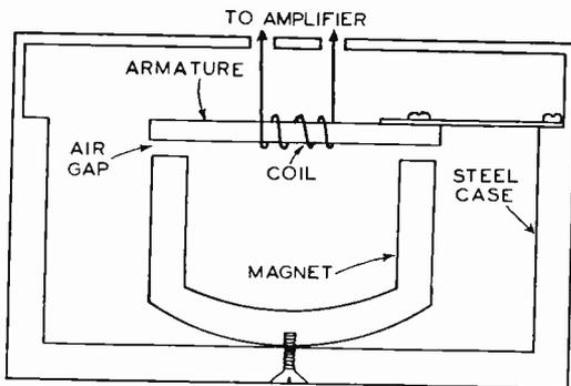
FIG. 3.—This is a geophone or seismometer, used for picking up sound vibrations and converting them into electrical signal vibrations. The sound waves cause the coil to move in the magnetic field, and a voltage is induced in the coil.
