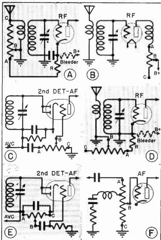
FIG. 5. Typical volume control connections.
