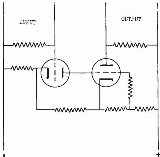
FIG. 3. A typical direct current amplifier.
