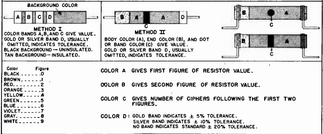
FIG. 3. The RMA color code for resistors.
