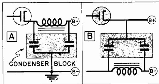
FIG. 1. Two styles of filter condenser blocks. These are NOT interchangeable, so be sure you get the proper replacement.
