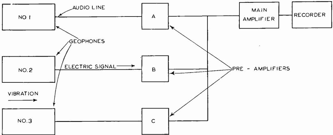
FIG. 4.—The geophones are connected by wire lines to audio pre-amplifiers which in turn work into the main a.f. amplifier. The recorder receives signal power from the main amplifier.
