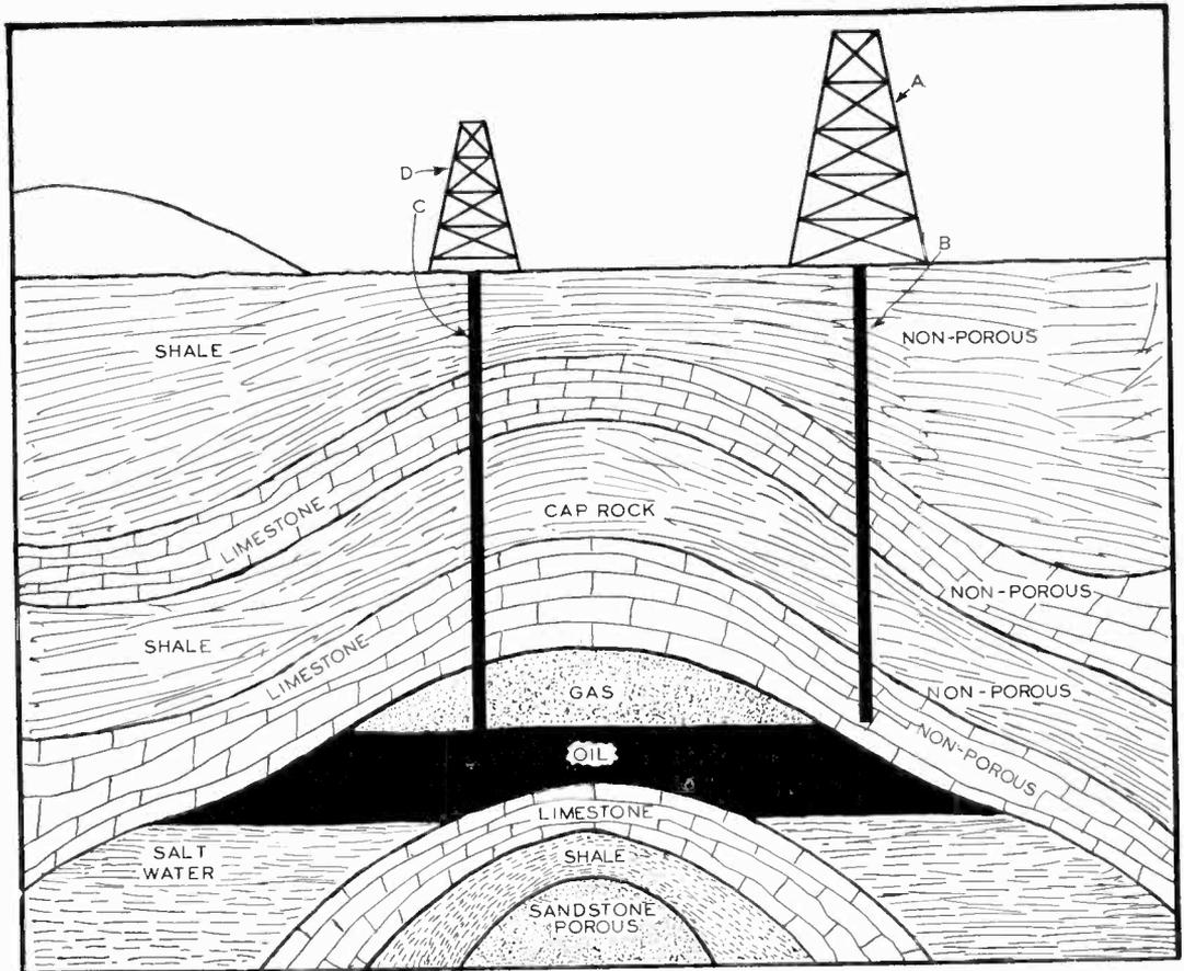
FIG. 1.—The geological layers below ground are shown. How easy it is to "miss oil" is shown by the well at "A". If the well is too far to the right or left, the oil will be "missed." To avoid drilling errors, seismic or radio-electronic prospecting is employed.
