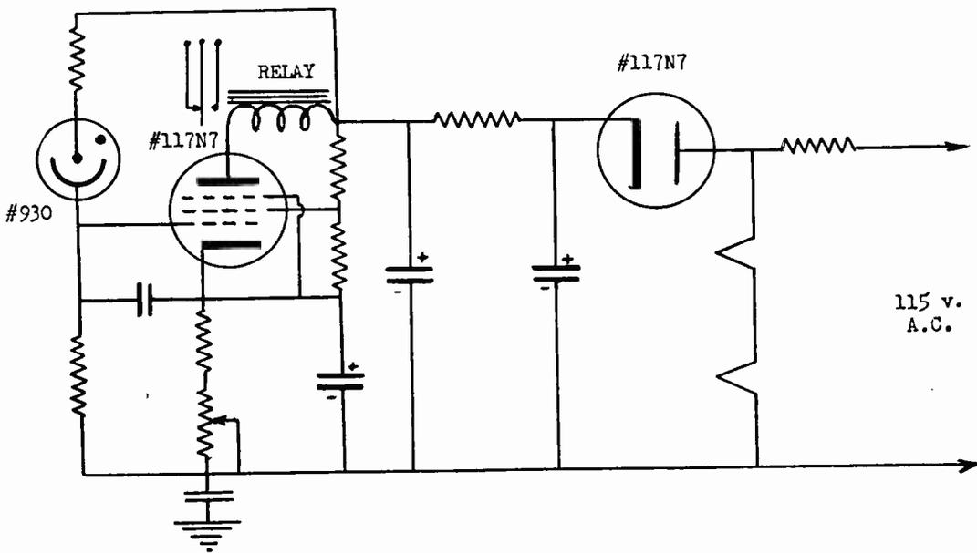
FIG. 2. This is how Fig. 1 might appear if drawn according to radio diagram practice. The circuits are identical except for the differences in the symbols representing the various parts.
