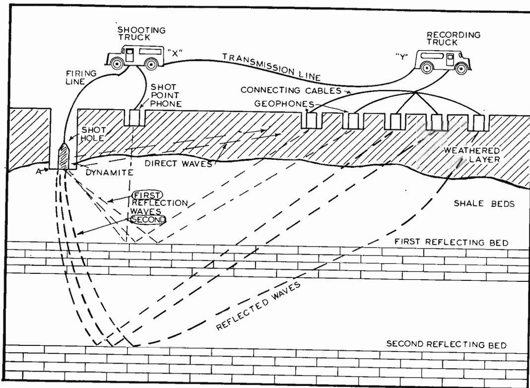
FIG. 2.—A typical radio-electronic prospecting set-up. Audio amplifier and recorder apparatus is located in truck "Y". Sound waves (earth vibrations) generated by the dynamite explosion travel down to the reflecting layers and back up to the geophones which are really special dynamic mikes. From the geophones, electrical signals travel to the amplifiers and recording equipment.
