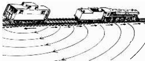
FIG. 7. Signal current flow from caboose to locomotive. Note that the earth forms the return circuit.
