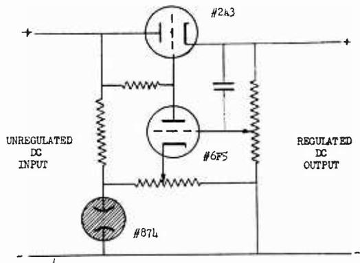
FIG. 5. Typical voltage regulator of the degenerative type.
