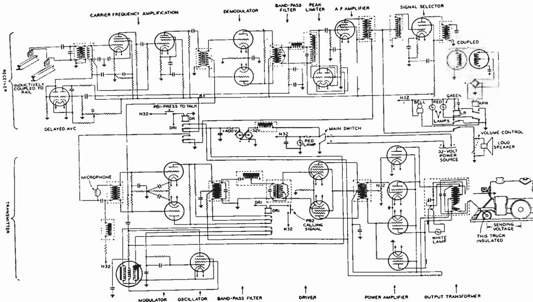
FIG. 8. Schematic diagram of a complete two-way unit showing both the transmitting and receiving equipments and the calling signals.
