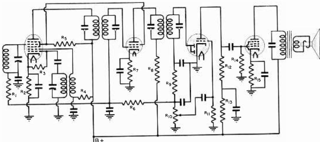
FIG. 4. This circuit shows the locations of most of the resistors used in modern radio receivers. (The diagram is incomplete otherwise.) Here are typical values used:
