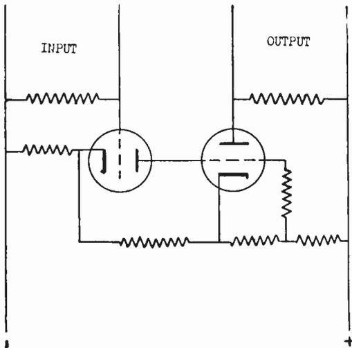
FIG. 3. A typical direct current amplifier.
