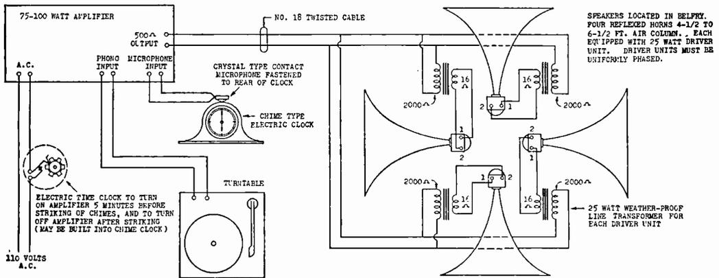
Fig. III 75-100 Watt Church Steeple Installation
