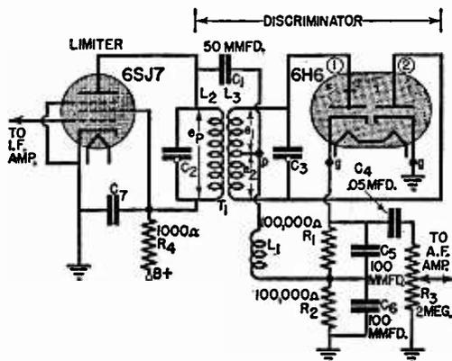
Fig. 6 Typical discriminator circuit for an f.m. receiver. The discriminator load resistors are the 100,000-ohm resistors  $R_1$  and  $R_2$ .
