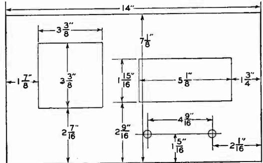
Sketch H (Above).  $\frac{1}{4}$ " 3-ply panel (make 1). Note: Holes for control shafts should be  $\frac{1}{2}$ " diameter.
