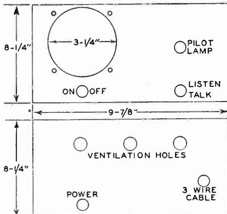
Fig. 2. Front and back panels of master unit.
