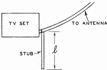
Fig. 19. A transmission line stub used to reduce interference at a fixed frequency. "L" is one-quarter wave-length long.
