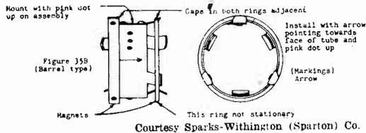
Fig. 1. A popular permanent magnet type "ion trap."
