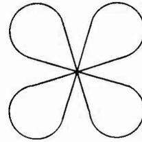
Fig. 4. Antenna pattern for 1 1/2 wave dipole.
