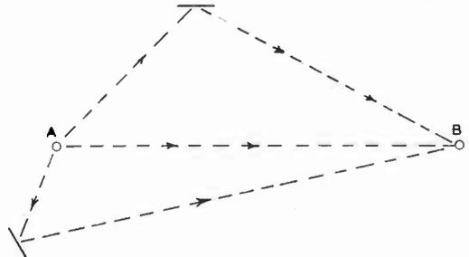
Fig. 17. How multiple signal paths may cause "ghosts."
