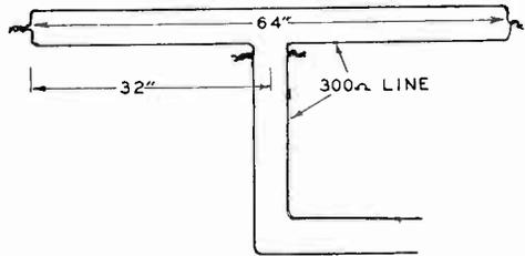
Fig. 11. Antenna made from transmission line.
