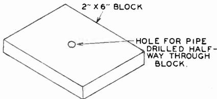
Fig. 8. Wood block for mounting antenna on a flat roof.
