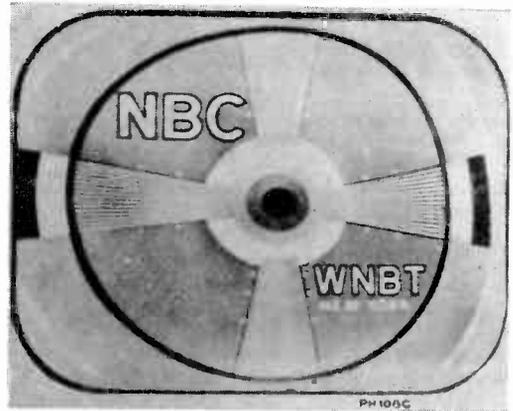
Fig. 11B. Test pattern obtained with horizontal drive control turned too high.
