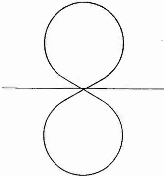
Fig. 3. Antenna pattern for half-wave dipole.
