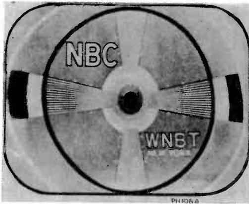
Fig. 11A. Test pattern obtained with horizontal linearity control misadjusted.
