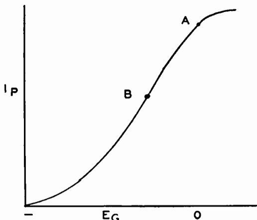
Fig. 1. The  $E_g$ - $I_p$  characteristic of a typical tube. Point A is the zero-bias point and point B is the normal operating point.
