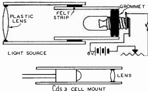
FIG. 9. Simple light source and light sensitive cell mountings.
