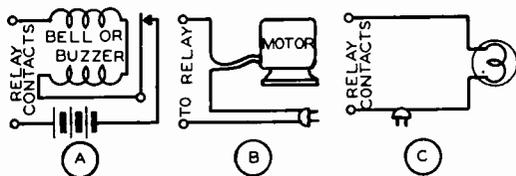
FIG. 4. How other devices can be connected to the capacity-operated control relay contacts.
