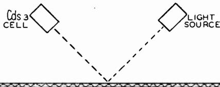
FIG. 8. How light is reflected from objects to be sorted.
