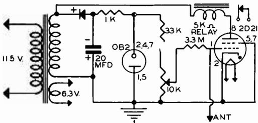
FIG. 3. This circuit provides both voltage regulation and isolation from the line.
