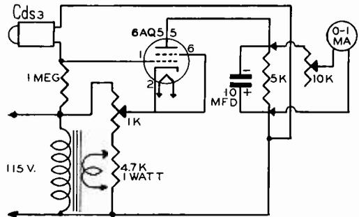
FIG. 7. This circuit gives greatest control over operating range.
