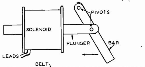
FIG. 11. Exaggerated view—retractor solenoid.
