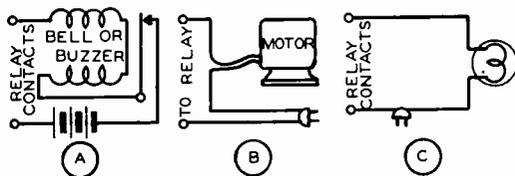
FIG. 4. How other devices can be connected to the capacity-operated control relay contacts.
