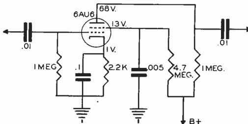
FIG. 4. Typical pentode audio amplifier circuit.
