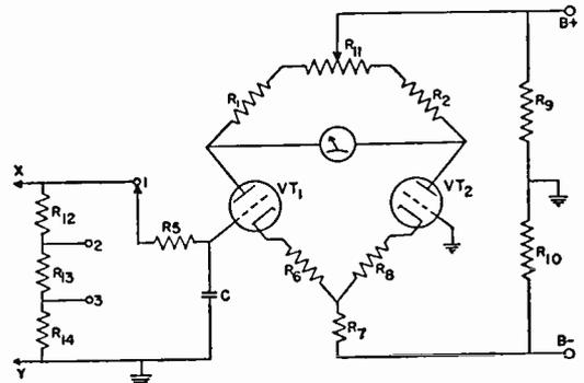
FIG. 2. Simplified basic circuit used in most bridge-type vacuum tube voltmeters.
