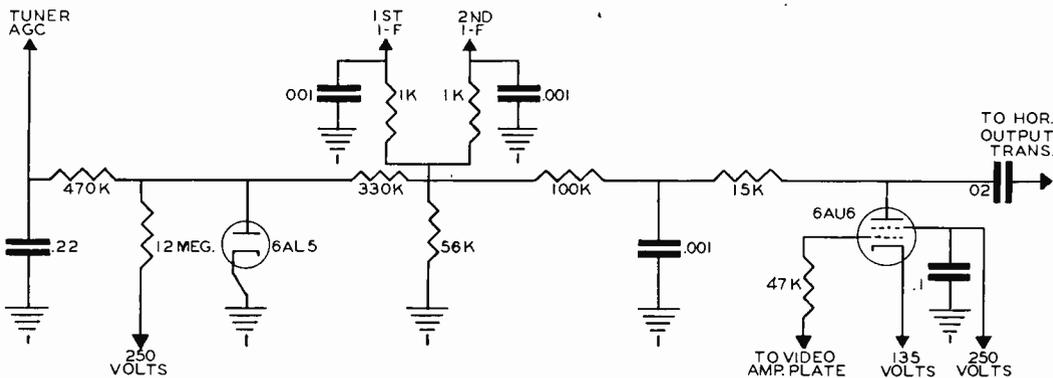
FIG. 5. A "keyed" agc circuit with a delay network to reduce the bias applied to the tuner and a bias clamper.
