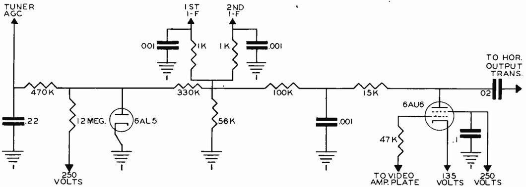
FIG. 5. A "keyed" agc circuit with a delay network to reduce the bias applied to the tuner and a bias clamper.
