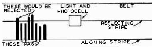
FIG. 10. How objects on a moving belt can be sorted for length.
