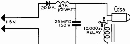
FIG. 5. A simple light-operated control circuit.
