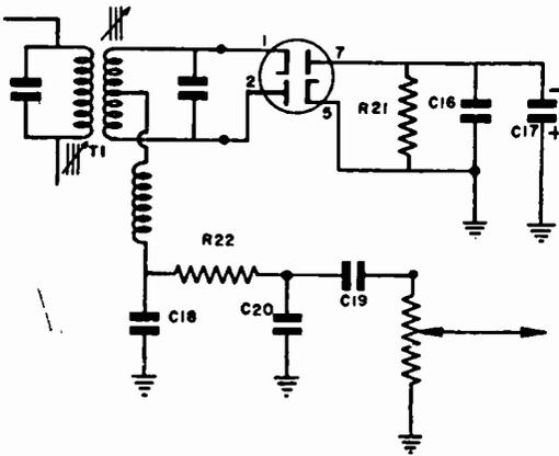
FIG. 6. Typical ratio detector circuit used in an FM or TV receiver.
