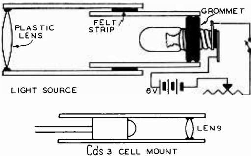
FIG. 9. Simple light source and light sensitive cell mountings.
