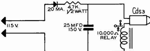
FIG. 5. A simple light-operated control circuit.
