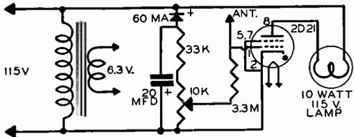
FIG. 1. A simple capacity-operated circuit using a type 2D21 tube as a "relay."
