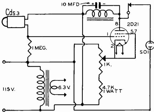
FIG. 6. A light-operated control circuit with greater control over operation.
