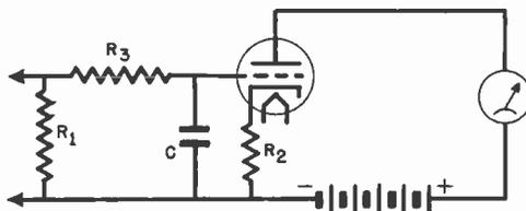
FIG. 1. Basic circuit for a vacuum tube voltmeter.
