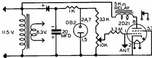
FIG. 2. A more stable version of the circuit shown in Fig. 1.
