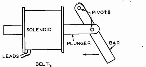
FIG. 11. Exaggerated view—retractor solenoid.
