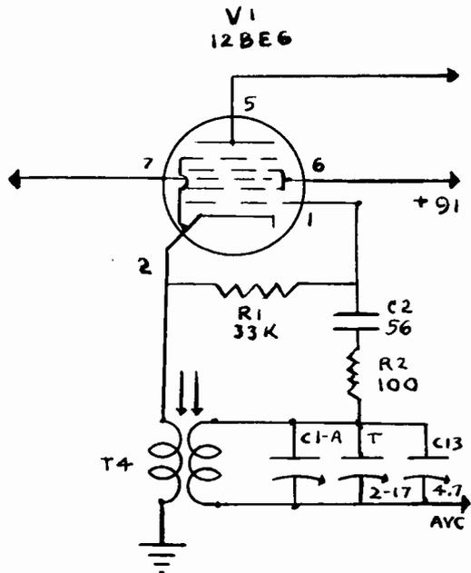
Fig. 3. Oscillator circuit of RCA receiver. For simplicity, other portions of the diagram have been omitted.
