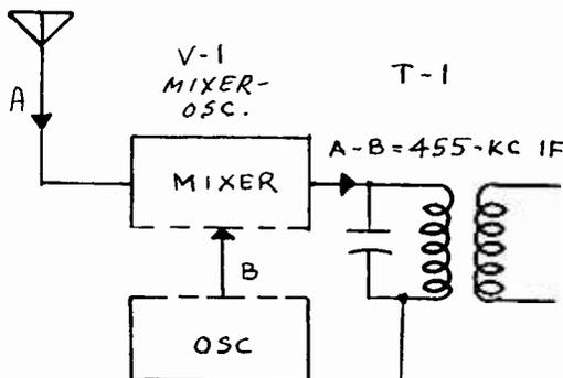
Fig. 1. Notice that when RF signal "A" is combined with oscillator signal "B" in the mixer tube, the difference is always 455-kc.
