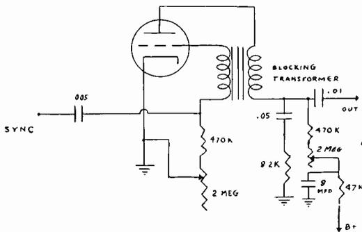
Fig. 6. Typical vertical oscillator circuit.
