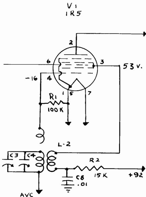
Fig. 5. Oscillator circuit of Emerson receiver.
