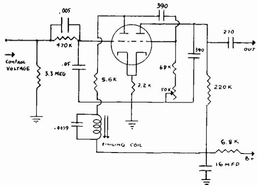
Fig. 7. Typical horizontal oscillator circuit.
