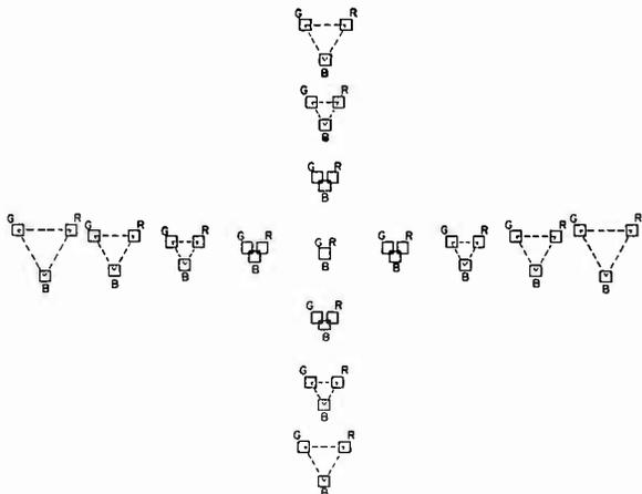
Fig. 2. Segment of screen showing convergence at the center but not at the edges.
