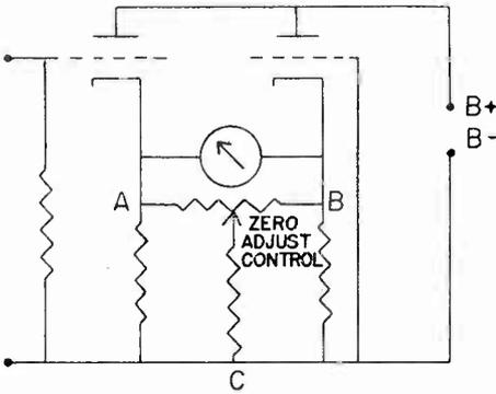
FIG. 4. The zero adjustment circuit.
