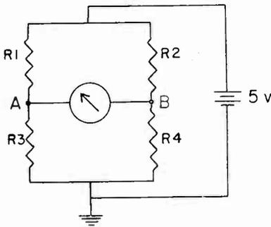
FIG. 2. A balanced bridge circuit.
