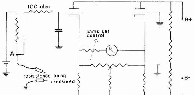
FIG. 8. The resistance measuring system.
