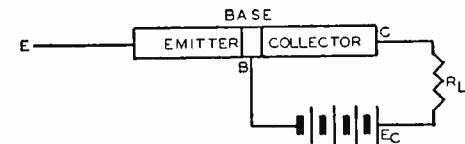
Fig. 1. A transistor in block form. The emitter and the collector are made of germanium which contain negative carriers (free electrons) and is therefore called N material. The base is made of material containing positive carriers (holes) and is for that reason called P material. The base is only a few thousandths of an inch thick. When the materials are arranged in this manner the resulting transistor is called a NPN type.
