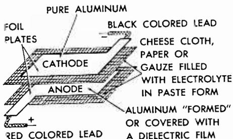
FIG. 1. How dry electrolytics are made.
