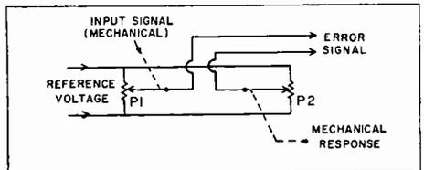
Fig. 5. Error detector using a pair of potentiometers.
