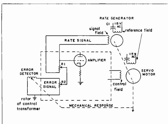
Fig. 7. The rate generator signal is fed to a resistor network at the input of the amplifier.
