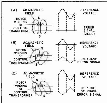
Fig. 2. The rotor winding of a synchro control transformer develops a zero error signal (A); an in-phase error signal (B) and a  $180^\circ$  out-of-phase error signal (C).
