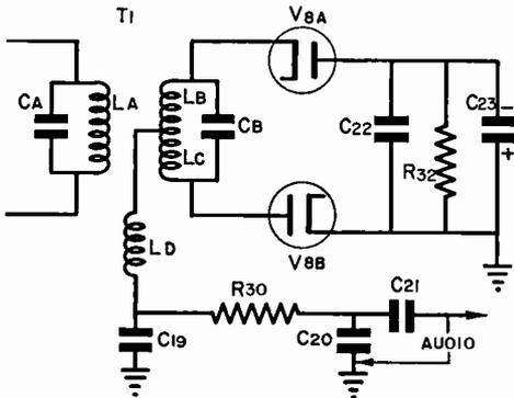
FIG. 12. The ratio detector.
