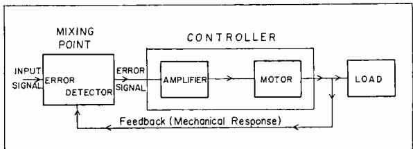
Fig. 3. Elements of a servosystem.
