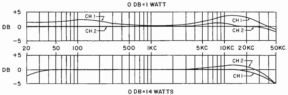
Fig. 2. Frequency response of the EICO HF-81. The top curve shows the response at 1 watt output per channel; the bottom curve shows the response at full 14 watt output per channel. See text.
