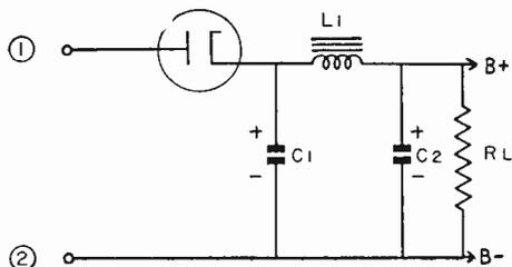
FIG. 7. Half-wave power supply.
