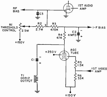
FIG. 16. A typical keyed agc system.
