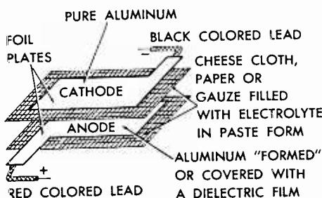
FIG. 1. How dry electrolytics are made.
