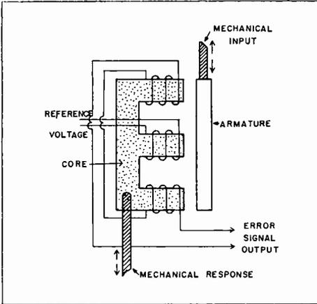
Fig. 4. E-coil differential transformer used as an error detector.
