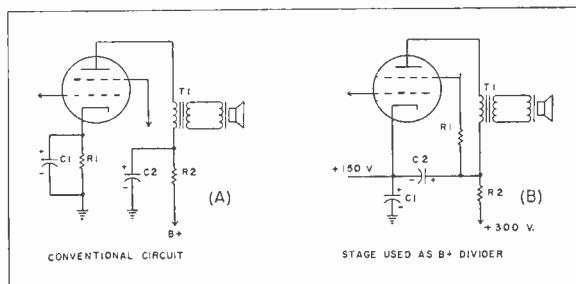
FIG. 10. Electrolytics in audio output stages.
