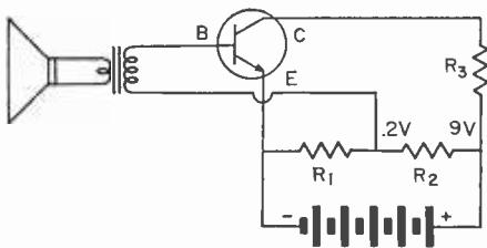
Fig. 5. Common emitter circuit using a single battery to provide forward bias for the emitter base and reverse bias for the collector base.
