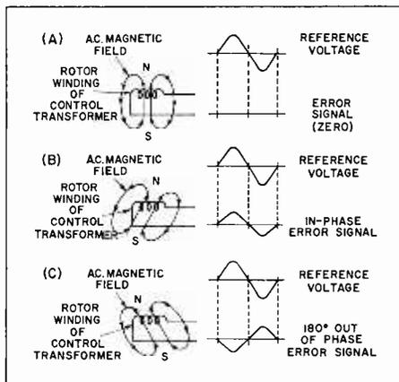
Fig. 2. The rotor winding of a synchro control transformer develops a zero error signal (A); an in-phase error signal (B) and a 180° out-of-phase error signal (C).
