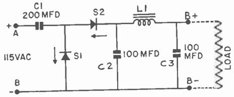
FIG. 5. A voltage-doubler circuit similar to circuits used in many TV sets.
