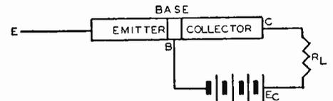
Fig. 1. A transistor in block form. The emitter and the collector are made of germanium which contain negative carriers (free electrons) and is therefore called N material. The base is made of material containing positive carriers (holes) and is for that reason called P material. The base is only a few thousandths of an inch thick. When the materials are arranged in this manner the resulting transistor is called a NPN type.
