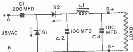
FIG. 5. A voltage-doubler circuit similar to circuits used in many TV sets.
