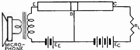
Figure 3. Signal currents from the low resistance microphone transformer will flow through the high resistance load  $R_L$ , producing a large signal voltage.
