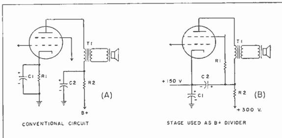
FIG. 10. Electrolytics in audio output stages.
