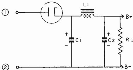
FIG. 7. Half-wave power supply.
