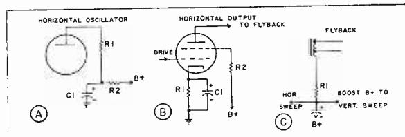
FIG. 15. Where electrolytics are used in hor. sweep stages.
