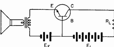
Fig. 4. Simplified common base circuit.
