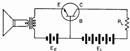
Fig. 4. Simplified common base circuit.
