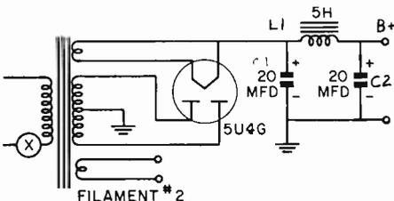
FIG. 3. A typical power supply using a transformer and full-wave rectifier.
