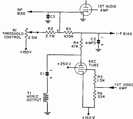
FIG. 16. A typical keyed agc system.
