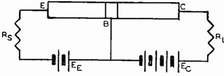
Figure 2. Here the emitter is biased in a forward direction and since current carriers are available at the junction of the emitter and the base current can flow from the emitter into the base.
