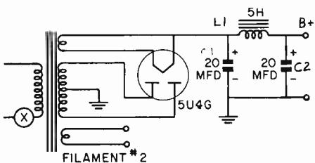
FIG. 3. A typical power supply using a transformer and full-wave rectifier.
