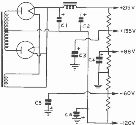
FIG. 9. Simplified circuit of a low-voltage power supply producing both positive and negative voltages.
