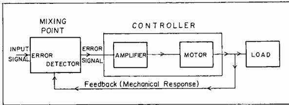
Fig. 3. Elements of a servosystem.
