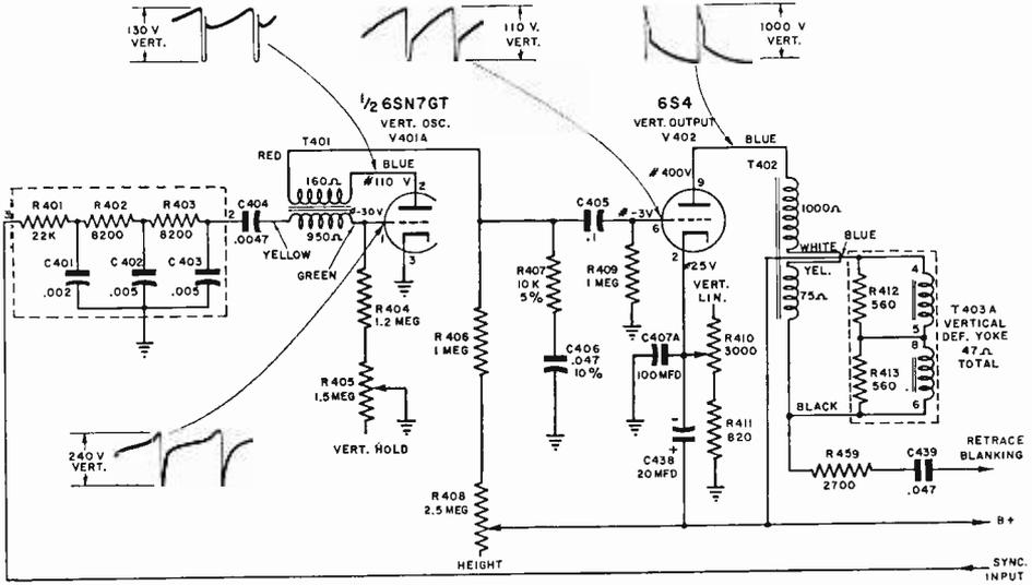
FIG. 14. The vertical sweep system of a typical TV receiver.
