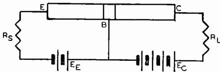
Figure 2. Here the emitter is biased in a forward direction and since current carriers are available at the junction of the emitter and the base current can flow from the emitter into the bias.
