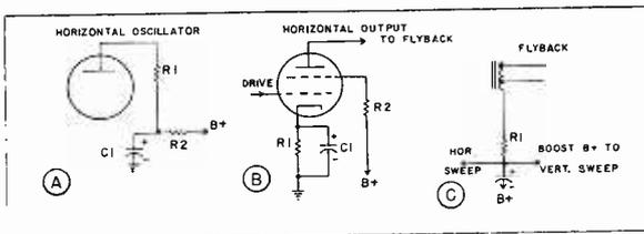
FIG. 15. Where electrolytics are used in hor. sweep stages.
