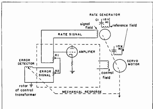
Fig. 7. The rate generator signal is fed to a resistor network at the input of the amplifier.
