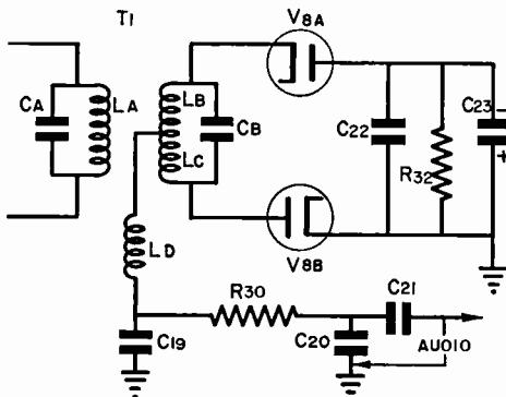
FIG. 12. The ratio detector.
