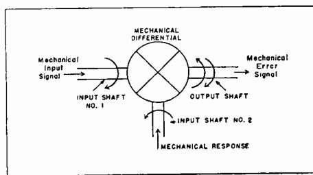
Fig. 6. Schematic diagram of a mechanical differential used as an error detector.
