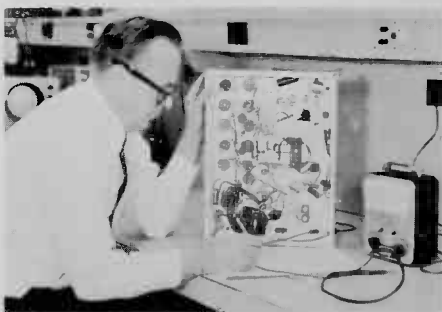
FIG. 2. A "breadboard" test.
