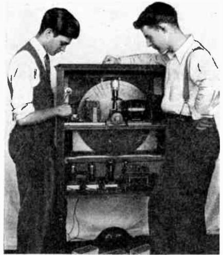
Above: View of a receiver to catch broadcast slight waves. The receiving disk, motor and neon lamp are easily recognized above. It will probably be a matter of only a short time until Television receivers will be as easily obtained as sound receivers are now.
