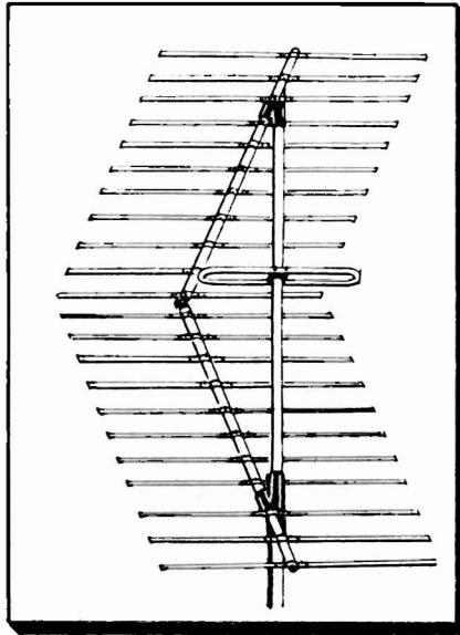
Fig. 5—A typical Corner Reflector antenna. Although a very effective high gain unit, this antenna is fairly large and heavy, and therefore is most practical on the high-band channels.—Illustration courtesy Radio Merchandise Sales, Inc.
