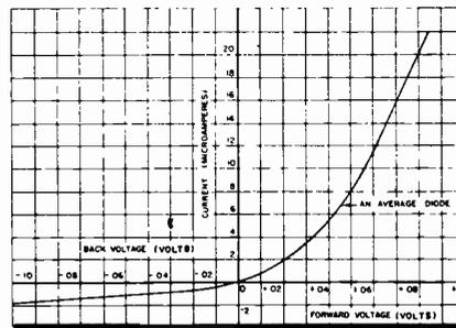
Fig. 16: Typical low voltage-current characteristic of type IN48 at 25°C.
