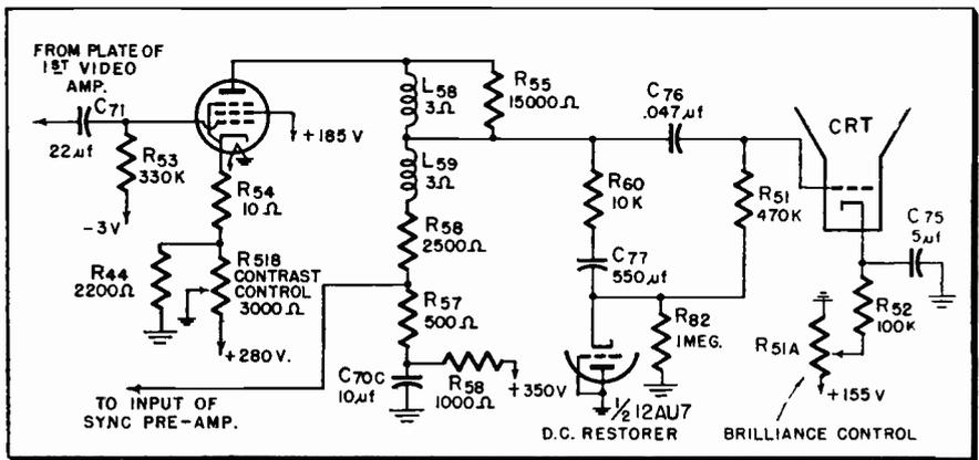
Fig. 4—DC diode restorer used in Philco models 50-T1400, 50-T1401, 50-T1402, 50-T1403. One-half of a 12AU7 is used as a vertical oscillator; the other half as a DC restorer. The triode section used as a restorer is made a diode by connecting grid and plate. A portion of the video amplifier's output signal is fed through  $R_{60}$  and  $C_{77}$  to the cathode of the restorer.
