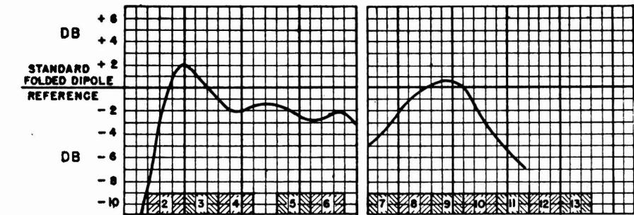
Fig. 2: Gain of a simple dipole (90" long) and reflector over the 12 channels, compared to "standard" cut for each frequency. Compare this broad-band, low-gain antenna with the narrow-band, high gain Yagi shown in fig. 3. Illustration courtesy American Phenolic Corp.
