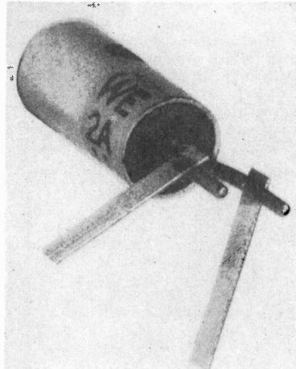
WESTERN ELECTRIC'S Type 2A transistor functions as an amplifier in the "card transistor" used with the new 4A toll crossbar system for automatic selection of routes in long distance telephone dialing. These units are used in conjunction with Type 3A phototransistors which are activated by light passing through a series of punched cards. The cartridge Type 2A has its base contact connected to the metal shell.
