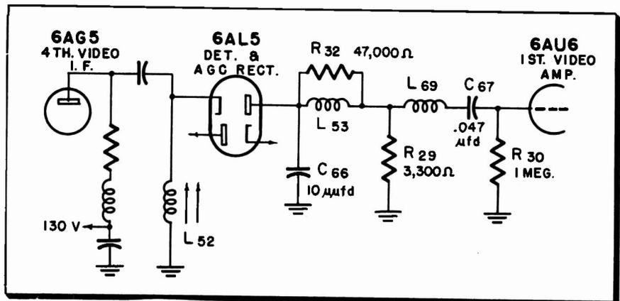
Fig. 1—Video detector circuit used in Philco 50-T1443. Filament circuit is not shown.
