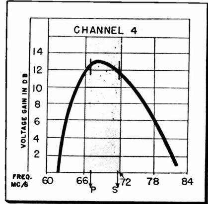
Fig. 3: Response of Telrex Y5X1-4, a 5-element Yagi cut for channel 4. "P" and "S" are pix and sound carriers. This high gain antenna shows less than 1 DB variation over the channel.
