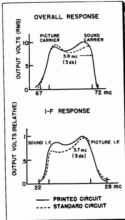
Fig. 9: Comparison of response characteristics of printed and standard 25 mc i-f circuits
