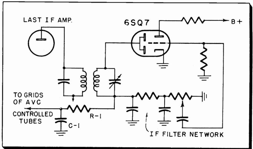
Fig. 2—Typical AVC circuit used in broadcast AM receivers.
