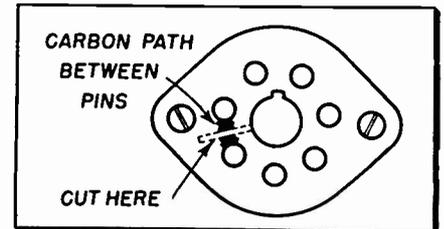
can be devised. So I used a key-hole hack saw to cut a slot from the center key of the socket to the space between the pins.
