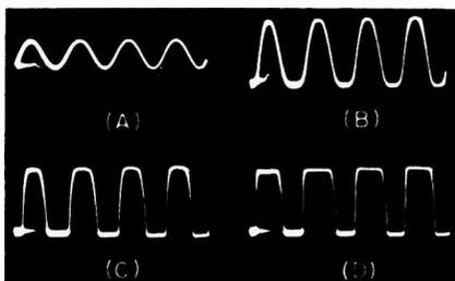
sively high input voltages, the output waveform becomes an almost perfect square wave (see fig. 2).
