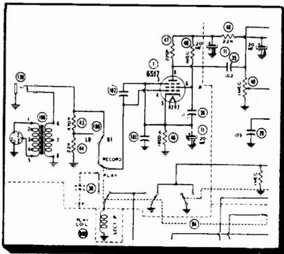
Fig. 1: Mike input stage for Brush Soundmirror BK403 uses a single-ended 6SJ7 (metal) for a gain of at least 40 DB, which is common for such stages. R49 and C11A and B provide isolation and additional filtering especially for this stage. On playback, the playback head feeds directly into this stage without additional compensation.
