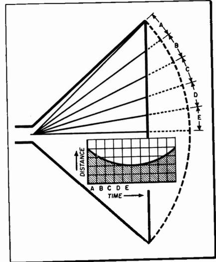
Fig. 2—Comparison of distances traveled in the same time period by the electron beam in curved or flat faced TV picture tubes.
