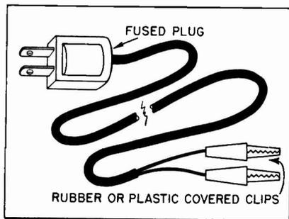
grips to protect the technician from shock and to keep the clips separated when they are used on terminals which are close to each other. This sort of cord can be used as a universal test cord for TV sets, particularly in the case of older sets such as GE, Philco, Emerson, which for some years had an AC interlock receptacle differing from what has now become standard for the industry.—Arthur Bertram, 247 West 13th St., New York, N. Y.
