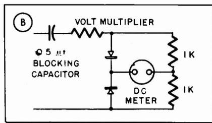
Figs. 6a, b: Where maximum output with minimum input is of primary importance, these circuits are suggested for frequencies between 25 cycles and 25 K.C. The circuit of Fig. 6a gives about 10% greater deflection than Fig. 6b, but Fig. 6b is less expensive, takes less room and has somewhat better temperature and frequency characteristics.
