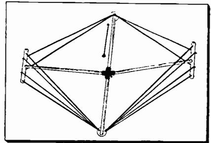
Fig. 6—An unusual rhombic in which the long axis is broadside to the station. Extra elements on the back are designed to improve pickup on the low band. By increasing the diameter of the elements, it is said to be possible to utilize shorter legs.—Courtesy Roger Phillips Research Labs.
