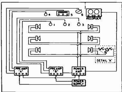
Fig. 2: Wiring diagram for auditorium reinforcement system similar to fig. 1. Placement of mikes and speakers is described in text.
