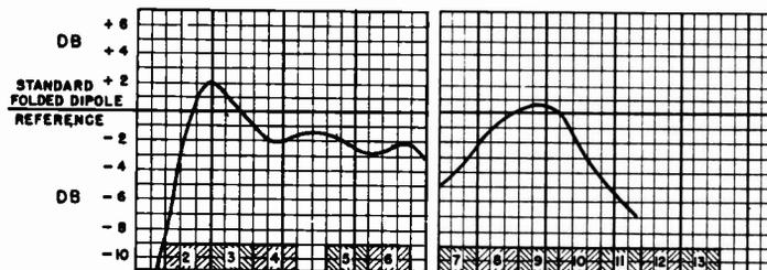
Fig. 6: Horizontal radiation patterns of a simple dipole (90" long) and reflector on low and high channels, showing development of side and back lobes on the high band, with change in direction of maximum pickup.
