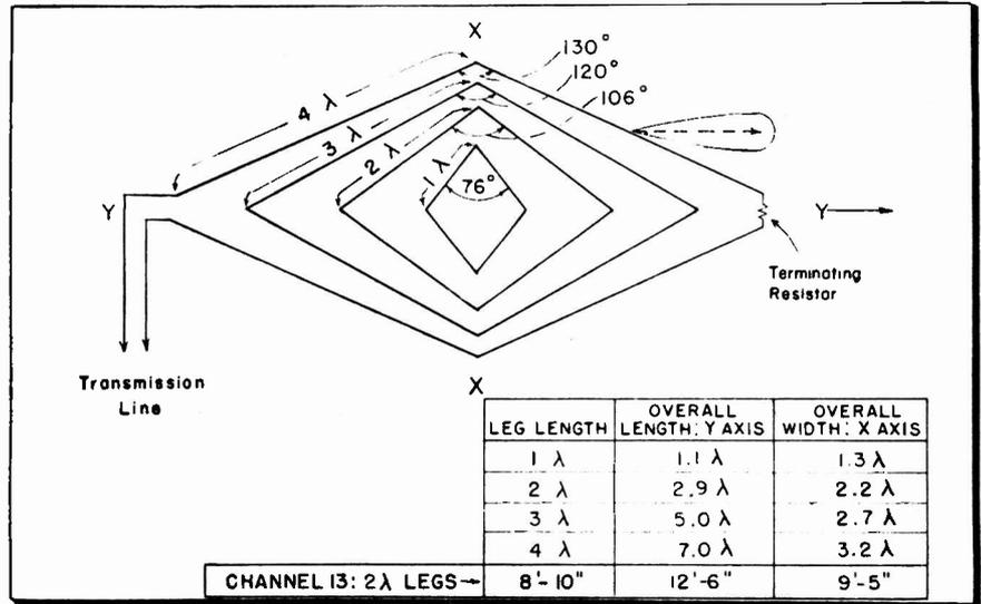
Fig. 2—Typical rhombic designs based on interior angles which complement those shown in fig. 3. When the legs or sides are larger multiples of a wave length at the operating frequency, the antenna gets longer and narrower as does the beam, and the gain goes up. Similarly, when the size remains the same but the frequency goes up: a leg which is 2 $\lambda$  long at 100 MC is 4 $\lambda$  at 200 MC.
