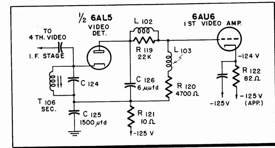
Fig. 2—Video detector circuit used in RCA models 9T270, 9TC272 and 9TC275.
