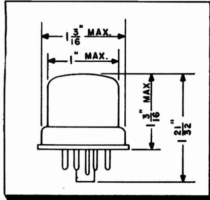
Fig. 15: Where the increased sensitivity of the 4 diode bridge rectifier shown in Fig. 14 d is desirable, a plug-in hermetically sealed assembly may be used. Some typical units are the type G9B, IN73 and IN74 with overall dimensions shown.
