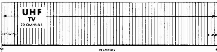
Fig. 1: UHF TV band is 2-4 times higher in frequency and almost 3 times as wide as VHF.
