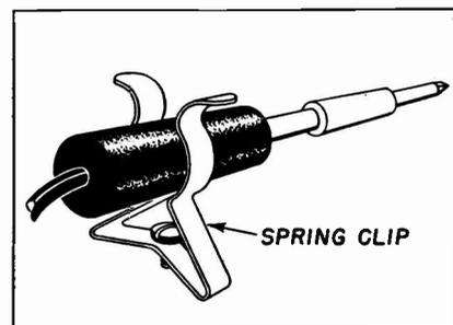
the bench, and so do away with the rather cumbersome sling that I had. So I screwed one of these clips down on the bench, and I find that it has quite adequate strength to hold my 125-watt iron. You can either hold the iron or the handle, depending on how large a clip you get. The handle is better, as then the clip doesn't conduct the heat away from the iron and into the bench. *M. LeGoff, New Orleans, La.*
