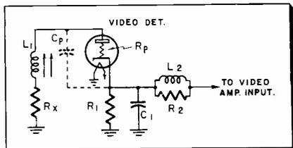
Fig. 3—Basic video detector circuit. C<sub>p</sub> is the plate-to-cathode capacitance. R<sub>x</sub> is the DC resistance of coil L-1. It is not actually a separate resistor, although it is represented as one.
