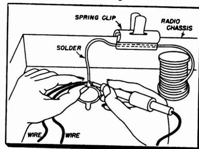
The drawing shows how I use a spring clip as a third hand to hold the solder in exactly the right position.—J. Amorose, Amorose Radio, Route 4, Hungary Rd., Richmond, Va.
