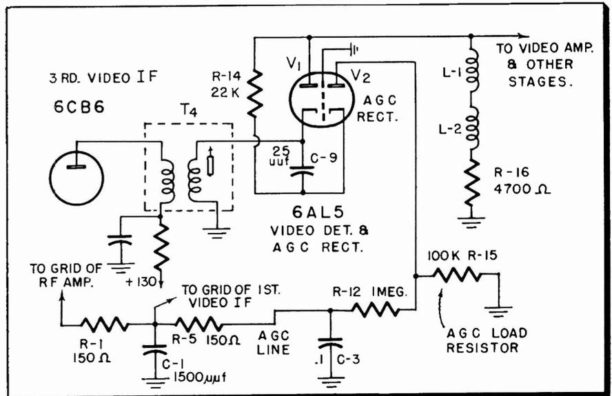
Fig. 6—Commercial form of simple AGC circuit using separate tube for AGC rectifier. Circuit is used in Emerson, Models 662B and 663B. R12 and C3 form the AGC time constant or filter network. R5, C1 and R1 are additional units, used to remove video signals from the AGC voltage.
