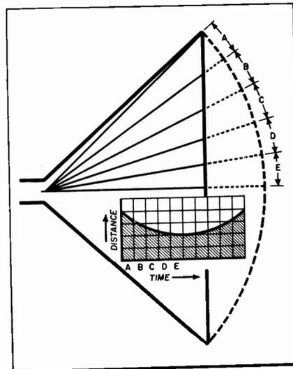
Fig. 2—Comparison of distances traveled in the same time period by the electron beam in curved or flat faced TV picture tubes.
