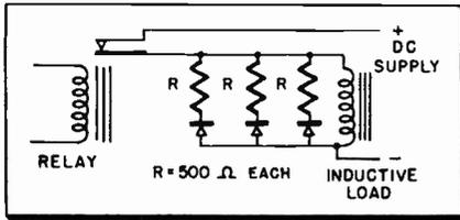
Fig. 13: For large relay of motor loads several diodes are connected in parallel, still preventing contact sparking. The series resistors help distribute the current more evenly among the several parallel diodes.
