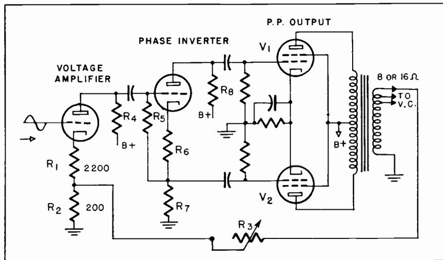
Fig. 1. In adjusting inverse feedback  $R_3$  is a variable potentiometer.  $R_1$  and  $R_2$  may vary. Some designers recommend omitting  $R_2$  and connecting  $R_3$  to cathode.  $R_7$  equals  $R_5$ .
