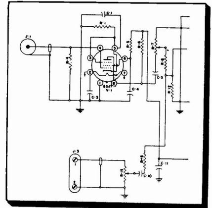
Fig. 2: Stromberg Carlson amplifier AU29 uses a 6SJ7 for mike input (J-1). J-3, the phono input, feeds the second stage. Circuit components are chosen for slightly lower element voltages on the tube and consequently slightly lower gain than the stage in fig. 1, which must handle the extremely low output tape head.
