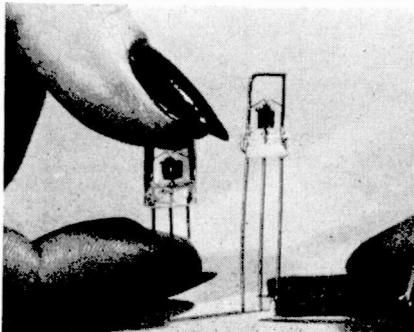
RCA transistors are imbedded in a thermo-setting resin to maintain power gains within a 2 db variation over extreme conditions of moisture,
