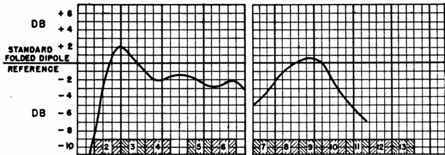
Fig. 2: Gain of a simple dipole (90" long) and reflector over the 12 channels, compared to "standard" cut for each frequency. Compare this broad-band, low-gain antenna with the narrow-band, high gain Yagi shown in fig. 3. Illustration courtesy American Phenolic Corp.
