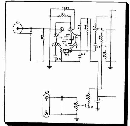
Fig. 2: Stromberg Carlson amplifier AU29 uses a 6SJ7 for mike input (J-1). J-3, the phono input, feeds the second stage. Circuit components are chosen for slightly lower element voltages on the tube and consequently slightly lower gain than the stage in fig. 1, which must handle the extremely low output tape head.
