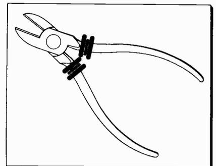
vides spring tension on the tool. To adjust the amount of spring return, merely slide the grommets up or down as is necessary until the desired amount of tension is achieved.—Nick Capellini, 639 N. 25th St., Camden 5, N. J.
