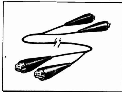
clamps attached at the ends, matching red and black on the same conductors of course so that the patch cords may be used in extending not only AC
