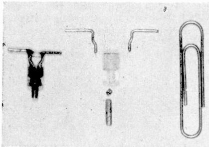
PHILCO'S potted transistor for video and r-f carrier amplification is enclosed in an impregnating plastic. The above picture shows the emitter and collector leads, base pin, germanium block from which the crystal wafer is cut, and the plastic case. Whisker crimp provides predetermined contact pressure on the crystal. Electrical characteristics are comparable to preliminary specifications for similar types.
