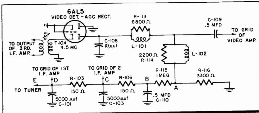
Fig. 1—Simple AGC circuit, in which video detection and AGC rectification are performed by the same diode. Elements of the unused diode are grounded out. The circuit shown is from the schematic of Hallicrafters Models 810A, 815, 822, 870, 871 and 880.
