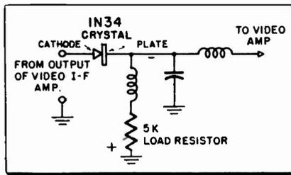
Fig. 6: Crystal detector circuit. A somewhat greater video output is possible with a crystal, due to the fact that 1. its internal resistance is lower than that of a diode and 2. the absence of interelectrode capacitance permits a higher value of load resistance to be used.
