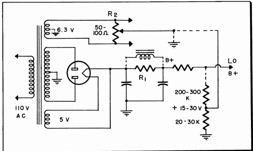
Fig. 2. Dotted lines show various methods for reducing hum due to design (not for hum due to component failures). 15-30 V may be applied to 6.3 winding centertap.
