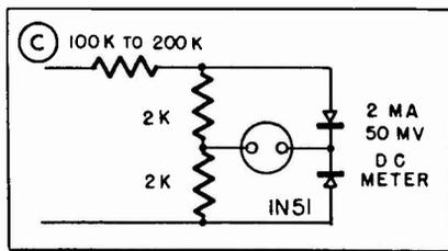
Figs. 10 a, b, c: Actual 30 v. meter rectifier circuits using 2 ma and 50 mv dc meters are good for frequencies from 60 to 5000 cycles with less than  $\pm 3\%$  change for the temperature range  $-25$  to  $+125^\circ\text{F}$  ( $-32$  to  $+87^\circ\text{C}$ ). The main difference in each of the three circuits is the increase in sensitivity in going from the single diode half wave rectifier to the dou-
