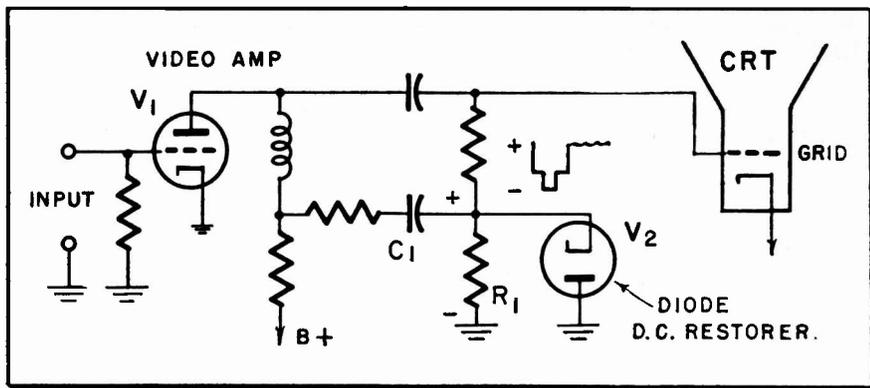
Fig. 1—Simplified sketch of positive diode DC restorer.
