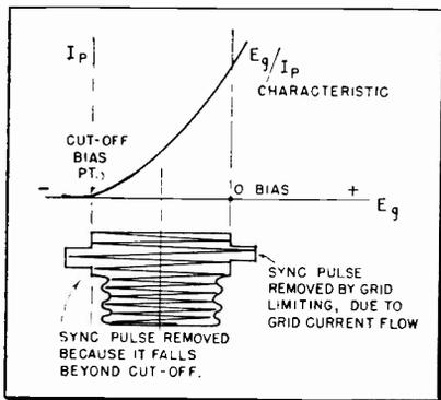
Fig. 1—A large-amplitude IF signal may force the grid bias to swing beyond 0 volts, into the positive region, on positive peaks of the signal, and to exceed cut-off, on negative signal peaks. This condition is most apt to occur in the last video IF amplifier, where the IF signal level is highest. A sharp cut-off tube is assumed.
