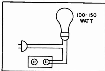
power-supply components, this fuse protector lights up brightly on shorts, dully if device is OK. J. L. Brody, Ab's Radio, Chapel Hill, N. C.
