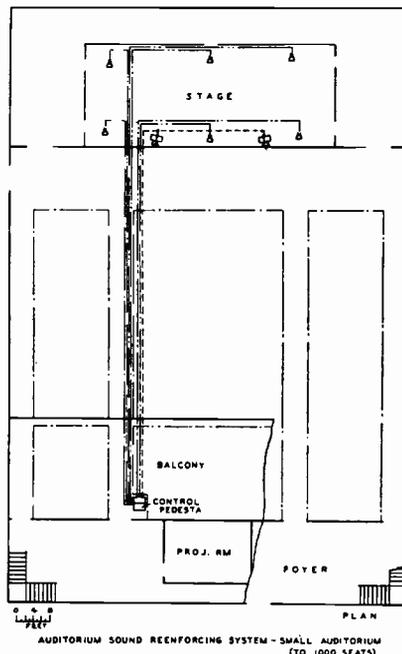
Fig. 1: Auditorium sound reinforcement system with 2 speakers and 4 mikes on stage.—Courtesy RCA.
