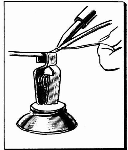
letting the lead (or solder) solidify while the end of the battery clamp is held in it. This "third hand" is a good item to carry along in the tool kit for those outside calls, too. M. Quisenberry, Bucks Radio & Appliance Co., Lexington, Va.
