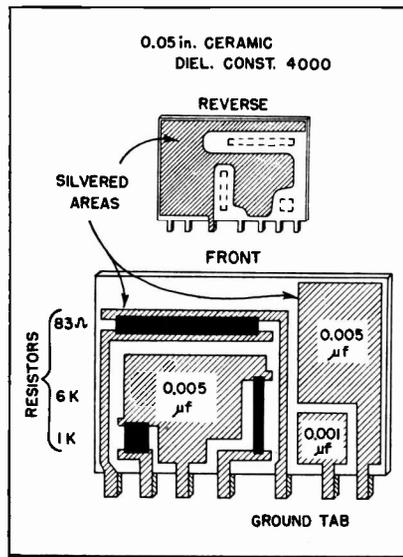
Fig. 8: RC card silk screened on dielectric
