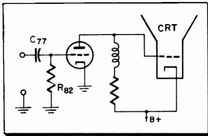
Fig. 3—Simplified grid-leak restoration circuit. Restoration action is achieved through the action of  $C_{77}$  and  $R_{82}$ . This type of restorer has two basic faults: 1—The plate current of the video amplifier is heavy in the absence of a signal input, which does this tube no good. 2—The control grid and cathode of the CRT will be at the same potential when the video amplifier conks out, causing zero CRT bias and permitting a possibly damaging current to flow through the CRT.
