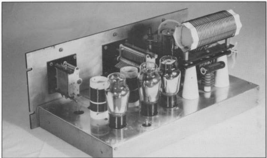
Figure 13. The Collins 4A transmitter. This was Collins' first and last try at the "low price" amateur transmitter market. Introduced in mid-1933 with a selling price around $60, less coils and tubes, it had 20 watts of CW output on 160/80/40 meter bands. (Author's collection...photo by author.)
