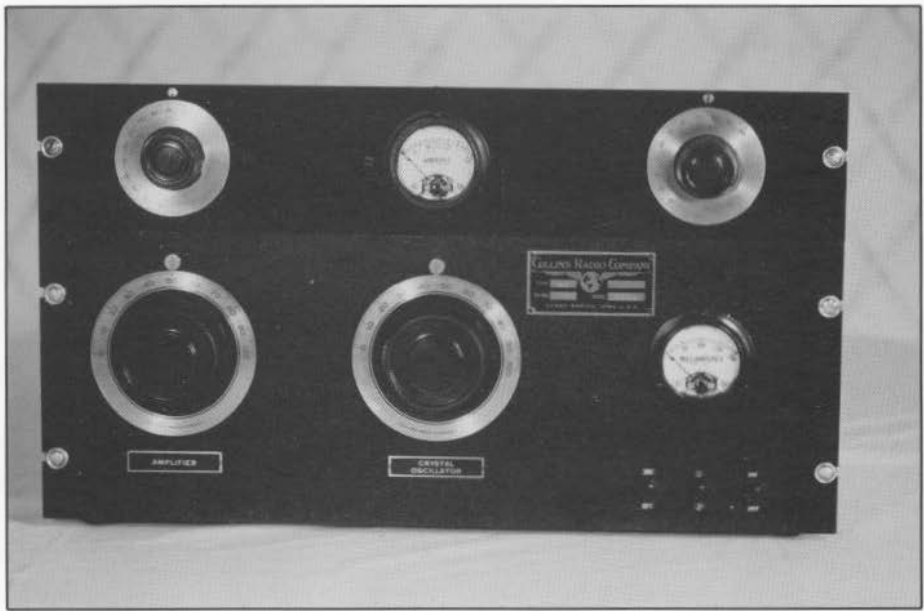
Figure 12. The Collins 10J RF deck. Announced in mid-1933, this RF deck was first used in the 42A and 42B lineup. (Author's collection...photo by author.)
