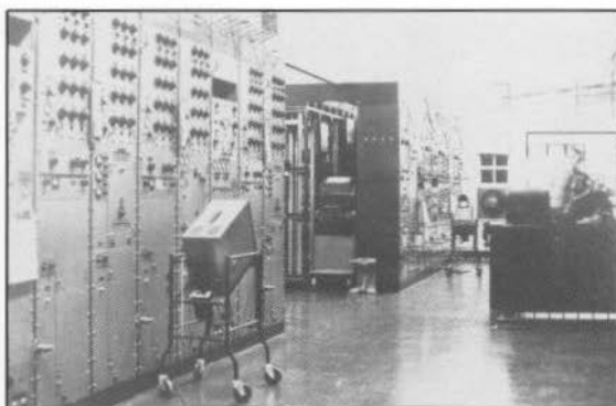
Figure 20. These three-set diversity receivers were built in 1936 to replace the original models. This picture, taken about 20 years later, shows them modernized with captive oscillators and FSK converters. Many of the receivers were still in service when the Riverhead station closed in 1975.
