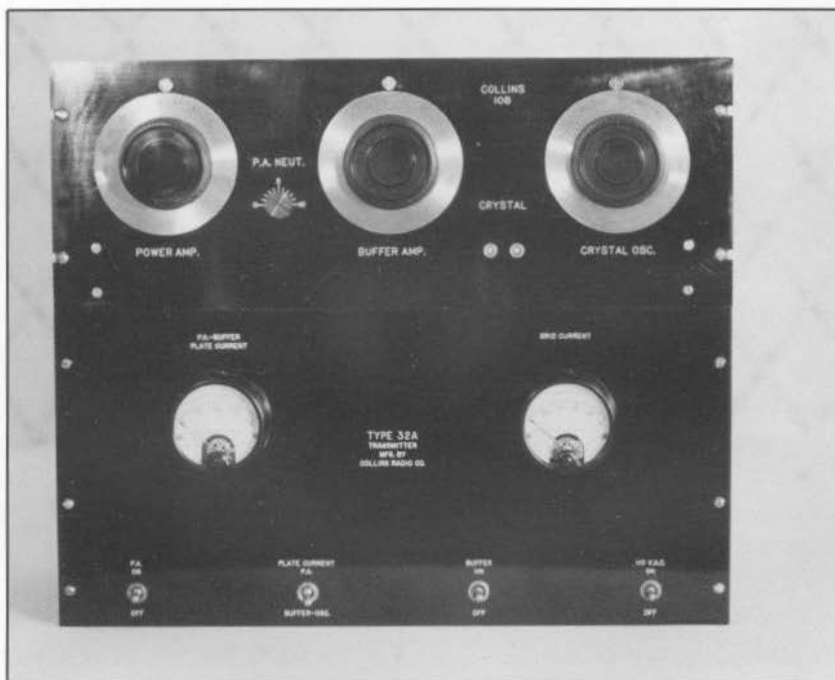
Figure 11. The Collins 32A transmitter. Running slightly less power (25 vs. 30 watts), this transmitter was a less expensive alternative to the 30W. It used the 10B RF deck which had parallel 46 tubes in the output stage rather than a single 210. (Author's collection...photo by the author.)
