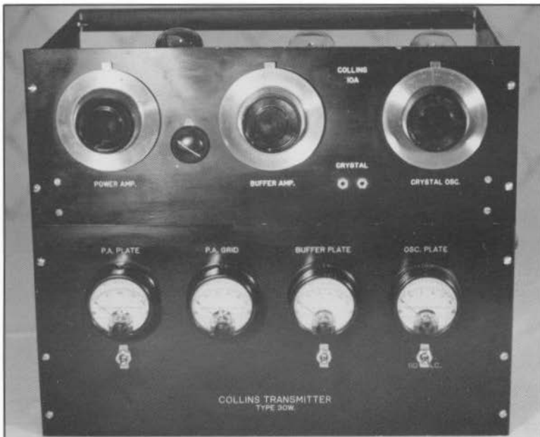
Figure 5. The Collins 30W transmitter. A 30-watt, CW-only unit, this was the first complete transmitter marketed by Collins. It used the 10A RF deck above with a 500 AX power supply below. (From the author's collection...photo by author.)
