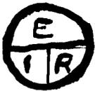
To use miliamps (1/1000 amps) divide by 1000 or move the decimal three places to the left. If your resistor is in the megohm range, move the decimal six places to the right. One megohm = 1,000,000 ohms. One kilo-ohms = 1,000 ohms so move the decimal three places to the right for ohms.
