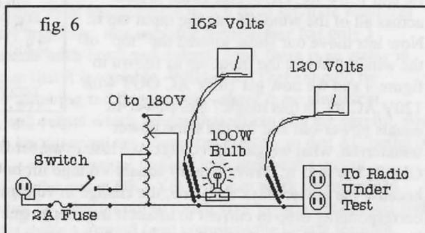
incorporating a switch from the AC plug line wouldn't be a bad idea either. If your variac isn't very big, it's probably a "control" type variac operating at a lower voltage, say 60V AC and 120V AC would pop it. But keep it anyway, we have other uses for lower voltage variacs later in this article (good junk must never be wasted!).
