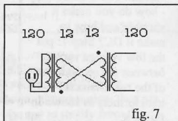
the secondaries in a cross-over arrangement because some transformers will not transfer power unless this is done. This is effectively an *isolation* transformer but in order to be useful, it must be large enough to transfer sufficient current for us to use at the output. This circuit has a LOT of
