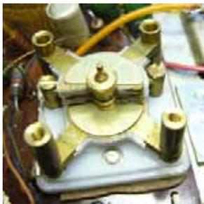
Now I could see the ragged line where the plates had gone cattywompus. I loosened the nut and tried to line them all up. I tightened the nut - and half the plates moved. The factory must use a jig. I discovered that if I pushed on the nut as I tightened it - preloading some friction into the washer stack I guess - it wasn't quite as bad. This requires a stack of backing washers in the nutdriver, or a pair of
