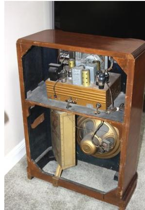
A solution to this is seen in a console radio cabinet. We use the entire distance that makes up the radio's front, outer and inner sides, just as if we were using a flat baffle. It is just as important for the cabinet walls not to vibrate and that a sound-tight fit from cone to baffle be made, just as if it were a flat surface. If you are like me, the bigger the BWH the better!
