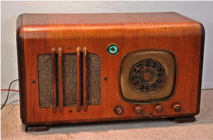
The term *farm radio* generally refers to radios made during the 1930's before electricity came to rural America. Some of these radios ran on one-time-use dry batteries as did portable tube radios. Other farm radios were designed to operate on a 6-volt lead-acid car battery that could be recharged using the farmer's truck or tractor. Some were even sold with wind-powered generators.
