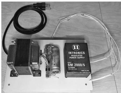
Marantz receiver and discovered that its power transformer had high enough voltage output on one of the secondary windings that it only had to be rectified and filtered to use for B+. Used a resistive voltage divider for the 45 Volts. Made chassis out of scrap 1/4" thick plastic panels. Used well regulated and filtered 5V 2-amp brick power supply for filament source and 3-"AA" holder for "C" supply...
