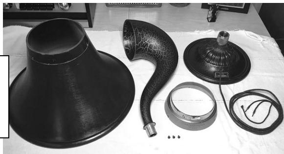
good condition (for age) of the Music Master horn speaker---disassembled and took a few pics to show off parts after careful detail cleaning with water-dampened, then dry soft cotton cloths. Used only a dry soft cotton cloth on wood horn itself to avoid risk of damage to finish. The nickel (or chrome ?) plated horn ring appears to have some type of coating (perhaps lacquer ?) which has discolored and worn off in areas.
