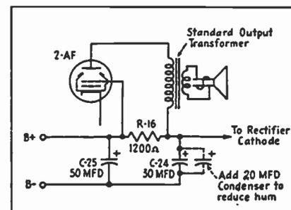
Fig. 2. One way to replace "hum bucking" transformer with standard unit.
