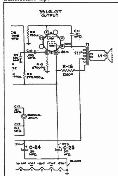
Fig. 1. Output stage with hum-bucking transformer.
