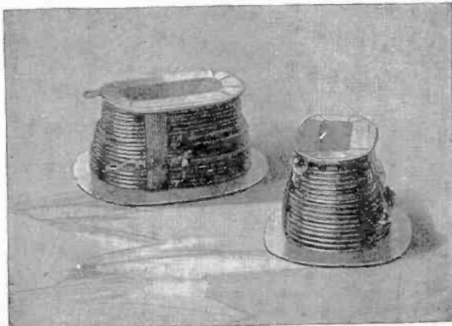
Figs. 965 and 966.—*Reliance motor construction 5.* Commutating coils.
