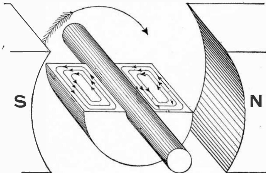
FIG. 717.—Eddy currents induced in a solid armature core. *Eddy currents* always occur when a solid metallic mass is rotated in a magnetic field, because the outer portion of the metal cuts more lines of force than the inner portion, hence the induced electric pressure not being uniform, tends to set up currents between the points of greatest and least pressure. Eddy currents consume a considerable amount of energy and often occasion harmful rise in temperature.
