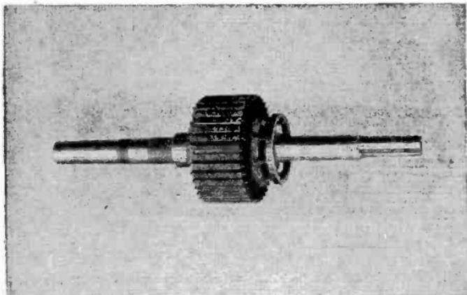
**FIG. 987.—Reliance motor construction 14.** Armature core with shaft. The flange acts as a support for the armature coil; and the pressed steel fingers provide an end support for the laminations extending to the edge of the teeth.
