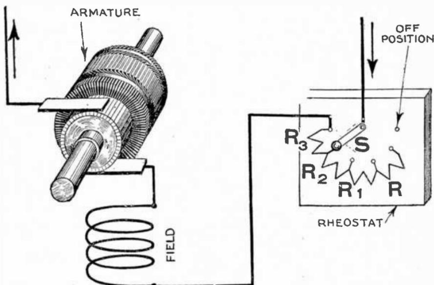
FIG. 1,021.—Series motor connections. A *series motor* on a constant voltage circuit does not have a constant field strength, and does not run at uniform speed. If the load be taken off it will run at excessive speed. To start the motor, the circuit is completed through a variable resistance or rheostat by moving the switch  $S$ , so that the resistances  $R$ ,  $R_1$ ,  $R_2$ ,  $R_3$ , are gradually cut out of the circuit. To stop, the switch  $S$  is moved back to its "off" position.
