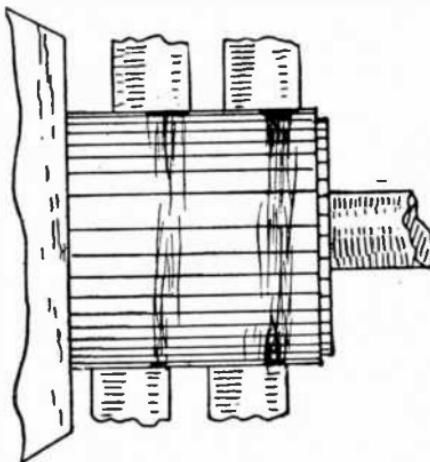
FIG. 912.—Rough and grooved commutator due to improper brush adjustment and failure to keep brushes in proper condition.
