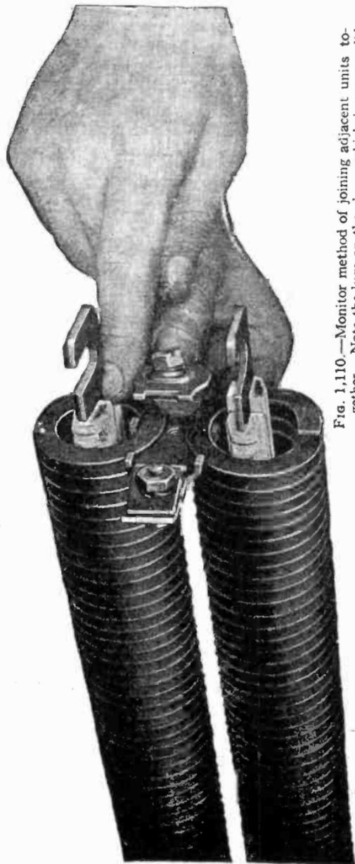
FIG. 1.110.—Monitor method of joining adjacent units together. Note the lugs on the clamp which insure a solid connection. Facilities are provided on the clamp for taking off a tap if desired.
