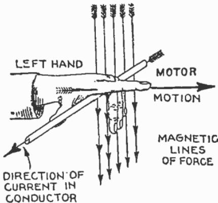
FIG. 1,010.—The "left hand rule" for direction of motion in motors. Place the left hand, as shown, so that the thumb points in the direction of the current, the 3rd, 4th and 5th fingers in the direction of the lines of force, then will the 2nd or forefinger, at right angles to the others, point in the direction in which the conductor is urged.
