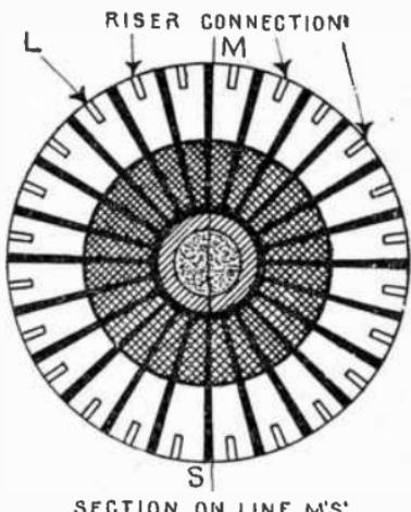
FIGS. 753 and 754.—Side and end sectional views of commutator showing construction. The parts are: C, segments; D, tubular iron hub; E, end nuts; F, clamps; G, insulation; L, riser connection.
