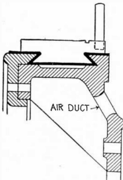
FIG. 93C.—Ventilated commutator; sectional view showing air ducts. Air is frequently circulated through a commutator in order to maintain it at a sufficiently low temperature, suitable openings being provided for this purpose as shown.
