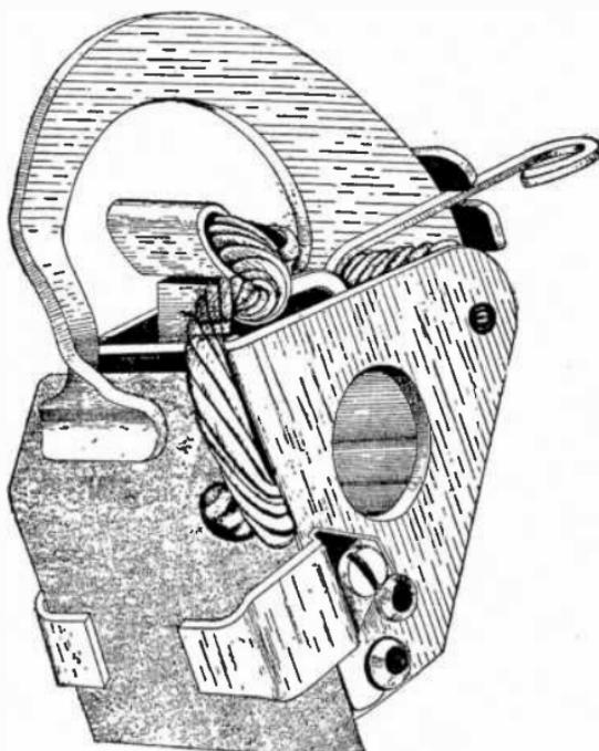
FIG. 913.—Crocker-Wheeler reaction type brush holder with brush.
