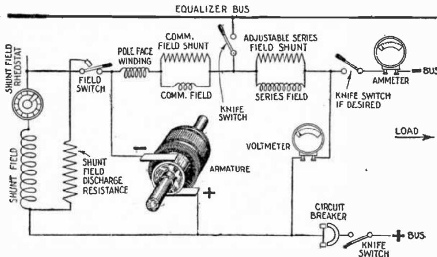
FIG. 849.—Connection diagram General Electric type LD dynamo.
