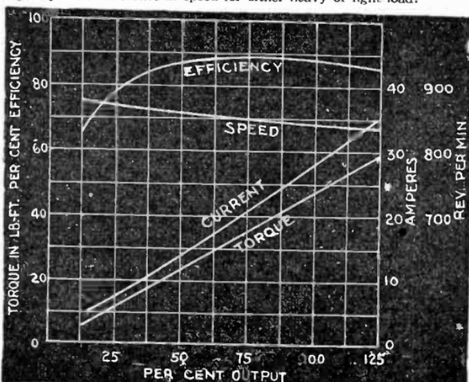
FIG. 1,039.—Characteristic curves for a General Electric type RC,  $7\frac{1}{2}$  horse power 230 volt commuting pole shunt wound motor of open construction.
