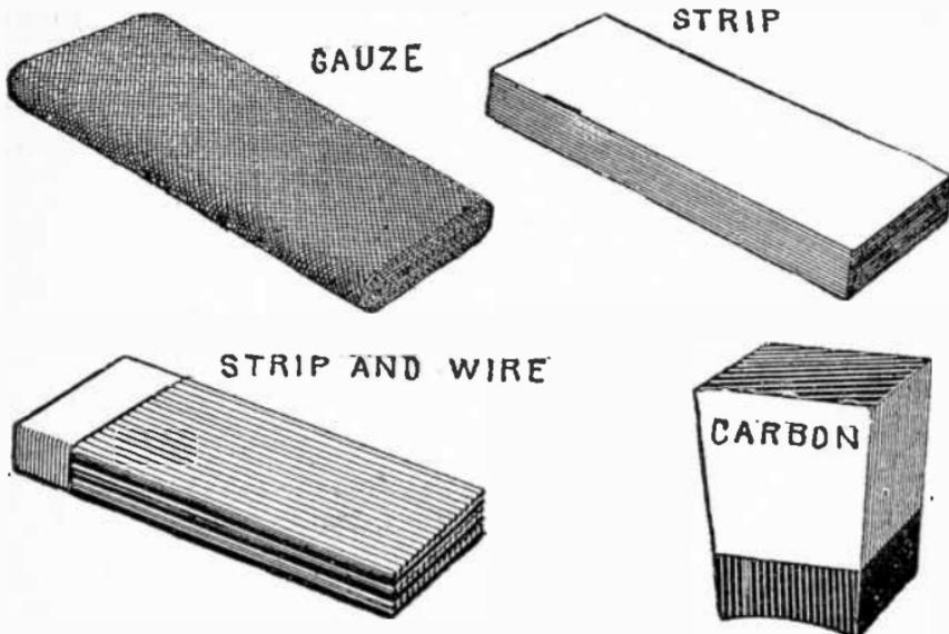
**Figs. 758 to 761.**—Various forms of brush. Fig. 758 gauze brush; fig. 759 laminated or strip brush; fig. 760 strip and wire brush as used on the early Edison machines; fig. 761 carbon brush. Carbon is preferred to copper for brushes on account of the reduction of sparking secured by its use and is now the prevailing type.
