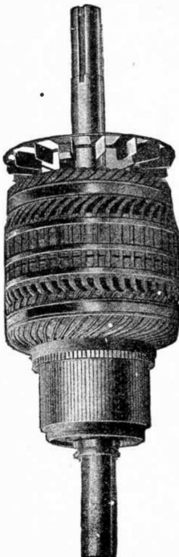
Fig. 798.—General Electric barrel-wound armature, having a fan attached at one end to induce a circulation of air for ventilation.
