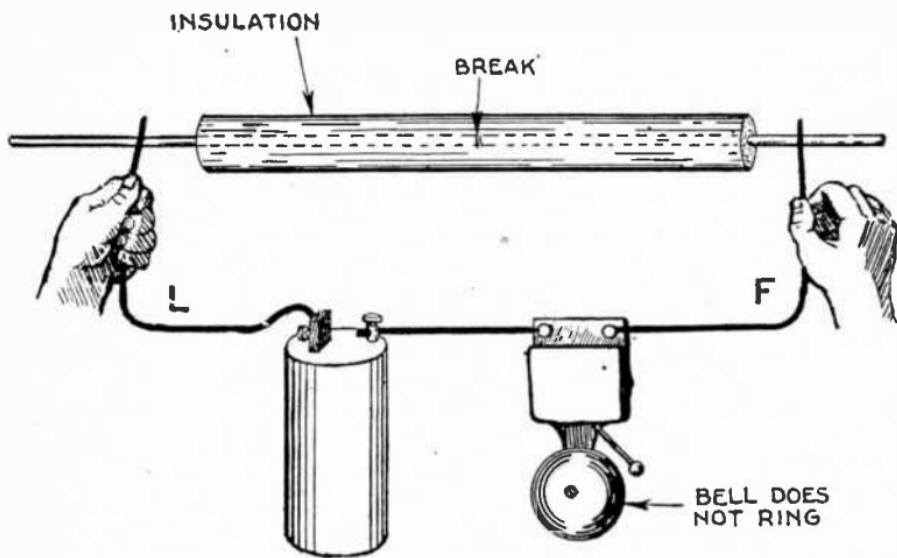
FIG. 874.—Test for break in insulated wire with bell and dry cell. Connect bell and dry cell in series and to ends of the wire to be tested by leads L and F. If the bell do not ring there is a break in the wire.
