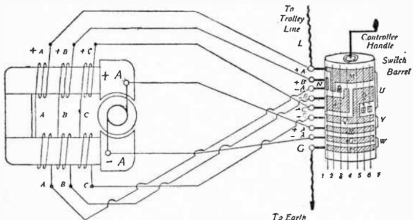
FIG. 1,086.—Speed regulation of a series motor by the method of short circuiting sections of the field winding. It will be seen that there are seven different positions for the contact springs on the barrel contacts. A, represents the armature and brushes, little A, B and C, the divided field magnet coils L, the line connection, and G, the earth connection. The diagram shows the connections for trolley car operation.
