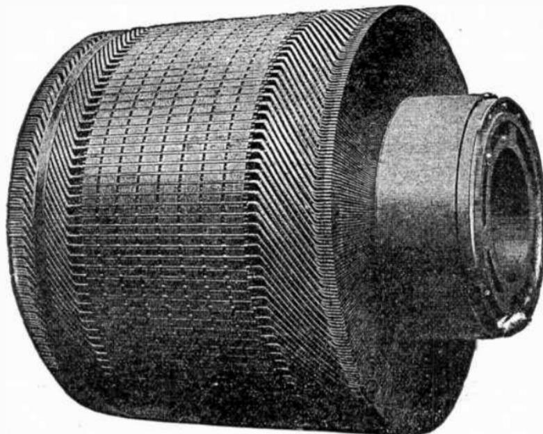
FIG. 809.—Westinghouse barrel wound armature. *The coils* are former wound from copper strap and are interchangeable. In the larger size machines they are of the single type. The illustration shows plainly the characteristic feature of barrel winding, namely the oblique end connectors carried out on the extended drum.
