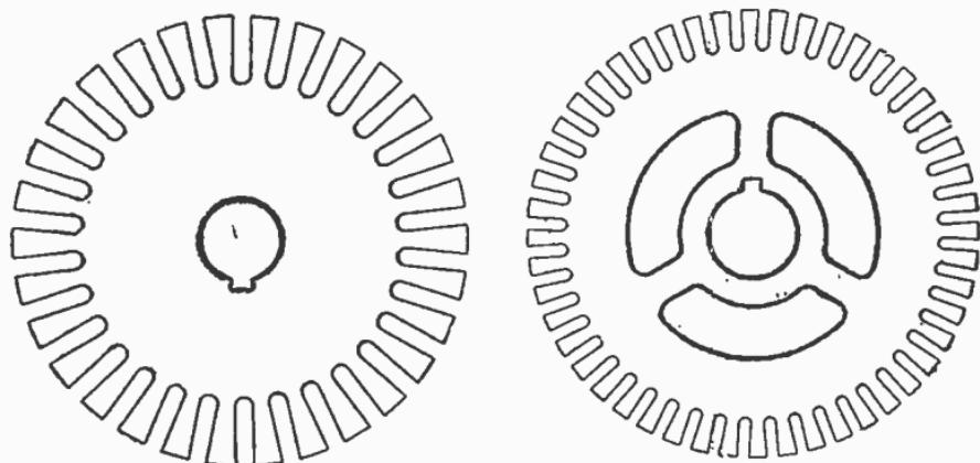
Figs. 785 and 786.—Solid and ventilated core discs. In fig. 785, the metal cut away near the center reduces the weight and provides passages for air circulation. *In some instances* a forced circulation is secured by means of a fan attached to the armature, as shown in fig. 793.
