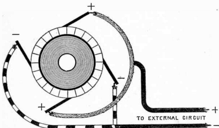
FIG. 705.—Brush connections for four pole dynamo. *It is usual* to connect all the positive brushes to one terminal and all the negative brushes to the other which gives four parallel paths as shown in the diagram, fig. 704. In a four pole machine, two separate currents can be obtained by omitting the parallel brush connections.
