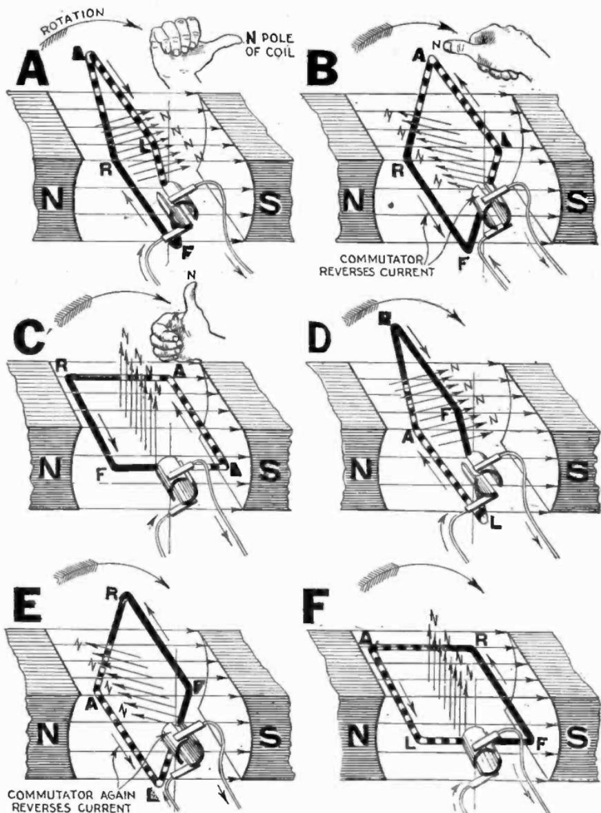
Figs. 947 to 952.—**How a D. C. motor works. III.** Fig. A, current flowing through the coil, LARF, induces a N, pole on the side next to the S, pole of the field magnet and a S, pole on the side next to the N, pole of the field magnet; the attraction of unlike poles causes the coil
