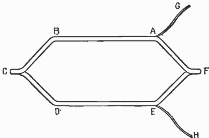
FIG. 817.—Appearance of diamond or hair pin loop coil after being opened out. *In opening out* the coil, the ends C and F, are put into a clamp and twisted at right angles to the plane of the coil. The letters correspond to the points indicated in fig. 816.
