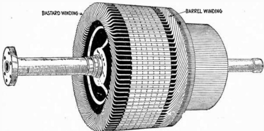
FIG. 815.—Westinghouse combination bastard and barrel winding. A bastard winding at the rear end is combined with a barrel winding at the commutator end, as shown in the illustration, to secure better ventilation.
