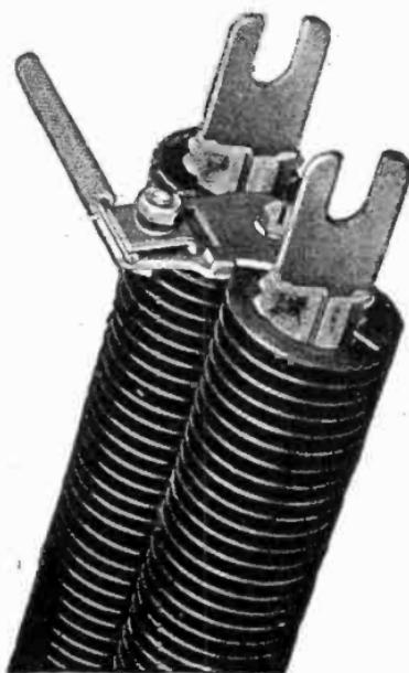
FIG. 1.111.—Monitor bridging clamp connecting adjacent edge-wound resistor units. Also used for taking off intermediate taps when units are in parallel. Clamp takes a firm grip on the ribbon and cannot work loose.
