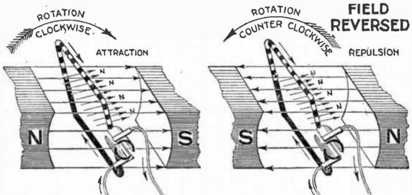
FIG. 997 and 998.—*D.C. Motor principles, 6.* If the polarity of the field be reversed (in practice by reversing the field current through the electro-magnet) the direction of rotation is reversed. In fig. 997, coil turns clockwise due to attraction of unlike poles; in fig. 998, coil turns counter-clockwise due to repulsion of like poles.
