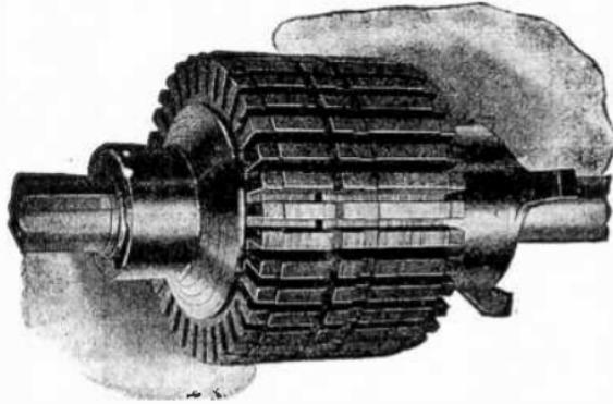
FIG. 787.—General Electric slotted armature core. *The laminations* are of sheet steel, annealed and japanned. They are mounted directly on the shaft (except in the large sizes), and held in place by substantial end plates.
