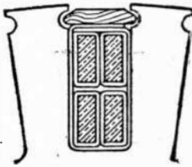
Figs. 792 and 793.—Projecting and notched teeth; cross sections showing inductors and retaining wedges in place.
