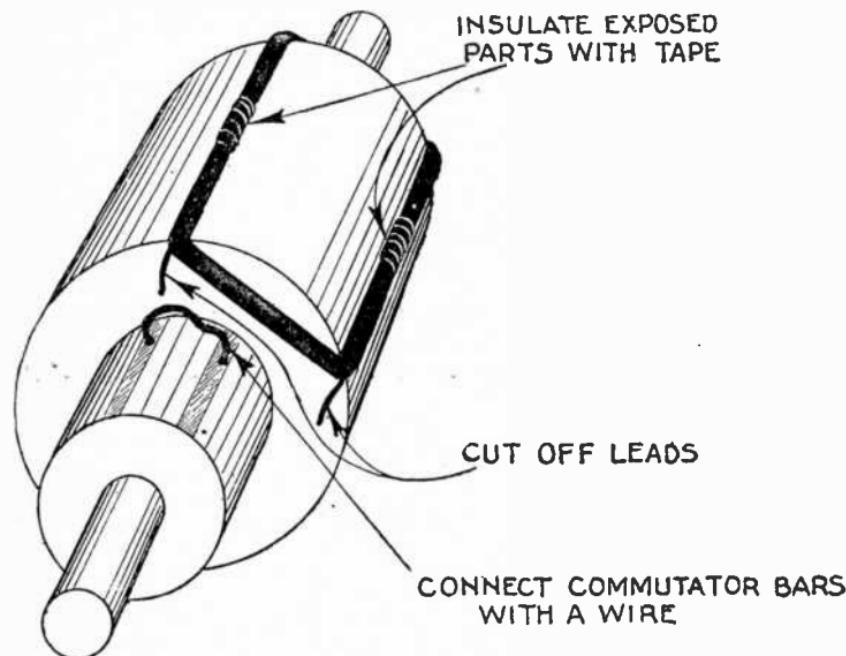
FIG. 894.—Method of cutting out damaged armature coil.
