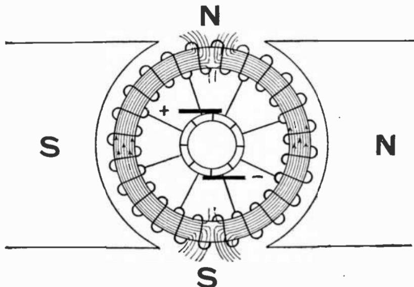
FIG. 708.—Cross magnetization. *This is defined* as lines of magnetic force set up in the windings of a dynamo armature which oppose at right angles the lines of force created between the poles of the field magnet. The figure shows this cross flux which is due to the armature current alone.
