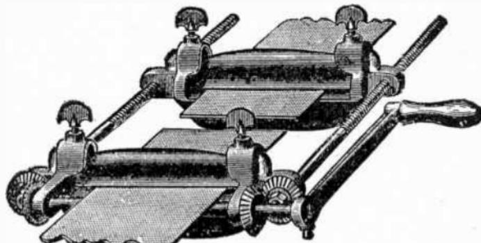
FIG. 1,247.—Belt clamp for stretching belt and holding the ends while making joint. It consists of a *stretching frame*, the two ends of which are coupled by screwed bars; used for pulling the ends of a belt together with the proper tension, when lacing or joining the ends.
