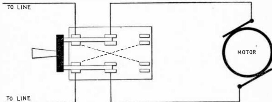
FIG. 1,056.—Double throw, double pole switch for reversing direction of rotation of a motor. The direction of rotation can be reversed by changing the direction of current in either the armature or the field coils. It is preferable, however, to reverse the direction of rotation by changing the direction of current through the armature. The switch is wired as shown, means of reversal being provided by running the wires as indicated by the dotted lines.
