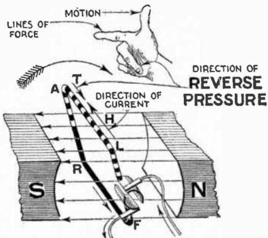
**FIG. 955.—D.C. Motor principles, 2.** The rotation of the coil in the magnetic field induces a reverse pressure which opposes the flow of current in the coil. Applying Fleming's rule to inductor LA, which is moving upward, it is seen that the induced pressure  $T'$ , is in a direction directly opposite to that of the current H, and so opposes its flow; it is accordingly called the reverse pressure.
