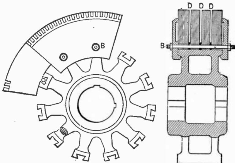
Figs. 794 and 795.—Side and end view of built up armature cores. *The sheet metal ring sections containing the teeth are fastened into dovetail notches in the spider as shown. The layers of ring sections are placed so as to break joints and are held by end clamps and through bolts B. Distance pieces are inserted at intervals to provide ventilating spaces D D D.*
