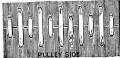
Figs. 1,253 and 1,254.—A simple and reliable method of lacing a belt joint for rubber belt. Fig. 1,253, outside view; fig. 1,254, inside view.
