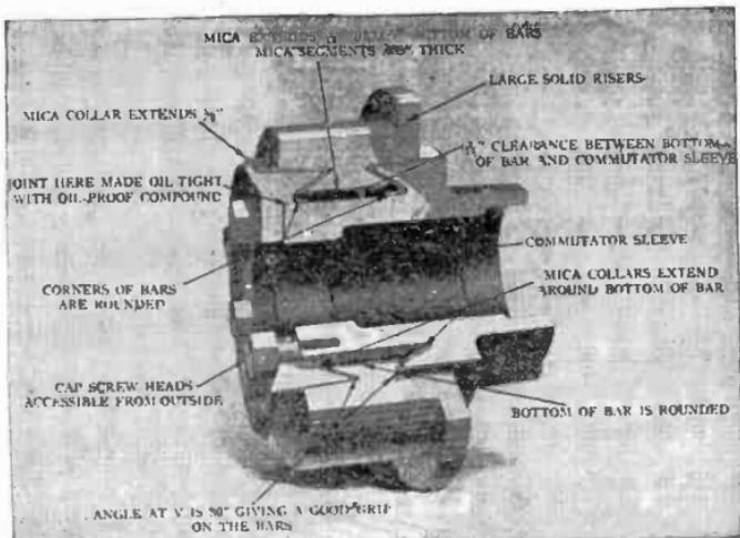
FIG. 1,026.—*Reliance motor construction 26.* Sectional view of commutator.
