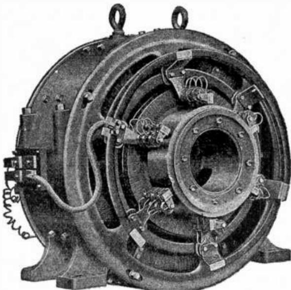
FIG. 853.—Diehl engine type dynamo 50 k.w. 250 volts.
