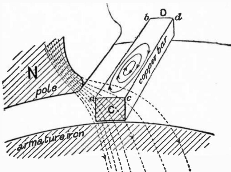
**FIG. 716.**—Formation of eddy currents in a solid bar inductor. On account of the appreciable size of the inductor, the field is sometimes weaker at one point than another, hence the unequal electric pressures thus produced will induce eddy currents.
