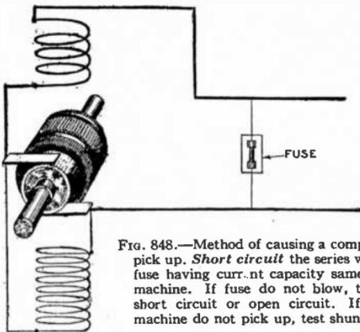
FIG. 848.—Method of causing a compound dynamo to pick up. *Short circuit* the series winding through a fuse having curr. nt capacity same as that of the machine. If fuse do not blow, test armature for short circuit or open circuit. If fuse blow, and machine do not pick up, test shunt winding.
