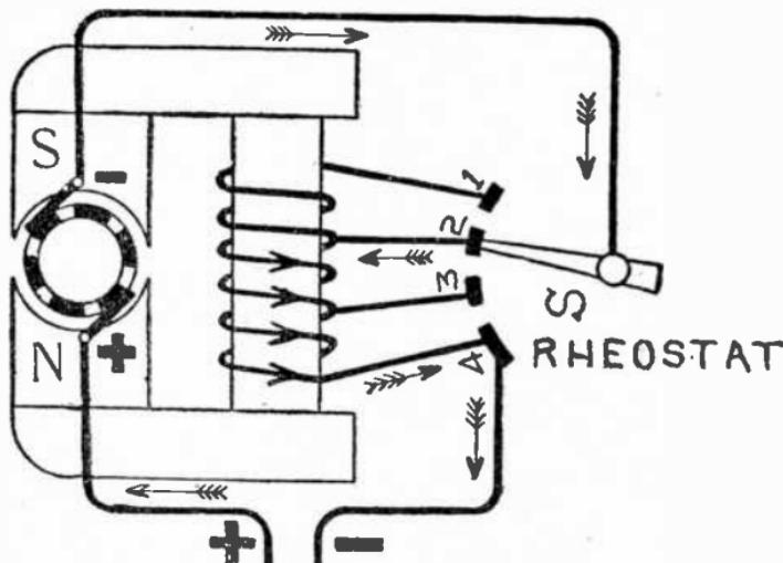
FIG. 1,055.—Variable field method of speed regulation of series motor. *The field winding is divided into a number of sections with leads connecting with switch contact points as illustrated. The speed then is regulated by cutting in or out of the circuit sections of the field winding thus varying the strength of the field.*
