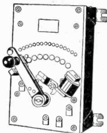
**FIG. 1,133.**—Compound starter. Designed for the double duty of starting a motor and regulating its speed, the resistance provided being a combination of armature resistance for starting duty and shunt field resistance for speed regulation.
