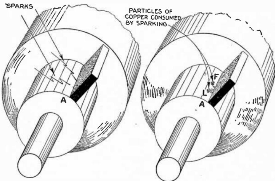
Figs. 902 and 903.—Damage to commutator segments due to sparking. Each spark burns out a particle of copper from the surface of the commutator. For instance, fig. 902 shows two sparks at segment A, passes from under the brush, with resulting burns L and F, as shown in fig. 903.
