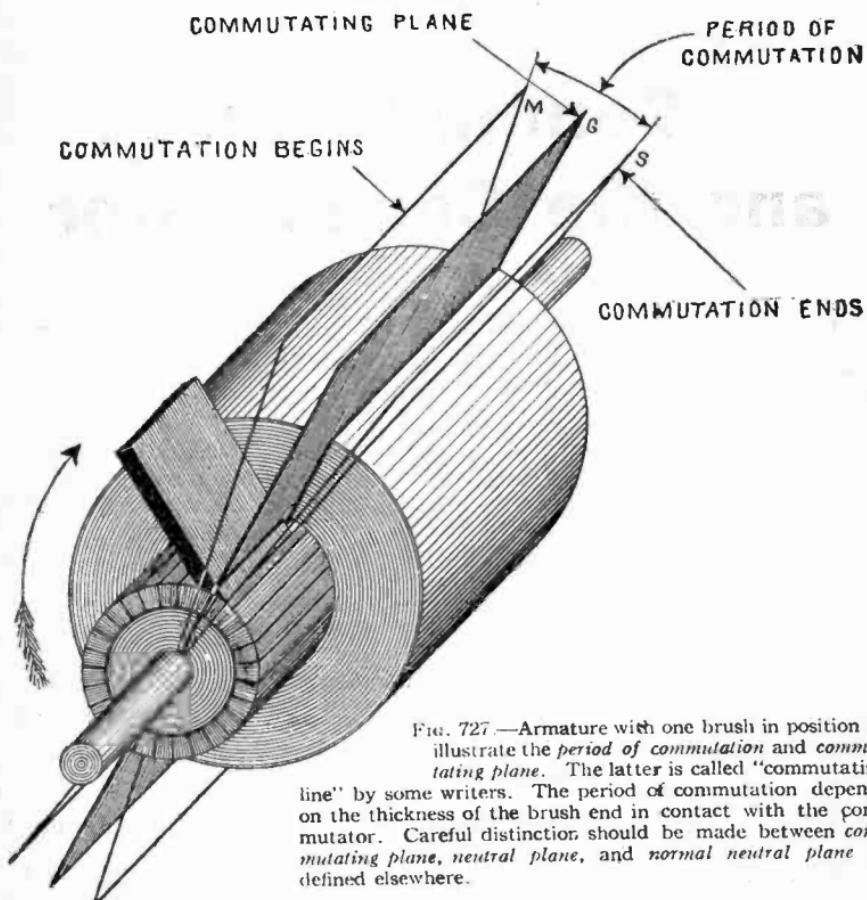
FIG. 727.—Armature with one brush in position to illustrate the *period of commutation* and *commutating plane*. The latter is called "commutating line" by some writers. The period of commutation depends on the thickness of the brush end in contact with the commutator. Careful distinction should be made between *commutating plane*, *neutral plane*, and *normal neutral plane* as defined elsewhere.
