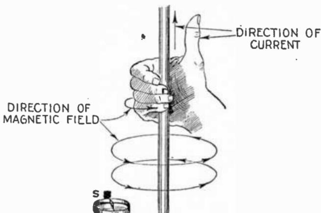
FIG. 967.—Magnetic field in a plane at right angles to a wire carrying an electric current
