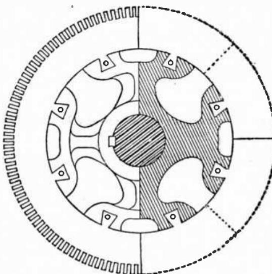
FIG. 796.—Built up core with four spoke spider, each spoke carrying two dovetail notches. *In this construction* a little more air space obtained for ventilation than where a separate spoke is provided for each notch.
