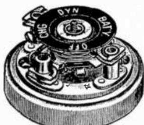
FIG. 1,167.—Gas engine snap switch. The first snap makes connection so that igniter is run from storage battery; second snap connections are changed so that igniter is supplied from dynamo; third snap makes connections so that dynamo supplies igniter and charges storage battery; fourth snap, all off.
