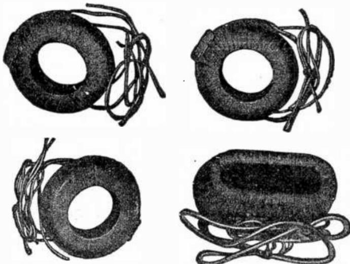
Figs. 1,062 to 1,065.—Diehl field coils. Figs. 1,062 to 1,064, main pole coils; fig. 1,065, interpole coil. The shunt field coils are of enameled wire, form wound and insulated. They are treated with a finishing coat of insulating varnish which aids materially in resisting the destructive action of oil, moisture and excessive dust or dirt.
