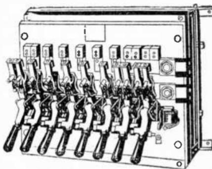
FIGS. 1.136 and 1.137.—Multiple switch starters. Fig. 1.135, starter with no voltage release; fig. 1.137, starter with no voltage release and circuit breaker. The multiple switch type of starter is designed to overcome the arcing on sliding contacts which, in the case of large motors would be very severe. The cutting out of each step of resistance is accomplished in the multiple switch starter by a separate carbon contact switch which breaks the circuit with a quick snappy action.
