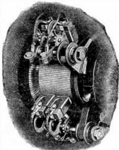
FIG. 504.—Bissell brush gear. The brushes are held in the brush holders radially and work equally well with armature running in either direction. Brushes can be renewed and adjustment made while machine is in operation.
