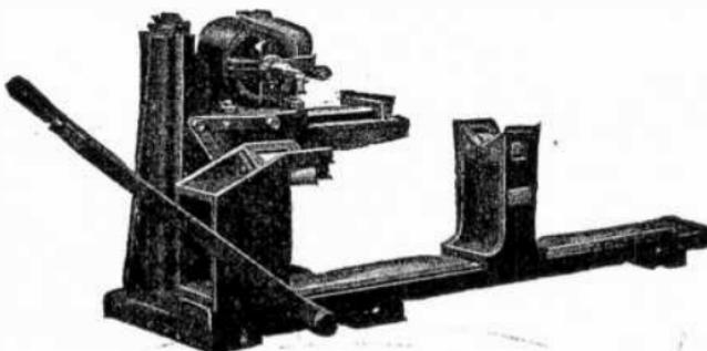
FIG. 928.—General Electric commutator grooving machine; stationary model. *In construction*, the rotating saw is mounted on the end of the motor shaft which is extended and supported by an offset bearing, which readily permits the grooving of commutators having ears. Owing to the small size of the motors used with these machines, no starting resistance is necessary.
