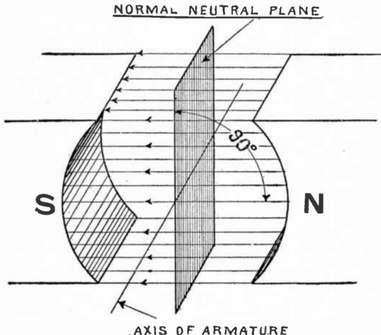
FIG. 711.—Normal neutral plane. This is a reference plane from which the lead is measured. As shown, the normal neutral plane lies at right angles to the lines of force of an undistorted field.
