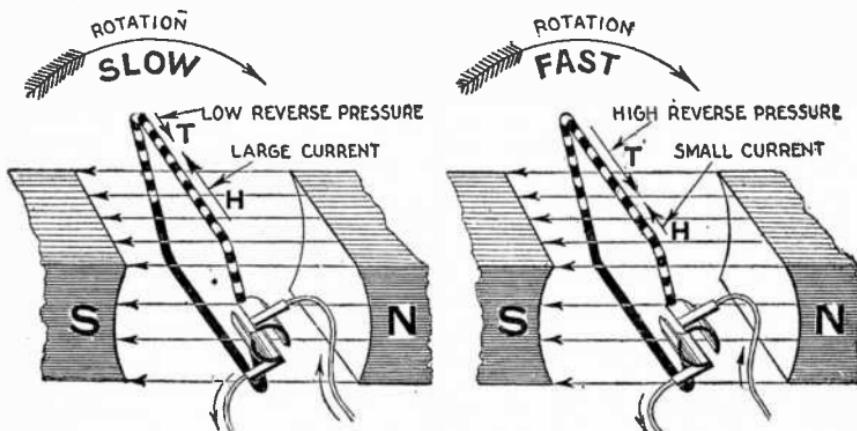
**FIGS. 956 and 957.—D.C. Motor principles, 3.** The amount of current flowing through the coil decreases as the speed increases. As the speed of rotation increases the reverse pressure increases, thus presenting more and more opposition to the current in the coil which reduces the amount of flow.
