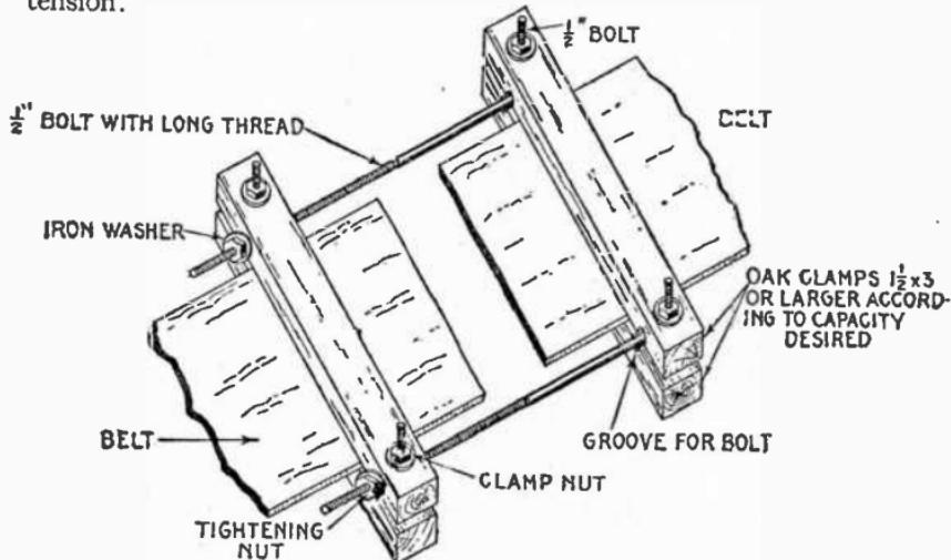
**Fro. 1,265.**—Home made belt clamp. It is made with four pieces of oak of ample size to firmly grip the belt ends where the bolts are tightened. The figure shows the clamp complete and in position on the belt and clearly illustrates the details of construction. In making the long bolts the thread should be cut about three-quarter length of bolt and deep enough so that the nuts will easily screw on.
