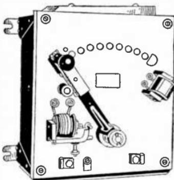
FIG. 1,125.—Starting rheostat with no voltage release and overload release. The no voltage release permits the starting lever to fly to the "off position" should the voltage fail momentarily, thus protecting the motor against damage should the voltage suddenly return to the line. The movement of the lever is due to a spring. The overload device causes the lever to back to the off position should the current exceed a predetermined maximum for which the release is adjusted.
