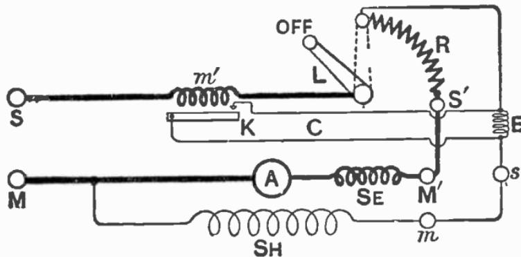
FIG. 1.1^5.—Simplified diagram of the connections of starter connected to compound motor as shown in fig. 1.132.
