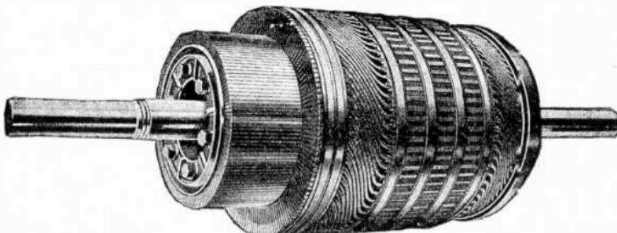
FIG. 800.—Typical iron clad barrel wound armature complete; view showing the openings for ventilation. *The advantage* of the form of winding adopted, is the ease with which a coil may be replaced in case of injury and the additional cooling surface. The coils are held in place by maple wedges secured by binding wires which are soldered throughout their length.
