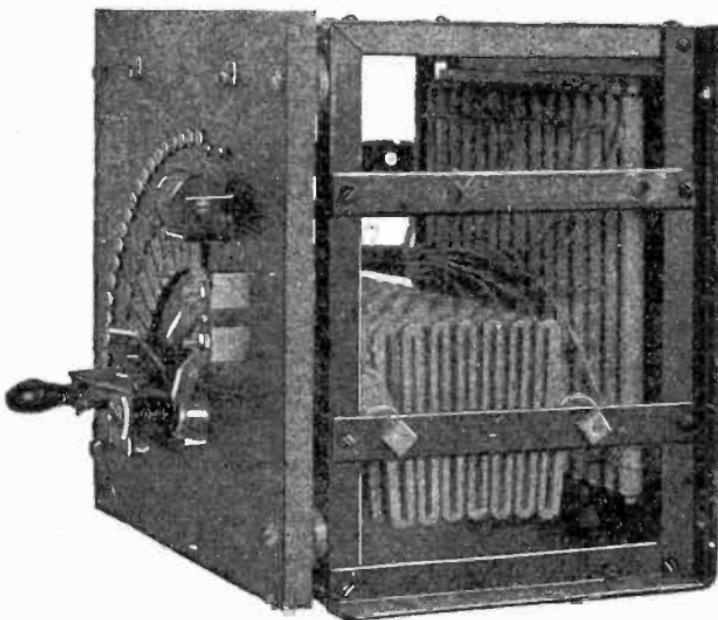
**FIG. 1,134.**—Union non-reversing compound starter and adjustable speed regulator for bringing a general purpose shunt or compound d.c. motor from rest to full normal speed by cutting out armature resistance, and for increasing the motor speed above normal by adding resistance to the shunt field circuit.
