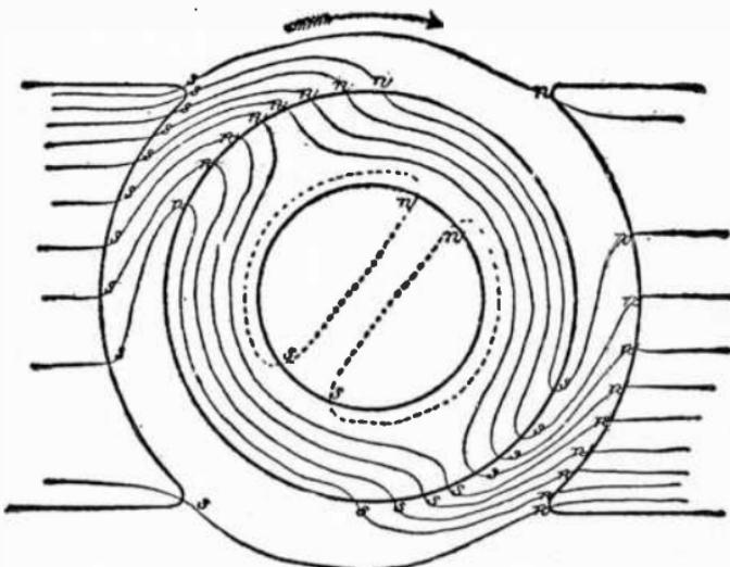
**FIG. 709.**—Distortion of magnetic field due to cross magnetization. *For clearness, the effect is shown somewhat exaggerated.* A drag or resistance to the movement of the armature is caused by the attraction of the north and south poles on the armature and pole pieces respectively.
