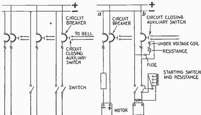
Figs. 1,212 and 1,213.—Common applications of air circuit breakers. Fig. 1,212 two wire d.c. feeder circuits protected by over current breakers with bell alarm switches; fig. 1,213 d.c. motors protected by over current breakers with bell alarm switches; *a*, double pole single coil breaker, no switch required, under voltage device is on the starting rheostat; *b*, single pole breaker in series lever switch, under voltage device on the breaker.
