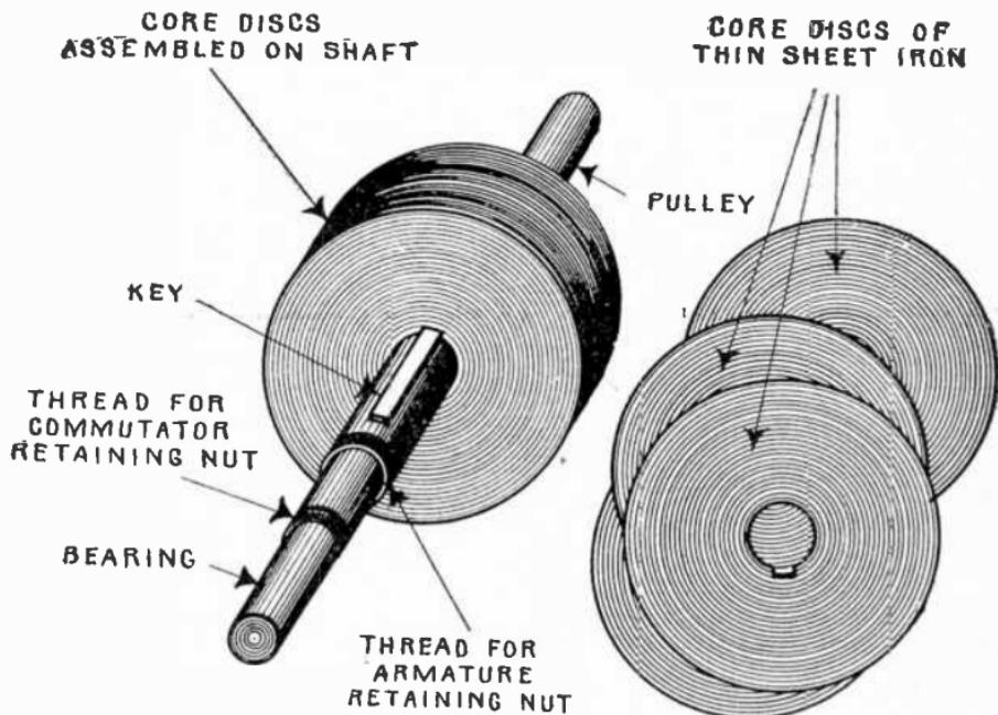
FIG. 781 and 782.—Laminated smooth core armature partly assembled. *It consists of* numerous discs of thin sheet iron threaded on the shaft and pressed together by end plates. The object of this construction is to prevent eddy currents.
