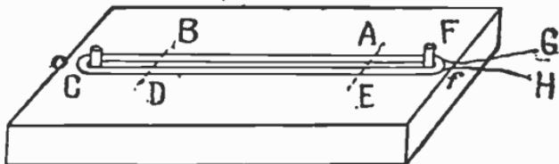
FIG. 818.—Another and simpler method of winding a diamond or hair pin loop coil. A board with only two pins is employed as shown; this plan, however, gives more trouble in the subsequent opening out of the coil.
