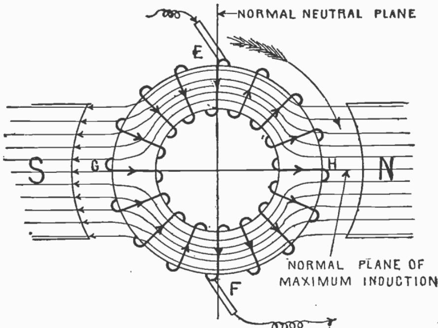
FIG. 728.—The proper position of the brushes, if there were no field distortion and self-induction in the armature coils, would be in the normal neutral plane. In the actual dynamo these two disturbing effects are present which makes it necessary to advance the brushes as shown in figs. 729 and 730 to secure sparkless commutation.
