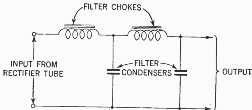
FIG. 6—Choke-input filter.
