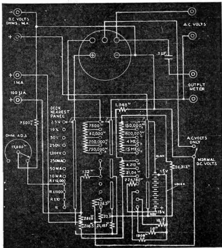
FIG. 14—Wiring diagram of Weston Model 772 analyzer.
