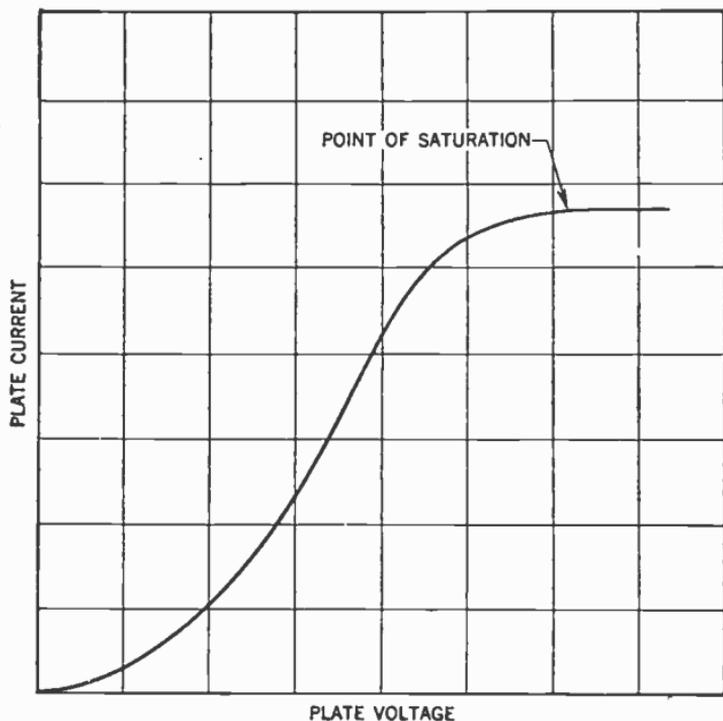
FIG. 6.—Characteristic curve of a diode.
