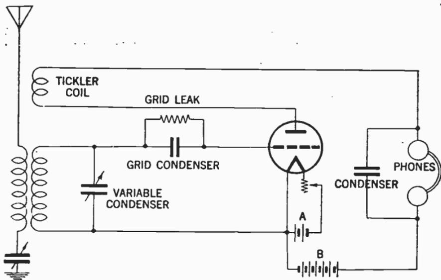
FIG. 17—Regenerative circuit. The scheme of combining a detector circuit with a separate oscillator circuit is called *heterodyning* and oscillators built exclusively for this purpose are called *heterodynes*. A circuit such as this is known as a *regenerative circuit*, and this term is applied to any detector circuit in which a coupling is provided between the plate and the oscillatory grid circuit.
