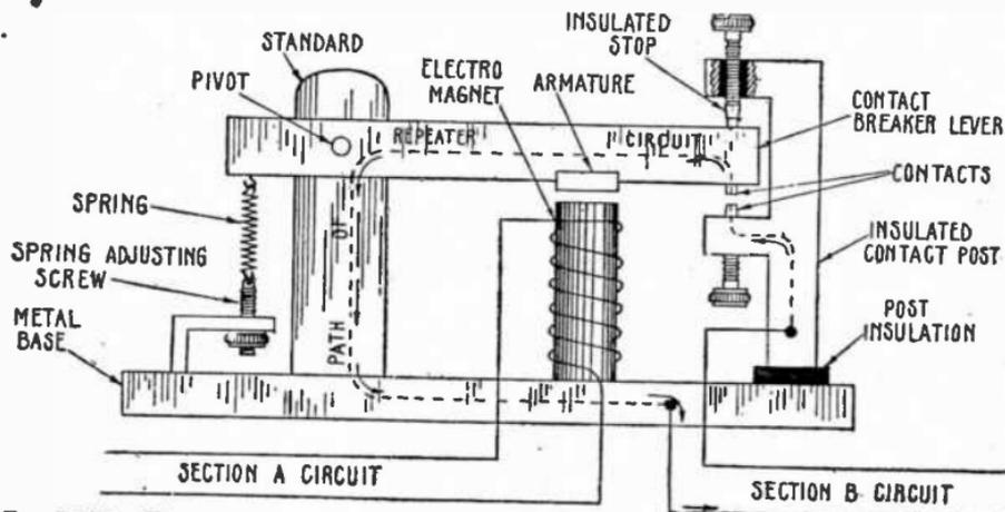
FIG. 7,700.—Elementary repeater showing the insulated parts essential for the contact maker, and path of the current through the repeater portion of the instrument. The insulated stop on the upper arm of the contact post is shown in sectional view to clearly indicate the insulation at this point. Compare this instrument with the elementary sounder fig. 7,696 and note the essential points of difference.
