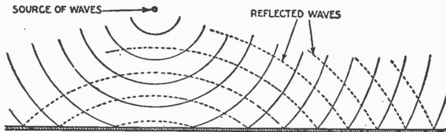
FIG. 7,845.—Reflection of waves from a plane surface.
