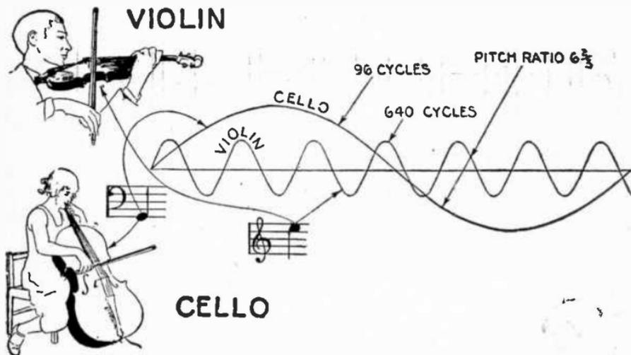
FIG. 7,849.—Properties of wave motion illustrating *pitch*.
