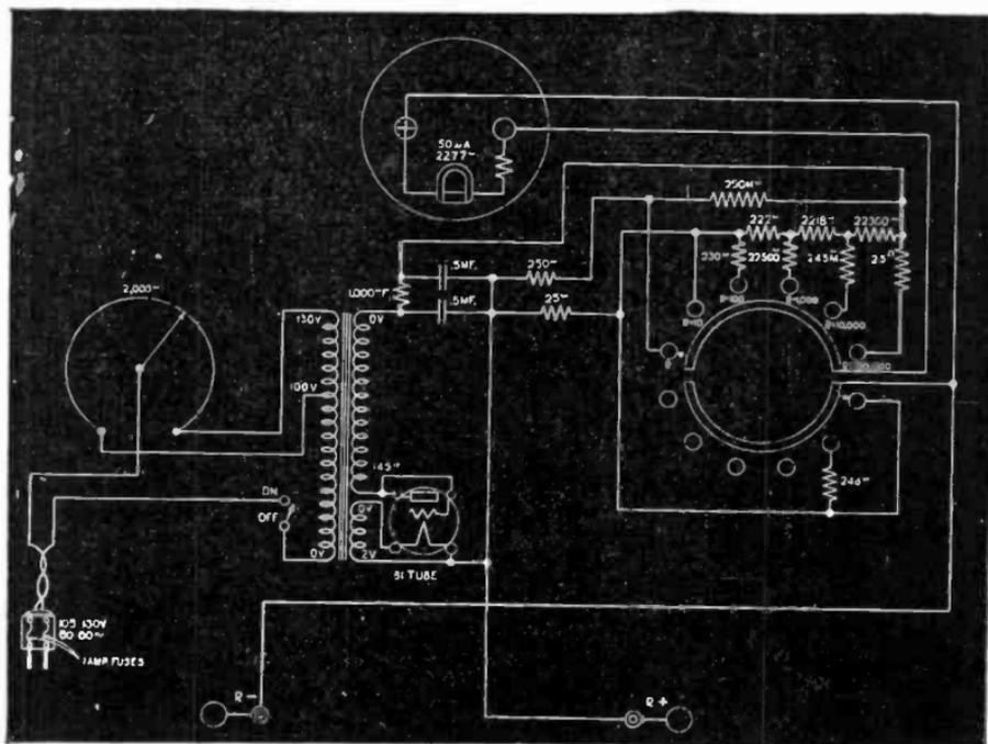
FIG. 10—Wiring diagram for internal connection of Weston Model 763 ohm-meter.
