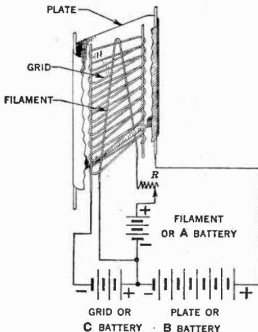
FIG. 7.—Schematic diagram showing triode connection to battery.
