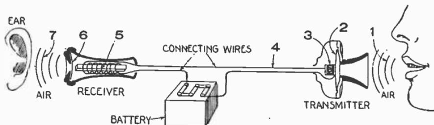
FIG. 7,478.—Electric telephone. *The parts are:* 1, air vibrations caused by voice; 2, diaphragm; 3, carbon buttons; 4, line wires; 5, electro-magnet; 6, diaphragm; 7, reproduced air vibrations representing speech.
