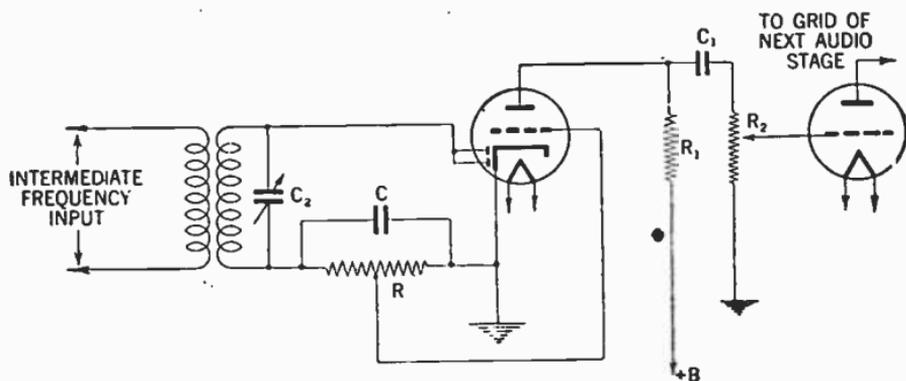
FIG. 23—Diode-biased detector circuit.
