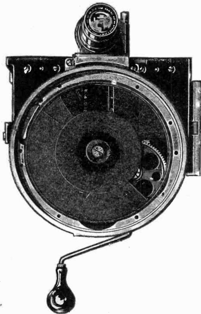
F. G. 7,788.—Bell & Howell camera. Front view with turret plate removed showing shutter, photographing aperture and part of brake mechanism.
