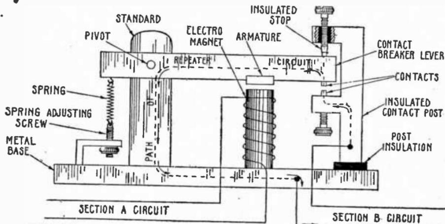
FIG. 7,700.—Elementary repeater showing the insulated parts essential for the contact maker, and path of the current through the repeater portion of the instrument. The insulated stop on the upper arm of the contact post is shown in sectional view to clearly indicate the insulation at this point. Compare this instrument with the elementary sounder fig. 7,696 and note the essential points of difference.
