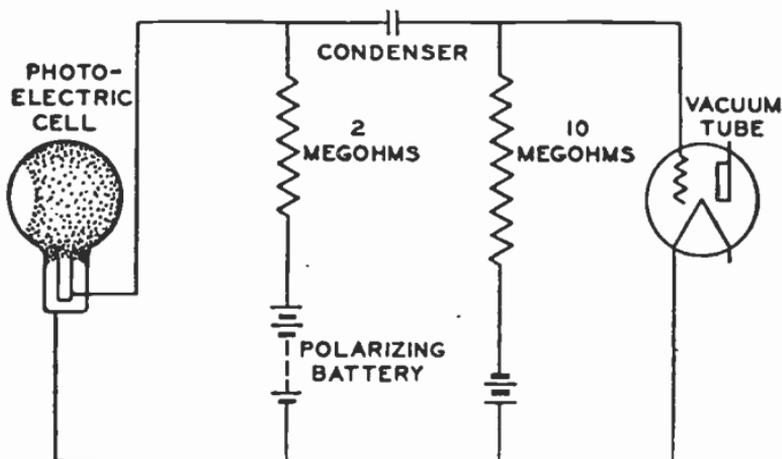
FIG. 7,830.—Photo-electric cell. The characteristic of this device is that when it is polarized by a proper voltage and is used within proper limits the current through it is proportional to the incident light.
