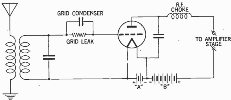
FIG. 26—Detector circuit grid-leak and condenser method.
