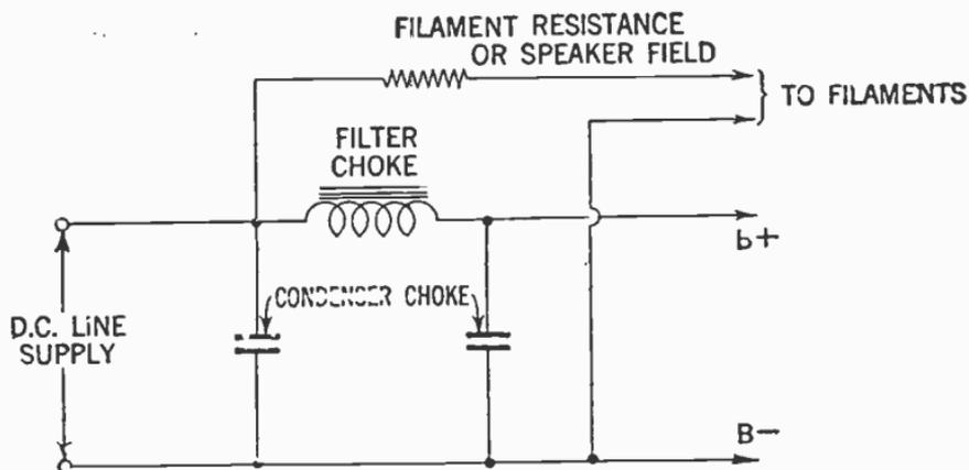
FIG. 9—Conventional filter system used on D.C. receivers.
