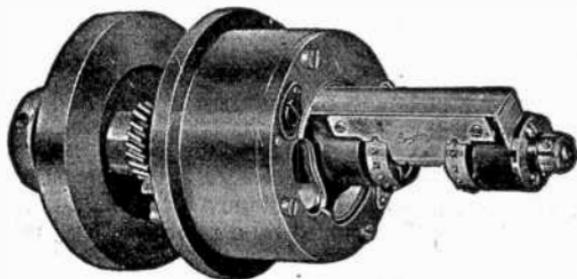
FIG. 7,791.—Simplex Geneva type intermittent movement.
