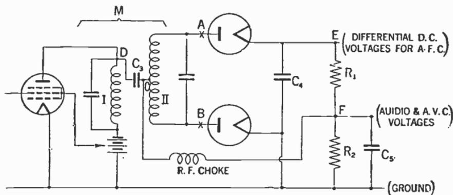
FIG. 3—Automatic radio frequency control detector diagram.
