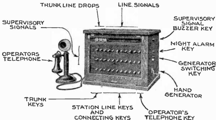
FIG. 7,568.—Cordless type P. B. X. switchboard. There are 3 rows of keys with 11 keys of the cam lever type in each row as follows: 3 keys for central office trunk lines (first 3 keys at left side), each with a trunk line drop above (details of drops shown in fig. 7,528). 7 keys for extension lines (keys 4 to 10), each with a magnetic line signal above; 1 key for the operator's line (last key at right). The keys provide for 5 simultaneous connections.
