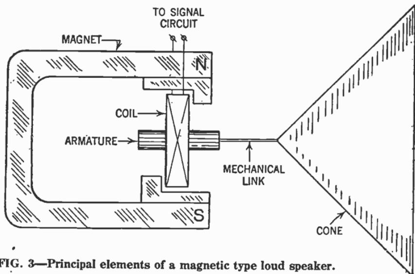
FIG. 3.—Principal elements of a magnetic type loud speaker.
