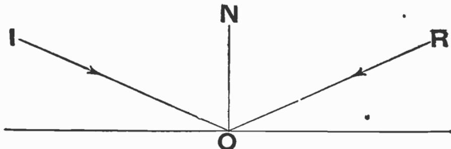
FIG. 7,751.—Angles of incidence and reflection. LAW: *The angle of reflection is equal to the angle of incidence.* The ray IO is called the incident ray; OR, reflected ray; angle ION, angle of incidence; angle NOR, angle of reflection; NO, normal or perpendicular to the reflecting surface.
