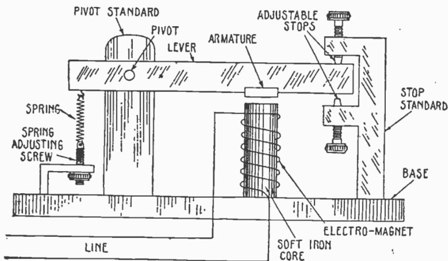
FIG. 7,696.—Elementary sounder showing essential parts.
