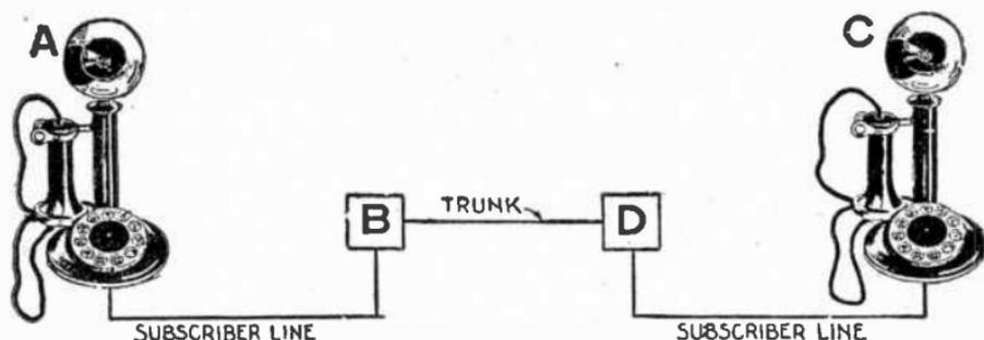
FIG. 7.628.—Simplified dial telephone system. A, telephone subscriber with number ATLantic 2357; B, ATLantic central office; D, MAYflower central office; C, telephone subscriber with number MAYuower 7348.
