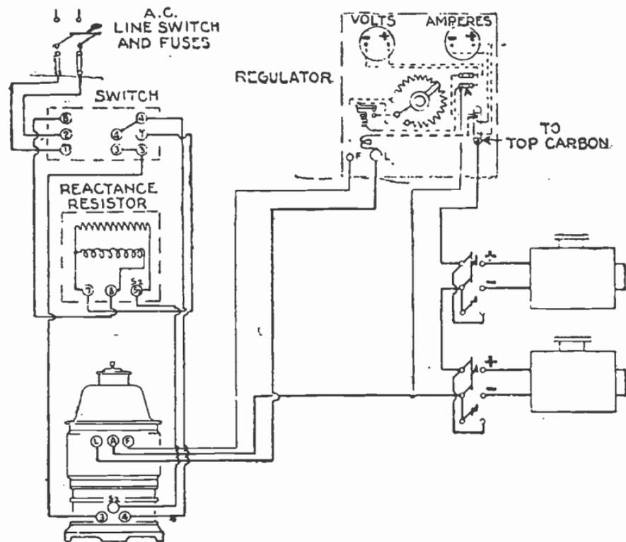
FIG. 7,931.—Wiring diagram of double arc *single phase* arc transverter with control panel. To start throw the handle of the switch to the position marked *start*. Hold there until unit comes up to speed, then throw over to position marked *run*. The starting time is approximately 20 to 30 seconds.
