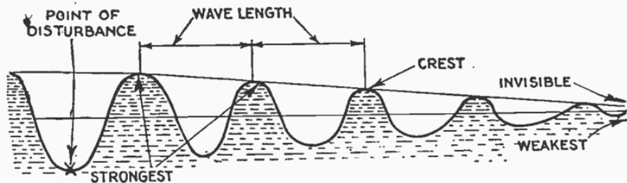
FIG. 7,181.—Sectional view of waves produced by throwing stone in still water, illustrating crest of wave, wave length and gradual weakening of the waves as they travel from the point of disturbance.
