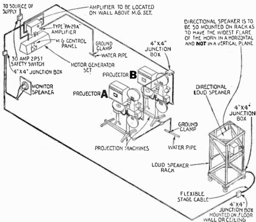
FIG. 7,943.—General layout of a typical RCA type PG-13 installation showing inter-apparatus conduit runs.
