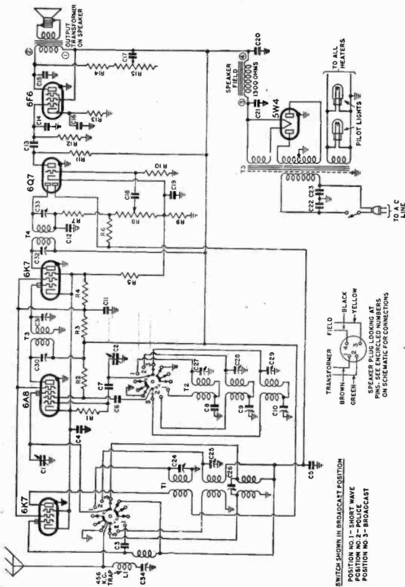
FIG. 7-331.—Circuit diagram of a 6-tube all-wave a.c. superheterodyne receiver. (Emerson Model S-147, S-151) i.f. peaked at 456 kilocycles. Voltage rating 105-125 volts. Current drain 0.55 amperes. Frequency ranges 550 to 1,750 kilocycles; 1,750 to 5.5(M) kilocycles; 5.7 to 18.0 megacycles.
