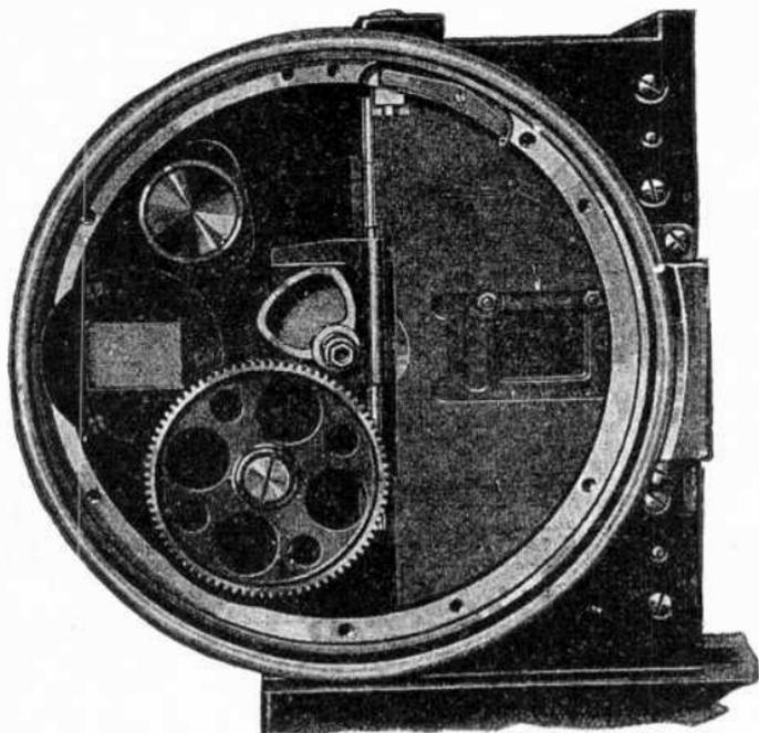
FIG. 7, '89.—Bell & Howell camera. Front view with turret plate and shutter removed showing focusing and photographing apertures; shuttle operating cam, part of brake mechanism and opening for mounting focusing magnifier above focusing aperture.
