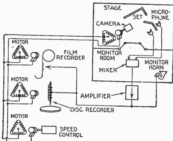
FIG. 7,854.—Studio sound recording system in its simplest form. The essential parts of such a system consist of microphone pick ups on the stage, a mixer and volume control in the monitor room, system and monitor amplifiers, recording machines, and a synchronous motor system for synchronizing the recorders with the cameras.
