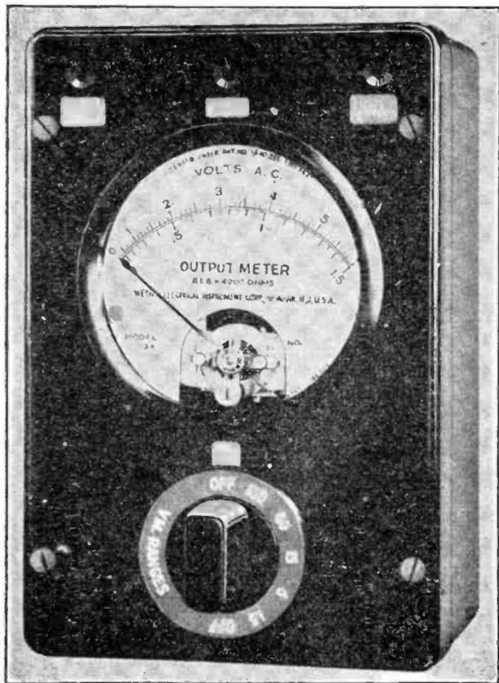
FIG. 7—Panel view of Weston Model 571 output meter.
