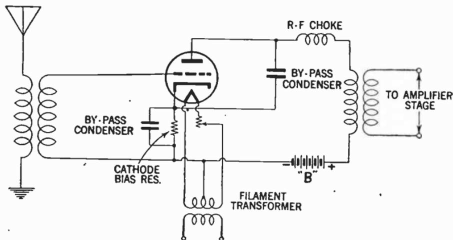
FIG. 25—Grid-biased detector circuit.
