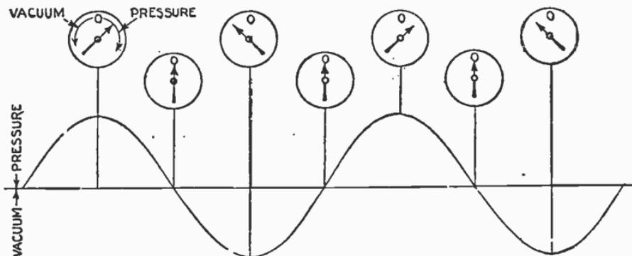
FIG. 7,843.—Diagram illustrating pressure variations due to sound waves. *It should be noted that the type gauges shown, register pressure above atmospheric when the pointer moves to the right of the vertical, and vacuum or pressure below atmospheric when it moves to the left of the vertical.*
