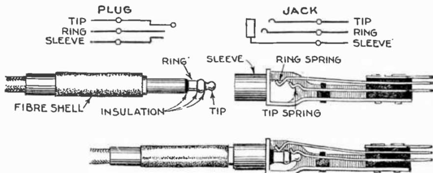
Figs. 7,545 to 7,551.—Jack and plug details showing how connections are made by inserting a cord plug into a jack. Each jack has three contacts known as tip, ring, and sleeve, and the cord plug has tip, ring and sleeve to correspond. Hard rubber is used for insulation of the contacts.
