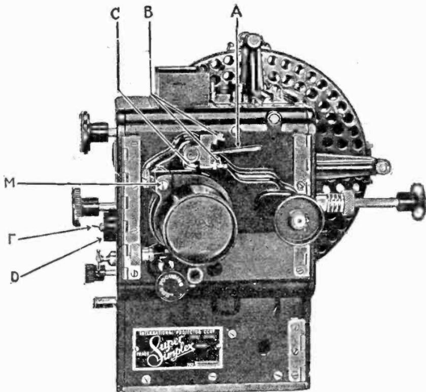
FIG. 7,824.—Super-Simplex projector; view showing adjusting lever, threading and framing lamp, etc. To replace lamp: Loosen screws which hold switch assembly and lamp socket in lacquered base; the entire assembly may then be removed and lamp readily replaced.
