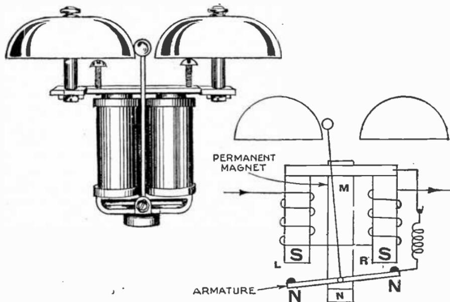
FIGS. 7,516 and 7,517.—Ringer and diagram of its operation.
