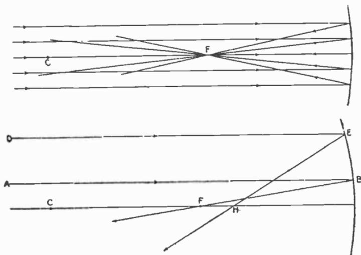
FIGS. 7,763 and 7,764.—The principal focus. *By definition*, it is that point where all the rays parallel with the principal axis meet after reflection, as, for instance, the rays from a source of light at an infinite distance from the mirror. The sun is so far distant that its rays are practically parallel. When they are reflected upon a concave mirror they are reflected to the principal focus F; forming a point of intense light and heat.
