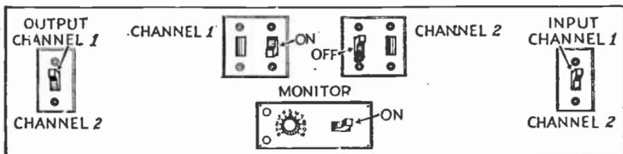
FIG. 7,892.—Patent amplifier cabinet showing how switches should be set for operation. *In starting:* 1, set the fader at zero. 2, throw on main switch for channel one on amplifier cabinet; throw on input and output switches for channel one on same cabinet; throw on exciter lamp switch; throw on filament supply switch for booster unit; throw on speaker field switch—if current supply be other than 50 or 60 cycles a.c., throw on switch for power supply unit for amplifier and power pack.
