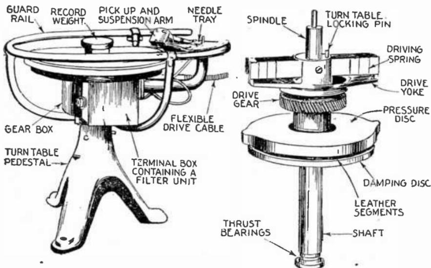
FIG. 7,885.—Typical synchronous turntable showing construction.
