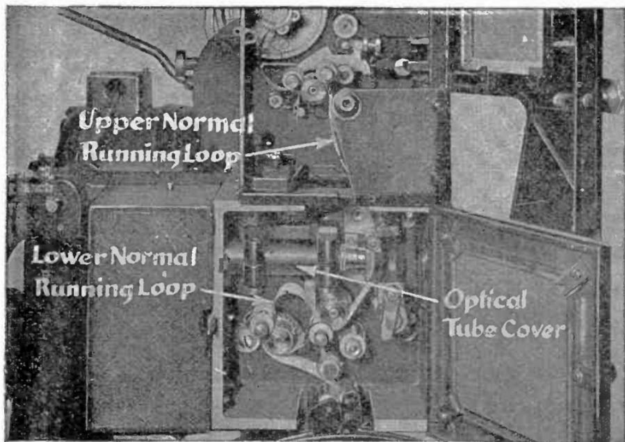
FIG. 7,894.—Pacent projector head and sound head showing proper size for lower normal running loop between constant speed sprocket and take up sprocket.
