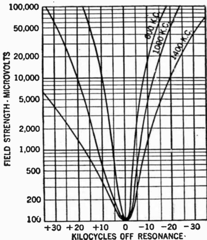
FIG. 5—A typical radio receiver selectivity curve.
