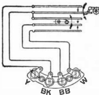
Figs. 7,632 and 7,633.—Assembled dial and wiring diagram.
