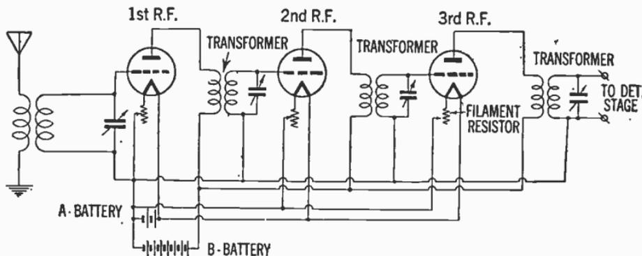
FIG. 14—Three stage radio frequency amplifier circuit.
