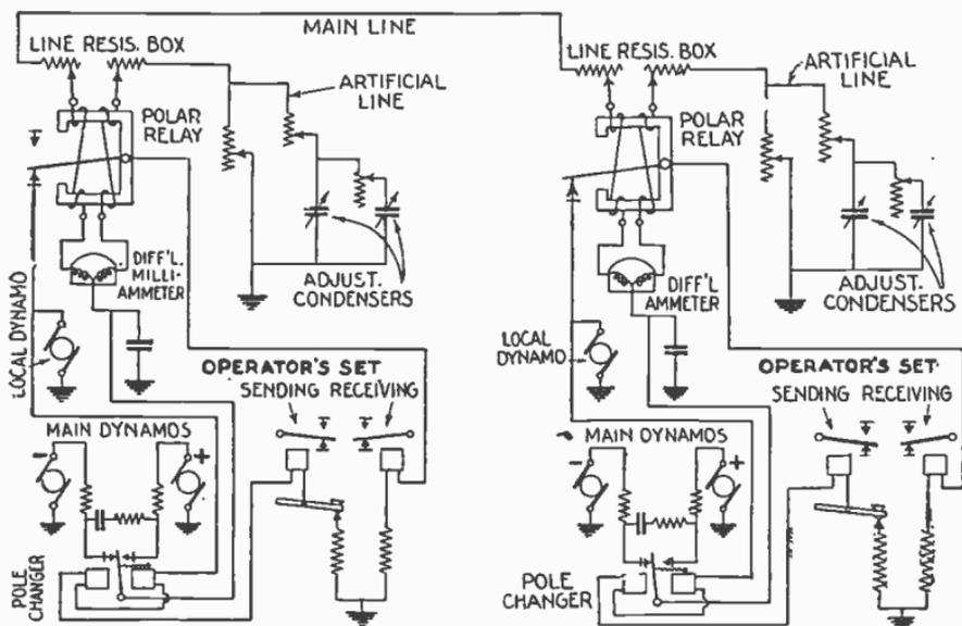
FIG. 7,744.—Teletype circuit diagram for duplex operation showing entire artificial line.
