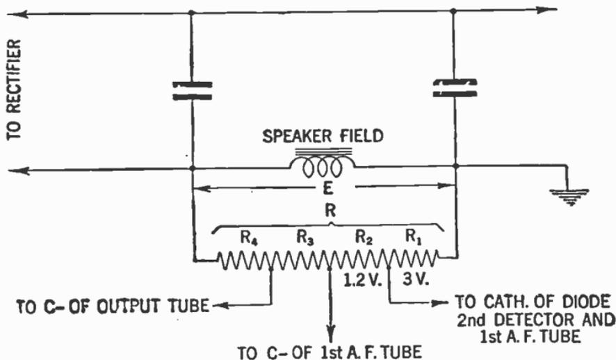
FIG. 41—Method of obtaining grid bias by utilizing voltage drop across speaker field coil.
