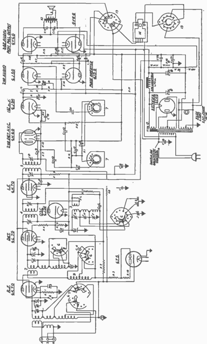
Fig. 7.335.—Schematic circuit diagram of a 12-tube superheterodyne, 3-band radio receiver. (Zenith Models 12-S-205, 12-S-252, 12-S-245, 12-S-265, 12-S-266, 12-S-267, 12-S-268.) *I.f.* frequency 456 kilocycles. Line voltage 117 volts a.c. 50 to 60 cycles. Power consumption 110 watts.
