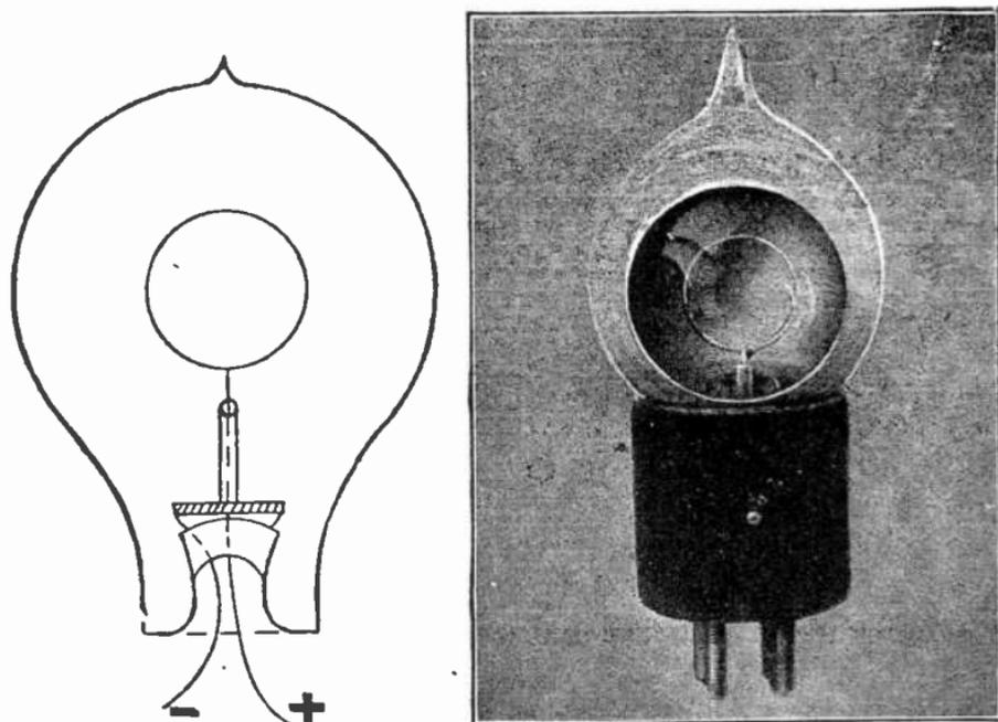
FIG. 7,878 and 7,879.—Jenkins type SR1 photo-electric cell. It is gas filled and suitable for sound moving picture work relay operation; also for television direct pick up work when the ionization voltage is properly chosen.
