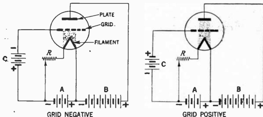
FIG. 8.—Illustrating the action of a grid in a triode vacuum tube.
