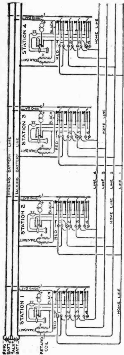
SCHEMATIC WIRING DIAGRAM OF INTERPHONE SYSTEM NO. 1
