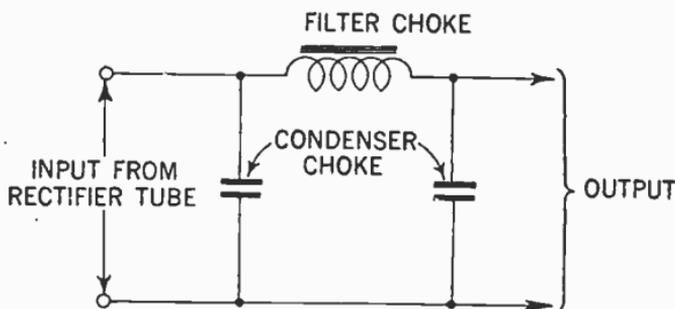
FIG. 7—Condenser-input filter.
