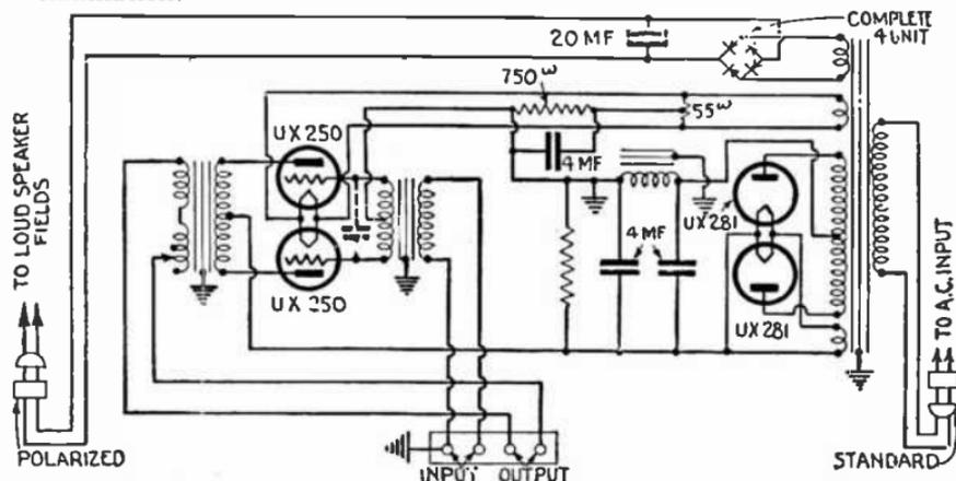
FIG. 7,951.—Wiring diagram for power amplifier. Note: Capacitor pack (3-4 mf. cond. 1-20 mf.). New SPU-62 includes 50 mmf. condenser across secondary of input transformer, also large radiating plates for Rectox.
