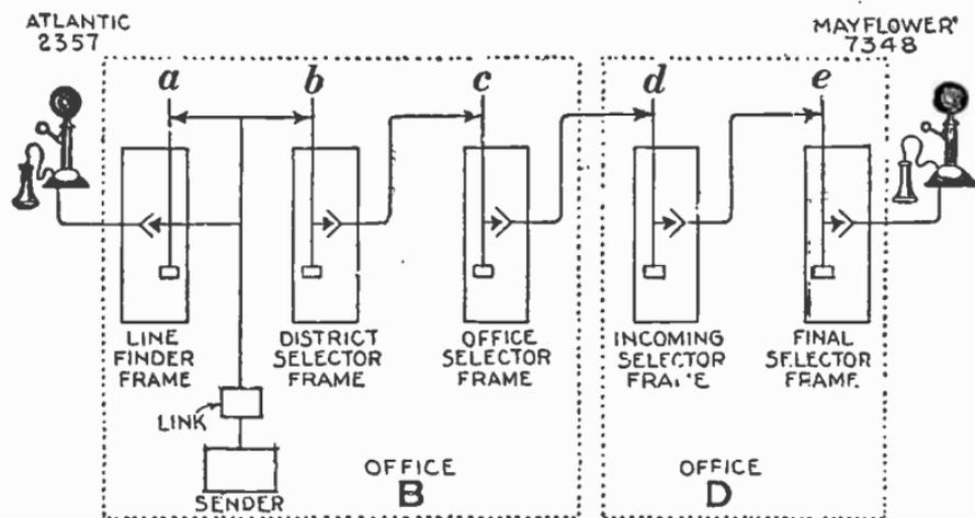
FIG. 7,631.—Panel dial system—routing of a call. a, line finder; b, district selector; c, office selector; d, incoming selector; e, final selector.
