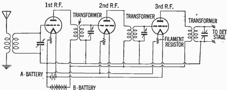
FIG. 14—Three stage radio frequency amplifier circuit.
