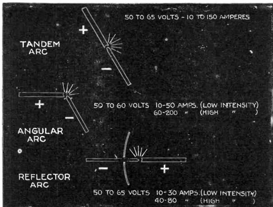
Figs. 7,935 to 7,937—Various projector arcs. Fig. 7,935, tandem arc; fig. 7,936, angular arc; fig. 7,937, reflector arc.
