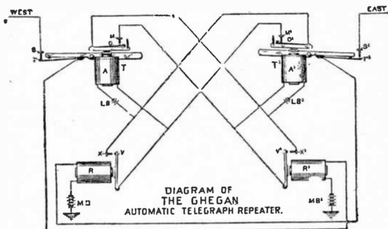
FIG. 7,717.—Diagram of Ghegan automatic repeater. Its principle of operation is based upon the fact that an armature, on being drawn toward a magnet becomes itself magnetic by induction, and that the closer it approaches the magnet core, the stronger the magnetism becomes. The circuits and operation are further explained in the accompanying text.
