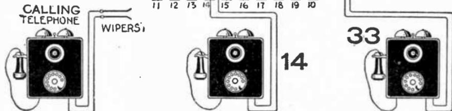
FIG. 7,687.—Diagram of line bank contacts, associated with each connector and numbering system of the telephone lines of which they are the terminals. The number of any set of terminals can be determined by noting the number of vertical and sidewise steps the wipers must be given to reach that set, remembering that ten steps are always represented by zero. Thus six vertical steps and ten rotary steps would cause the wipers to reach contact No. 60.
