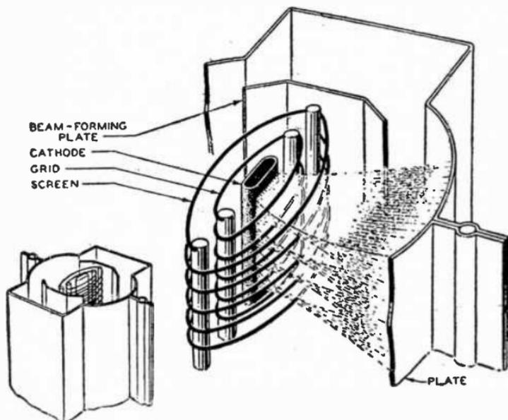
FIG. 13.—Internal structure of beam power tube.
