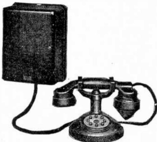
FIG. 7,598.—Graybar selective ringing common talking cradle type inter phone system. *It consists of a hand set with a cradle type mounting having push buttons mounted in the base. The hand set is black moulded bakelite. The interphone set includes an apparatus box containing a bell and a connecting block.*
