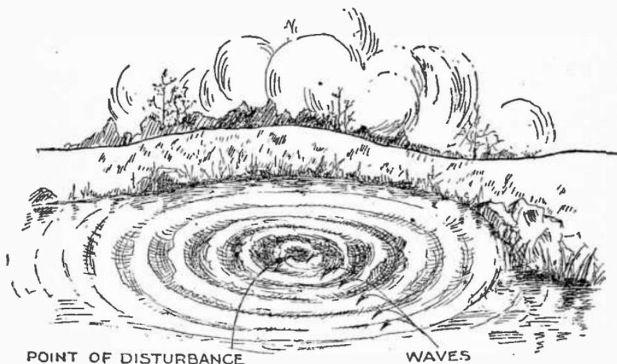
FIG. 7,180.—Effect of throwing stone in still water; production of waves which radiate or travel from the point where stone enters the water, or "point of disturbance."
