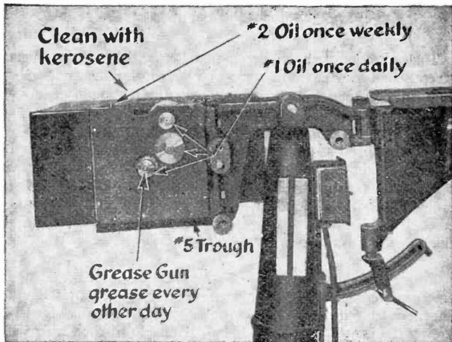
FIG. 7,913.—Patent film head with oiling and greasing indications.
