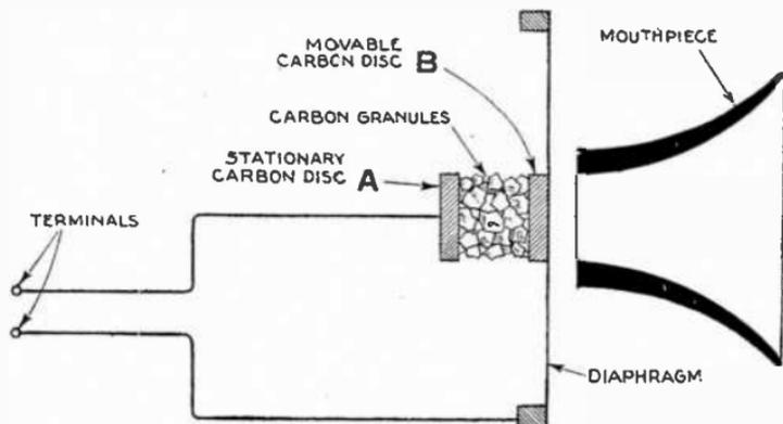
FIG. 7,479.—Simple electric telephone transmitter.
