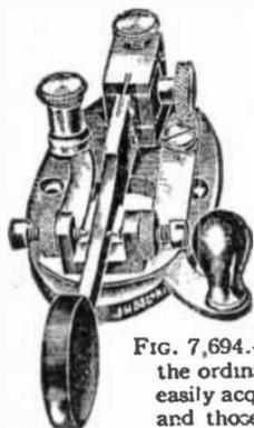
FIG. 7,694.—Bunnell double speed key. *It requires only one-half the motions of the ordinary key, and these are made by a sidewise rocking motion of the hand, easily acquired, which guarantees that operators will not be affected with cramp, and those who are so affected will soon recover their speed.*
