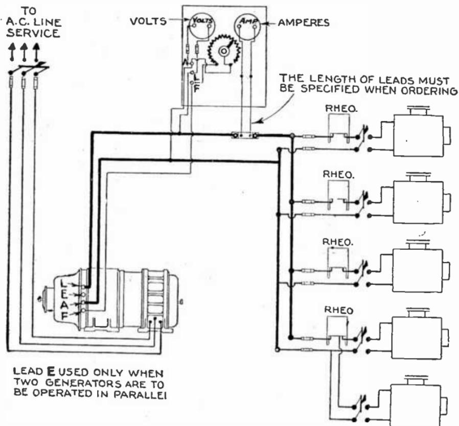
FIG. 7,953.—Wiring diagram of multiple arc transverter, three phase motor.
