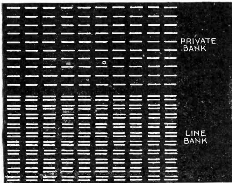
FIGS. 7,672.—Diagram showing contacts of line and private banks of a 100 line system. These banks form a part of the connector switch.
