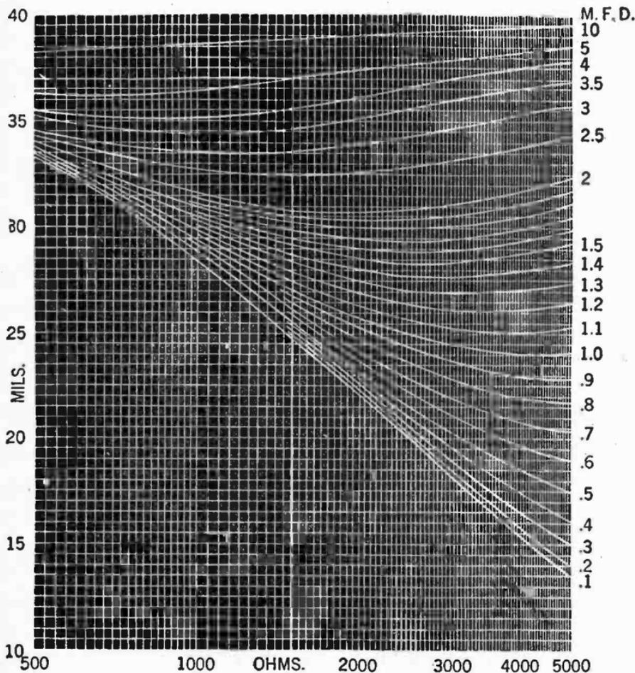
FIG. 3—Parallel resistance-capacity chart. Charts may conveniently be designed to suit individual requirements.
