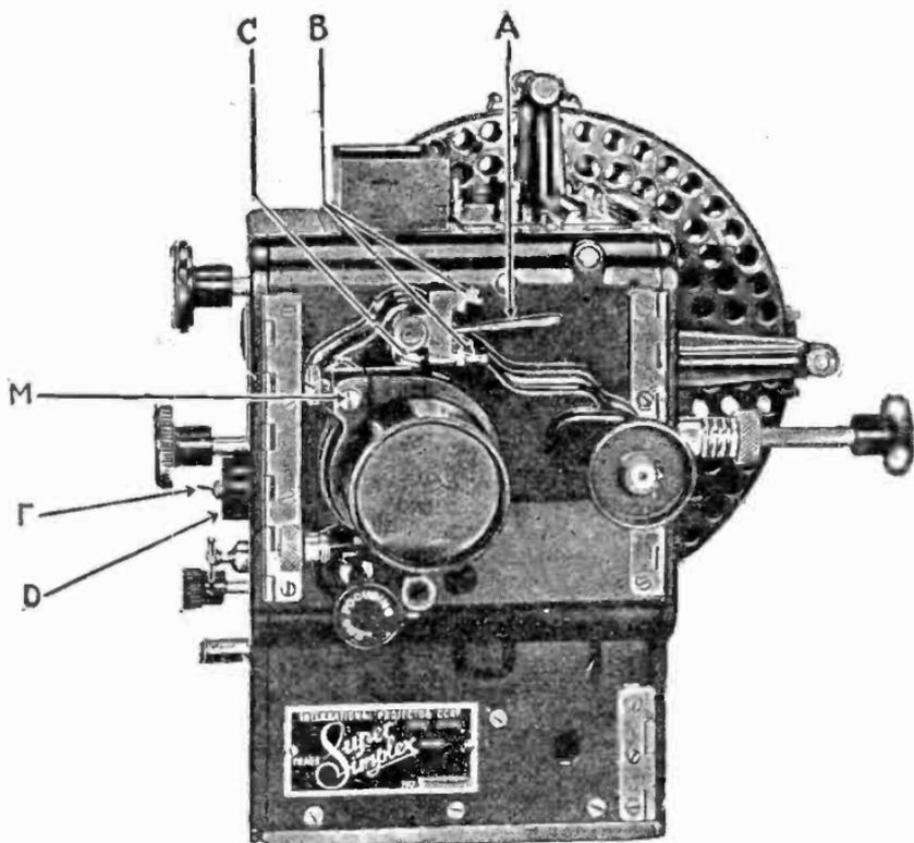
FIG. 7,824.—Super-Simplex projector; view showing adjusting lever, threading and framing lamp, etc. **To replace lamp:** Loosen screws which hold switch assembly and lamp socket in lacquered bakelite; the entire assembly may then be removed and lamp readily replaced.
