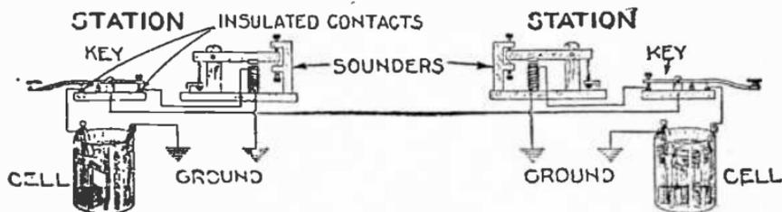
FIG. 7,701.—Elementary diagram showing a simple short line *open circuit* system. In Europe this system is in general use; it consists essentially of so arranging the apparatus that the battery shall only be placed on the line when a message is being transmitted. A main battery is necessary at each station, whereas in the *closed system*, employed in America, main batteries are required only at the terminal stations.
