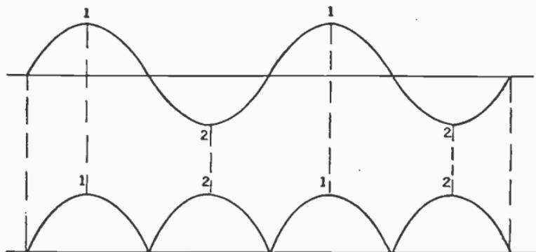
FIG. 5.—Connection diagram and depiction of the action of a full-wave rectifier tube.
