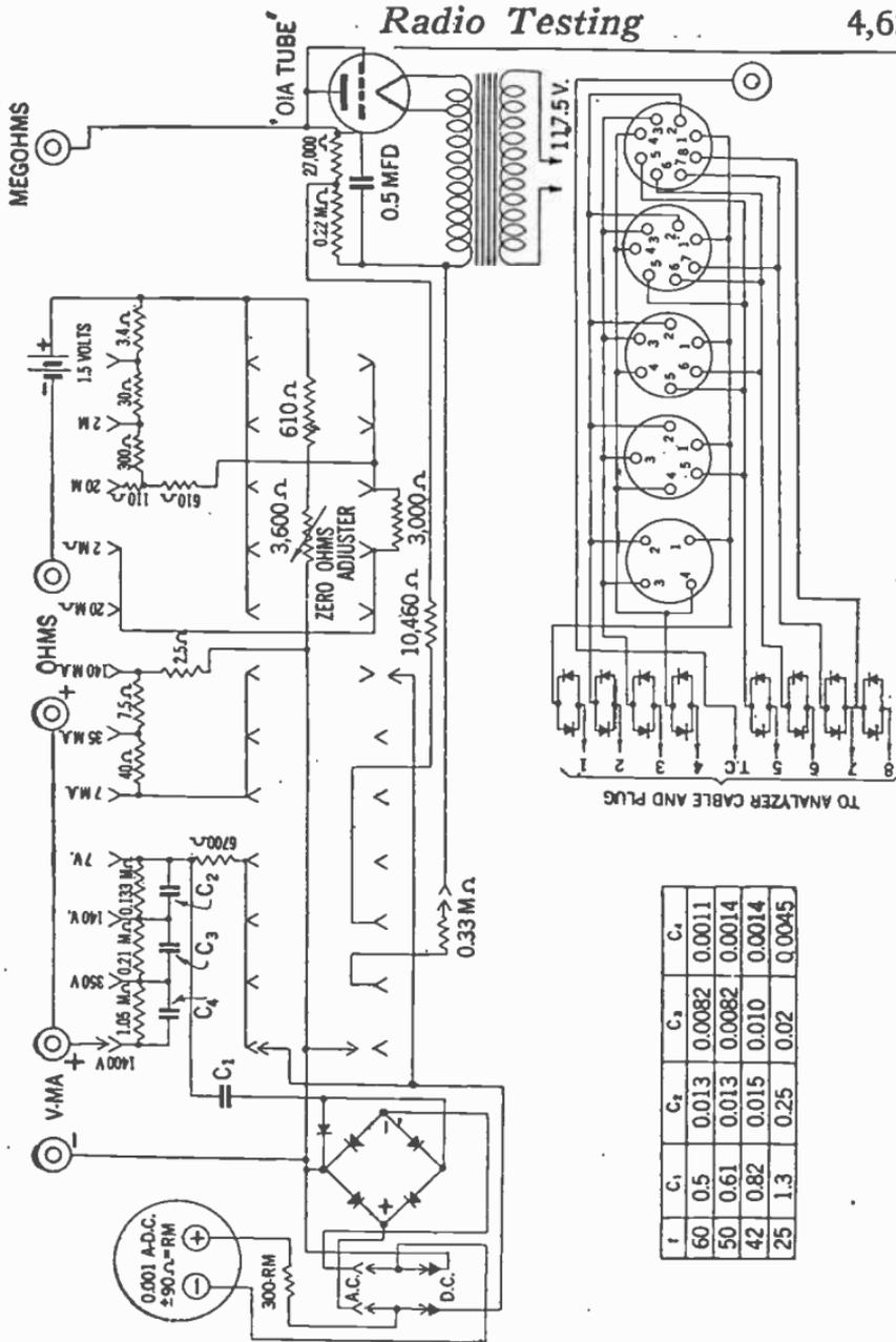
FIG. 27—Wiring diagram of Supreme Model 551 analyzer.
