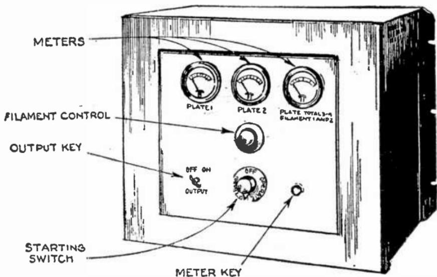
FIG. 7,916.—Western Electric type 46-B amplifier.
