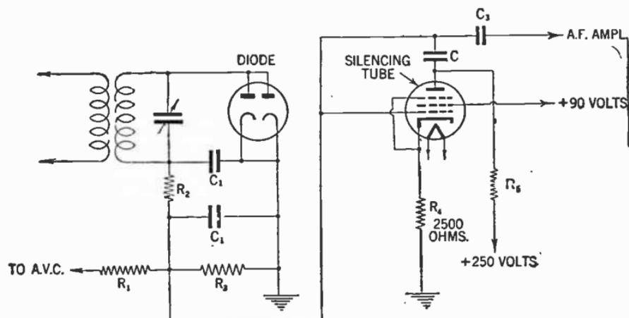
FIG. 14—Automatic tone control circuit.
