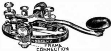
FIG. 7,693.—Bunnell open circuit key. *When it is preferable to use dry cells instead of closed circuit cells this type of key is recommended. Even though a closed circuit be maintained for communication in either direction no current is being used except when key is depressed. Each individual station supplies its own current.*
