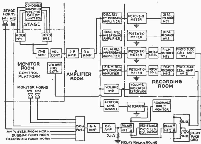
FIG. 7,855.—One complete recording channel.
