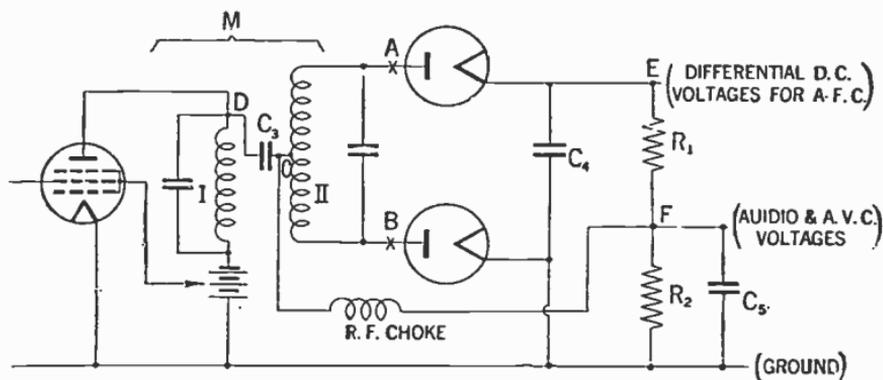
FIG. 3—Automatic radio frequency control detector diagram.
