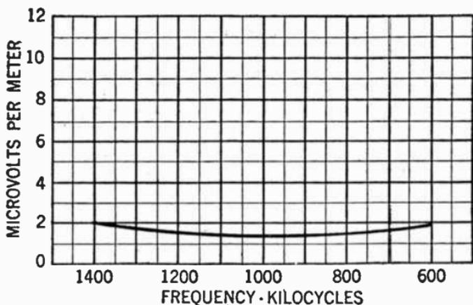
FIG. 7.—Typical radio receiver, sensitivity characteristics.
