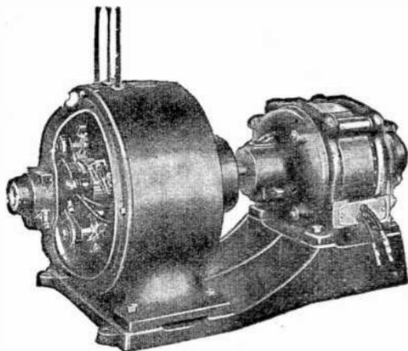
FIG. 7,906.—General Electric *a.c.* to *d.c.* motor dynamo compensarc. For use when the source of power is *a.c.* The equipment operates from an *a.c.* circuit and delivers *d.c.* of proper voltage to the projection arc. Sixty per cent of the moving picture theatres are located so that only *a.c.* is obtainable. The motor in this set, being a standard induction motor, can be obtained for any commercial lighting or power circuit whether single, two or three phase.
