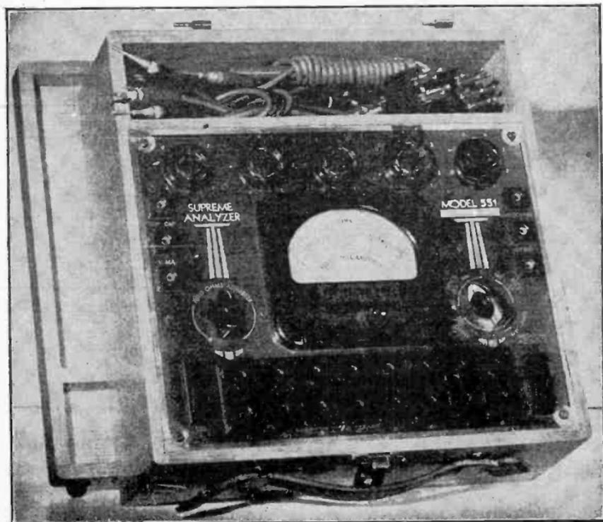
FIG. 26—Exterior view of Supreme Model 551 analyzer.
