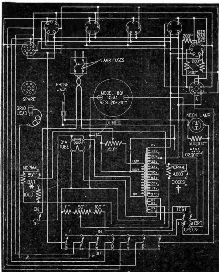
FIG. 16—Diagram of connection for Weston instruments Model 773.
