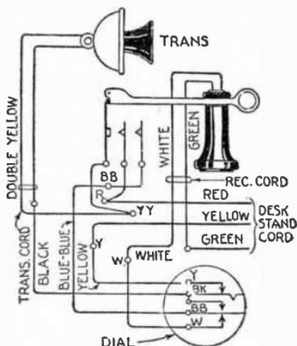
FIGS. 7.629 and 7.530.—Telephone with dial and circuit diagram.
