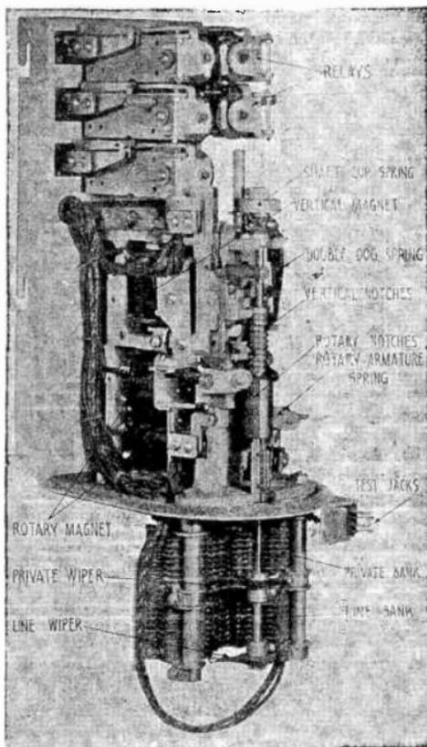
Fig. 7,675.—Step-by-step selector. It consists of a multiple bank and wipers and a mechanism similar to the connector in fig. 7,633. This is a one digit switch. The vertical motion is controlled by the dial, and the rotary motion automatically.
