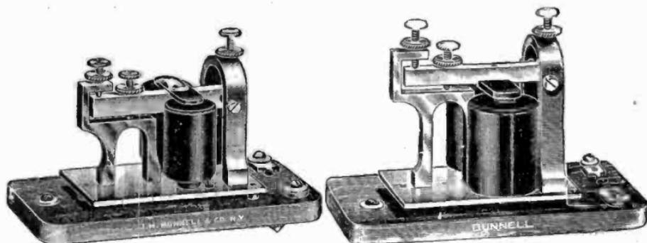
FIG. 7,697.—Bunnell aluminum lever giant sounder. Sounders wound to 4 ohms can be used on lines up to  $\frac{3}{4}$  mile in length; while 20 ohm sounders will operate on main lines up to 15 miles in length, without using a relay.
