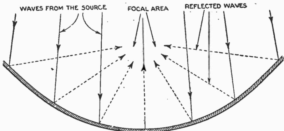
FIG. 7.846.--Reflection of waves from a curved surface. The solid lines show the direction of the original waves and the dotted lines show the direction and focusing of the reflected waves. Focusing of waves results in their reinforcement, which may cause them to build up to considerable proportion at one point.
