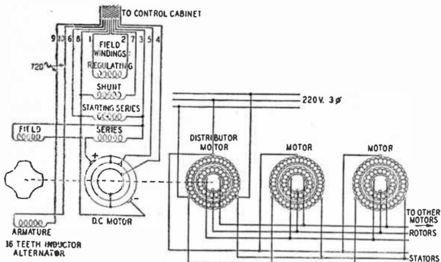
FIG. 7,900.—Diagram of motor system.
