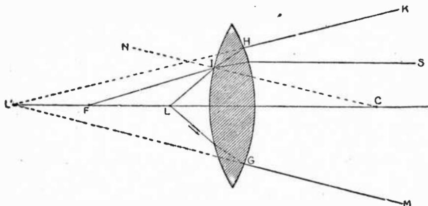
FIG. 7,769.—Virtual focus in double convex lens. In the figure, L is the position of the luminous source between the principal focus and the lens; F is the principal focus, and L', the virtual focus corresponding to the position L of the luminous source.
