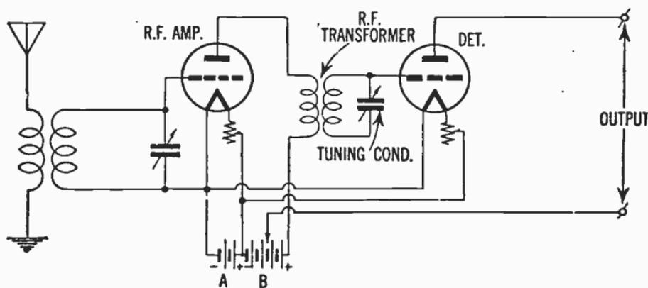
**FIG. 27**—Diagram illustrating principle of tuned radio frequency. The usual method of tuning is by means of a variable condenser in parallel with the secondary of the radio frequency transformer. A potentiometer is used to control oscillations, as the greatest amplification is obtained when the circuits are operated just at the point before self oscillation starts.
