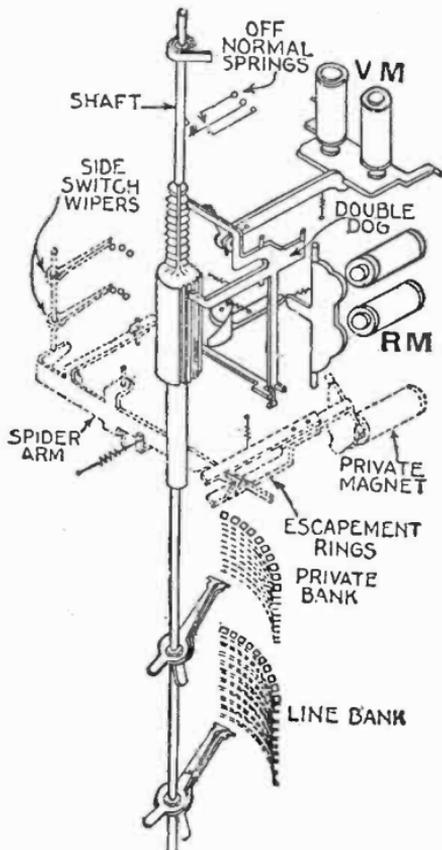
FIG. 7,360.—Step-by-step connector switch. It consists of a double bank and double wipers, or brushes, and a mechanism whereby the shaft can be lifted and rotated step-by-step. This is a two digit switch. The vertical motion is controlled by the first digit dialed and the rotary motion by the second digit.
