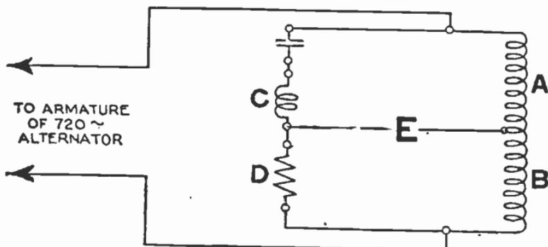
FIG. 7.9C3.—Sound picture governing circuit proper. Voltage E, shifts 180° in phase as the speed changes from any value below 1,200 r.p.m. to any value above it.
