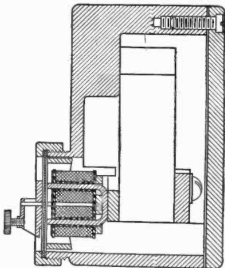
FIG. 7,874.—Reproducer for disc record.
