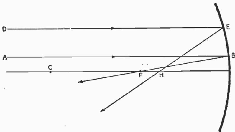
FIG. 7,777.—*Spherical aberration.* The reflected rays of concave spherical mirrors do not meet at exactly the same point. For instance, the ray AB, will be reflected to F, but DE will be reflected to H, a point closer to the mirror. This is called *spherical aberration*. It has been observed that the reflected rays only pass through a single point when the aperture of the mirror does not exceed 8 or 10 degrees.
