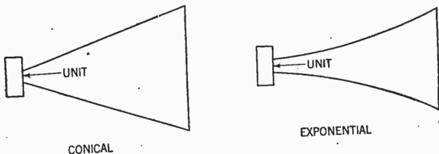
FIGS. 1 and 2—Conical and exponential horn forms.
