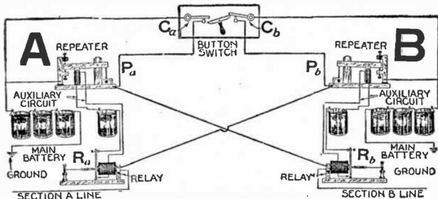
FIG. 7,713.—Diagram showing essentials of the so called button repeater, consisting of two relays, two simple repeaters, a button switch and connections as shown.
