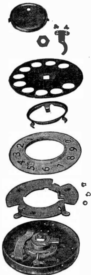
FIGS. 7,641 to 7,653.—Disassembly of dial set showing various parts; the number plates consist of a copper base coated with a vitreous white enamel. Small pins projecting from the back fit into holes in the dial frame, thereby insuring proper alignment of the number plate with regard to the finger wheel of the dial.
