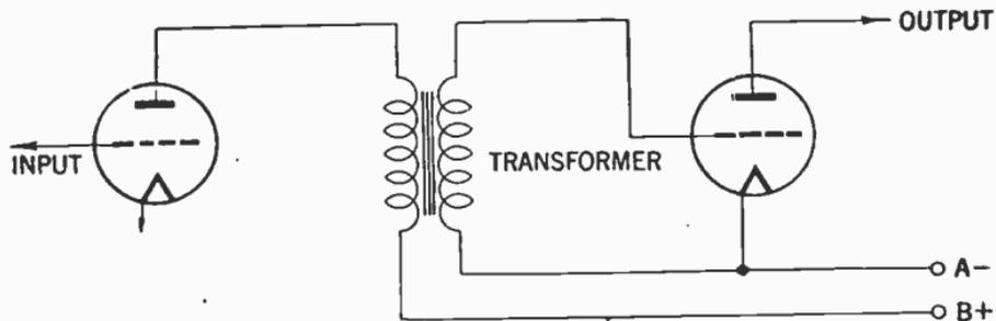
FIG. 32—Method of inter-stage connection of transformer coupled audio frequency amplifier.
