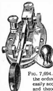
FIG. 7,694.—Bunnell double speed key. *It requires only one-half the motions of the ordinary key, and these are made by a sidewise rocking motion of the hand, easily acquired, which guarantees that operators will not be affected with cramp, and those who are so affected will soon recover their speed.*
