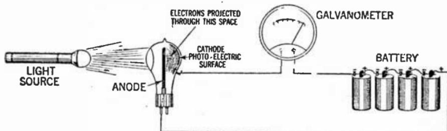
**FIG. 2—**To increase the amount of deflection (efficiency of light conversion) various methods of current amplification similar to that associated with current amplification in radio circuits is employed.
