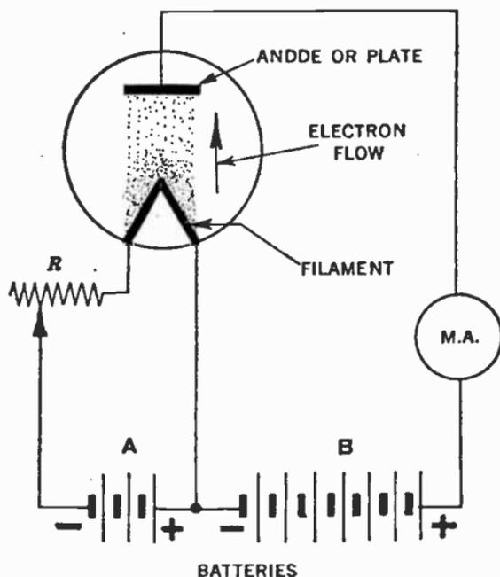
FIG. 3.—Connection diagram for a two electrode tube.
