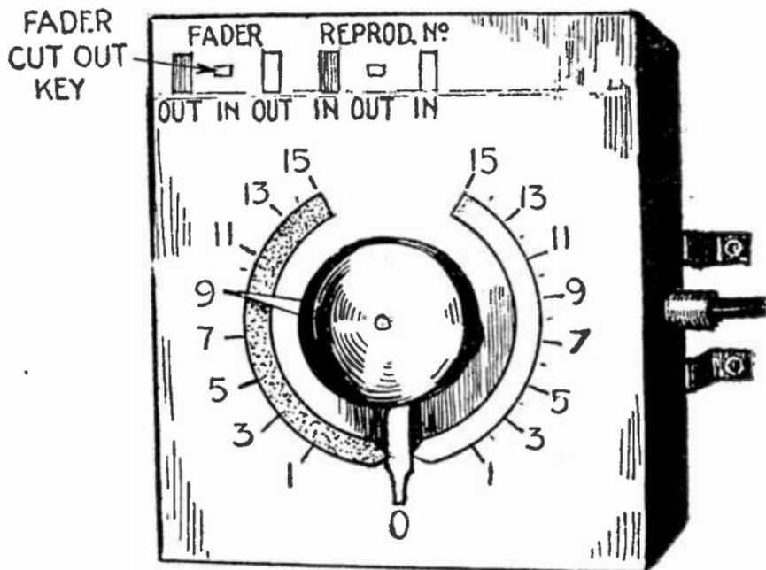
FIG. 7,915.—Western Electric fader.
