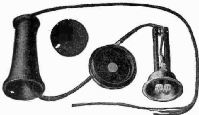
FIGS. 7.488 and 7.489.—Kellogg subscriber's receiver disassembled showing construction.
