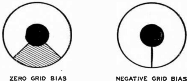
FIG. 33—Electron pattern on the 6E5 target for various grid bias.
