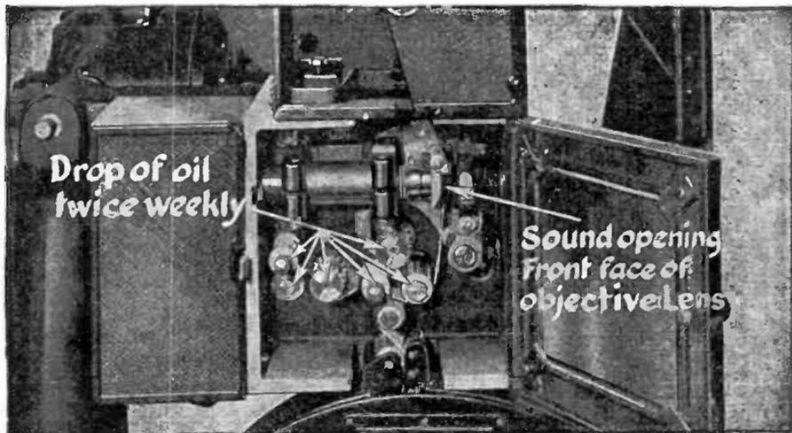
FIG. 7,917.—Paent optical chamber with oiling indications.
