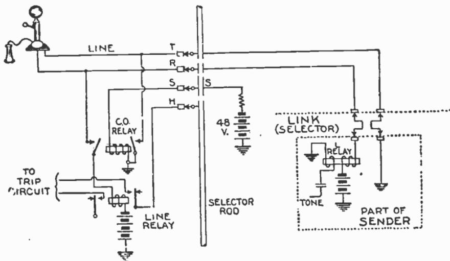
FIGS. 7,664 and 7,665.—Line finder brushes stopped at calling line terminals and sender connected. The calling telephone receives the "dial" tone.
