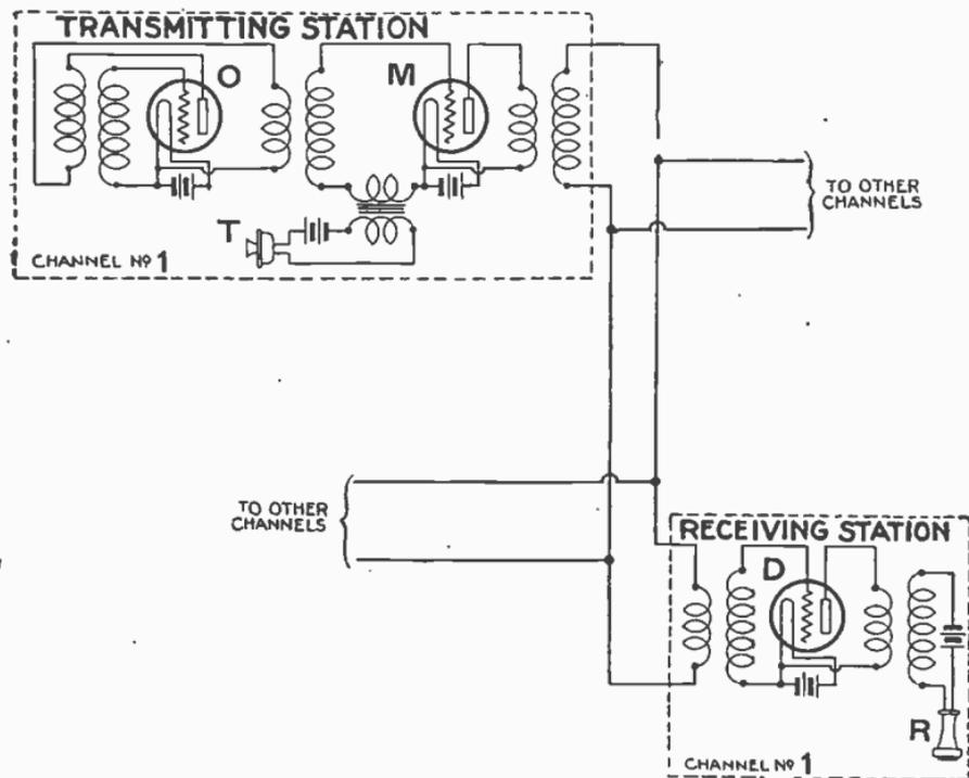
FIG. 7,576.—One channel of a carrier current telephone circuit *the transmitting station consists of: O, vacuum tube oscillator circuit, which generates the high frequency carrier current; M, vacuum tube modulator circuit, which impresses the voice currents on the carrier current; T, transmitter. The receiving station consists of: D, vacuum tube demodulator circuit, which separates the voice currents from the carrier current wave; R, receiver which reproduces the speech.*
