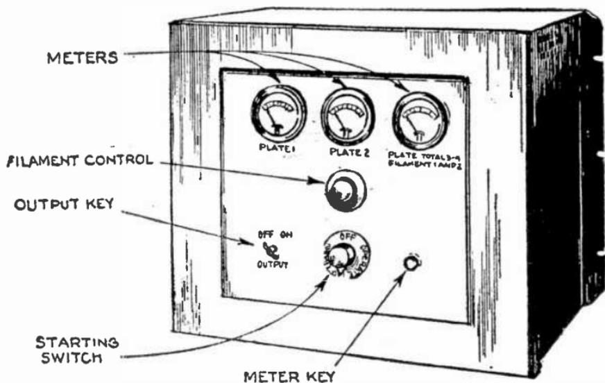
FIG. 7,916.—Western Electric type 46-B amplifier.
