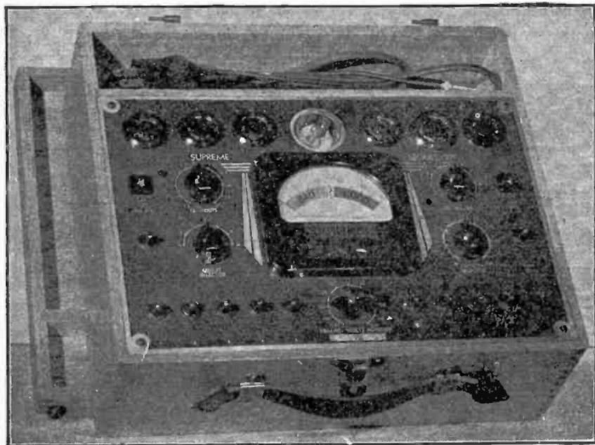
**FIG. 24**—Front view of Supreme Model 501 tube tester.
