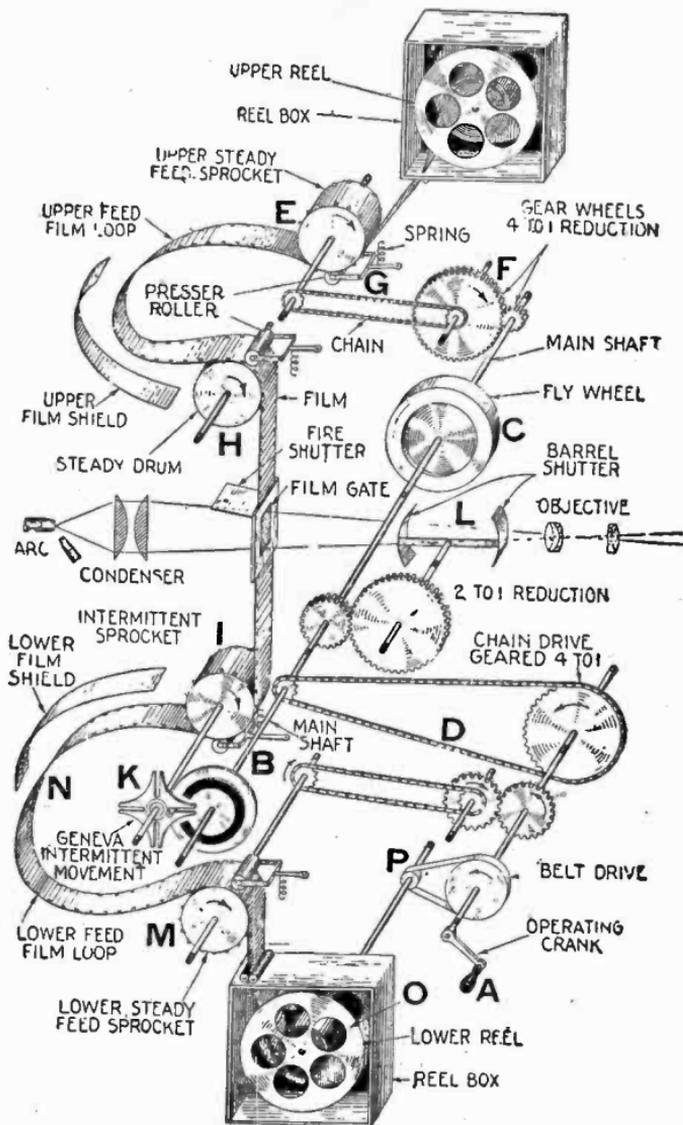
FIG. 7,700.—Elementary moving picture machine without case showing essential parts arranged to illustrate plainly the motion system.
