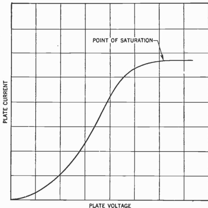
FIG. 6.—Characteristic curve of a diode.
