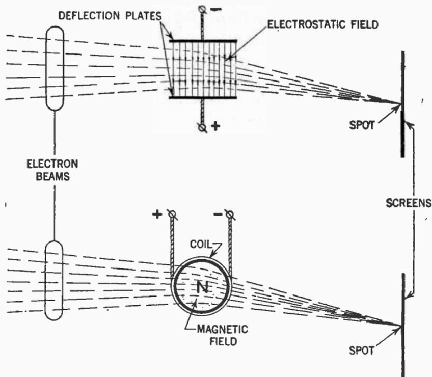
**FIGS. 13 and 14**—Indicating how an electron beam may be deflected either electrostatically or electromagnetically. When the former method is used deflection plates are placed at certain points along the tube; in the later deflection method the beam is deflected by means of a special coil or coils placed around the neck of the tube.
