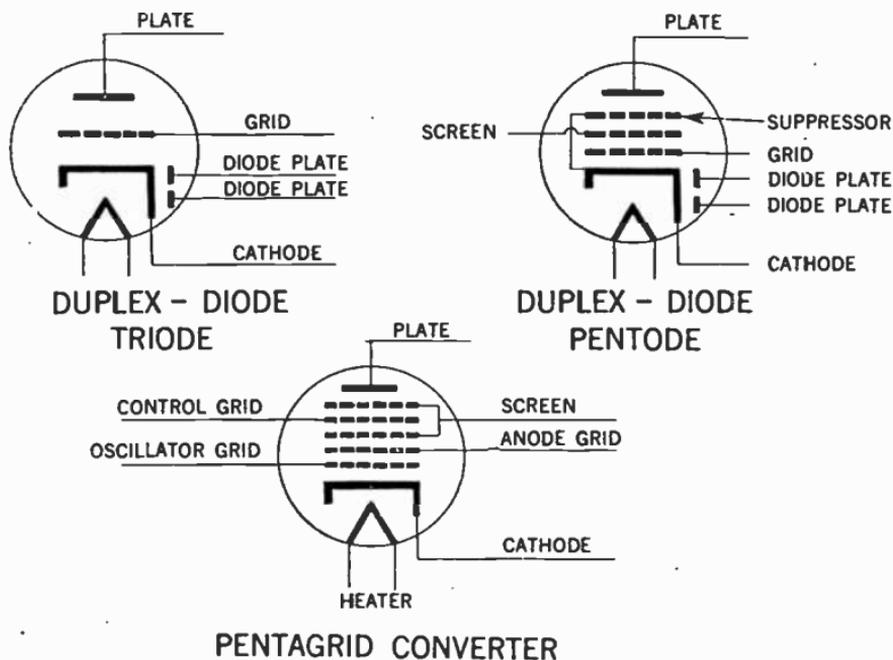
FIGS. 14 to 16.—Schematic representation of multi-purpose tubes.
