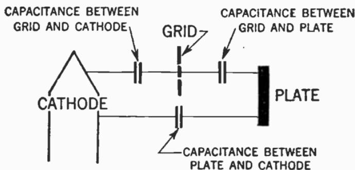
FIG. 9.—Diagram showing inter-electrode capacitances in a triode.
