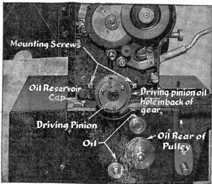
FIG. 7,919.—Patent driving pinion with oiling indications.
