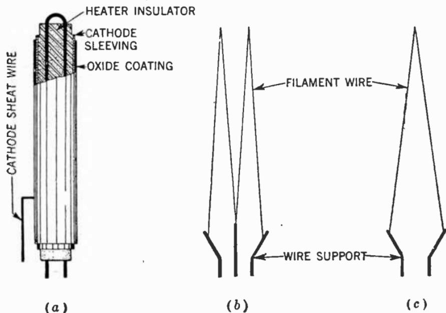
FIG. 1.—Schematic diagram of directly and indirectly heated cathodes.
