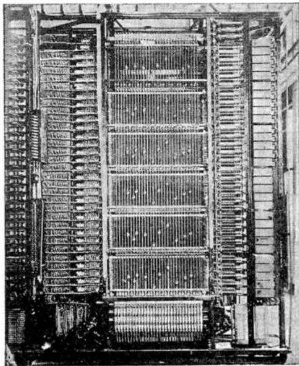
FIG. 7,654.—Panel type selector frame.
