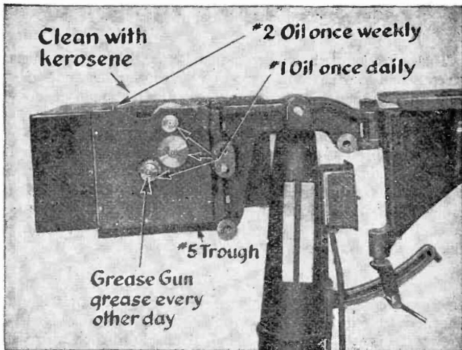
FIG. 7,913.—Pacent film head with oiling and greasing indications.
