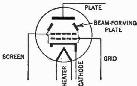
FIG. 12.—Conventional representation of beam power tube.
