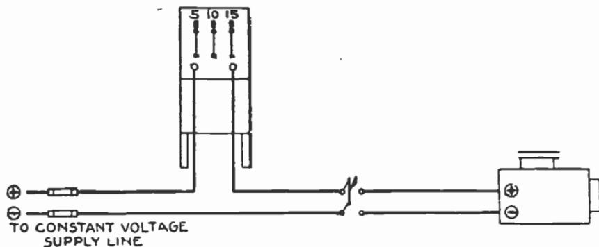
FIG. 7,923.—Hertner wiring diagram showing method of connecting type AA, and A ballast rheostats.
