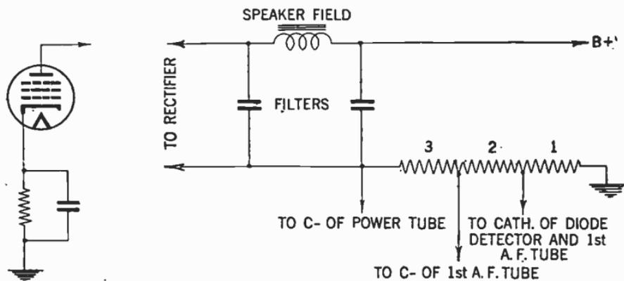
FIG. 39—Showing how grid bias may be obtained by the use of self biased bypassed resistor.
