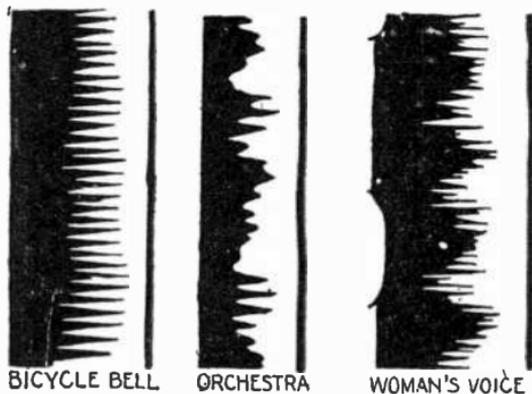
FIGS. 7,858 to 7,867.—Details of "sound track" with *variable area* method of recording. The juncture of the opaque and transparent parts of the sound track form a wavy line which is practically an exact representation of the sound pressures of the original sound waves.
