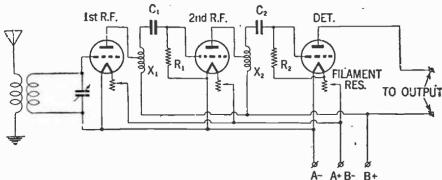
FIG. 13—Two stage impedance coupled radio frequency amplifier.
