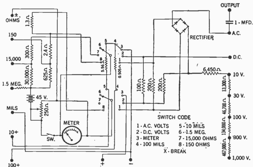
FIG. 36—Wiring diagram of Philco Model 025 radio tester.
