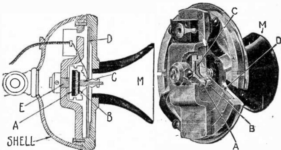
Figs. 7,513 and 7,514.—Commercial transmitter. *The parts are:* A, fixed carbon disc attached to the bridge at E; B, movable carbon disc attached to the center of the aluminum diaphragm D, at C; M, hard rubber mouth piece. The shell is for protection and for mounting the transmitter to a stand or bracket.
