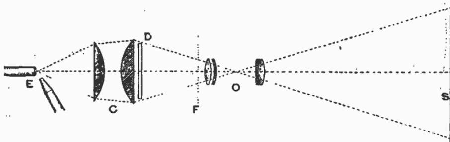
FIG. 7,783.—Diagram showing the various lenses of a motion picture machine and illustrating the principles of optical projection.
