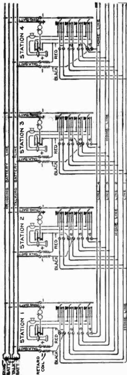
Fig. 7,603.—Wiring diagram of Graybar selective ringing, selective talking inter-phone system; *full metallic*.
