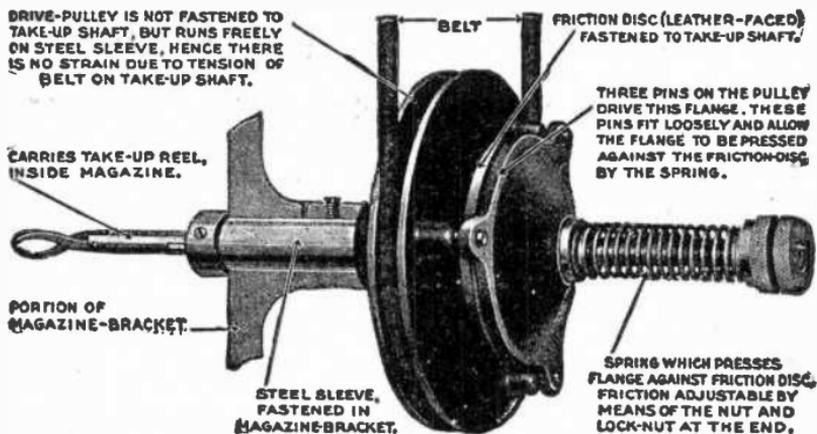
FIG. 7,805.—Simplex take-up device. *It is driven from the main driving gear, thus balancing the entire mechanism and equalizing the strain on the main driving gear. The unit is adjustable for any desired tension. Two grooved pulleys are furnished permitting the use of reels with either 2 in. or 5 in. hubs.*
