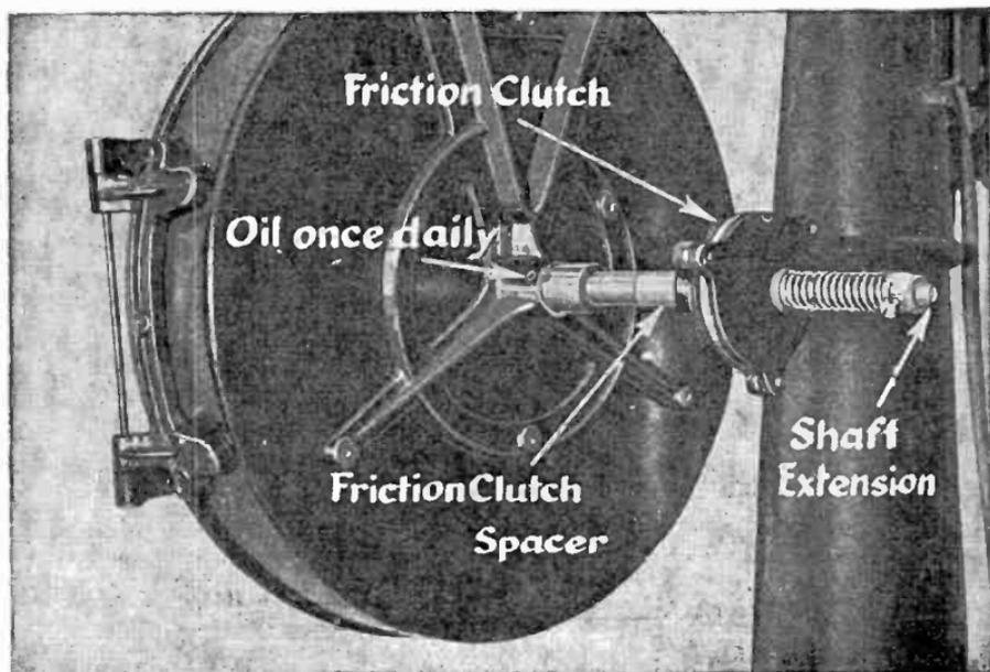
FIG. 7,914.—Patent friction clutch spacer with oiling indications.
