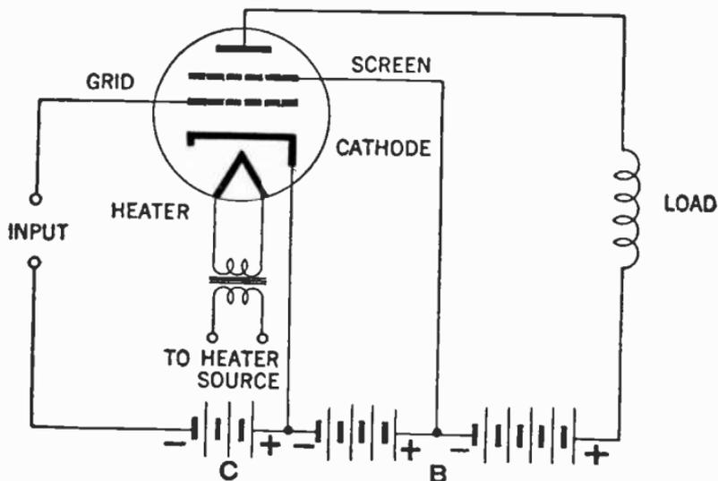
FIG. 10.—Connection of electrodes of a screen grid tube.
