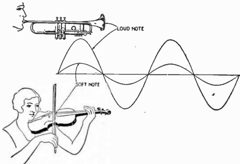
Fig. 7,847.—Properties of wave motion illustrating what causes loudness of tone.
