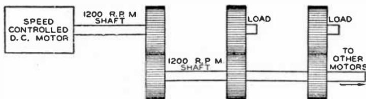
FIG. 7,901.—Mechanical analogy of motor system.
