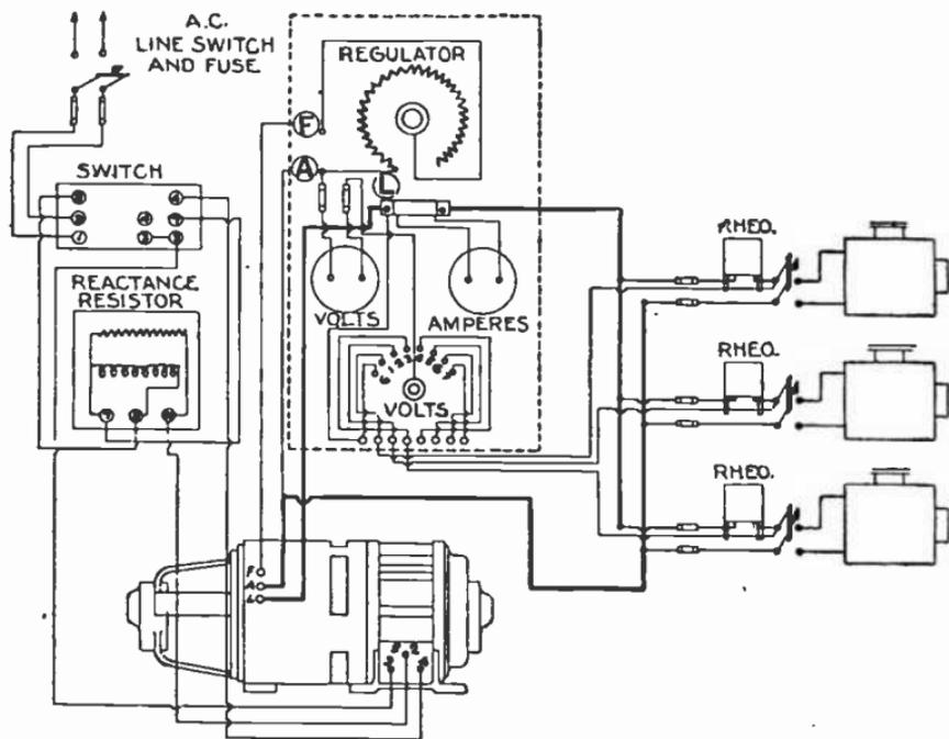
FIG. 7,955.—Wiring diagram of single phase (split phase starting) multiple arc set.
