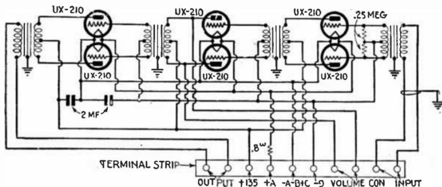
FIG. 7,953.—Wiring diagram for voltage amplifier.
