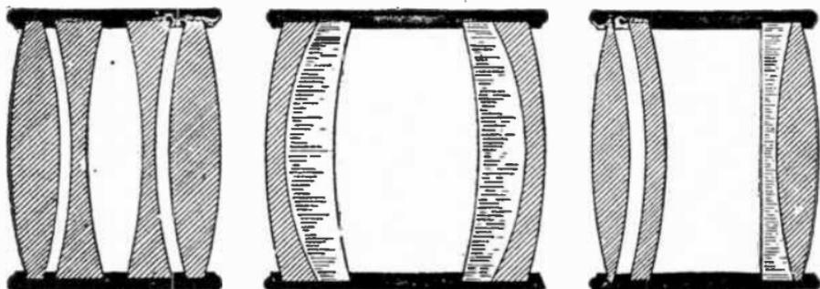
FIGS. 7,780 to 7,782.—Various achromatic lenses. FIG. 7,780 and fig 7,781 are types usually used in photography, and fig. 7,782, a combination used in motion picture and stereopticon projection.
