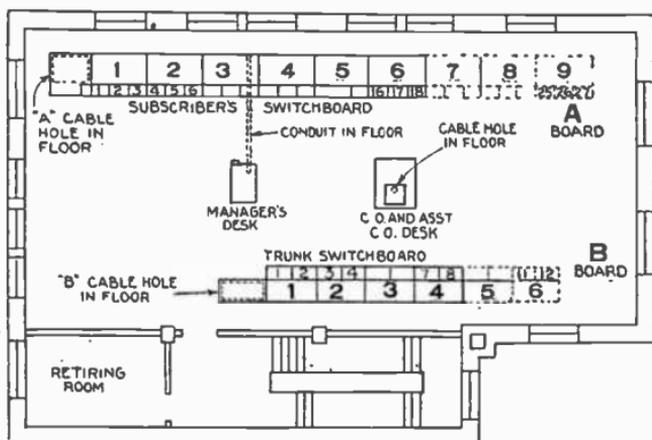
FIG. 7,529.—Typical layout of a Central Office operating room showing the A and B boards.
