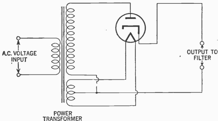
FIG. 4—Illustrates connection and rectifier tube to obtain half-wave rectification.
