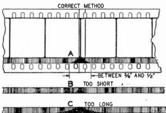
FIGS. 7,897 to 7,899.—Method of splicing film with film track.
