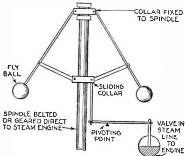
FIG. 7.9C2.—Familiar fly ball steam engine governor showing how sensitivity may be changed by moving the pivoting point to the left or right.
