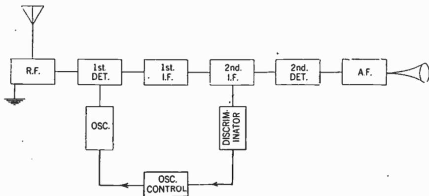
FIG. 1—Conventional block diagram of an automatic radio frequency control circuit.
