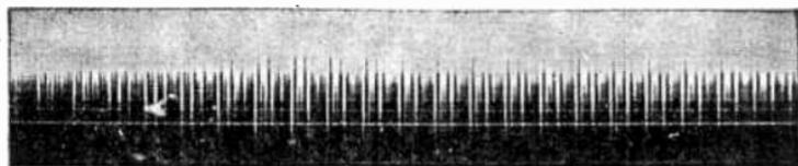
FIGS. 7,863 and 7,864.—Comparison of sound tracks showing difference between the variable density, fig. 7,863, and fig. 7,864, variable area methods of recording.
