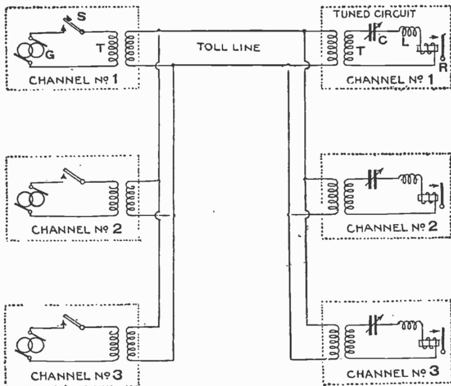
FIG. 7,575.—Simplified Multiplex circuit, consisting of three channels, each equipped alike and arranged to operate simultaneously over the same toll line. Each sending station is equipped with a high frequency generator G, a sending key S and a repeating coil T. Each receiving station is equipped with a repeating coil T, a variable condenser C, an inductance L, and a sounder relay R.
