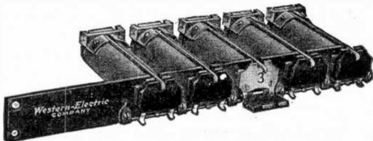
FIG. 7,528.—Mounted trunk drops. Tubular trunk drops are mounted on a metal strip each being held by two small screws underneath the drop shutter. The tubular casing of each drop is soft iron inside of which is the drop winding; the ends of the coil wires terminating at lugs which protrude from the casing and are insulated therefrom. The drop shutters are then screwed fast to the metal strip and adjusted so that they may fall easily when the armature is held up by the magnet.
