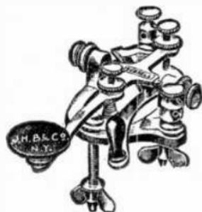
FIG. 7,692.—Fry open circuit key. *It has a circuit closer which must be worked like an ordinary key. With circuit closer in closed position, the battery cannot be put to line or short circuited by pressing down on key lever, hence leaving a book or other heavy object on key does not waste the battery, but the relay is always in circuit ready to receive signals.*
