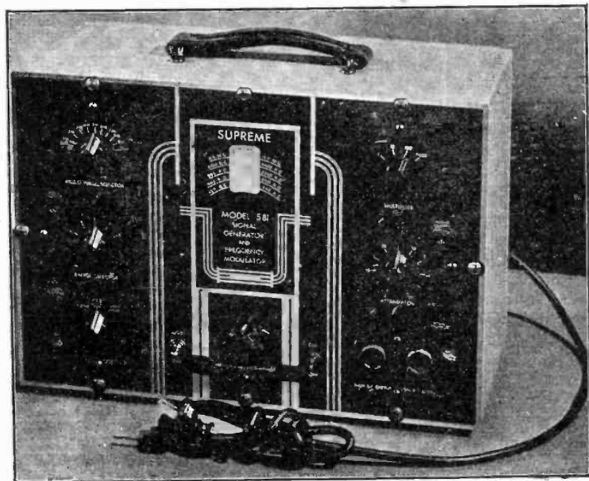
FIG. 28—Panel view of Supreme Model 581 signal generator.
