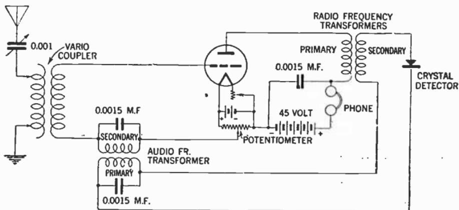
FIG. 28—Diagram showing typical reflex circuit.
