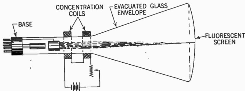
**FIG. 12—Cathode ray tube with external concentration coils. The concentration coils generally consists of one or more solenoid of wire placed as shown for focusing the ray. For a practical utilization of this form of ray concentration, however, it is necessary that the position of the coils be definitely fixed and the current through them suitably controlled.**
