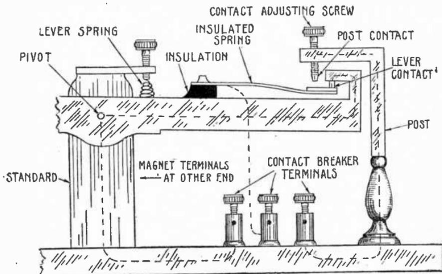
FIG. 7,727.—Detail of contact breaker end of a transmitter showing the three contacts, method of mounting the spring contact, and the circuits from the contacts to terminals. The duration of contact, or portion of the stroke of lever during which the circuit through the post contact and spring contact remains closed is regulated by the contact adjusting screw. This adjustment and other construction details are clearly shown in the illustration.
