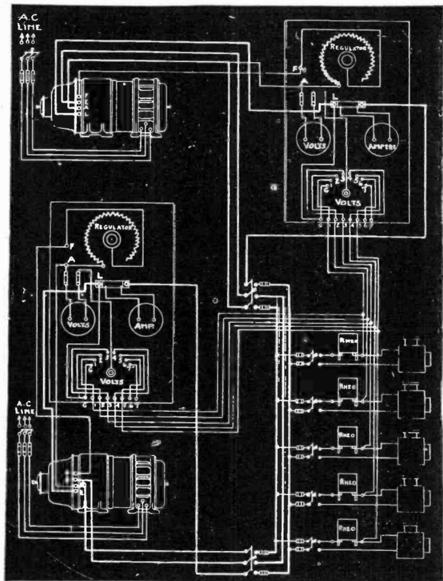
FIG. 7,957.—Wiring diagram showing installation of two multiple arc units in parallel and control panel.
