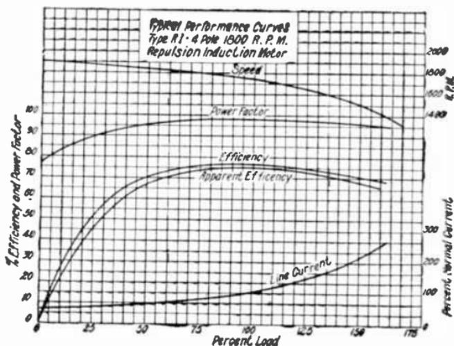
FIG. 2,124.—Performance curves of General Electric single phase repulsion induction motor.
