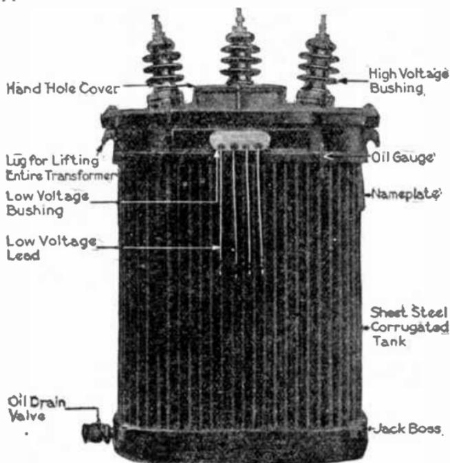
FIG. 2,365.—General Electric small power high voltage three phase transformer in corrugated tank. Three phase tanks are identical in construction with corresponding type single phase tanks, except for the difference in shape necessary to accommodate differently shaped cores and coils. The smaller three phase transformers are provided with smooth cast iron tanks, while the moderate and large sizes have tanks with corrugated sheet steel sides cast welded into cast iron bases and top rims.
