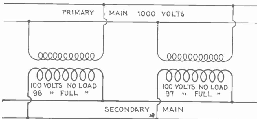
FIG. 2,431.—Diagram showing unlike single phase transformers in parallel.
