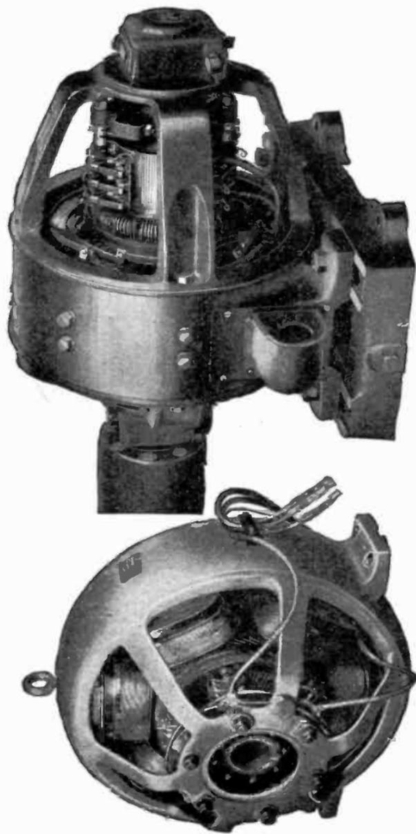
FIGS. 2,215 and 2,216.—General Electric exciters. Fig. 2,215, direct connected exciter; fig. 2,216, belted exciter.
