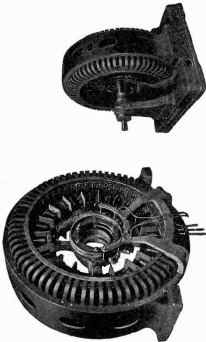
FIG. 2,167.—Westinghouse direct connected engine driven alternator. Capacities 50 to 3,000 *kva*. This type alternator is applicable to all prime movers, being suitable for direct connection to steam, gas or oil engines, or slow speed horizontal water wheels.
