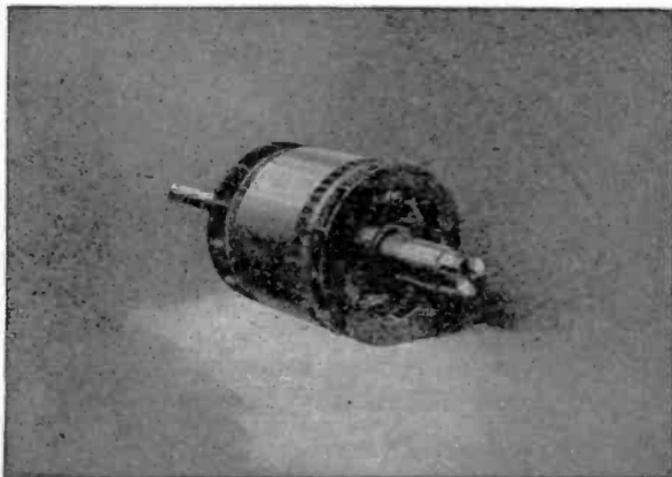
FIG. 2,553.—*Reliance induction motor construction 17.* Completed field with shaft. Laminations are mounted on cast iron spider. Shafts can be easily removed.
