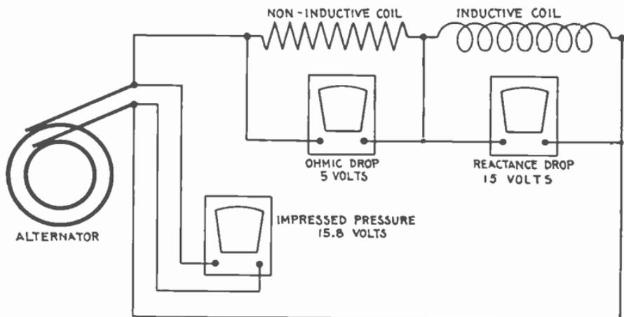
FIG. 2,084.—Diagram of circuit containing 5 volts ohmic drop, and 15 volts reactance drop.
