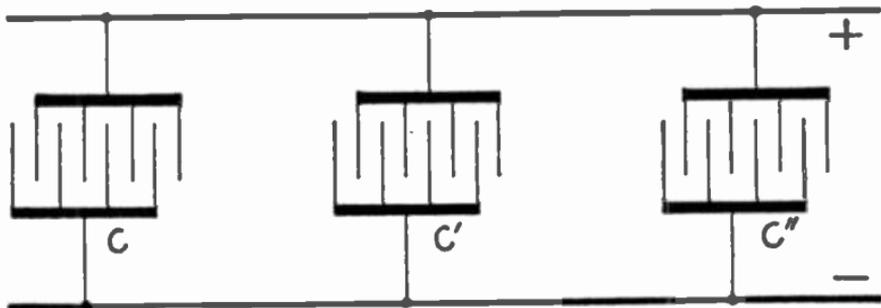
FIG. 2,032.—Parallel connection of condensers. Like terminals are joined together. The capacity of such arrangement is equal to the sum of the respective capacities, that is  $C = c + c' + c''$ .
