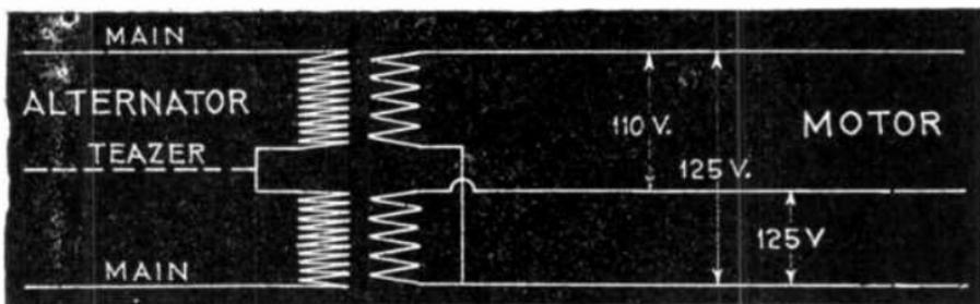
FIG. 2,190.—Monocyclic system diagram showing transformer connections.
