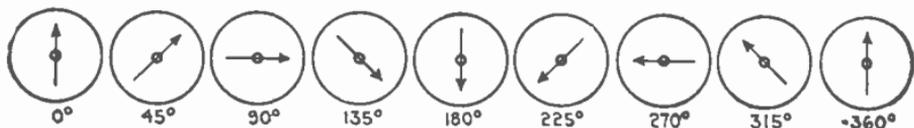
FIGS. 2,567 to 2,576.—Diagram showing resultant poles due to two phase current.
