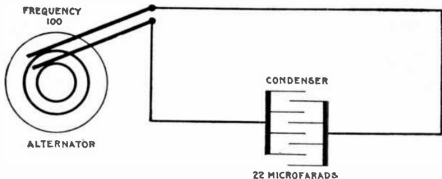
FIG. 2,035.—Diagram showing alternating circuit containing capacity. Formula for calculating the ohmic value of capacity or "capacity reactance" is  $X_c = 1 / 2 \pi f C$ , in which  $X_c$  = capacity reactance;  $\pi = 3.1416$ ;  $f$  = frequency;  $C$  = capacity in farads (not microfarads). 22 microfarads =  $22 + 1,000,000 = .000022$  farad. Substituting,  $X_c = 1 / (2 \times 3.1416 \times 100 \times .000022) = 72.4$  ohms.
