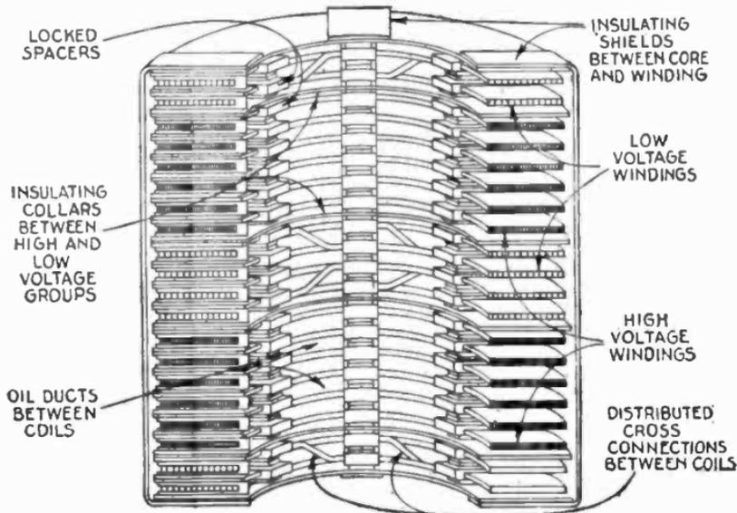
FIGS. 2,340.—Details of coil construction of General Electric type H, form KDD, transformer.
