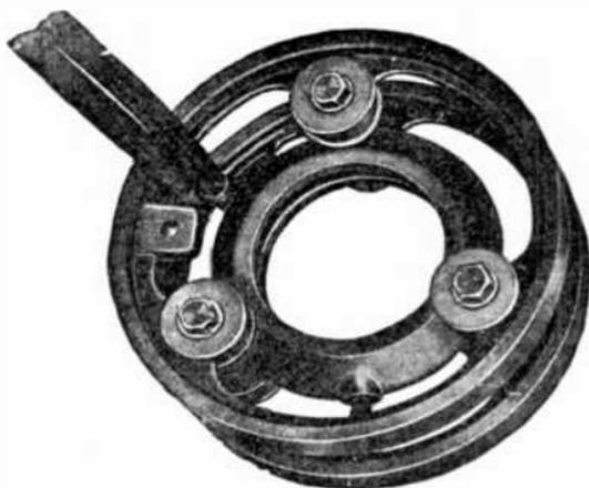
FIG. 2,270.—General Electric slip rings; view showing construction and attachment of cable leads to field winding. They are so designed that all surfaces of the rings have easy access to the air, in order to obtain good ventilation.
