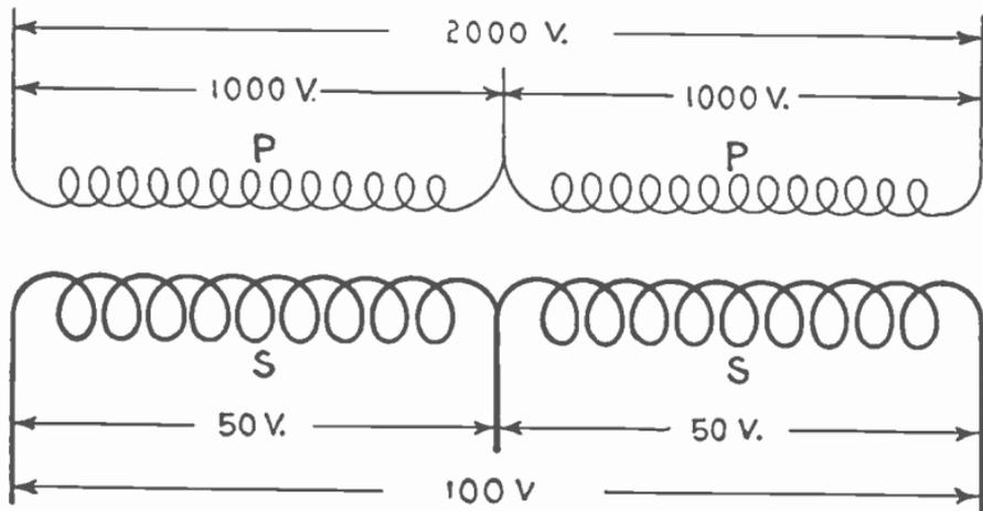
FIG. 2,424.—Diagram of single phase transformer having primary and secondary windings in two sections, showing voltages per section with series connections.
