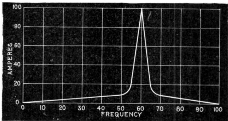
FIG. 2,068.—Curve showing variation of current by increasing the frequency in a circuit having inductance and capacity. The curve serves to illustrate the “critical frequency” or frequency producing the maximum current. The curve is obtained by plotting current values corresponding to different frequencies, the pressure being kept constant.
