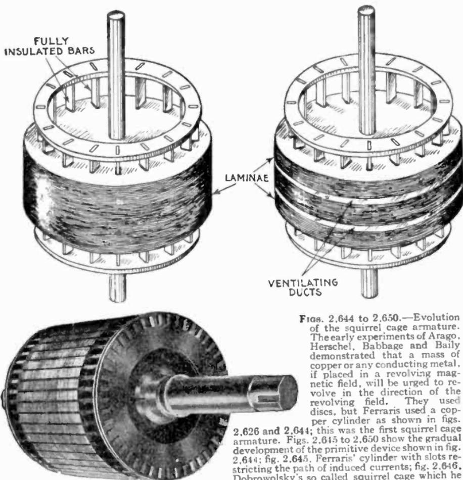
FIGS. 2.644 TO 2.650.—Evolution of the squirrel cage armature. The early experiments of Arago, Herschel, Babbage and Baily demonstrated that a mass of copper or any conducting metal, if placed in a revolving magnetic field, will be urged to revolve in the direction of the revolving field. They used discs, but Ferraris used a copper cylinder as shown in figs.
