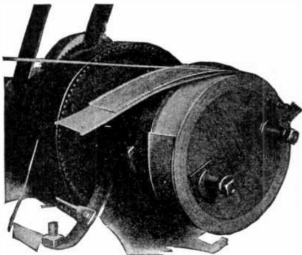
FIG. 2,310.—Wagner transformer construction 4. Circular type coil for high voltage units. Method of applying crimped paper insulation. After a layer of wire has been placed on the coil two strips of crimped insulation back to back are placed on the coil and the winding operations continued to bind the insulation to the coil.
