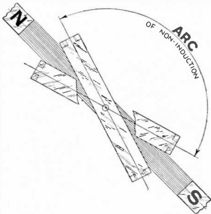
FIG. 2,654.—*Squirrel cage principles 3.* Top view of elementary four bar squirrel cage and rotating field showing *extensive zones or periods in which there is no induction and consequently no torque produced.*
