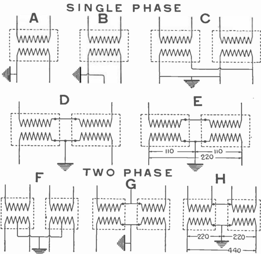
**Figs. 2,452 to 2,459.**—Ground connections to secondaries of *single phase* transformers. A, two wire; B, three wire; C, two separate 110 volt transformers in parallel, the secondary ground is attached to either wire; D, two windings, two wire; E, two windings, three wire; F, four wire; G, three wire; H, three wire with four wire primary.
