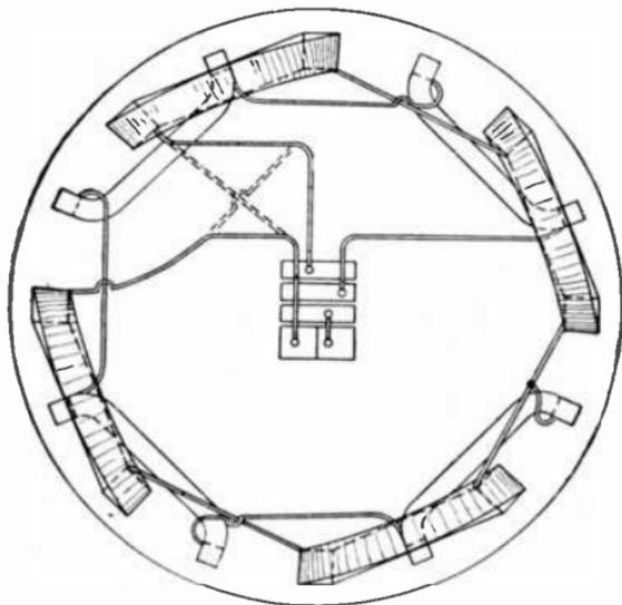
FIG. 2,193.—Diagram showing connections of General Electric monocyclic alternator. The solid lines show standard connections for counter-clockwise rotation; the broken lines show connection changed for clockwise rotation.
