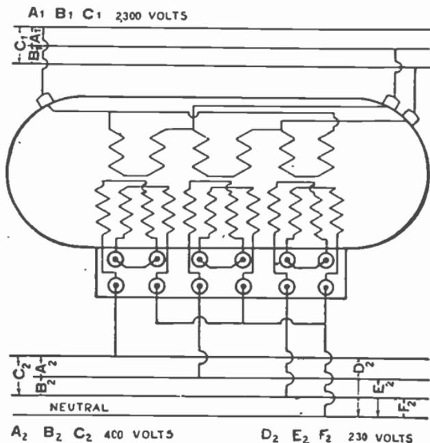
FIG. 2,441.—Pittsburgh connection diagram for three phase 3-wire closed delta primary to three phase 4-wire star secondary.
