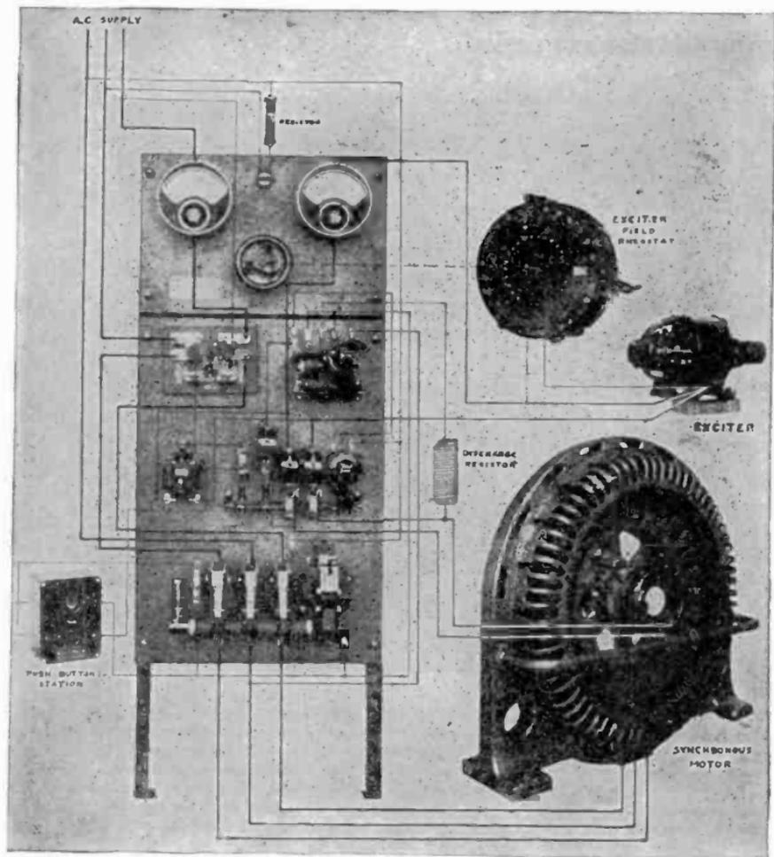
FIG. 2,519.—Pictured representation of General Electric *across the line* starter showing its connections and relations to a synchronous motor and exciter.
