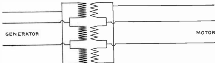
FIG. 2,464.—Three phase motor transformer connections; the so-called delta connected transformers.
