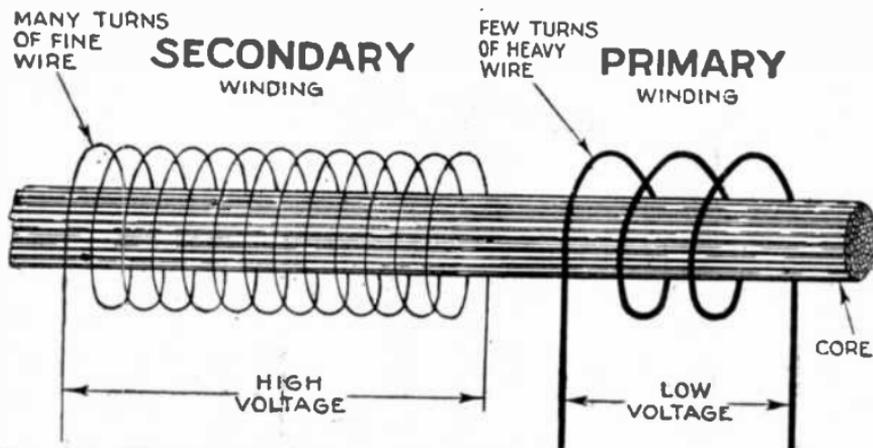
FIG. 1,919.—Elementary transformer consisting of: 1, core; 2, primary winding; 3, secondary winding.
