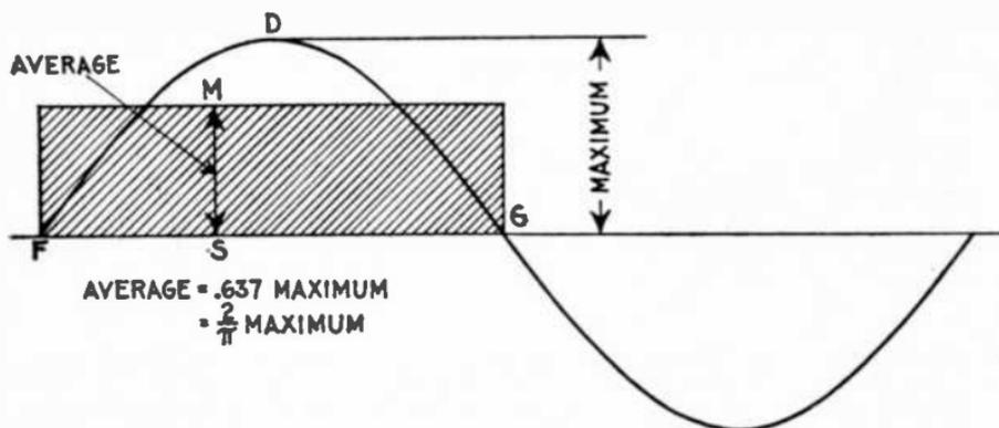
FIG. 1,955.—Maximum and average values of the sine curve. The average value of the sine curve is represented by an ordinate MS, of such length that when multiplied by the base line FG, will give a rectangle MFSG, whose area is equal to that included between the curve and base line FDGS.
