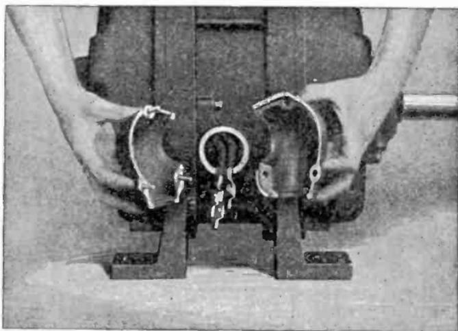
FIG. 2,554.—*Reliance induction motor construction 18.* Removing or replacing outlet for conduit connections. Three accessible screws hold the two halves together.
