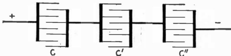
FIG. 2,033.—Series or cascade connection of condensers. Unlike terminals are joined together as shown. The total capacity of such connection is equal to the reciprocal of the sum of the reciprocals of the several capacities, that is,  $C = 1 + \left( \frac{1}{c} + \frac{1}{c'} + \frac{1}{c''} \right)$ .
