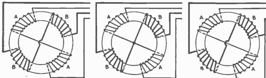
FIGS. 1,982 to 1,984.—Various two phase armature connections. Fig. 1,982, two separate circuit four collector ring arrangement; fig. 1,983, common middle connection, four collector rings; fig. 1,984, circuit connected in armature for three collector rings. In the figures the black winding represents phase A, and the light winding, phase B.
