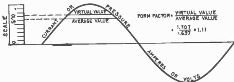
FIG. 1,959.—Current or pressure curve illustrating *form factor*. It is simply the *virtual value* divided by the *average value*. For a sine wave the virtual value is  $\frac{1}{\sqrt{2}}$  times the maximum, and
