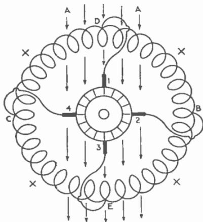
FIG. 2,256.—Diagram of connections of self-exciting image current alternator.
