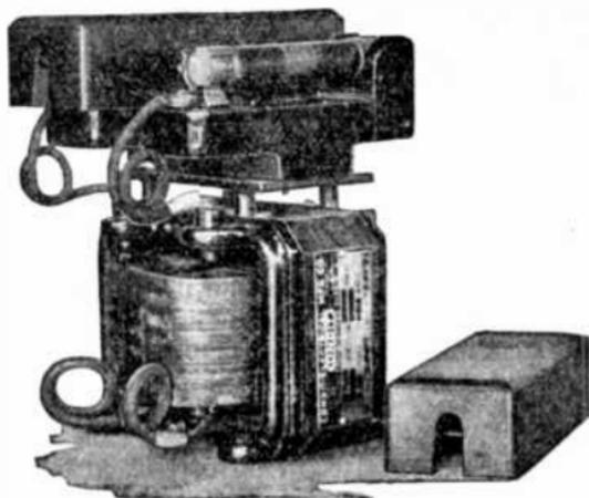
FIG. 2,420.—Condit pressure (potential) transformer. Maximum volts, dry insulated 4,400. Maximum volts, oil insulated 13,200, 25 or 60 cycles, for use in connection with under-voltage trip attachments and *a.c.* instruments, also suitable for use in connection with industrial or switchboard work.
