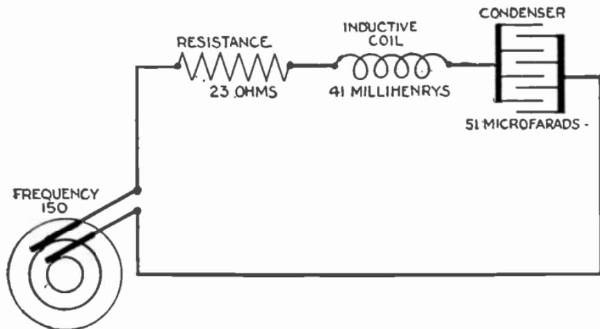
FIG. 2,107.—Diagram of circuit containing 23 ohms resistance, 41 millihenrys inductance, and 51 microfarads capacity, with current supplied at a frequency of 150.
