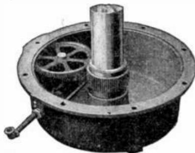
FIG. 2,244.—Westinghouse vertical water wheel alternator oil pan and pump. A positive type of pump geared to the alternator shaft provides continuous lubrication for the two guide bearings and the thrust bearing.
