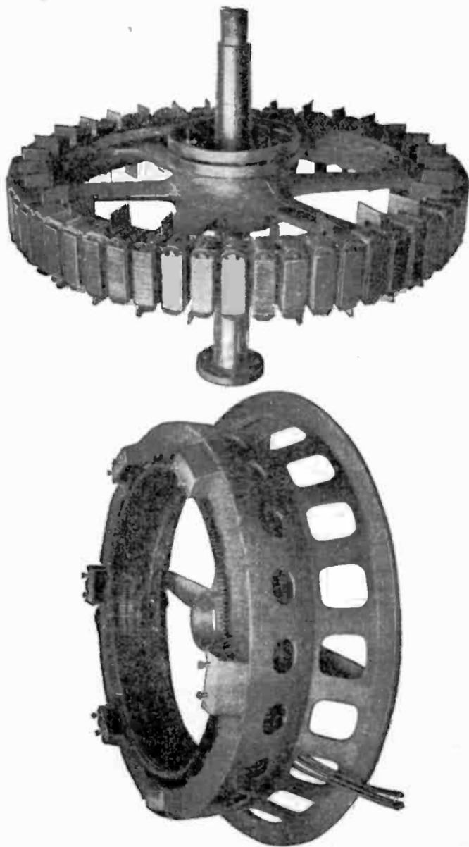
FIG. 2,238.—Westinghouse vertical water wheel alternator armature with armature winding. The frame is of cast iron in which the armature core, built up of annealed and jappanned sheet steel punchings, is held by dovetail slots. The open type frame and vent ducts in the armature core assure ample ventilation. The armature winding consists of form wound interchangeable coils, insulated with mica over the imbedded portion and has treated cloth tape on the end turns.
