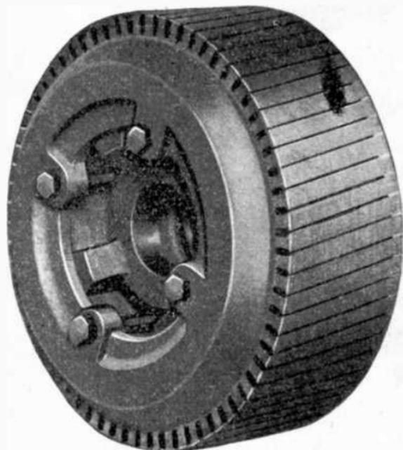
FIG. 2,671. — Fairbanks-Morse squirrel cage armature core construction. The cores are made up of laminations clamped between heads. In the larger sizes these cores are mounted on spiders giving ventilation through the core.
