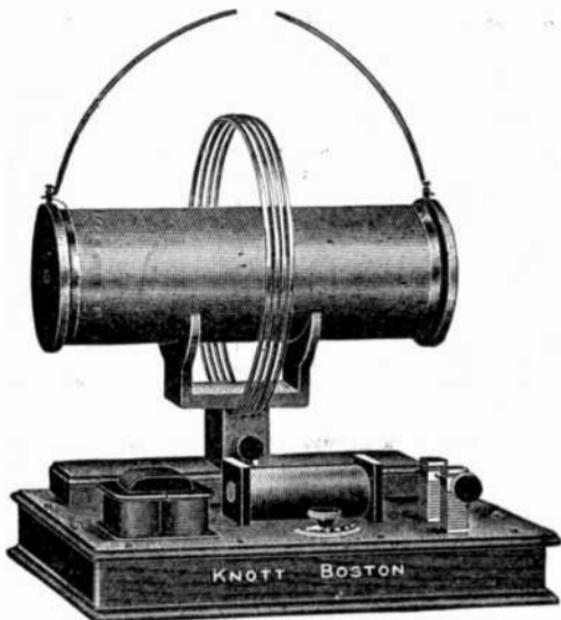
**FIG. 1,944.**—Knott frequency inductive apparatus. *It consists of an open type of resonator with closed core type of transformer and silver spark gap. Designed for a comprehensive study of the high frequency field, including wireless telegraph waves and kindred subjects. Excites all types of vacuum tubes and will produce X-Rays. Connected on a 110-volt alternating current, will furnish a discharge of any desired value up to its full capacity—about 12 inches.*
