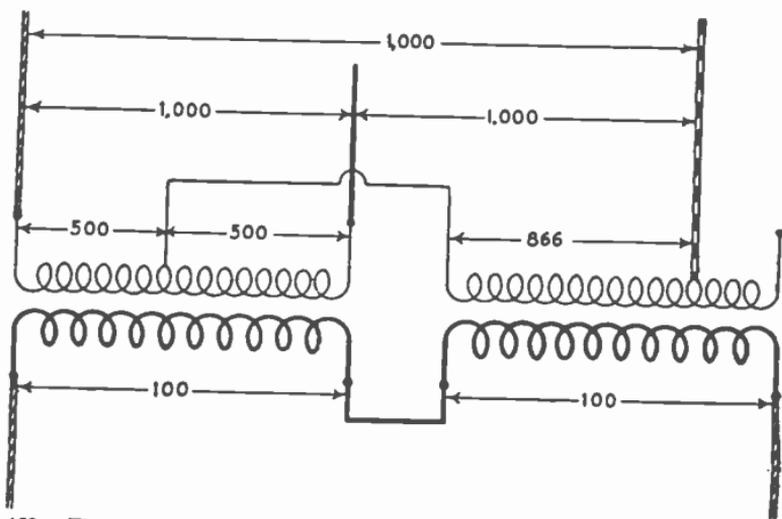
FIG. 2,468.—Three phase to one phase transformation with two transformers. The diagram shows the necessary connections and the relative pressures obtained.
