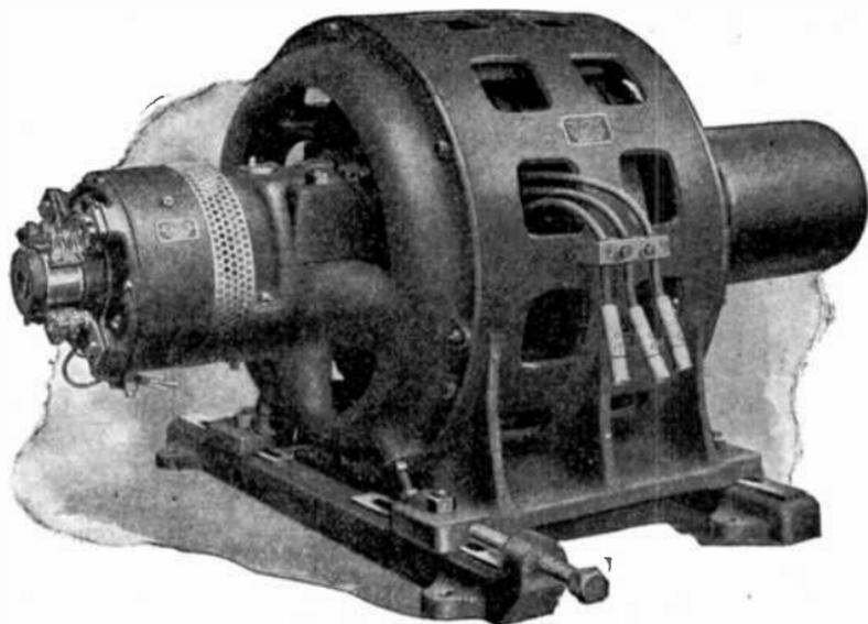
FIG. 2,214.—Allis Chalmers 225 kva; 900 r.p.m. belted alternator with direct connected exciter
