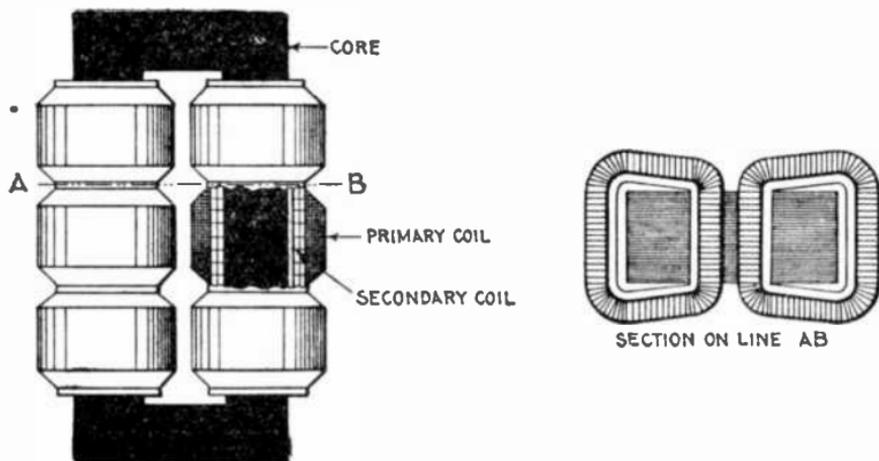
FIGS. 2,316 and 2,317.—Core type transformer with concentric winding. *It consists of a central core of laminated iron, around which the coils are wound. A usual form of core type transformer consists of a rectangular core, around the two long limbs of which the primary and secondary coils are wound, the low tension coil being placed next the core.*
