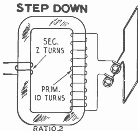
FIG. 2,315.—Diagram of elementary step down transformer. As shown the primary winding has 10 turns and the secondary 2, giving a ratio of voltage transformation of  $2 \div 10 = .2$ . The current in the secondary being 5 times greater than in the primary will require a proportionately heavier wire.
