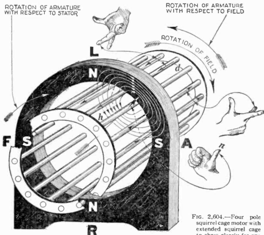
FIG. 2,604.—Four pole squirrel cage motor with extended squirrel cage to show clearly for one
