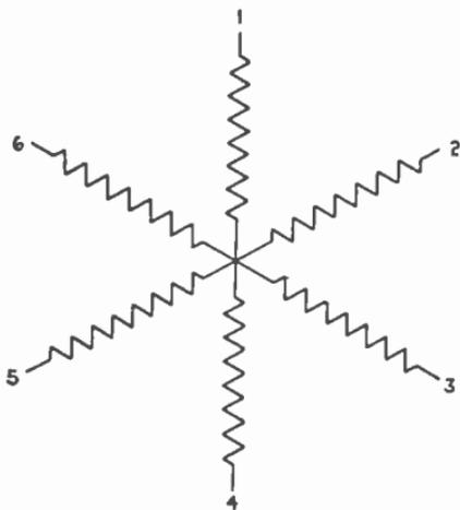
FIG. 2,156.—Diagram of six phase winding with star grouping, being equivalent to a three phase winding in which the three phases are disconnected from each other and their middle points united at a common junction.
