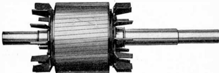
FIG. 2,696.—Louis Allis squirrel cage armature with skew slots and ventilation fans.
