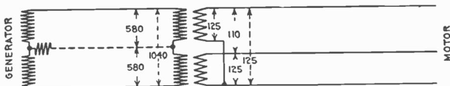
FIG. 2,467.—Diagram of transformer connections for motors on the monocyclic system.
