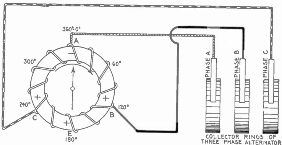
FIG. 2,601.—Production of a rotating magnetic field by three phase current. A ring, wound as shown is tapped at points A, B, and C, 120° apart, and connected with leads to a three phase alternator. As described on page 1,804, a rotating magnetic field is produced in a manner similar to the two phase method.
