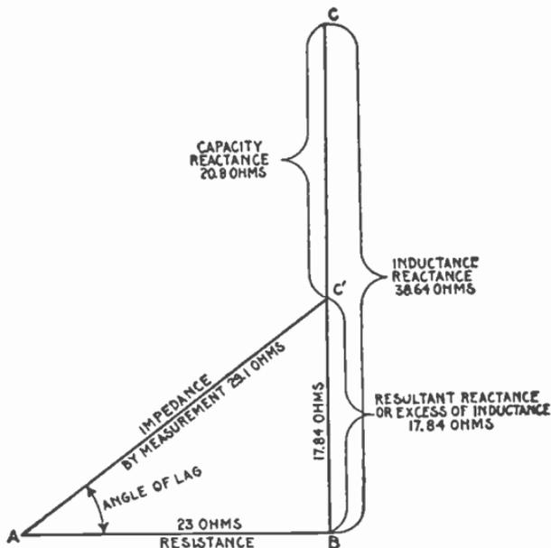
FIG. 2,108.—Impedance diagram for the circuit shown in fig. 2,107. Note that the resultant reactance being due to excess of inductance, the impedance line  $AC'$ , falls above the horizontal line AB. This indicates that the current lags behind the pressure.
