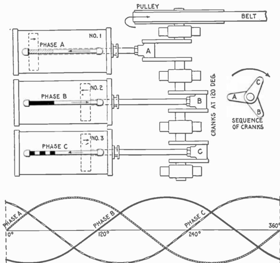
FIGS. 1,988 to 1,990.—Hydraulic analogy illustrating three phase alternating current. Three cylinders are here shown with pistons connected through Scotch yokes to cranks placed 120° apart. The same action takes place in each cylinder as in the preceding cases, the only difference being the additional cylinder, and difference in phase relation.
