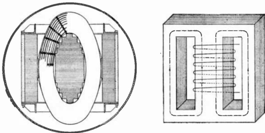
FIGS. 2,324 and 2,325.—Sectional view of Pittsburgh single phase transformer, and magnet circuit.
