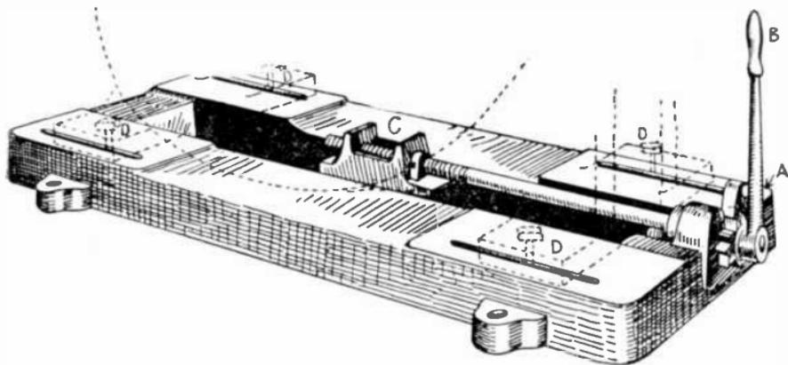
FIG. 2,161.—Sub-base and ratchet device for moving alternator to tighten belt. A ratchet A, operated by lever B, works the block C, by screw connection, causing it to move the block. The latter, engaging with the frame, causes it to move, thus providing adjustment for belt. After tightening belt, the bolts D, which pass through the slots in the sub-base, are tightened, thus securing the machine firmly in position.
