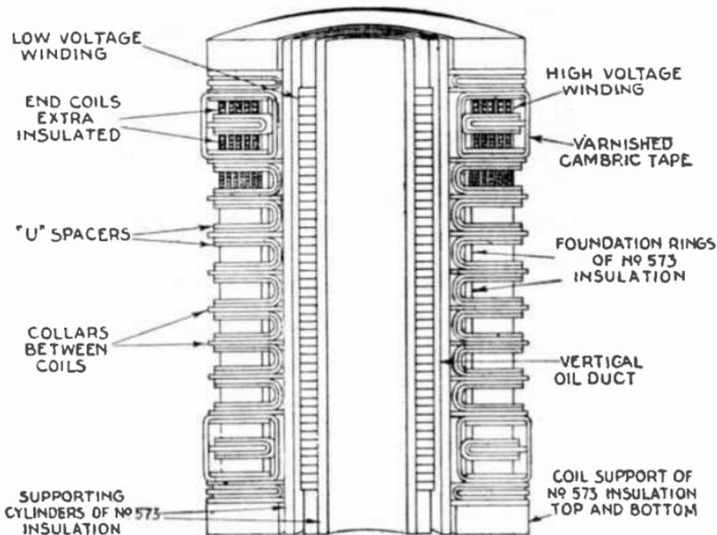
FIG. 2,341.—Details of coil construction of General Electric type H, form KD, transformer.
