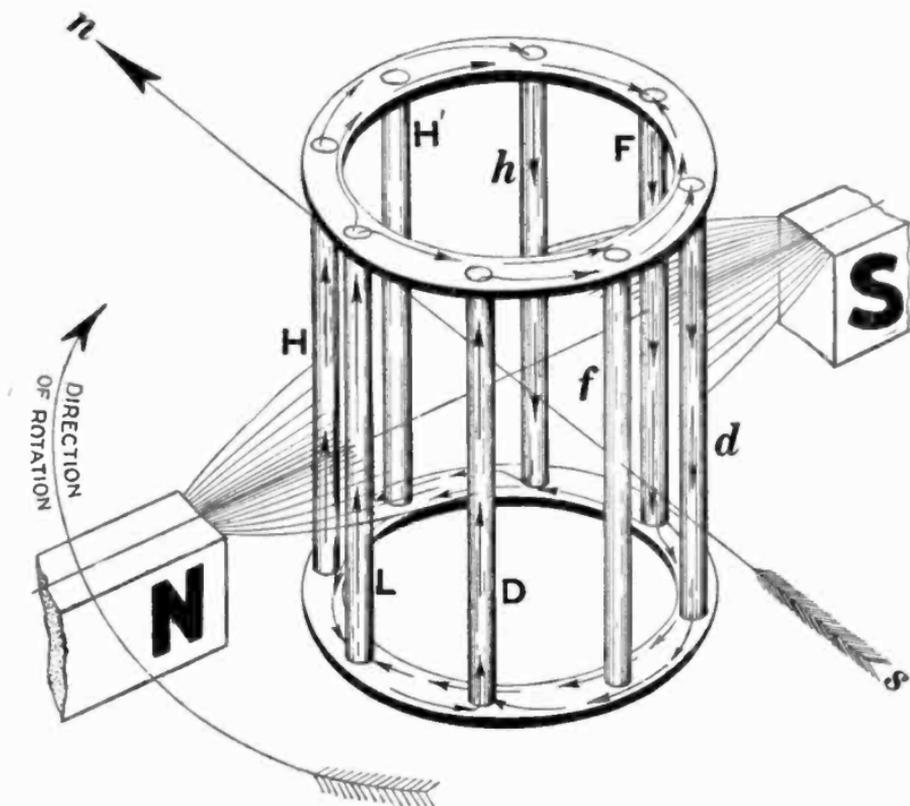
FIG. 2,656.—Squirrel cage principles. 3. Elementary eight bar squirrel cage and rotating field showing that an increase in the number of bars will cause the torque to become nearer constant and stronger.
