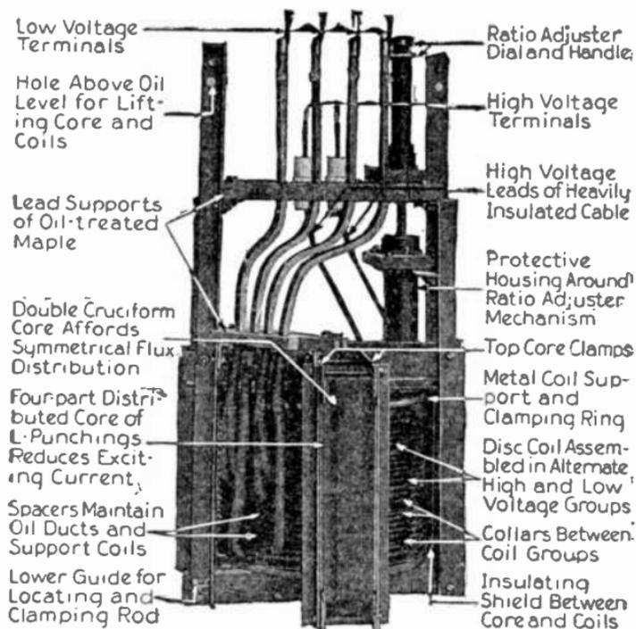
FIG. 2,338.—General Electric core and coils of a 2,300 volt type H, form KDD, interleaved disc coil distribution transformer.
