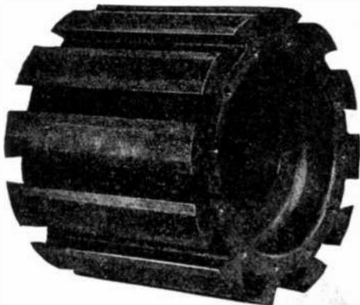
FIG. 2,268.—Wagner cast steel hub with dovetail grooves for attaching the revolving field magnets. Such construction is generally used on machines of small and medium size.
