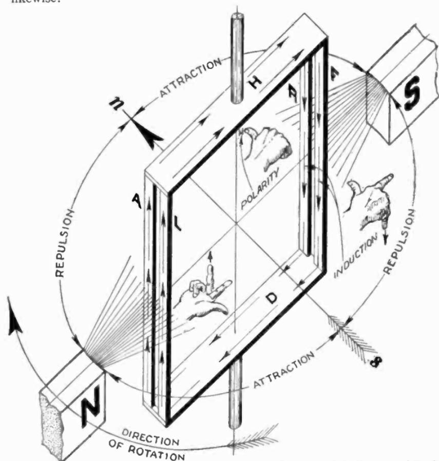
FIG. 2,652.—Squirrel cage principles. 1. Elementary four bar squirrel cage and rotating field with application of right hand rule for direction of induced polarity, and Fleming's rule for direction of induced current showing the polarity of the cage upon which the torque depends. The plates H and D, form connecting links for the bars L, A, and R, F, thus completing the circuits for the induced current.
