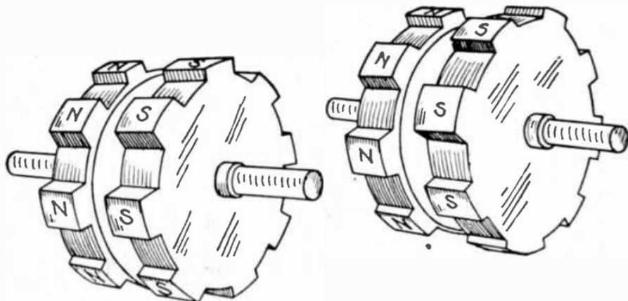
FIGS. 2,183 and 2,184.—Homopolar and heteropolar "inductors." Homopolar inductors have their N and S poles opposite each other, while in the heteropolar type, they are "staggered" as shown.
