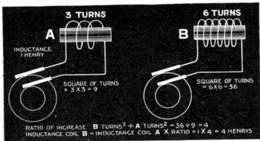
Figs. 2,007 and 2,008.—Diagrams illustrating relation of number of turns of an inductive coil and the inductances.
