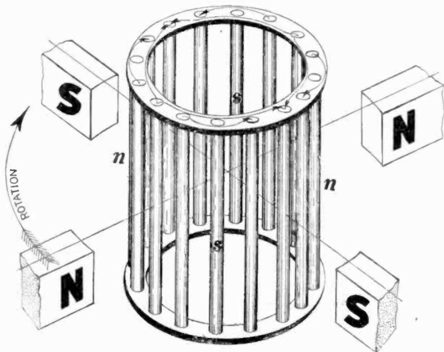
FIG. 2,665.—*Squirrel cage principles 7.* Elementary sixteen bar squirrel cage and four pole rotating field showing distribution of the induced currents in the armature with resulting approach to continuous and constant torque due to increase of bars and poles.
