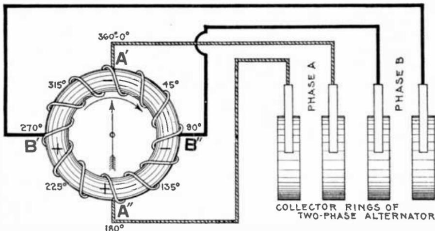
FIG. 2,565.—Production of a rotating magnetic field by two phase currents. The figure represents an iron ring, wound with coils of insulated wire, and supplied with two phase currents at the four points A, B, C, and D. The action of the two phase current on the ring in producing a rotating magnetic field is explained in the accompanying text.
