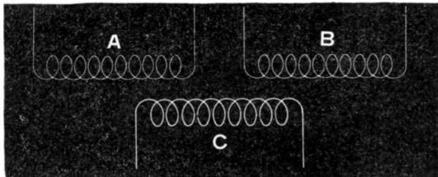
FIG. 2,421.—Diagrammatic sketch of one phase of a three winding transformer.
