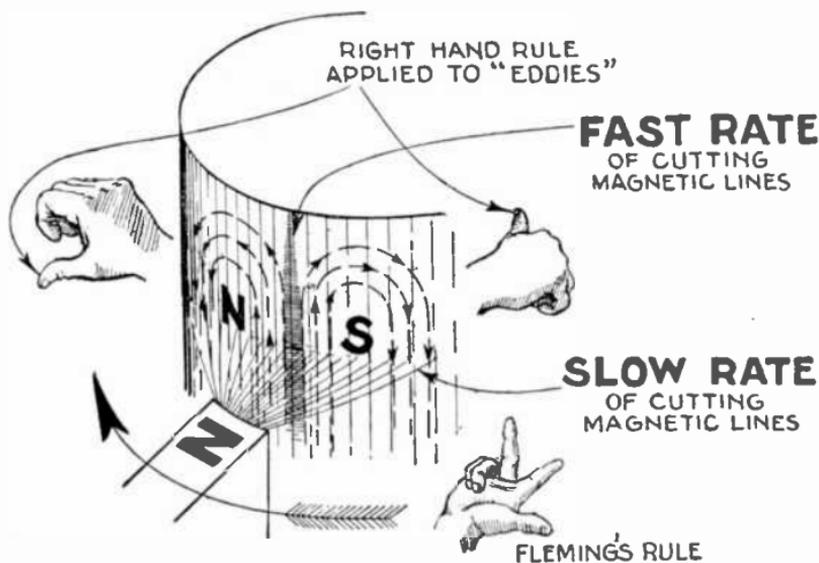
FIG. 2,627.—Detail of elementary copper cylinder and rotating magnet showing the variable rate of cutting *magnetic lines* which gives rise to eddy currents and resulting N and S poles.
