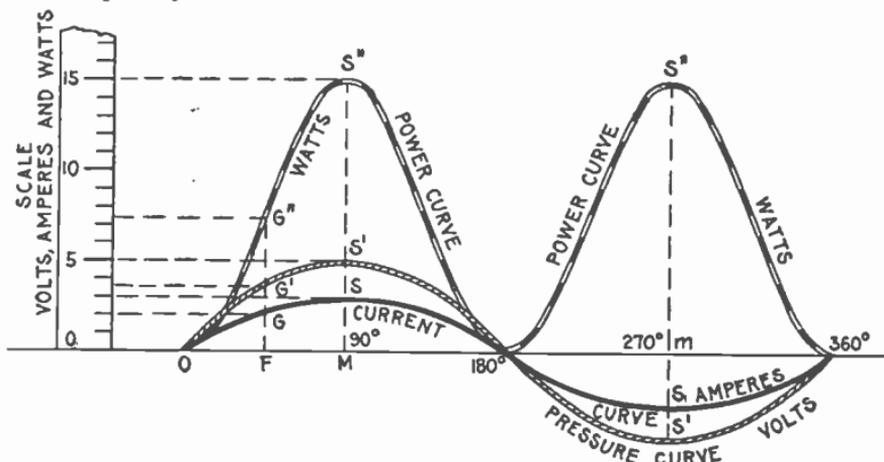
FIG. 2.114.—Method of drawing the power curve from the pressure and current curves. As shown, the same scale is used for all curves. This as a rule, makes the power curve inconveniently high, hence it is usually drawn to smaller scale as in fig. 2.115.
