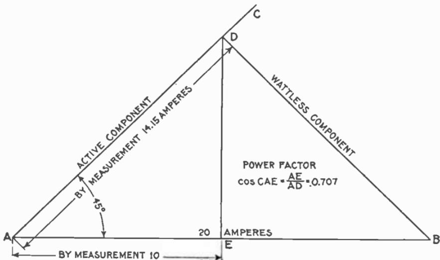
FIG. 2,131.—Diagram for obtaining the power factor for example 2. With convenient scale, lay off  $AB = 20$  amperes. From  $A$ , draw  $AC$ , at  $45^\circ$  to  $AB$ , and from  $B$ , draw  $BD$ , perpendicular to  $AC$ . Then, the power factor which is equal to cosine of angle of lag,  $= AD \div AB =$  (by measurement)  $14.15 \div 20 = .707$ .
