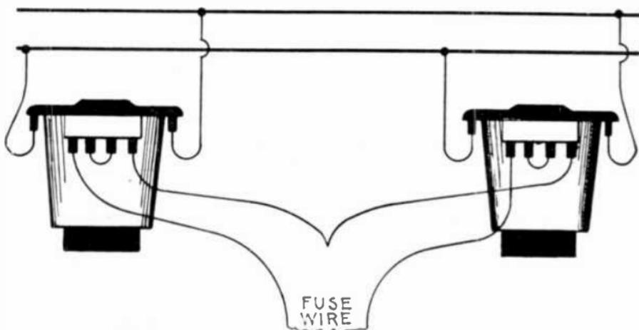
FIG. 2,430.—Method of comparing instantaneous polarities. Two of the terminals are connected as shown by a small strip of fuse wire, and then touching the other two terminals together. If the fuse blow, then the connections must be reversed; if it do not, then they may be made permanent.
