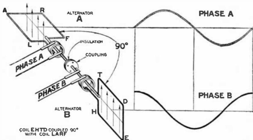
FIGS. 1,980.—Method of generating two phase alternating current with two single phase alternators coupled with coils at  $90^\circ$  to each other.
