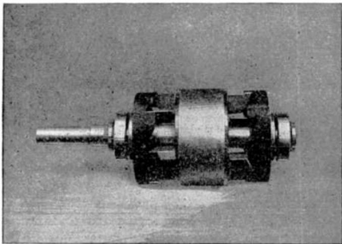
FIG. 2,546.—*Reliance induction motor construction 12.* Completed armature with shaft and ball bearings. The surface of the armature is ground to size. Blowers at each end are provided for ventilation.
