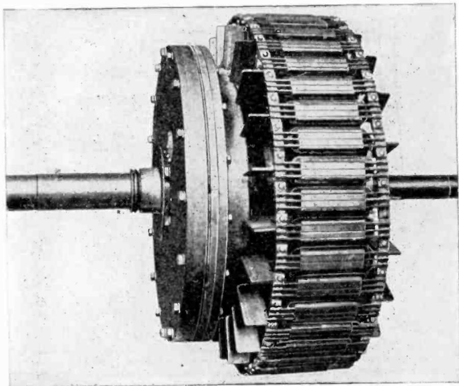
FIG. 2.522—Rotor of Westinghouse magnetic clutch type synchronous motor showing magnetic clutch, welded damper squirrel cage, field, fan, etc.
