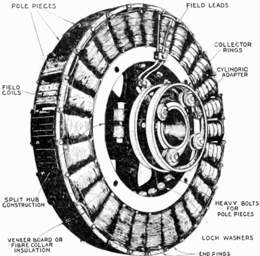
FIG. 2,175.—Revolving field of General Electric 375 kva., 200 r.p.m. slow speed synchronous alternator. The complete machine is shown in fig. 2,171.
