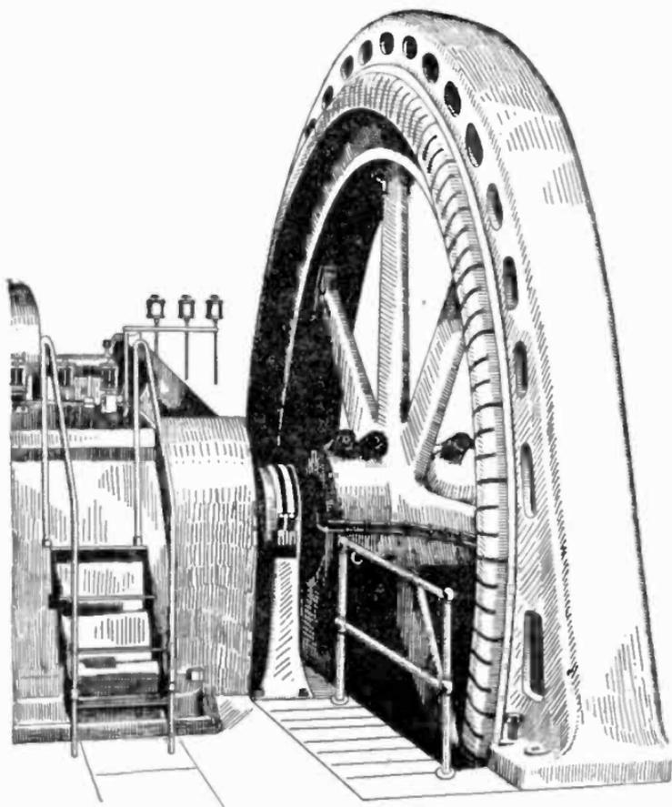
FIG. 2,219.—General Electric 48 pole 750 *kva.*, three phase fly wheel type alternator. It runs at a speed of 150 revolutions per minute, giving a frequency of 60 cycles per second and a full load pressure of 2,300 volts. The slip rings and leads to the field winding are clearly shown in the figure. The field magnets are mounted directly on the rim of the spider, which resembles very closely a fly wheel, and which in fact it is—hence the name “fly wheel alternator.”
