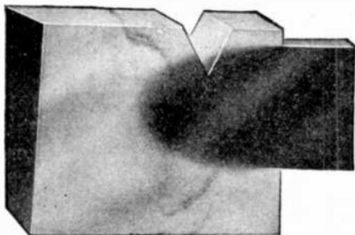
FIG. 2,672.—Section of Fairbanks-Morse "cast-on" joint showing union of end ring and inductor. The view shows the V-shape inspection groove as described in fig. 2,700.
