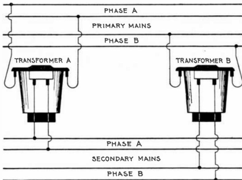
FIG. 2,432.—Two phase transformer connections. Two single phase transformers are used and connections made just as though each phase were an ordinary single phase system.
