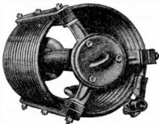
FIG. 2,009.—General Electric 400 ampere suspension copper choke coil. *The copper coil* has the advantage over other materials of being practically non-corrosive and non-crystallizing. The coils with braces and end spiders are interchangeable in all mountings, for the same ampere capacity. The turns are separated from one another and braced, the braces being held by end spiders. Weight of coil proper is supported on end spiders.
