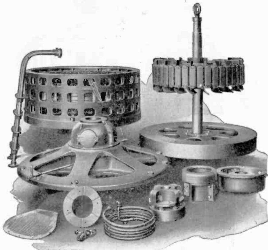
FIGS. 2,223 TO 2,233.—Disassembly of Allis Chalmers 200 kva; 180 r.p.m. vertical water wheel alternator.
