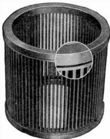
FIG. 2,700.—Appearance of Fairbanks-Morse squirrel cage if it could be removed from the core. The enlarged section shows the inspection groove cut in the end ring to prove the solidity of construction.
