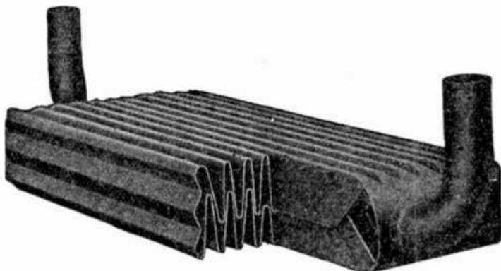
FIG. 2,355.—Pittsburgh Transformer Co. film radiator with section cut out, showing large radiating surface with very small film of oil.
