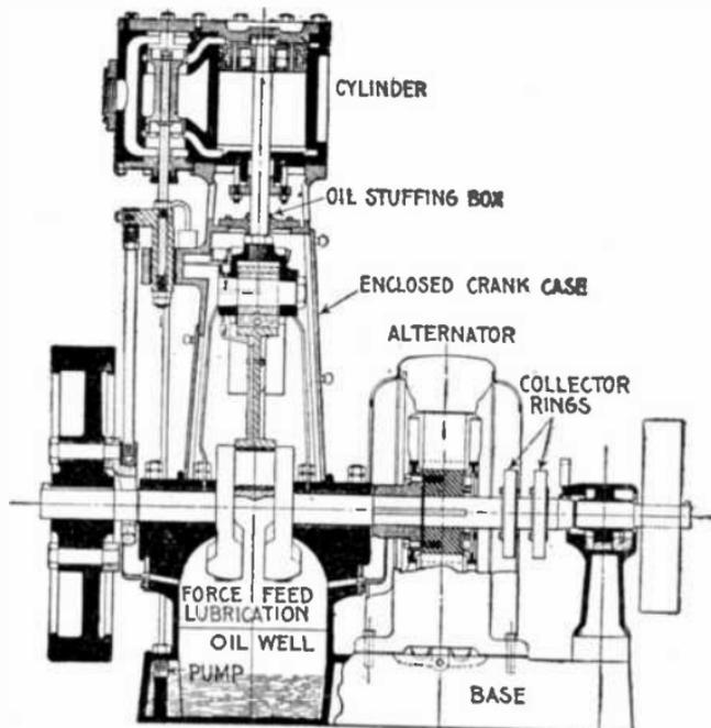
FIG. 2,169.—Endberg direct connected, or "engine type" alternator. In many places direct connected units are used, owing to the great saving in floor space, convenience of operation, and absence of belts.
