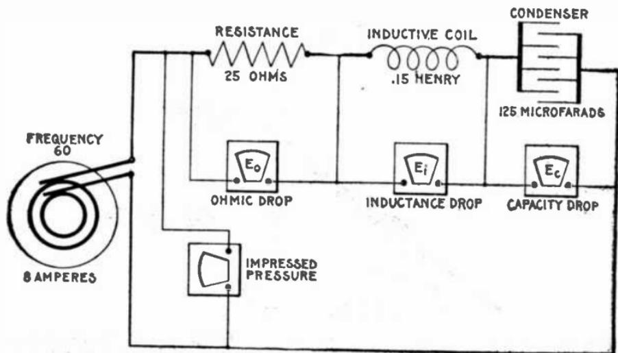
FIG. 2,109.—Diagram of circuit containing 25 ohms resistance, .15 henry inductance, and 125 microfarads capacity, with current of 8 amperes at 60 frequency.
