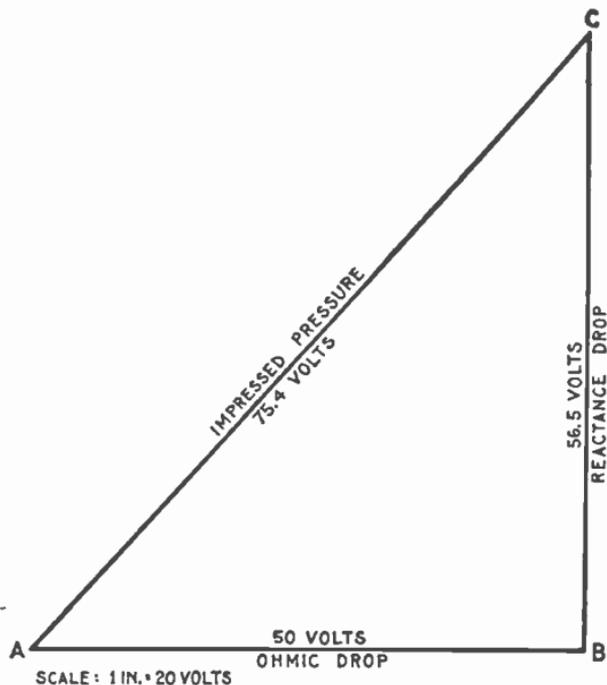
FIG. 2,088.—Diagram for impressed pressure on circuit containing 5 ohms resistance and inductance of 15 milli-henrys, the current being 10 amperes with frequency of 60.
