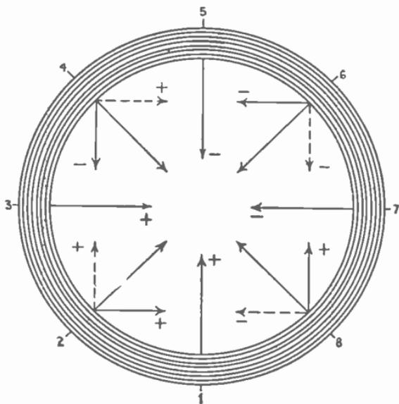
FIG. 2,560.—Method of obtaining resultant flux of Tesla's rotating magnetic field. The eight small diagrams here seen show the two components and resultant for eight equivalent successive instants of time during one cycle. At 1, the vertical flux is at + maximum and
