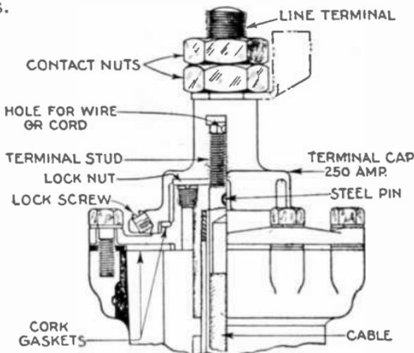
FIG. 2,385.—Terminal detail of General Electric solid interchangeable bushing.
