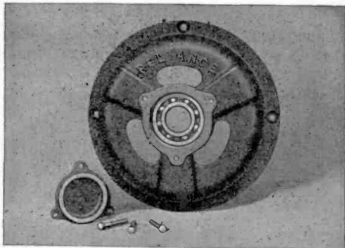
FIGS. 2,536 to 2,540.—*Reliance induction motor construction 7.* Bearing bracket. Extra strength is obtained by the channel shaped sections.
