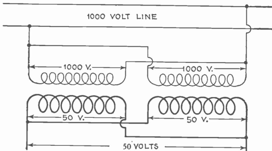
FIG. 2,425.—Diagram of single phase transformer with primary and secondary windings of two sections each, showing voltages per section with parallel connection.
