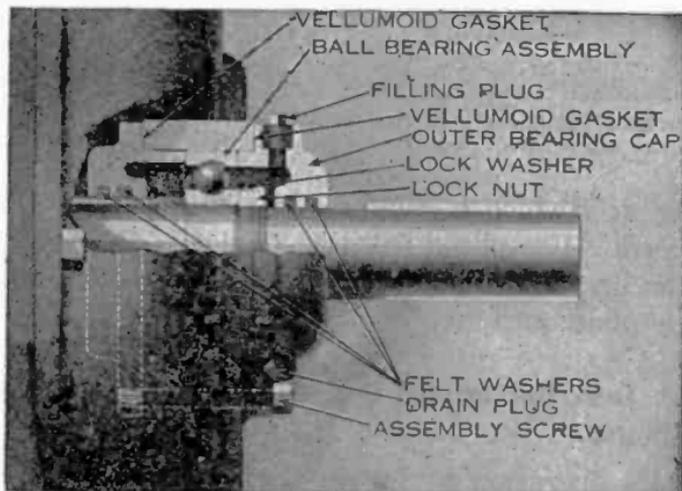
FIG. 2,541.—*Reliance induction motor construction 8.* Bearing mounting.
