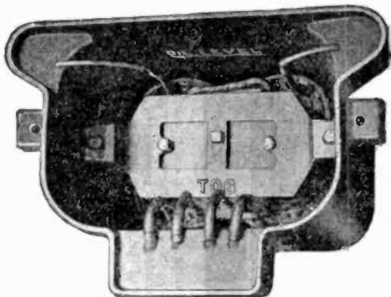
FIG. 2,357.—Duncan type B, 5 kva, 2, 300 volt transformer viewed from the top, showing oil level marking and method of sealing in leads.
