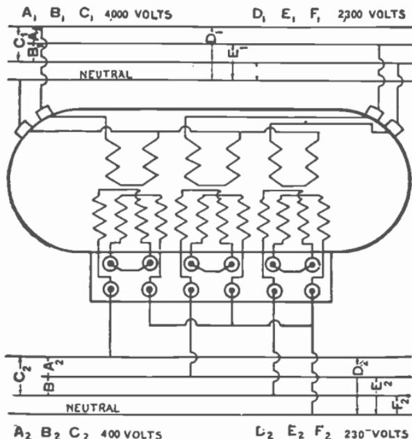
FIG. 2,142.—Pittsburgh connection diagram for three phase 4-wire star primary to three phase 4-wire star secondary.
