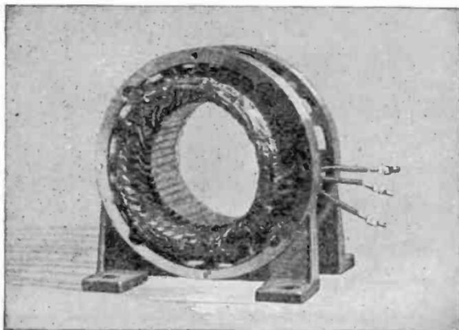
FIG. 2,530.—*Reliance induction motor construction 5.* Complete field with windings.
