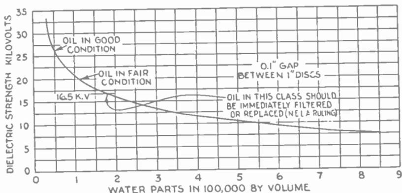
FIG. 2,422.—Curve showing the great reduction in dielectric strength produced by the presence of water in amounts up to 8 parts in 100,000.
