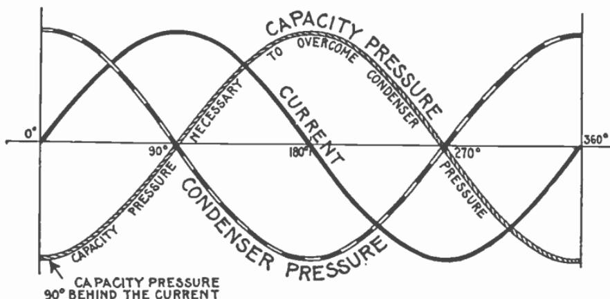
FIG. 2,096.—Current and pressure curves, showing phase relation between the current, condenser pressure, and impressed or *capacity* pressure necessary to overcome the condenser pressure. The capacity pressure, since it must overcome the condenser pressure, is equal and opposite to the condenser pressure, that is, the phase difference is  $180^\circ$ . The condenser pressure being  $90^\circ$  ahead of the current, the impressed pressure is  $90^\circ$  behind the current.
