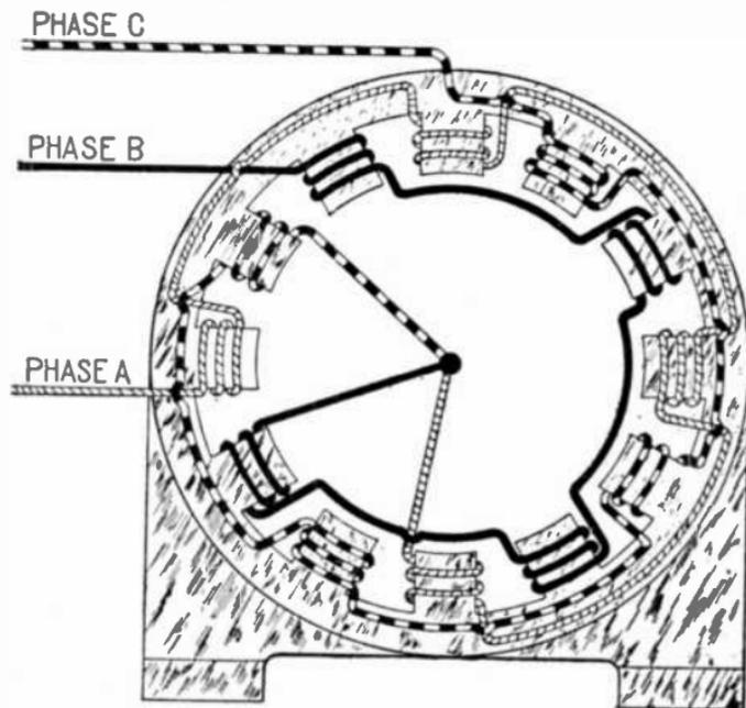
FIG. 2,602.—Diagram of three phase, four pole Y connected field winding.
