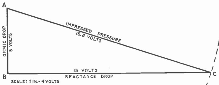
FIG. 2,085.—Diagram for obtaining reactance drop in circuit containing 5 volts ohmic drop and 15.8 volts impressed pressure.
