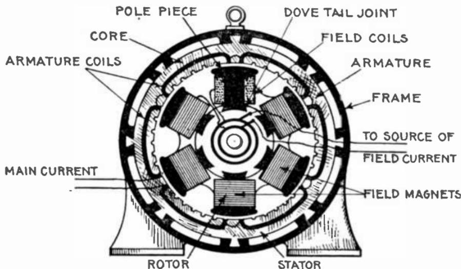
FIG. 2,176.—Diagram showing essential parts of a revolving field alternator and method of joining the parts in assembling.
