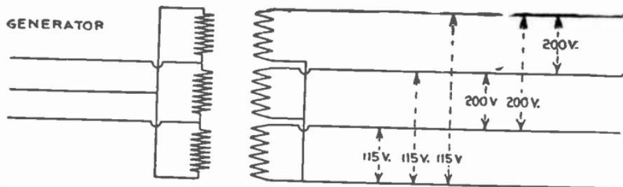
FIG. 2,466.—Delta-star connection of three transformers for low pressure, three phase, four wire system.
