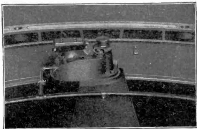
FIG. 2,235.—Allis-Chalmers vertical water wheel alternator brake and lifting jack.
