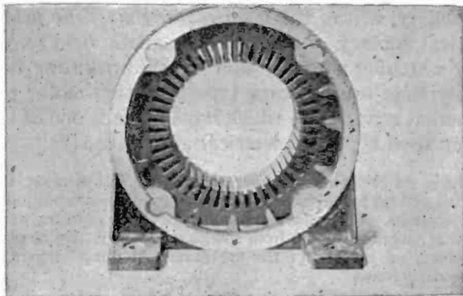
FIG. 2,527.—*Reliance induction motor construction 2.* Field laminations assembled with end flanges and ready for winding. End flanges are cast steel. The feet are cast integral with the steel flanges. All machine work on the flanges is done after assembly with the laminations.
