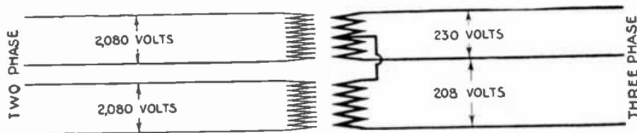
FIG. 2,470.—Diagram showing a method of operating a three phase motor on a two phase circuit, using a transformer having a tap made in the middle of the secondary winding, so as to get the necessary additional phase. While this does not give a true balanced three phase secondary, it is close enough for motor work. In the above arrangement, the main transformer supplies 54 per cent. of the current and the other with the split winding 46 per cent.
