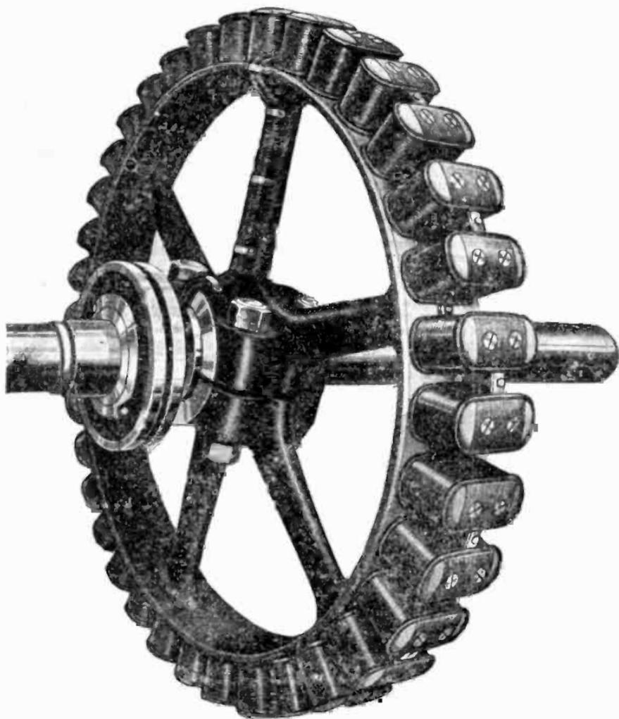
FIG. 2,274.—Triumph 36 pole fly wheel type revolving field. The spider has the form of a fly wheel having spokes and rim to which the field magnets are attached by through bolts. The field coils are of copper strap bent on end, the kind generally used on large machines. The series connection of the coils is plainly shown, also the two cables leading via one of the spokes to the slip rings.
