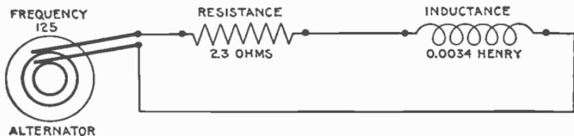
FIG. 2,043.—Diagram of circuit for example 2.
