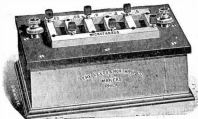
FIG. 2,023.—Condenser of one microfarad capacity. It is subdivided into five sections of .5, .2, .2, .05 and .05 microfarad. The plates are mounted between and carried by lateral brass bars which are fastened to a hard rubber top. Each pair of condenser terminals is fastened to small binding posts mounted on hard rubber insulated posts.
