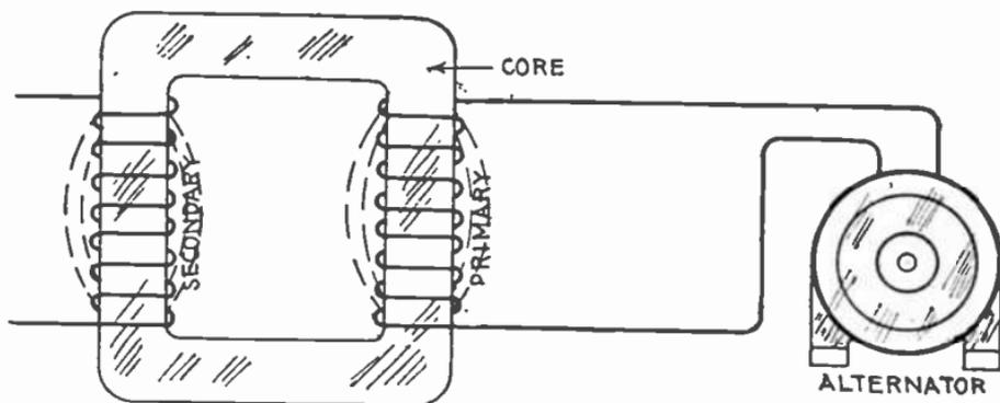
FIG. 2,294.—Diagram of elementary transformer with continuous core and connections with alternator. The dotted lines show the leakage of magnetic lines. To remedy this the arrangement shown in fig. 2,295 is used.
