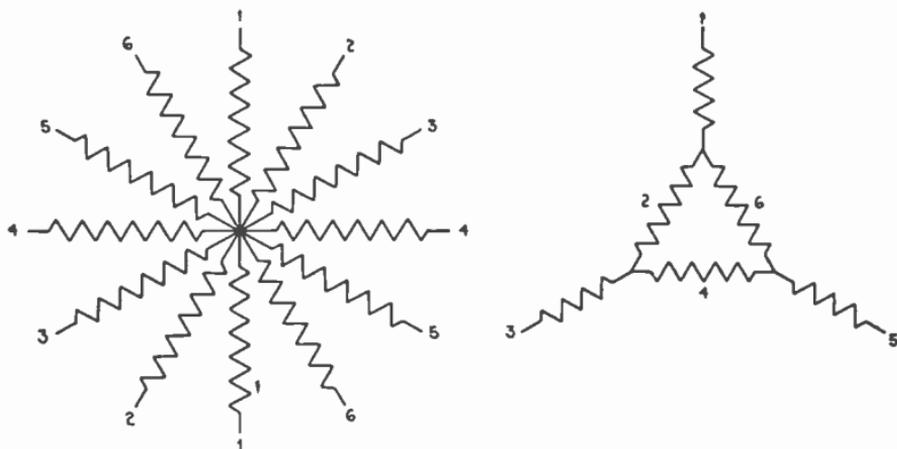
FIG. 2,158.—Diagram of twelve phase winding with star grouping.
