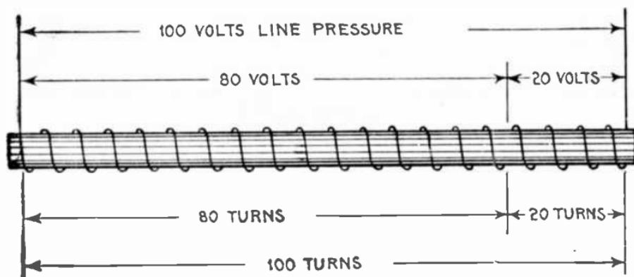
FIG. 2,404.—Diagram illustrating connections and principles of auto-transformers as explained in the accompanying text.
