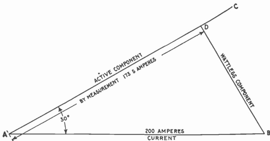
FIG. 2,130.—Diagram for obtaining the active component of the current in a circuit having a current of 200 amperes and angle of lag of  $30^\circ$ .
