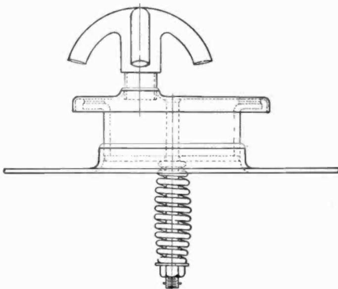
FIG. 2,358.—Pittsburgh automatic safety valve with Pittsburgh breather mounted. It has four outlets to the air and each outlet contains a copper gauze screen to prevent dust and dirt entering the transformer. These breathers allow for sufficient "breathing" in the transformer, at the same time preventing the entrance of moisture and dirt.
