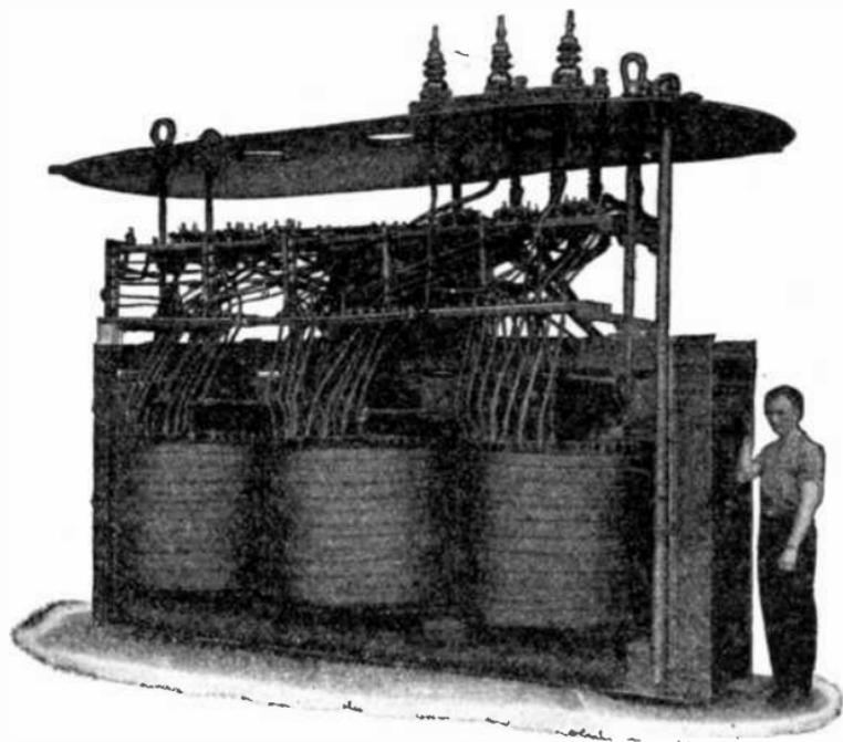
FIG. 2,353.—Core and coils of large 15,000 kva. Pittsburgh self-cooled by external radiator transformer on freight car ready for shipment.
