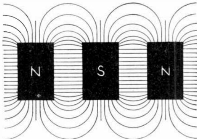
FIG. 2,209.—Diagram showing lateral field between adjacent poles.
