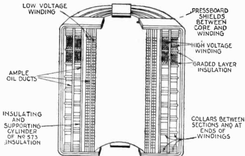
FIG. 2,339.—Details of coil construction of General Electric type H, form KR, transformer.
