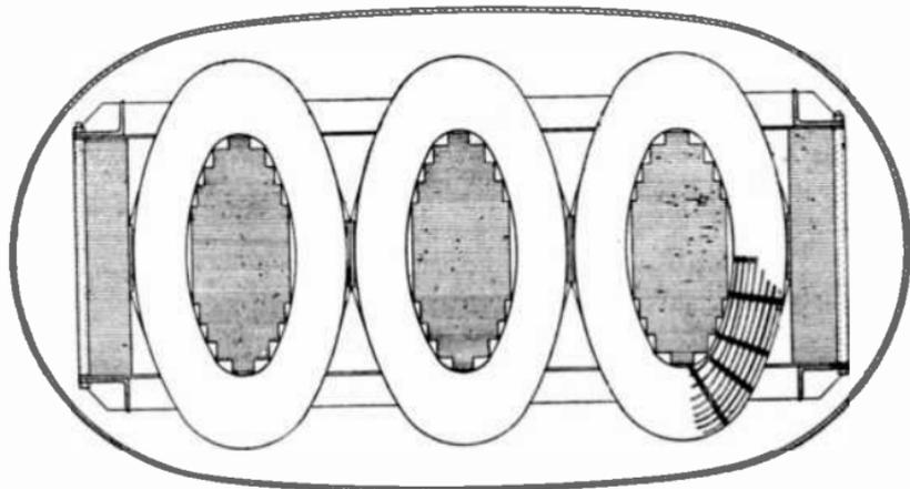
FIG. 2,326.—Cross section of Pittsburgh polyphase transformer.
