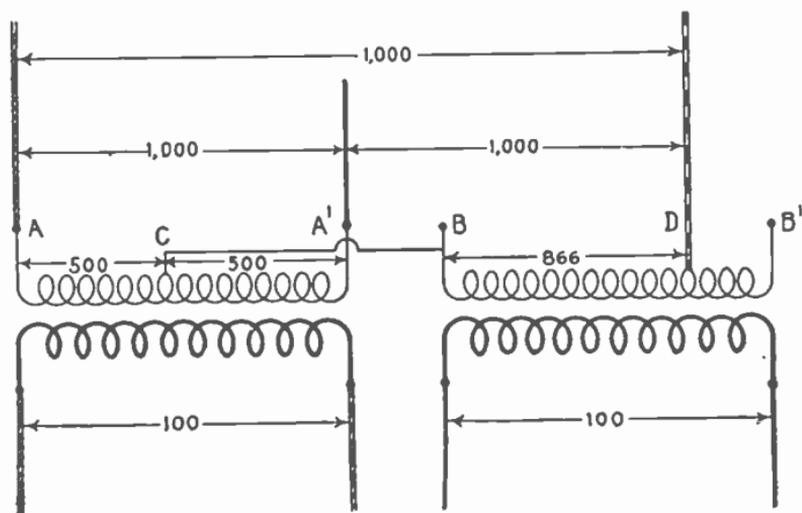
FIG. 2,469.—The Scott connection for transforming from three phase to two phase. In this method one of the primary wires B, of the .866 ratio transformer is connected to the middle of the other primary as at C, the ends of which are connected to two of the three phase wires. The other phase wire is connected at D, the point giving the .866 ratio. The secondary wires are connected as shown.
