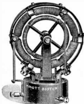
FIG. 2,034.—Knott alternating current demonstration apparatus; *three phase Tesla motor*. This motor is wound for use on a pressure of not over 4 volts. The windings are made of three colors of wires and there are six fields with a short circuited rotor. All connections are open and are connected in star and colored.
