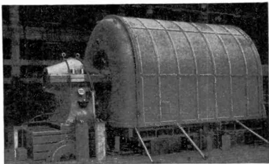
FIG. 2,251.—Westinghouse turbine alternator, view showing machine with SK frame completely assembled for testing revolving elements.
