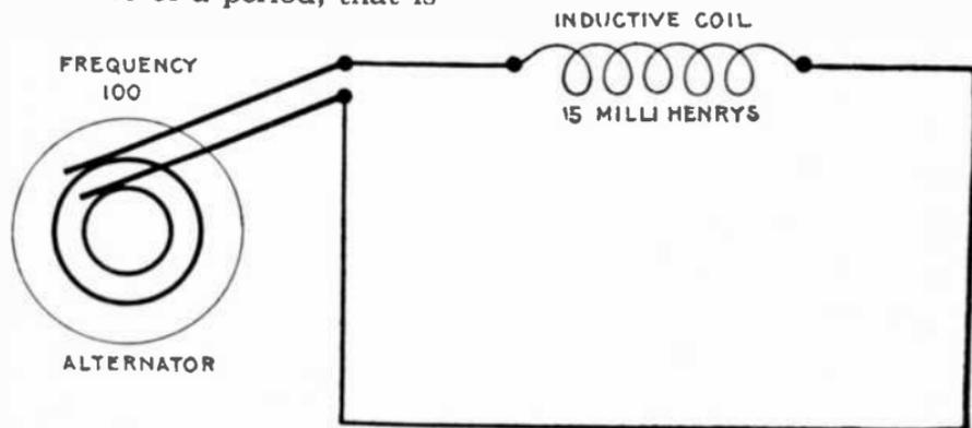
FIG. 2,013.—Diagram showing alternating circuit containing inductance. Formula for calculating the ohmic value of inductance or "inductance reactance" is  $X_L = 2 \pi f L$  in which  $X_L$  = inductance reactance;  $\pi = 3.1416$ ;  $f$  = frequency;  $L$  = inductance in henrys (not milli-henrys).  $L = 15$  millihenrys =  $15 + 1000 = .015$  henrys. Substituting,  $X_L = 2 \times 3.1416 \times 100 \times .015 = 9.42$  ohms.
