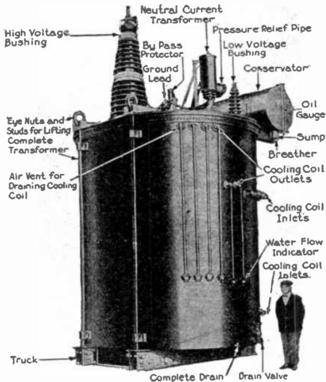
FIG. 2,361.—General Electric single phase water cooled outdoor transformer.
