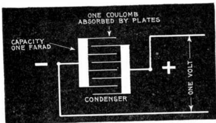
FIG. 2,022.—Diagram illustrating a farad. A condenser is said to have a capacity of one farad if it will absorb one coulomb of electricity when subjected to a pressure of one volt. The farad is a very large unit, and accordingly the microfarad or one millionth of a farad is often used, though *this must be reduced to farads before substituting in formulæ*.
