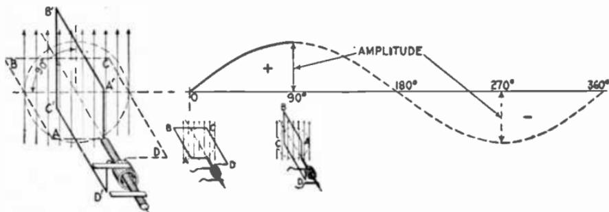
FIG. 1,941.—Diagram illustrating *amplitude* of the current. The current reaches its amplitude or maximum value in one quarter period from its point of zero value, as, for instance, while the generating loop moves from position ABCD, to A'B'C'D'. At three-quarter revolution, the current reaches its maximum value in the opposite direction.
