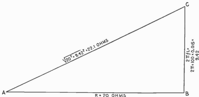
FIG. 2,092.—Diagram for impedance of circuit containing 20 ohms resistance, and inductance of 15 millihenrys, when the frequency is 100.
