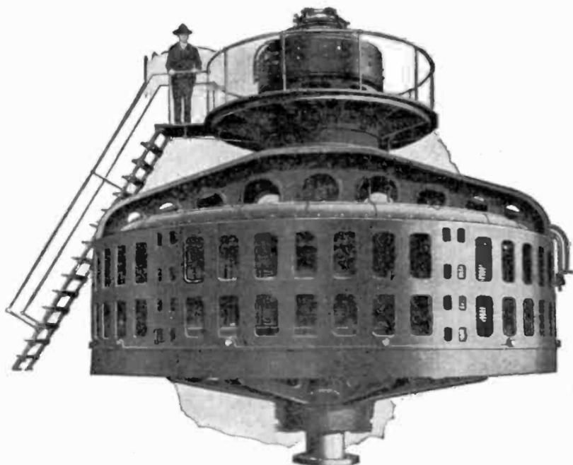
FIG. 2,234.—Allis-Chalmers 18,750 *kva.*, 6,600 volt,  $112\frac{1}{2}$  *r.p.m.* vertical water wheel alternator.
