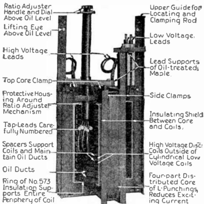
FIG. 2,337.—General Electric medium size 33,000 volt transformer with disc coil high voltage winding showing application of ratio adjuster.
