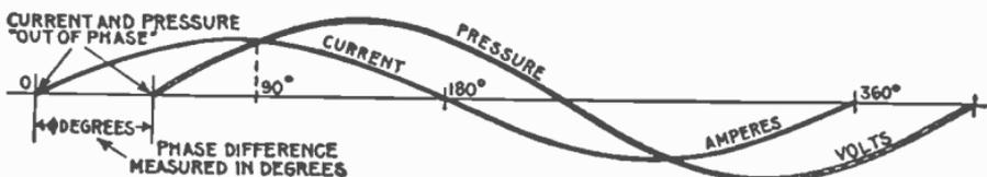
FIG. 1,949.—Pressure and current curves illustrating the term “out of phase.” The current is said to be *out of phase* with the pressure when it *either lags or leads*, that is when the current is not in synchronism with the pressure. In practice the current and pressure are nearly always out of phase.
