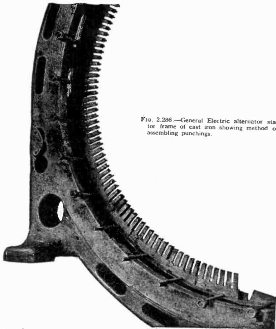
FIG. 2,286.—General Electric alternator stator frame of cast iron showing method of assembling punchings.
