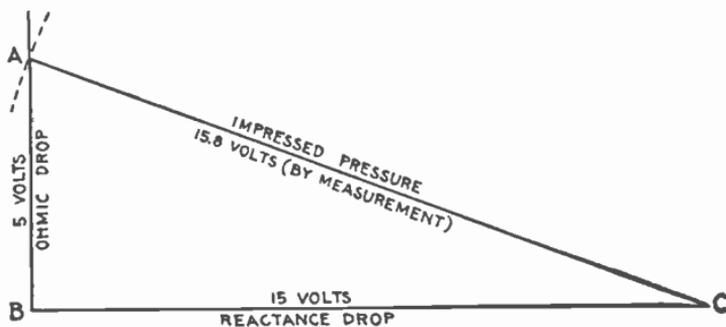
FIG. 2,086.—Diagram for obtaining ohmic drop in the circuit fig. 2,084 when impressed pressure and reactance drop are given. Lay off  $BC$ , to scale = reactance drop; draw  $AB$ , at right angles and of indefinite length; with  $C$ , as center and radius of length = impressed pressure, describe an arc cutting ohmic drop line at  $A$ , then  $AB$  = ohmic drop = 5 volts by measurement.
