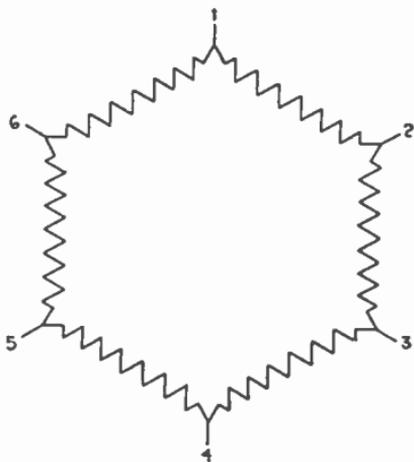
FIG. 2,157.—Diagram of six phase winding with mesh grouping.
