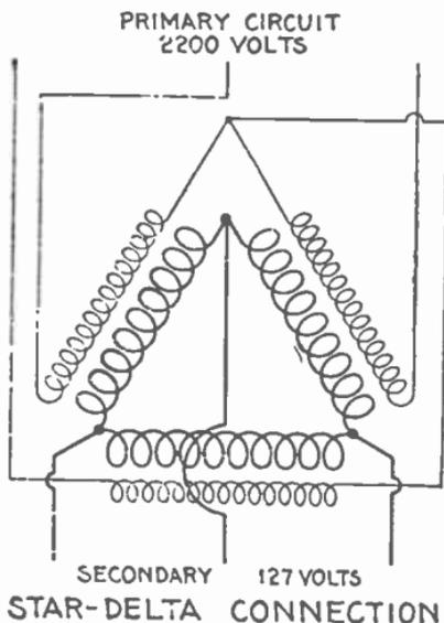
Figs. 2,434 to 2,437.—Three phase transformer connections. Fig. 2,434 delta connection; fig. 2,435 star connection; fig. 2,436 delta-star connection; fig. 2,437 star-delta connection.
