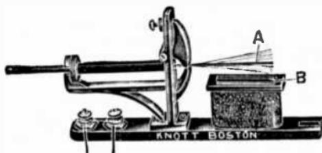
FIG. 2,001.—Knott frequency indicator for 100 volt *a.c.* circuit. This instrument is designed primarily to show on the screen the effect produced by an alternating current on an electromagnet. The length of the vibrating reed is such as to show clearly on the screen, the  $\frac{1}{4}$ -wave length, the  $\frac{1}{2}$ -wave length and the  $\frac{3}{4}$ -wave length. *In use* the instrument is connected directly to 110 volt circuit without additional resistance.
