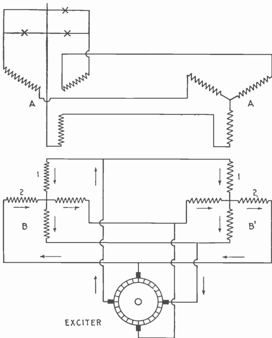
FIG. 2,255.—Diagram of constant pressure image current alternator connections. The image or reproduced currents are characteristic of all types of asynchronous machines, and are called image currents because they are actually the reflection from the load currents delivered by the armature circuit. The principle of operation is explained in the accompanying text.
