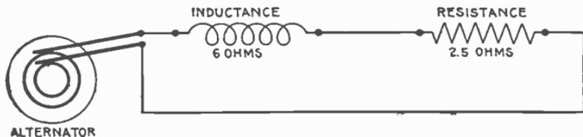
FIG. 2,042.—Diagram of circuit for example 1.
