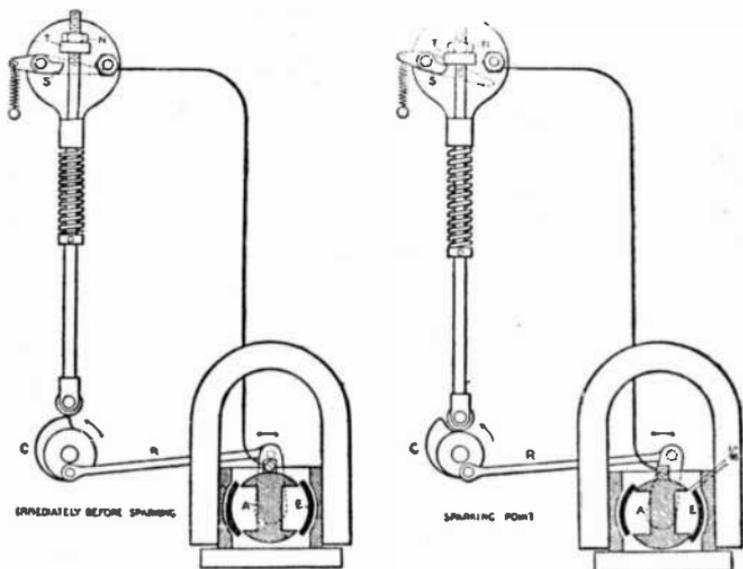
FIGS. 2,179 and 2,180.—A low tension ignition system with an inductor magneto of the oscillating type. The inductor B, is rotated to and fro by means of a link R, one end of which is attached to the inductor crank, and the other to the igniter cam C. Two views are shown: immediately before and after sparking. S, is the grounded electrode of the igniter; T, an adjustable hammer which is secured in position by a lock nut N.
