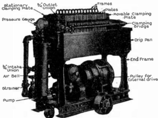
FIG. 2,423.—General Electric transformer oil dryer and filter for freeing the oil from moisture, slime and sediment. *In operation*, the oil is forced through several layers of dry blotting paper. The complete equipment consists of a filter press with motor driven oil pump, electric drying oven for thoroughly drying the filter paper before placing it in the press.
