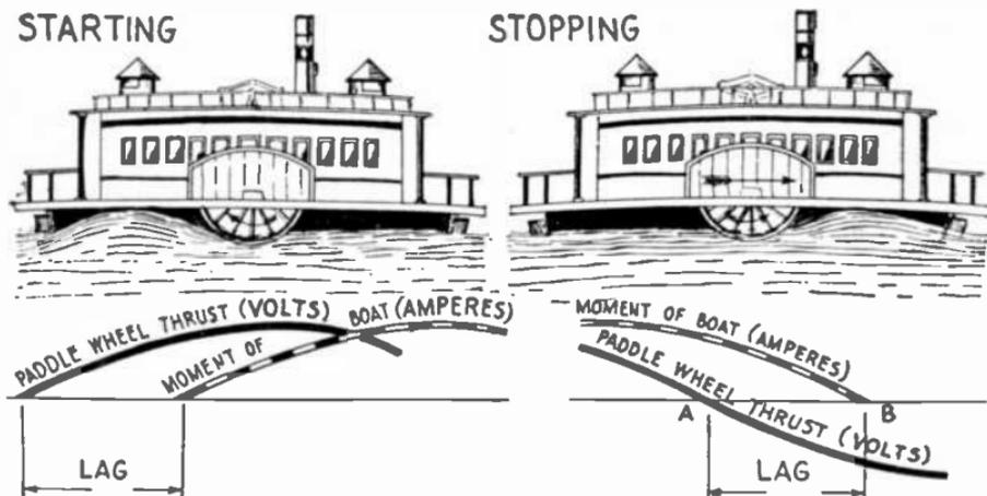
FIGS. 2,052 and 2,053.—Ferry boat analogy of lag. In starting, the paddle wheels make an appreciable thrust (*volts*) before the boat begins to move (*amperes*). Thus the movement of the boat (*amperes*) lags behind the thrust of the paddle wheels (*volts*). In stopping, the paddle wheels make several reverse turns (*reversal of a. c. volts*) before the movement of the boat (*amperes*) ceases, thus lagging behind the thrust of the paddles (*volts*).
