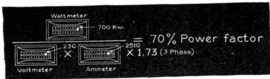
FIG. 2,146.—Meter reading on three phase circuit 70% power factor.
