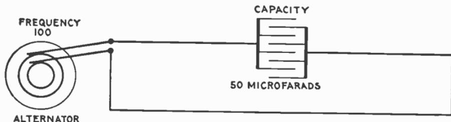
FIG. 2.056.—Diagram of circuit for *example 3*.
