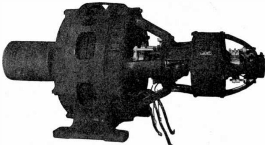
FIG. 2,213.—Westinghouse type SK alternator with revolving armature and direct connected exciter.
