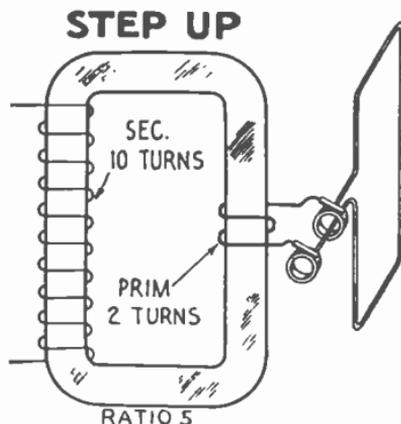
FIG. 2.314.—Diagram of elementary *step up* transformer. As shown the primary winding has two turns and secondary 10 turns, giving a ratio of voltage transformation of  $10 \div 2 = 5$ . Since only  $\frac{1}{5}$  as much current flows in the secondary winding as in the primary, the latter requires heavier wire than the former.
