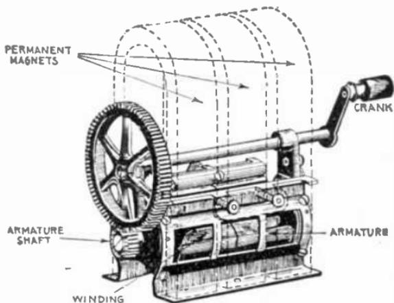
FIG. 2,262.—Connecticut magneto; view showing permanent magnets in dotted lines. It consists of three permanent U shape magnets, between the poles of which is a shuttle type armature. The latter is geared to a hand crank in sufficient velocity ratio to give the desired speed without too rapid turning of the crank. This type of magneto is used to generate current for operation of telephone call bells.
