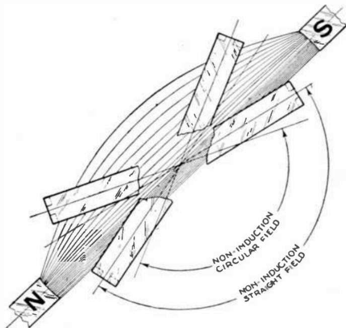
FIG. 2,655.—*Squirrel cage principles 4.* Top view of elementary four bar squirrel cage and rotating field (curved lines of force) showing zones of non-induction, weak and strong induction.
