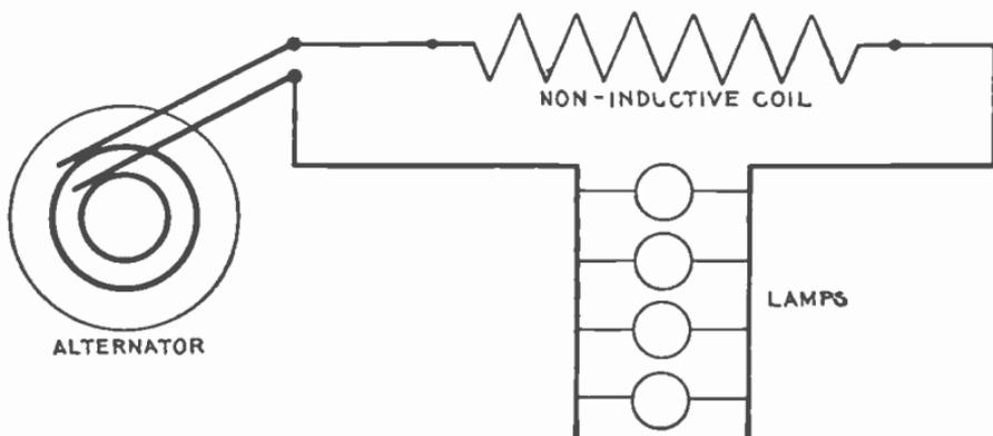
FIG. 2,117.—Diagram of circuit containing only resistance; in such a circuit the power factor is unity.
