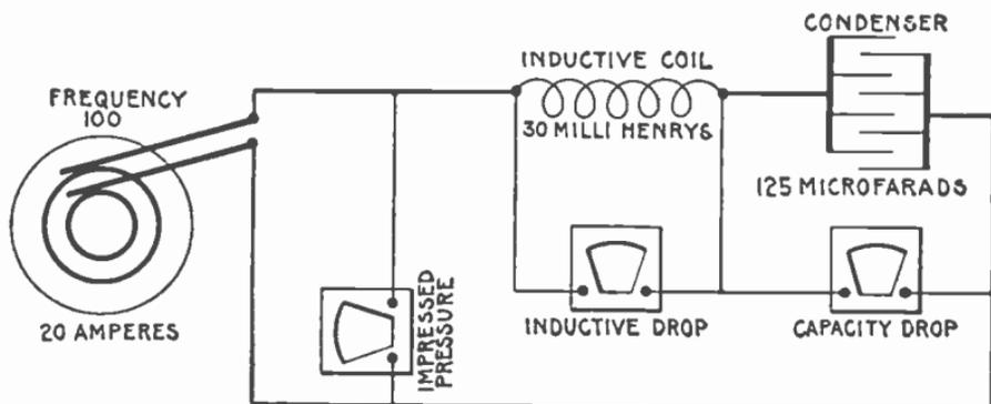
FIG. 2,102.—Diagram of circuit containing 30 millihenrys inductance and 125 microfarads capacity, with current of 20 amperes, 100 frequency.
