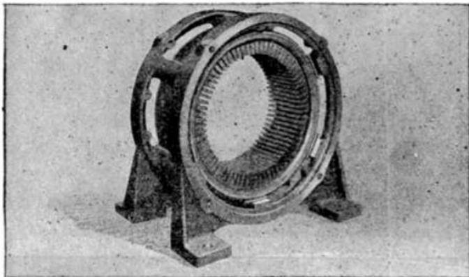
FIG. 2,551.—*Reliance induction motor construction 15.* Skeleton frame with laminations. Open slots are used in the field punchings.
