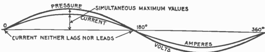
FIG. 1,948.—Pressure and current curves illustrating the term “in phase.” The current is said to be *in phase* with the pressure when it *neither lags nor leads*.
