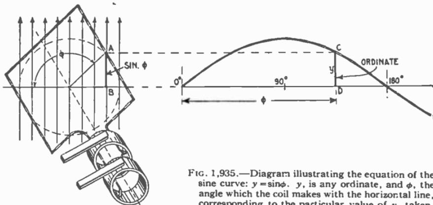
FIG. 1,935.—Diagram illustrating the equation of the sine curve:  $y = \sin \phi$ .  $y$ , is any ordinate, and  $\phi$ , the angle which the coil makes with the horizontal line, corresponding to the particular value of  $y$ , taken.
