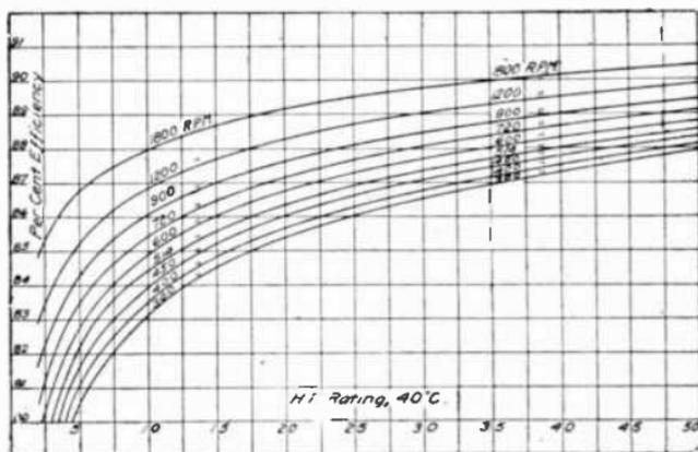
FIG. 2,702.—Efficiency of 60 cycle, squirrel cage induction motors at 100% load, 3 to 50 h.p.
