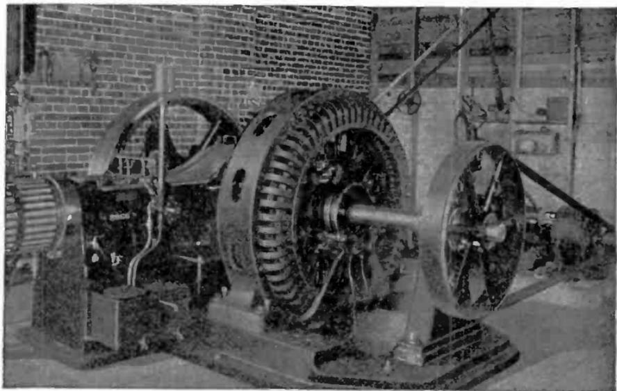
FIG. 2,217.—Diagram showing a Westinghouse 50 kva., 2,400 volt, three phase, 60 cycle revolving field separately excited alternator direct connected to a steam engine. The exciter is belted to the alternator shaft, the driving pulley being located outside the main bearing. The small pulley on the exciter gives an indication of its high speed as compared with that of the alternator.
