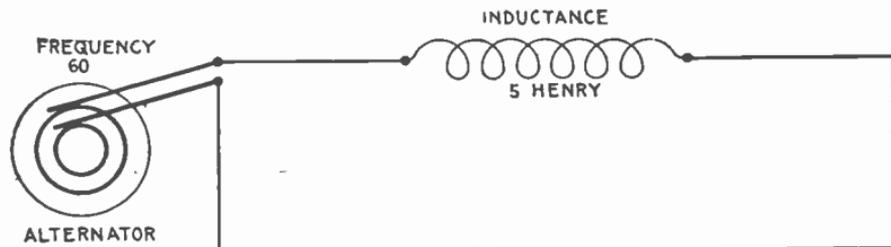
FIG. 2,055.—Diagram of circuit for *example 2*. As in *example 1*, resistance is disregarded.
