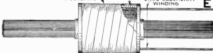
BEND OVER LOOSE ENDS OF CORE WIRES
