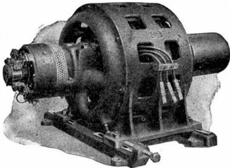
FIG. 2.485.—Allis Chalmers synchronous motor with direct connected exciter. This type machine is made only in the smaller sizes and is of self-contained or bracket bearing construction for more or less high speed work. The feet of the stator yoke rest directly on the base or slide rails, a base being provided where three bearing belted parts are required
