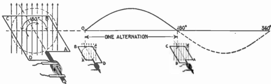
FIG. 1,940.—Diagram showing one *alternation* of the current in which the latter varies from zero to maximum and back to zero while the generating loop ABCD, makes one half revolution.
