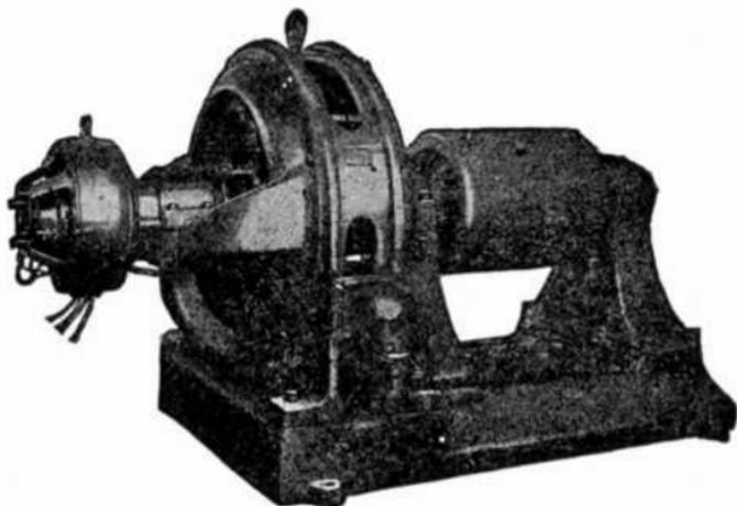
FIG. 2,516.—General Electric 12 pole, 600 r.p.m., 250 h.p. synchronous motor with 3 kw. 125 volt exciter.
