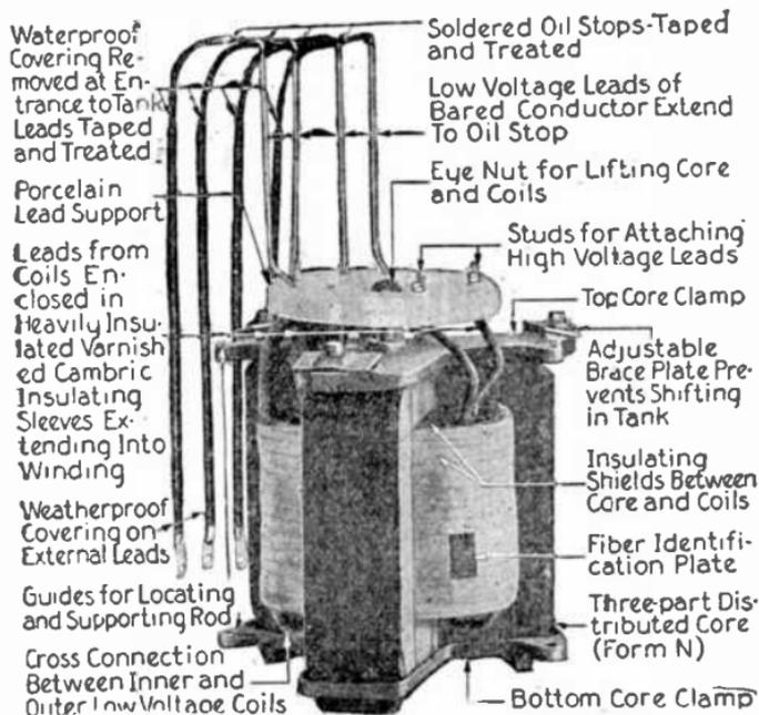
FIG. 2,321.—General Electric core and coils of a core wound type H single phase, 60 cycle, 2,300 volt transformer, using three part distributed core. The coils are provided with vertical oil ducts, which cross each conductor in the adjacent layers and assure uniform cooling. The number and location of these ducts vary with the size of the transformer.
