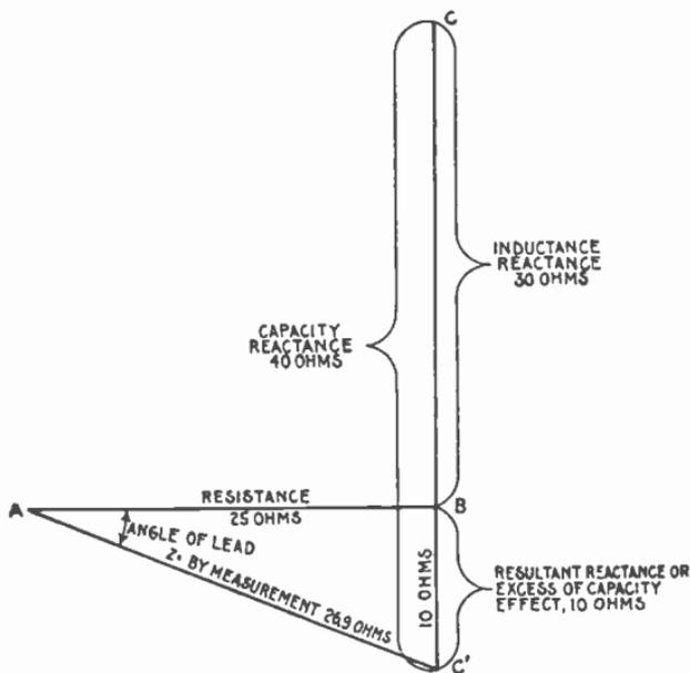
FIG. 2,105.—Impedance diagram of a circuit containing 25 ohms resistance, 30 ohms inductance, and 40 ohms capacity. The resultant reactance being due to excess of capacity, the impedance line  $AC'$  falls below the horizontal line  $AB$ , indicating that the current leads pressure.
