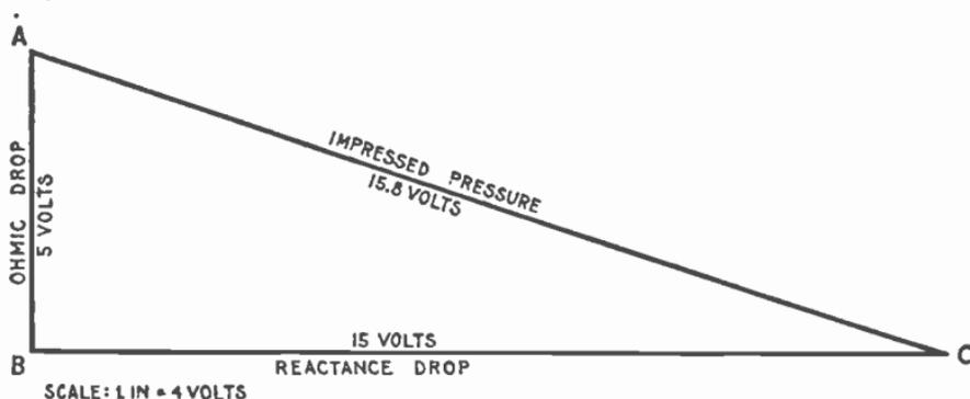
FIG. 2,083.—Diagram for impressed pressure on circuit containing 5 volts ohmic drop and 15 volts reactance drop.
