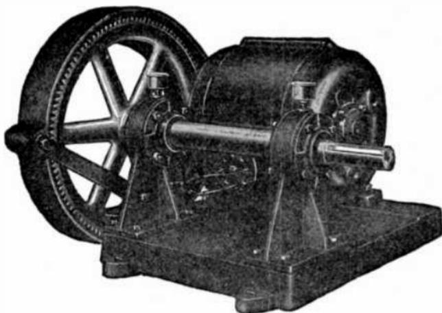
FIG. 2,633.—Triumph back geared polyphase induction motor. A great many applications, especially for direct attachment, require the use of either a very slow or special speed motor. As these are quite costly, the preferable arrangement, and one equally as satisfactory, is the use of a standard speed motor combined with a back geared attachment. Rawhide pinions are furnished whenever possible, insuring smooth running with a minimum of noise.
