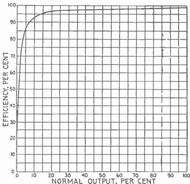
FIG. 2,374.—Efficiency curve of Westinghouse 375 *kva.* transformer. Pressure 500 to 15,000 volts; frequency 60. Efficiencies at different loads: full load efficiency, 98%;  $\frac{3}{4}$  full load efficiency, 98%;  $\frac{1}{2}$  full load efficiency, 97.6%;  $\frac{1}{4}$  full load efficiency, 96.1%; regulation non-inductive load, 1.4%; load having .9 power factor, 3.3%.
