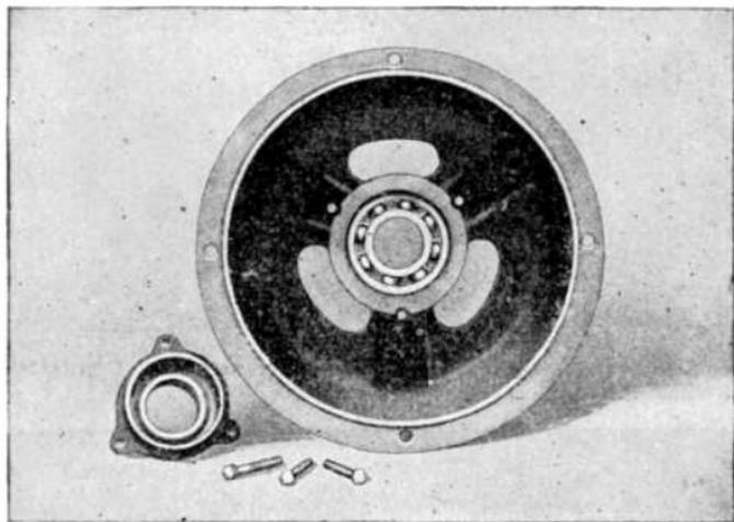
FIG. 2,531 to 2,535.—*Reliance induction motor construction 6.* Bearing bracket with outside bearing cap removed. Bearings are interchangeable for both ends of the motor.
