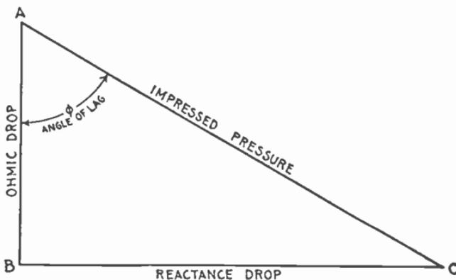
FIG. 2,087.—Graphical method of finding angle of lag when the ohmic drop and reactance drop are given. The angle of lag  $\phi$ , is that angle included between the impressed pressure and the ohmic drop lines, that is, between AC and AB.
