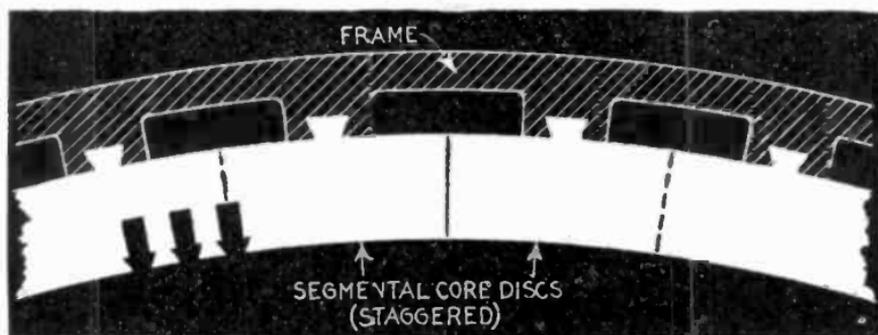
FIG. 2,283.—Construction of large stationary armature; view showing section of core and frame. The core discs are in segments and are attached to the frame by dovetail joints as shown. The joints are staggered in building up the core, that is, they are overlapped so as not to unduly increase the reluctance of the magnetic circuit. Through bolts are seldom used for securing the laminations, because if not insulated, are liable to give rise to eddy currents by short circuiting the discs.
