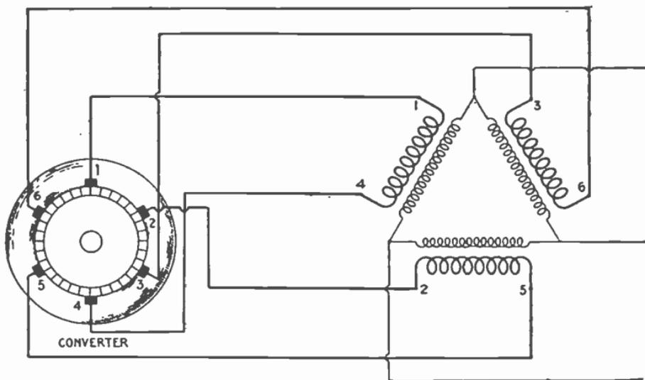
FIG. 2,472.—Diagram of *diametrical connection, three phase to six phase*. It is obtained by bringing both ends of each secondary winding to opposite points on the rotary converter winding, utilizing the converter winding to give the six phases. This transformation of phases may also be obtained with transformers having two secondary windings.
