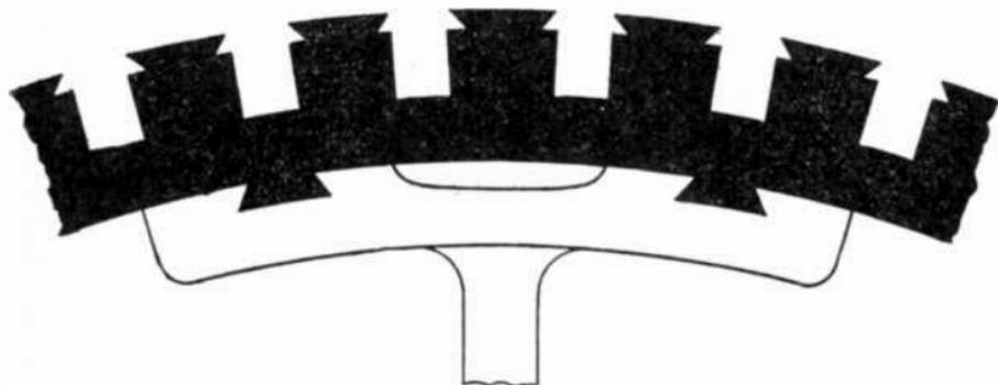
FIG. 2,281.—Large revolving armature construction with segmental punchings dovetailed to spider spokes.
