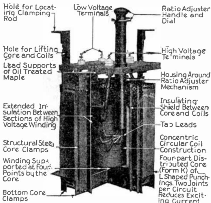
FIG. 2,333.—General Electric core and coils of a form wound, type H form KR distribution transformer.
