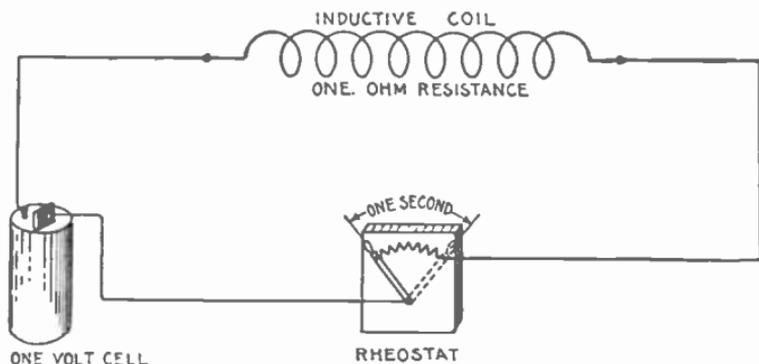
FIG. 1,997.—Diagram illustrating the henry. *By definition: A circuit has an inductance of one henry when a rate of change of current of one ampere per second induces a pressure of one volt. In the diagram it is assumed that the internal resistance of the cell and resistance of the connecting wires are zero.*
