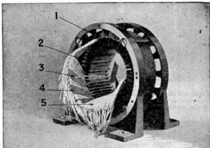
FIG. 2,528.—*Reliance induction motor construction 3.* The details are: 1, slot cell insulation extends  $\frac{1}{4}$  in. beyond slot; 2, fibre separator inserted in slot between coils; 3, slot stick; 4, oiled muslin used for insulating coils between phases; 5, heads of coils are taped with linen tape.
