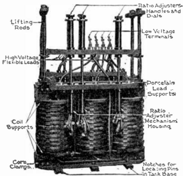
FIG. 2,366.—General Electric core and coils of small power high voltage, three phase transformer. The windings of three phase distribution and small power transformers are formed in all sizes, with one phase assembled on each leg of the core. In arrangement, spacing and insulation the same general practice is followed as in the single phase designs.
