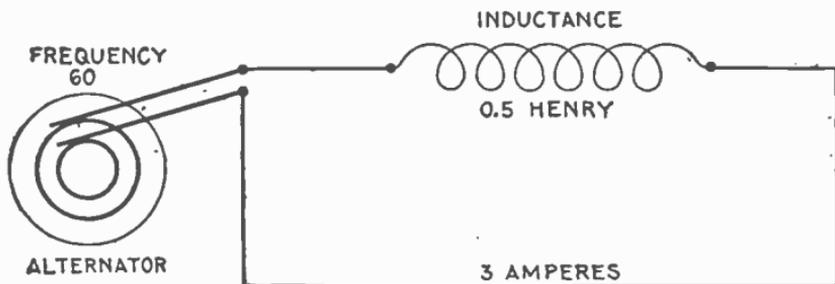
FIG. 2,054.—Diagram of the circuit for *example 1*. Here the resistance is taken at zero, but this would not be possible in practice, as all circuits contain more or less resistance though it may be, in some cases, negligibly small.
