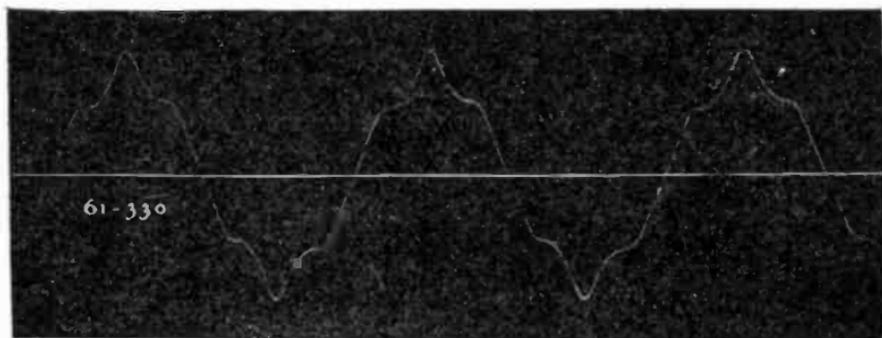
FIG 1,968 —Reproduction of oscillograph record of wave form of alternator with one coil per phase per pole Here the so-called "super-imposed harmonic" is clearly indicated.
