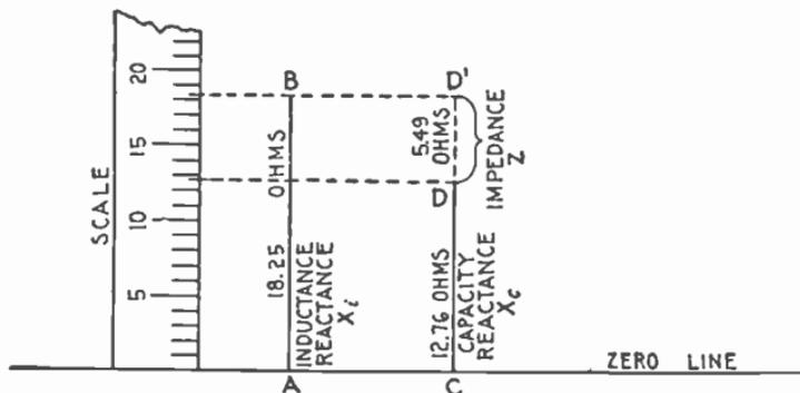
FIG. 2,103.—Impedance diagram for circuit (of above example) containing inductance and capacity. With any convenient scale, erect a perpendicular  $AB = 18.25$  ohms, and  $CD = 12.76$  ohms. Continue  $CD$  by dotted line to  $D'$  so that  $CD' = AB$ , then  $DD' = AB - CD =$  inductance reactance  $-$  capacity reactance, which is equal to the impedance. Expressed by letters  $Z = X_l - X_c = DD'$ , which by measurement  $= 5.49$  ohms.
