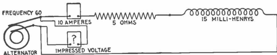
FIG. 2,089.—Diagram of circuit containing 5 ohms resistance, 15 milli-henrys inductance, with 8 ampere 60 frequency current.
