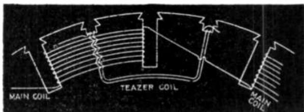
FIG. 2,191.—Diagram showing section of monocyclic alternator armature illustrating the armature winding. The main coils are wound on every other tooth, and the teaser coils are placed in quadrature with them, as shown.
