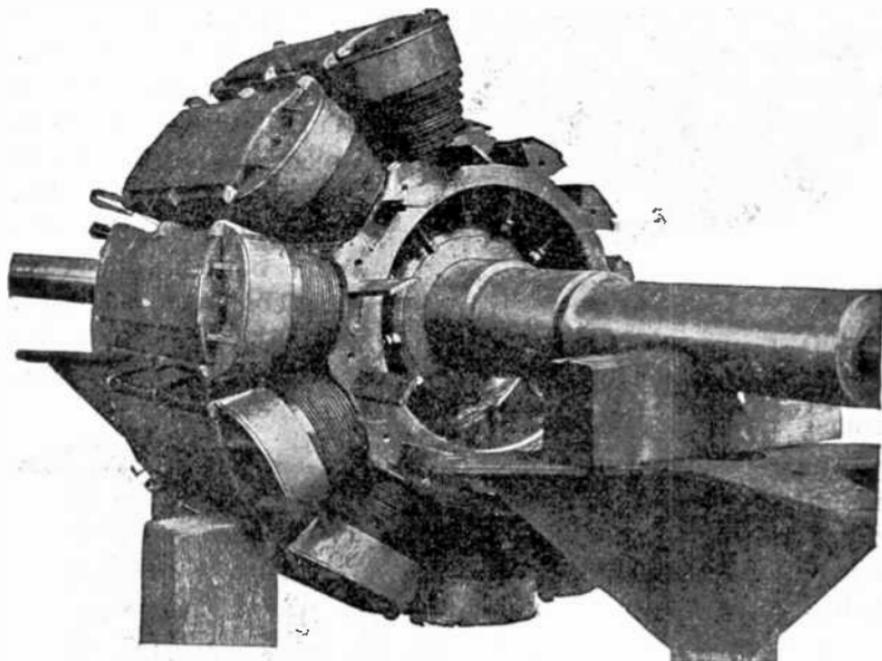
FIG. 2,267.—Wagner revolving field of 300 kilowatt alternator during construction, illustrating the method of attaching the field magnets to the hub by dovetail joints. After the notched ends of the pole pieces are pushed into the grooves in the hub, tapered keys, which are plainly seen, are driven in, thus making a tight joint which will not shake loose.
