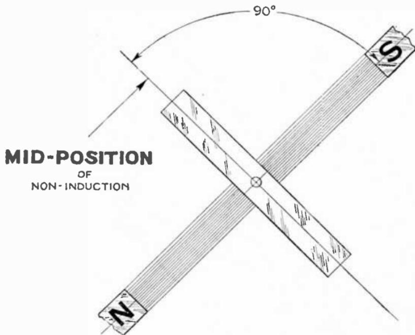
FIG. 2,653.—Squirrel cage principles. 2. Top view of elementary four bar squirrel cage and rotating field (straight line of force) showing *mid-position of non-induction*.
