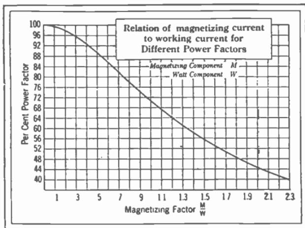
FIG. 2,142.—Power factor curve. By aid of this curve the magnetizing *kva.* can be determined for any power factor. For instance, a line with 60 per cent. power factor and a load of 150 *kw.* requires 150 multiplied by 1.3 = 195 magnetizing *kva.*
