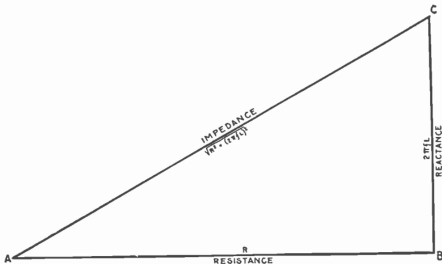
FIG. 2,090.—Graphical method of obtaining the impedance in circuits containing resistance and inductance, having given the resistance and reactance, that is, the ohmic resistance and spurious resistance. With any convenient scale lay off  $AB = \text{resistance}$ , and erect the perpendicular  $BC = \text{reactance}$  (using the same scale); join  $AC$ , whose length (measured with the same scale) will give the *impedance*.
