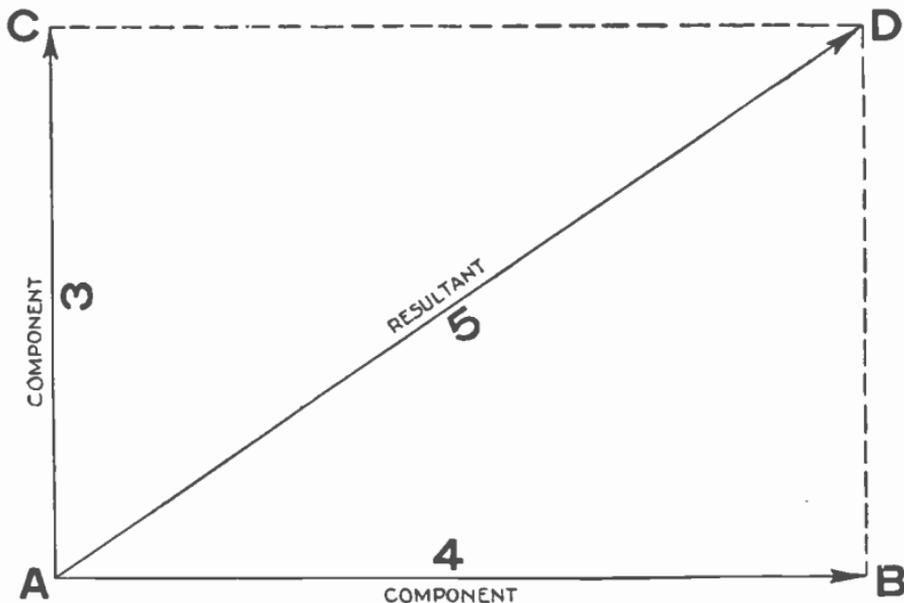
FIG. 2,080.—Parallelogram of forces; method of obtaining the resultant of two components acting at right angles.
