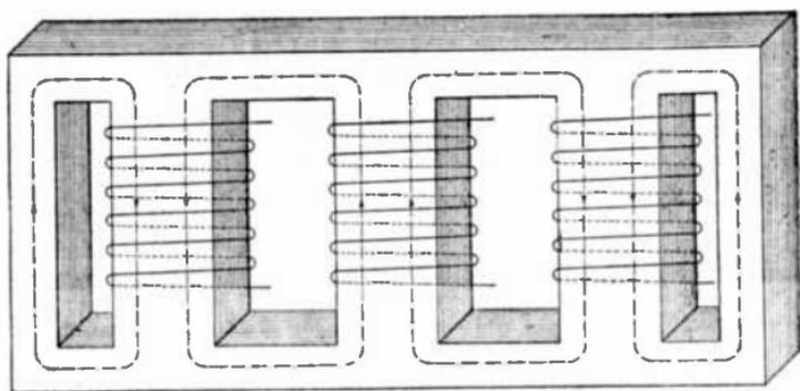
FIG. 2,327.—Diagram showing magnetic circuit of Pittsburgh polyphase transformer.
