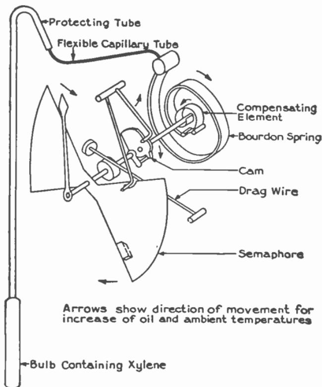
FIG. 2,377.—General Electric thermotel mechanism. *It consists of two thermometers connected in series; one, of the capillary tube type, is immersed in the oil; the other, of the bimetallic type, is located in the external case and corrects for the ambient temperature. The combination actuates the hand and danger signal as shown in the figure.*
