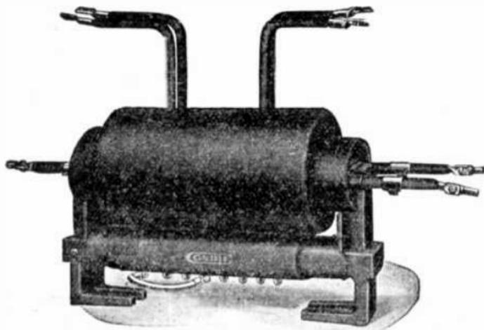
FIG. 2,419.—Condit current transformer maximum volts 15,000; amperes 5 to 800; cycles 25 to 60; double ratio. It may be used in any combination of instruments, trip coils, or relays where the secondary load does not exceed 40 volt amperes with 5 amperes flowing in the secondary circuit at 60 cycles and 20 volt amperes at 25 cycles.
