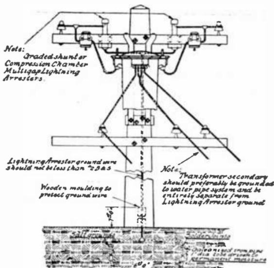
FIG. 2,439.—Installation of a transformer on pole; view showing method of attachment and disposition of the primary and secondary leads, cutouts, etc.
