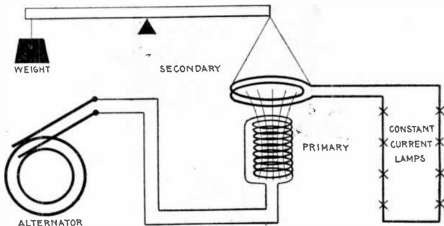
FIG. 2,400.—Elementary diagram illustrating the principles of constant current transformer as used for series arc lighting.
