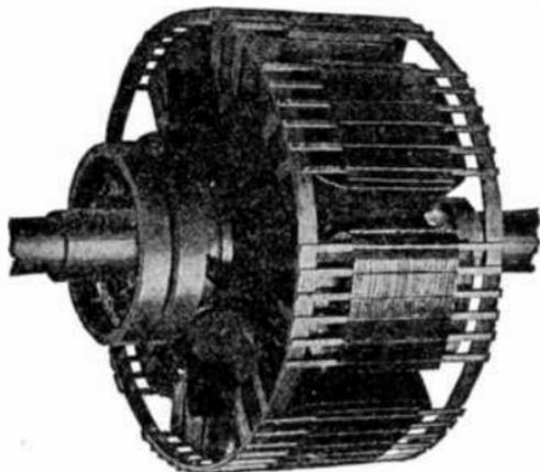
FIG. 2.186.—Revolving field with amortisseur or damper winding of a revolving field 75 *kva.* belted alternator, which prevents hunting and reduces eddy currents in the pole pieces. The copper bars of the amortisseur cage winding are arranged in partially closed slots in the pole pieces.
