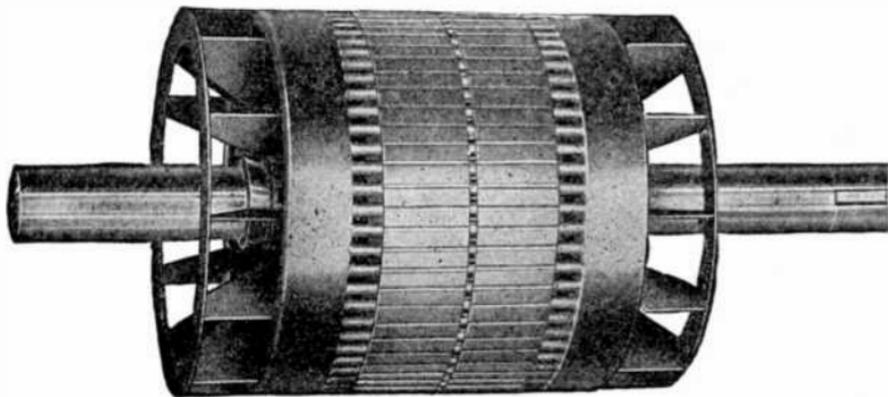
FIG. 2,651.—Century squirrel cage armature. *It consists of 1, shaft; 2, armature laminations; 3, inductor bars; 4, end rings; 5, end flanges; 6, ventilating fans.*
