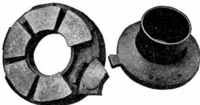
FIGS. 2,242 and 2,243.—Details of Kingsbury thrust bearing for Westinghouse vertical water wheel alternator. The bearing is self-cooled, operating in a bath of oil which is continually circulated by the oiling system.
