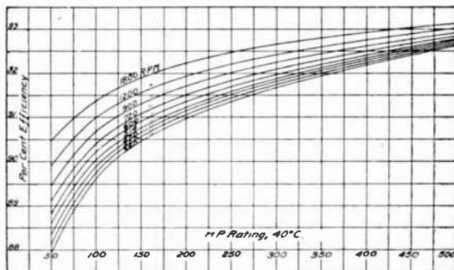
FIG. 2,703.—Efficiency of 60 cycle, squirrel cage induction motors at 100% load, 50 to 500 h.p.
