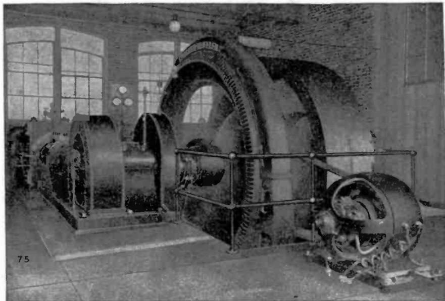
FIG. 2,218.—Crocker-Wheeler 350 kva., slow speed alternator direct connected to a Corliss engine. In front is seen a belted exciter driven from a pulley on the main shaft between the alternator and the large band wheel. The latter serves to give the additional fly wheel effect needed for close speed regulation.
