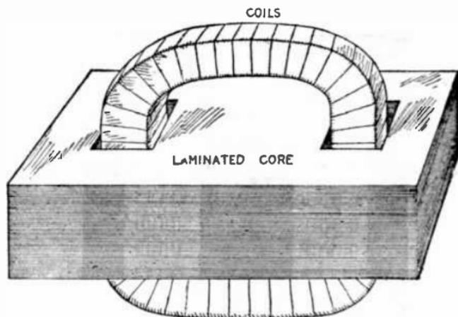
FIG. 2,318.—Shell type transformer. *In construction*, the laminated core is built around and through the coils as shown. For very heavy current ratings at low voltage this type has some advantages with respect to mechanical construction of windings, whereas in other ratings, particularly at high voltages, the core type is to be preferred, both in this respect and with respect to insulation.
