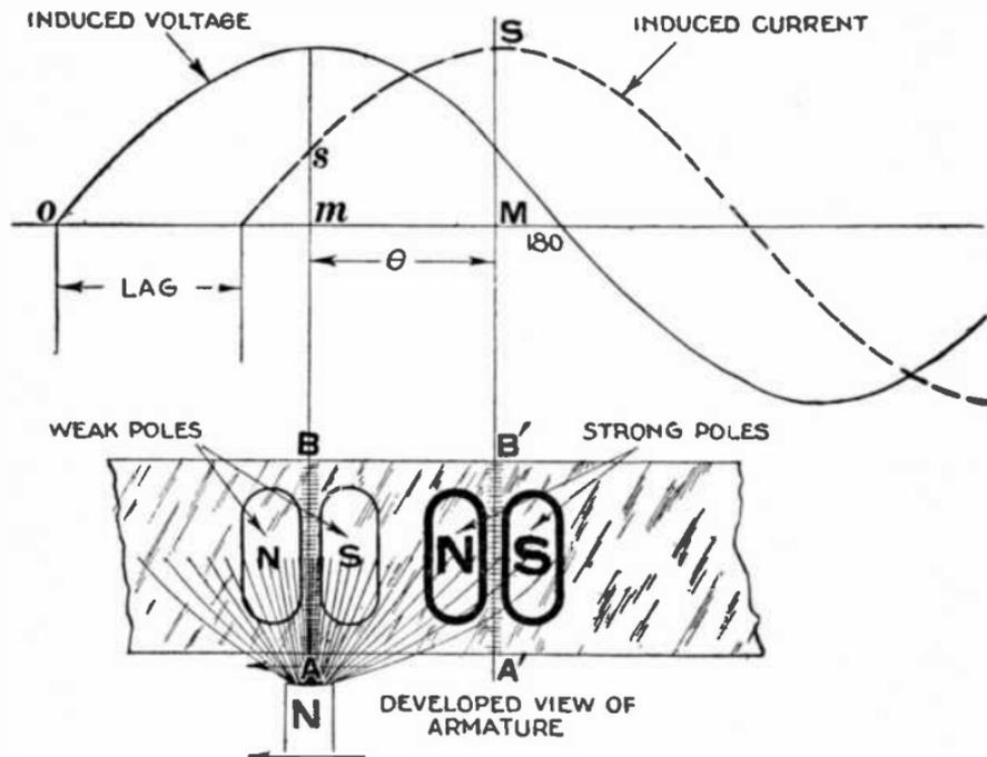
Figs. 2,639 and 2,640.—Pressure and current sine curves and developed view of copper cylinder armature illustrating the effect of lag on the torque in starting a squirrel cage motor.
