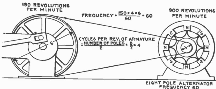
FIG. 1,942.—Diagram of alternator and engine, illustrating frequency. The frequency or cycles per second is equal to the revolution of armature per second multiplied by one-half the number of poles per phase. In the figure the armature makes 6 revolutions to one of the engine; one-half the number of poles =  $8 \div 2 = 4$ , hence frequency =  $(150 \times 4 \times 6) \div 60 = 60$ . The expression in parentheses gives the cycles per minute, and dividing by 60, the cycles per second.
