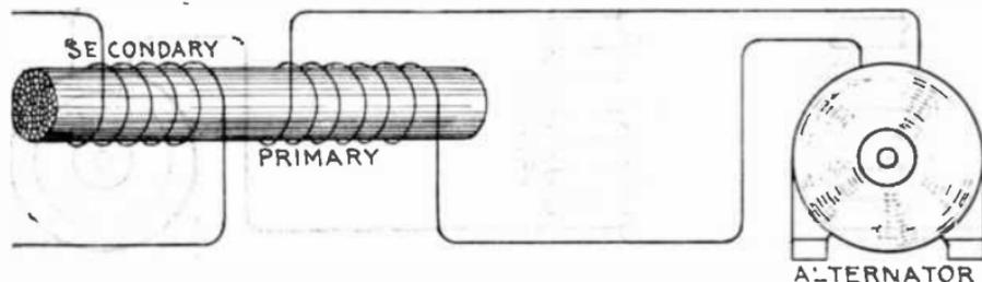
FIG. 2,293.—Diagram of elementary transformer with non-continuous core and connection with single phase alternator. The three essential parts are: primary winding, secondary winding, and an iron core.
