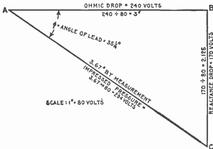
FIG. 2,099.—Diagram for obtaining the impressed pressure of the circuit shown in fig. 2,098.
