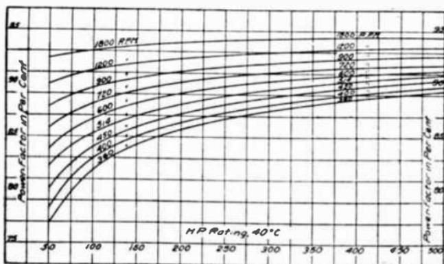
Fig. 2,705.—Power factor of 60 cycle, squirrel cage induction motors at 100% load, 50 to 500 h.p.
