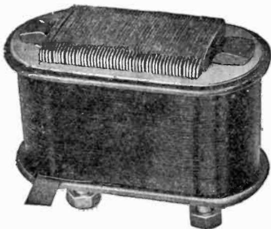
FIG. 2,273.—General Electric field coil, showing another method of winding. In the smaller machines the wire is wound on spools which are slipped over the pole pieces, the latter being built of sheet iron, spreading at the pole face so as to secure not only a wide polar arc for the proper distribution of the magnetic flux, but also to hold the field winding in place.
