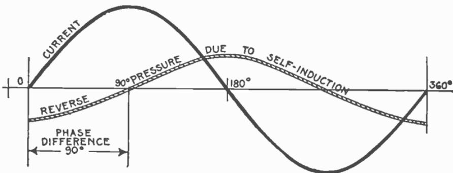
FIG. 2,075.—Sine curves showing phase relation between current and reverse pressure of self-induction. This reverse pressure, being proportional to the rate of change in the current strength, is greatest when the current is at zero value, and zero when the current is maximum, and in phase is 90° behind the current.
