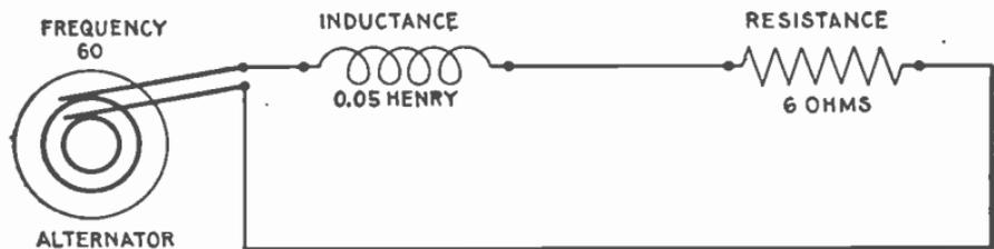
FIG. 2,058.—Diagram of circuit for *example 2*.
