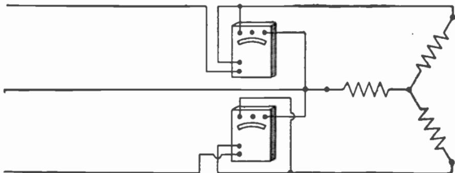
FIG. 2,141.—Watt meter method of three phase power measurement. Two watt meters are required in unbalanced systems as shown in the illustration. The total power transmitted is then the algebraic sum of the readings of the two watt meters. If the power factor be greater than .5, the power is the arithmetical sum, and if it be less than .5, the power is the arithmetical difference of the readings.
