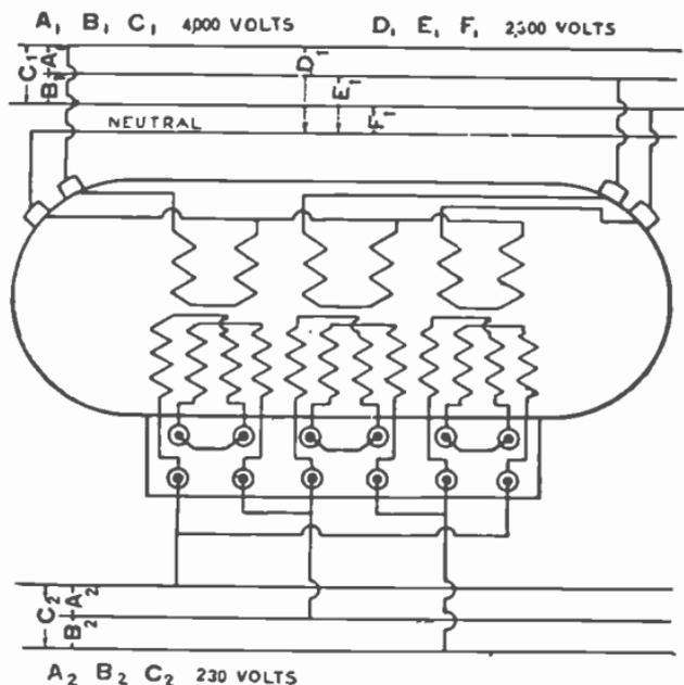
FIG. 2,440.—Pittsburgh connection diagram for three phase 4-wire star primary to three phase 4-wire star secondary.
