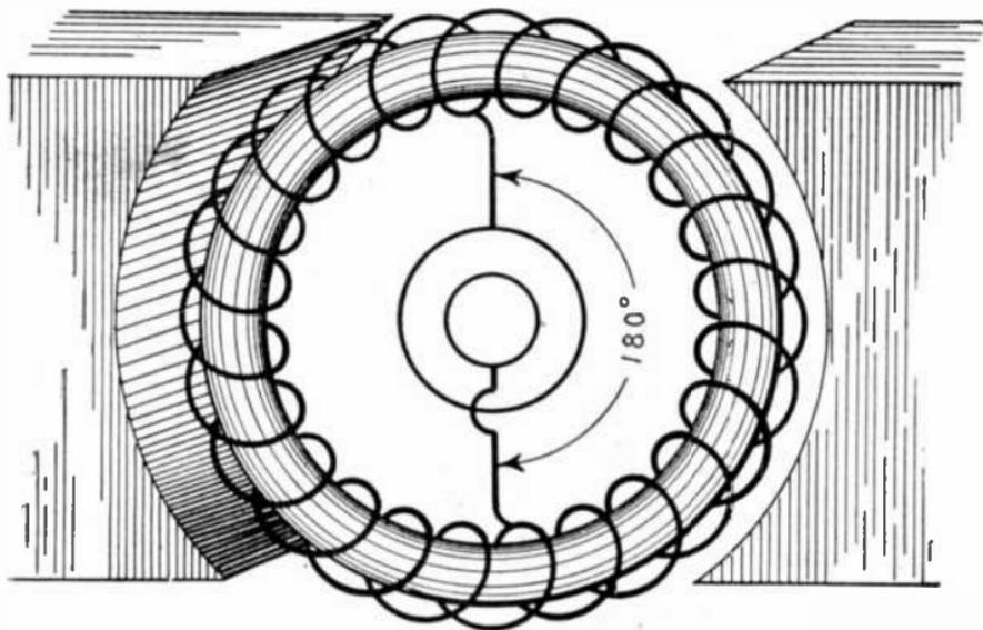
FIG. 2,172.—Ring wound dynamo arranged as alternator by replacing commutator with collector rings connected to the winding at points  $180^\circ$  apart.
