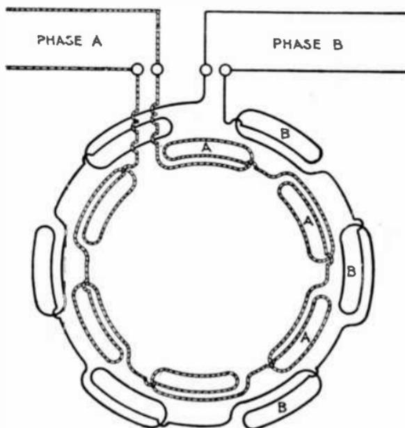
FIG. 2,577.—Diagram of two phase, six pole field winding. There are six coils in each phase as shown. The coils of each phase are connected in series, adjacent coils being joined in opposite senses, thus, for each phase, first one coil is wound clockwise, and the next counter clockwise.
