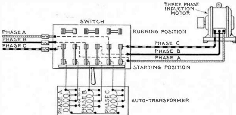
FIG. 2,694.—Auto-transformer or compensator connections for three phase induction motor.
