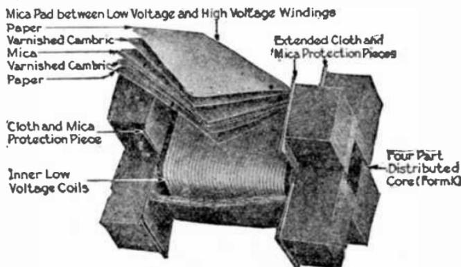
FIG. 2,363.—General Electric partially assembled type H transformer, showing mica insulation. It is necessary to have fireproof insulation in smaller sizes in order to insure protection of the low voltage circuit in case of burnout from abnormal operating condition.
