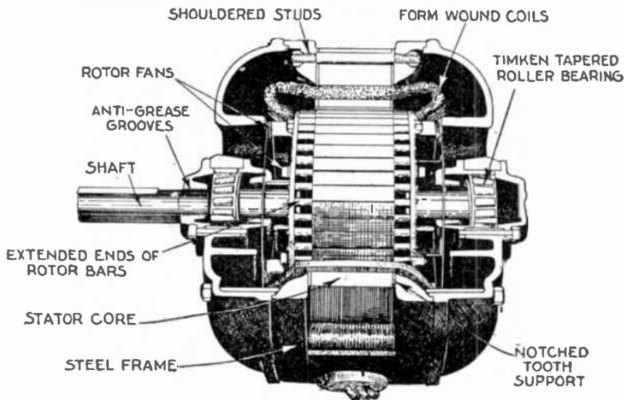
FIG. 2,691.—Sectional view of Allis-Chalmers polyphase squirrel cage induction motor.
