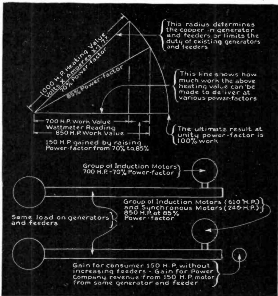
Figs. 2,143 to 2,145.—Typical power factor diagram showing gain by raising the power factor; fig. 2,145 shows benefits to consumer and power company on the basis shown in fig. 2,144.
