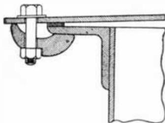
FIG. 2,354.—Pittsburgh method of clamping cover on transformer.
