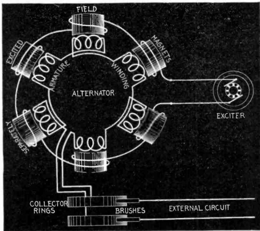
FIG. 2,259.—Diagram of separately excited alternator. The field winding is supplied with direct current, usually at 125 volts pressure by a small dynamo called the "exciter." The latter may be driven by independent power, or by belt connection with the main shaft, and in some cases the exciter is directly connected to the alternator shaft.
