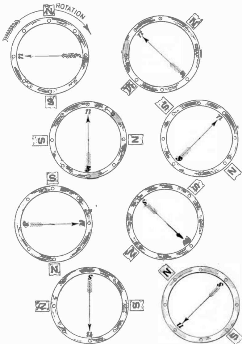
FIGS. 2,657 TO 2,664.—Squirrel cage principles. 4. Elementary eight bar squirrel cage and rotating field for each 45° advance of the field around the squirrel cage showing cycle of polarization.
