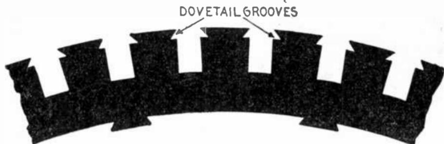
FIG. 2,280.—A style of punching largely used for armature cores. The teeth are provided with dovetail grooves near the circumference. After the coil is inserted in a groove, a wooden wedge is driven in the groove which encloses the coil and secures it firmly in position. This obviates the necessity of bands to resist the centrifugal force acting on the inductors.
