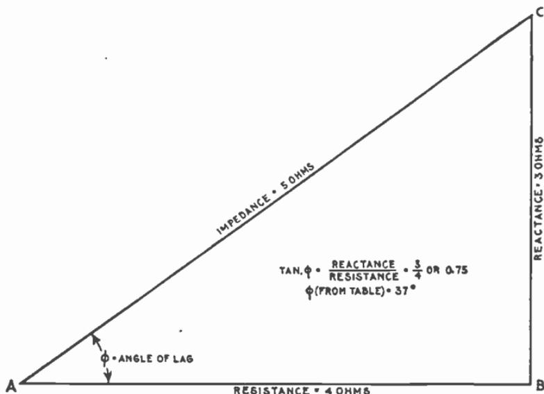
FIG. 2,093.—Diagram showing angle of lag for current containing 4 ohms resistance and 3 ohms reactance.
