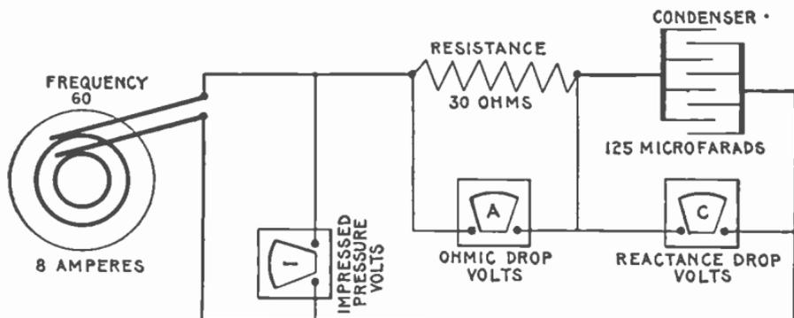
FIG. 2,098.—Diagram of circuit containing a resistance of 30 ohms and capacity of 125 microfarads. The calculation for impressed pressure, ohmic drop, and reactance drop for a current of 8 amperes at frequency 60 is given in the example given below, the diagram for impressed pressure being given in fig. 2,099.
