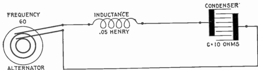
FIG. 2,059.—Diagram of circuit for *example 3*.
