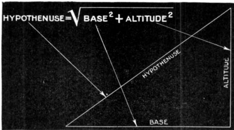
FIG. 2,077.—Graphical representation of the formula:  $\text{hypotenuse} = \sqrt{\text{base}^2 + \text{altitude}^2}$ .
