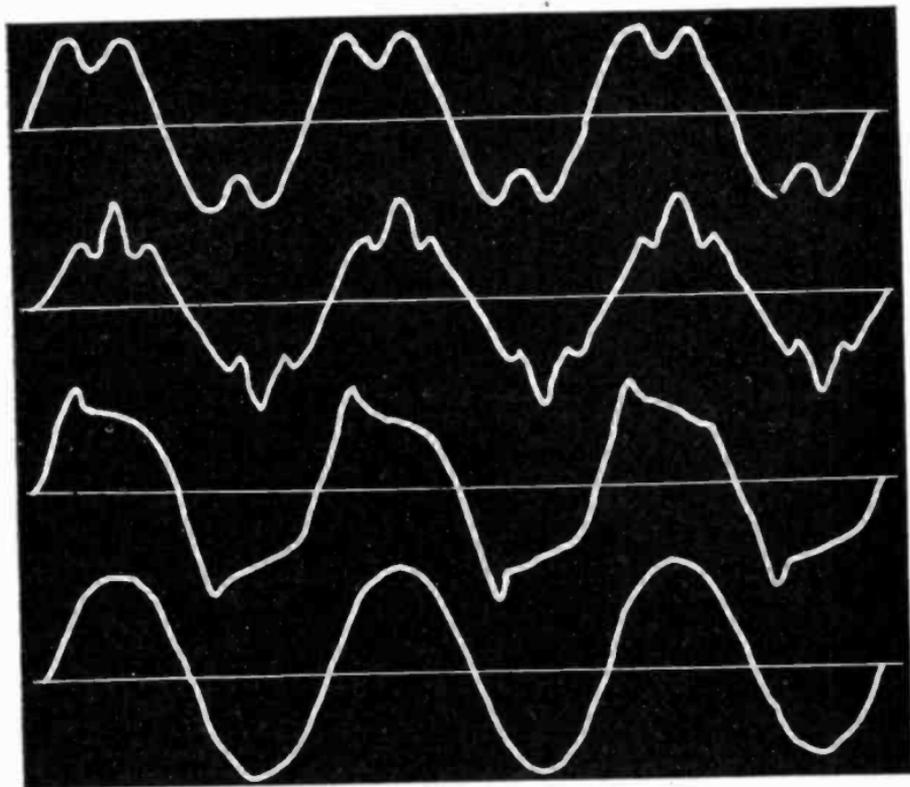
FIGS. 1,962 to 1,965.—Various forms of pressure or current waves. Figs. 1,962 to 1,964 show the general shape of the waves produced by some alternators used largely for lighting work and having toothed armatures. The effect of the slots and shape of pole pieces is here very marked. Fig. 1,965 shows a wave characteristic of large alternators designed for power transmission and having multi-slot or distributed windings.
