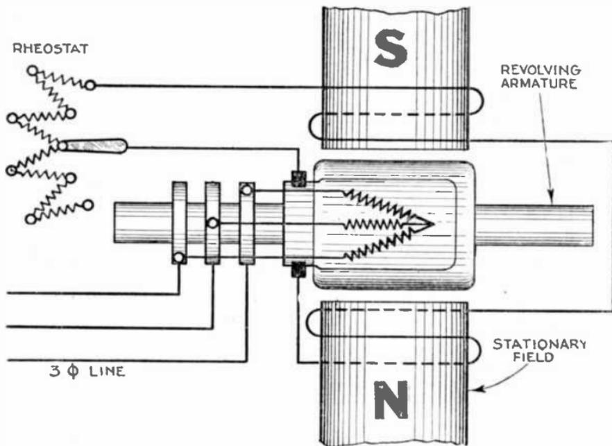
FIG. 2,187.—Connection diagram of General Electric belt driven revolving armature alternator. Illustrations showing construction and general appearance of this machine are shown in the chapter following.
