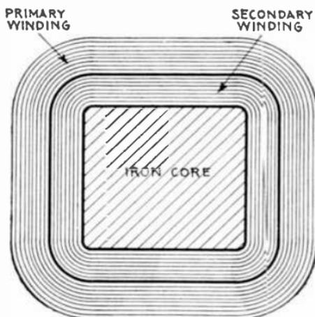
FIG. 2,295.—Cross section showing concentric arrangement of primary and secondary windings on core. One is superposed on the other. This arrangement compels practically all of the magnetic lines created by the primary winding to pass through the secondary winding.
