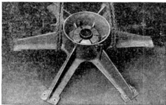
FIG. 2,241.—Westinghouse vertical water wheel alternator upper guide bearing and thrust bearing pot, Kingsbury thrust bearing in place.
