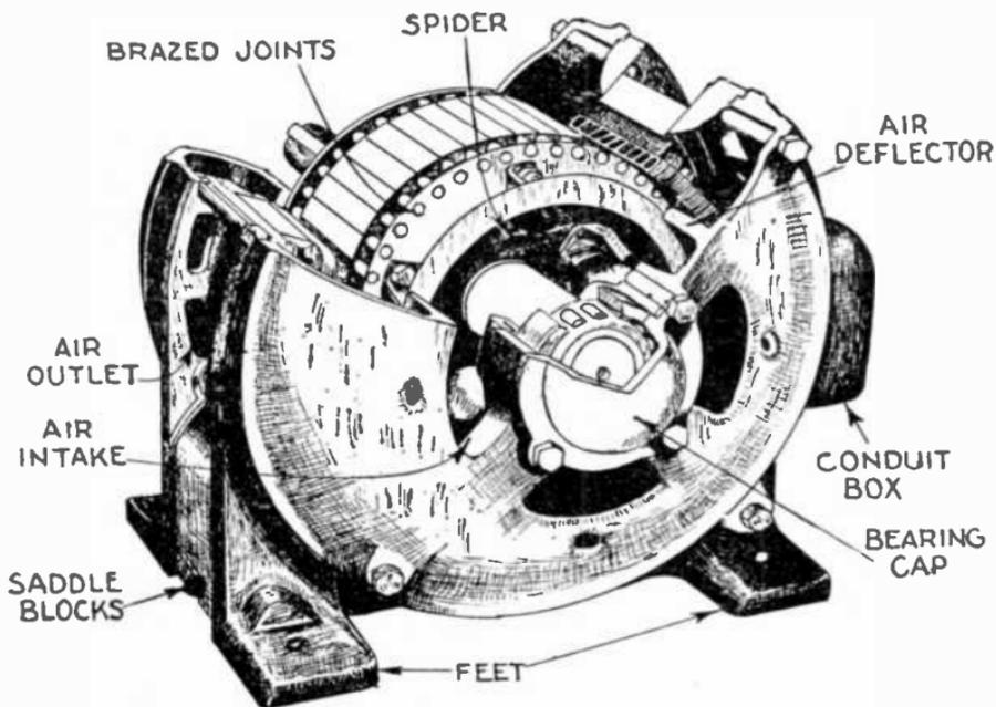
FIG. 2,692.—Sectional view of Allis-Chalmers polyphase squirrel cage induction motor.
