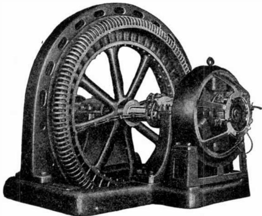
FIG. 2,212.—General Electric alternator with direct connected type MPI exciter mounted on the field shaft at such distance as to permit a pedestal and bearing to be mounted between the exciter and revolving field.
