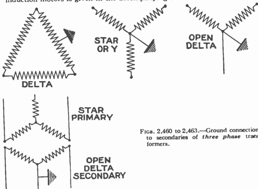
FIGS. 2,460 to 2,463.—Ground connections to secondaries of three phase transformers.
