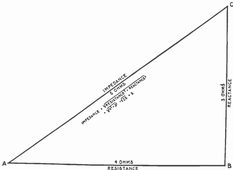
FIG. 2,091.—Diagram for obtaining the impedance of a circuit containing 4 ohms resistance and 3 ohms reactance. •
