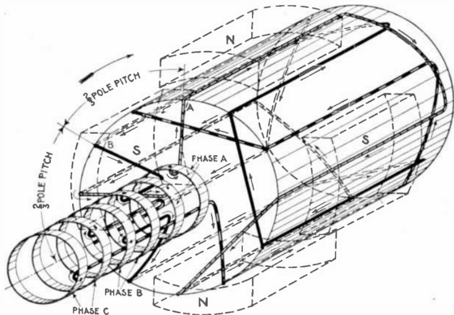
FIG. 2,153.—Elementary four pole three phase alternator. There are three sets of inductors, each set connected in series and spaced on the drum with respect to each other two-thirds pole pitch apart. As shown, six collector rings are used, but on actual three phase machines only three rings are employed, as previously explained. The inductors have distinctive coverings for the different phases. The arrows indicate the direction in which the induced pressures tend to cause currents.
