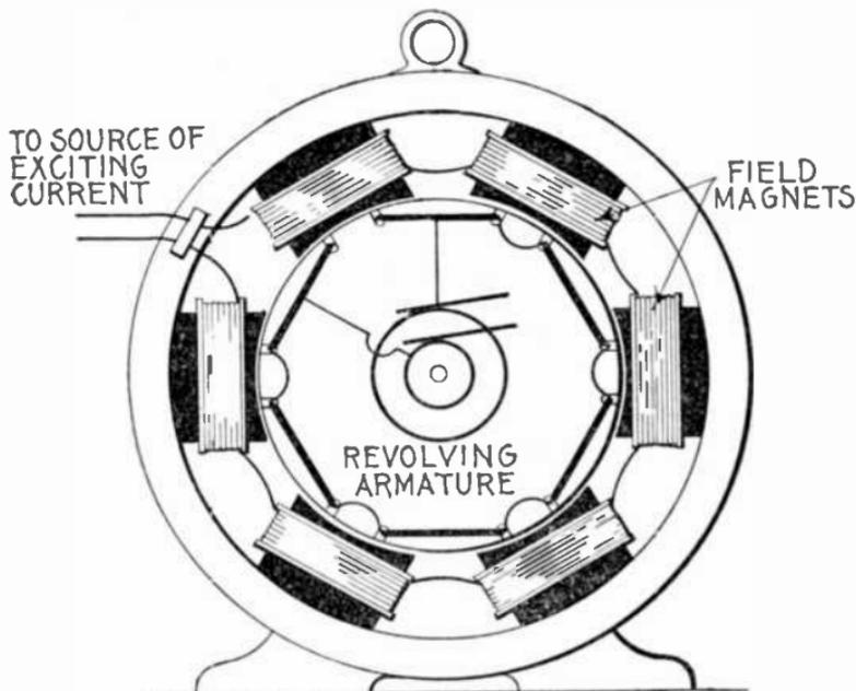
**FIG. 2,170.**—Revolving armature alternator. Revolving armatures are suitable for machines generating current at comparatively low pressure, as no difficulty is experienced in collecting such current. Revolving armature alternators are also suitable for small power plants, isolated lighting plants, where medium or small size machines are required.
