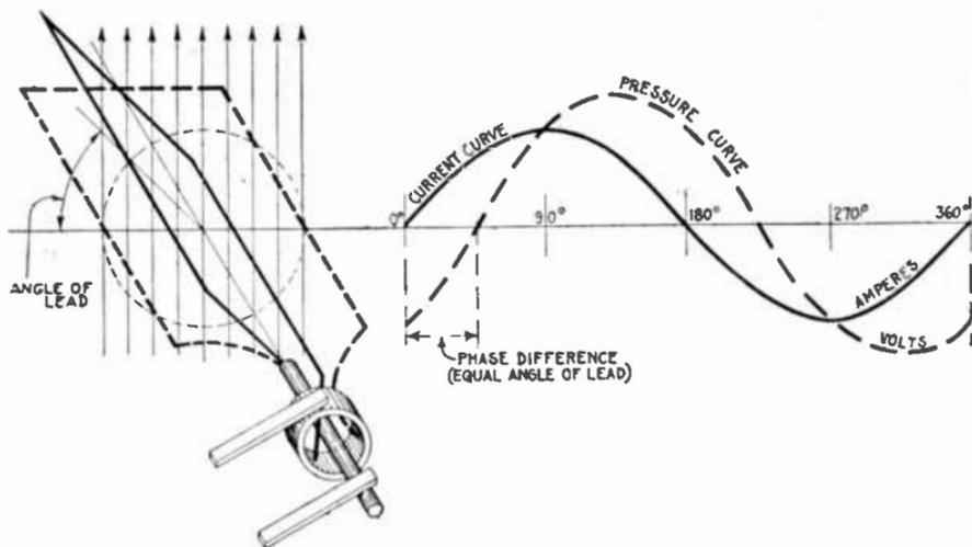
FIG. 2,037.—Pressure and current curves illustrating *lead*. The effect of capacity in a circuit is to cause the current to rise to its maximum value sooner than it would otherwise do; capacity produces an effect exactly the opposite of inductance. The phase relation between current and pressure with current leading is shown graphically by the two armature positions in full and dotted lines, corresponding respectively to current and pressure at the beginning of the cycle.
