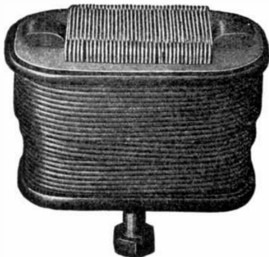
FIG. 2,271.—General Electric field coil showing one method of winding. The field coils on the larger machines consist of a single strip of flat copper, wound on edge as shown, so that the surface of every turn is exposed to the air for cooling. The flat sides of the copper strip rest against each other and the entire coil forms a structure of great solidity which can be easily removed for inspection and repair.
