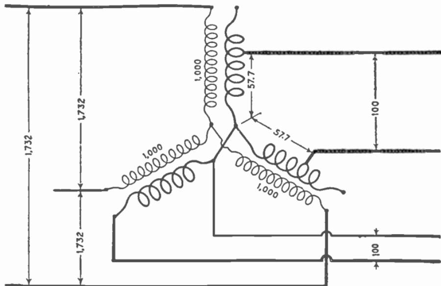
FIG. 2,471.—Three phase to two phase transformation with three star connected transformers. Two of the secondary windings are tapped at points corresponding to 57.7% of full voltage; these two windings are connected in series to form one secondary phase of voltage equal to that obtained by the other full secondary winding.
