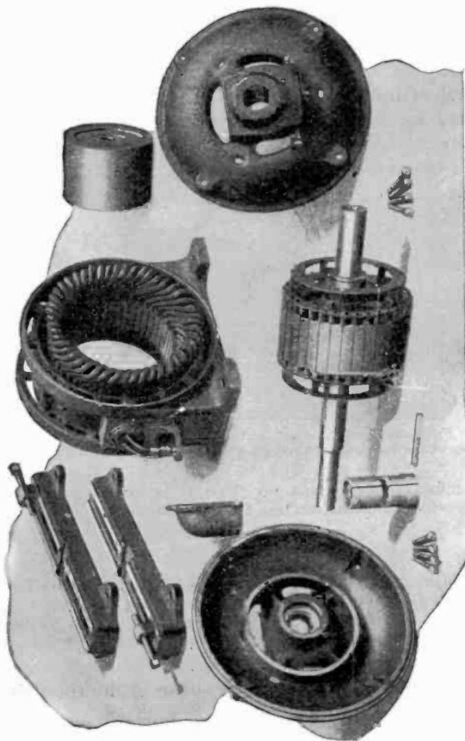
FIGS. 2,673 to 2,690.—Disassembly of Allis-Chalmers type AR belted squirrel cage induction motor showing field armature, etc.
