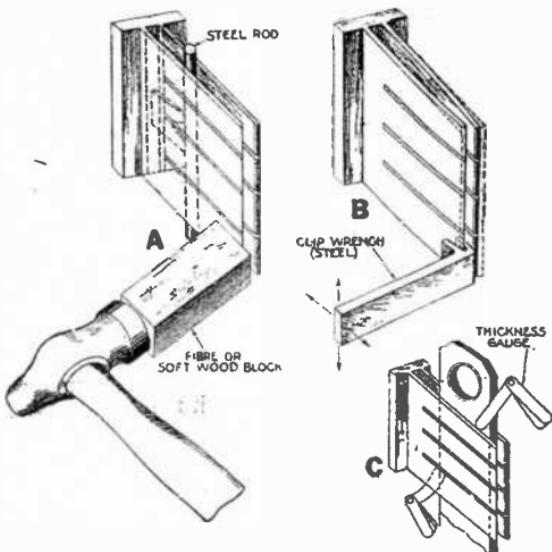
Figs. 4,047 to 4,049.—Methods of adjusting knife switch jaws.
