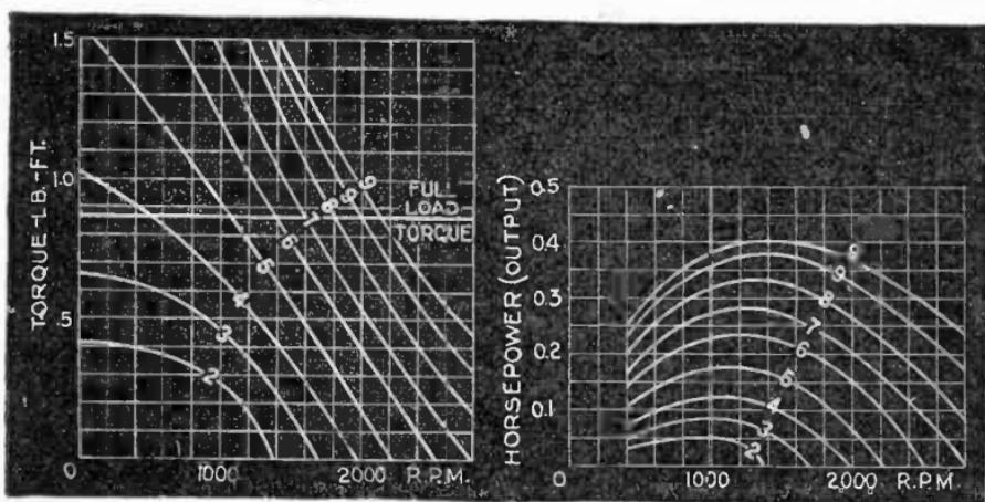
torque curves of a  $\frac{1}{4}$ -h.p. motor with the brushes set a distance corresponding to 2,3,4 etc. bars from neutral, as indicated by the numerals. However, it should be understood that the brush positions are not limited to these settings. Fig 3,013 gives speed output curves at the same brush settings. By the aid of these curves the load on the motor can be found. While these curves are accurate only for one rating, they indicate the general characteristics of all type L.K. motors.
