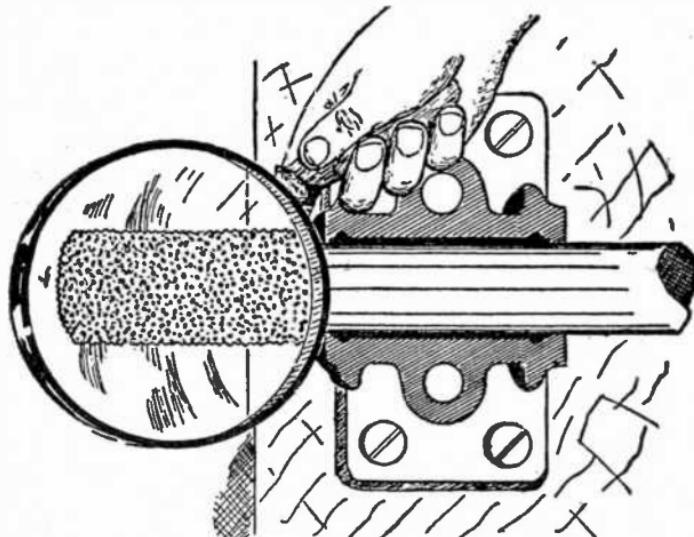
FIG. 2,947.—Magnified view of a shaft showing its rough granular structure. *In operation*, these minute irregularities interlock and act as a retarding force, or *frictional resistance*. Hence, the necessity for lubrication which prevents actual contact by presenting a thin intervening film against which the surfaces rub. The magnifying glass shown above is simply suggestive of magnification, in fact, to see the rough granular structure the shaft would have to be viewed under a microscope.
