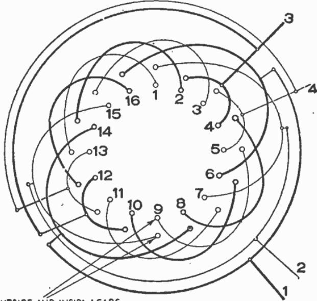
FIG. 3,250.—2 phase, 8 pole, 4 circuit. Connections between coil groups only.
