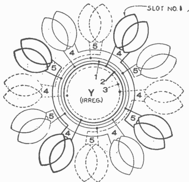
FIG. 3.258.—3 phase, 4 pole, 2 circuit Y (irregular).
