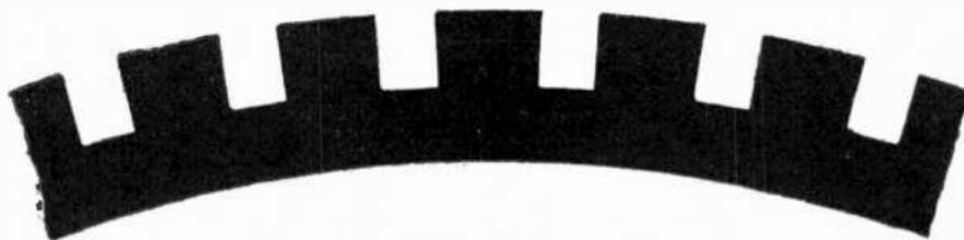
FIG. 3,132.—Style of armature core stamping used with bar wound machines. This construction, since there are no indentations in the teeth for wedges, makes it necessary to provide bands to hold the bars in place.
