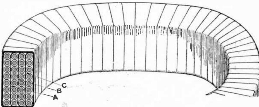
FIG. 3,121.—Method of winding a coil containing a large number of turns, when there is considerable difference of pressure between the layers. In such cases to guard against short circuits or breakdown of the insulation, each layer of turns is insulated from the next layer by the insulating strips A, B, C, in addition to the regular insulation around each wire. After the coil is made up it is wound with insulating tape, varnished and baked.
