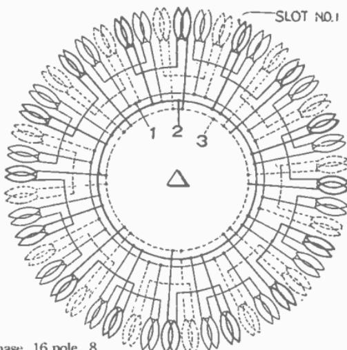
FIG. 3,290.—3 phase, 16 pole, 8 circuit Delta.
