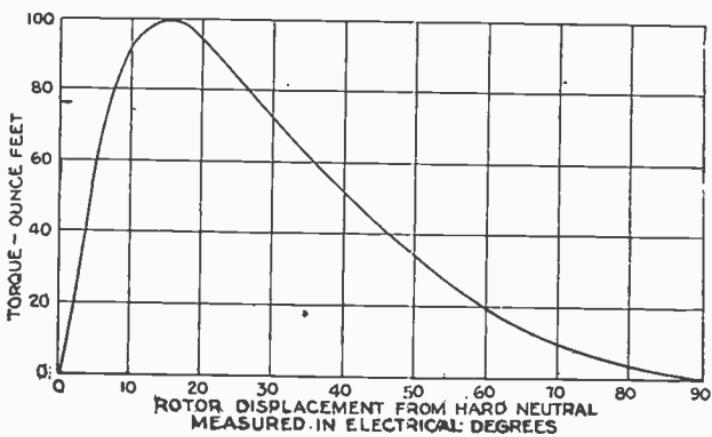
FIG. 3,003.—Locked torque of repulsion motor.
