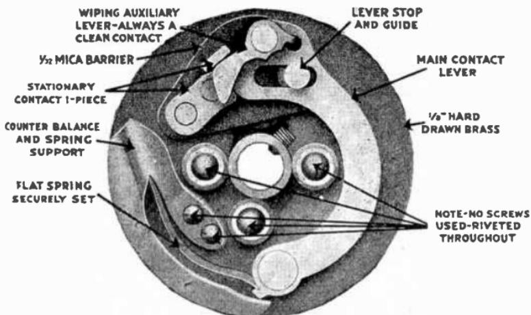
FIG. 2,851.—Janette split phase induction motor cut out switch for making and breaking the starting circuit. There is an auxiliary contact which gives a wiping effect both in opening and closing the switch. Obviously the contact points are always clean.
