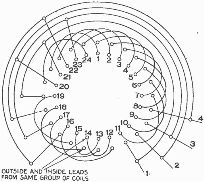
FIG. 3,252.—2 phase, 12 pole, 3 circuit. Connections between coil groups only.
