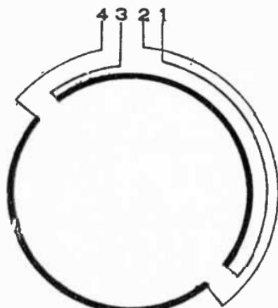
FIG. 3,207.—Diagram showing connections for a 2 pole repulsion-induction motor.
