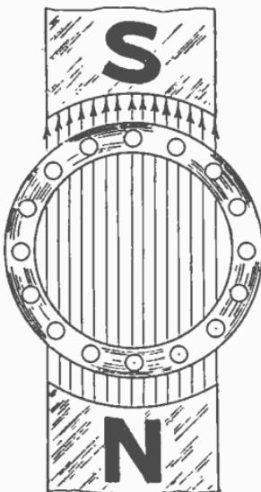
Figs. 2,818 and 2,819.—Diagrams illustrating a single phase or reciprocating field. A motor is not self starting with a reciprocating field because the magnetization alternates in reversed directions.
