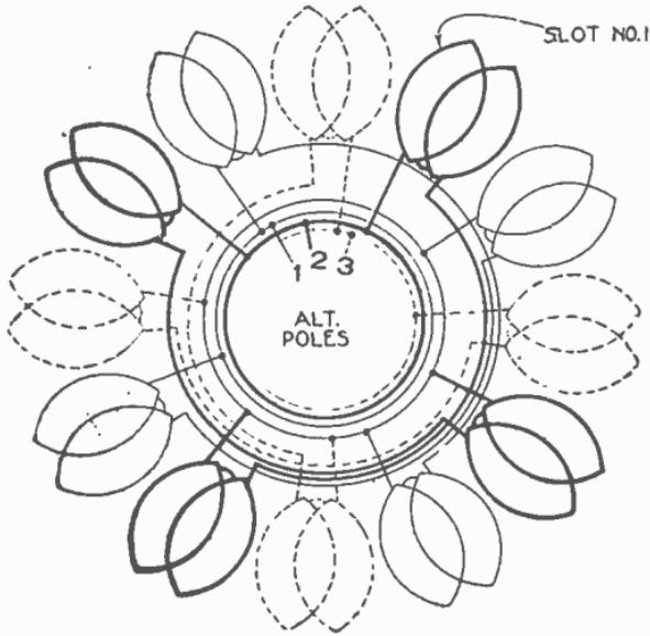
FIG. 3.259.—3 phase, 4 pole, 2 circuit, alternate poles.
