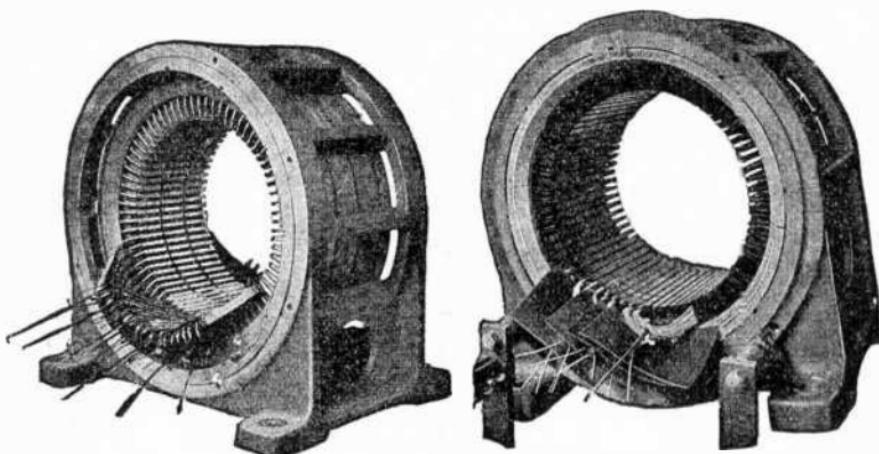
FIGS. 2,787 and 2,788.—*General Electric slip ring motor construction 1.* Partially wound fields showing exposed laminations, oiled paper and linen slot insulation, form wound coils wrapped with "assembly" or (sacrifice) tape which affords protection while installing, and a perfect fit in the slots.
