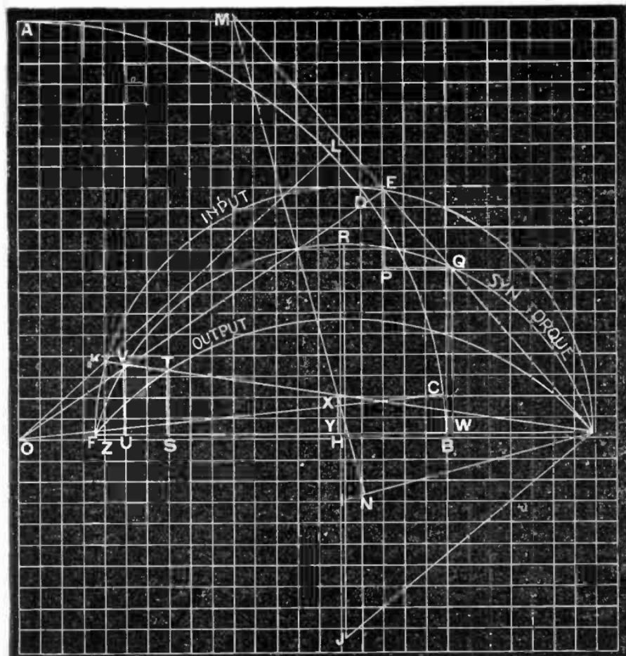
FIG. 2,817.—Heyland diagram for calculating horse power output, *kva* input, amperes per terminal, per cent power factor for different loads, per cent inrush at starting under full voltage, per cent torque at starting, maximum or pull out torque, per cent slip of motor at different loads, and actual *r.p.m.* of motor at different loads.
