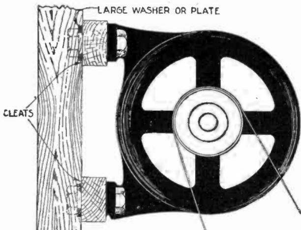
FIG. 3,938.—Method of mounting motor on wooden wall.
