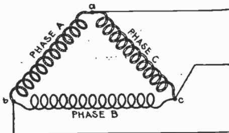
FIG. 3,163.—Diagram of three phase mesh grouping, commonly called delta grouping owing to its resemblance to the Greek letter  $\Delta$ . The voltage at the terminals is equal to the voltage in one phase, and the current in each line is equal to the vector sum of the currents in two phases, that is, it is equal to  $\sqrt{3}$  multiplied by the current in one phase.
