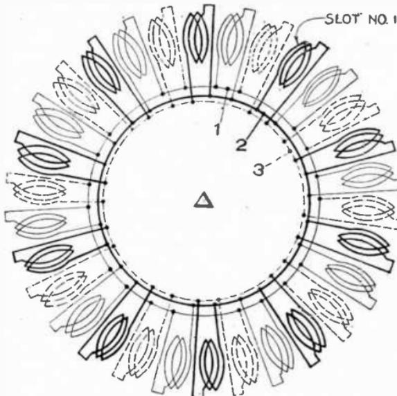
FIG. 3,275.—3 phase, 10 pole, 10 circuit Delta.
