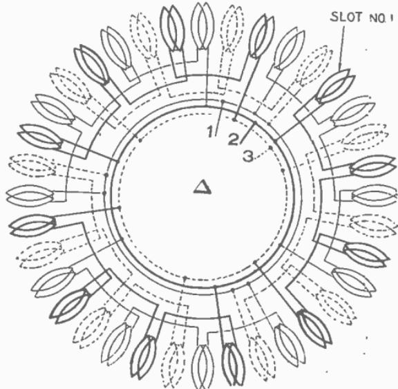
FIG. 3,283.—3 phase, 12 pole, 3 circuit Delta.
