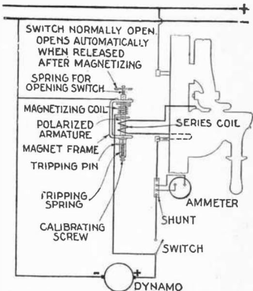
FIG. 4,191.—Connection diagram for General Electric reverse current air circuit breaker for capacity up to 600 amperes.
