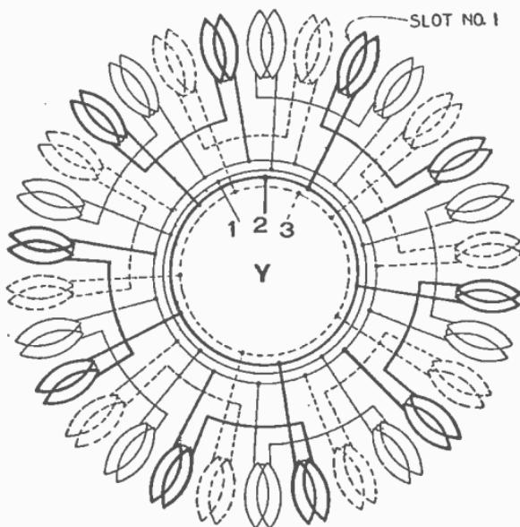
FIG. 3,272.—3 phase, 10 pole, 5 circuit, Y.
