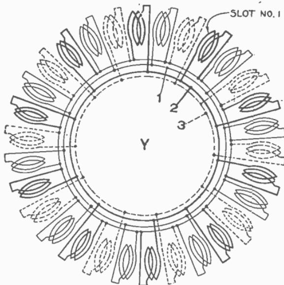
FIG. 3,274.—3 phase, 10 pole, 10 circuit Y.
