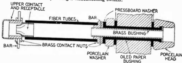
FIGS. 4,045 and 4,046.—*Bus transfer plug switch.* The method of supporting the contact farthest from the panel consists of a porcelain pillar of the same height as the receptacle, clamped to a brass connecting or bus bar which in turn is fastened to the receptacle.
