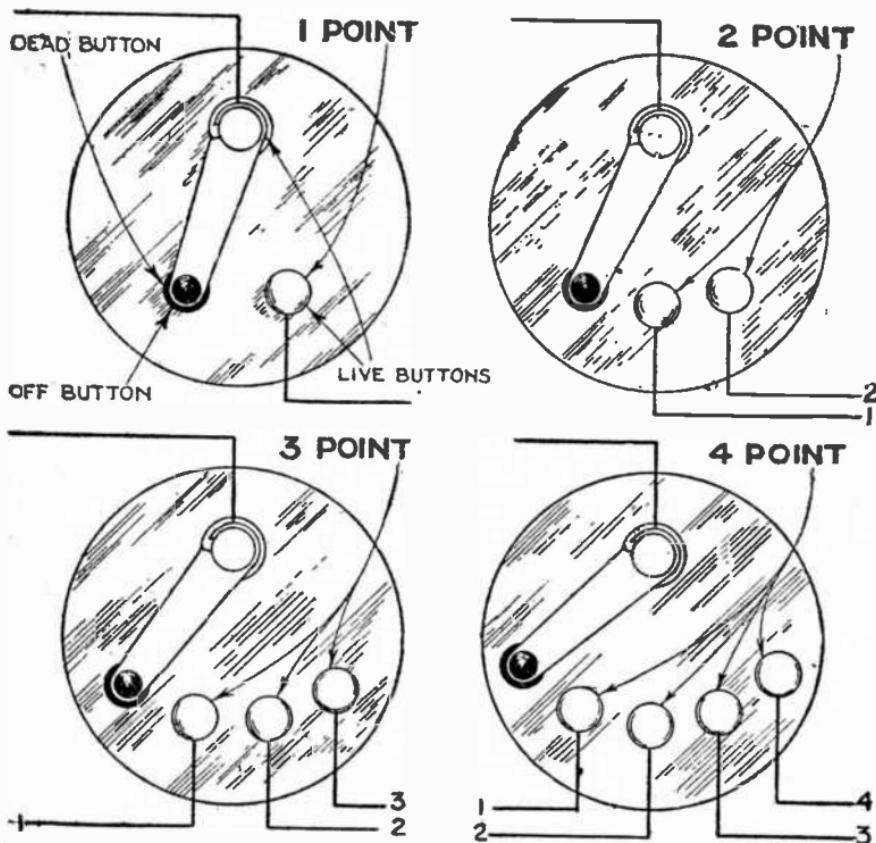
Figs. 3,977 to 3,980.—Lever switches illustrating the term "*point*." Here are shown 1, 2, 3 and 4, point switches controlling 1, 2, 3 and 4 circuits respectively. The use of these switches is explained at the end of this chapter.
