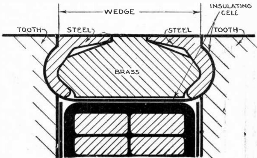
FIG. 3,214.—Cross section through a magnetic wedge.
