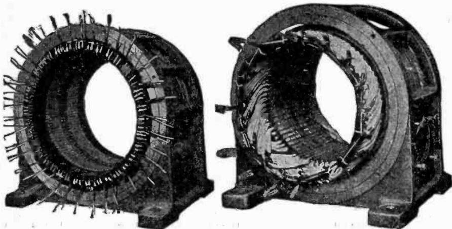
Figs. 2,796 and 2,797.—**General Electric slip ring motor construction 2.** Field windings being connected. Views show partially closed slots, heavy fibre and hard wood wedges, end shields, etc.
