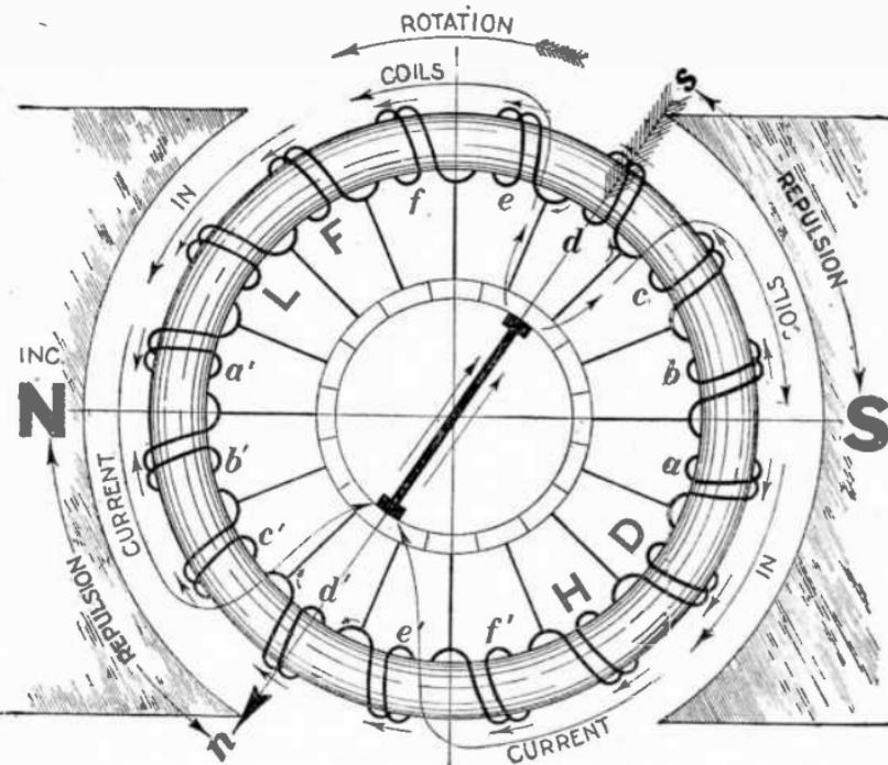
FIG. 2,977.—Ring armature in a.c. field with brushes shifted on other side of live neutral showing reversal of rotation. Compare this diagram with fig. 2,976.
