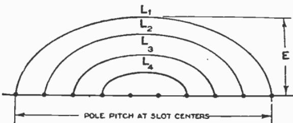
FIG. 3,179.—Diagram illustrating method of determining length of loop.
