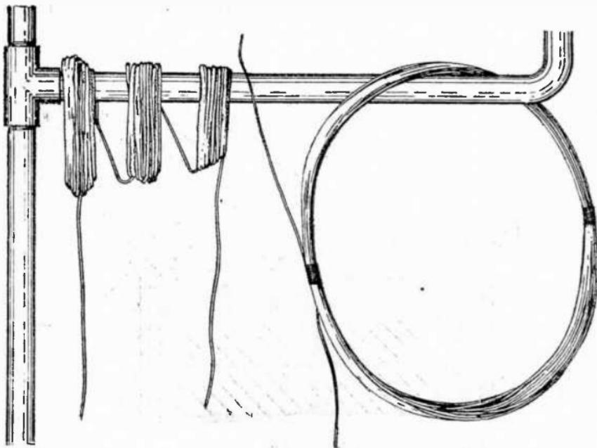
FIG. 3,215.—Typical mould wound and skein wound coils.
