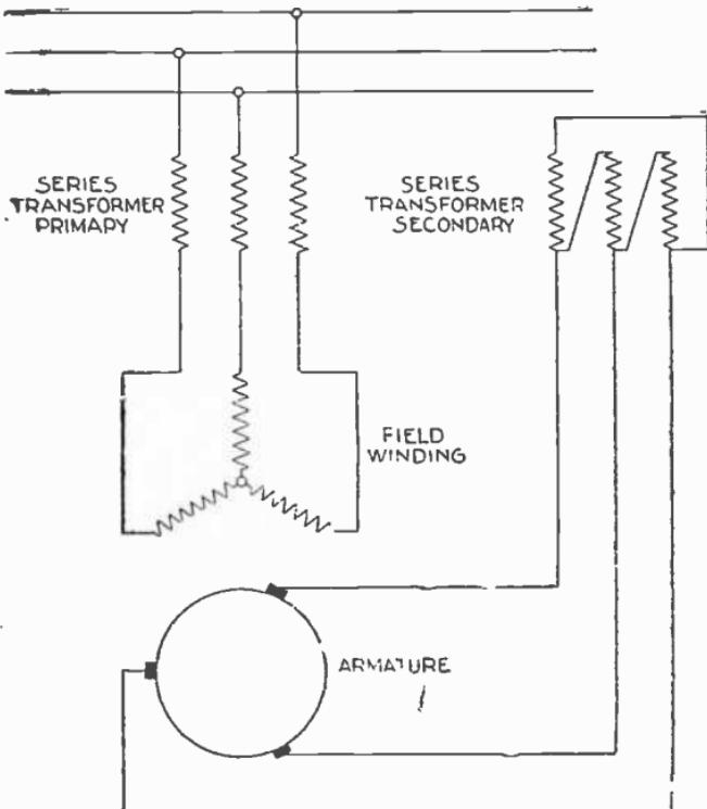
FIG. 3,010.—Connections of a three phase brush shifting series motor. A series transformer is generally used to step down the voltage for the armature as low voltage is necessary to good commutation. The secondary of this transformer is connected for three phases and the armature has three sets of brushes per pole pair. The transformer, by its ability to become saturated, limits the no load speed of the motor to a safe value, which is usually about 150 per cent normal.
