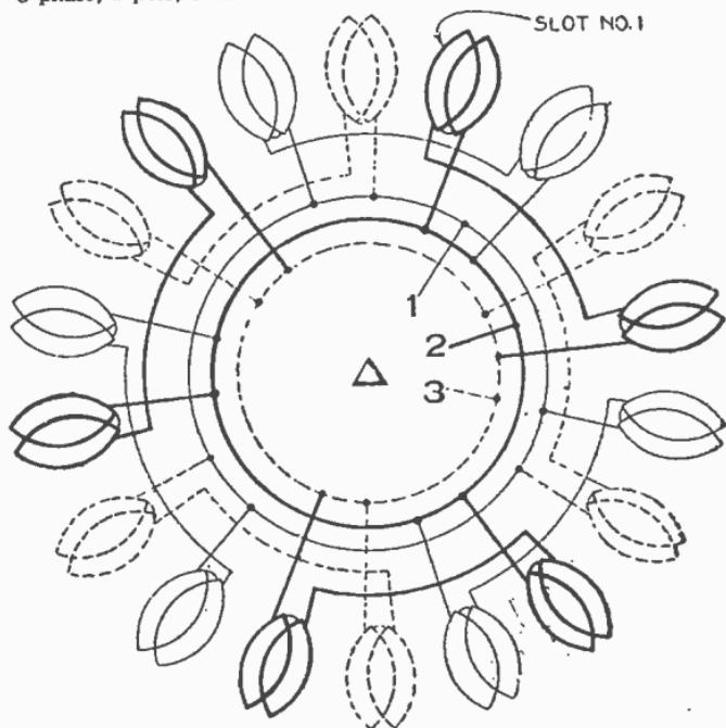
FIG. 3,265.—3 phase, 6 pole, 3 circuit Delta.
