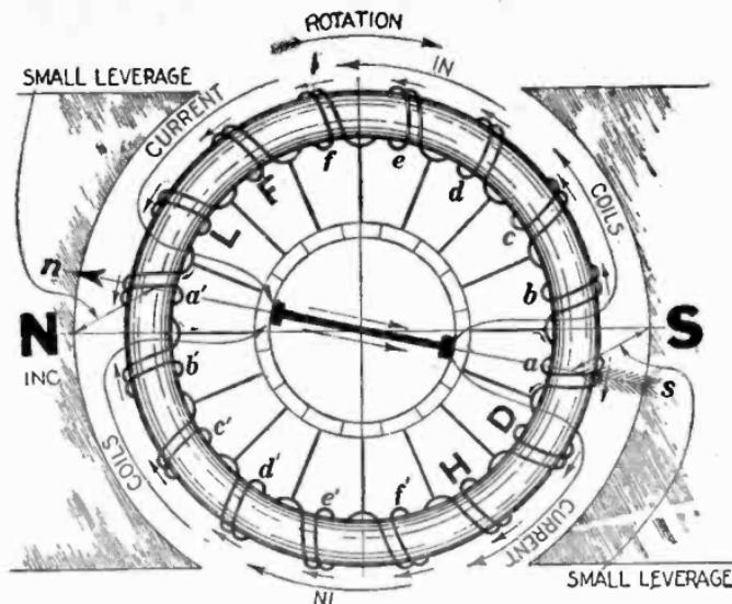
FIG. 2,975.—Ring armature in a.c. field with short circuited brushes shifted *close to the live neutral* showing weakening of torque (as compared with torque in fig. 2,974) due to decrease of magnetic leverage.
