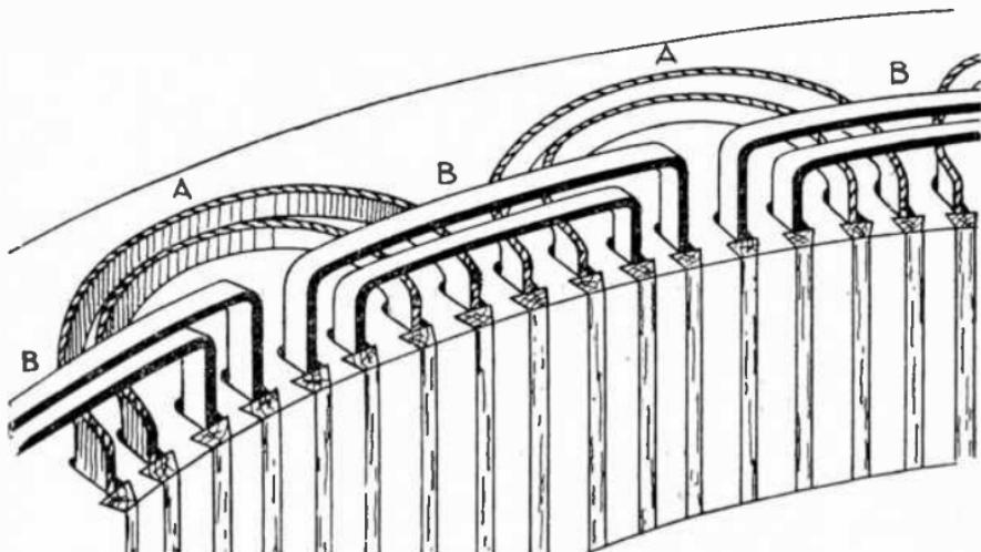
FIG. 3,138.—Treatment of coil ends in two phase, two range concentric chain windings. In this arrangement *straight out* B and *bent up* A coils are used which are placed on the armature as is clearly shown in the illustration.
