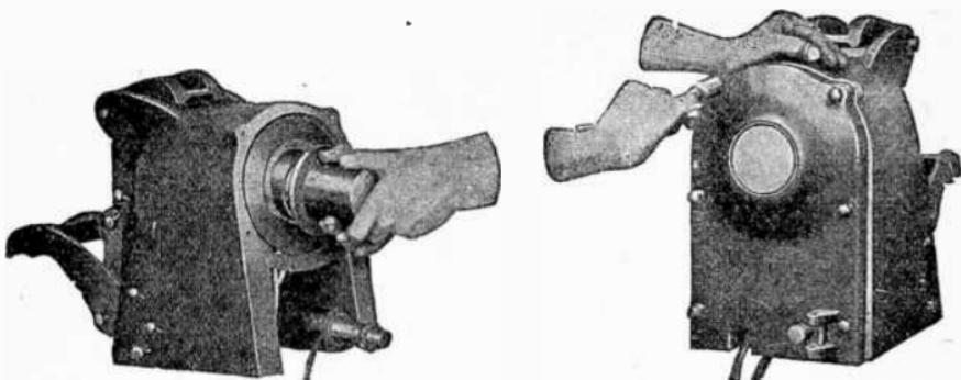
FIG. 4,171.—How to assemble an air circuit breaker 19.—Attaching the plungers and collars.
