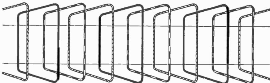
FIG. 3,143.—Diagram showing chain or nested winding. In this method of winding the coils are all similar with long and short sides. It obviates the extra cost of making coils of several different shapes. The diagram represents a winding for one slot per pole per phase.
