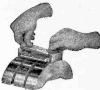
FIG. 4,135.—*How to assemble an air circuit breaker 5.* Method of attaching overload magnet frame.
