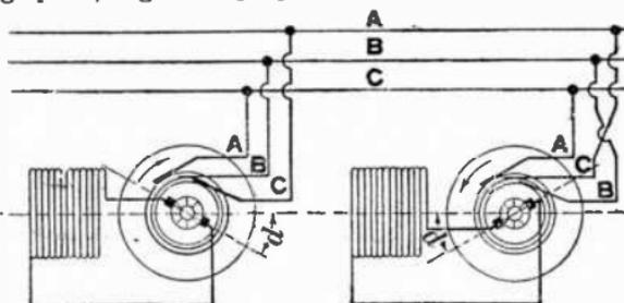
FIG. 3,017.—Fynn-Weichsel motor running connections. To reverse the direction of rotation reverse two line wires and shift commutator brushes.
