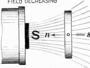
Figs. 2,925 to 2,928.—*Repulsion motor principles 6.* When the plane of a pivoted copper ring is at right angles to the axis of an a.c. magnet there is no tendency for the ring to turn.
