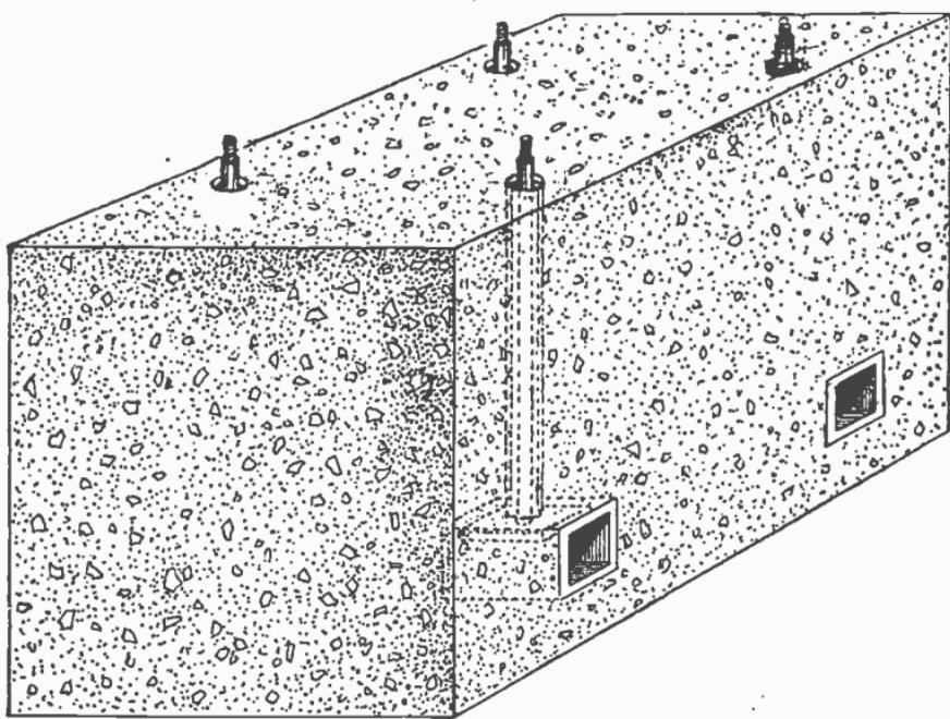
FIG. 3,937.—Concrete foundation, showing method of installing the anchor bolts.
