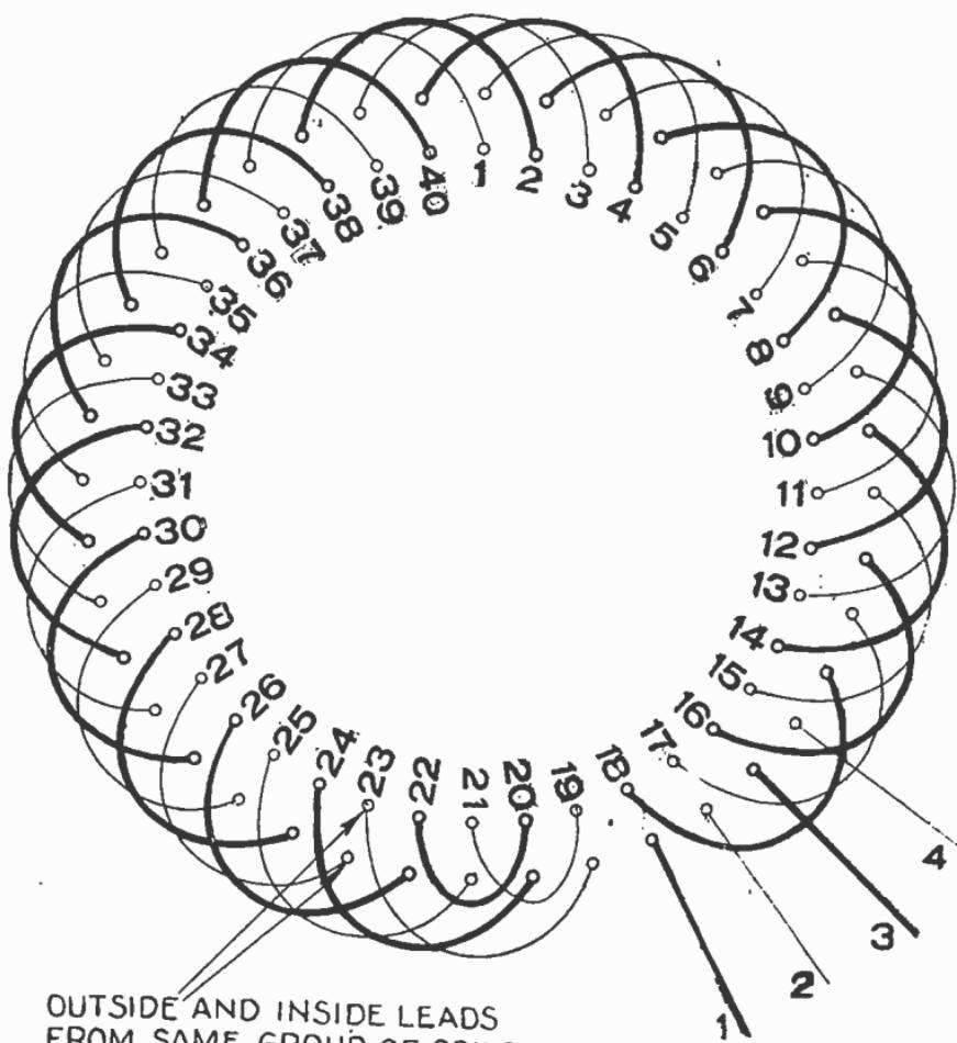
FIG. 3,253.—2 phase, 20 pole, 1 circuit Connections between coil groups only.
