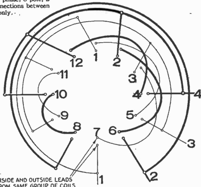
FIG. 3,248.—2 phase, 6 pole, 3 circuit. Connections between coil groups only.
