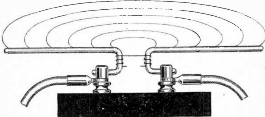
FIG. 4,019.—Flat horizontal horn break fuse.
