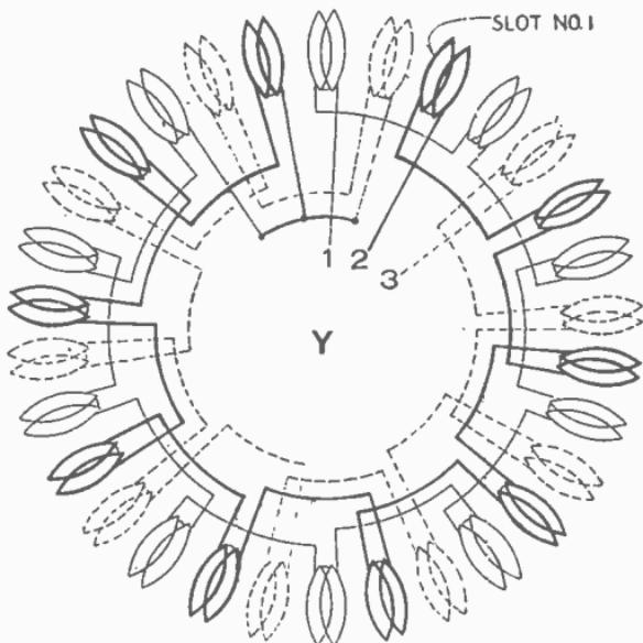
FIG. 3,268.—3 phase, 10 pole, 1 circuit Y
