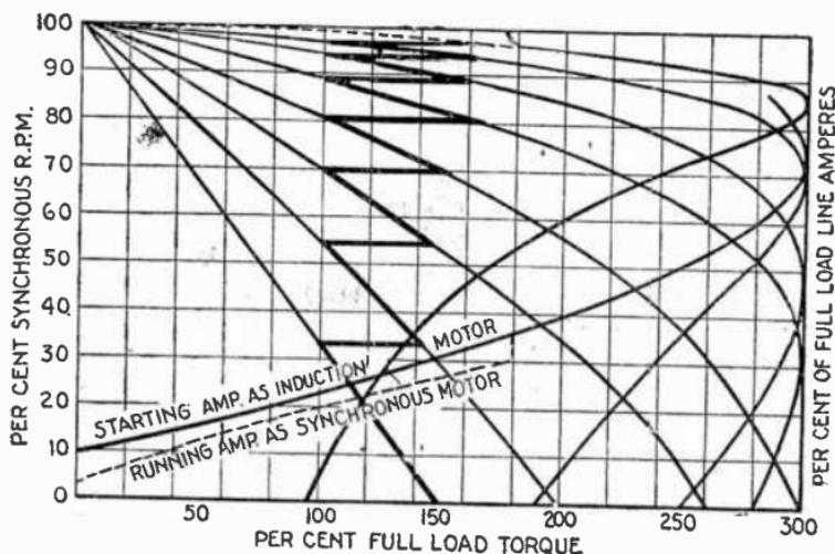
FIG. 3,016.—Fynn-Weichsel motor starting characteristics. *It will be noted* that the average current required during the starting period at full load torque is equal to 1 to 1.5 times normal full load running current.
