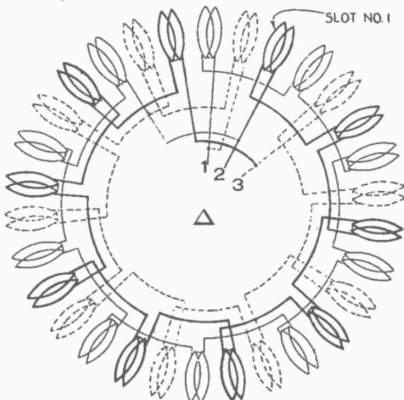
FIG. 3,269.—3 phase, 10 pole, 1 circuit Delta.
