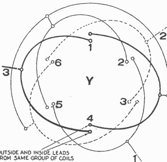
FIG. 3,256.—3 phase, 2 pole, 2 circuit Y.
