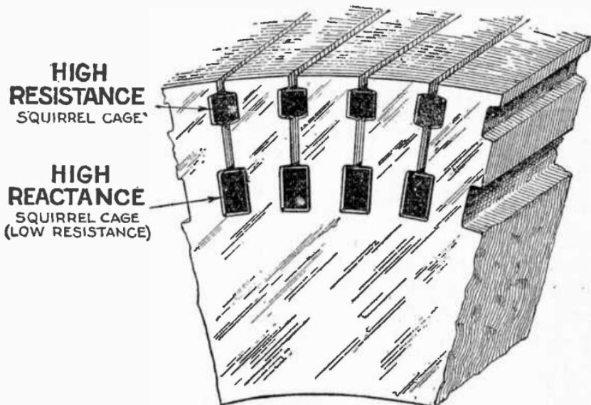
**Fig. 2,762.**—Detail of double squirrel cage windings showing placement of the high resistance and high reactance (low resistance) squirrel cages.
