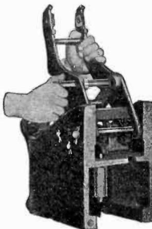
FIG. 4,167.—*How to assemble an air circuit breaker 16.* Connecting the links to the brush support.
