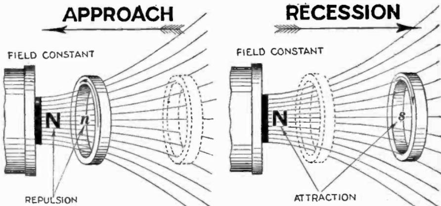
Figs. 2,919 and 2,920.—**Repulsion motor principles 3.** LENZ LAW: The approach or recession of a copper ring from a magnet pole induces a current in the ring in such direction as to set up a magnetic field which opposes the motion which produces it.
