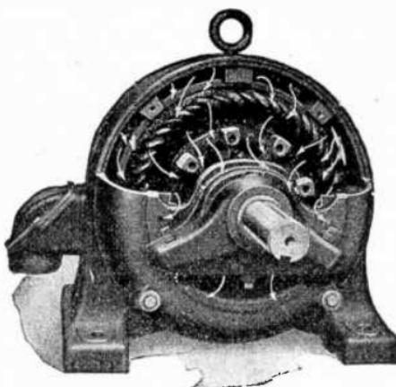
FIG. 2.815.—Sectional view of Wagner internal resistance motor showing directed draught ventilation.
