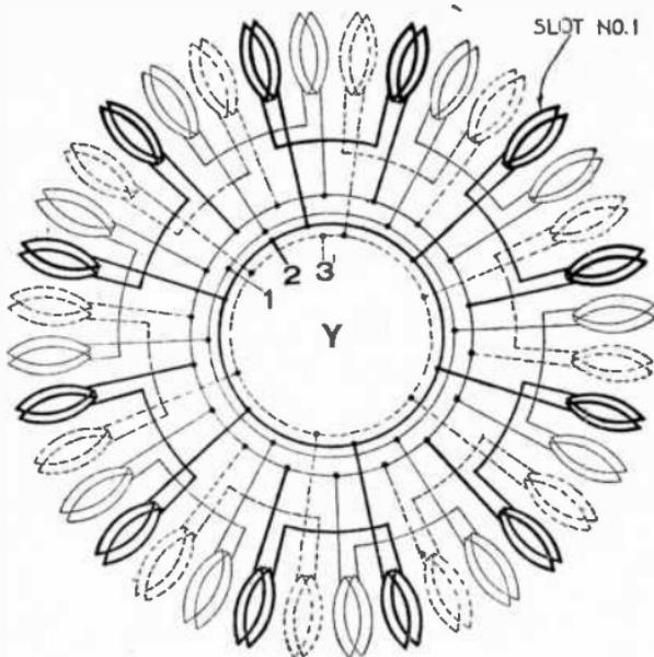
FIG. 3.286.—3 phase, 12 pole, 6 circuit Y.
