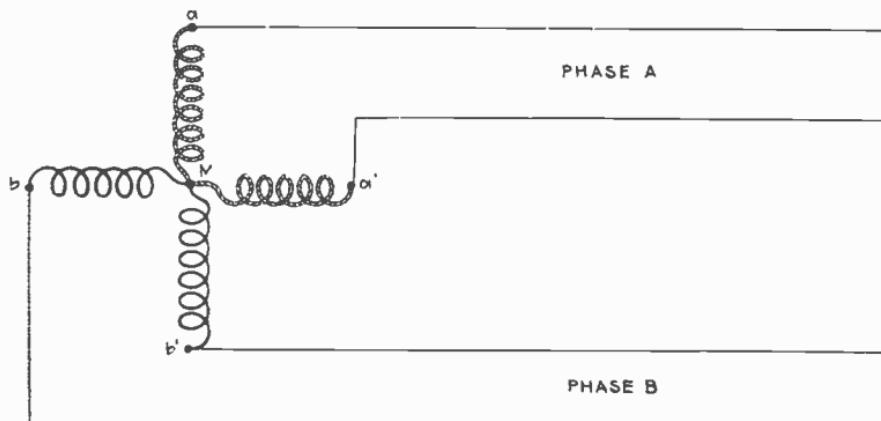
FIG. 3,158.—Diagram of two phase star grouping.
