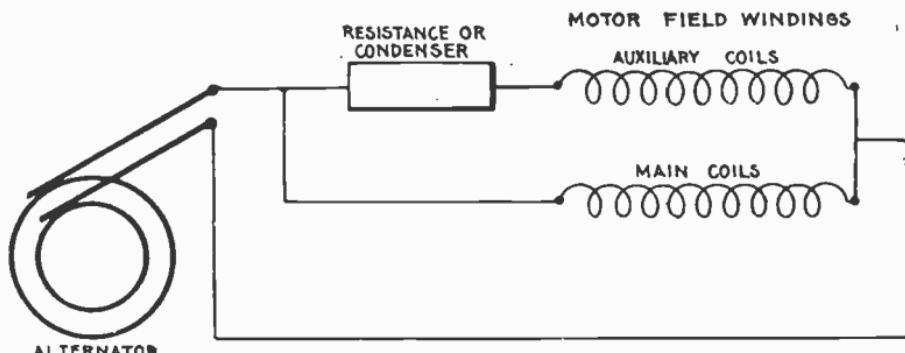
FIG. 2,844.—Simplified diagram showing the principle of phase splitting for starting single phase induction motors. By the use of an auxiliary set of coils connected in parallel with the main coils and having in series a resistance or condenser as shown, the single phase current delivered by the alternator is "split" into two phases, which are employed to produce a rotating field on which the motor is started.
