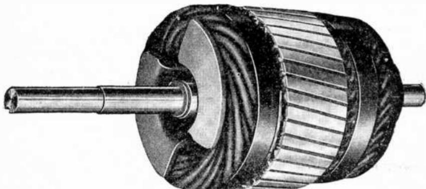
FIG. 2,999.—Jeanmin single phase repulsion start induction motor armature showing governor weights which when acted upon by centrifugal force close the short circuiting switch. This operation is shown in figs. 2,996 and 2,997.
