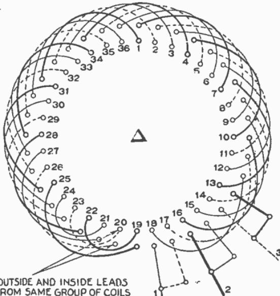
FIG. 3,279 —3 phase, 12 pole, 1 circuit Delta. Connections between coil groups only.
