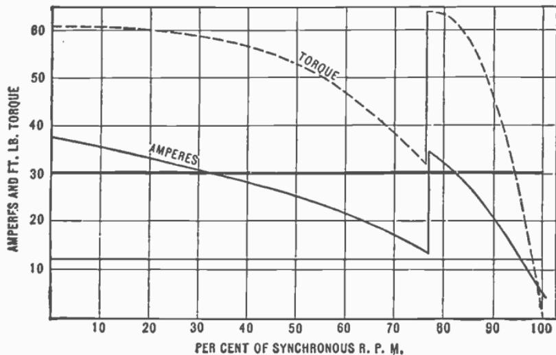
Fig. 2,753.—Starting characteristics of Wagner *internal resistance* motor.
