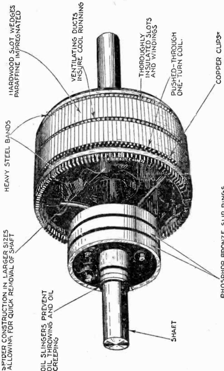
Fig. 2,789.—*Triumph* slip ring motor construction.—1. Armature showing winding and slip rings. The slip ring and brush rigging are shielded to prevent accident to the operator.
