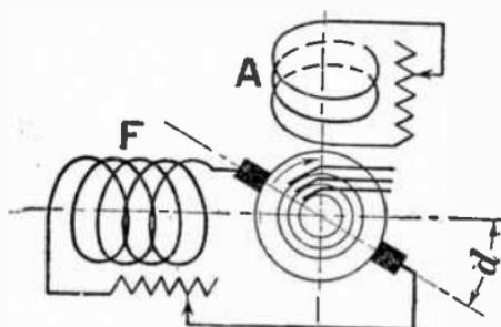
FIG. 3,015.—Fynn-Weichsel motor starting connections. The starting equipment is similar to that of a slip ring induction motor and as easily manipulated. Pilot circuit automatic starting may be used if desired.
