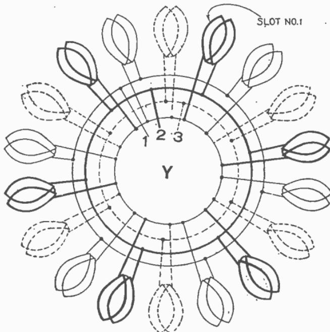
FIG. 3,267.—3 phase, 6 pole, 6 circuit Y.
