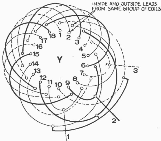
FIG. 3,262.—3 phase, 6 pole, 2 circuit Y. Connections between coil groups only.
