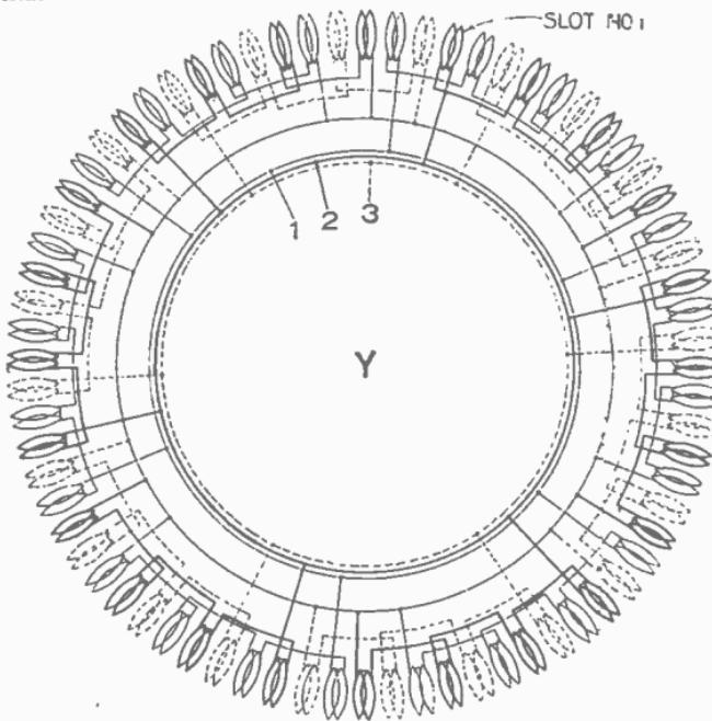
FIG. 3,291.—3 phase, 24 pole, 6 circuit Y.
