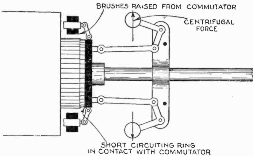
Figs. 2,986 and 2,987 —Diagrams illustrating operation of brush lifting mechanism of repulsion start induction motor. Fig. 2,986, brushes in contact with commutator during repulsion starting; fig. 2,987, brushes lifted from commutator and short circuiting ring pressed against commutator, short circuiting the latter, thus causing motor to run as an induction motor.
