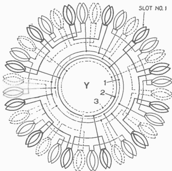
FIG. 3,282.—3 phase, 12 pole, 3 circuit Y.
