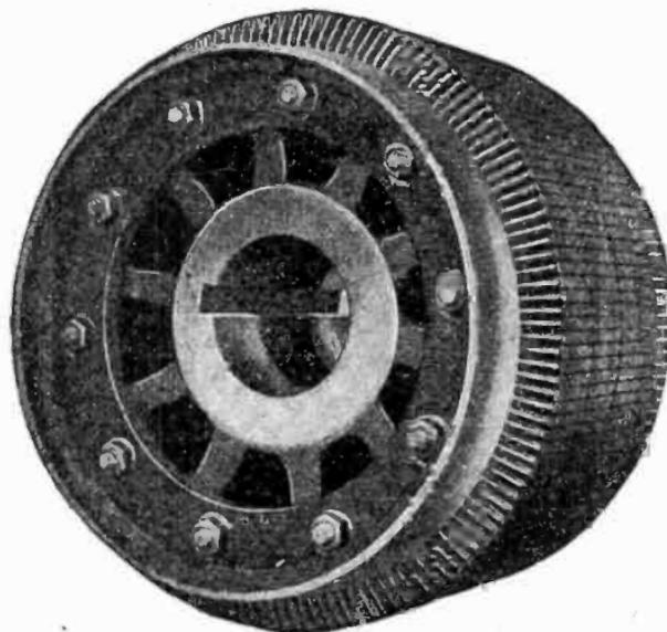
FIG. 2,800.—*General Electric slip ring motor construction 4.* Armature ready for winding showing heavy end flanges secured by through bolts and end fingers.
