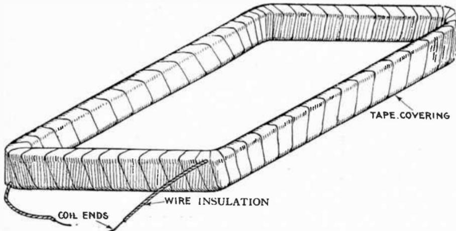
FIG. 3,120.—Simple form of alternator coil, consisting of numerous turns of insulated wire wound around a form, then covered with a tape winding, varnished and baked.
