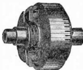
FIG. 2,991.—Baldor fractional horse power single phase repulsion start induction motor commutator showing sectional view of the short circuiting switch. This switch is designed for rolling contact to render it self-cleaning.
