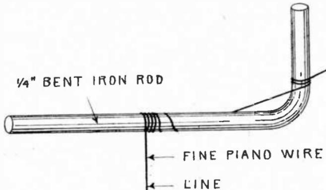
FIG. 3,940.—Small bent lever of  $\frac{3}{8}$  round iron to secure wire center line\*taut in position.
