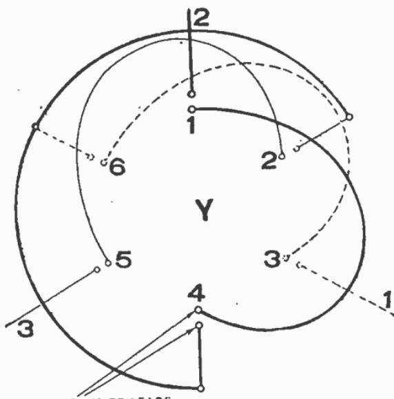
FIG. 3,254.—3 phase, 2 pole, 1 circuit Y. Connections between coil groups only.
