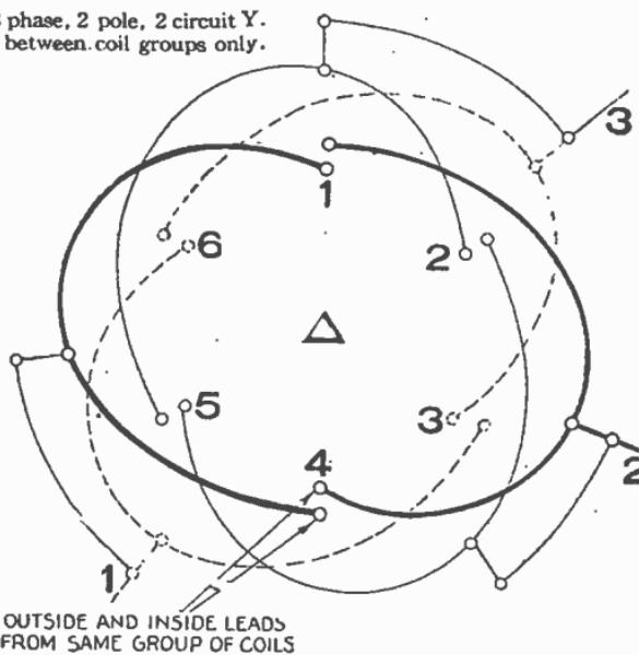
FIG. 3,257.—3 phase, 2 pole, 2 circuit Delta. Connections between coil groups only.
