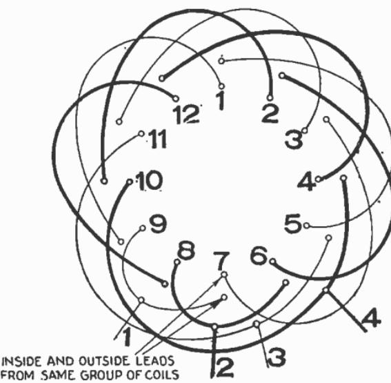
FIG. 3,247.—2 phase, 6 pole, 2 circuit. Connections between coil groups only.
