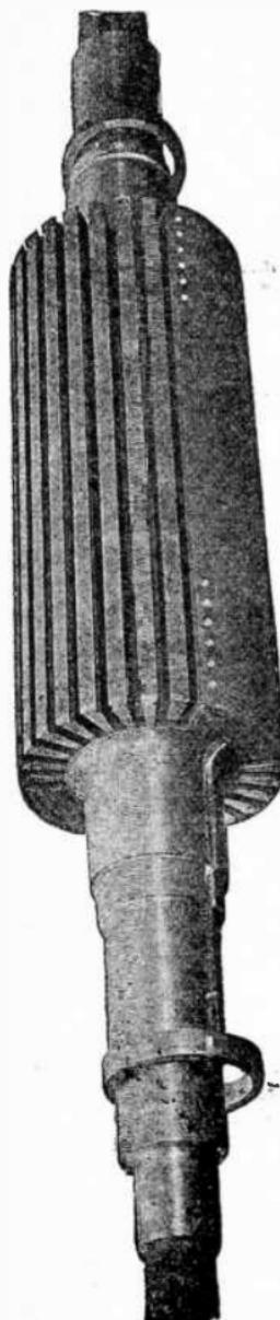
FIG. 3,154.—Westinghouse field core ready for winding. *It is made from a solid steel forging and has machined radial slots for the field winding. Tie slots and field winding are distributed so that the flux distribution of the field poles will be such that the generated voltage wave of the armature winding will be practically free from harmonics of an appreciable magnitude.*
