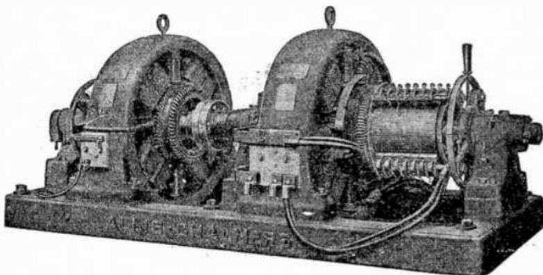
FIG. 3,094.—Allis Chalmers 600 volt motor driving 120 volt, 100 *kw.* series booster. If the voltage of a feeder is to be raised or a higher voltage is wanted to charge a storage battery a booster is useful.
