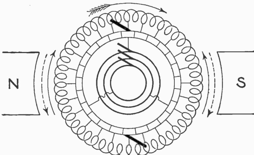
FIG. 3,031.—Diagram of three phase rotary converter. In this type, the winding is tapped at three points  $120^\circ$  distant from each other, and leads connected with the corresponding commutator segments.
