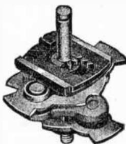
FIG. 4,069.—Diamond snap switch base showing terminals and steel detent which locks the mechanism. The detent is supported by a steel plate which is prevented turning by lugs set into the porcelain at its outside edge.
