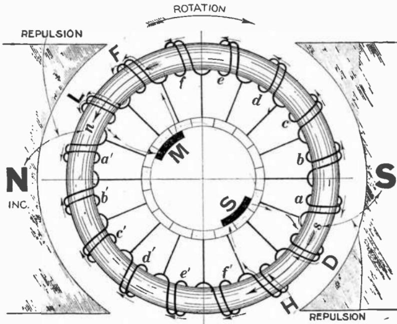
FIG. 2,972.—Ring armature in a.c. field with two thick brushes placed to short circuit two pairs of coils L,F, and H,D. *With this arrangement, clockwise rotation will result due to repulsion by the two pairs of short circuited coils. The resultant effect of the other coils is zero as may be seen from the diagram.*
