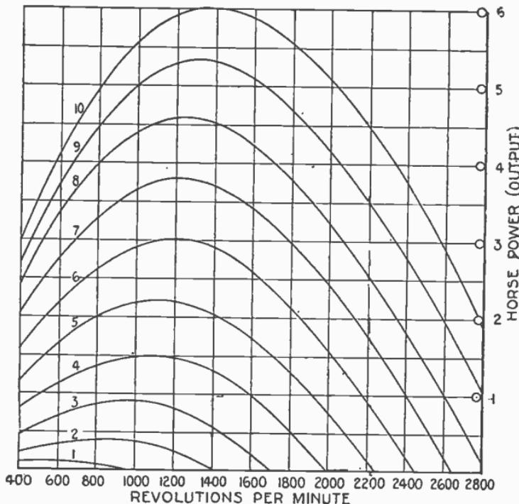
FIG. 3.008.—Horse power output curves for Kimble single phase class L brush shifting variable speed motor.
