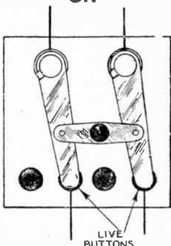
Figs. 3,991 and 3,992.—*Double pole lever switch showing essentials and operation.* Fig. 3,991, off position; fig. 3,992, on position.
