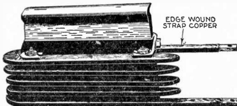
FIG. 3,027.—*Westinghouse synchronous converter construction 4. Commutating pole with winding.* The commutating pole field coils are made from edge wound strap copper. The coil is insulated from the pole piece by a heavy fullerboard shield which completely surrounds the pole piece. Insulating washers are placed between turns, allowing a free circulation of air around each conductor.
