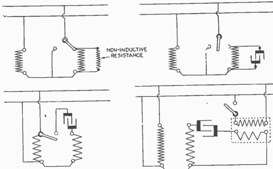
Figs. 2,820 to 2,823.—Four ways in which the phase can be split for starting split phase motors. Fig. 2,820, non-inductive shunt resistance; fig. 2,821, shunt condenser; fig. 2,822, series condenser; fig. 2,823, series condenser with transformer.
