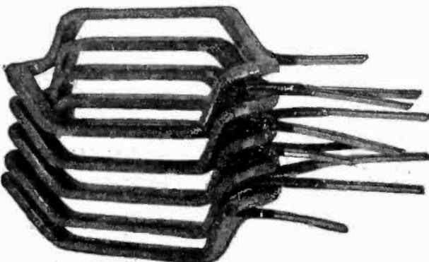
**FIG. 3,116.**—Allis-Chalmers "diamond" coils forming a five slot distributed coil unit. In construction, the coils are form wound, covered with insulating material and treated with insulating compound. The coils where they pass through the core and for some distance on each side, are further protected by insulating material placed in the slots. Each coil is held in place by means of leatheroid slot wedges. The ends of the coils, where they project beyond the slots, are heavily taled.
