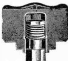
FIGS. 4,071 to 4,073.—Diamond snap switch handle. Fig. 4,071 external view of handle; fig. 4,072, spring in normal position; fig. 4,073, spring compressed.
