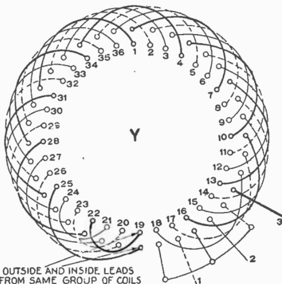
FIG. 3,278.—3 phase, 12 pole, 1 circuit Y. Connections between coil groups only.
