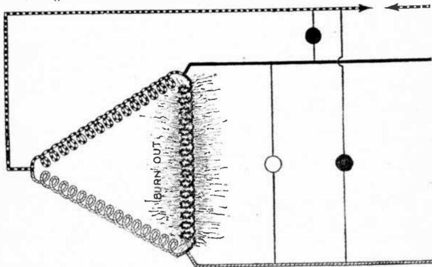
FIG. 3,972.—Single phasing of delta connected motor.
