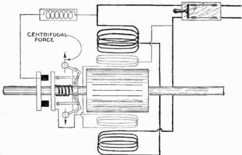
Figs. 2,846 and 2,847.—Elementary split phase induction motor *with cut out switch*. Fig. 2,846, cut out switch closed at start; starting winding in circuit; fig. 2,847, motor speeded up to point where centrifugal force acting on governor weights has overcome the tension of spring and opened switch cutting out starting winding.
