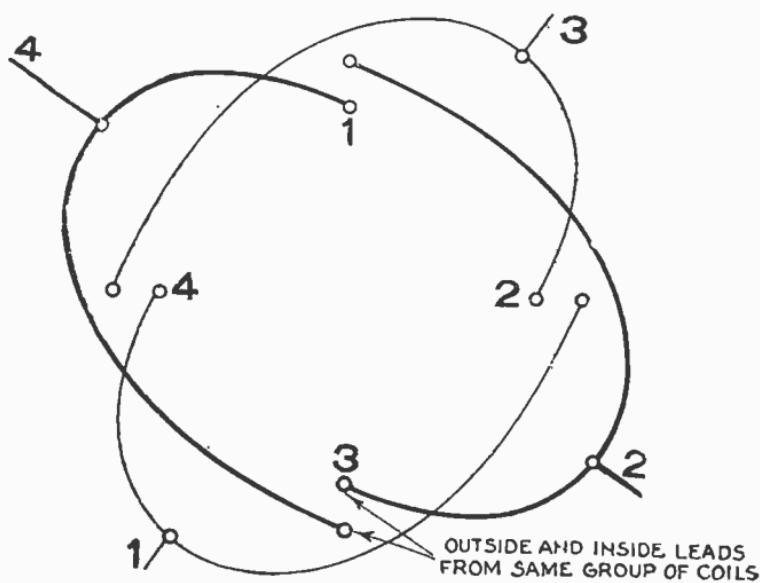
FIG. 3,244.—2 phase, 2 pole, 2 circuit. Connections between coil groups only.
