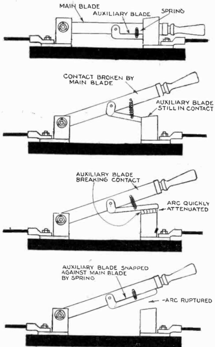
FIGS. 4,012 to 4,015.—Construction of *quick break switch* and its operation progressively shown. Fig. 4,012, switch in *ON* position; fig. 4,013, main blade out of contact; fig. 4,014, auxiliary blade breaking the circuit; fig. 4,015, *OFF* position, auxiliary blade held against main blade by spring.
