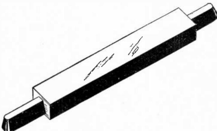
FIG. 3,223.—Wedge driver for lipped wedges.
