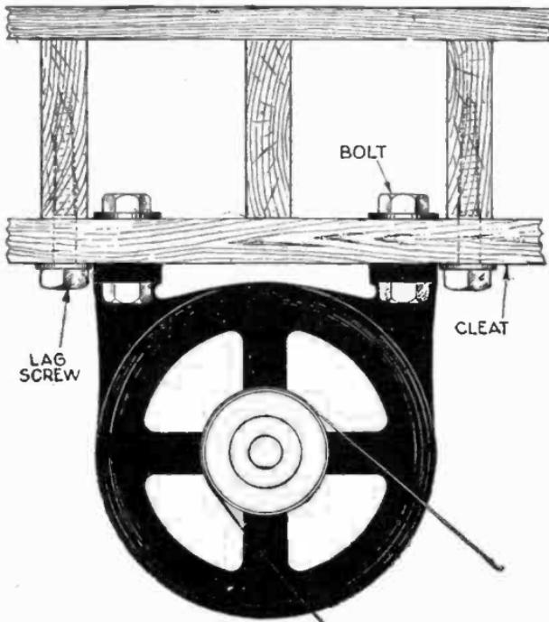
FIG. 3,939.—Method of mounting motor on wooden ceiling.
