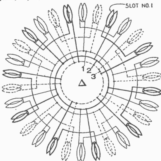
FIG. 3,273.—3 phase, 10 pole, 5 circuit Delta.
