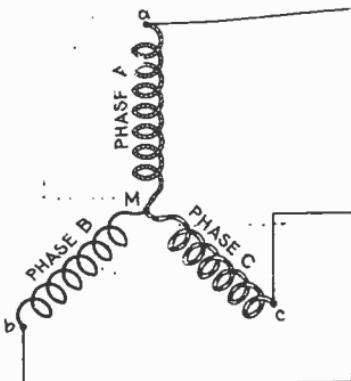
FIG. 3,160.—Diagram of three phase star grouping, commonly called Y grouping owing to its resemblance of the letter Y. The current in each main is obviously equal to the current in each phase winding, but the terminal pressure is the vector sum of the pressures in the component phase windings, that is,  $\sqrt{3}$  multiplied by the pressure in one phase.
