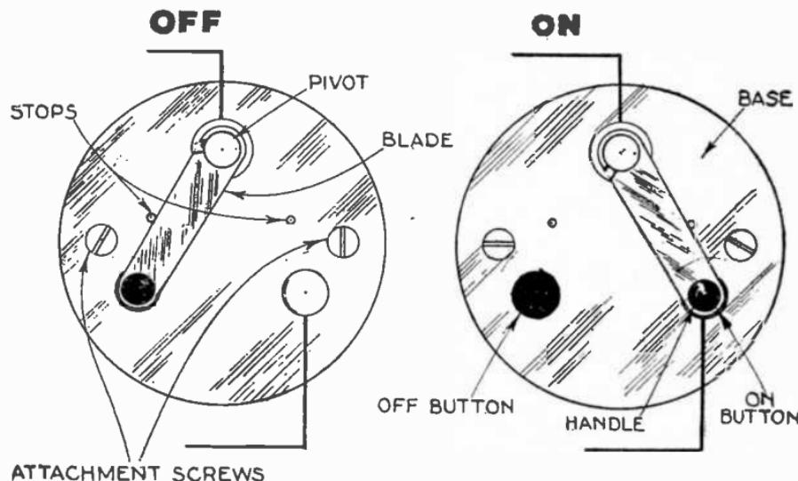
Figs. 3,975 and 3,976.—Lever switch illustrating construction and operation.
