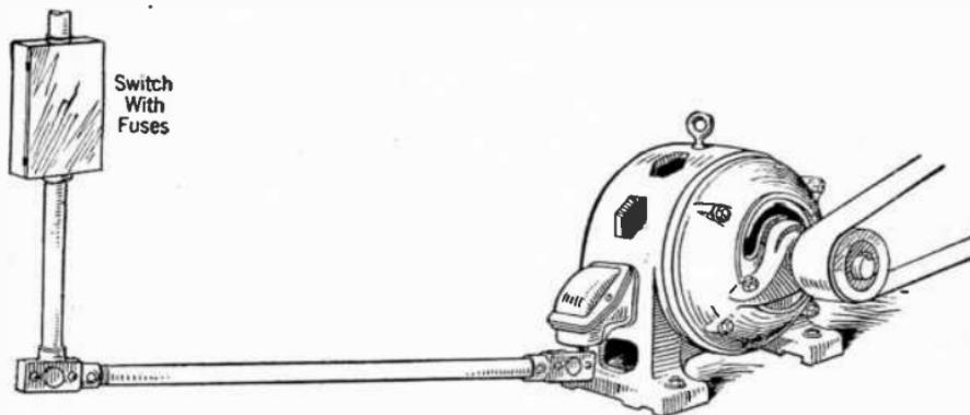
FIG. 2,779.—Installation of Wagner internal resistance motor showing three phase wiring connections.
