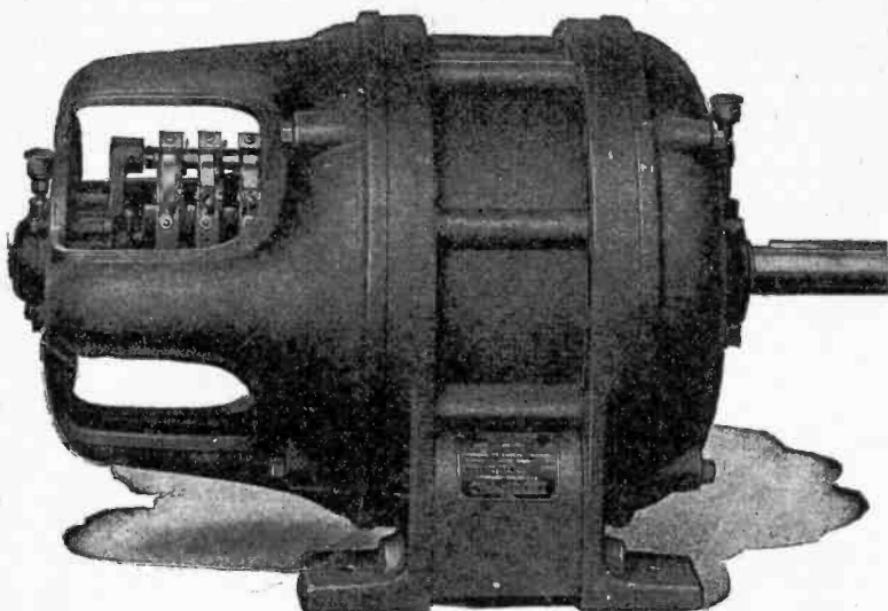
**FIG. 2,805.**—Allis Chalmers type ARY external resistance or slip ring motor. This type motor is adapted to keep the starting current within limits, or where a large starting torque is required, the slip ring or wound rotor type is used. This type requires a smaller current to develop a given starting torque, and is therefore used where frequent starting is necessary.
