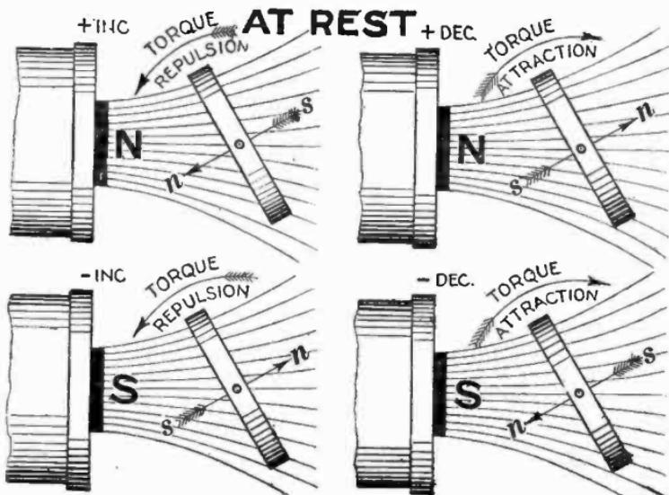
FIGS. 2,937 to 2,940.—*Repulsion motor principles 8.* When the plane of a pivoted copper ring at rest is oblique to the axis of an a.c. magnet, torque is produced by repulsion and attraction alternately, no useful torque; ring vibrates.
