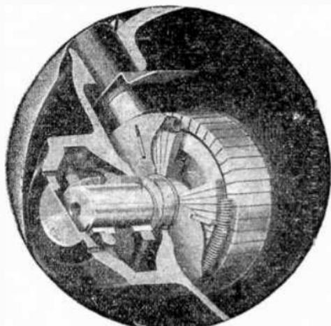
FIG. 2,995.—Leland single phase repulsion start induction motor short circuiting device. The construction is clearly shown in the illustration.
