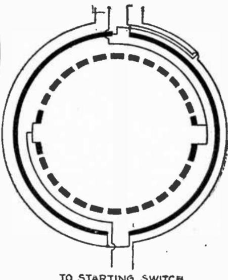
FIG. 3.203.—Diagram showing series connections for a two pole motor.
