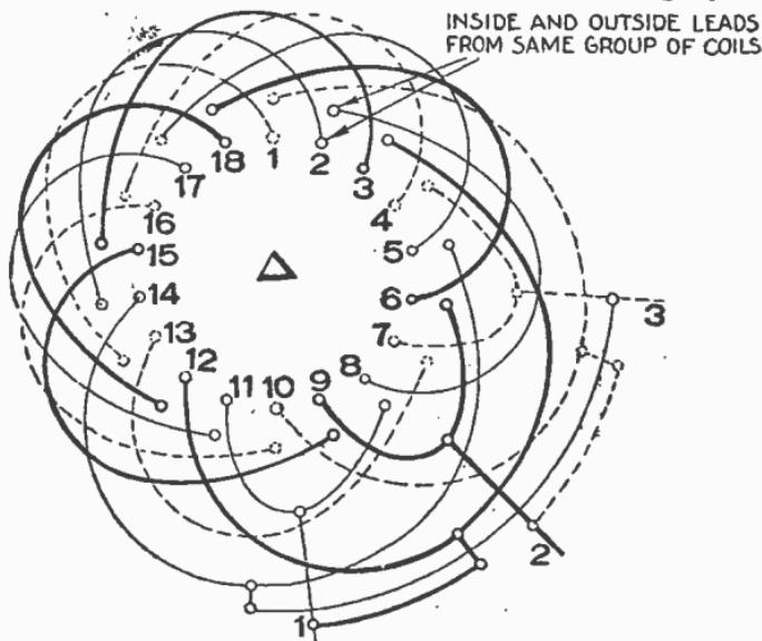
FIG. 3,263.—3 phase, 6 pole, 2 circuit Delta. Connections between coil groups only.
