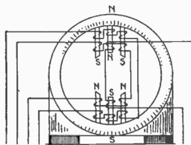
Figs. 3,064 to 3,066.—Woodbridge split pole rotary converter. Each pole is split into three sections and provided with windings as indicated in fig. 3,064. When excited as in fig. 3,065 the commutator voltage is at its highest value; when excited as in fig. 3,066, the commutator voltage is low. The change in commutator voltage for constant collector ring voltage is in virtue of the property of rotary converters that the ratio of these two voltages is a function of the width of the pole arc.
