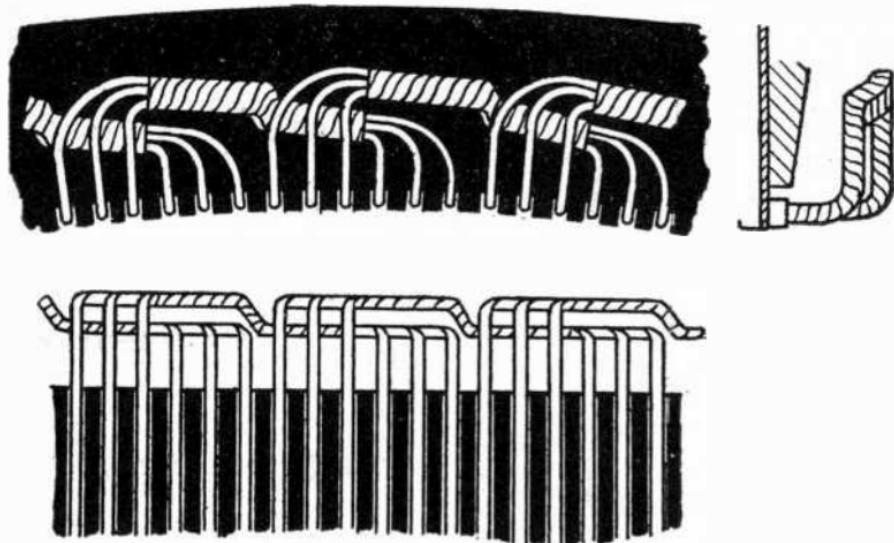
FIGS. 3,146 to 3,148.—Views of a section of skew coil winding; so called on account of the skew shape given to the coil ends in order that all the coils may be of one shape
