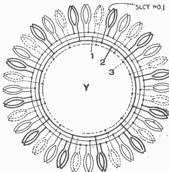
FIG. 3.287.—3 phase, 12 pole, 12 circuit Y.
