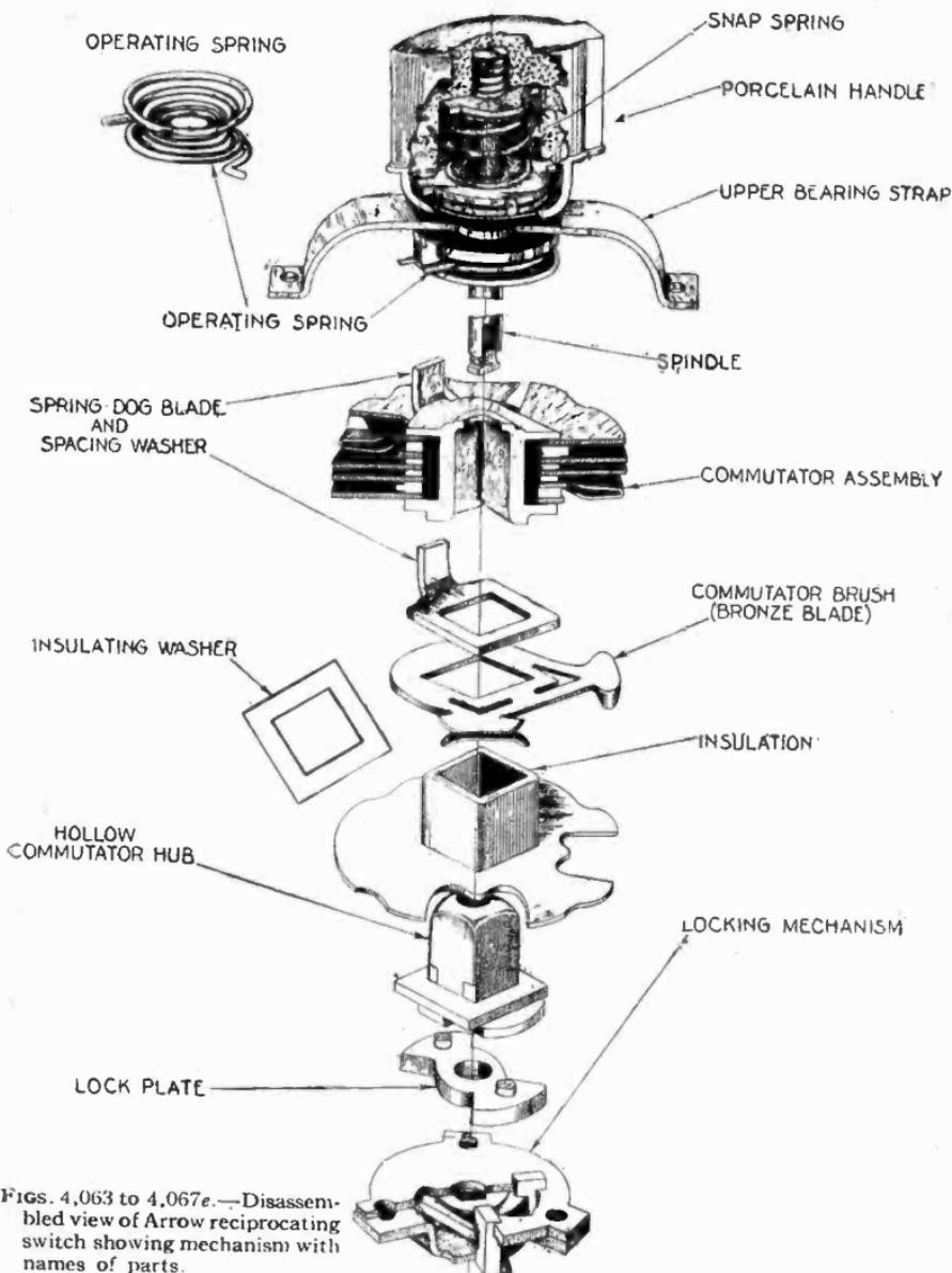
Figs. 4,063 to 4,067e.—Disassembled view of Arrow reciprocating switch showing mechanism with names of parts.
