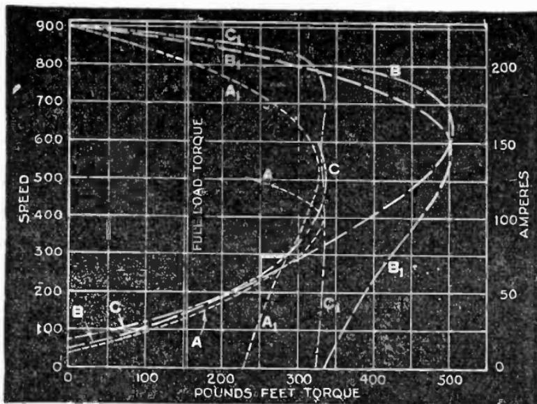
FIG. 2,778.—Speed torque and current curves of 25 h.p., 8 pole, 60 cycle induction motors according to F. J. Johns (of Westinghouse Co.) A<sub>1</sub>, speed torque of a high slip motor; B<sub>1</sub>, speed torque curve of a high torque motor; C<sub>1</sub>, speed torque curve of a line start motor; A, current torque curve of a high slip motor; B, current torque curve of a high torque motor; C, current torque curve of a line start motor.
