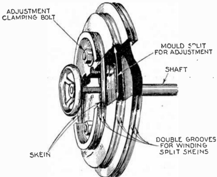
FIG. 3,175.—Winding head for winding skeins. The double grooving permits winding two skeins of the same size or one split skein. When the skein is over  $\frac{1}{4}$  in. square and of wire larger than No. 19, it should be wound in two sections. Note that the winding mould is split through the center so as to be adjustable for different sizes of skeins.
