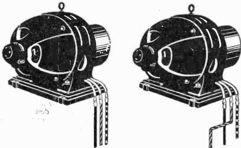
Figs. 3,934 and 3,935.—Reversing three phase motor. *Interchange the connection of any two leads.*
