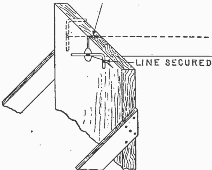
FIG. 3,941.—Method of securing wire center line.
