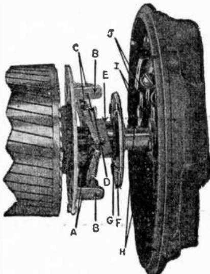
FIG. 2,886.—Wagner split phase induction motor switch mechanism with plate in exaggerated position to show construction.
