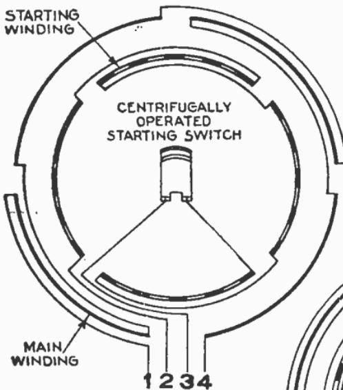
FIG. 3,197.—Diagram showing series connections of four pole motor. *Clockwise rotation:* Connect 1 and 2 to one line; connect 3 and 4 to other line. *Counter clockwise rotation:* Connect 1 and 3 to one line; connect 2 and 4 to other line.
