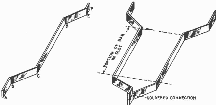
FIGS. 3,126 and 3,127.—Bent bar inductor and method of connection with soldered joint.
