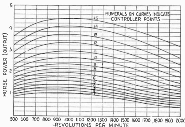
FIG. 3,006.—Horse power output curves for Kimble single phase class A, variable speed motor. The curves show the speeds at various horse powers of a 3 h.p. motor at various controller points.
