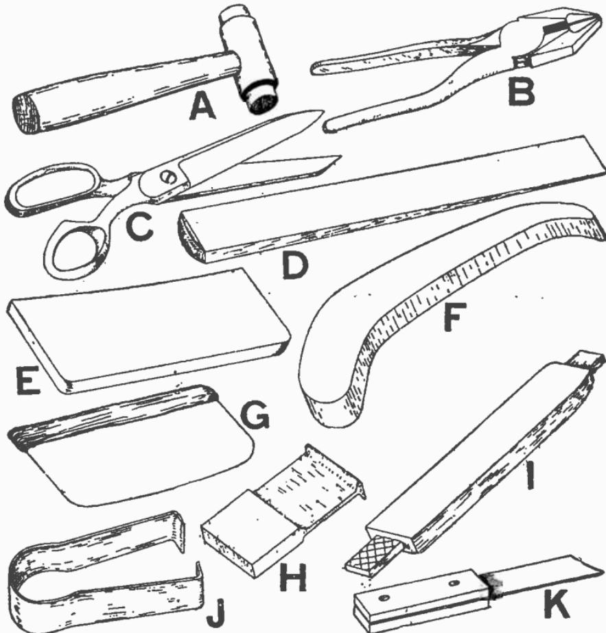
Figs. 3,229 to 3,239.—Hand tools ordinarily used in winding induction motors. *These are:* A, rawhide mallet; B, pliers; C, scissors; D, steel winding drift; E, assorted thicknesses of fibre slot drifts; F, fibre shaping drift; G, fibre cell drift; H, steel T-shaped cell drift; I, wedge driver; J, lead scraper; K, knife.
