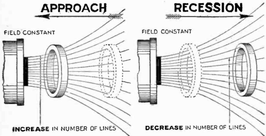
Figs. 2,917 and 2,918.—*Repulsion motor principles 2. The approach or recession of a copper ring from a magnet pole is respectively equivalent to an increase, or decrease in the number of lines of force which pass through the ring.*
