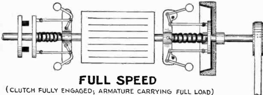
Figs. 2,879 to 2,881.—Elementary split phase induction motor with *cut out switch* and *clutch*, showing working of these automatic devices; the windings are not shown. Fig. 2,879 at start; 2,880, about  $\frac{3}{4}$  speed; fig. 2,881, full speed.
