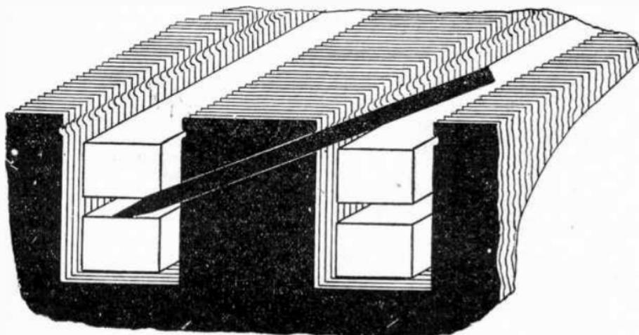
FIG. 3.227.—Wrong way to remove a coil. Don't use the lower coil as a fulcrum.
