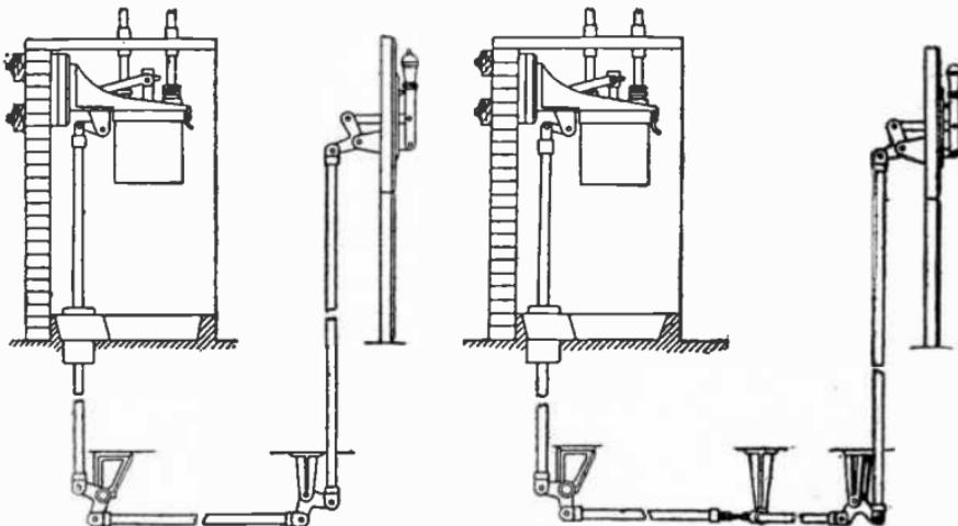
Figs. 4,039 and 4,040.—Views showing mechanism of hand operated remote control switches.
