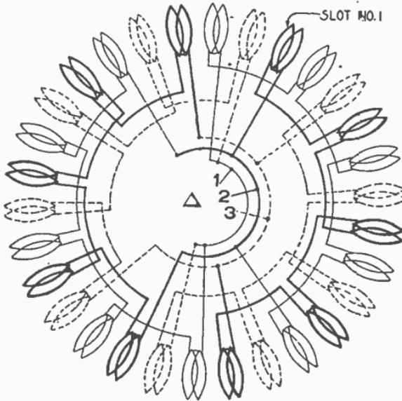
FIG. 3,271.—3 phase, 10 pole, 2 circuit Delta.
