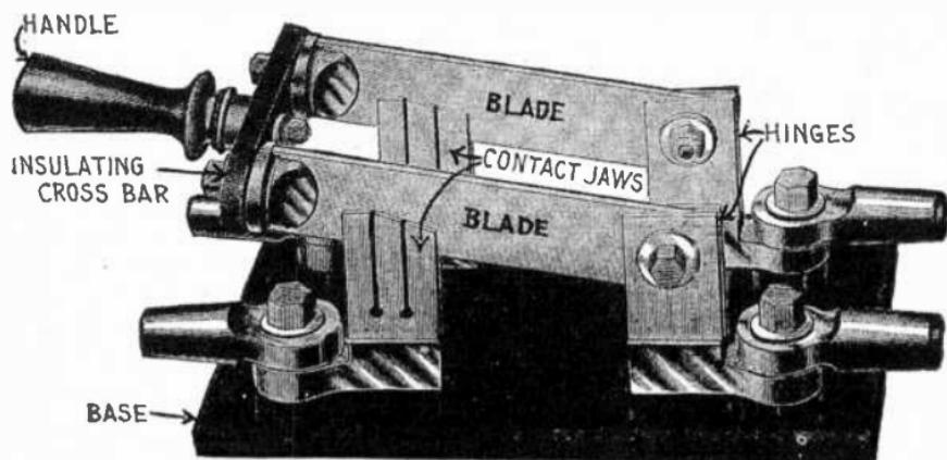
FIG. 4,001.—A single throw, two pole knife switch. As usually constructed it is made of hard drawn copper with cast terminal lugs and fibre cross bar.
