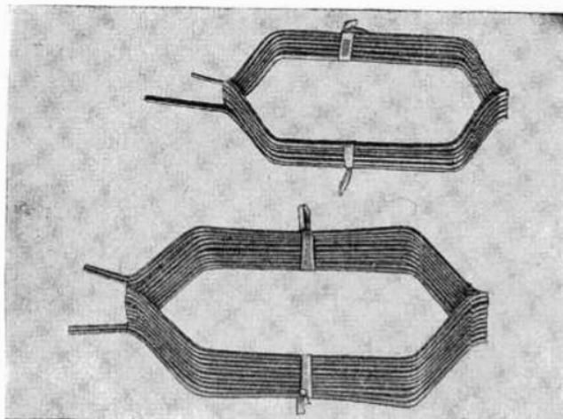
FIGS. 2,808 and 2,809.—Continuous windings of taped copper ribbon as used on Fairbanks-Morse slip ring motors. The continuous winding has for its object the elimination of a multiplicity of soldered connections.
