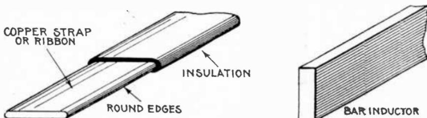
FIG. 3,122.—Copper strap or ribbon with insulation. These are generally from  $\frac{1}{8}$  to  $\frac{1}{4}$  inch thick with rounded edges as shown to avoid cutting the insulation.
