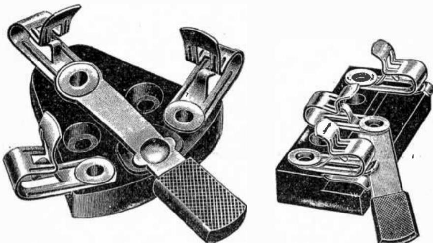
FIGS. 3,989 and 3,990.—Fahnestock *double throw, lever switches*. Fig. 3,989 short arc swing; fig. 3,990, long or  $180^\circ$  arc swing. The latter amplitude of swing is that used on knife switches.
