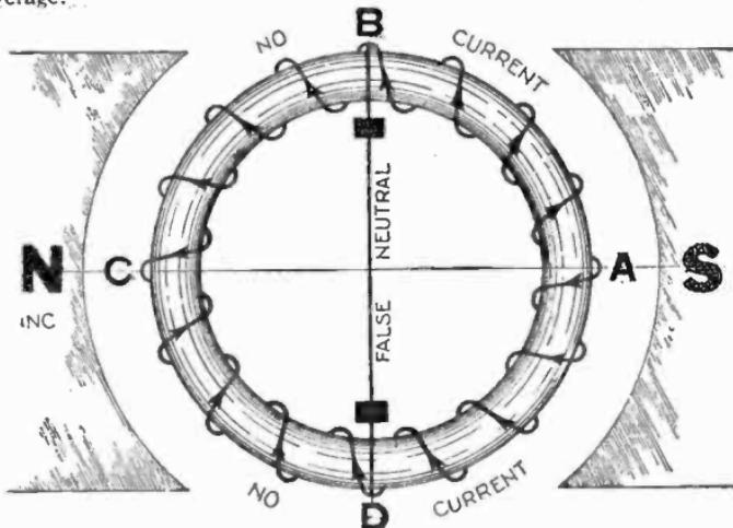
FIG. 2,971.—Ring armature in a.c. field with short circuited brushes located at 90° from magnet axis, that is, from *live neutral*. Since the induced pressures in quadrant AB, are balanced by the opposing pressures in quadrant AD, and similar conditions obtain in the other two quadrants BC and CD, there will be no current flow, consequently no torque tending to produce rotation.
