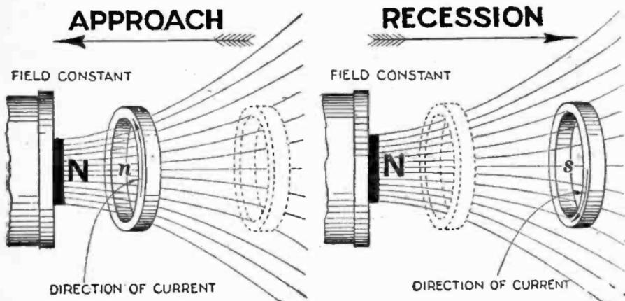
Figs. 2,915 and 2,916.—*Repulsion motor principles 1. The approach or recession of a copper ring from a magnet pole will induce currents alternating in direction.*
