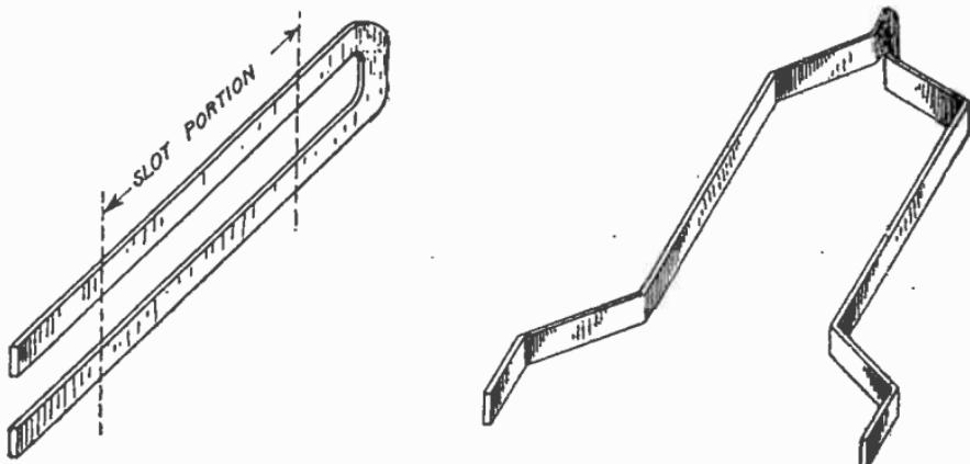
FIGS. 3,128 and 3,129.—Method of avoiding a soldered joint at one end of a bar inductor by using a bar of twice the length shown in fig. 3,126, and bending it into a long U form, as in fig. 3,128, after which it is spread out forming two inductors, as in fig. 3,129.
