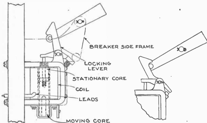
Figs. 4,173 and 4,174.—Westinghouse carbon circuit breaker electric lockout attachment. There are times when it is desired to lock a breaker in the open position when certain conditions exist. For this purpose a lockout attachment is provided which either latches the breaker open or else interposes an arm which opposes the movement of the brush. Depending upon requirements the coil may lock the breaker open when energized or it may be so arranged as to lock the breaker open when de-energized.
