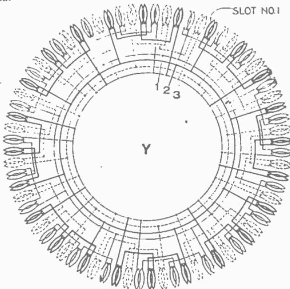
FIG. 3,293.—3 phase, 24 pole, 8 circuit Y.
