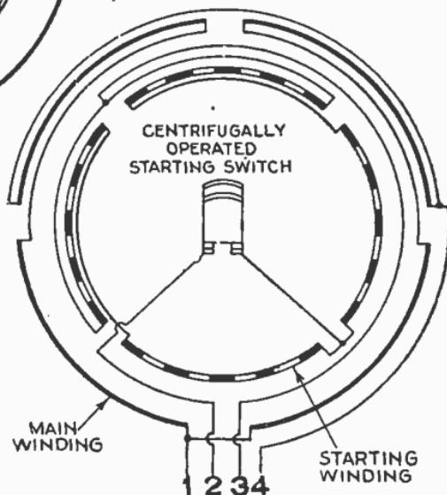
FIG. 3,198.—Diagram showing connections of a four pole, two path motor. *Clockwise rotation:* Connect 1 and 2 to one line; connect 3 and 4 to other line. *Counter clockwise rotation:* Connect 1 and 3 to one line; connect 2 and 4 to other line.
