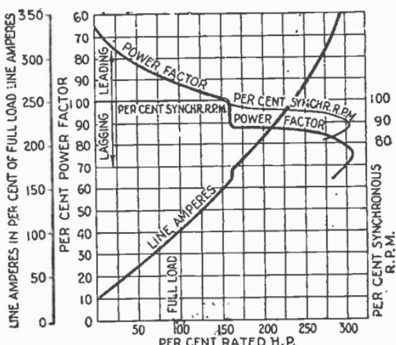
FIG. 3,018.—Fynn-Weichsel motor running characteristics; motor adjusted to operate in parallel with induction motors. It will be noted that the motor operates at synchronous speed with a leading power factor to about 160% load. Above this value it drops into induction motor characteristics and continues to run as a slip ring motor, to the breakdown point of approximately 300% load before it stops.
