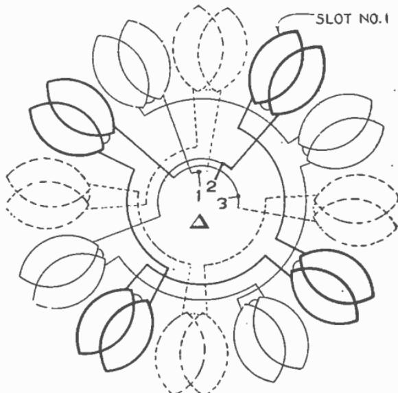
FIG. 3,277.—3 phase, 4 pole, 1 circuit Delta
