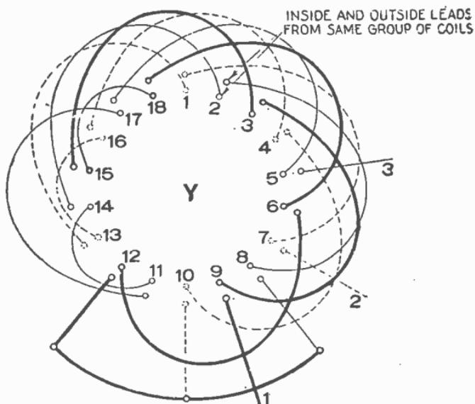
FIG. 3,260.—3 phase, 6 pole, 1 circuit Y. Connections between coil groups only.
