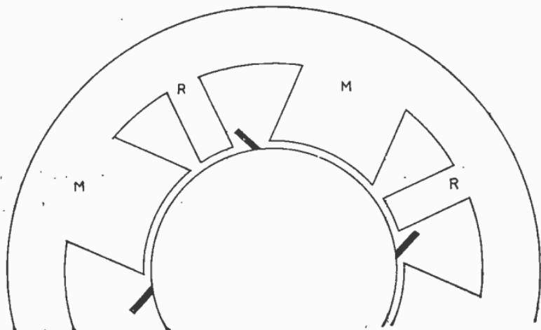
FIG. 3,074.—Diagram illustrating placement of regulating poles. In practice machines are not built as indicated diagrammatically in fig. 3,070, that is, with regulating poles spaced midway between the main poles, because a better construction is obtained by placing the regulating pole closer to the corresponding main pole, as shown above.
