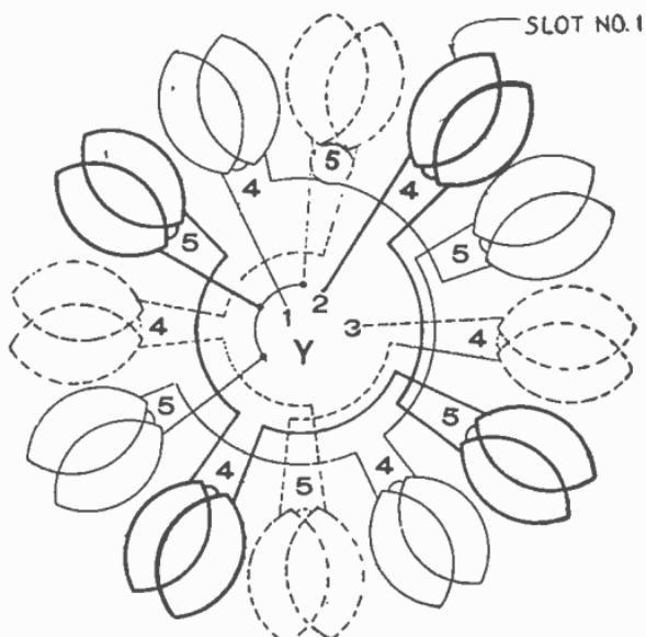
FIG. 3,276.—3 phase, 4 pole, 1 circuit Y, irregular.
