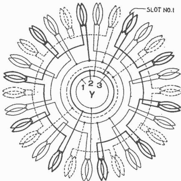
FIG. 3,270.—3 phase, 10 pole, 2 circuit Y, regular.
