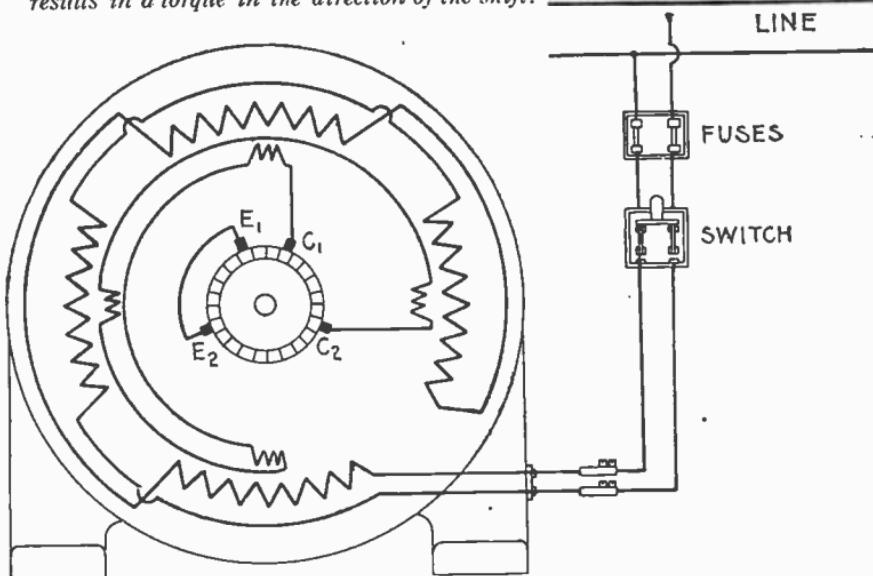
FIG. 2,979—Diagram of connection of Sprague single phase compensated repulsion motor. To reverse direction of rotation interchange leads  $C_1$  and  $C_2$  and slightly shift the brush holder yoke. Brushes  $E_1$  and  $E_2$  are permanently short circuited. This diagram of connections applies also to fig. 2,981.
