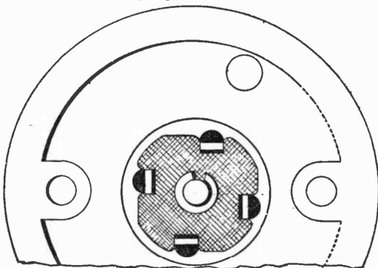
FIG. 4,059.—H & H snap switch method of attaching mechanism to base. **In construction**, metal plates on top and bottom of the porcelain base, riveted together, form the supports for the spindle and act as bearings for it. No matter how the spindle is yanked or wrenches in service these plates hold the spindle and mechanism in alignment.
