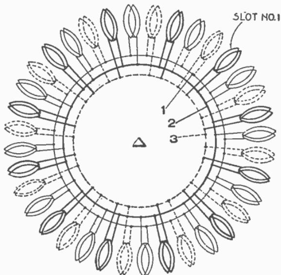
FIG. 3,288.—3 phase, 12 pole, 12 circuit Delta.
