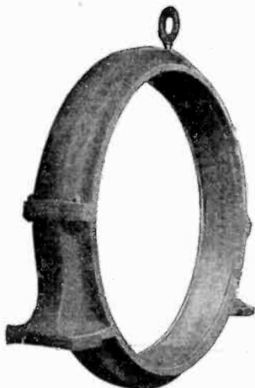
FIG. 3,023.—*Westinghouse synchronous converter construction 1. Field frame.* Material, cast steel. The frames of machines of 500 *k.w.* capacity and above are split horizontally and the upper half is provided with eye bolts so that it can be readily lifted off with its field winding. The supporting feet are cast integral with the frame.
