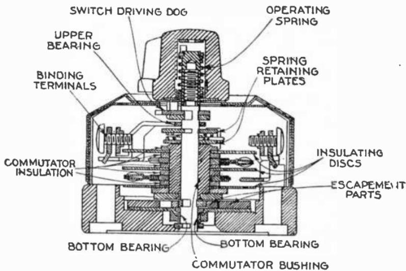
FIG. 4,082.—Sectional view of Bryant heater switch.
