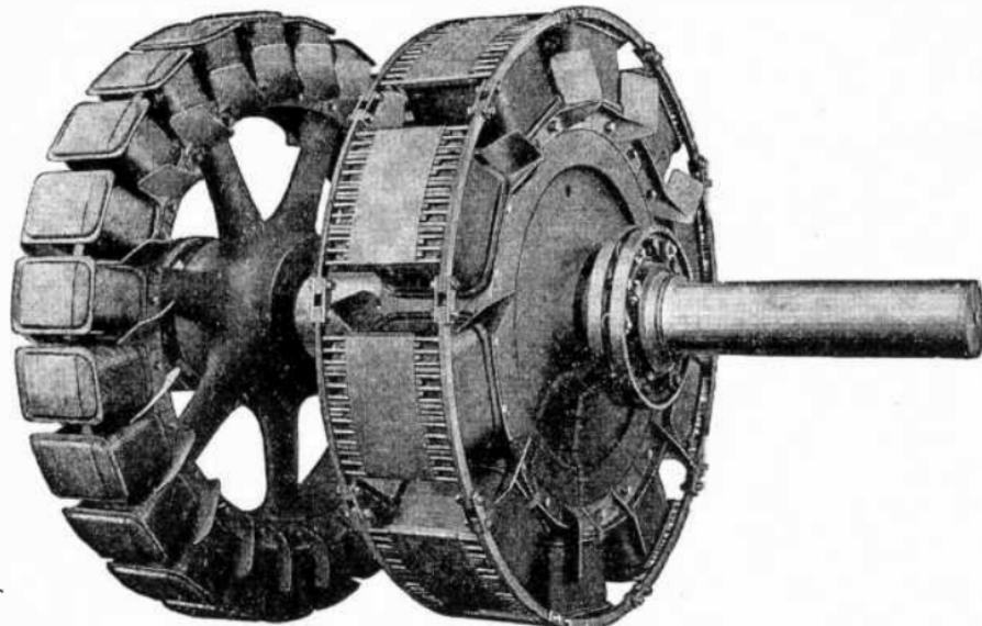
FIG. 3,096.—Allis Chalmers rotor of 1200 *kva.*, 300 *r.p.m.* frequency changing set, showing fans for ventilation and arrangement of dampers used to facilitate starting and to insure parallel operation without hunting.
