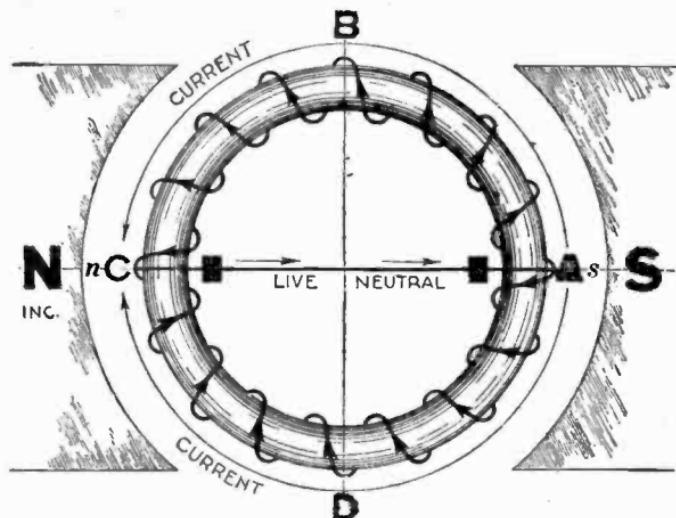
FIG. 2,970.—Ring armature in a.c. field with short circuited brushes located on magnet axis. *For this connection there will be a maximum flow of current; this position of the brushes is called the live neutral.* Since the armature is polarized in the direction *ns*, parallel to the field lines of force, there will be no torque tending to produce rotation because there is no leverage.
