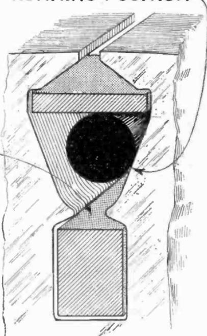
Figs. 2,771 and 2,772.—Operation of choker rod of Fairbanks Morse choker type double squirrel cage motor. Fig. 2,771, armature at rest, choker rods held in ***closed position*** by magnetic attraction; fig. 2,772, armature nearly up to running speed, choker rods thrown out by centrifugal force to ***open position***, opening the leakage gaps.
