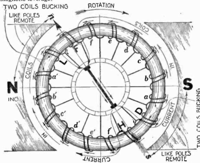
FIG. 2,976.—Ring armature in a.c. field with short circuited brushes shifted *close to false neutral* showing weakening of torque (as compared with torque in fig. 2,974) due to increase in number of bucking coils.
