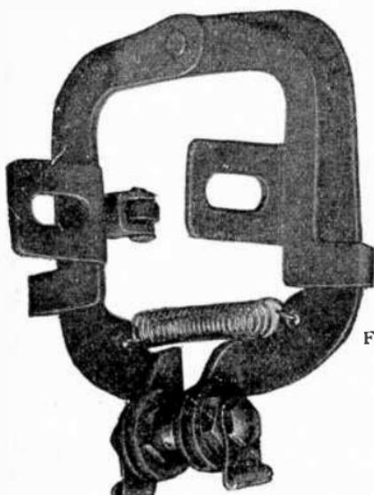
FIG. 2,850.—Century split phase induction motor cut out switch. It is adjusted for a predetermined speed. The governor fig. 2,849 which actuates the cut out is positive in action and opens the starting or phase coil circuit with a rapid break of silver contacts.
