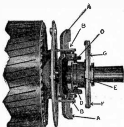
FIG. 2,885.—Wagner split phase induction motor switch mechanism; side view.
