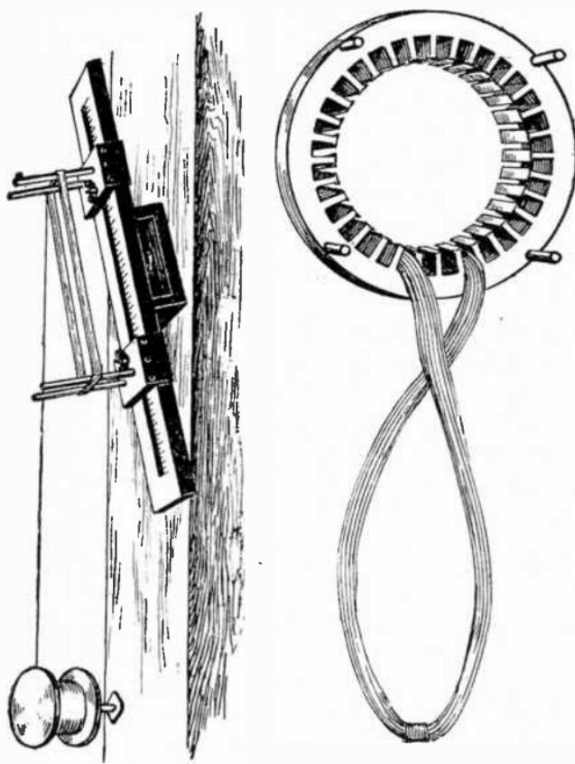
FIG. 3,174.—Adjustable shuttle or skein winder showing operation of winding a skein corresponding to fig. 3,175.
