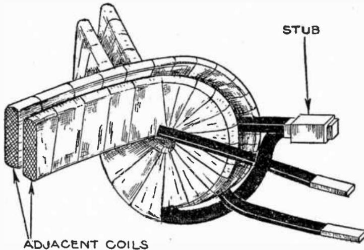
FIG. 3.224.—Stub or connection between adjacent coils.
