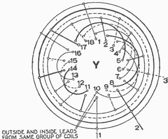
FIG. 3,264.—3 phase, 6 pole, 3 circuit Y. Connections between coil groups only.
