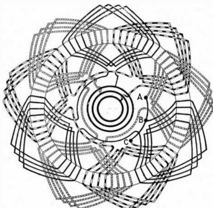
FIG. 3,164.—Radial diagram of three phase *lap* winding with star connection.
