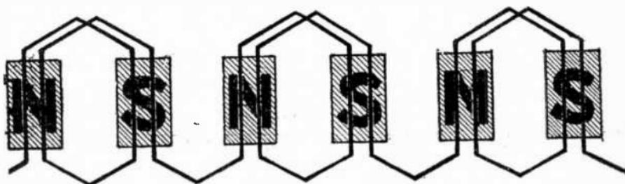
FIG. 3,100.—Single phase *lap* winding suitable for the same conditions as for the wave winding in fig. 3,101.
