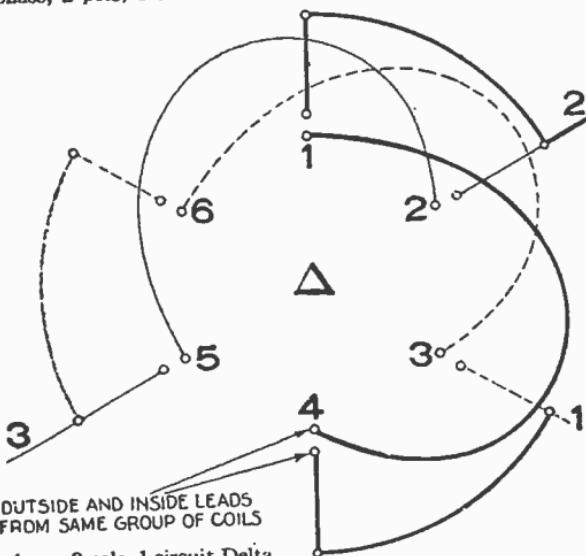
FIG. 3,255.—3 phase, 2 pole, 1 circuit Delta.
