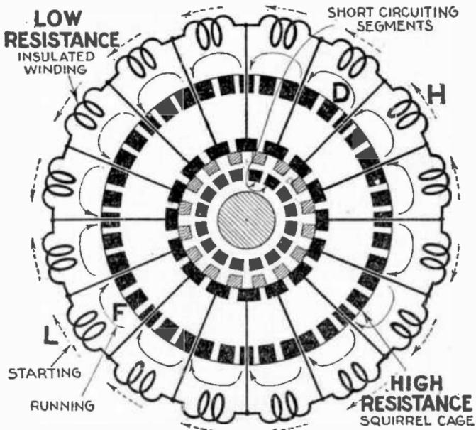
FIG. 2,747.—End view diagram of Wagner *high resistance squirrel cage low resistance winding* type of internal resistance motor showing the shaft, the low resistance squirrel cage, the high resistance insulated winding, and the segments of the multi-contact switch which short circuits the insulated winding when the armature attains 70 per cent of running speed.
