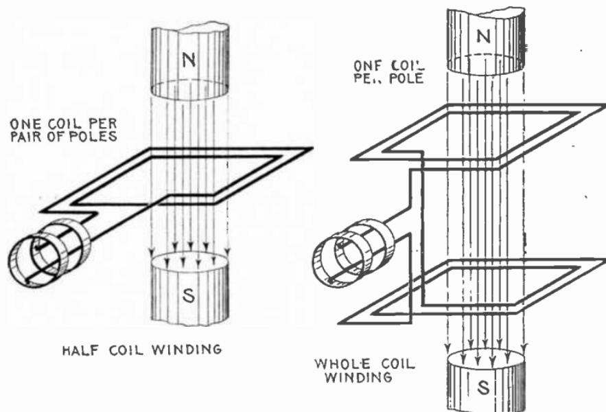
Figs. 3,102 and 3,103.—Elementary bipolar alternators with *half coil* and *whole coil* windings. In a half coil winding there is one coil per phase *per pair of poles*; in a whole coil winding there is one coil per phase *per pole*.
