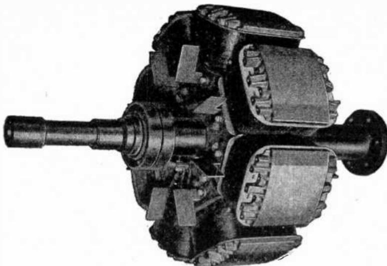
FIG. 3,166.—Westinghouse general turbine alternator field.
