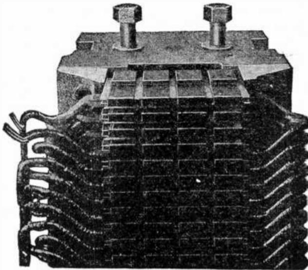
FIG. 3,942.—Detail of joint showing split stator construction of Ideal 60 h.p., 2,200 volt, 3 phase, 25 cycle, synchronous motor.
