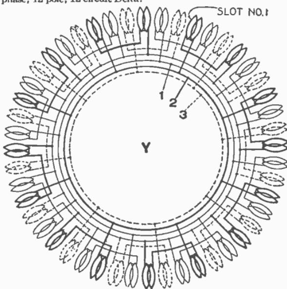
FIG. 3,289.—3 phase, 16 pole, 8 circuit Y.
