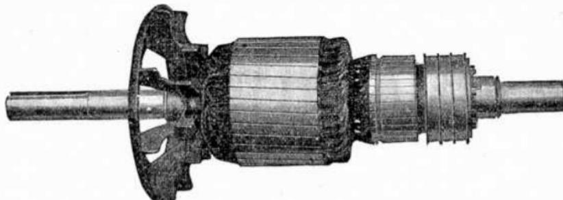
FIG. 3,020—Fynn Weichsel motor armature with windings in which are induced the load and exciting currents.
