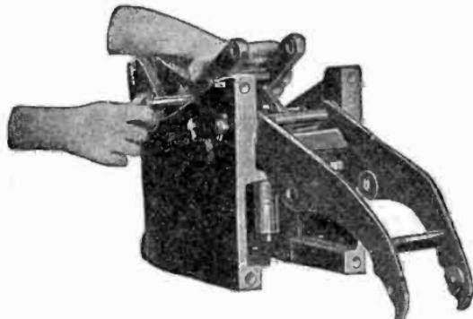
FIG. 4,166.—*How to assemble an air circuit breaker 15.* Connecting the toggle links to the main toggle.
