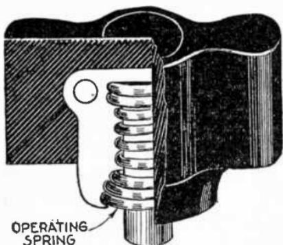
the eccentric on the spindle forces the stop out to the cam point where it is released just when the spring is at proper tension. This stop and cam receive the shock of the snap. To resist the wear and at the same time retain their toughness, these parts are carefully case hardened. They are, furthermore, formed with
