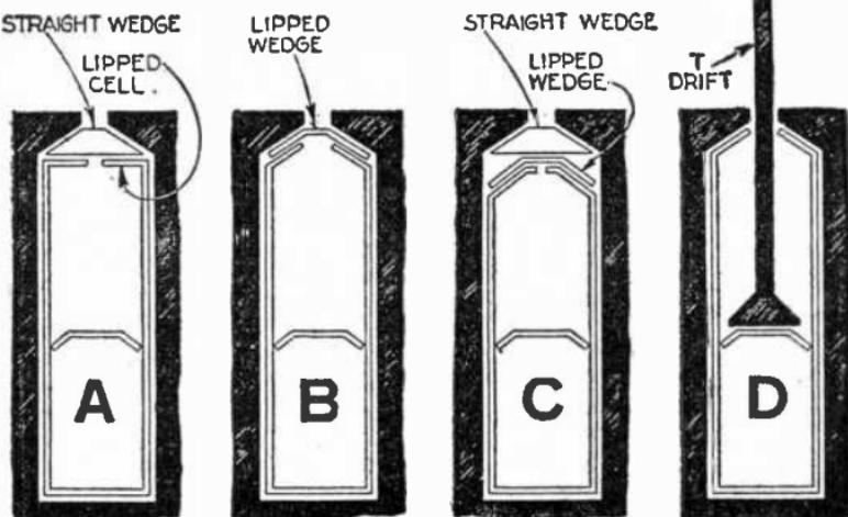
Figs. 3,219 to 3,222.—Slot details showing: A, lipped cell and straight wedge; B, lipped wedge; C, both lipped and straight wedges; D, use of T drift.
