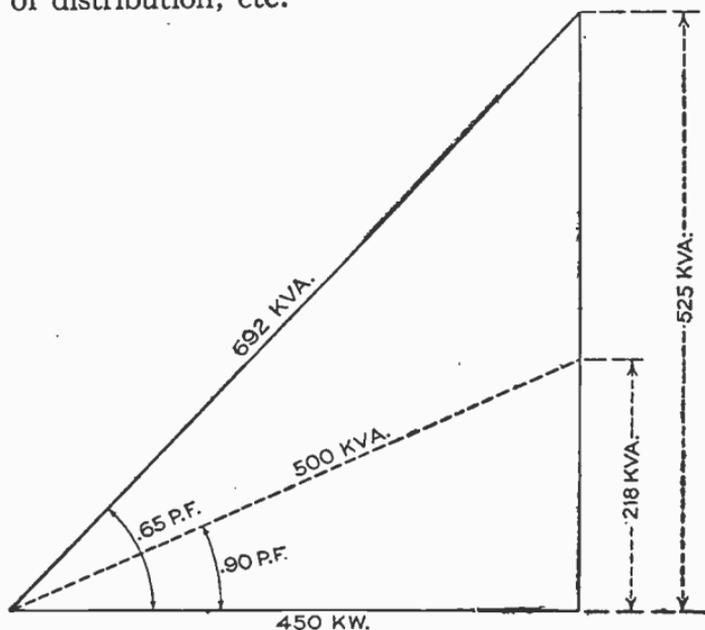
FIG. 4,261.—Diagram for synchronous condenser calculations.
