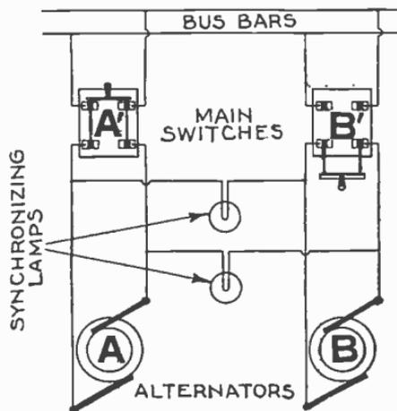
FIG. 4,836.—Synchronizing, *two dark lamp method*. When the machines are in phase there will be no difference of pressure between the left hand terminals or between the right hand terminals of the two machines. Hence, if the synchronizing lamps be connected as shown, both will be dark, and the switch may be thrown in connecting the machines in parallel.
