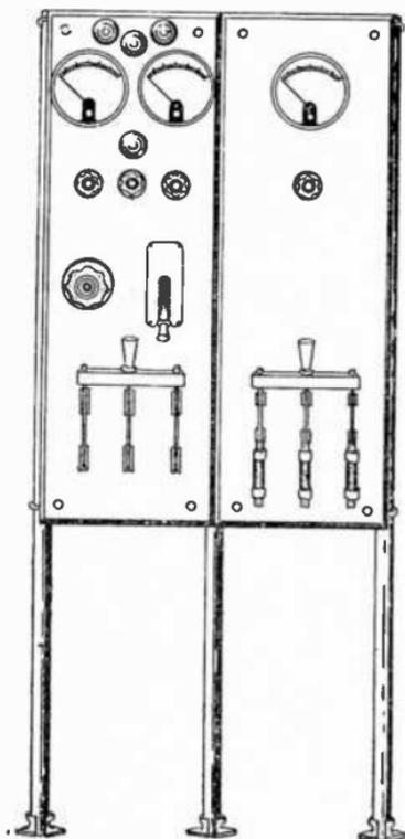
The oil circuit breakers or other switching devices are operated by means of suitable operating rods and links attached to a handle or handles on the front of the panels. Fig. 4,650 shows a manual remote control board.
