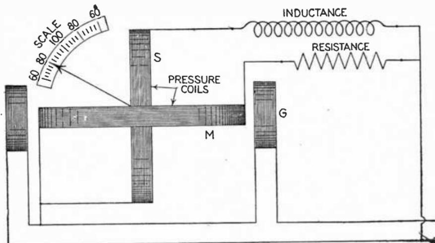
FIG. 4,538.—Single phase power factor meter of the rotating field or disc type.
