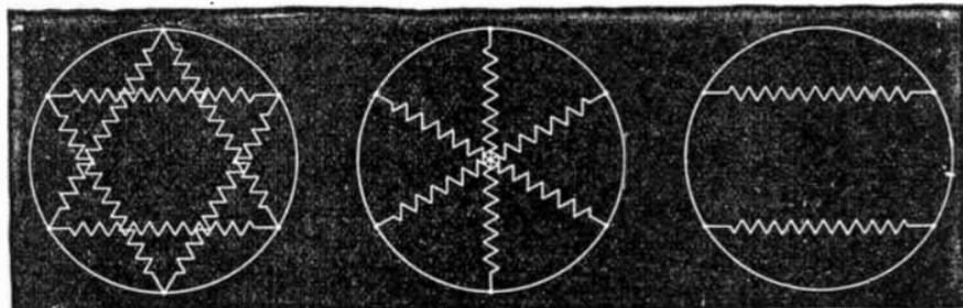
FIGS. 4,842 to 4,844.—Converter connections. Fig. 4,842, double delta connection; 4,843, diametrical connection; 4,844, two circuit single phase connection.
