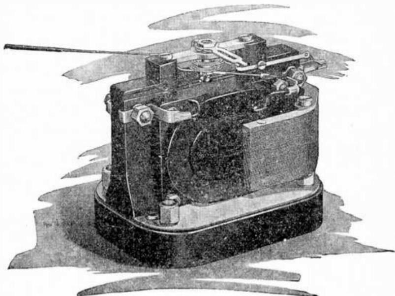
FIG. 4,472.—Jewel dynamometer movement with left half of magnetic shield removed.
