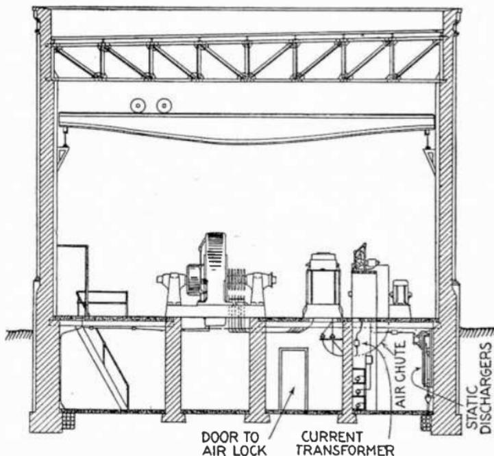
FIG. 4,778.—Plan of sub-station with air blast transformers and motor operated oil switches and underground 11,000 or 13,200 volt high tension lines.
