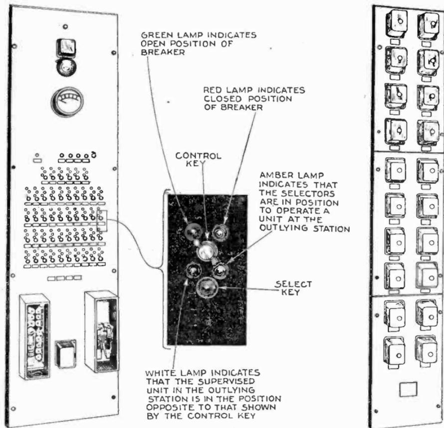
FIGS. 4,793 TO 4,795.—General Electric supervisory equipment: *Dispatchers' control equipment*.
