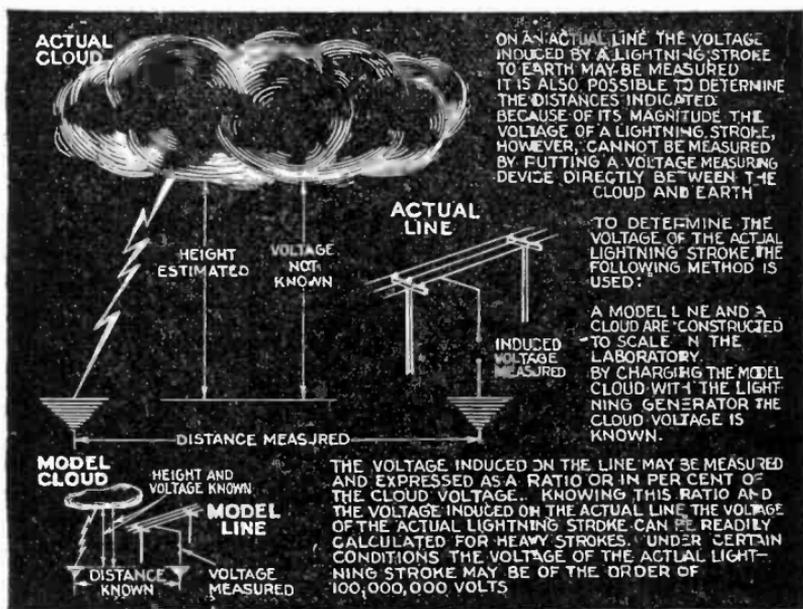
FIGS. 4,393 and 4,394.—Method of measuring the voltage of an actual lightning stroke.
