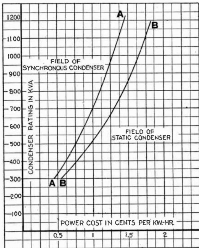
FIG. 4,238.—Curves showing fields of application for static and synchronous condensers 2,300 volt service, 60 cycles.
