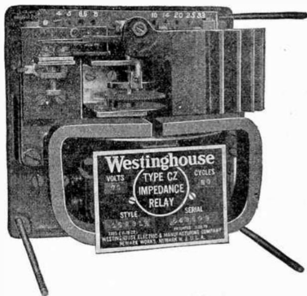
FIG. 4,224.—Westinghouse non-directional impedance relay with cover removed.
