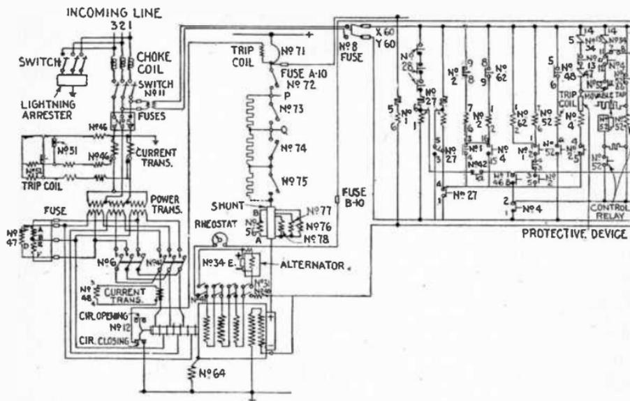
FIG. 4,786.—Wiring diagram of a typical automatic sub-station.
