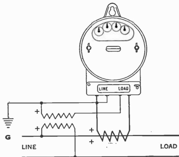
FIG. 4,495.—Connections for Sangamo type H primary meter with current and potential transformers, all capacities.
