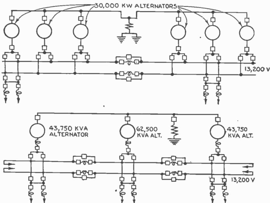
FIGS. 4,766 and 4,767.—Typical examples of "H" system.
