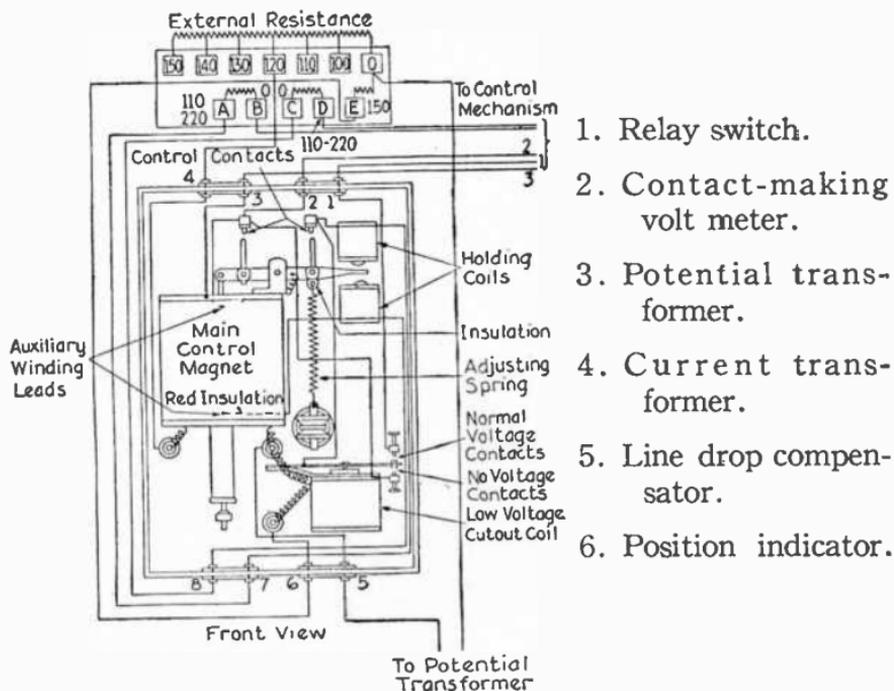
FIG. 4,289.—Contact making volt meter connections.
