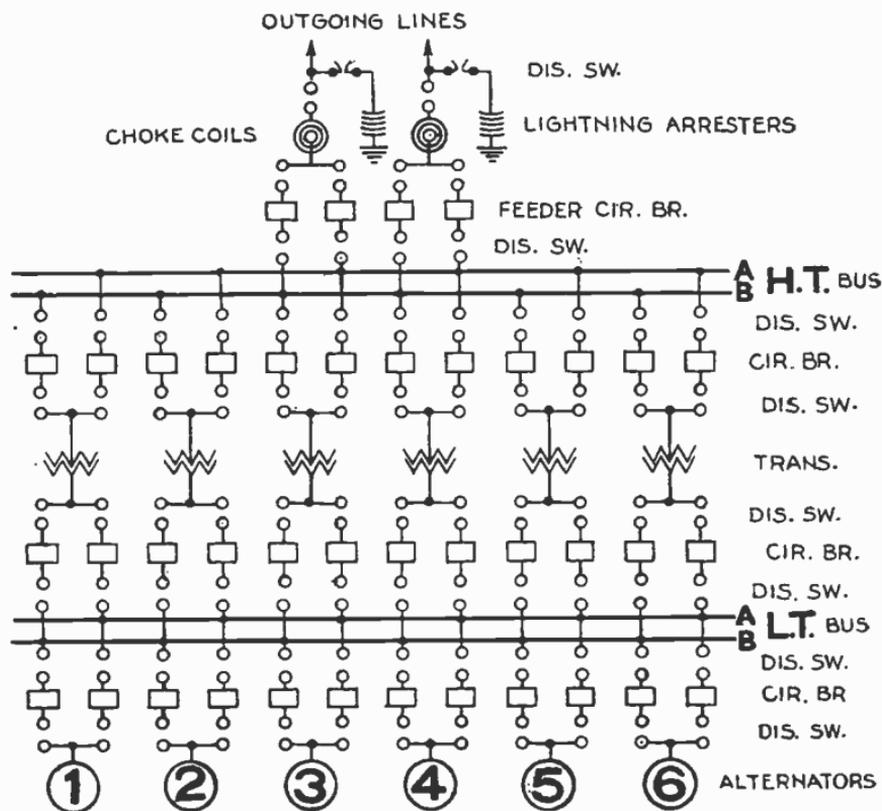
FIG. 4,775.—Double bus, double circuit breaker system. This arrangement permits the use of any or all of the alternators, without regard to which of the transformers may be in operation. It is particularly suitable where the station output is taken over but two or three transmission lines to the same destination.
