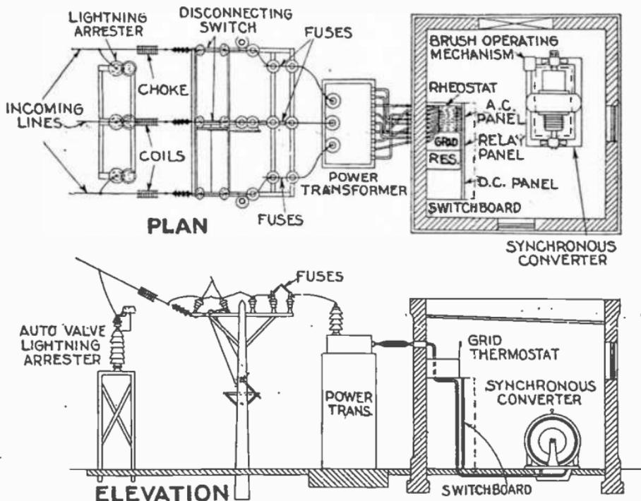
Figs. 4,787 and 4,788.—Plan and elevation of typical outdoor semi-automatic sub-station.
