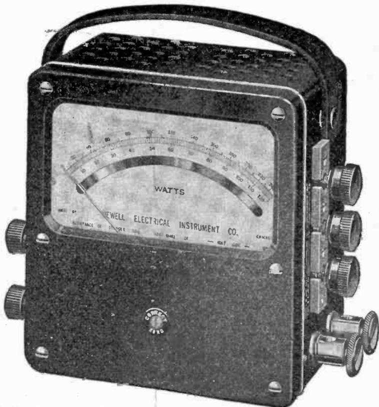
FIG. 4,872.—Jewell two scale single phase portable testing watt meter. The moving element is effectively shielded from outside magnetic fields by a special laminated construction. The method of obtaining series and parallel readings is such as to avoid metal links.
