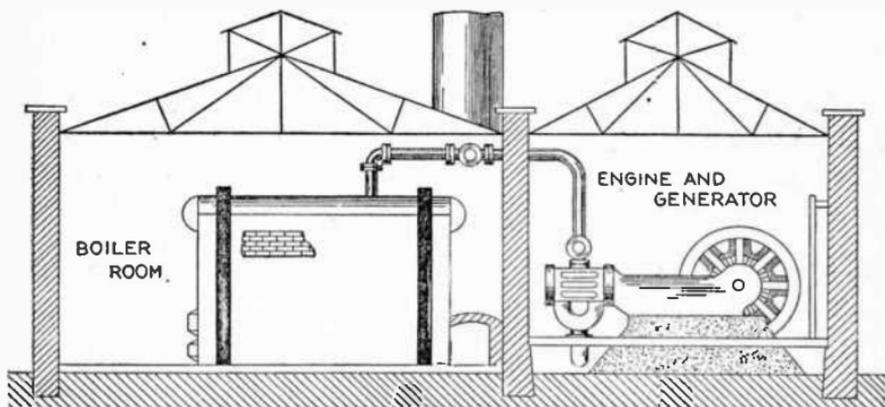
FIG. 4.728.—Elevation of small station with direct drive, showing arrangement of the boiler and engine, piping, etc.
