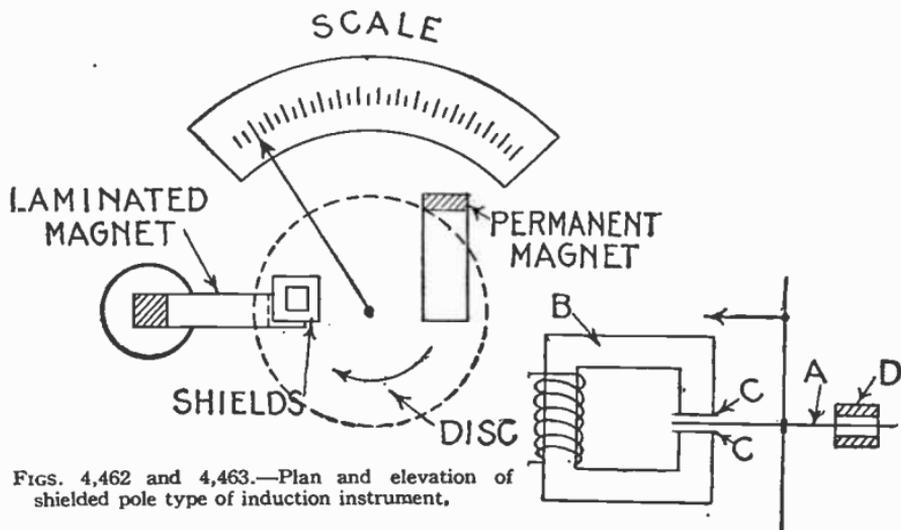
FIGS. 4,462 and 4,463.—Plan and elevation of shielded pole type of induction instrument,
