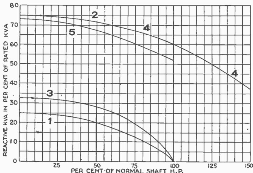
FIG. 4,260.—Curves for synchronous motors; reaction *kva.* available for power factor correction at different *h.p.* outputs. Assume motor field current is held constant at normal value. These curves are based on average values and therefore are approximate. 1, 1 *p.f.* belt driven motors; 2, .8 *p.f.* belt driven motors; 3, 1 *p.f.* air compressor motors; 4, .8 *p.f.* motors of 50% overload MG sets; 5, .85 *p.f.* motors of continuous rated MG sets.
