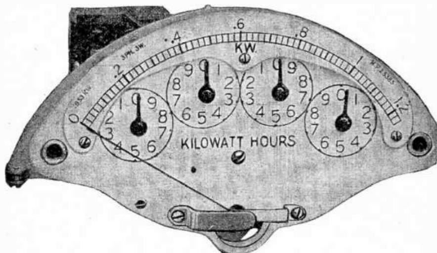
FIG. 4,512.—General Electric demand watt hour meter register. Scale shown is for 5 ampere, 110 volt, 3 wire, 3 phase meter.
