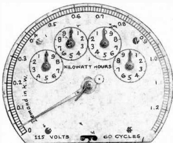
FIG. 4,525.—Duncan maximum demand watt hour meter register dial; front view.
