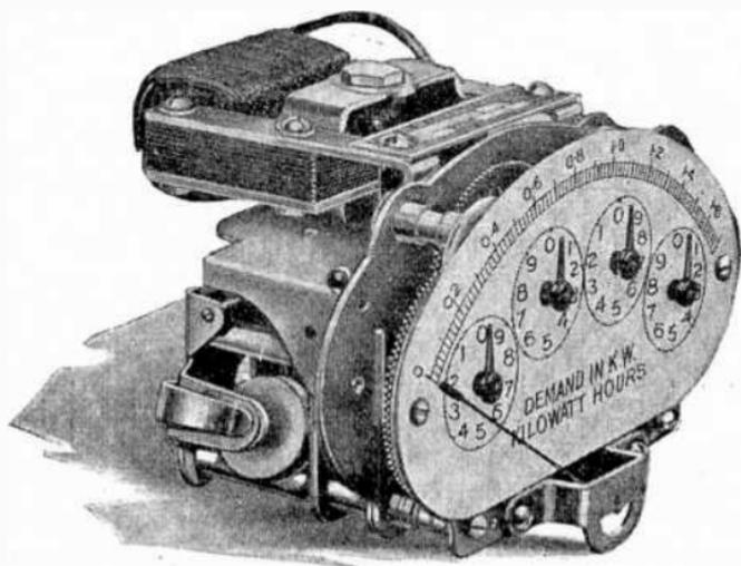
FIG. 4,535.—Front view of Sangamo maximum demand register, showing kw. demand scale and kw. hour cials for a 10 ampere, 110 volt, single phase meter.
