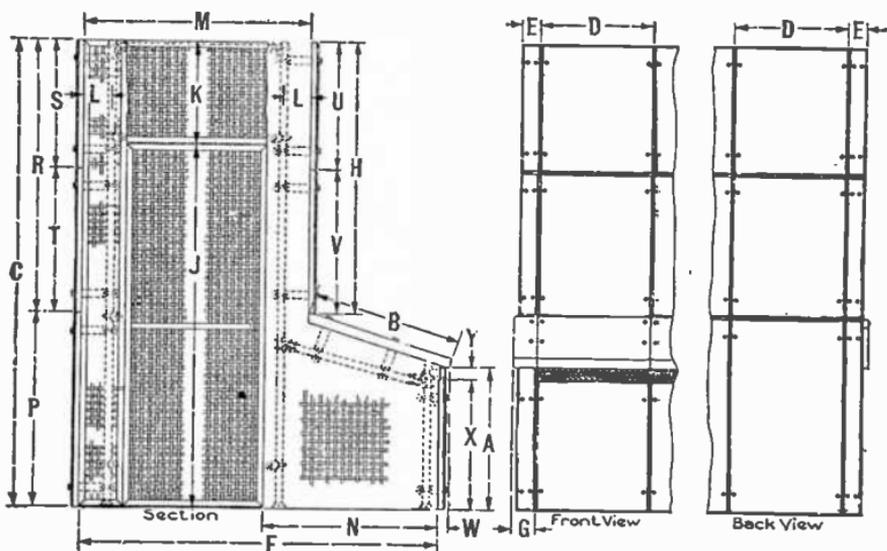
FIGS. 4,638 to 4,640.—Typical bench board construction. Fig. 4,638 cross section, fig. 4,639 front view; fig. 4,640, back view.
