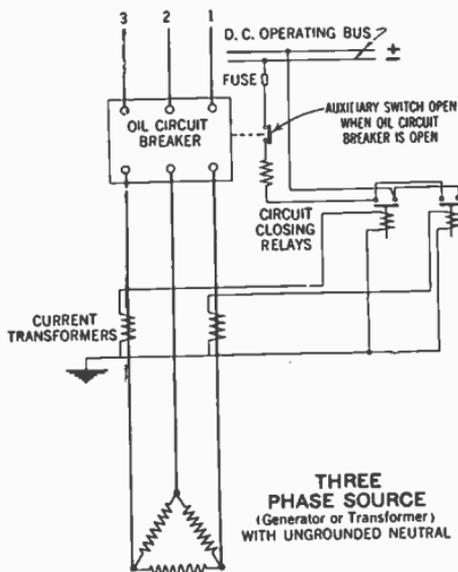
FIG. 6.—Indicating method of connection for over-current circuit-closing relays when a direct current source be available for tripping of the oil circuit breaker. Normally the trip coil circuit is open at the relay contacts. When the over-current becomes sufficiently large for the relays to close its contacts, the trip coil becomes energized tripping the oil circuit breaker, removing the machine or source from the over-load.
