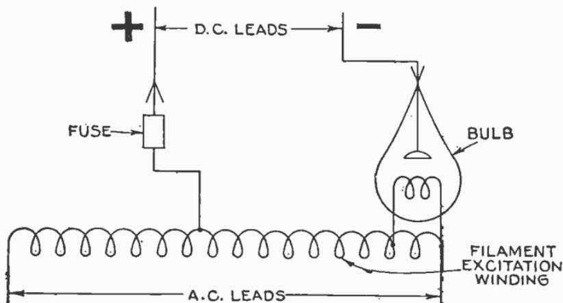
FIG. 4,372.—Half wave Rectigon schematic diagram of connections.
