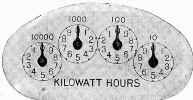
FIG. 4,504.—Sangamo single phase inductive watt hour meter register dial. The dial circles read 10, 100, 1,000, and 10,000 k.owatt hours from right to left.
