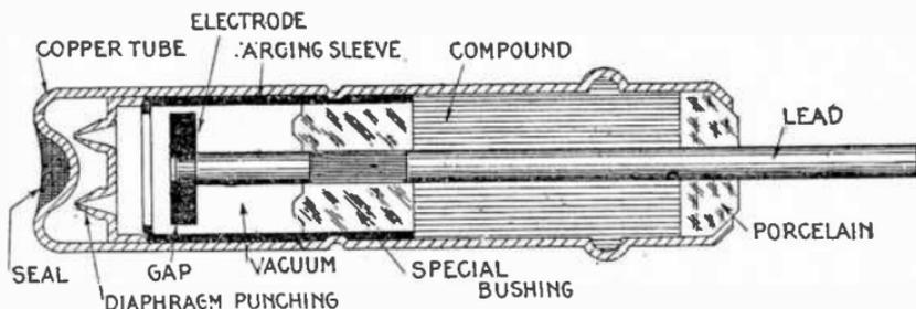
FIG. 4,440.—Sectional view of vacuum tube arrester for railway signal circuits. This arrester has a spark pressure of from 350 to 500 volts *d.c.* and an equivalent needle gap of about .005 inch. The arrester will not stand a continuous flow of current due to excessive heating, hence if there be a possibility of this due to high pressure crosses, fuses should be used.
