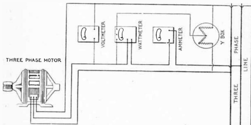
FIG. 4,877.—Three phase motor test; *one watt meter and Y box method.*
