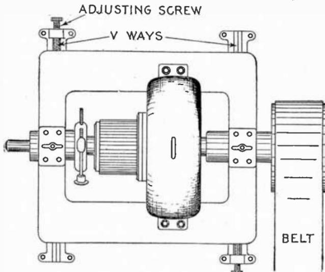
FIG. 4.822.—Plan of belt driven machine showing V ways and adjusting screws for moving the machine forward from the engine or counter shaft to take up slack in the belt.
