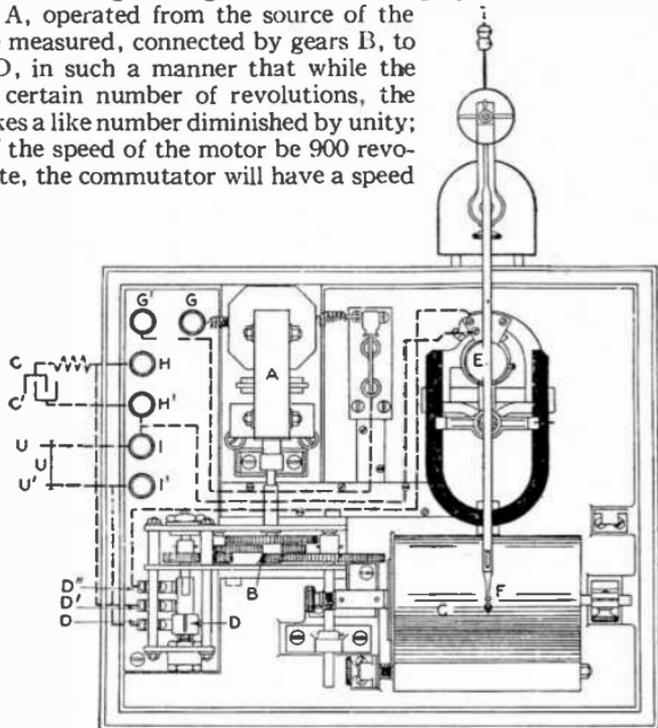
FIG. 4,609.—Diagram of Hospitalier ondograph showing mechanism and connections. It represents a development of Joubert's step by step method of wave form measurement.
