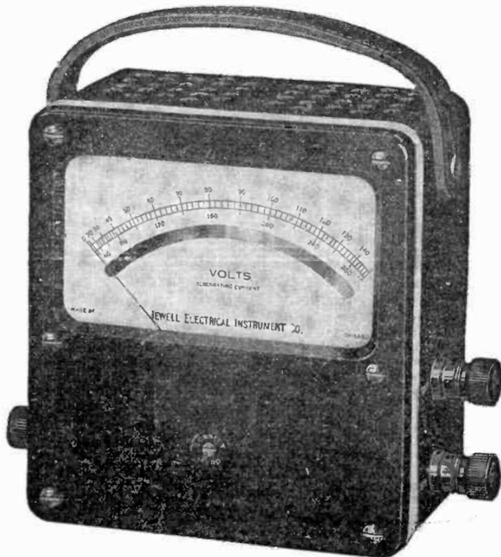
FIG. 4,858.—Jewel two scale *a.c.* portable testing volt meter. The *a.c.* movement used is shielded and is an advanced design of the repulsion iron vane type, embodying a bakelite form for the coil, a moulded bakelite damping chamber and a moving element, which is light, but rugged.
