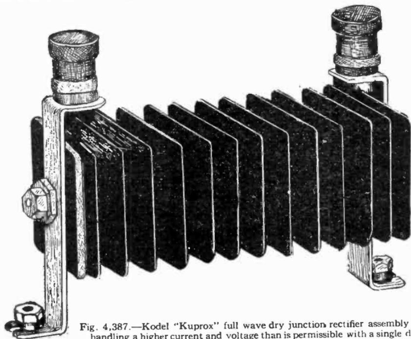
Fig. 4,387.—Kodel "Kuprox" full wave dry junction rectifier assembly for handling a higher current and voltage than is permissible with a single disc.
