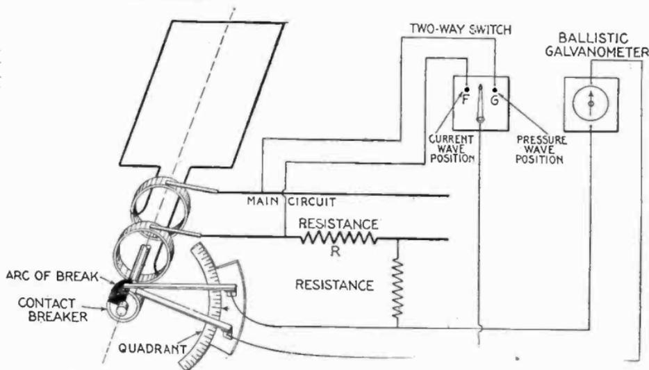
FIG. 4,608.—Diagram illustrating zero method of wave measurement with *contact breaker*. The voltage of the battery must be at least as great as the maximum pressure to be measured and must be kept constant.
