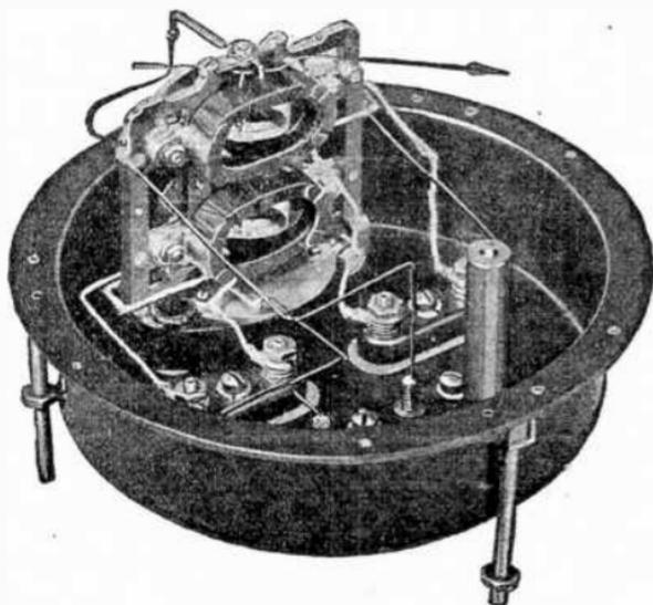
FIG. 4,507.—Westinghouse polyphase watt meter with cover and dial removed.
