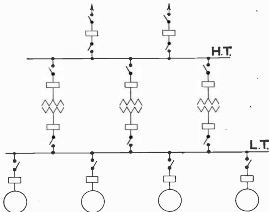
FIG. 4,768.—System using single low and high tension bus.
