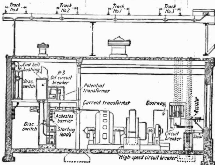
As a concrete illustration, assuming a 600 volt, normal trolley pressure the automatic equipment starts the synchronous converter or motor generator when the voltage falls for instance, to 540 volts or below.
