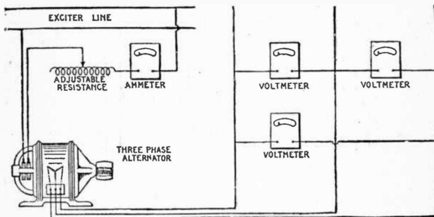
FIG. 4,880.—Alternator excitation or magnetization curve test.
