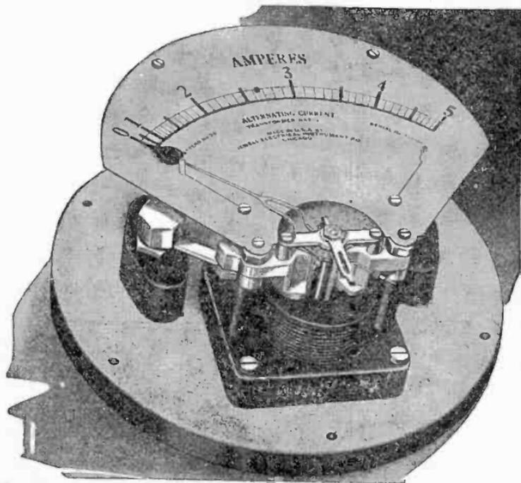
FIG. 4,459.—Jewell repulsion iron vane type instrument. *The principle of operation is the repulsion between two iron vanes which are magnetized by the surrounding coil.*
