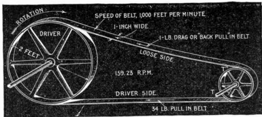
FIG. 4,830.—Conditions for transmitting one horse power by belt. *Rule:* A single belt one inch wide and traveling 1,000 feet per minute will transmit one horse power; a double belt under the same conditions, will transmit two horse power.
