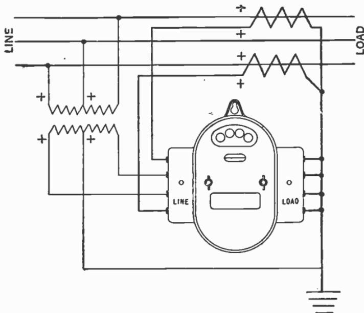
FIG. 4,506.—Connections for Sangamo type H vertical polyphase meter, all capacities, 1,100 volts and above, two and three phase with current and potential transformers.
