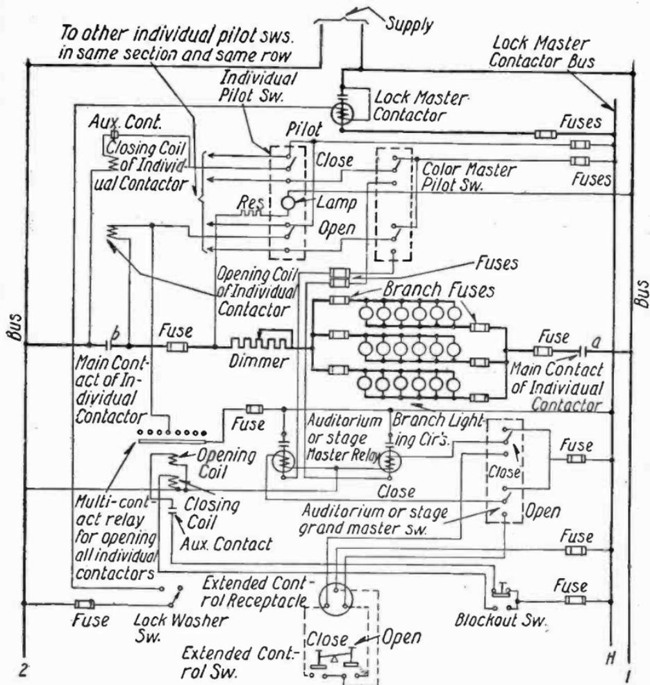
FIG. 4,723.—Westinghouse diagram of connections of a pre-selective type theatre switchboard.
