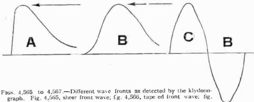
FIGS. 4,565 to 4,567.—Different wave fronts as detected by the klydonograph. Fig. 4,565, sheer front wave; fig. 4,566, tapered front wave; fig. 4,567, alternating wave.
