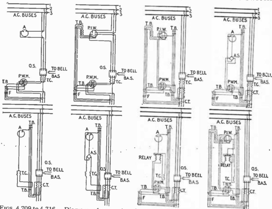
FIGS. 4,709 TO 4,716.—Diagrams of connections for three phase feeder panels. **Key to symbols:** A, ammeter; A.S., three way ammeter switch; B.A.S., bell alarm switch; C.T., current transformer; F, fuse; O.S., oil switch; P.I.W., polyphase indicating watt meter; P.W.M., polyphase watt hour meter; T.B., terminal board; T.C., trip coils for oil switch.
