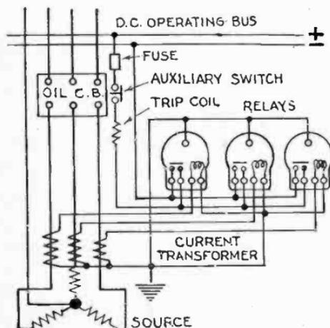
FIG. 4,220.—Connections for three phase, four wire circuit with General Electric induction overload relay. Auxiliary switch open when oil circuit breaker is open.
