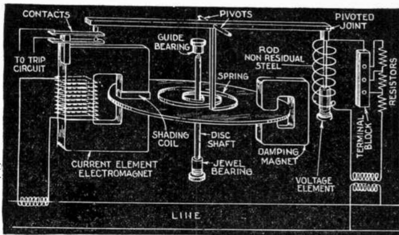
FIG. 4,227.—Pictorial diagram of Westinghouse impedance (distance) relay. As usually applied this relay requires for its operation the use of current and voltage transformers. The current element tries to close its contacts in a time varying inversely as the current whereas the voltage coil holds them open for a time varying directly as the voltage. Stated mathematically
