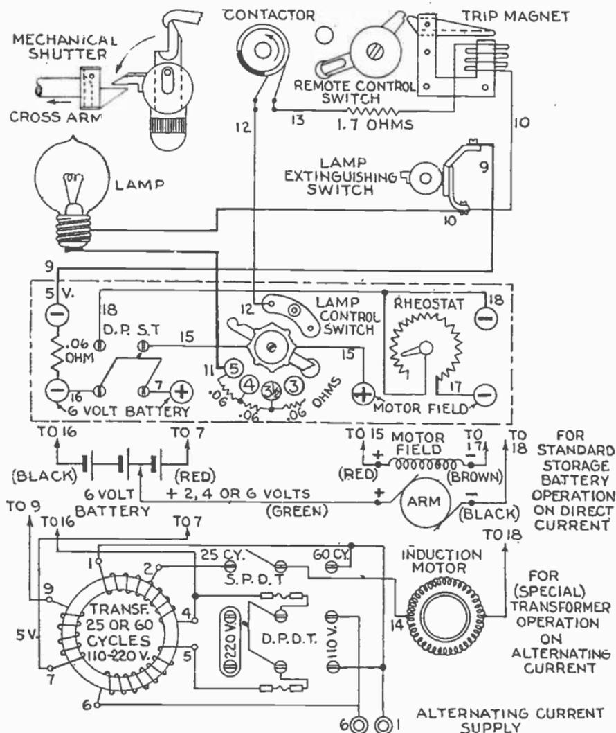
Figs. 4,624 and 4,625.—Connection diagrams of Westinghouse six element portable oscillograph, showing hook ups for d.c. and a.c. operation.
