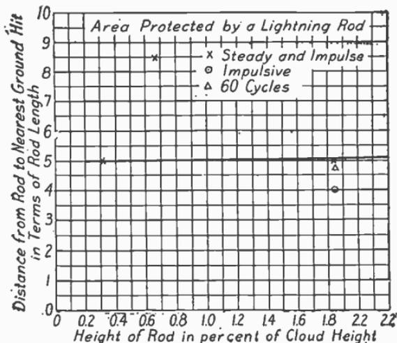
FIG. 4,422.—Area protected by a lightning rod.
