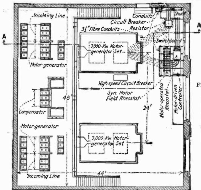
Figs. 4,781 and 4,782.—Plan and transverse section of General Electric 4,000 kw. automatic substation installed by N. Y. C. R.R. Co. at 110th St., N. Y. City.
