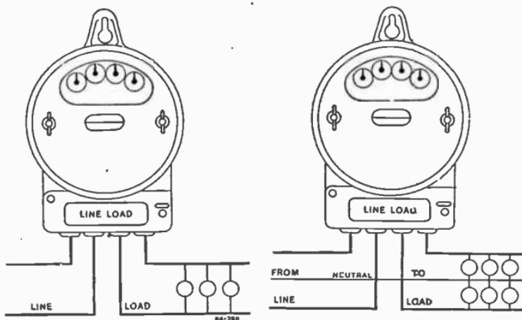
FIG. 4,491.—Sangamo type H single phase watt hour meter. Two wire, capacity 5 to 100 amperes inclusive.
