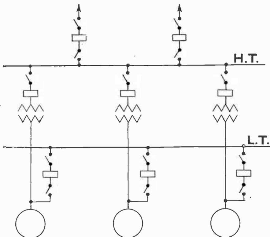
FIG. 4,770.—Common arrangement where station is at a distance from the load center.
