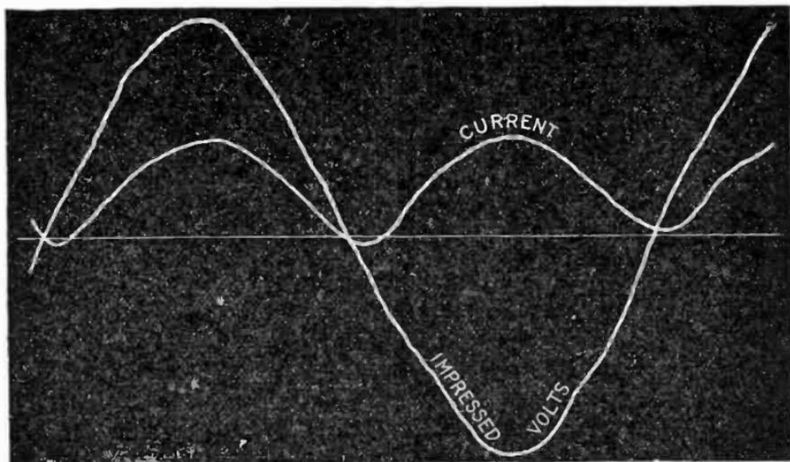
FIG. 4,348.—Oscillograph record from Nodon valve showing original supply voltage and the corresponding pulsating current at the terminals of such a valve.
