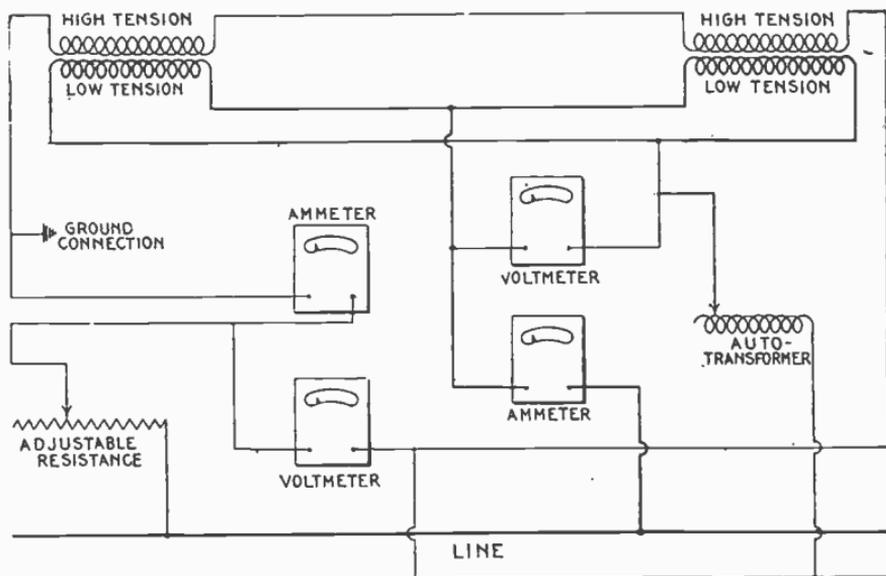
FIG. 4,866.—Transformer temperature "bucking test."
