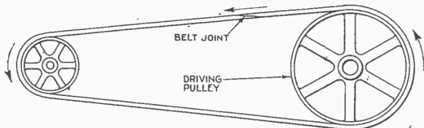
FIG. 4832—Inclination of belt lap joint. *Rule:* The leading point of the joint should be on the outside when the driven pulley is the smaller, but on the inside when the driving pulley is the smaller of the two.
