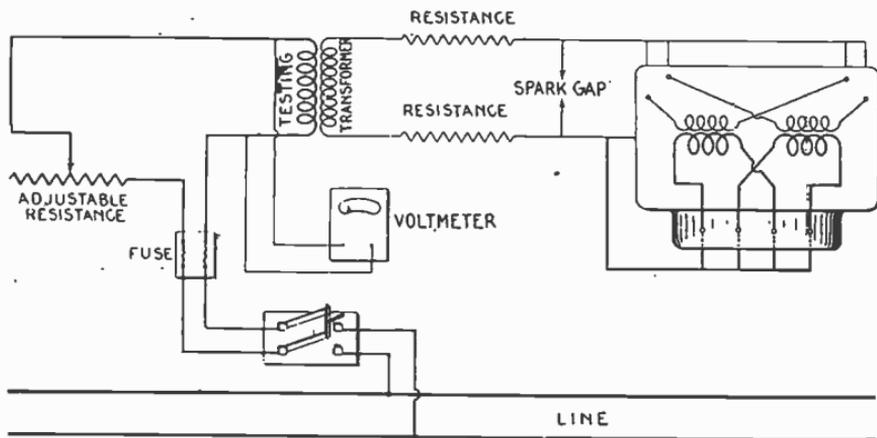
FIG. 4,867.—Transformer insulation test.
