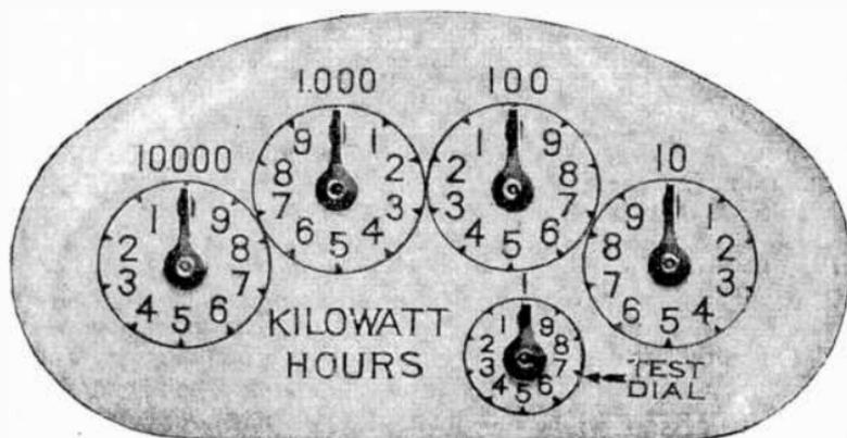
FIG. 4,505.—Sangamo single phase inductive watt hour meter register dial with test dial. It has a small test circle indicating one kilowatt hour per revolution in all sizes where the first regular circle indicates 10. This is provided to conform with the requirements of the Canadian Government and it is intended that the hand on the test circle shall make not less than  $\frac{1}{2}$  revolution in one hour with full load on a meter.
