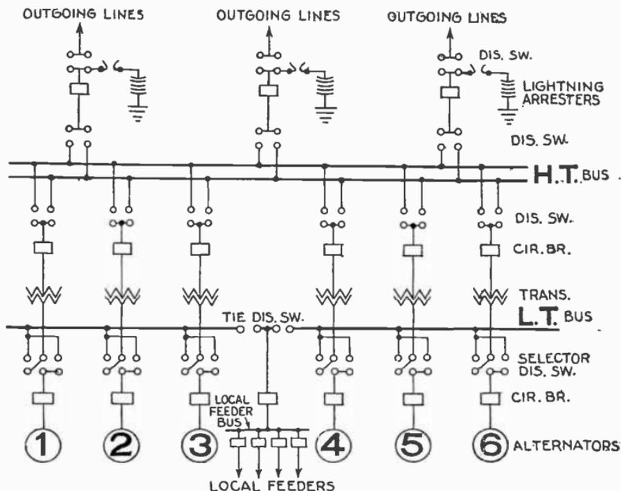
FIG. 4,776.—Single low tension, double high tension bus, single circuit breaker scheme. Low tension disconnecting switches permit the connection of an alternator direct to a transformer (with or without connection to bus bar) connection of alternator to bus bar with transformer dead or connection of transformer to bus bar with alternator dead. All apparatus may be in service while the load is removed from either section of either bus bar for repairs or additions.
