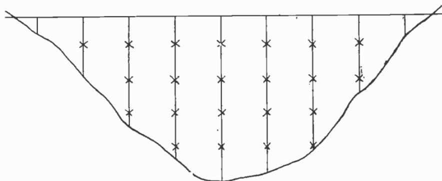
FIG. 4,759.—Method of measuring large flows.
