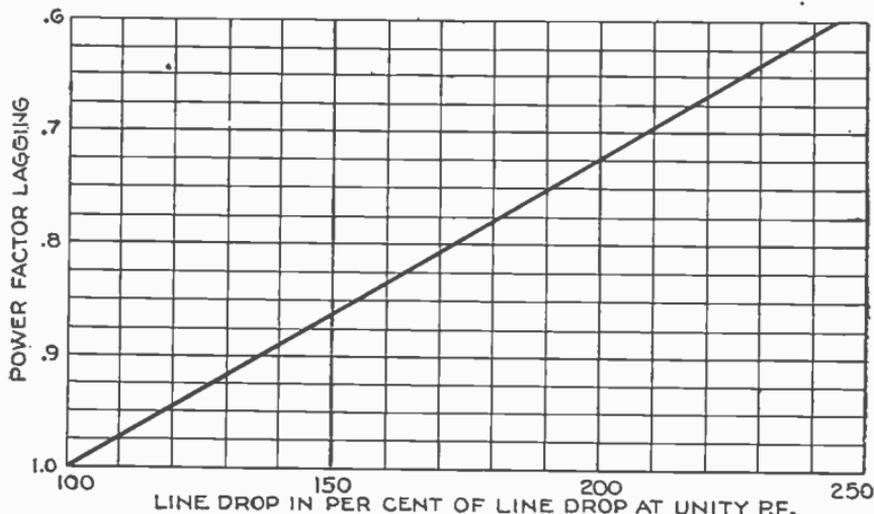
FIG. 4,246.—Curve showing relation between power factor and line drop for constant *kw.* load over a 1000 ft. 3 phase, 60 cycle circuit of No. 0 wire, 9 in. spacing, 440 volts at motor. It will be noted that the drop increases more rapidly than the power factor decreases, which in turn is due to the reactance of the circuit. This circuit might be considered as typical.
