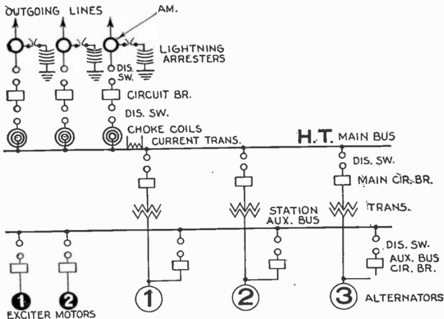
FIG. 4,777.—Single high tension bus scheme. The alternator and transformer are treated as a unit and all low tension switching is thereby omitted. The station auxiliaries are fed from any alternator or transformer circuit by means of the auxiliary bus.
