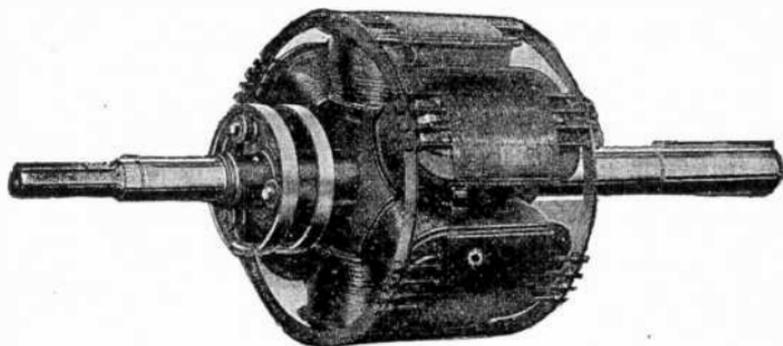
FIG. 4,257.—Field of a synchronous condenser. Note the *amortisseur winding*, erroneously called *squirrel cage winding*, consisting of two end rings which serve to short circuit spokes passing through the pole tips as shown. The *amortisseur winding* assists in starting and serves also as a damping device to minimize hunting.
