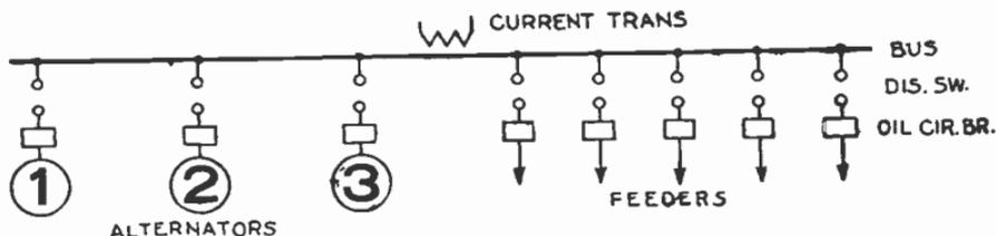
FIG. 4,761.—Single bus, single circuit breaker system
