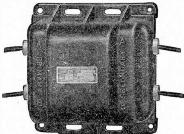
FIG. 4,466.—Jewell potential transformer. Rated at 25 volt amperes, and will amply take care of the load of several instruments. The relative polarity of the terminals is clearly marked so that watt meters and power factor meters can be connected up, knowing that they will indicate correctly.
