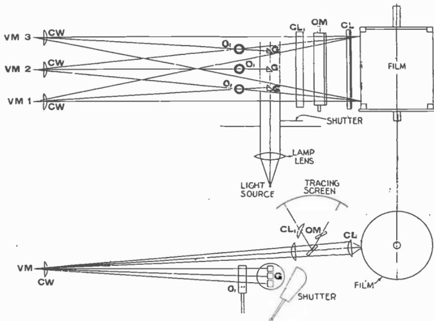
FIGS. 4,603 and 4,604.—Diagram of optical system of General Electric oscillograph. *The parts are:* VM, vibrator mirror; CW, cell window; O<sub>1</sub>, light cut-off; G, prism cylindrical; CL, cylindrical lens; OM, oscillating mirror.
