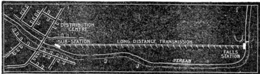
FIG. 4,734.—Example of central station located remote from the distributing center and furnishing alternating current at high pressure to a sub-station where the current is passed through step down transformers and supplied at moderate pressure to the distribution system. In some cases the sub-station contains also converters supplying direct current for battery-charging, electro-plating, etc.
