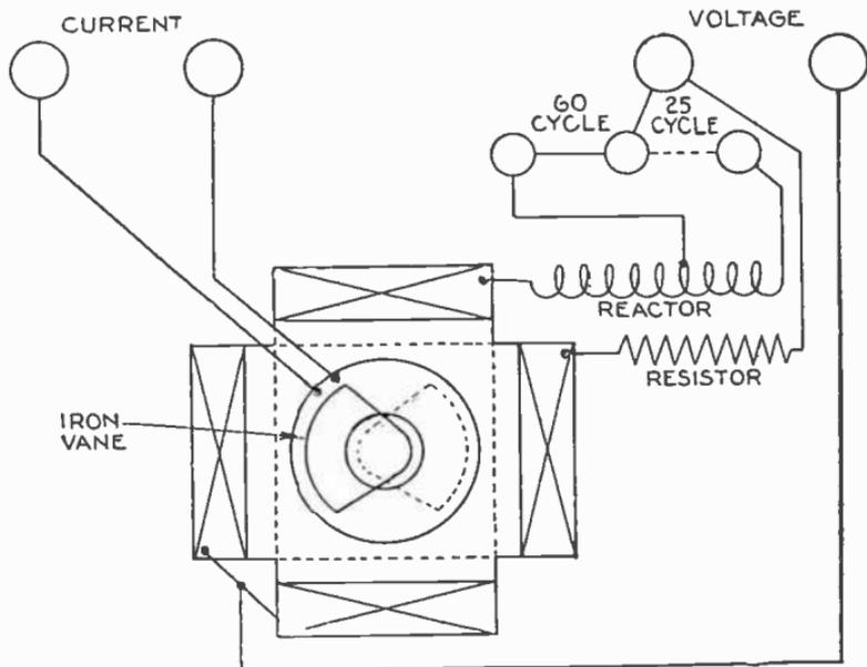
FIG. 4,546.—Diagram of Westinghouse portable phase indicator.
