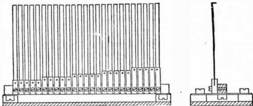
FIGS. 4,554 and 4,555.—Side and end views of Frahm resonance type frequency meter reeds. Owing to the principle employed in the meter it is evident that the indications are independent of the voltage, change of wave form, and external magnetic fields.
