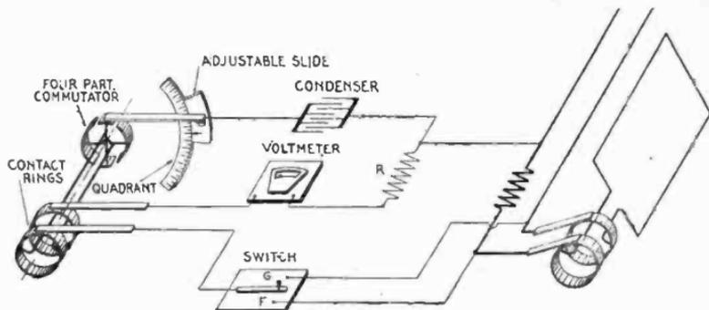
FIG. 4,600.—*Four part commutator method* of wave form measurement. The contact device consists of two slip rings and a four part commutator. One slip ring is connected to one terminal of the source, the other to the voltmeter, and the commutator to the condenser. By adjusting  $R$ , when a known direct current pressure is impressed across the terminals, the volt meter can be rendered direct reading.
