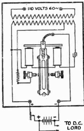
FIG. 4,337.—Circuit diagram of Leich electro-magnetic rectifier, railroad type.
