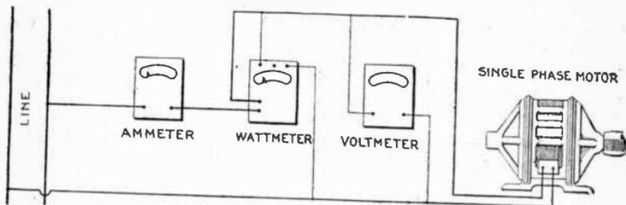
FIG. 4,873.—Single phase motor test.
