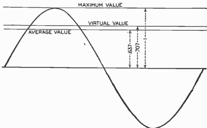
FIG. 4,443.—Sine curve of alternating current, illustrating various current or pressure values. The virtual value, or  $.707 \times$  maximum value, is the value indicated by an ammeter or volt meter. Thus, if the maximum value of the current be 100 volts, the virtual value as indicated by an ammeter is  $100 \times .707 = 70.7$  amperes.
