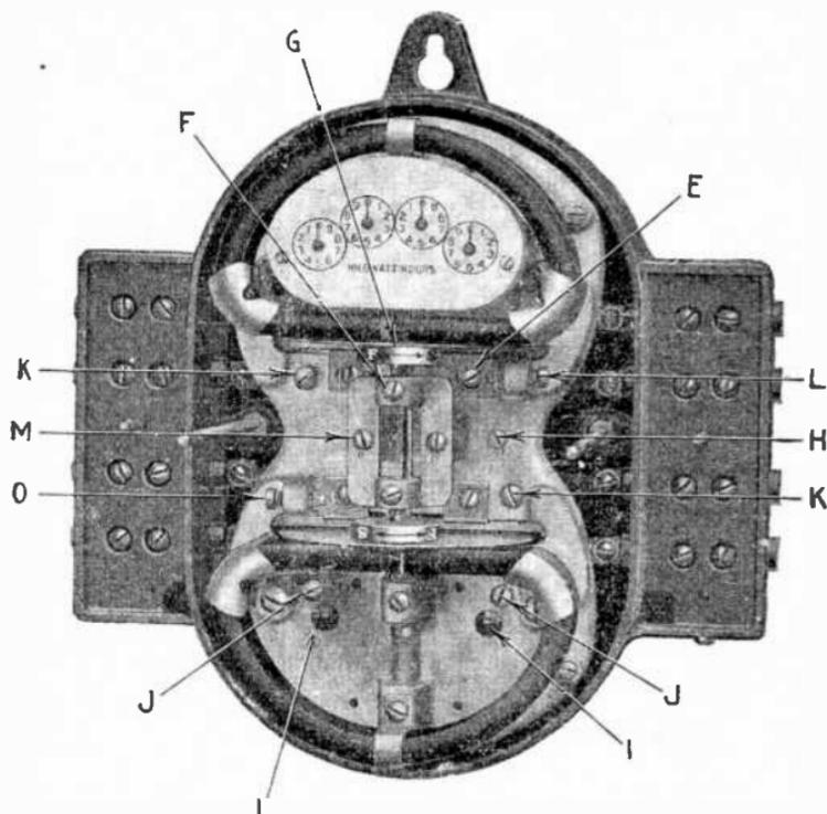
FIG. 4,500.—Duncan polyphase induction watt hour meter. *The parts are:* L and O, light load adjustment screws; E, upper light load adjustment clamp screw; KK, balance adjustment clamp screws; H, balance adjustment screw; F, full load adjustment clamp screw; G, full load adjustment clamp; J, full load adjustment screw; JJ, inductive load adjustment clamp screws for lower element; II, inductive load adjustment for lower element; M, holding screw for dowelled full load adjustment screw plate.
