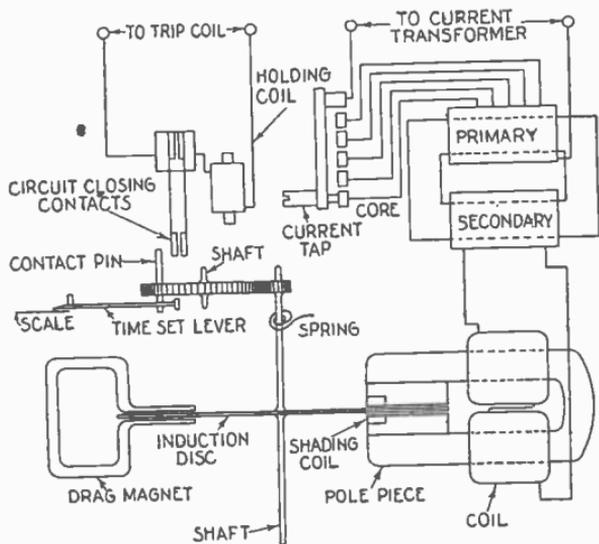
As shown in fig. 4,229 the movement of a contact pin on a gear closes the contacts. The current calibration is obtained by using different taps in the current coil, and in this way controlling the speed of the disc. The time calibration is obtained by adjusting the distance through which the disc travels before contact is made.
