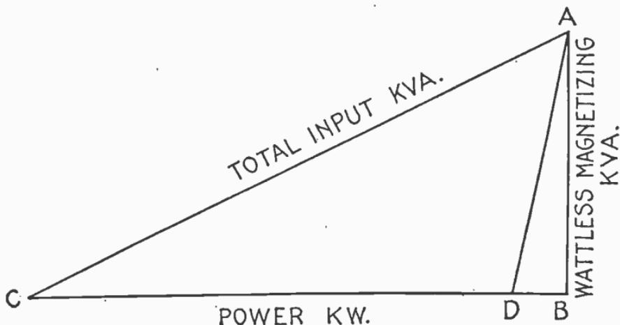
FIG. 4,241.—Diagram showing relative effect of fully loaded and lightly loaded induction motors on power factor.
