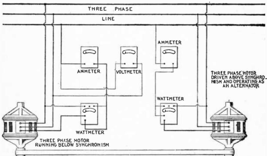
FIG. 4,879.—Temperature test of a large three phase induction motor.
