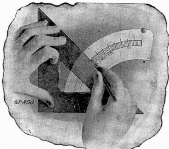
FIG. 4,446.—A *calibrated* scale. This means that printed scales are not employed, but each instrument has its scale divisions plotted by actual comparison with standards, after which the division lines are inked in by a draughtsman. There are makes of direct current instruments employing printed scales in which the scale deflections are fairly accurate, even though the scales are printed, but printed scales should not be used on alternating current instruments.
