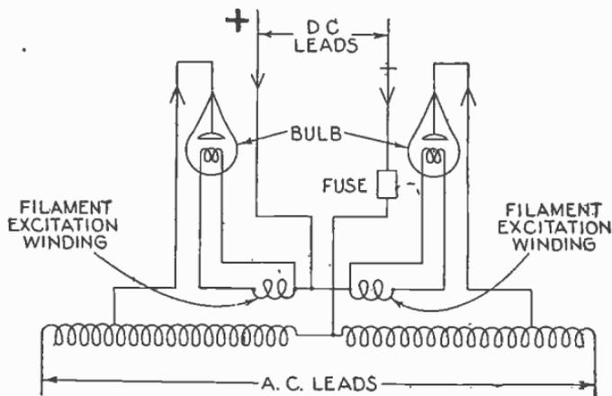
FIG. 4,373.—Full wave Rectigon schematic diagram of connections.
