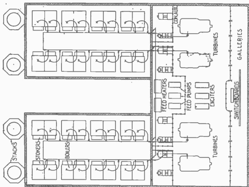
Fig. 4.748.—Arrangement commonly adopted for 15,000 and 20,000 kw. turbines.
