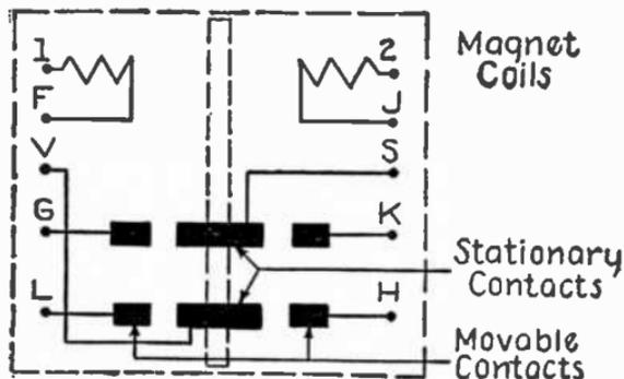
FIG. 4,287.—Wiring diagram of relay switch.
