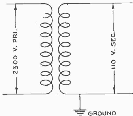
FIG. 4,850.—Low tension grounding for single phase transformer, two wire system. This method should not be used for pressures over 250 volts. The ground wire should be of the same size as the transformer leads.
