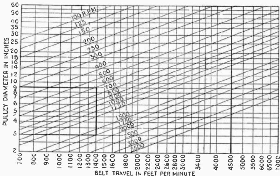
FIG. 4,829.—Chart for finding belt travel in feet per minute.
