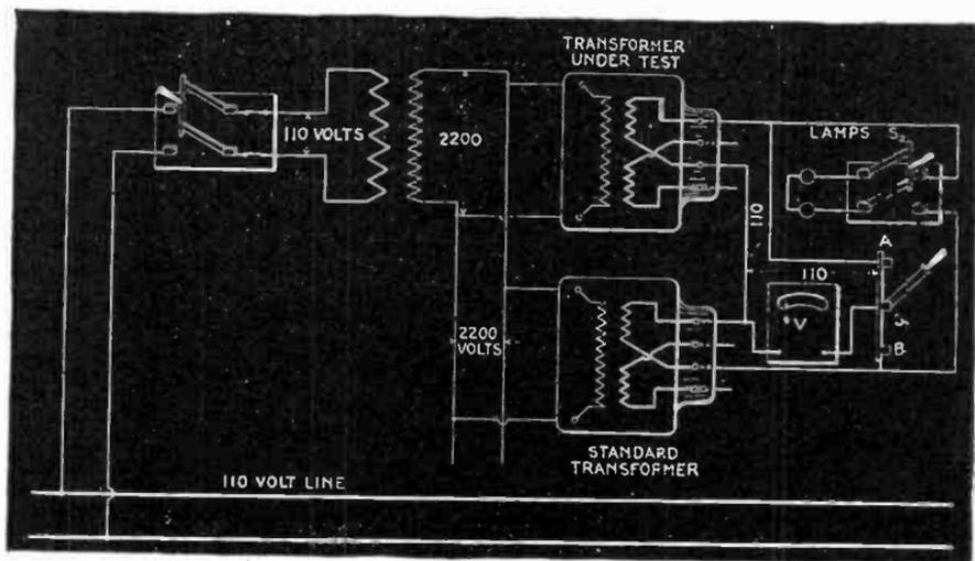
FIG. 4,871.—Transformer winding or ratio test.
