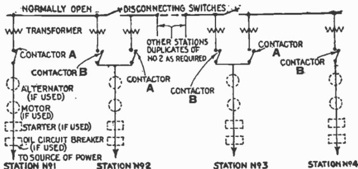
FIG. 4,804.—Diagram of General Electric automatic switching system, for *a.c.* railway signal and train control feeders. Two classifications of feeder equipments are made: 1, operation *without a.c.* reclosing relay; 2, operation *with a.c.* reclosing relay. The operation is described for any section of the line, a section consisting of the line with an A, contactor at one end and a B, contactor at the other.
