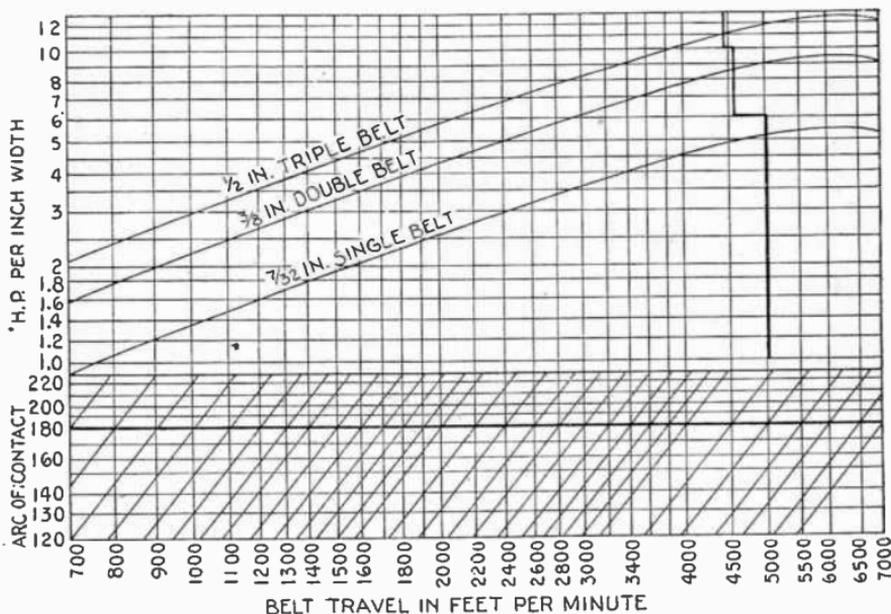
FIG. 4,831.—Chart for calculating belt horse power. Leather belt on iron pulley. Maximum permissible stress 400 lbs. per sq. in. For paper pulleys add 30% to *h.p.* For 4 ply canvas or rubber use single belt curve.
