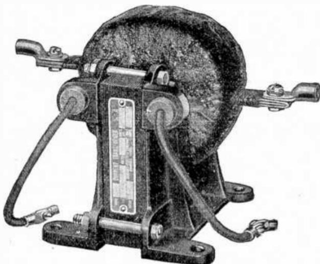
FIG. 4,467.—Jewell two wire current transformer. Rated capacities from 5 to 400 amperes inclusive, for a nominal secondary reading of 5 amperes and is rated at 15 volt amperes. This type will function satisfactorily at any frequency from 25 to 133 cycles and is insulated for 3,300 volts.
