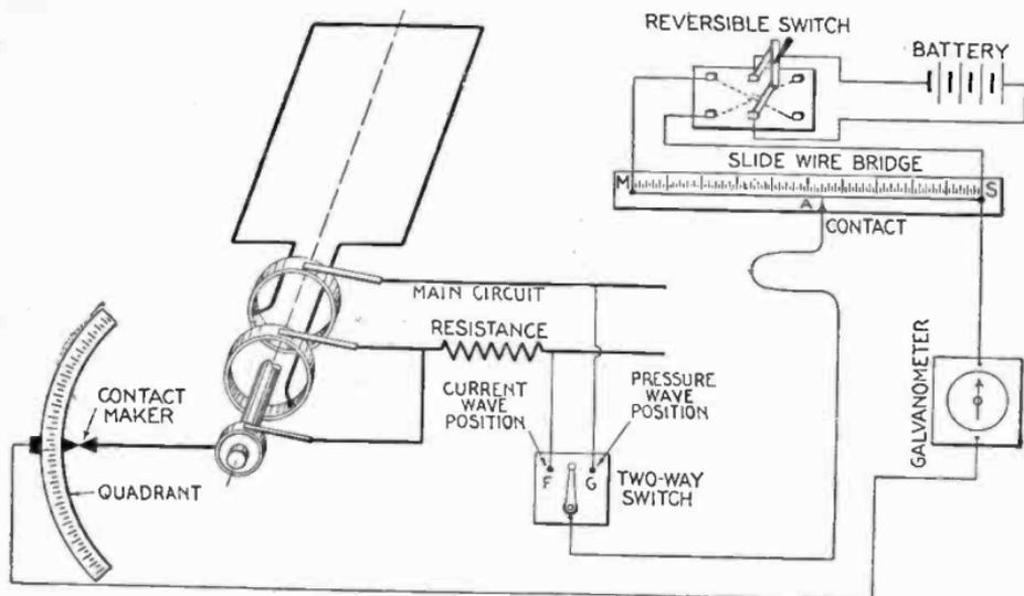
FIG. 4,607.—Diagram illustrating zero method of wave measurement with *contact maker*. The voltage of the battery must be at least as great as the maximum pressure to be measured and must be kept constant.
