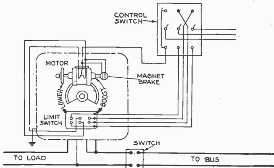
FIG. 4,282.—General Electric connection diagram for motor operated feeder induction voltage regulator using three phase operating motor.
