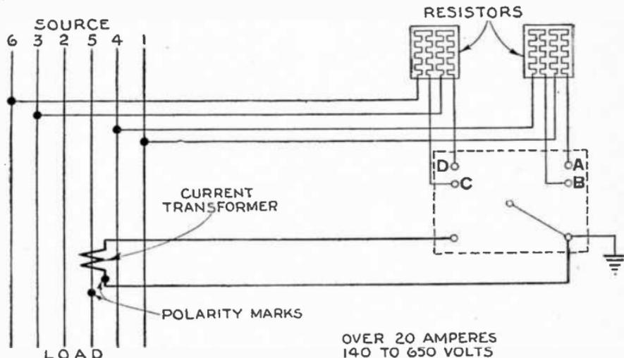
FIG. 4,540.—Connection diagram for General Electric power factor meter; 6 wire, 4 phase circuits.
