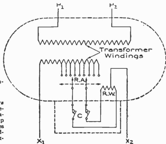
FIG. 4,306.—General Electric load ratio control in a Y connected transformer.
