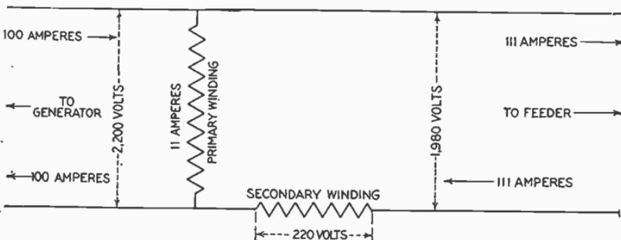
FIG. 4,279.—Diagram of induction regulator *lowering the voltage 10%*. The diagram shows the regulator lowering the feeder pressure to 1,980 volts with an increase of the secondary current to 111 amperes, the additional 11 amperes flowing from the feeder, through the primary back to the feeder.
