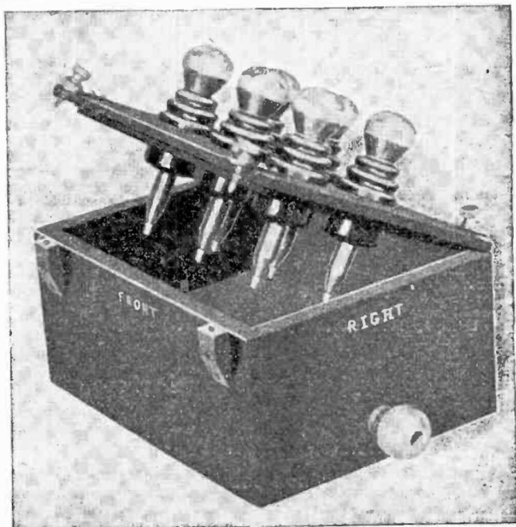
FIG. 4,568.—Type of klydonograph used to record the surges shown in the accompanying illustrations.
