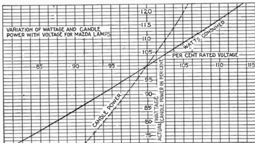
FIG. 4,277.—Curves showing variation of wattage and candle power with voltage for Mazda lamps. The curves show that a slight variation in voltage seriously affects the performance of the lamp. For example, a 2% drop reduces the candle power to 93½% of normal and the wattage to 96¼% of normal.
