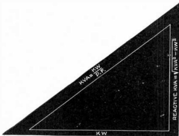
FIG. 4,240.—Vector diagram of a typical a.c. load.
