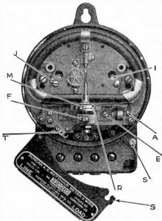
FIG. 4,496.—Duncan single phase induction watt hour meter with register removed. *The parts are:* A, light load adjustment screw; E, light load adjustment clamp screw; S, terminal chamber cover sealing screw; S, sealing ear on terminal chamber cover; R, disc; T, test link; F, full load adjustment clamp screw; M, full load adjustment screw; J, inductive load adjustment clamp screw; I, inductive load adjustment.
