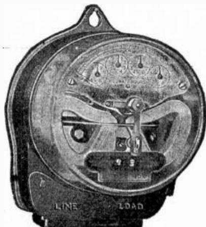
FIG. 4,514.—General Electric polyphase watt hour demand meter.
