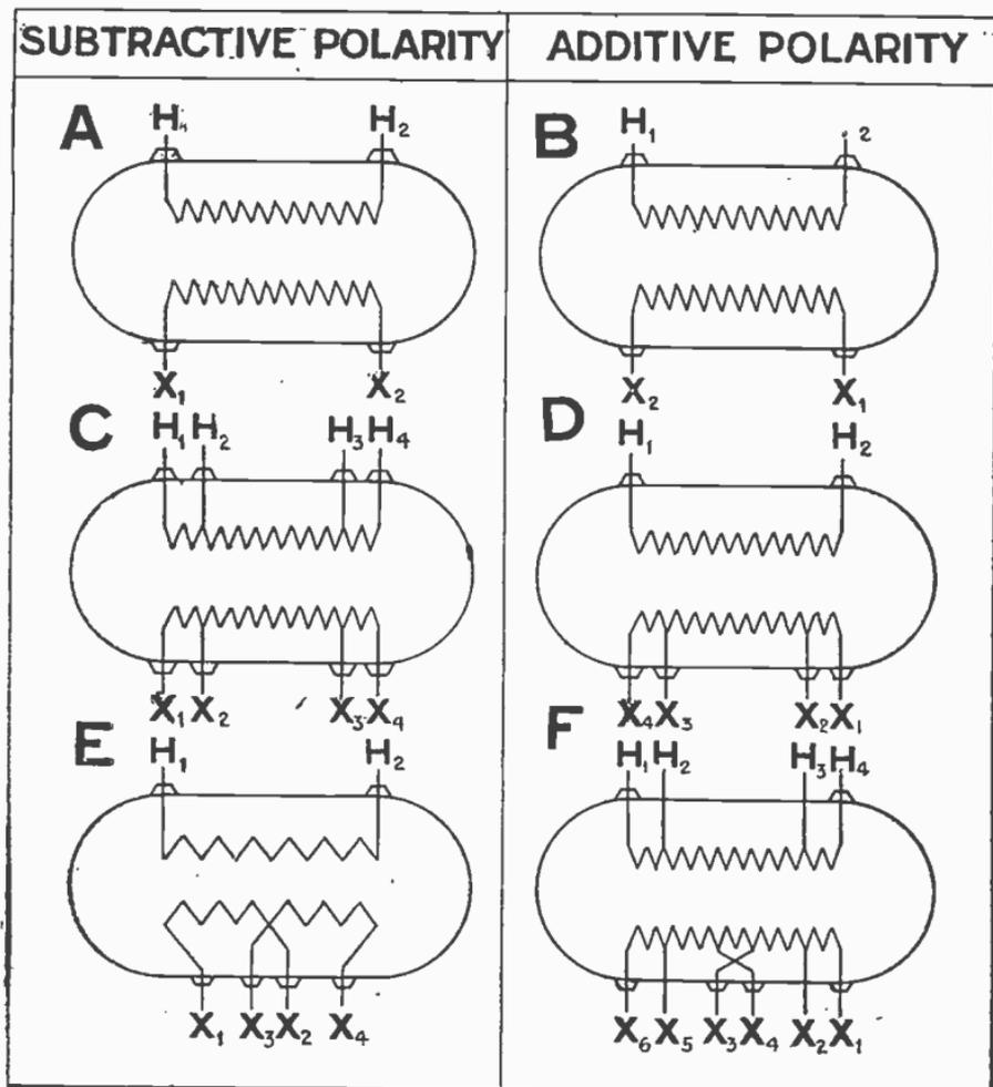
FIGS. 4,813 to 4,818.—Lead markings; single phase transformers. **A** and **B**, simple high and low voltage windings without taps; **C** and **D**, simple high and low voltage windings, with taps; **E**, series parallel low voltage winding without taps; **F**, series parallel low voltage winding, with taps. The leads are marked.
