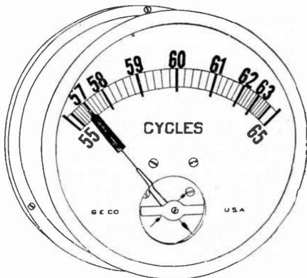
FIG. 4,559.—General Electric resonant circuit type frequency meter.
