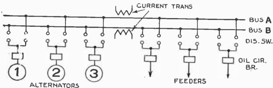
FIG. 4,762.—Double bus, single circuit breaker system. This arrangement greatly increases the chances for continuity of service over that shown in fig. 4,761. One bus bar may be used as an auxiliary only, or one may feed a lighting load while the other feeds a power load.
