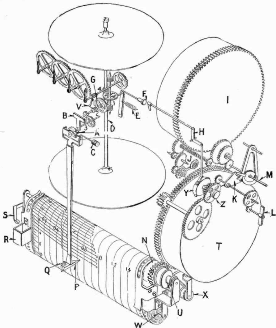
FIG. 4,532.—Westinghouse type RA recording watt hour demand meter. *In operation*, under load the disc shaft D, registers watt hours on the counter through the gearing of the shaft assemblies 1 and 4. At the same time, the ink carrying pen P, is positively advanced through shaft assemblies 1, 2, and 3. At the end of the time interval the tripping rod,
