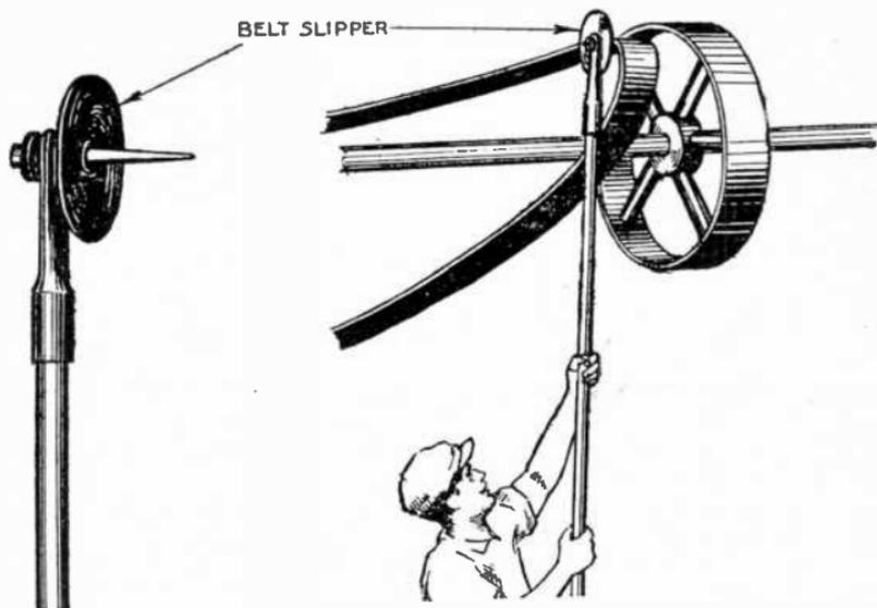
FIGS. 4,827 and 4,828.—Method of putting on belts when the driver is in motion, and device used. The latter is called a *belt slipper*, and consists, as shown in fig. 4,827, of a cone and shield, which revolve upon the stem, thus yielding easily to the pull of the belt. A staff or handle of any convenient length can be fastened to the socket. The mode of operation is illustrated in fig. 4,828, which is self explanatory.
