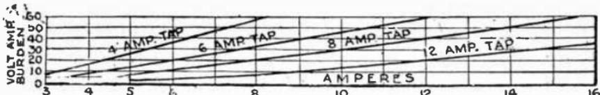
FIG. 2,436.—Characteristic curves showing burden placed on the current transformer with various currents flowing in the relay windings.
