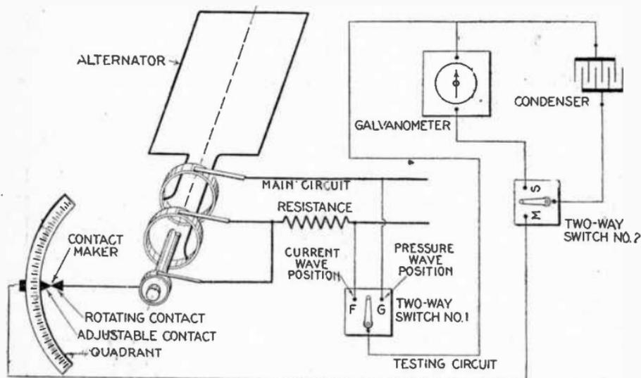
FIG. 4,599.—Diagram illustrating Joubert's *step by step method* of wave form measurement.
