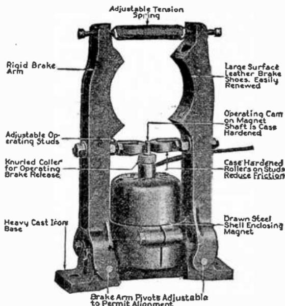
FIG. 4,283.—General Electric torque motor brake for motor operated automatic induction voltage regulator, station type.
