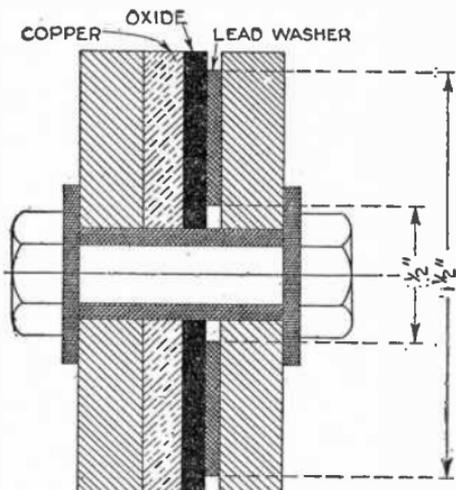
FIG. 4,389.—Assembly of single half wave rectifier.
