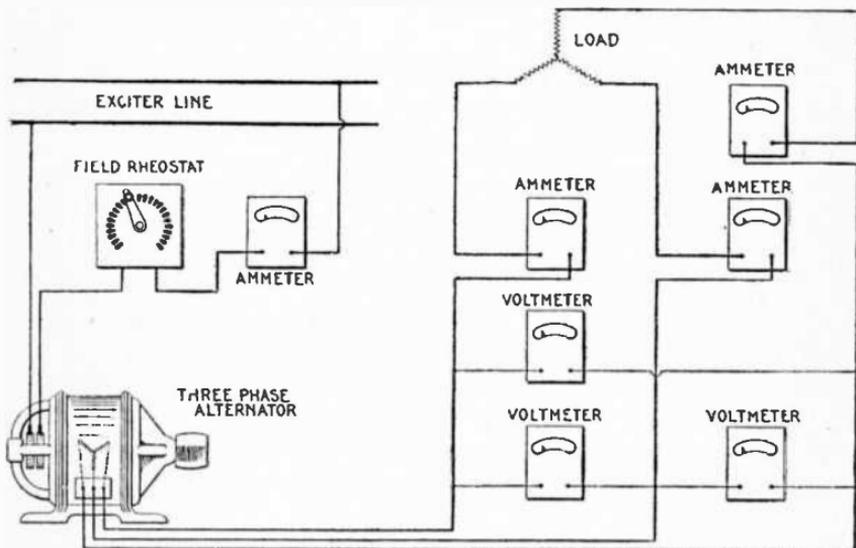
FIG. 4,881.—Three phase alternator synchronous impedance test.
