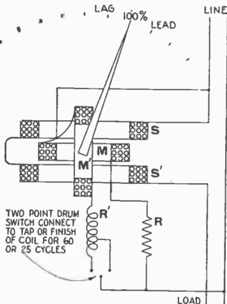
FIG. 4,543.—Diagram of single phase rotating field type power factor meter showing operation.
