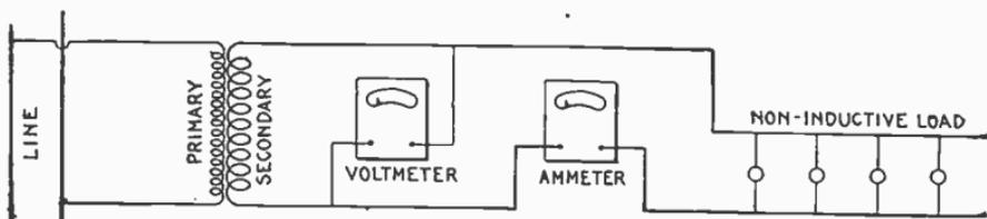
FIG. 4,865.—Temperature test of transformer with non-inductive load.
