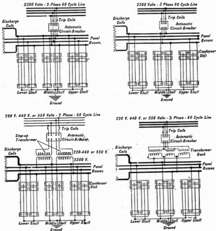
FIGS. 4,268 and 4,269.—Wiring diagrams for 2,300 volt static condensers. Fig. 4,268, two phase; fig. 4,269, three phase.
