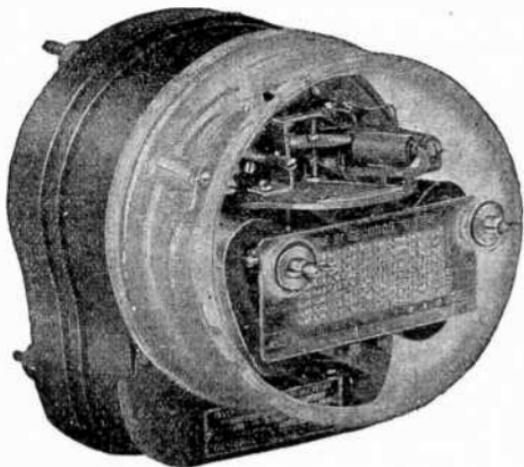
FIG. 4,211.—General Electric single pole induction overload relay. *The principles of operation* are similar to those of induction meters. These relays are *circuit closing* and operate with a time relay which is inverse at low current values and which approaches a definite time at high current values. *In operation*, the holding magnet keeps the contact closed until circuit breaker opens. The trip circuit must be opened by a separate auxiliary switch.
