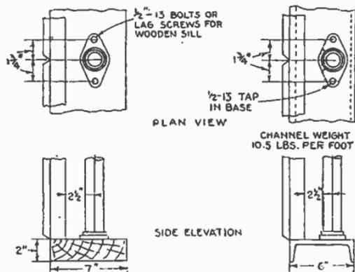
Figs. 4,626 to 4,629.—Standard sill and switchboard sub-base arrangements.
