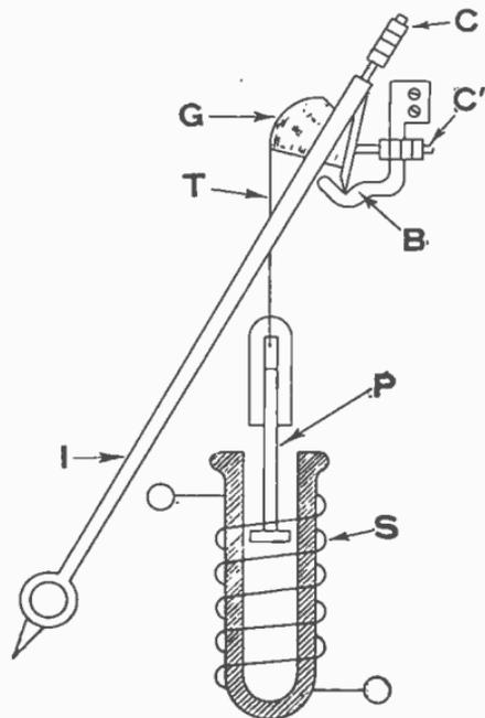
FIG. 4,450.—Kelvin solenoid principle.
