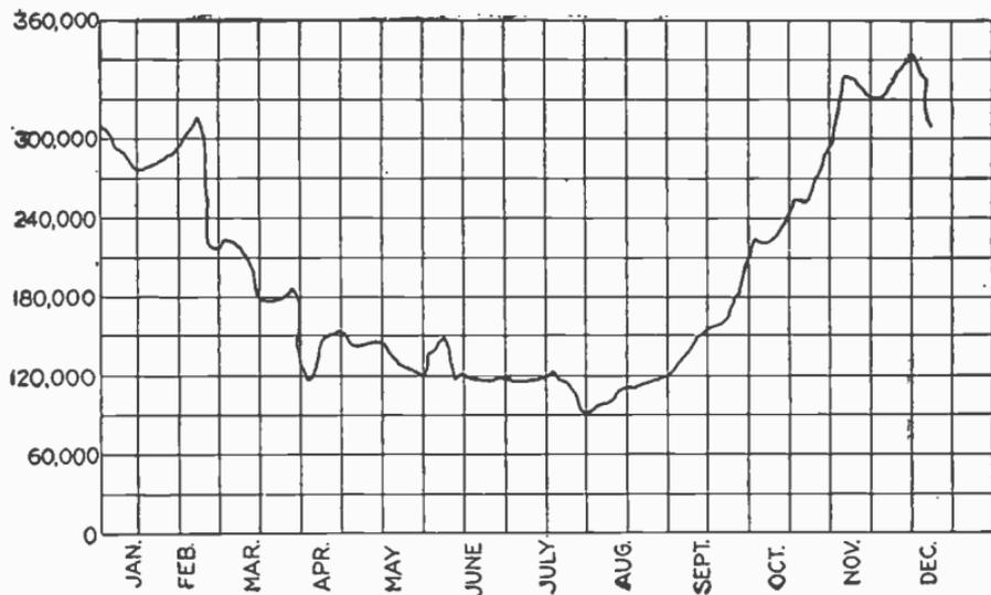
FIG. 4,739.—Load curve for one year.
