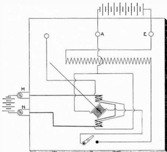
FIG. 4,856.—Diagram of connections for calibrating a watt meter.
