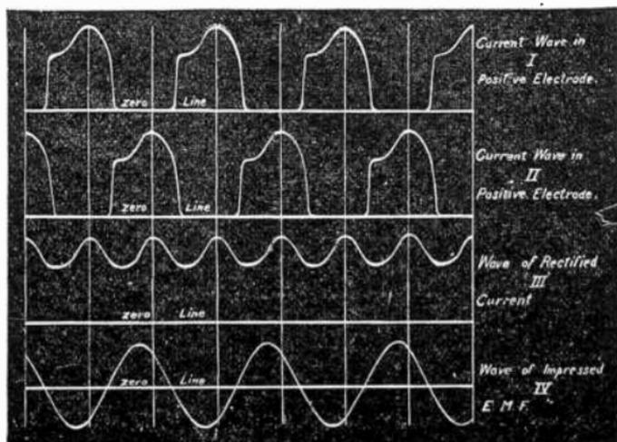
FIGS. 4,356 to 4,359.—Diagram of current waves and impressed pressure of Westinghouse-Cooper Hewitt mercury vapor rectifier. The whole of the alternating current wave on both sides of the zero line is used. The two upper curves in the diagram show the current waves
