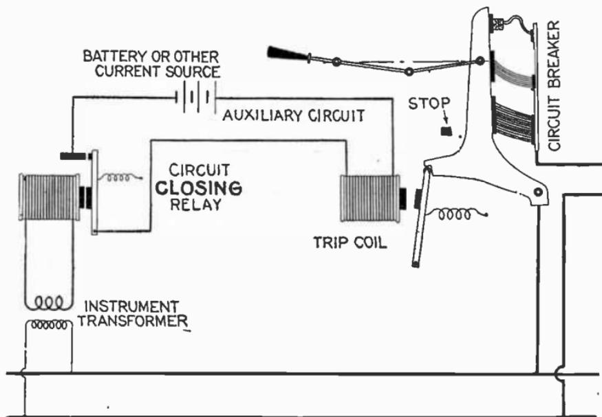
FIG. 4,210.—Diagram illustrating the operation of a *circuit closing relay*. When the pre-determined abnormal condition is reached in the main circuit, the relay closes the auxiliary circuit, thus energizing the trip coil and opening the breaker.
