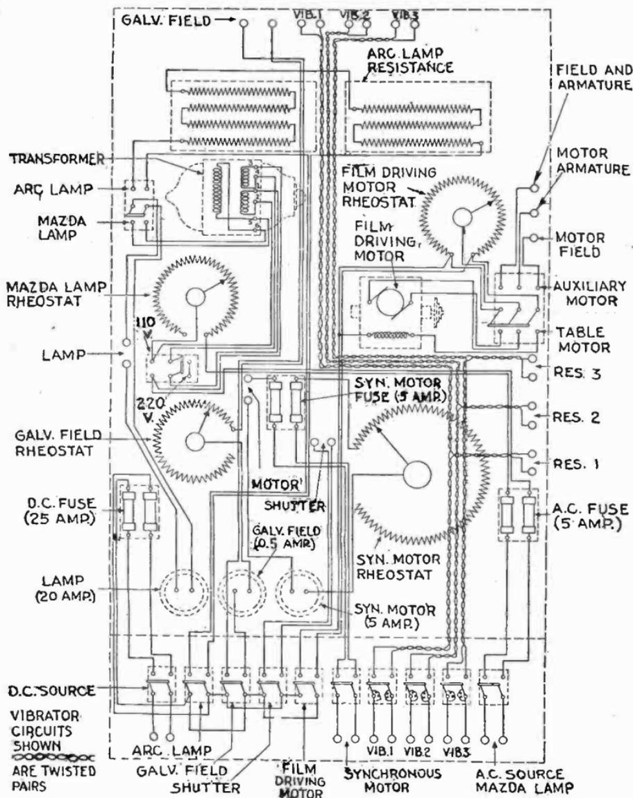
FIG. 4,602.—General Electric oscillograph. Connections for portable table for use with arc or mazda lamp.
