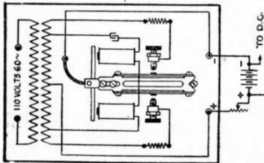
FIG. 4.339—Circuit diagram of Leich full wave electro-magnetic track or battery rectifier. This differs from the half wave type in that it utilizes both halves of the a. c. wave and accordingly has an output sufficient to charge 1 lead cell battery at 2 amperes and 2 volts or 2 to 10 cells at one ampere and 4 to 20 volts. This rectifier can, because of its higher charging rate, be used on work consuming a greater amount of current than can be supplied by the half wave type.
