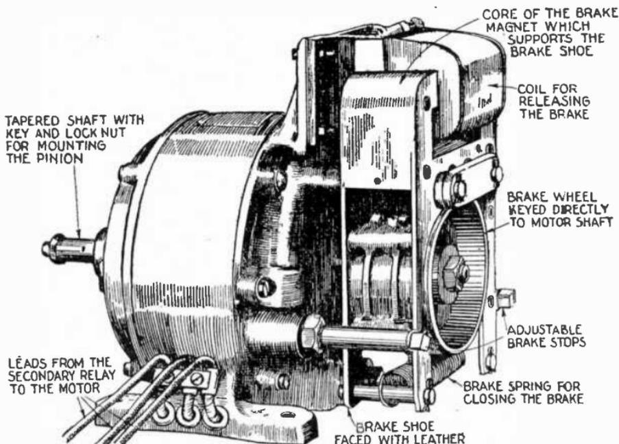
FIG. 4,331.—Westinghouse operating motor for single phase induction voltage regulator showing brake, etc.
