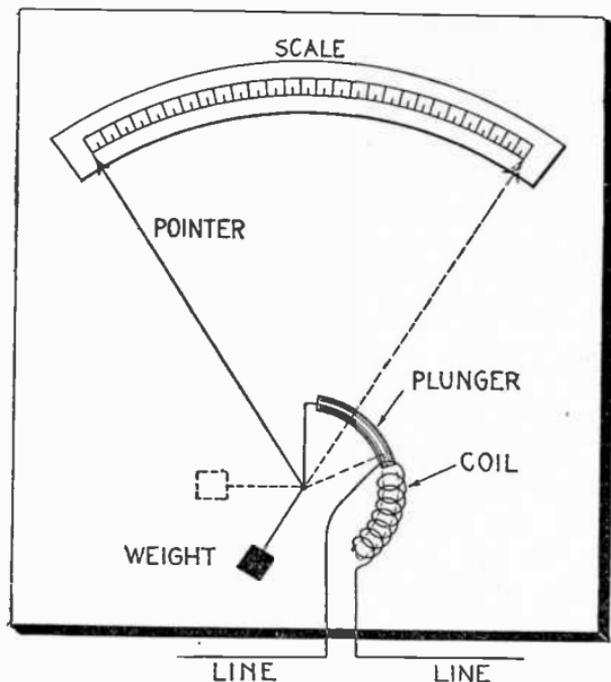
FIG. 4,448.—Plunger form of electro-magnetic or moving iron type of ammeter.
