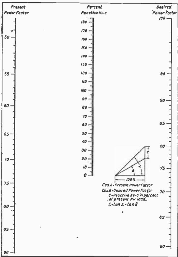
Figs. 4,250 to 4,253.—Chart for use in determining the per cent reactive *kva*. required to raise the power factor to a desired value. *Example:* To find the "per cent reactive *kva*," necessary to raise the power factor from present power factor to desired power factor, lay a straight edge across the chart connecting these two values. Read the reactive *kva*. in per cent of the present *kw*. load on the middle scale.
