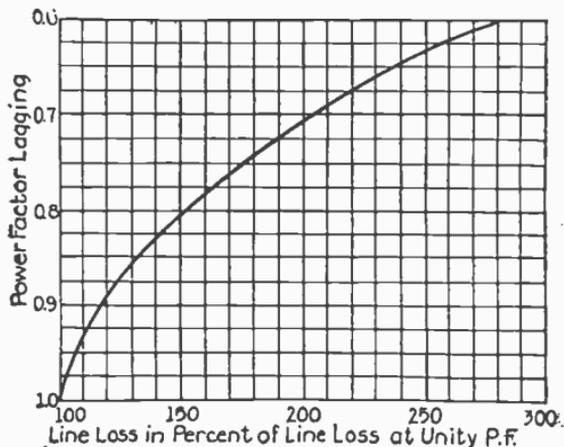
FIG. 4,245.—Curve showing relation between power factor and line loss when carrying constant *kw.* load.
