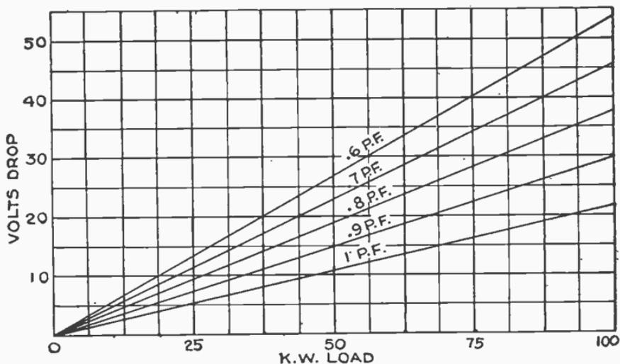
FIG. 4,247.—Curves showing volts drop over a 1,000 ft. 3 phase, 60 cycle, circuit of No. 0 wire, 9 in. spacing, 440 volts at motor. The curves show the actual volts drop in this circuit carrying various loads at various power factors. These curves are intended to give a picture of the effect of reduction of power factor and are not intended to be used in actual calculations.
