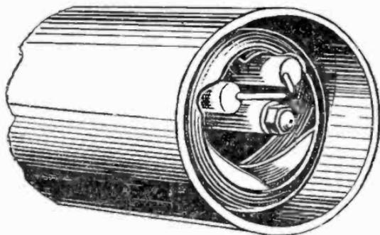
FIG. 8,704.—Oil-Electric draft tube, air diffuser and spray nozzle showing location of spark in relation to spray nozzle.
