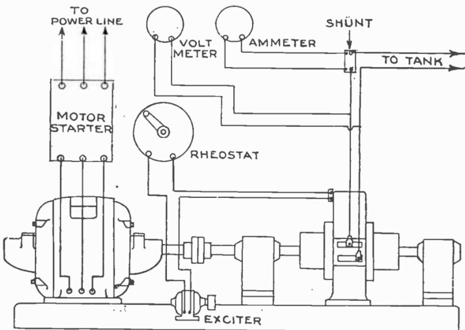
FIG. 8,267.—Method of connecting a motor dynamo set, consisting of a *separately excited* dynamo with separate exciter and *a.c.* motor.
