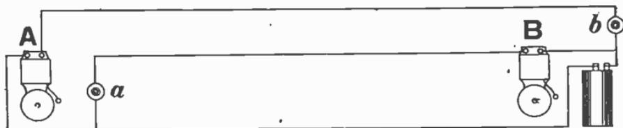
FIG. 8,487.—Two bell diagram so connected that push *a* rings bell B, and push *b* rings bell A.
