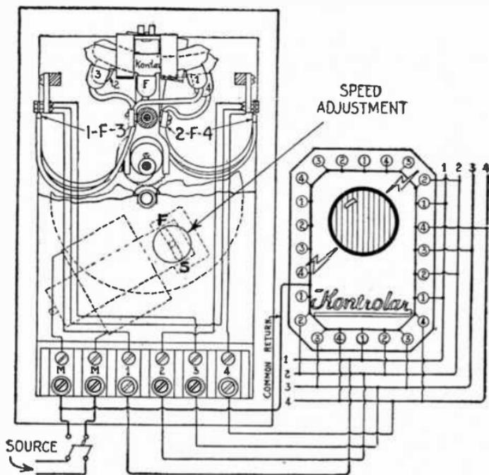
FIG. 8,570.—Leland unit speed flasher wired to sign. It is wired with four circuits with a common return. It has an extensive range, operating such arrangements as running or traveling borders, revolving wheels, lightning, radiating rays, flames, smoke, clouds, rain, sparks, dust, steam, fireworks, waving flags, fountains, etc.
