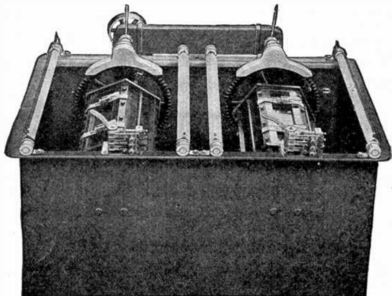
FIG. 8,282.—Hanson-Munning plating barrel. Electro-plating small metal parts in bulk eliminates racking, wiring and individual handling of pieces and thereby saves time and labor. Suitable for nickel, silver, copper, brass, cadmium, zinc, tin and lead. The type of cylinder and tank is determined by the solution to be used and the size and type of work to be plated.
