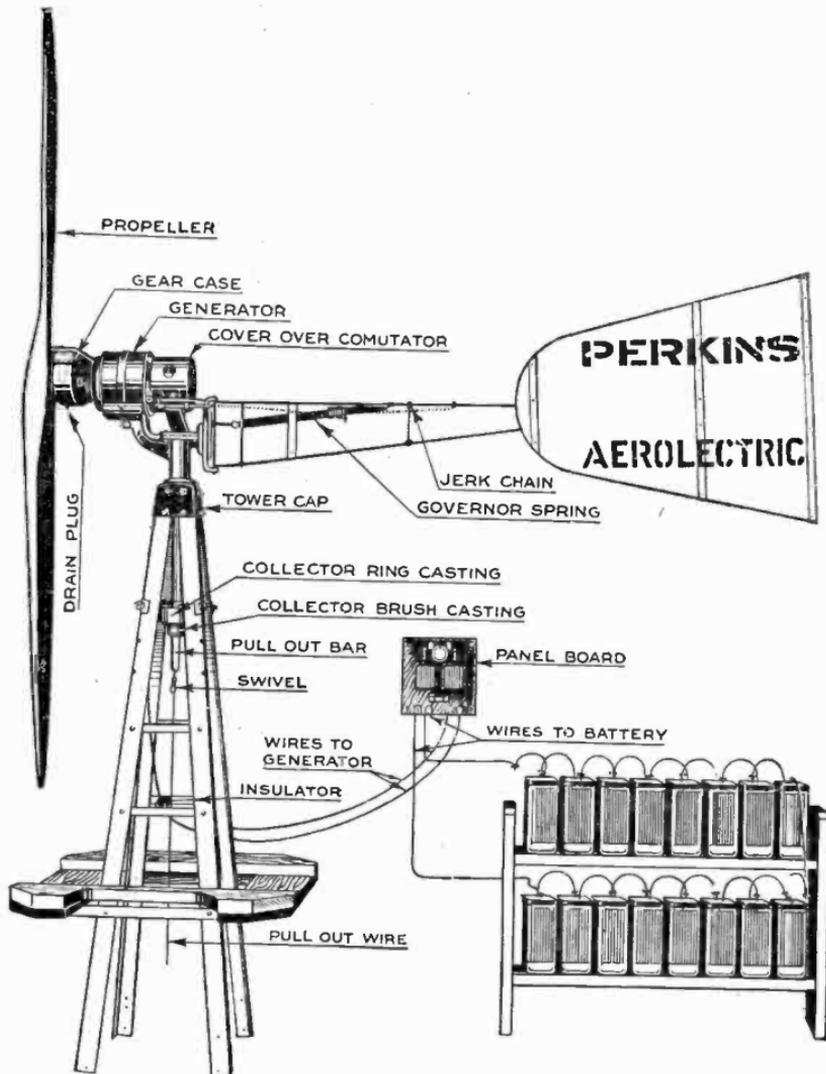
FIG. 8,791.—Aeroelectric generating mechanism with gear case cover removed, showing transmission between wheel and dynamo. This is a wind mill suitably geared to a dynamo forming a unit for charging a storage battery, the latter being used as current source for house lighting.
