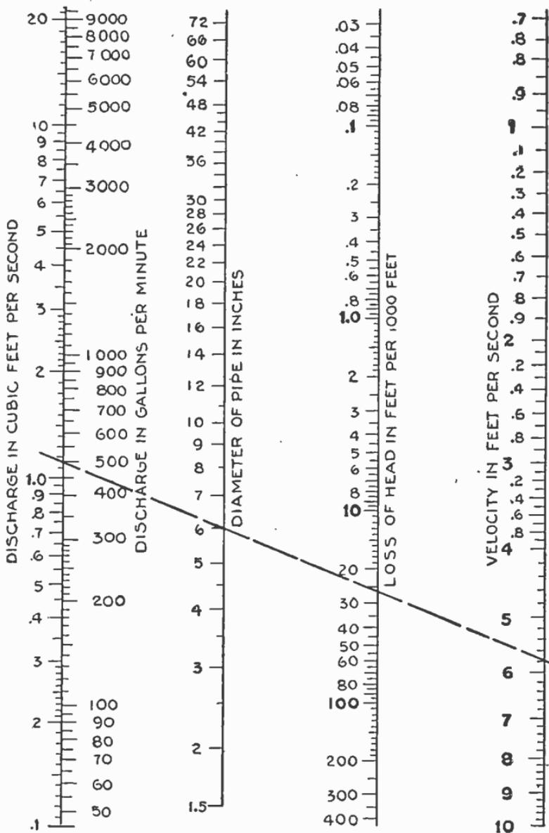
FIG. 8,918.—Diagram for calculating pipe sizes, discharge velocities and loss of head in water pipe. Lay a straight edge on scales at the points for any two known quantities and the unknown quantities will lie at the intersection of the straight edge with the other scales. *Example.*—To discharge 500 gals. per minute through a 6 in. pipe following the dotted line would show a loss of head for 1,000 ft. of approximately 25 ft. head and a velocity of 5.8 ft. per second.
