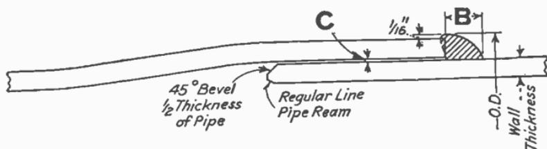
FIG. 8,174.—Dimensions of weld for various sizes and weights of pipe; values given in table below:
