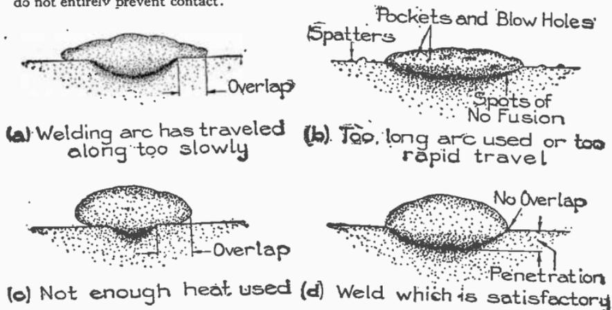
FIGS. 8,066 to 8,069.—Cross section of beads deposited under different conditions.
