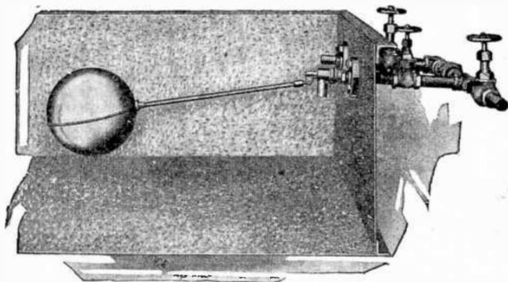
FIG. 8,745.—Buffalo automatic make up and quick filler. The required water level in the tank is automatically maintained by the float valve here shown. This allows constant operation of the pump at uniform suction head. It is also essential that provision be made for rapid filling of the tank after cleaning, and this is provided for by the extra flanged pipe inlet, which also serves as a hose connection.
