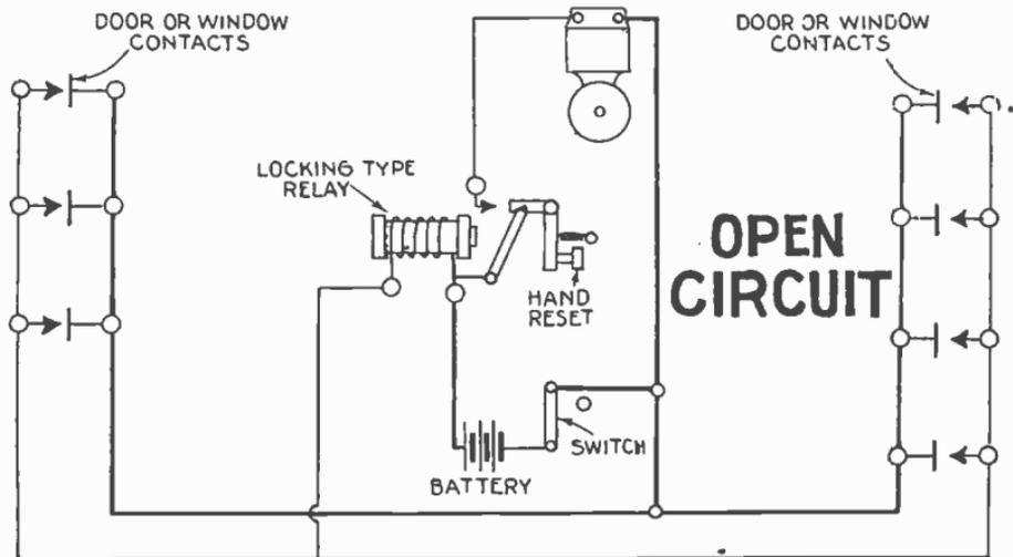
FIG. 8,498.—Open circuit burglar alarm system to be operated in parallel. *In hook up there must be:* 1, one common wire to one side of all window or door springs, switch and bell.
