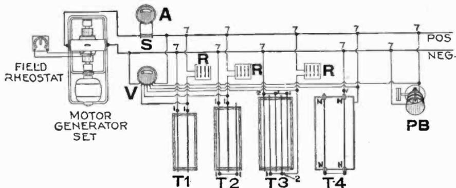
FIG. 8,280.—Diagram of two wire system showing method of connecting dynamo, tanks, plating barrel, volt meter, ammeter and rheostat. A, ammeter; V, volt meter; S, ammeter shunt; R, tank rheostat; T-1, two rod tank, one row work; T-2, three rod tank, one row work; T-3, five rod tank, two row work; T-4, electric cleaner, steel tank; PB, reliance plating barrel; N, insulator; 1, No. 1 brass connections; 2, No. 2 brass connections; 7, No. 7 brass connections.
