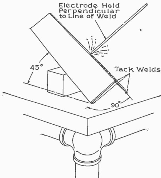
FIG. 8,085.—Lesson 7. Right angle butt weld inclined 45° to horizontal. This is the same as Lesson No. 6, except that, after tacking the plates as shown in fig. 8,083, they are placed so the weld makes an angle of 45° with the horizontal. The end having the  $\frac{1}{8}$  in. opening should be at the top. Begin at the lower end, and weld upward and away from the operator, as shown.
