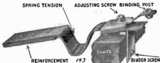
FIG. 8.577.—Detail of Reynolds brush and holder. The brush is built up with copper leaves and has phosphor bronze spring back, reinforced at contact point.
