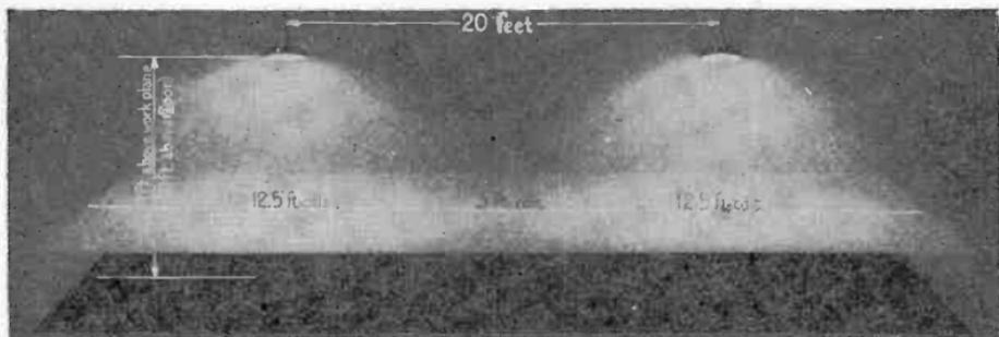
FIG. 8.385.—Spacing between luminaires should not exceed  $1\frac{1}{2}$  times the mounting height above the work plane, non-uniform lighting (foot candle values based on 200 watt luminaires).
