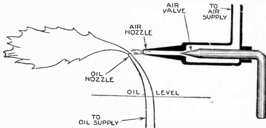
FIG. 8,708.—Atomizing oil by air jet or spray.
