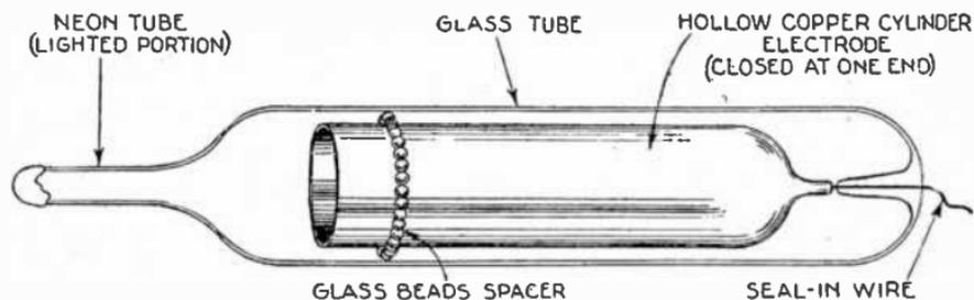
FIG. 8,337.—Neon luminous tube. View showing construction.
