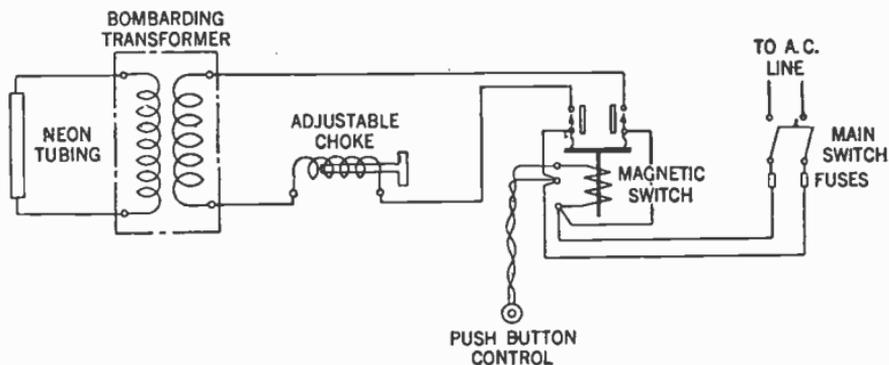
FIG. 5.—Schematic wiring diagram of bombarding transformer with auxiliary equipment.
