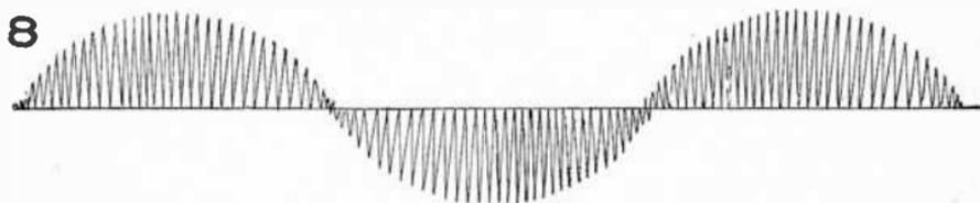
FIG. 9,011.—Pulsating galvanic sinusoidal. In this modality only one-half of each oscillation produced by the penetrator is employed, consequently the frequency of the voltage change is only one-half as great as with modality No. 9 (oscillatory wave); and the intensity of the impressed voltage is changed 170 times per second, while the peak voltage is on for only 1-1,360th of a second, with a rest period of 3-1,360ths of a second.
