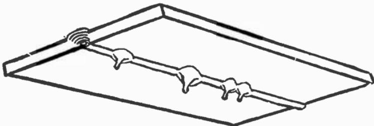
FIG. 8,160.—Underside of overheated weld showing excess metal hanging.
