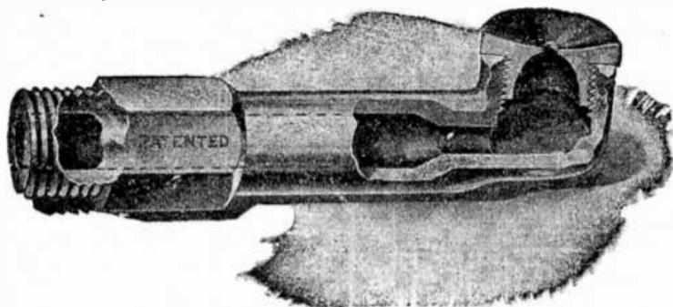
FIG. 8,733.—Carrier spray nozzle. The water entering through the small circular chamber tangentially, acquires a whirling motion and is discharged through a small orifice in the center of the cap. The approach to the orifice is conical in shape, so that the rotation, or whirling speed of the water is greatly increased at the instant of discharge.
