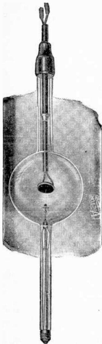
FIG. 8,998.—Coolidge water cooled deep therapy type tube. Except for the anode construction and mounting, this tube is very similar in appearance to the air cooled treatment tube and has similar characteristics. The anode is constructed to provide for the circulation of water immediately behind the focal spot to remove the heat as rapidly as it is generated, thereby making it possible to use much greater energy than heretofore.
