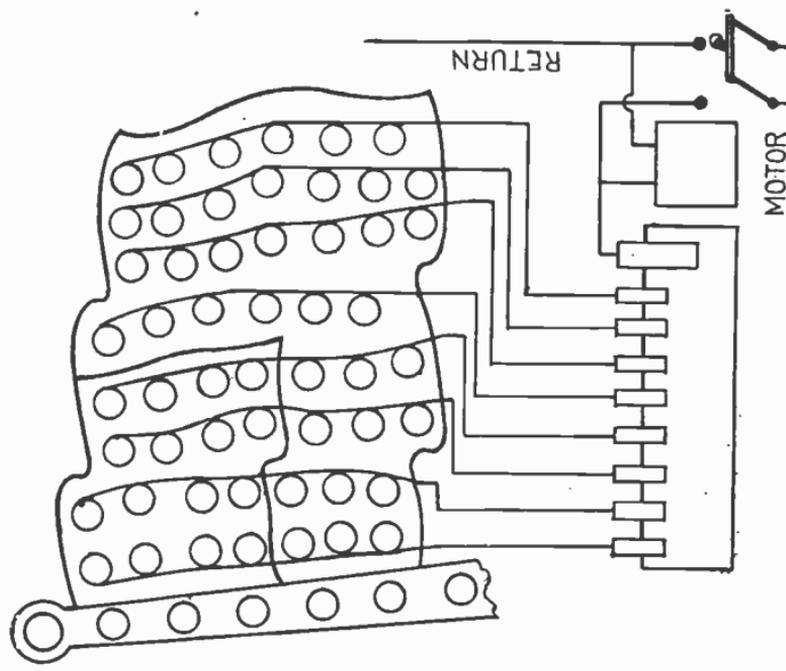
FIG. 8,612.—Waving flags, pennants, etc. Flags are wired in staggered rows as here shown, and require a flasher brush for each row.
