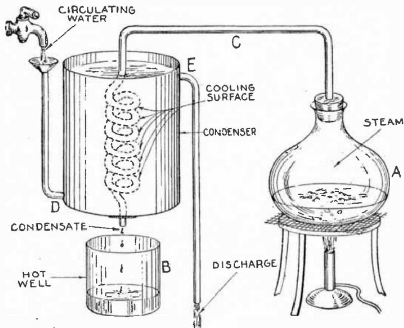
FIG. 8,646.—Experiment illustrating *condensation*. If water for instance be boiled in a flask A, and the steam thus produced led off through pipe C, having a coiled section surrounded by cold water, it will here be cooled below the boiling point and will therefore condense, the *condensate* passing out into the receptacle B, as water. The cooling or "circulating" water enters the condenser at the lowest point D, and leaving at the highest point E.
