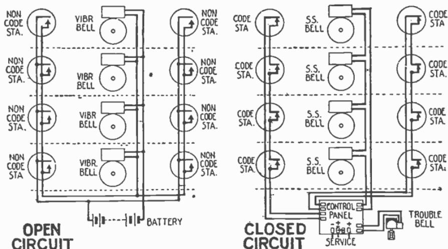
FIG. 8,514.—Edwards' open circuit fire alarm system. In the open circuit system any contact made in any box on a floor sets all the bells in operation.
