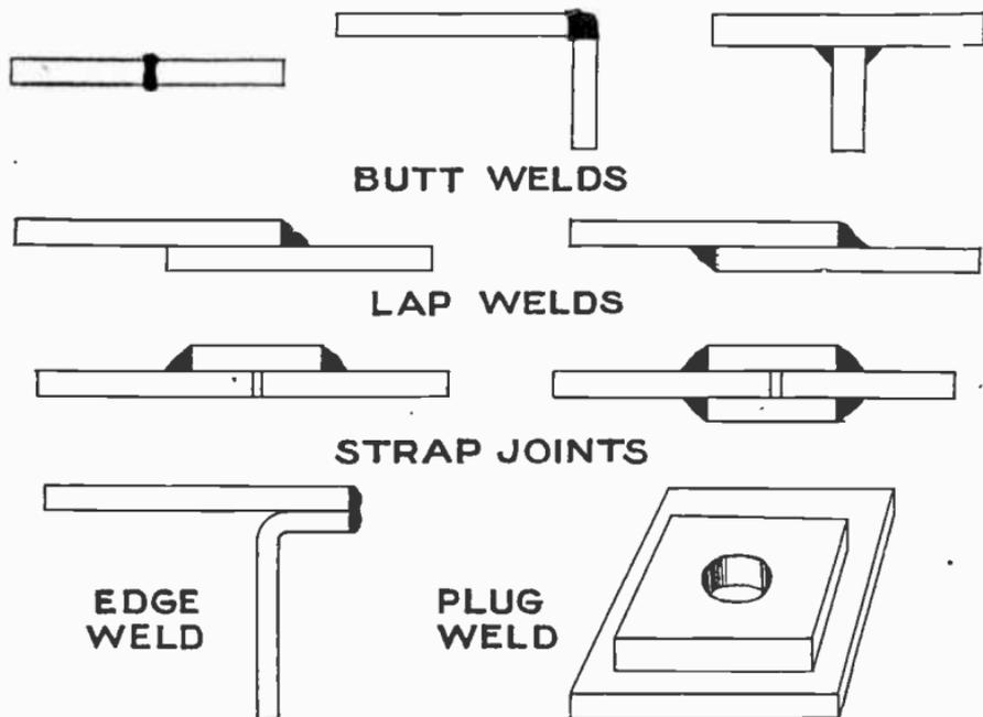
Figs. 8,032 to 8,040.—Various types of welded joints.
