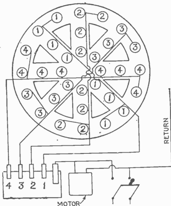
FIG. 8,605.—Wiring for revolving wheel.
