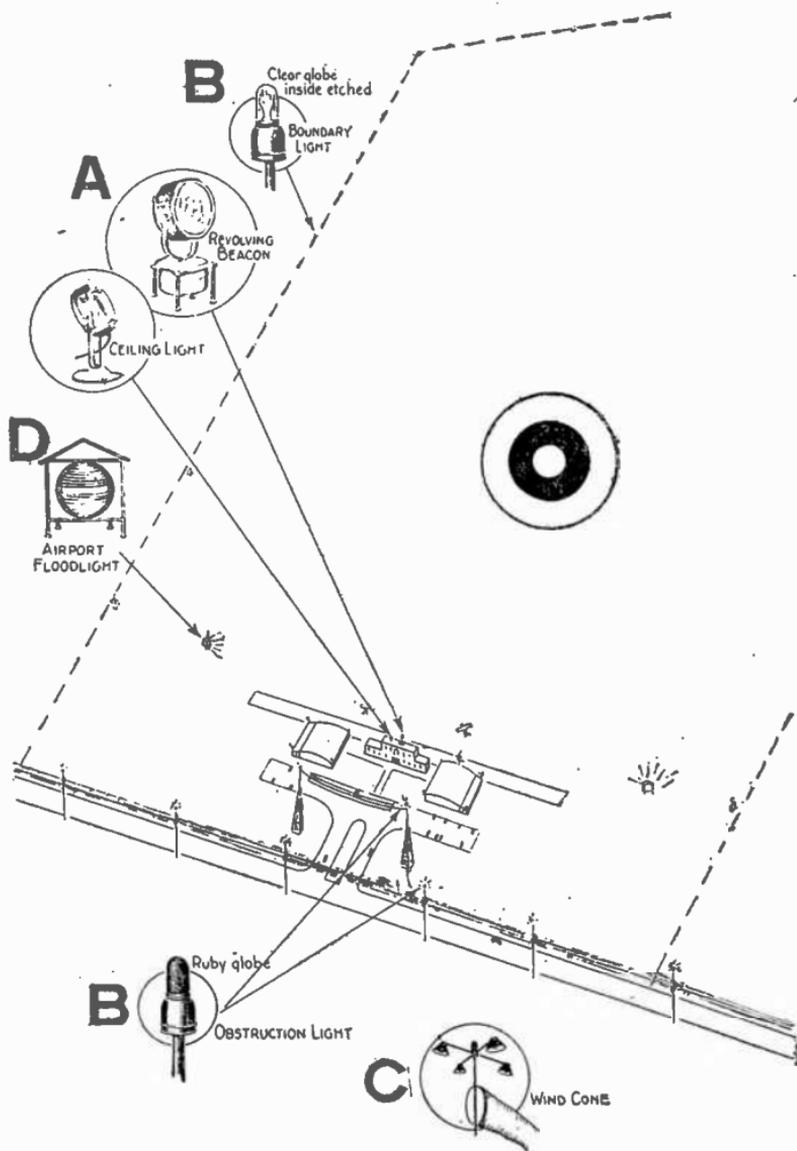
FIG. 8.406 to 8.412.—Minimum lighting facilities required for an air port to obtain an "A" rating
