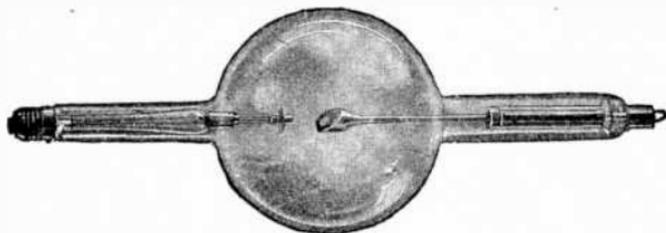
FIG. 8,985.—Coolidge *universal type tube*. Adapted for all classes of X-ray work, radiographic, fluoroscopic and therapeutic, but should be used only on rectified current and at voltages not exceeding 140 *kv.* maximum.
