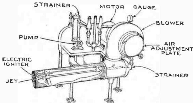
FIG. 8,707.—Motor driven atomizer burner of the electric ignition type.
