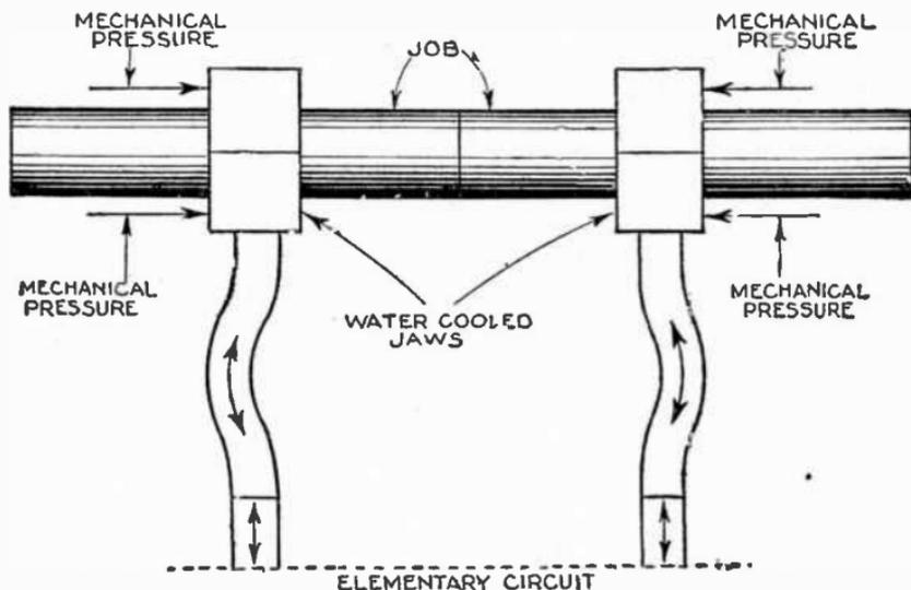
FIG. 8,117.—Circuit diagram for butt welding.
