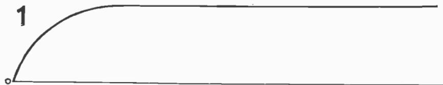
FIG. 9,004.—Galvanic current. It is obtained from a copper-oxide rectifier which changes the *a.c.* to *d.c.* The galvanic current then passes to a choke coil and condenser, known as the filter circuit, where all ripples or pulsations are removed or filtered out.
