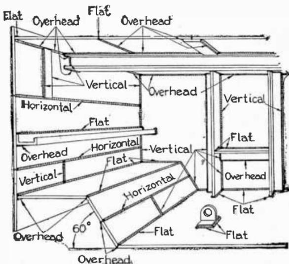
FIG. 7,981.—Various positions of weld.
