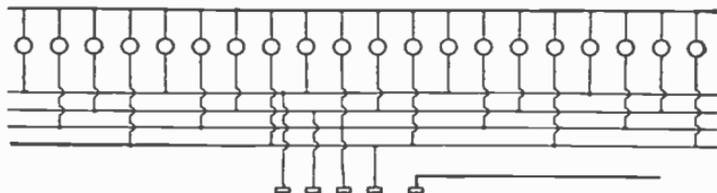
FIG. 8.596.—Pulsating, twinkling or shimmering effects are accomplished by transposing leads (hooking lead No. 2 to flasher brush No. 4, lead No. 3 to brush No. 1, etc.).
