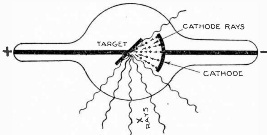
FIG. 8,983.—Diagram of an X-ray tube. *In operation*, cathode rays strike the positive terminal or target of the tube and cause rays to emanate from the target, which have the quality of penetrating objects and are known as X-rays.
