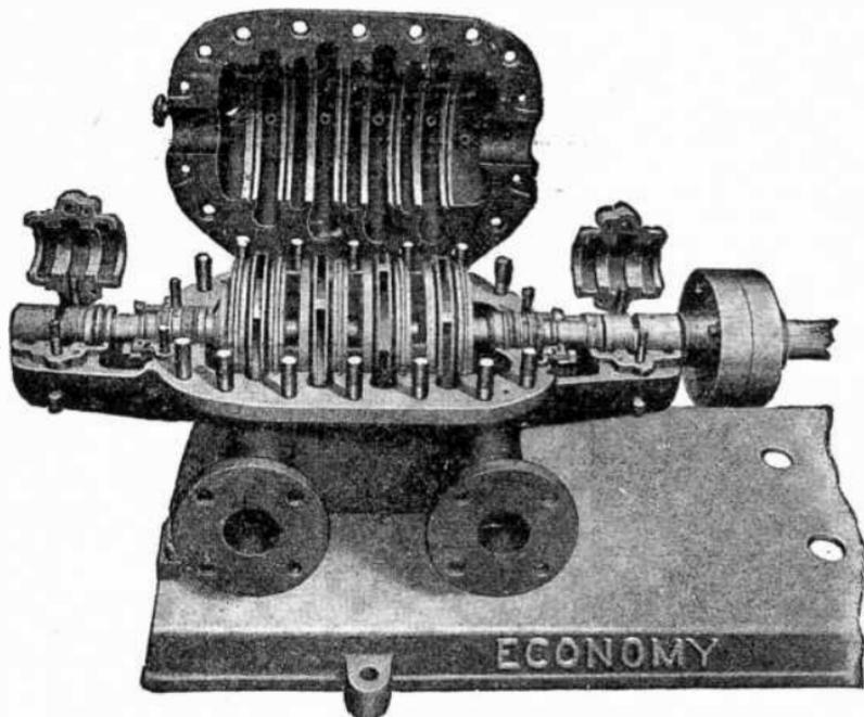
FIG. 8,892.—Economy four stage centrifugal pump, with cover lifted showing one piece bronze diaphragm.
