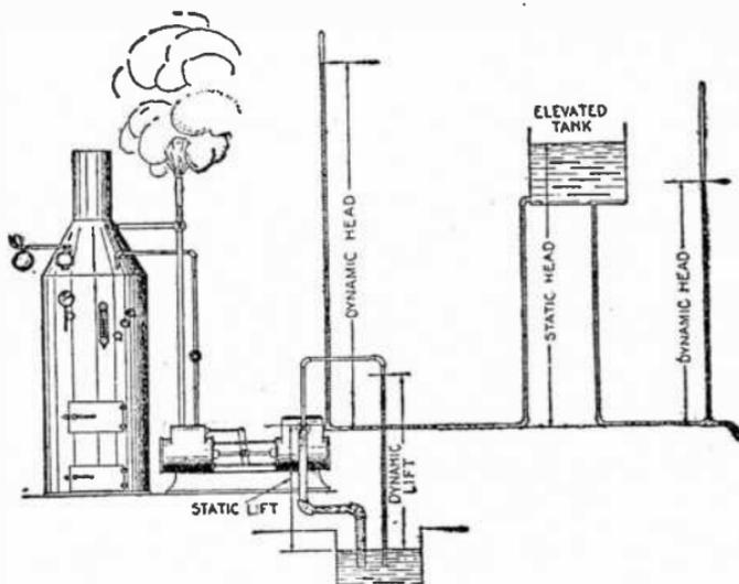
FIG. 8,805.—View of elevated tank with pump in operation maintaining the supply which is being drawn upon as shown, illustrating the terms static lift, dynamic lift, static head, and dynamic head.
