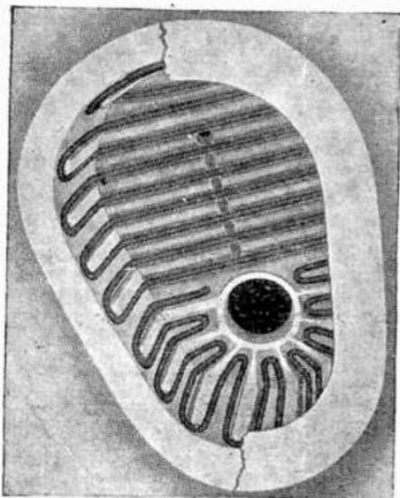
FIG. 8,202.—Electrical heating elements as used on Chapman "Allatonce" commutator soldering machine. Rating of heating elements 1600° to 2200° Fahr. but operated at only about 1200°.
