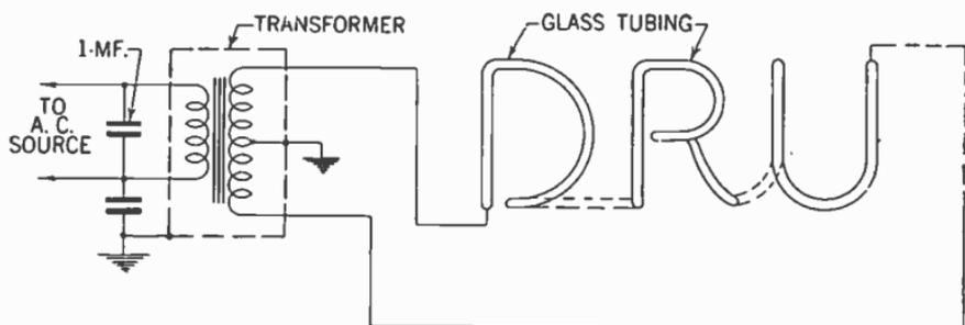
FIG. 6.—Typical wiring diagram showing radio interference suppressor in transformer primary.
