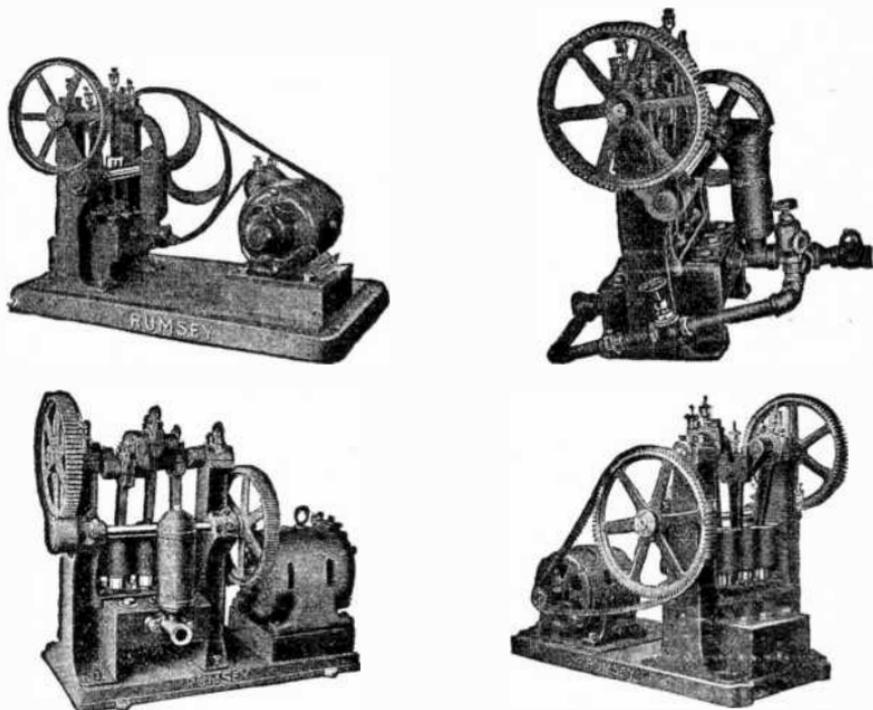
FIGS. 8,846 to 8,849.—Various drives as used on Rumsey single acting triplex pumps. Fig. 8,846, belt with idler; fig. 8,847, single reduction, toothed gear; fig. 8,848, double reduction toothed gear; fig. 8,849, chain.
