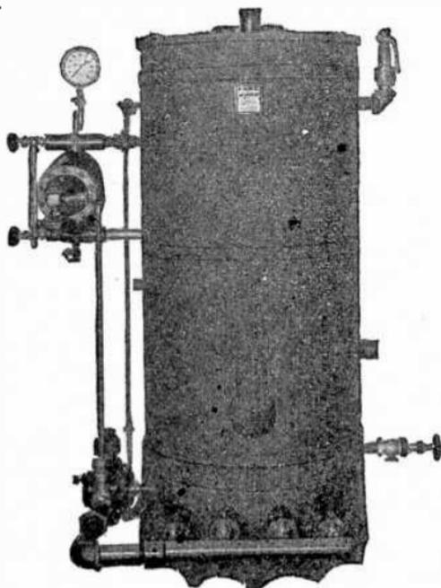
FIG. 8,248.—Reliance steam boiler. A boiler is necessary in large plating rooms where hot water is not available, or where close temperature regulation of hot solutions is desired. In general practice, one boiler *h.p.* will heat 25 gals. of water or its equivalent from 60° (boiling) Fahr. in one hour, to a temperature rise of 150°. Using this as a basis gives the following formula for determining the *h.p.* required for a given job:
