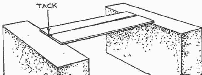
FIG. 8,148.—Plates tacked for welding. *Instructions:* Tack the left end of the plates together. This is done by holding the flame close to the joint until the steel melts and runs together. Remove the flame instantly when the metal flows, as otherwise a hole will be burned through. Warm the two plates by passing the flame over them lengthwise two or three times.
