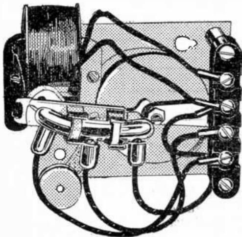
FIG. 8,572.—Leland junior flasher. 12 ampere capacity. It is operated by an *intermittent* induction disc motor. The motor circuit is led through the mercury switch so that when the flasher breaks the sign circuit, it also breaks the flasher motor circuit. The mechanism then returns by gravity action to its starting position from where the cycle is repeated.
