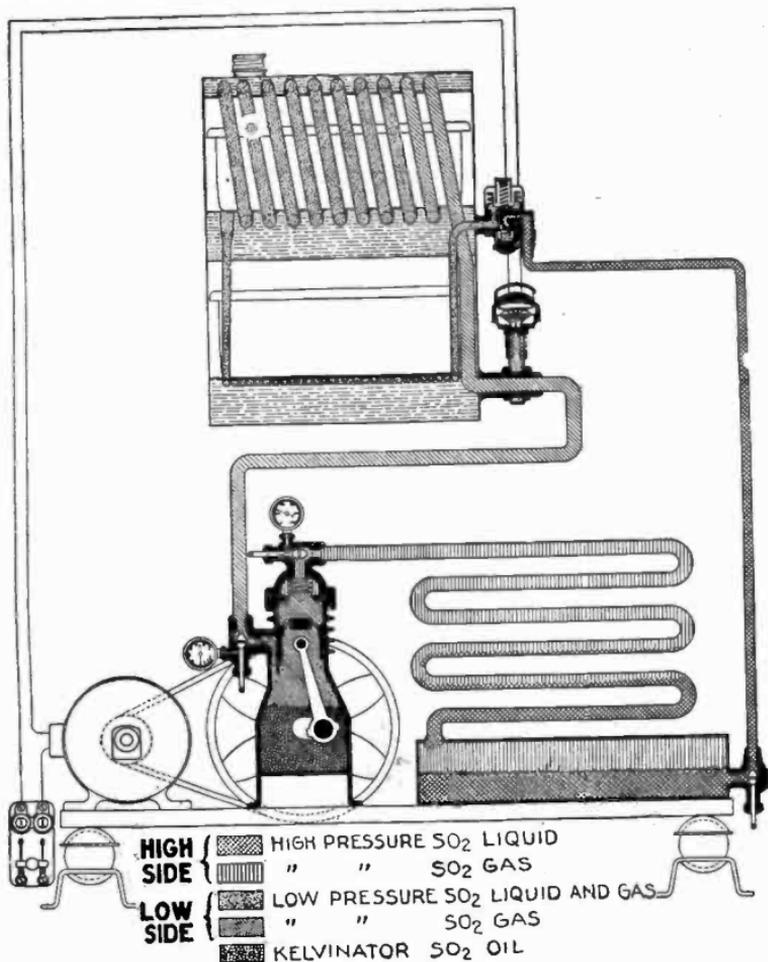
FIG. 8,681.—Kelvinator dry system cycle.
