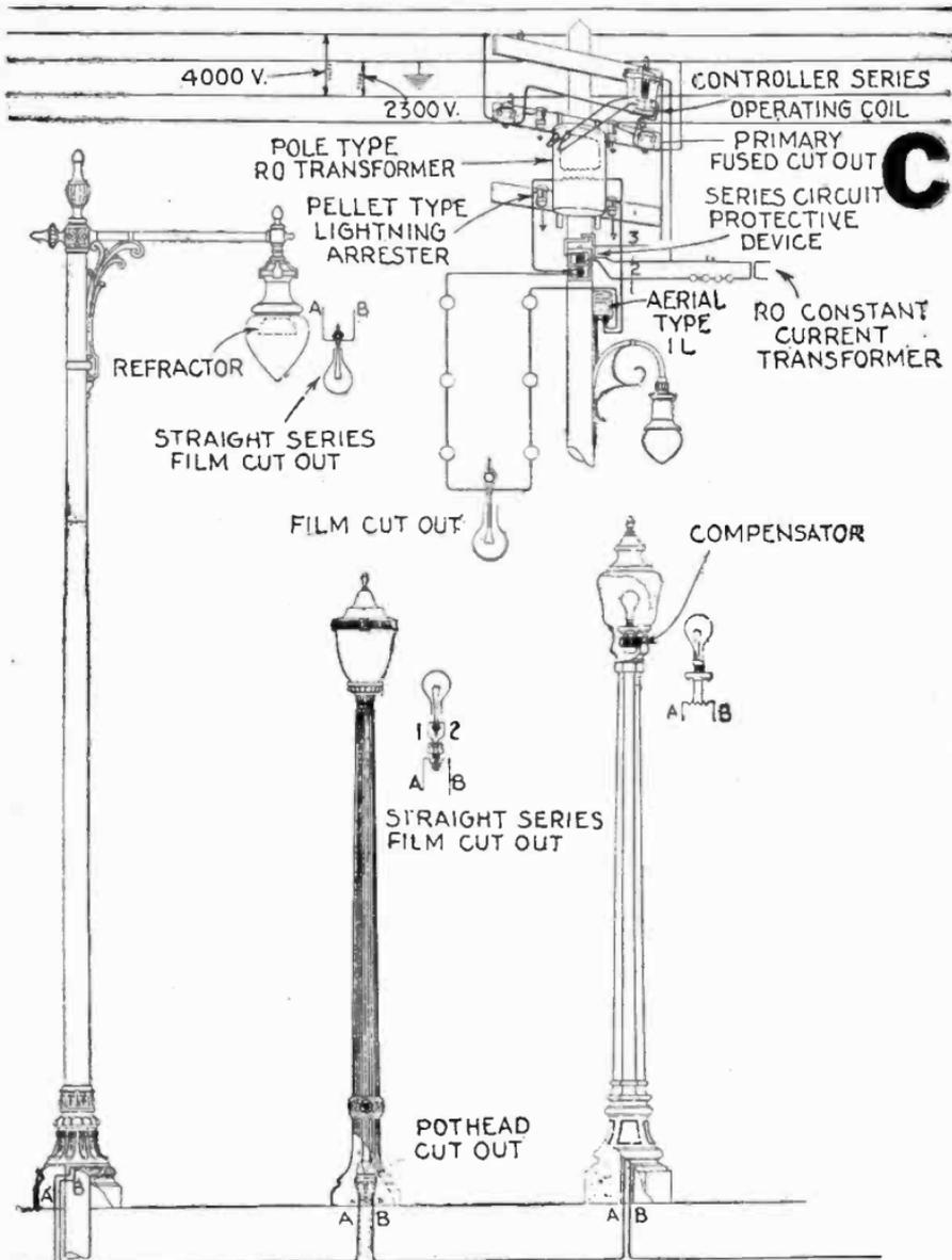
FIGS. 8,350 to 8,353.—General Electric Novalux series street lighting system. Section C.
