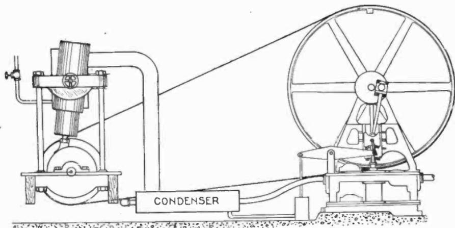
FIG. 8,920.—Graham jacketed, transfer expansion oscillating engine, and Dunham power pump with belt transmission. *It must be evident* that this arrangement permits the engine and pump to work under the most favorable conditions for economy. Hence by proper proportion of pulleys, the engine may run at *high speed*, thus reducing the size of the cylinder and loss by condensation, leakage, etc., and the pump may be run at *slow speed*, thus eliminating water hammer, slamming of valves, etc.
