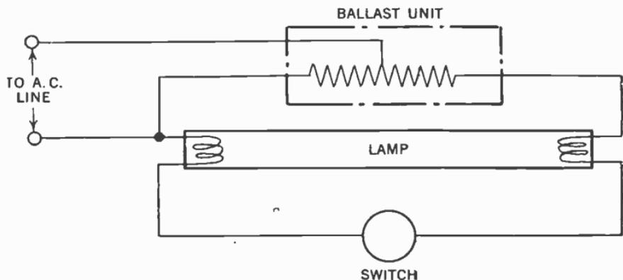
FIG. 14.—Method of connection for single unit fluorescent lamp, with uncorrected power factor.
