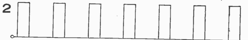
FIG. 9,005.—Interrupted galvanic. The motor and transformer switches must both be snapped on to obtain this modality, as well as the remainder, except Nos. 5 and 16. A special commutator affords a make and break in the current flow, which by means of a regulator may be timed for the proper duration.
