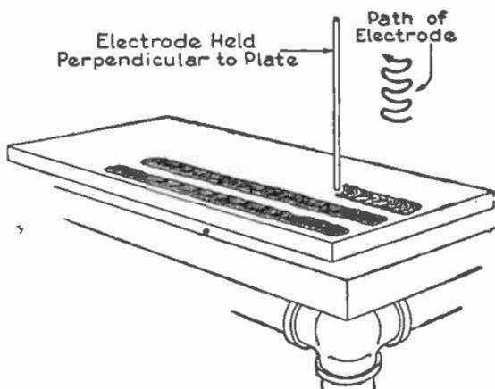
FIGS. 8,072 and 8,073.—*Lesson 2. Three parallel beads.* In this and all following lessons, the deposited metal should meet all the requirements of a good weld, uniformity of height and width, regularity of ripples, good penetration, and no overlap nor signs of porosity. These
