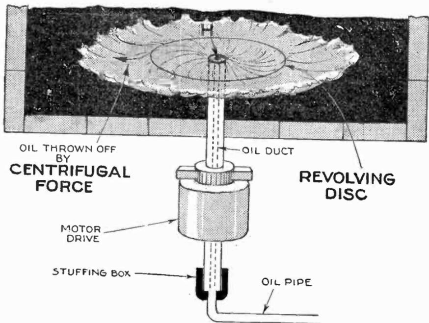
FIG. 8,705.—Elementary centrifugal force atomizing burner. The oil flows through the hollow spindle of a disc which is rotated at high speed by a motor. The oil overflowing at H, onto the disc at its center is hurled off the disc by centrifugal force, and ignited by a torch or pilot light, produces a ring of flame.
