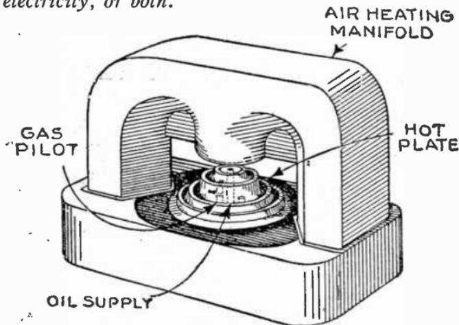
FIG. 8,713.—Casting of a vaporizing burner with which is incorporated the continuous burning gas pilot and plate heating flame.
