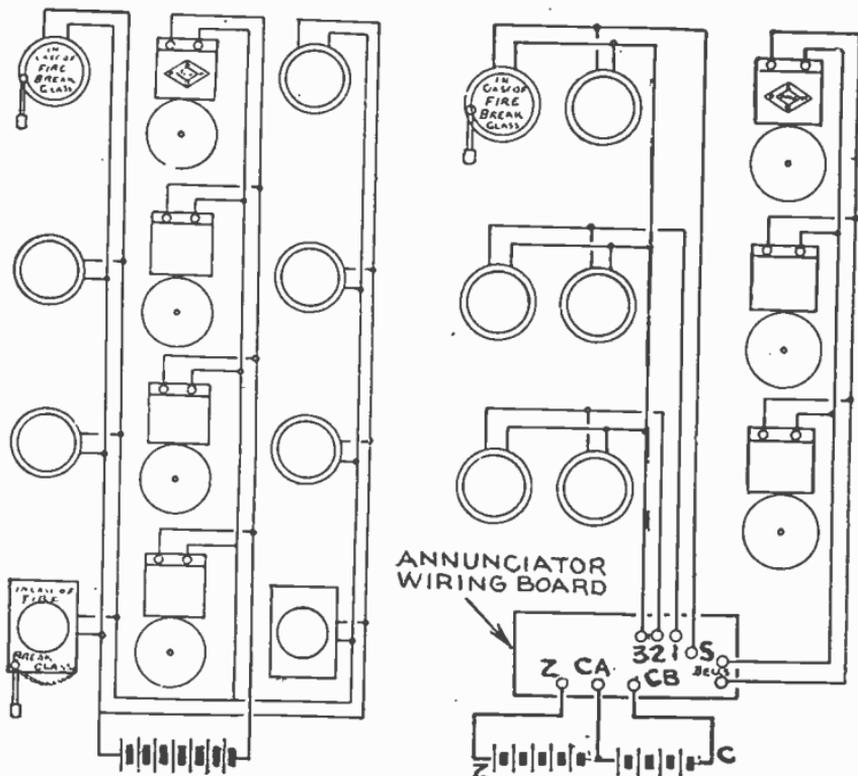
FIG. 8.512.—Patrick & Wilkins *open circuit* fire alarm system with break glass signals and vibrating bells. *In operation*, the breaking of the glass of any of the fire alarm signal boxes will cause all of the bells on the circuit to ring simultaneously until switched off.
