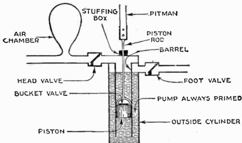
FIG. 8,919.—Elementary so called syphon pump showing pump barrel projecting down into a concentric or outside cylinder providing an annular space which traps water so that the pump is always primed. Anyone having any experience with pumps, especially old and worn pumps, will appreciate this feature.
