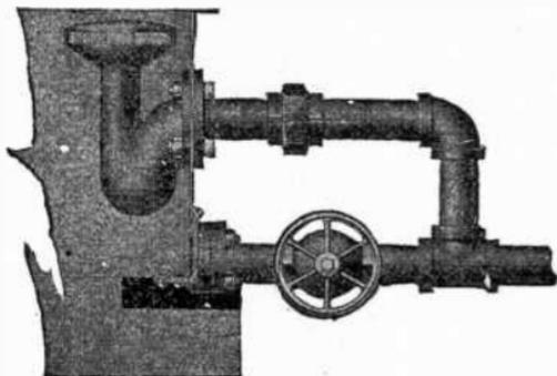
FIG. 8,746.—Buffalo water sealed overflow and drain. The water sealed overflow pipe is bolted to the side of the tank. Hooded construction prevents waste of the spray water. A drain box connection which can be easily cleaned is provided under the tank.
