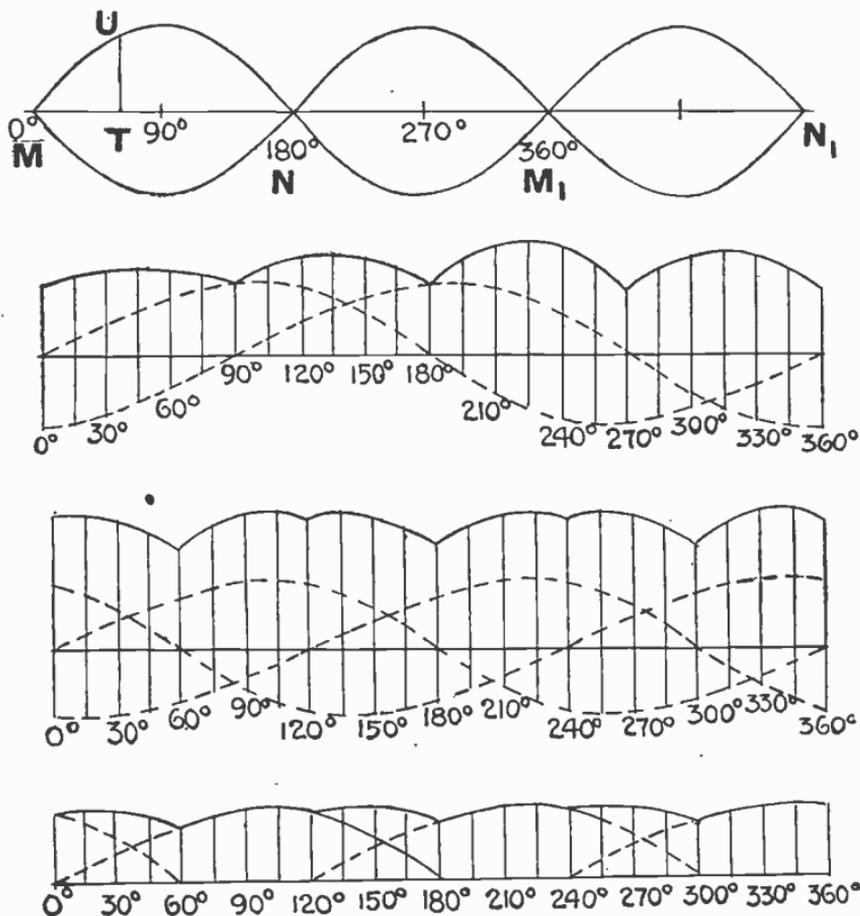
FIG. 8,833.—Flow curve of single double acting power pump.
