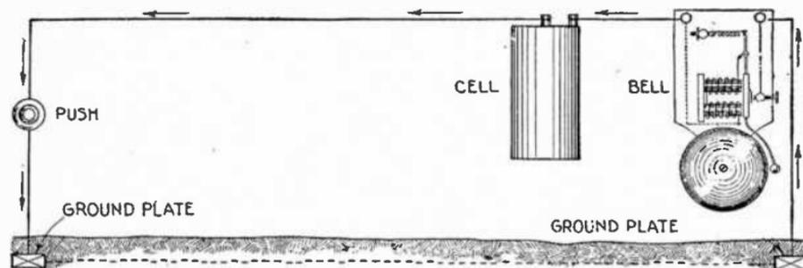
FIG. 8,482.—Simple bell circuit with *ground* return. Instead of using ground plates, a more convenient method consists in connecting the ground wires to a gas or water pipe.
