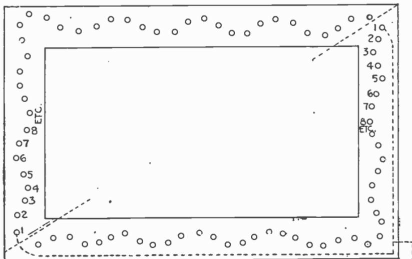
FIG. 8,603.—Chaser wiring diagram for two snakes.
