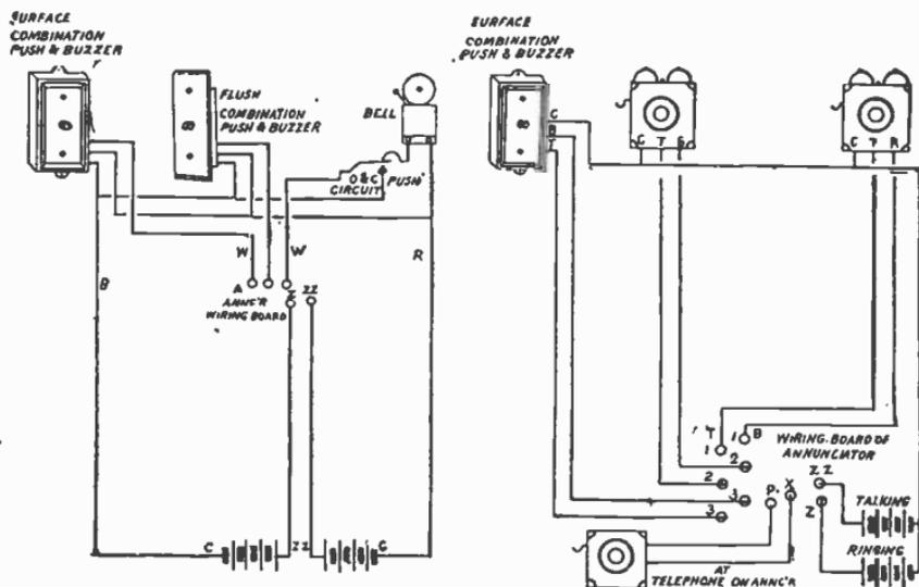
FIG. 8,479.—Partrick & Wilkins return call system using combination buzzers and buzzer pushes and buzzer or bulb separate.
