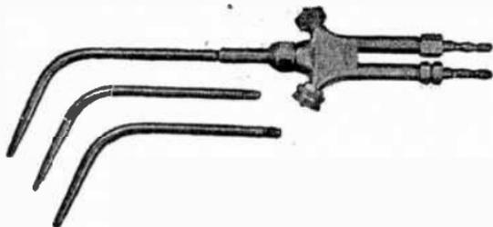
FIGS. 8,213 to 8,215.—Airco-Davis-Bouronville lead burning torch designed for "burning" or welding lead. By attaching a proper mixing head and using City gas instead of acetylene, this torch may be used for soldering. The temperature with gas is about 3,500° Fahr.
