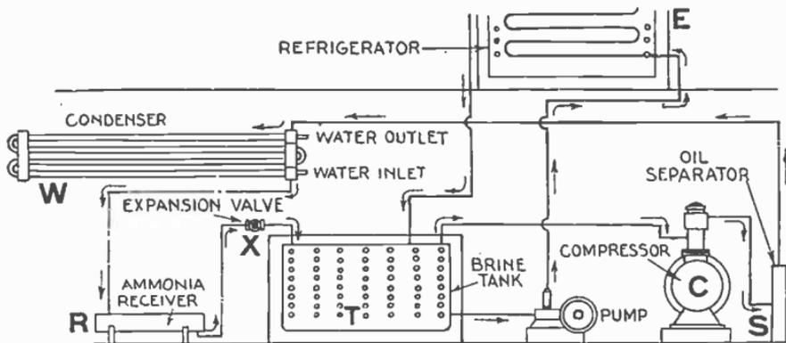
FIG. 8,661.—Ammonia compression system; 2, brine circulating method. In operation, ammonia is expanded through piping submerged in a brine tank, or through a special cooler or evaporator. The brine, after being reduced to a low temperature, is pumped through piping placed in the compartments to be chilled. C, compressor; E, refrigerator; R, receiver; S, oil separator; T, brine tank; W, condenser; X, expansion valve.
