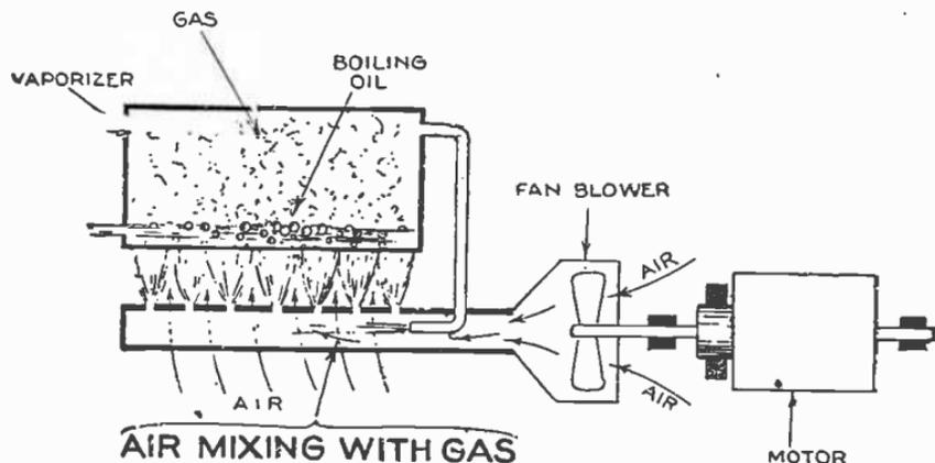
FIG. 8,702.—Elementary gravity feed *mixing*, vaporizing burner. Connected to the burner is a fan blower with outlet pipe surrounding the gas pipe as shown. *In operation*, air from the fan blower mixes *inside* the burner with the gas coming from the vaporizer. Thus the air is mixed with the gas before ignition, resulting in a blue flame and efficient combustion.
