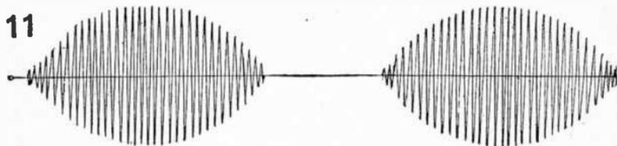
FIG. 9,014.—Interrupted oscillatory wave. This form of wave has the same frequency and duration of impulse as No. 9 (oscillatory wave), and will likewise be found to be free from skin effect.
