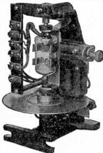
FIG. 8,589.—Time-O-Stat rotary speed flasher for 110 volt, 60 cycle *a.c.* only. *It is operated* by means of an induction disc, similar to that used in the watt hour meter. A single 11-watt contactor containing all the contacts is given a rotary motion so as to flash the circuits in rotation, producing the standard speed effect. The contacts as in the other types of this make of flasher are from mercury to mercury.
