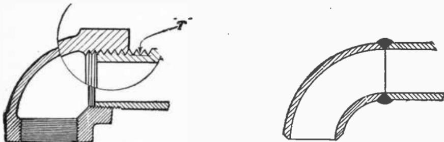
FIGS. 8,185 and 8,186.—Sections of screwed, and welded joints. When a screwed fitting is used there is interference with the flow on account of the internal projection of the pipe. This is avoided in the welded joints. It will be noted in fig. 8,186 that the weld metal does not project inside the pipe.
