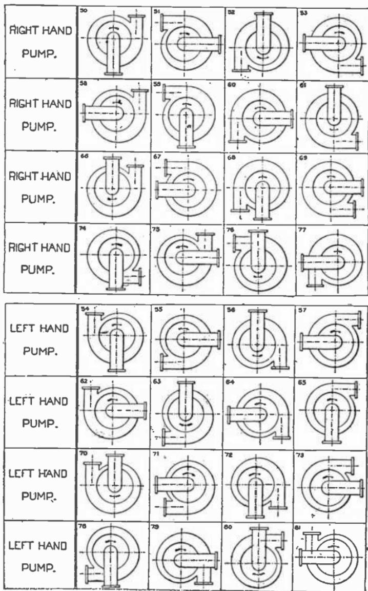
Figs. 8,860 to 8,891.—Various patterns of centrifugal pumps.
