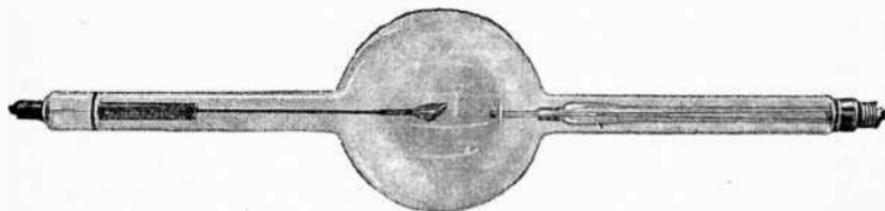
FIG. 8,997.—Coolidge air cooled deep therapy type tube. This tube is similar to the universal tube, but is larger and is designed to operate on rectified current at a voltage not exceeding 200 *kv.* maximum at 5 milli-amperes and 8 milli-amperes continuously under proper cooling conditions.
