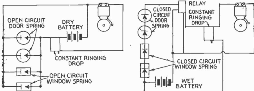
FIGS. 8,500 and 8,501.—Open and closed circuit diagrams of Edwards' burglar alarm systems. These show the window and door contact springs of the open and closed types, the constant ringing drop to make the bell ring continuously when once started, and the actuating relay to close the bell circuit on the closed circuit system.
