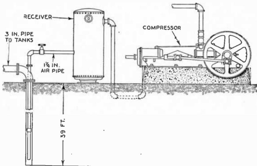
FIG. 8,926.—Pohle air lift plant showing compressor, air tank and connections.
