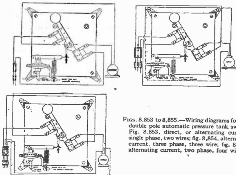
FIGS. 8,853 TO 8,855.—Wiring diagrams for Hill double pole automatic pressure tank switch. Fig. 8,853, direct, or alternating current, single phase, two wires; fig. 8,854, alternating current, three phase, three wire; fig. 8,855, alternating current, two phase, four wire.
