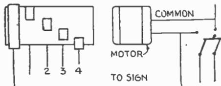
FIG. 8,614.—Smoke, steam, etc. These effects are wired in crescent form. The shapes, sizes and lengths being irregular; semi-circles being numbered 1-2-3-4 in an upward and outward direction. A speed type flasher is used for this work.
