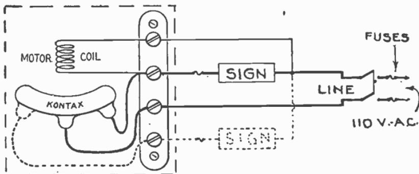
FIG. 8,571.—Wiring Diagram for Leland junior flasher. One on and off circuit or two alternating circuits. Dotted connections not used with single circuit flasher.
