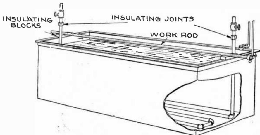
FIG. 8,276.—Cleaning tank. Typical installation of steam heating coils for heating plating solutions and cleaners. Approximate length of pipe needed for each 10 gals. of solution:  $\frac{3}{4}$  stranded pipe, 4 lineal ft.; 1 in. stranded pipe, 3 lineal ft.;  $1\frac{1}{4}$  in. stranded pipe,  $2\frac{1}{2}$  lineal ft.;  $1\frac{1}{2}$  in. stranded pipe, 2 lineal ft.
