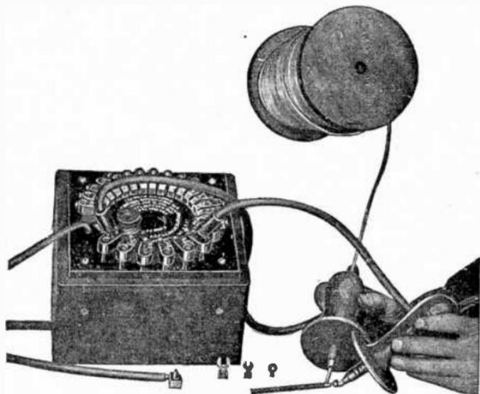
FIG. 8,216.—Chapman universal armeter used with carbon contact resistance soldering leads. Connect pair of No. 8 flexible leads to say 0 and 5V terminals.
