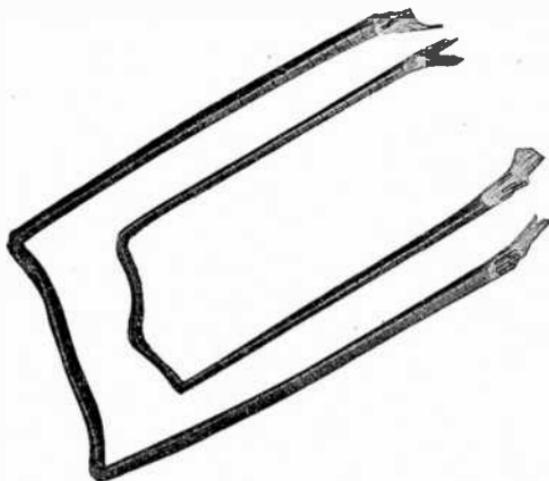
FIGS. 8,245 and 8,246.—Reliance armature coils. *They are made* of strands of insulated copper wire, formed and taped together and further insulated with a coat of varnish. After winding the entire armature is painted with a special high temperature, non-flowing black finish, and baked. Each coil is then carefully tested.
