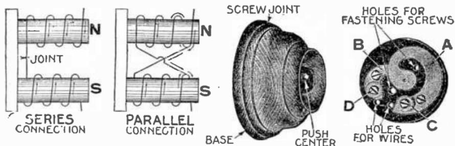
FIGS. 8,464 and 8,465.—Reducing resistance of bell coils. When connected in parallel (fig. 8,465) the resistance is reduced one half, allowing more current to flow through the coils for a given voltage.
