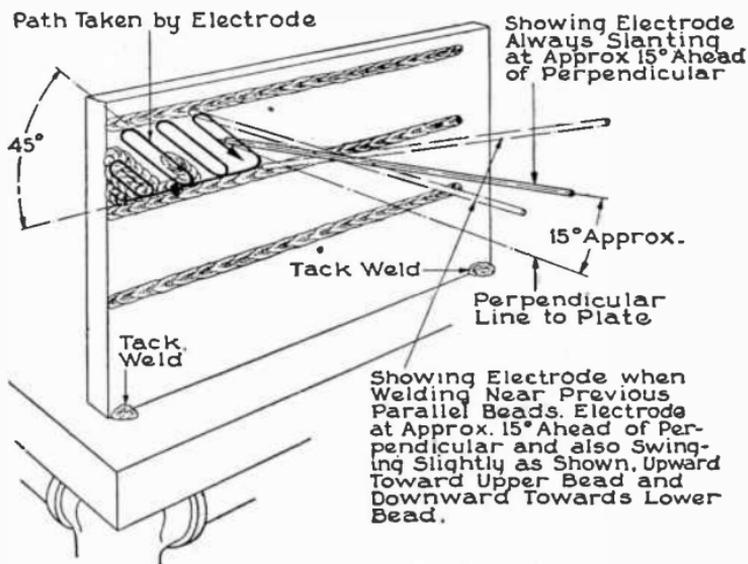
FIG. 8,096.—Lesson II. Method of filling in between parallel, horizontal spread beads on vertical plate.
