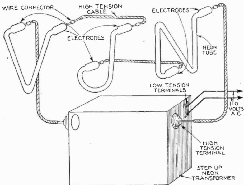
FIG. 8,338.—Neon tubes showing wiring connections.
