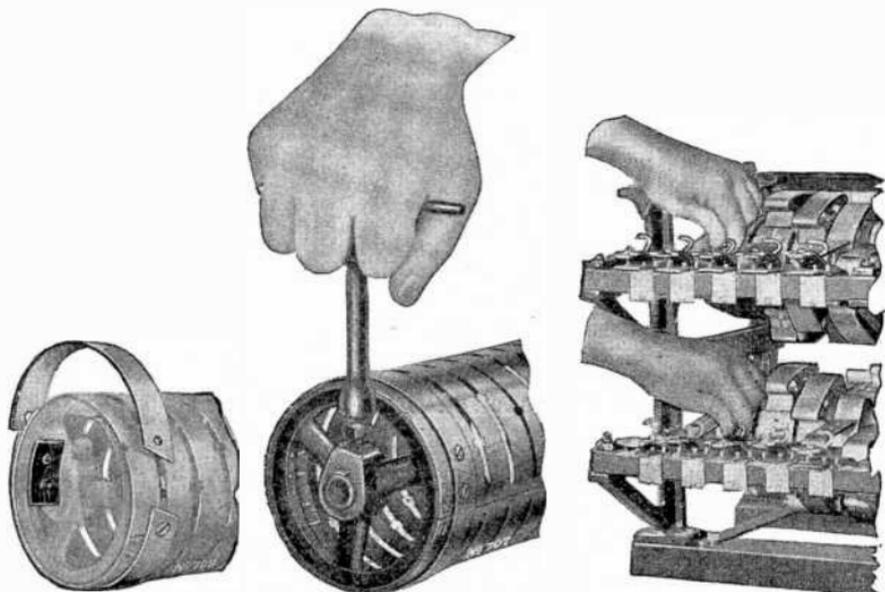
FIGS. 8,580 to 8,582.—Reynolds flasher details. *Fastening collector rings* (fig. 8,580). Spicer plate which acts as a duplex nut, enables the repair man to renew the collector rings quickly and easily. *Keep drums tight on shaft* (fig. 8,581); a socket wrench should be used for this purpose. *Resetting brushes* (fig. 8,582) use fingers as shown.
