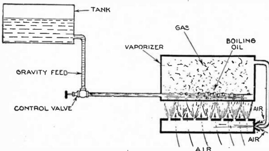
FIG. 8,701.—Elementary gravity feed induction mixing vaporizing burner. *In operation*, oil flows from tank to vaporizer, regulated by the control valve. The flame from the burner vaporizes the oil entering the vaporizer producing a gas which passes out to the mixer. The gas is injected through a nozzle into the mixer sucking in air, the mixture passing out and igniting at the top.
