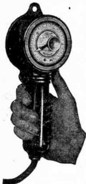
FIG. 8.999.—General Electric Victor hand timing switch for timing the exposure of radiographs. *In operation* the dial is set to the point on the scale indicating the desired number of seconds for the exposure, and upon pressing the button on the side of the handle, this time interval is automatically measured.
