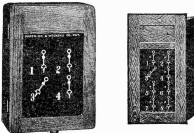
FIG. 8,477.—Partrick & Wilkins 4 point hand reset annunciator for *d.c.*, 4 to 6 volts or *a.c.* (transformer) not less than 12 volts, 25 watts. The hand reset is operated by a button at the bottom of the case.
