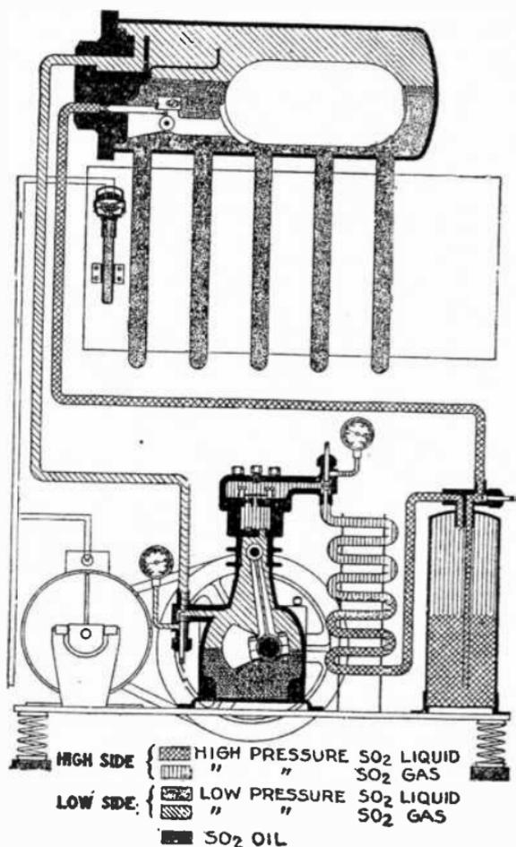
FIG. 8,680.—Kelvinator flooded system cycle.
