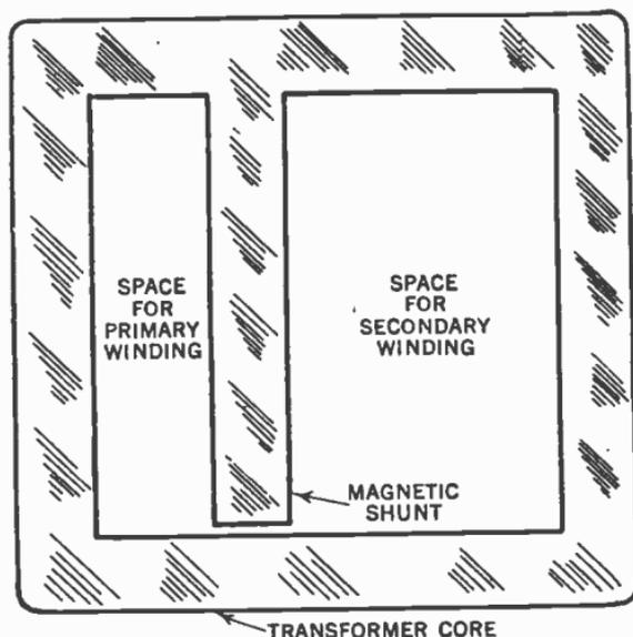
FIG 1.—Outline of neon sign transformer core.
