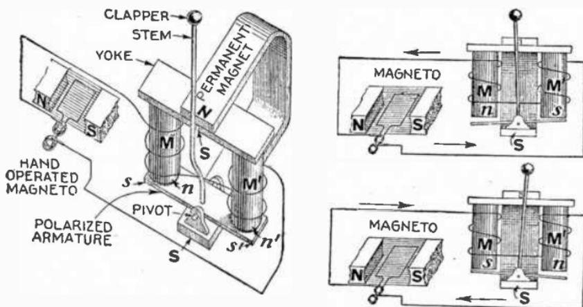
FIG. 8,454.—Elementary *a. c.* bell polarized by magnetic induction. N and S, are permanent magnet poles, and *n* and *s*, poles induced by the permanent magnet.
