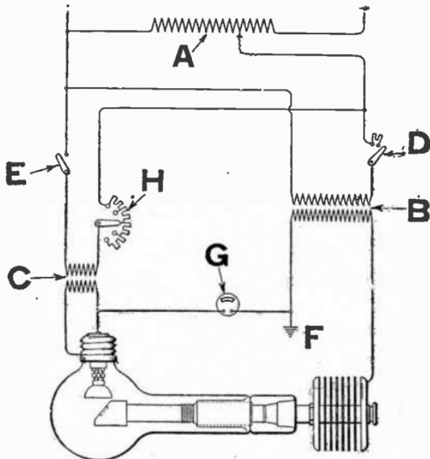
FIG. 8,989.—Coolidge wiring diagram of radiator, dental type tube circuit. *The parts are* A, auto transformer, 100 to 120 volts; B, X-ray transformer; C, filament transformer; D, X-ray switch with resistance; E, filament-switch; F, ground connection; G, milli-ammeter; H, filament control.
