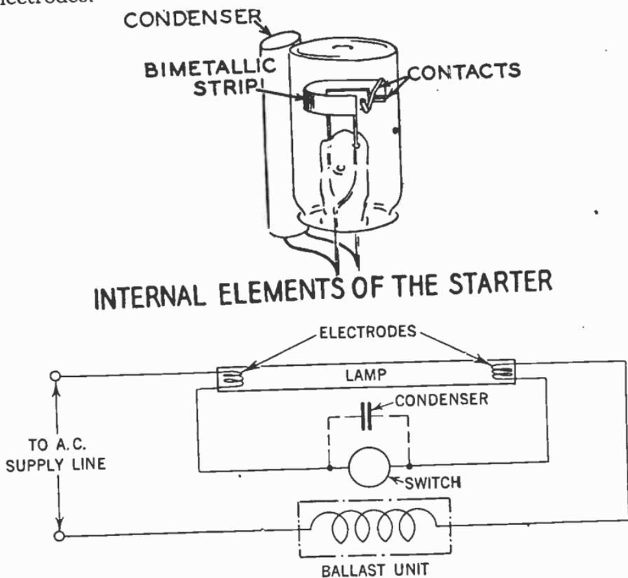
Figs. 9 and 10.—Glow switch starter and connection to lamp unit.
