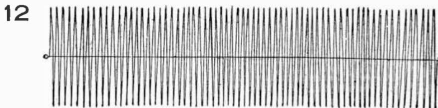
FIG. 9,015.—Waveless oscillatory current. This modality is somewhat comparable to No. 16 (rapid sinusoidal), excepting that it does not follow the sine wave form and its frequency is higher, while the duration of each impulse is the same as with No. 9 (oscillatory wave).
