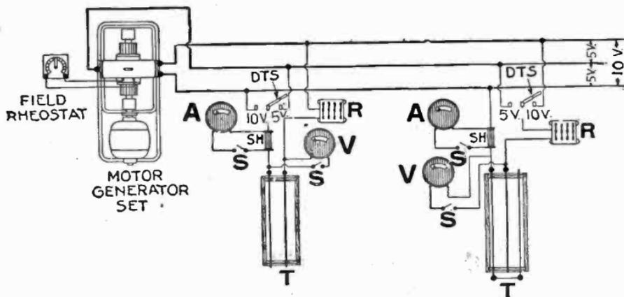
FIG. 8,279.—Diagram of three wire system with double throw tank switches for 5 or 10 volts. A, ammeter; V, volt meter; SH, ammeter shunt; R, tank rheostat; S, single pole switch; DTS, single pole double throw switch; T, plating tanks.
