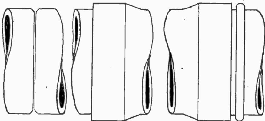
FIGS. 8,166 to 8,168.—Various pipe joints for welding. Fig. 8,166, butt weld; fig. 8,167, bell and spigot weld; fig. 8,168, bell and spigot weld with welding dam.
