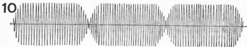
FIG. 9,013.—Oscillatory wave sustained peak. The curve shows the general form of the wave.
