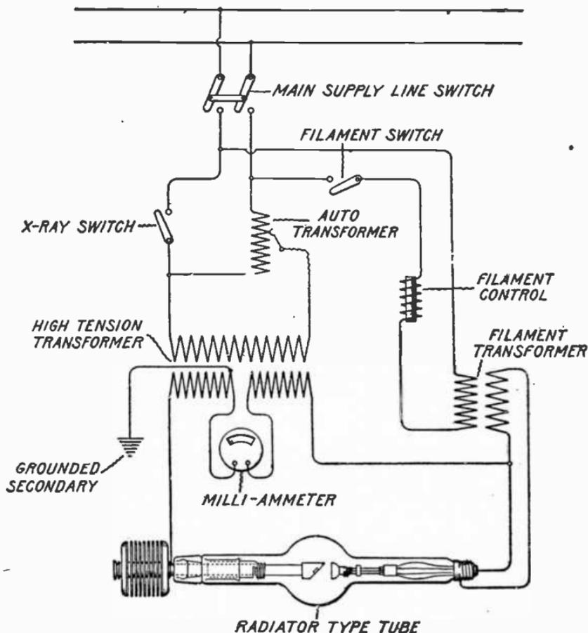
FIG. 8.992.—Coolidge wiring diagram of radiator type tube on unrectified current.
