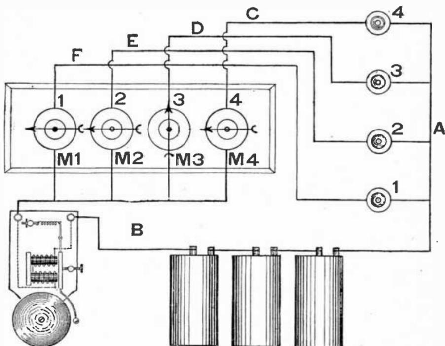
FIG. 8,489.—Method of wiring an annunciator; diagram shows the various circuits, bell, battery, push button, drops, etc.
