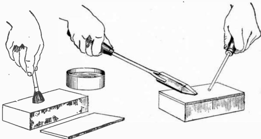
FIGS. 8,209 to 8,212.—*Sweating*. When two surfaces are to be united by sweating, first see that the surfaces are perfectly clean, then flux as in fig. 8,209. Put a piece of tinfoil over one surface and the other surface on top. They should be held firmly together by a clamp or other means and heated as in fig. 8,212 by a hot bit, or if the metal have considerable thickness by a torch, until the solder melts. When cool, the surfaces will be found to be firmly united.
