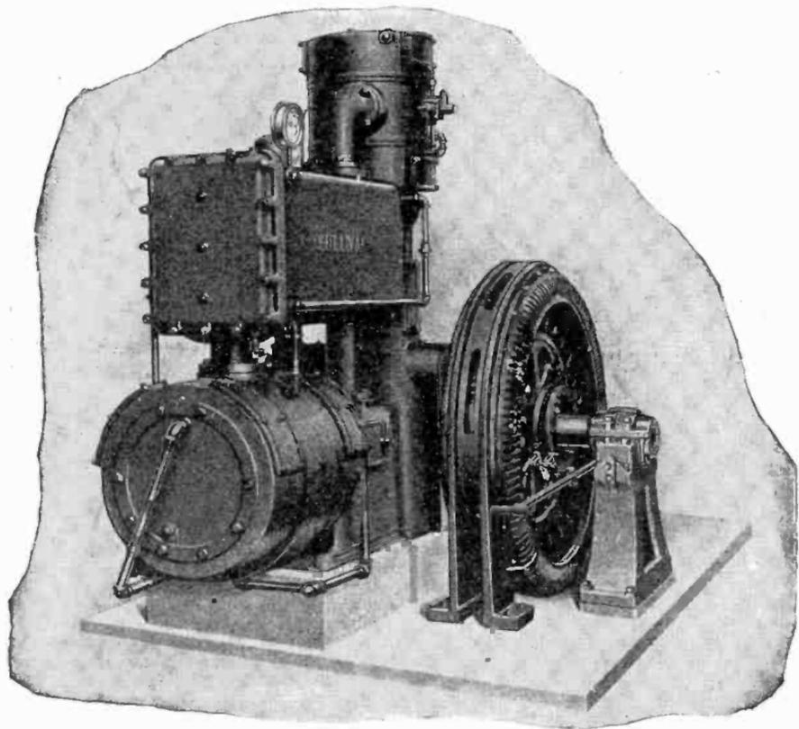
FIG. 8,943.—Sullivan angle-compound compressor direct connected to electric motor. Recent improvements in synchronous motors have made it possible to employ a simple and compact design of direct connected motor drive on angle-compound compressors. The rotor is mounted directly on the crank shaft close to the compressor frame, allowing sufficient room for getting at the bearing boxes.
