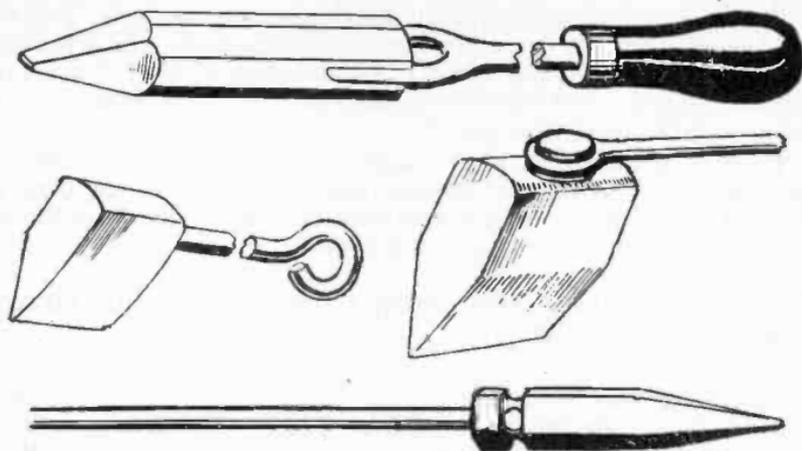
FIGS. 8,194 to 8,197.—Various soldering bits, or so called "irons." Fig. 8,194, ordinary edge bit; figs. 8,195 and 8,196, hatchet bits; fig. 8,197, pointed bit.
