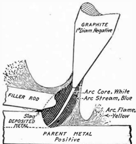
FIG. 8,105.—Correct position for graphite electrode and metal filler rod.
