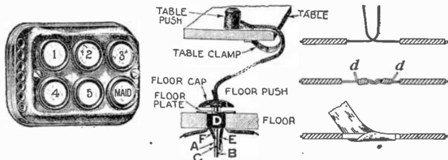
FIG. 8,469.—Paper weight type of multi-push button, suitable for desk use.
