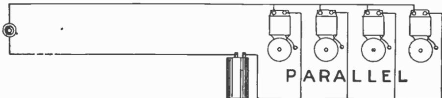
FIG. 8,485.—Several bells connected in parallel to ring from one push button.
