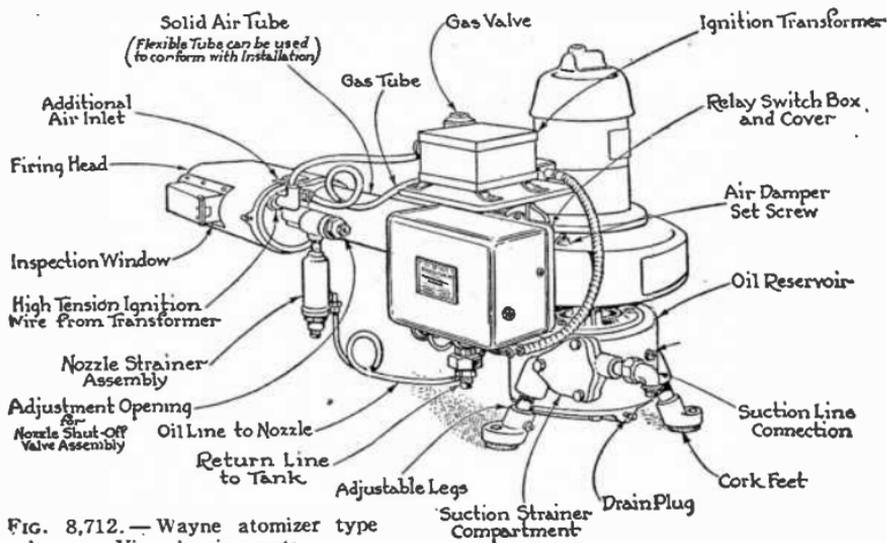
FIG. 8,712. — Wayne atomizer type burner. View showing parts.
