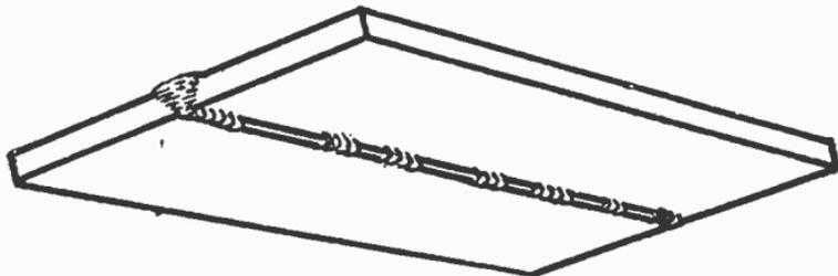
FIG. 8,159.—Underside of weld showing incomplete penetration.
