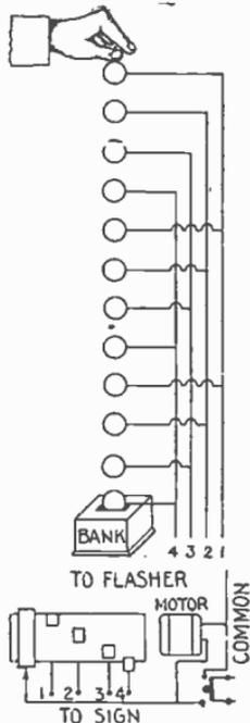
FIG. 8,604.—Dropping coins, juggling clowns, flying sparks. These and similar effects are wired 1-2-3-4 as here shown. This method gives a realistic action and is inexpensive, as it takes only a four brush flasher. The contacts on the flasher are set so that only one brush is in circuit at one time.
