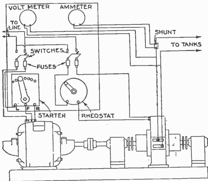
FIG. 8,268.—Method of connecting motor dynamo set, consisting of a *separately excited* dynamo and *d.c.* motor.
