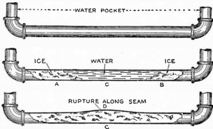
FIGS. 8,800 to 8,802.—Familiar occurrence illustrating the rupture of water pipes due to the expansion of water in freezing.
