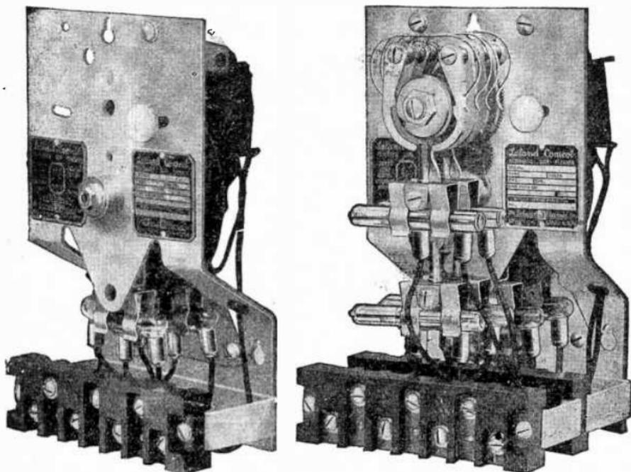
FIG. 8,568.—Leland speed border flasher; unit type for four circuits. The usual practice is to divide the display into four circuits or groups of circuits, and order the flasher for 1-2-3-4 wiring; or 1 to 4 wiring. The flasher then turns on the four circuits in succession and repeats interminably, each circuit going dark before the one preceding it is lighted up, so that there is always one or two circuits dark out of each set of four.
