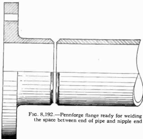
FIG. 8,192.—Pennforge flange ready for welding to pipe. Note the space between end of pipe and nipple end of flange.
