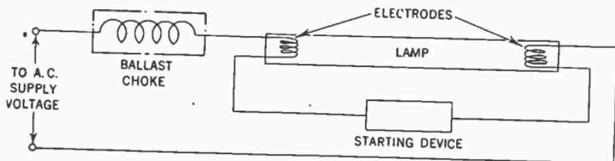
FIG. 8.—Schematic diagram showing connection of fluorescent lamp.
