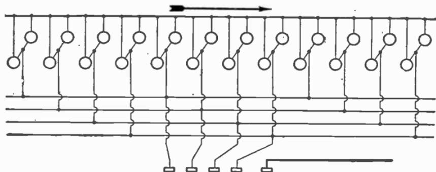
FIG. 8.595.—Number sockets 1-2-3-4. Connect all No. 1 to circuit No. 1 and to flasher brush No. 1. Nos. 2, 3, and 4 likewise. Keep in mind, that the direction of the numbering determines the direction of movement of the shadows.
