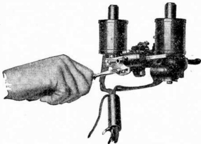
FIG. 8,777.—Delco electro-magnetic throttle control with cover removed showing method of adjusting.
