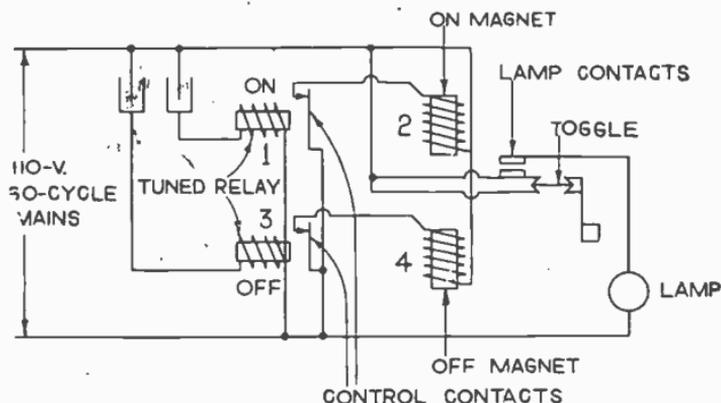
FIG. 8,429.—Diagram of Westinghouse resonant control unit. The tuned relays are shown at 1 and 3. The switch or contactor in the lamp circuit is of the toggle type; that is, it is pulled over a center and will remain permanently open or closed as the case may be. The operating coils of this toggle switch are indicated at 2 and 4.
