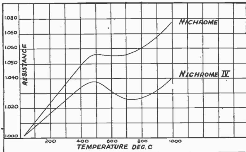
FIG. 8,217.—Temperature coefficient curves of "Nichrome" and "Nichrome" IV here shown represent wire slowly cooled from 1000° C. as specified by the American Society for Testing Materials. Slight variations from this curve may be expected due to variations in methods of annealing of different sizes of wire.
