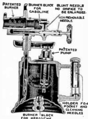
FIG. 8,203.—Bernz gasoline torch with holder for heating soldering bits.
