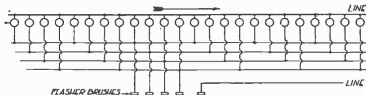
FIG. 8.593.—The number of sockets must always be a multiple of 4, 6, or 8, otherwise at some point a jump will occur.
