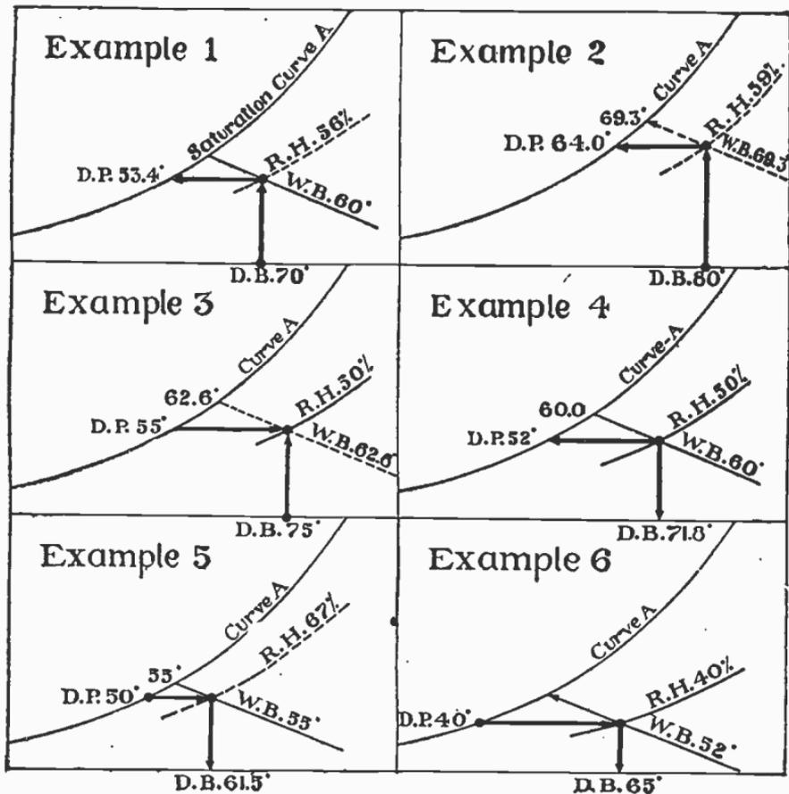
Figs. 8,766 to 8,771.—Diagrams to accompany the examples illustrating methods of using the psychrometric chart.
