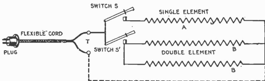
FIG. 8,241.—Arrangement of internal circuit for heaters giving three heating values. *In the diagram A*, represents one-third of the heating circuit; *BB*, two-thirds. With switch *S*, on, one-third of full heat is given; with *S'*, two-thirds, while with both *S*, and *S'*, on, the heater works with full power. At *T*, are two terminals to which the ends of the flexible cord from the plug are secured.
