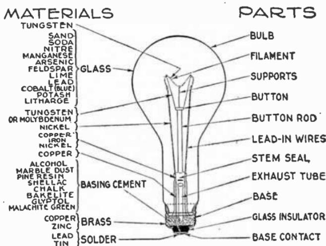
FIG. 8,294.—Materials and parts of an incandescent lamp.
