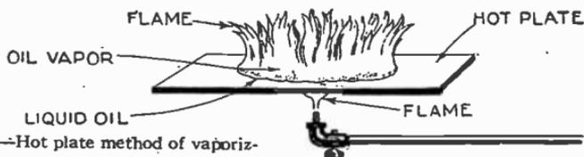
FIG. 8,714.—Hot plate method of vaporizing oil.
