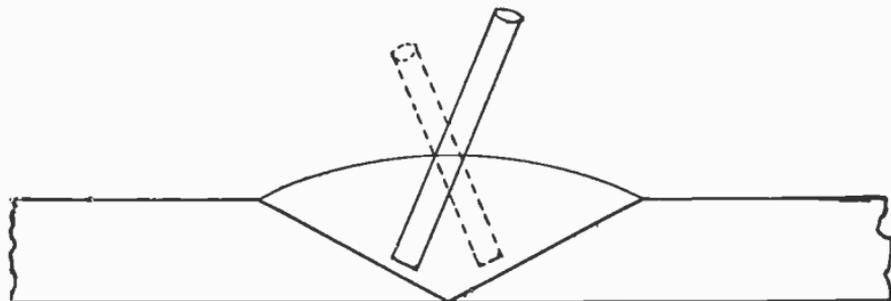
FIG. 8,056.—Best theoretical welding angle.
