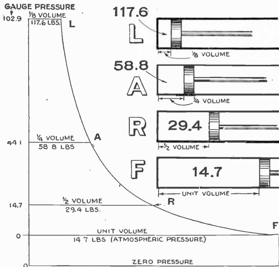
Figs. 8,927 to 8,931.—Diagram and compression stroke progressively shown illustrating *Boyle's law*. As the piston travels from position F, to R, A, L, the pressures are 14.7, 29.4, 58.8, 117.6 lbs absolute, respectively, being *inversely proportional to the volume*. The points F, R, A, L, on the compression curve correspond to the piston positions F, R, A, L as shown.
