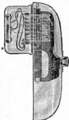
FIGS. 8,441 and 8,442.—Bunnell *a.c.* and *d.c.* single stroke bell for series or parallel circuits. In construction the only moving part is a heavy plunger, which travels within a moulded condensite tube when the current is turned on. The plunger strikes the gong a single, direct blow, setting it in complete vibration.
