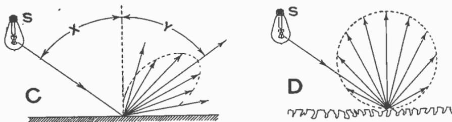
FIGS. 8,374 and 8,375.—Effect of various media on light rays. C, reflection from semi-mat surface; D, reflection from rough mat surface.
