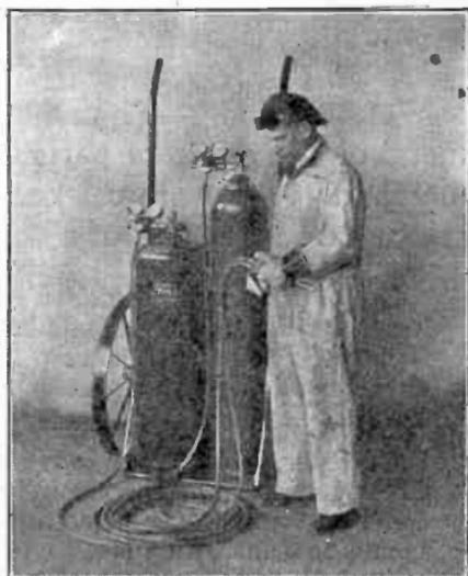
FIG. 8,143.—*Connecting the hose to torch.* (Airco-Davis-Bournonville.) Connect the red acetylene hose to the needle valve stamped "ac" and the black oxygen hose to the "ox" needle valve.
