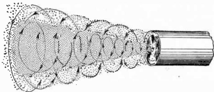
FIG. 8,709.—Method of commingling air and atomized oil by whirling each in contrary direction in conical streams. The oil stream comprises the inner cone, while the air stream comprises the outer.
