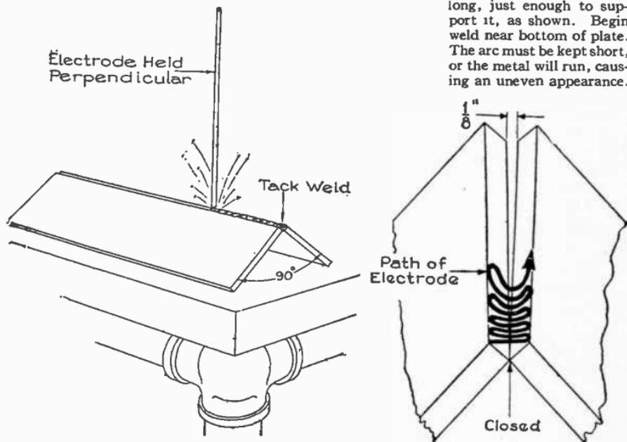
FIGS. 8,083 and 8,084.—Lesson 6. Straight butt weld method of making right angle butt weld in horizontal position. Good appearing weld, even across the top without bumps, cracks, or
