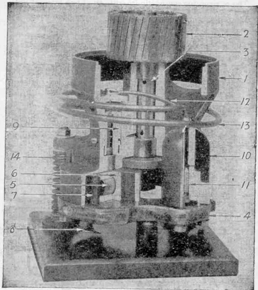
FIG. 8,685.—Cutaway section of General Electric refrigerator machine. The parts are: 1, main frame; 2, rotor; 3, main shaft; 4, bearing plate; 5, piston; 6, cylinder; 7, muffle box; 8, oil screen; 9, unloader; 10, surge chamber; 11, check valve plunger; 12, unloader tube; 13, suction tube; 14, supporting springs.
