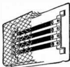
FIGS. 8,231 and 8,232.—Application of space heaters under floor and on wall.
