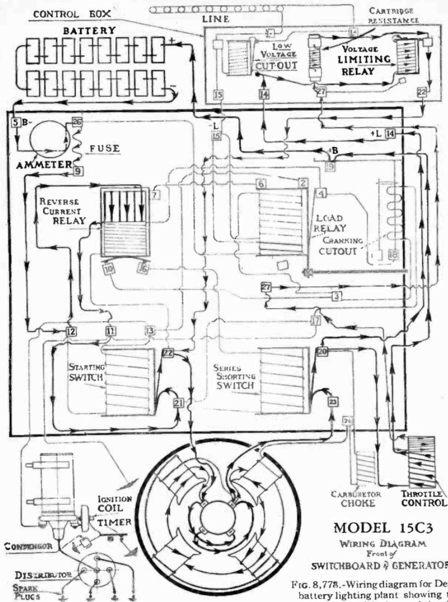
FIG. 8, 778. -Wiring diagram for DeLco battery lighting plant showing the various control devices and circuits,
