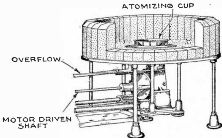
FIG. 8,706.—Motor driven centrifugal atomizing burner.
