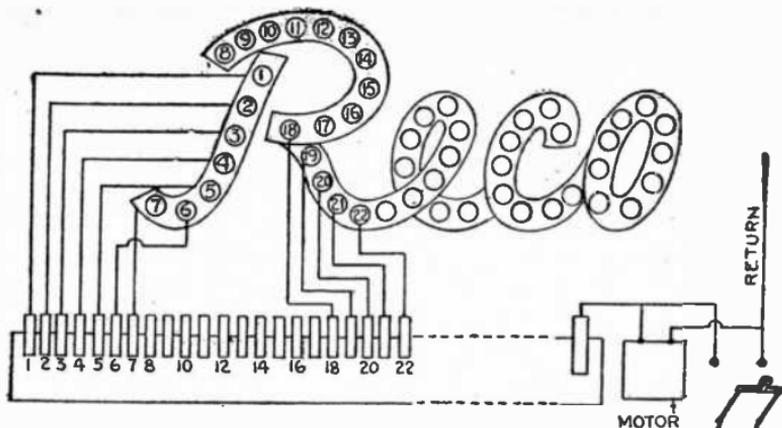
FIG. 8,615.—Reproducing invisible handwriting effect in script letter signs. Script letter signs are usually wired two sockets to a circuit; thus if the total number of sockets be 100, 50 circuits and 50 brushes on the flasher are required. The flourish or tail (if any) can be flashed as one, to save wiring. Letters of large size can be wired 4, 6, 8 or more sockets to a circuit without impairing the effect.
