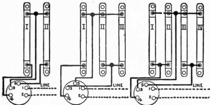
FIG. 8,238.—Two heaters and snap switch. *High*, full heat, heaters 1 and 2; *medium*, one-half heat, heater 2 only; *low*, one-quarter heat, heaters 1 and 2; *off*.
