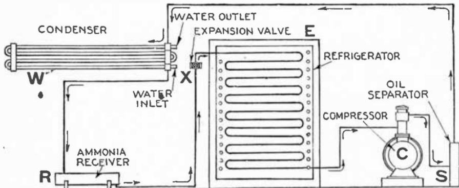
FIG. 8,660—Ammonia compression system; 1, direct expansion method. In operation, liquid ammonia stored in receiver R, passes through expansion valve X, into coils or piping located in the refrigerator E, to be cooled. After expanding, it returns to the compressor C, where it is compressed and pumped through the oil separator S, to the condenser W, where, by water circulation, the ammonia is condensed and drains in liquid form to receiver R.
