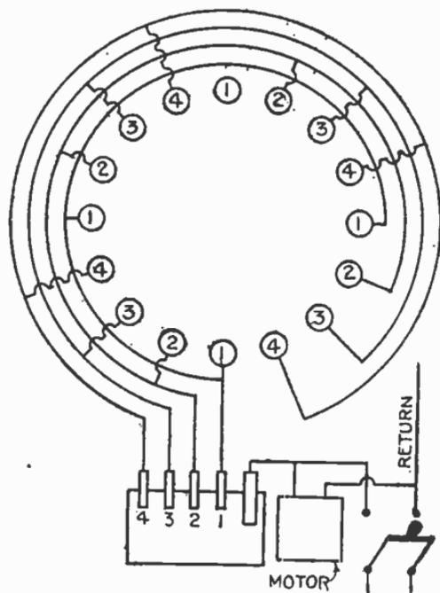
FIG. 8,616.—Traveling borders. circles and movements in general. The number of sockets must always be a multiple of 4, otherwise at some point a jump will occur.
