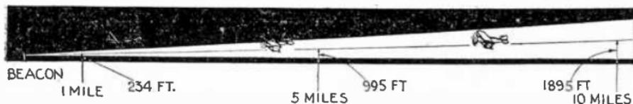
FIG. 8,413.—A beacon with only a slender pencil of light is ineffective at close range at normal flying height. *Requirements for air port beacons:* 1, high candle power for long range visibility; 2, visibility from all normal flying heights; 3, suitable duration of flash period; 4, positive identification.
