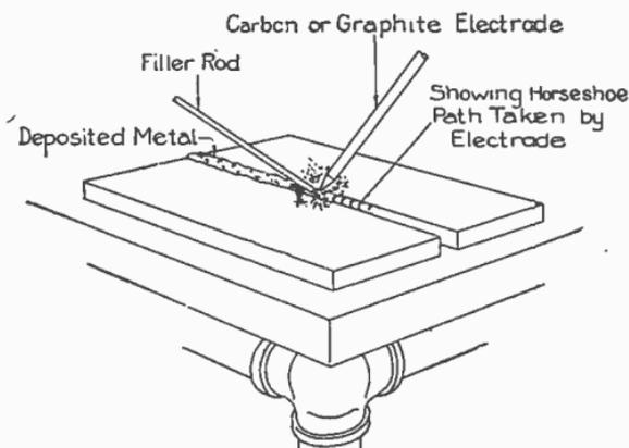
FIG. 8,107.—Electrode travel in making a butt weld with the carbon arc.
