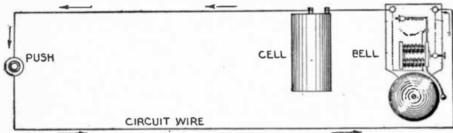
FIG. 8,481.—Simple bell metallic circuit.
