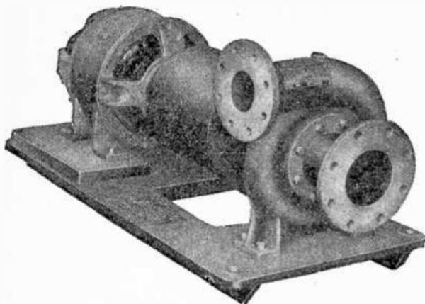
FIG. 8,795.—Fitz Rualite turbo-generator set comprising a completely self-contained hydro-electric power unit, including Fitz high speed water turbine direct connected to electric generator and provided with built in automatic governor. Standard units available in capacities ranging from  $\frac{1}{2}$  kw., capacity to 100 kw. capacity.
