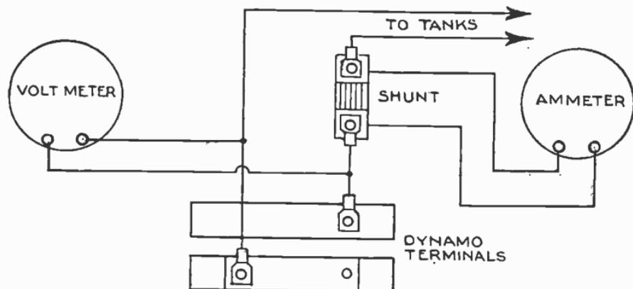
FIG. 8,265.—Volt meter and ammeter connections for two wire system.
