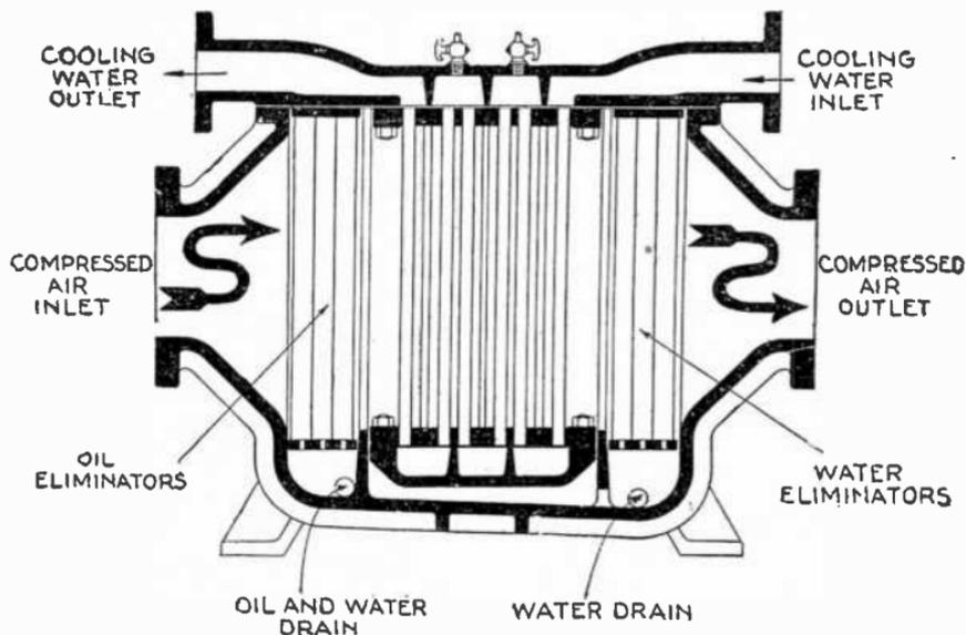
FIG. 8,953—Sullivan air or gas after cooler.
