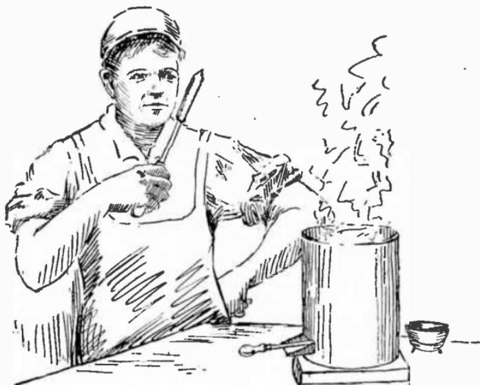
FIG. 8,628.—Method of judging the heat of a soldering bit or so-called "iron," illustrating *sensible heat*.
