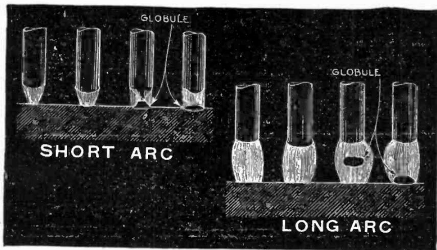
Figs. 8,024 to 8,027.—Short arc. From the globular formation it will be noted that the globule never is subjected to full heat of the arc, as it is in contact with molten metal in plate before it leaves tip of electrode. It will therefore be readily seen that the length of a short arc will vary with the diameter of electrode used, and what would be a long arc on  $\frac{1}{8}$  in. electrode might be too short for a  $\frac{1}{4}$  in. electrode.
