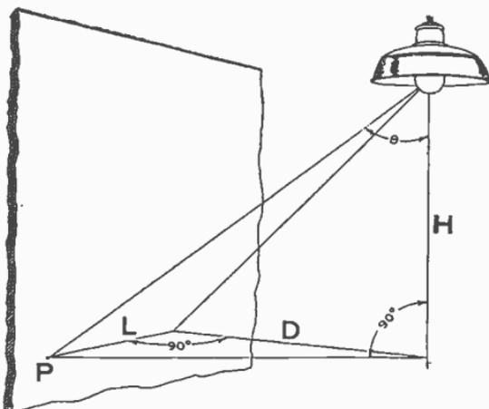
FIG. 8.388.—Illumination of vertical surfaces. *In calculating* the illumination at the point P on a vertical surface the distance H (vertical), D (horizontal), and L (horizontal to the surface) must be known. From  $\tan \theta = \frac{\sqrt{D^2 + L^2}}{H}$  the angle  $\theta$  may be found. From the distribution curve of the luminaire, determine the candle power at the angle  $\theta$  ( $CP_{\theta}$ ). Then the vertical illumination in foot candles at P is as follows:
