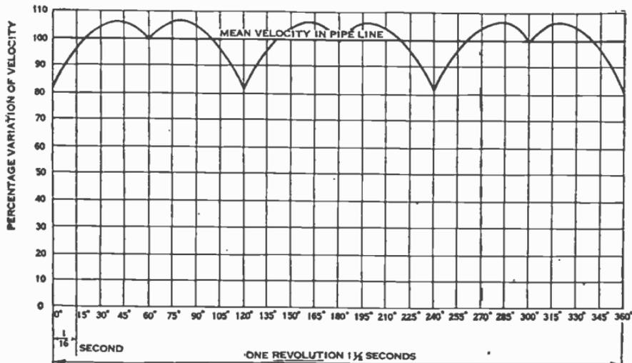
FIG. 8,840.—Diagram showing rate of delivery of single acting triplex pump expressed in percentage of mean velocity in pipe line.
