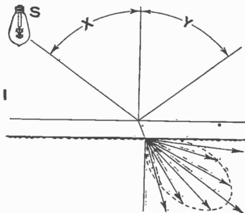
FIG. 8,380.—Effect of various media on light rays.  $P_r$ , reflection and transmission by etched glass.
