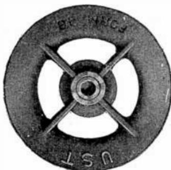
Figs. 6,190 and 6,191.—Trolley wheels. Fig. 6,190, Ideal trolley wheel; fig. 6,191, Union standard trolley wheel. The trolley wheel must not be hard enough to wear the wire unduly, it must not be soft enough itself to wear out readily, and it must have maximum conductivity. Union standard trolley wheels are made of phosphor bronze, while the Ideal trolley wheel is made with a forged copper center on either side of which steel flanges are pressed.
