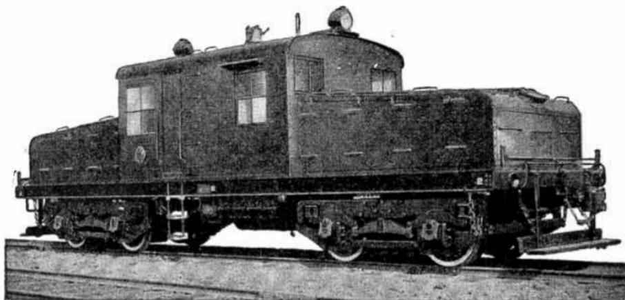
FIG. 6,146.—General Electric 60 ton storage battery type industrial haulage locomotive. The particular application is handling heavy loads for short hauls as is found in yard shifting, dock service, quarries, etc. Operation and repairs can be performed by men of ordinary ability.
