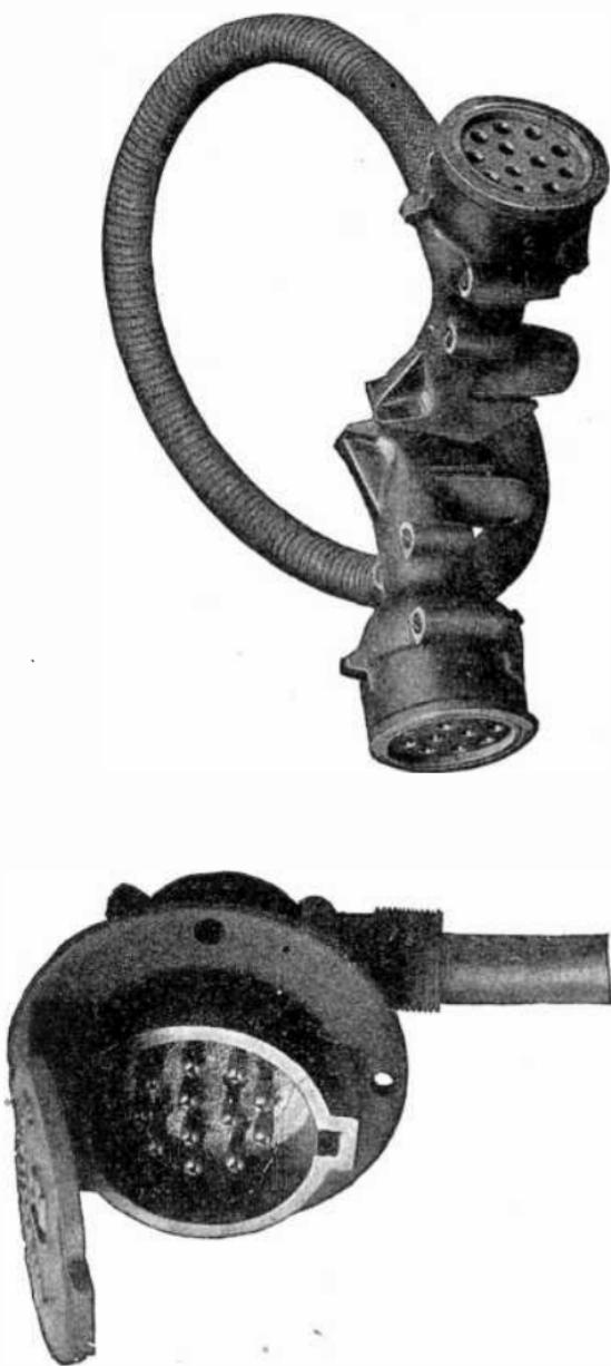
Figs. 6,269 and 6,270.—Westinghouse train line receptacle and jumper for connecting the control wires of one car with those of another thereby enabling the motors of several cars to be controlled from one controller.
