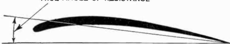
Figs. 7,127 and 7,128.—Angle of resistance as usually and incorrectly measured, and real angle of resistance. This error has crept in no doubt on account of the difficulty of measuring the angle shown in fig. 7,128.
