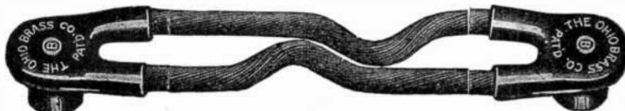
FIG. 6,416.—Ohio compressed terminal rail bond intended for installing on web of rail under splice bar. Can be used singly to span one or more bolts or can be combined for double or quadruple bonding. This is a balanced bond, the two cables being of the same size.
