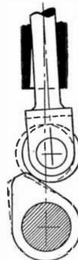
Figs. 7,034 and 7,035.—Valve push rod with roller shown in lifting and seating position, showing the serious defects of a worn push rod bushing. The dotted cams and rollers indicate the position these parts would have with the same amount of lift if there were no lost motion.
