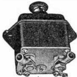
FIG. 7,089.—North East starting switch and cut out as used on Graham Bros. buses. Cut out 12 volt metal contacts. Shunt and series coils wound together.
