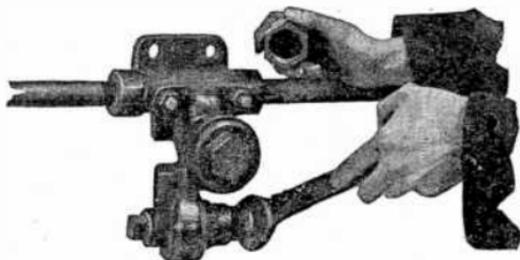
FIG. 6,273.—*Westinghouse control operation 2.* Adjusting reducing valve to change air pressure.
