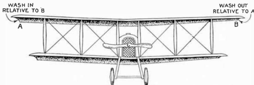
FIG. 7.130.—Front view of aeroplane illustrating the terms *wash in* and *wash out* which mean respectively the increase and decrease in the angle of incidence of the wings from the center toward the tips.
