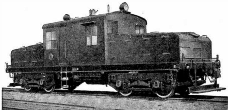
FIG. 6,146.—General Electric 60 ton storage battery type industrial haulage locomotive. The particular application is handling heavy loads for short hauls as is found in yard shifting, dock service, quarries, etc. Operation and repairs can be performed by men of ordinary ability.
