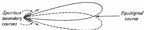
FIG. 17.—Typical antenna patterns that can be used to produce an ultra-high-frequency radio-range signal.
