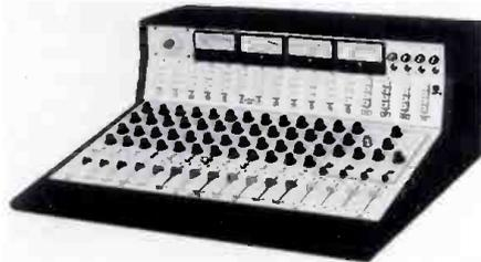
Individual input channels feature mix pot, cue switch, input select switch, echo send, and output assign. Low frequency EQ: 40 cy, 100 cy, 300 cy. High frequency EQ: 1.5KC, 3KC, 5KC, 10KC.
