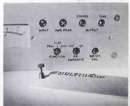
Pacific Recorders and Engineering Corporation has just announced the "MULTI limiter," an all new, multi-purpose limiter with selectable pre-emphasis for FM, FM Dolby, or Television; automatic polarity correlation and adjustable asymmetry for AM, and independent adjustment of RMS and peak limiting.
