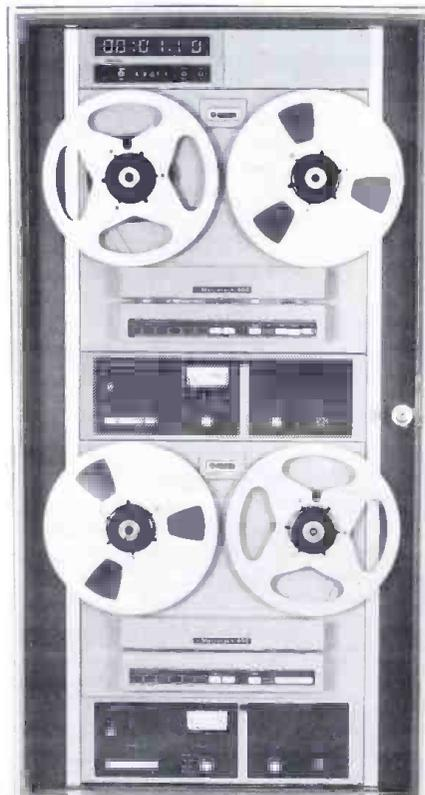
The system provides for automatic transfer to second deck at the end of the reel, or in the case of a tape break or time recording malfunction. Models include 1 channel 4 pass for up to 153.6 hours unattended at 5/16 ips; 2 channel 2 pass
