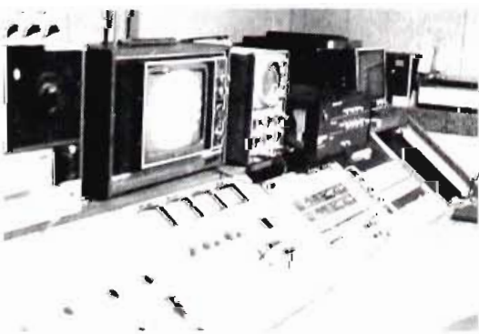
3M switcher, audio panel, 2020 time base corrector, and video control panel at Avonix Production Center.
