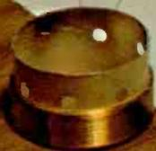
The voice coil is the heart of any speaker. A coil of wire. It moves the cone that makes the music. And in most speakers, that's all it does. But in the new E-V FIVE-A we've found a way to make this little coil of wire much more useful. Instead of one or two layers of wire, we wind the E-V FIVE-A woofer coil *four* layers deep.
