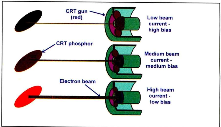
**Figure 13.** In order for a CRT to produce an image on the screen, the intensity of the electron beam from the cathode to the phosphor screen must be made to vary. Changing the bias voltage in step with the video image to be produced varies the beam current. White and bright colors require high beam current, while grays and dark colors require a small beam current.
