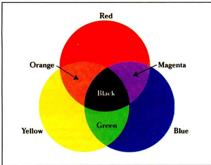
**Figure 3.** When paints, dyes, or pigments of two different colors are mixed, a third color results. The resulting material absorbs all the light energy that was absorbed by each of the two original materials.
