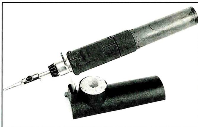
The iron utilizes catalytic conversion for the majority of its application configurations, delivering heat to the tip by means of infrared radiation. The fuel is liquid/butane/propane gas, stored in the translucent handle of the tool in a similar fashion to a disposable cigarette lighter. This tank is refilled with a squirt from a gas canister — a low-cost consumer item in use around the world. Each refill provides around 45 minutes of continuous use at a typical setting.
