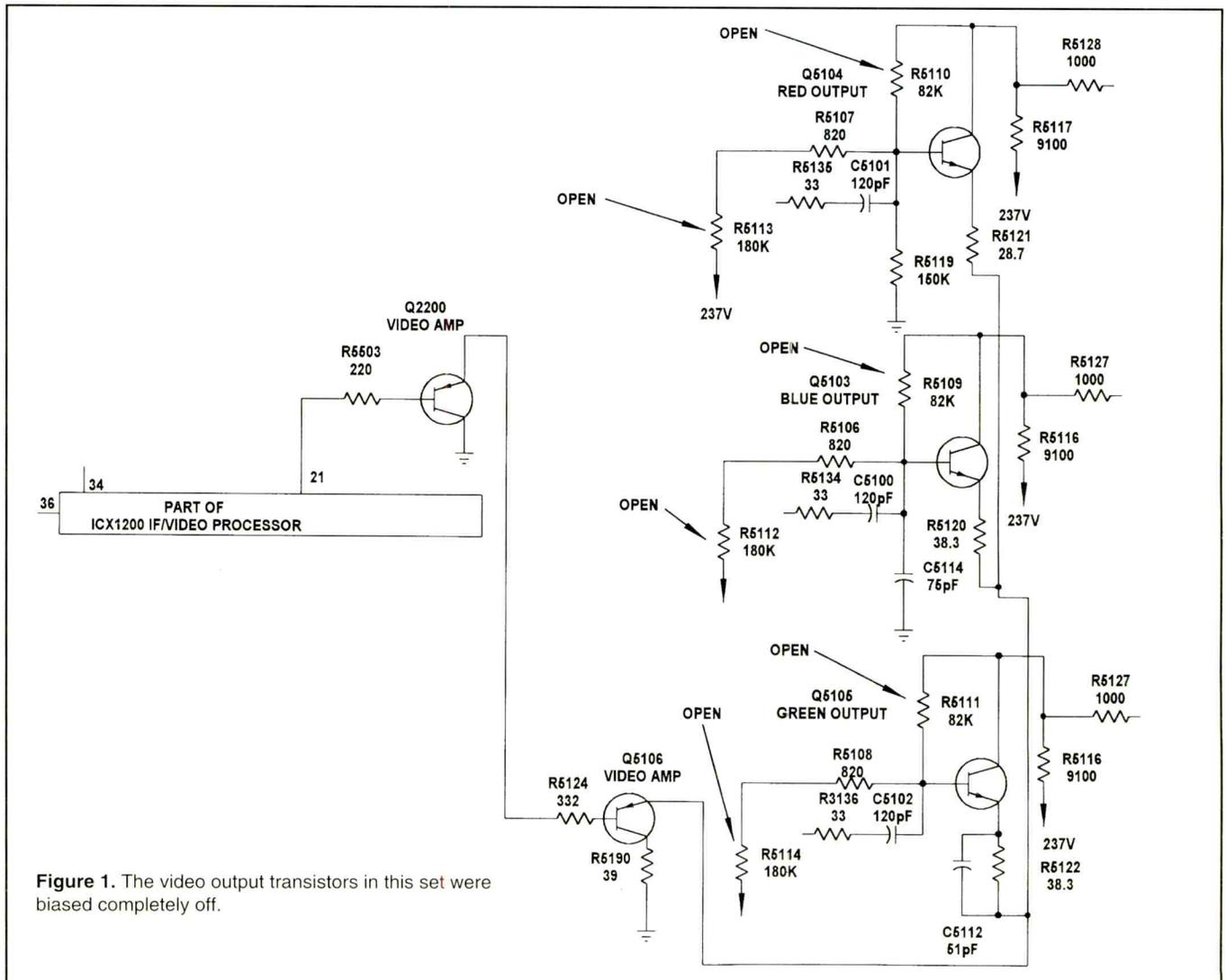
Figure 1. The video output transistors in this set were biased completely off.
