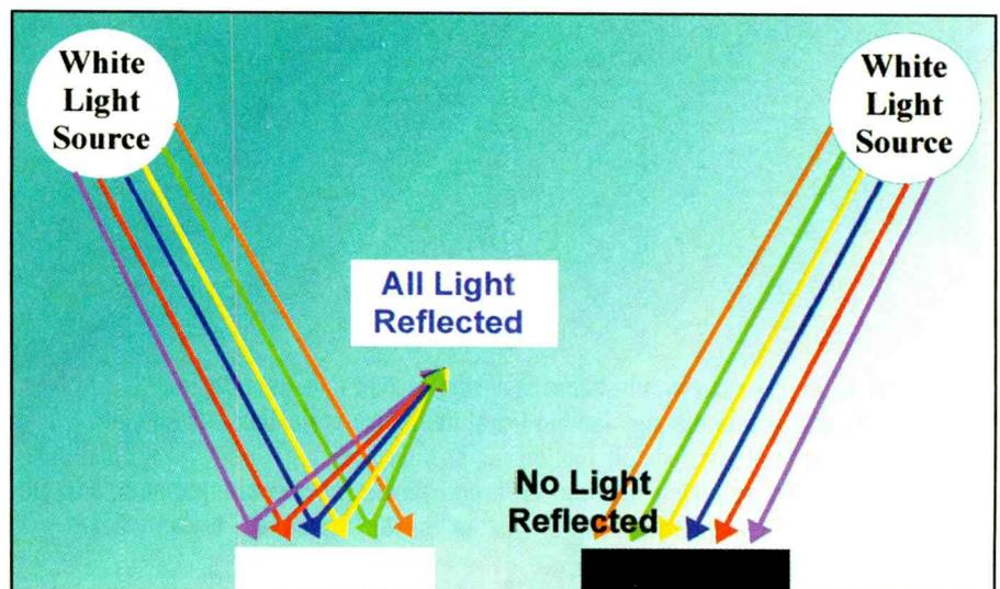
Figure 2. If the light energy from the sun is all equally reflected from some surface, the eye/brain sees the surface as white. If another surface absorbs all light energy and reflects none, the surface appears black to the human eye/brain.
