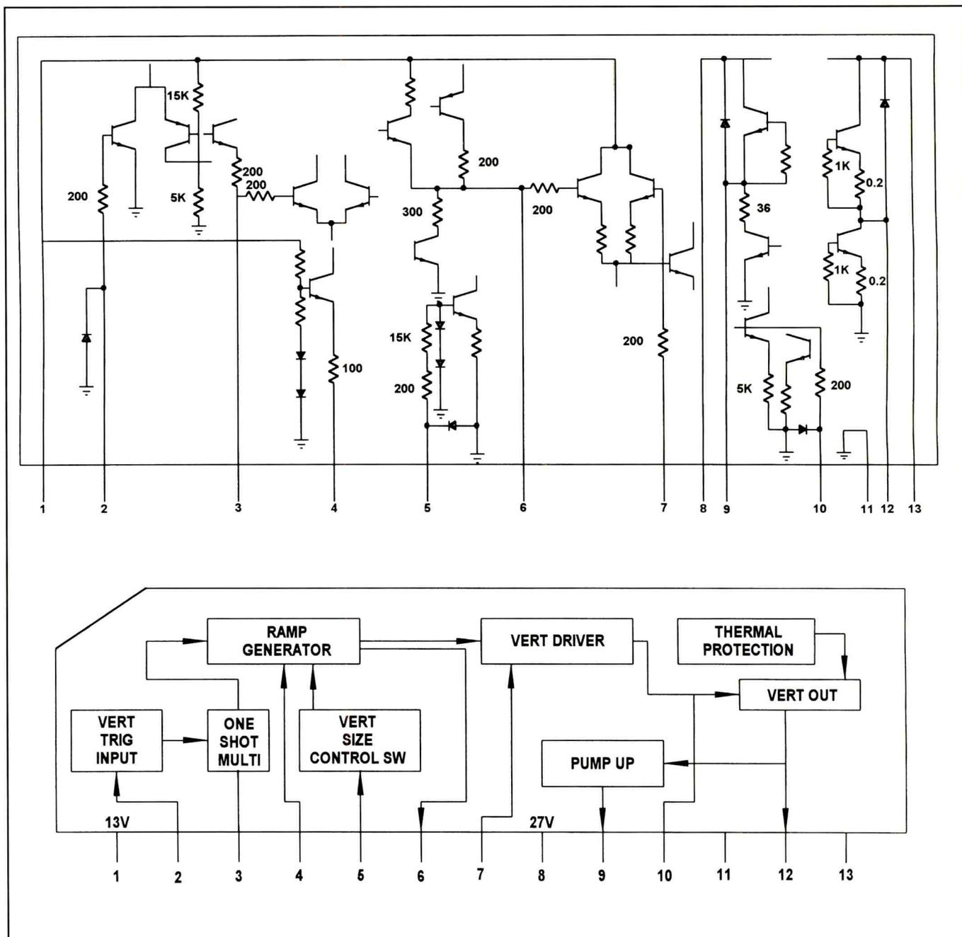
**Figure 4.** The LA78XX series of vertical output ICs (of which IC451 in the Quasar TS2523EK is an example) is used in a number of TV sets. The exact part number depends on the screen size, but the pinout remains unchanged. This particular one reproduces the insides of an LA7838 from the perspective of a Sharp engineer.
