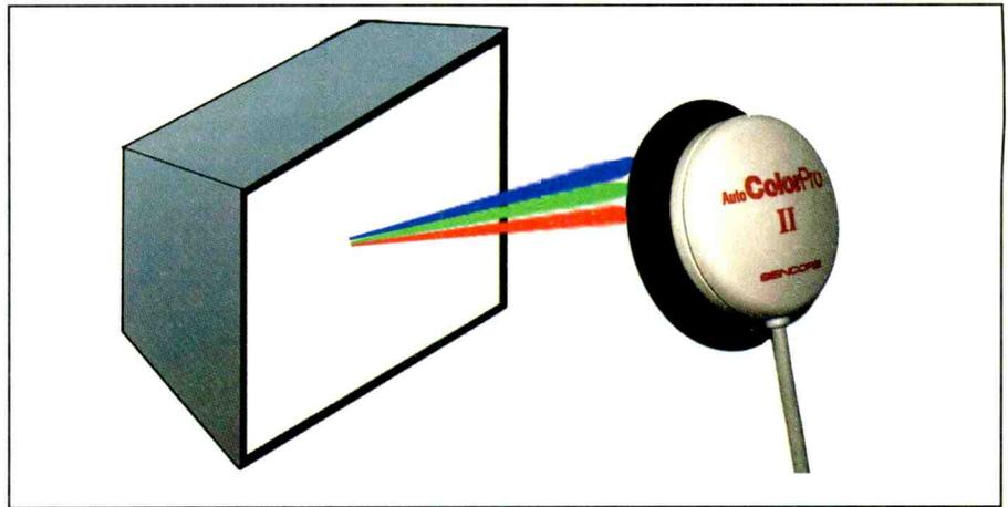
**Figure 15.** A color analyzer measures the x and y chromaticity and Y luminance or brightness parameters required for making computer monitor color and brightness adjustments.
