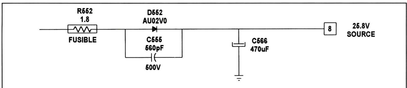
**Figure 3.** An open R552 in the +26V line of this Quasar model TS2523EK was the cause of failure of vertical deflection. Replacement of that component, and several other suspect components, restored the set to operation, and assured a long-term fix.
