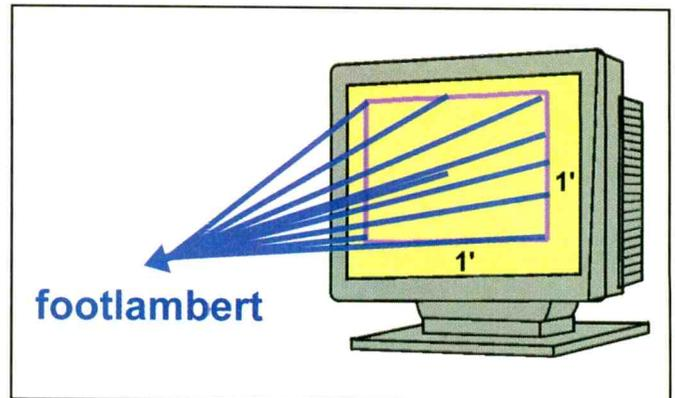
**Figure 8.** The footlambert is the U.S. measurement unit of luminance. It specifies the amount of light energy, per square foot, emitted from a light source (such as a CRT) or reflected from a lighted surface.
