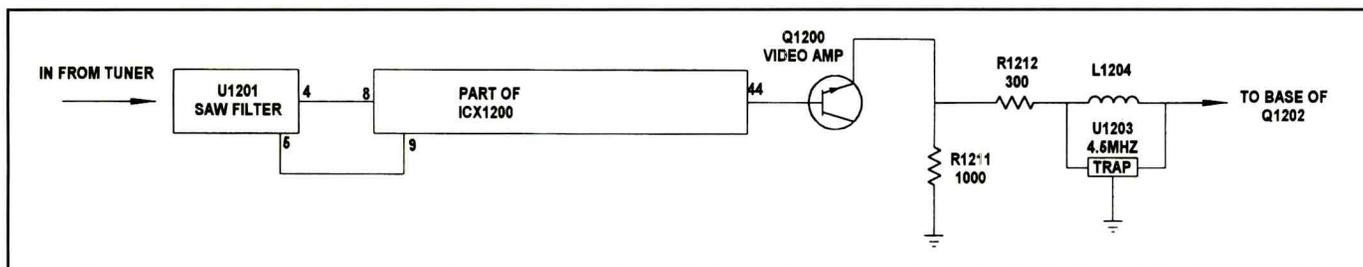
**Figure 2.** Video is processed in IC1200 and exits at pin 44 for further processing.
