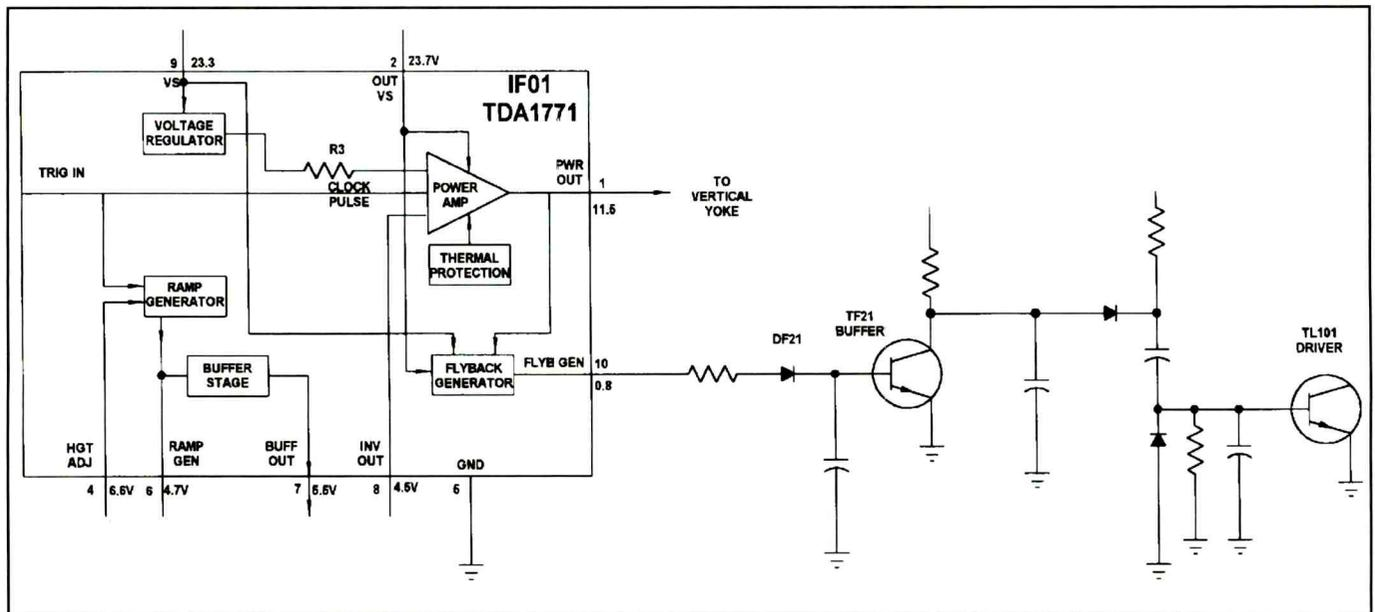
**Figure 6.** I was faced with an RCA T1960GY combi that had no vertical deflection. In this set, vertical drive exits pin 1 of IF01 and goes to the vertical yoke. Horizontal drive exits at pin 10, goes to TF21, configured as a buffer transistor, and on to the horizontal driver transistor (TL01). In this set, a shorted IF01 caused the unit to lose the +24V supply, which caused the horizontal drive to stop, and the set to shut down.
