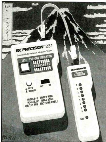
and RJ45/RJ11 modular cables, TIA-568A, TIA-568B, and Token Ring cables by comparing one transmitting end to the corresponding receiving end. It tests point-to-point rather than pair-to-pair. By utilizing the supplied remote kit, the Model 231 can test cables installed as far away as 1,000 feet, either on a wall plate or patch panel.
