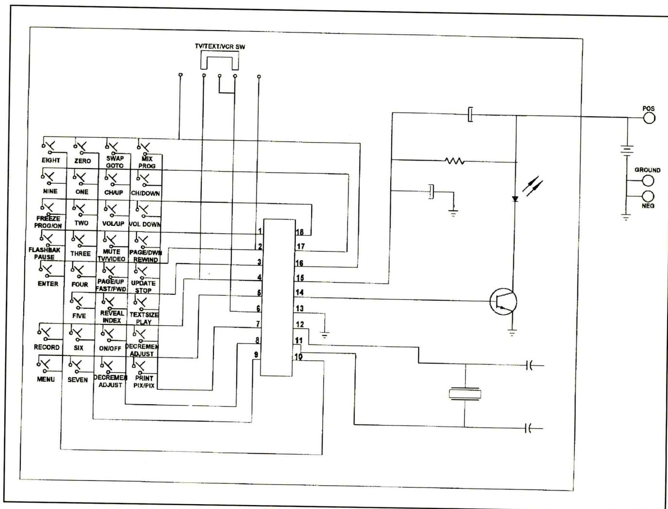
**Figure 1.** This drawing of a Zenith remote control manufactured sometime between 1985 and 1995 shows the functioning of a typical hand-held unit. If any of the push-button switches are dirty, the unit won't send the correct signal to the receiving unit in the TV set or VCR.
