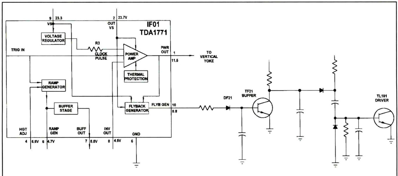
**Figure 6.** I was faced with an RCA T1960GY combi that had no vertical deflection. In this set, vertical drive exits pin 1 of IF01 and goes to the vertical yoke. Horizontal drive exits at pin 10, goes to TF21, configured as a buffer transistor, and on to the horizontal driver transistor (TL101). In this set, a shorted IF01 caused the unit to lose the +24V supply, which caused the horizontal drive to stop, and the set to shut down.
