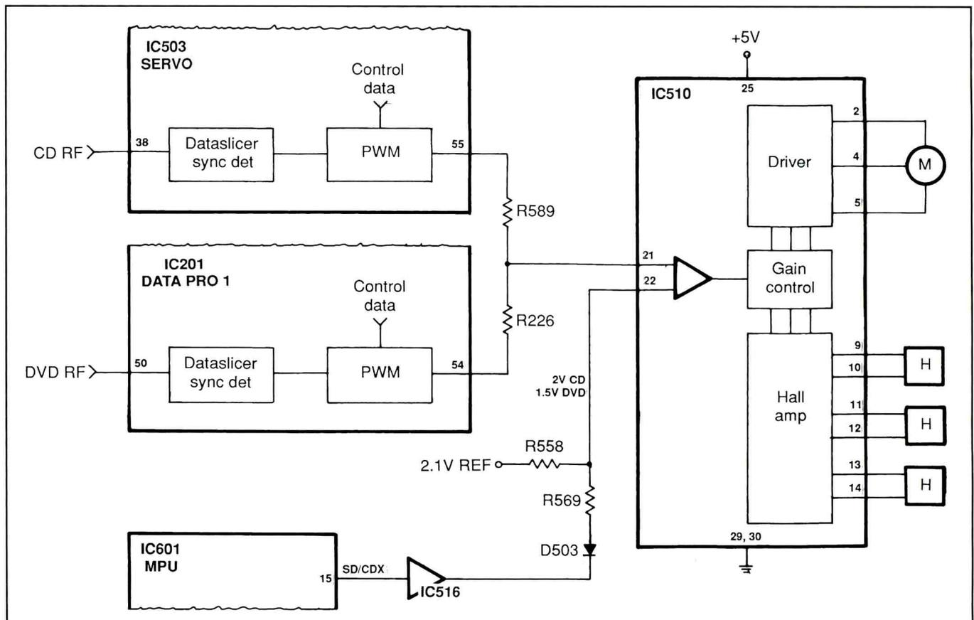
**Figure 3.** When a DVD disk is inserted into the player, after focus has been achieved, the pickup begins to generate an RF signal which is applied to pin 50 of IC201, the so-called "data processor one."
