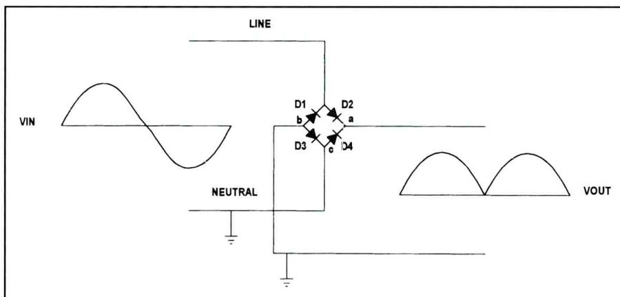
**Figure 2.** If point b were grounded, in effect diode D3 would have a short circuit placed across it, as both ends are at ground potential. Now when the line voltage goes negative the voltage forward biases D1, effectively placing the entire  $V_{max}$  across that diode.
