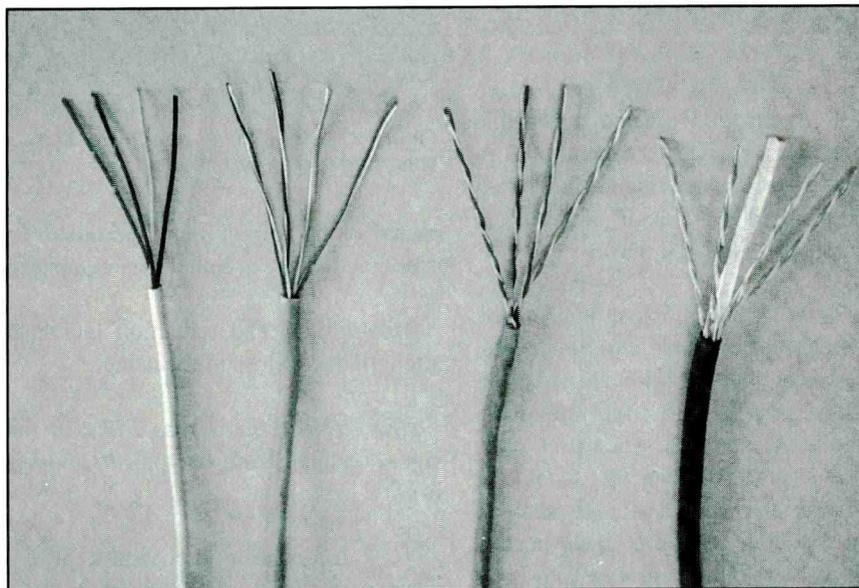
**Figure 1.** These are examples of unshielded twisted pair cable, comprised of 4 pairs of copper conductors.
