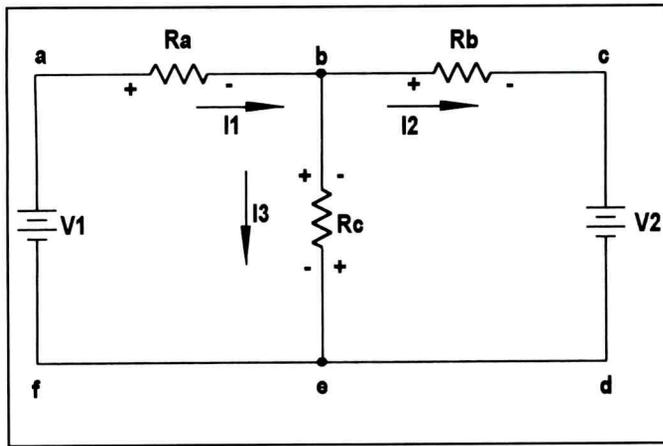
**Figure 2.** The values in this circuit can be determined by using one current node equation and two voltage loop equations.
