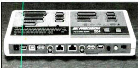
The Model 205 is a portable, stand-alone cable/harness tester that can be used for testing any type of wired assembly with up to 128 points. A universal connector card is designed to accept up to 28 of the most commonly used cable connectors. It is fast and detects opens, shorts, and miswires in less than 50 ns.
