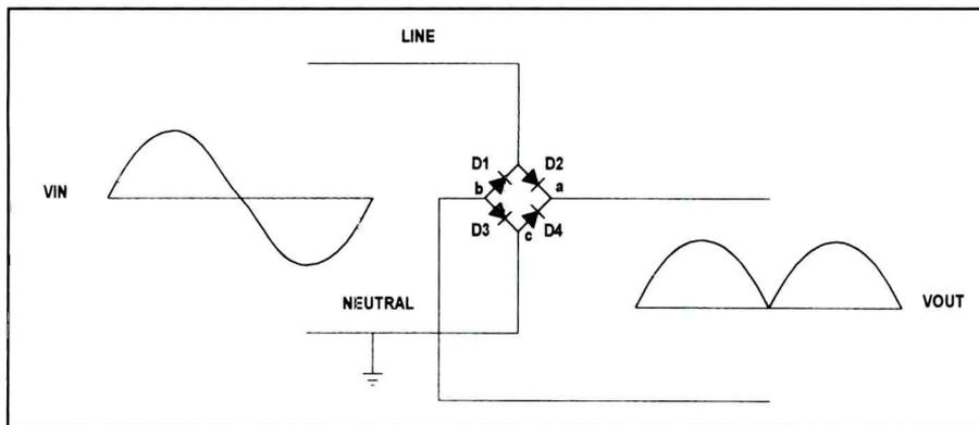
Figure 1. A full-wave bridge rectifier effectively inverts the negative-going segment of the power line ac. Note that the common side of the rectifier's output is not grounded.
