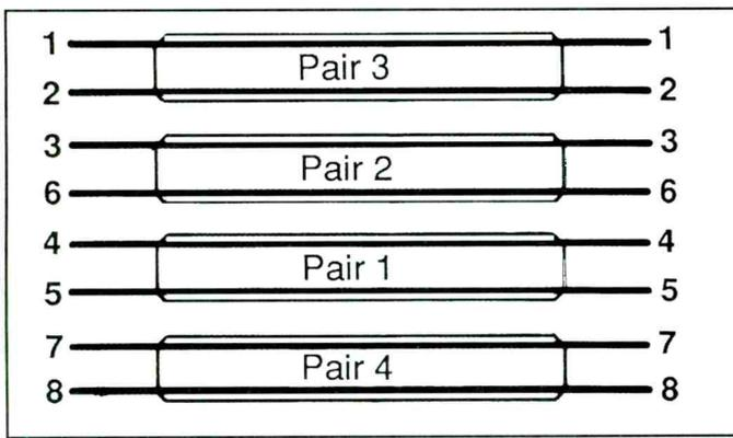
**Figure 8.** Wiremapping simply means that each wire is hooked up correctly, with no open wires or shorts. Most wiremapping failures are simple enough to understand, like reversed wires in a pair, crossed pairs or opens and shorts. The most difficult wiremap problem is a split pair, when one wire on each pair is reversed on both ends.
