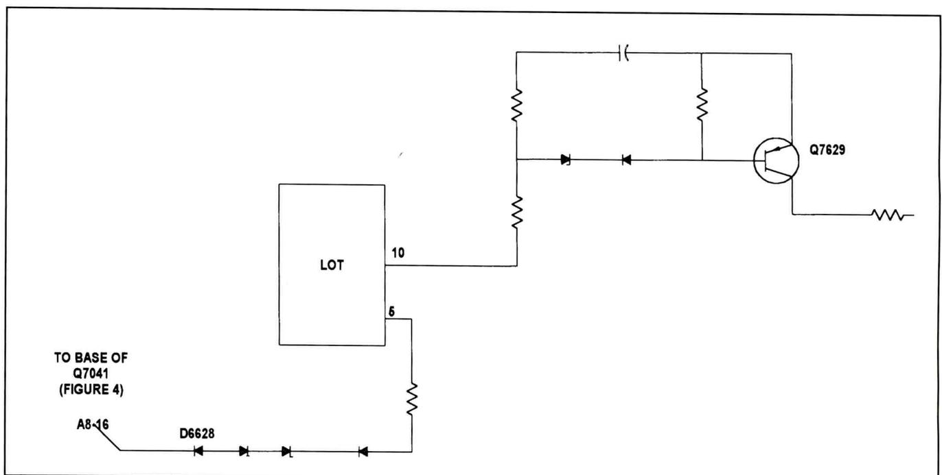
**Figure 1.** Under normal operating conditions, the voltage on the base of 7629 is just slightly negative. But it swings increasingly negative as the CRT draws more current. If the voltage swings sufficiently negative, transistor 7629 turns on, activating the circuit, and the TV shuts down.
