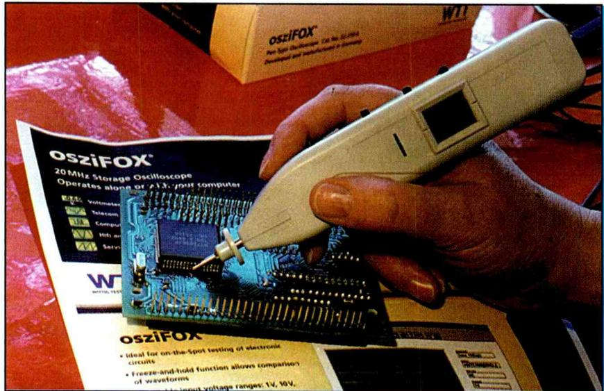
This oscilloscope is small enough to fit in a technician's pocket, and provides a 5Mhz bandwidth.
