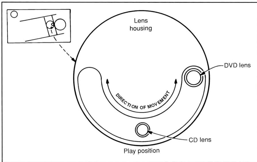
**Figure 2.** Some DVD players utilize two optical pickups, one to play audio CDs and another to play DVDs. The Magnavox player uses one optical block equipped with two lenses to achieve the same purpose.
