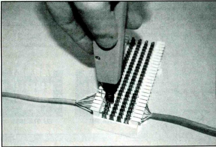
**Figure 4.** A 66 block. This type of connecting block is most often used for telco.
