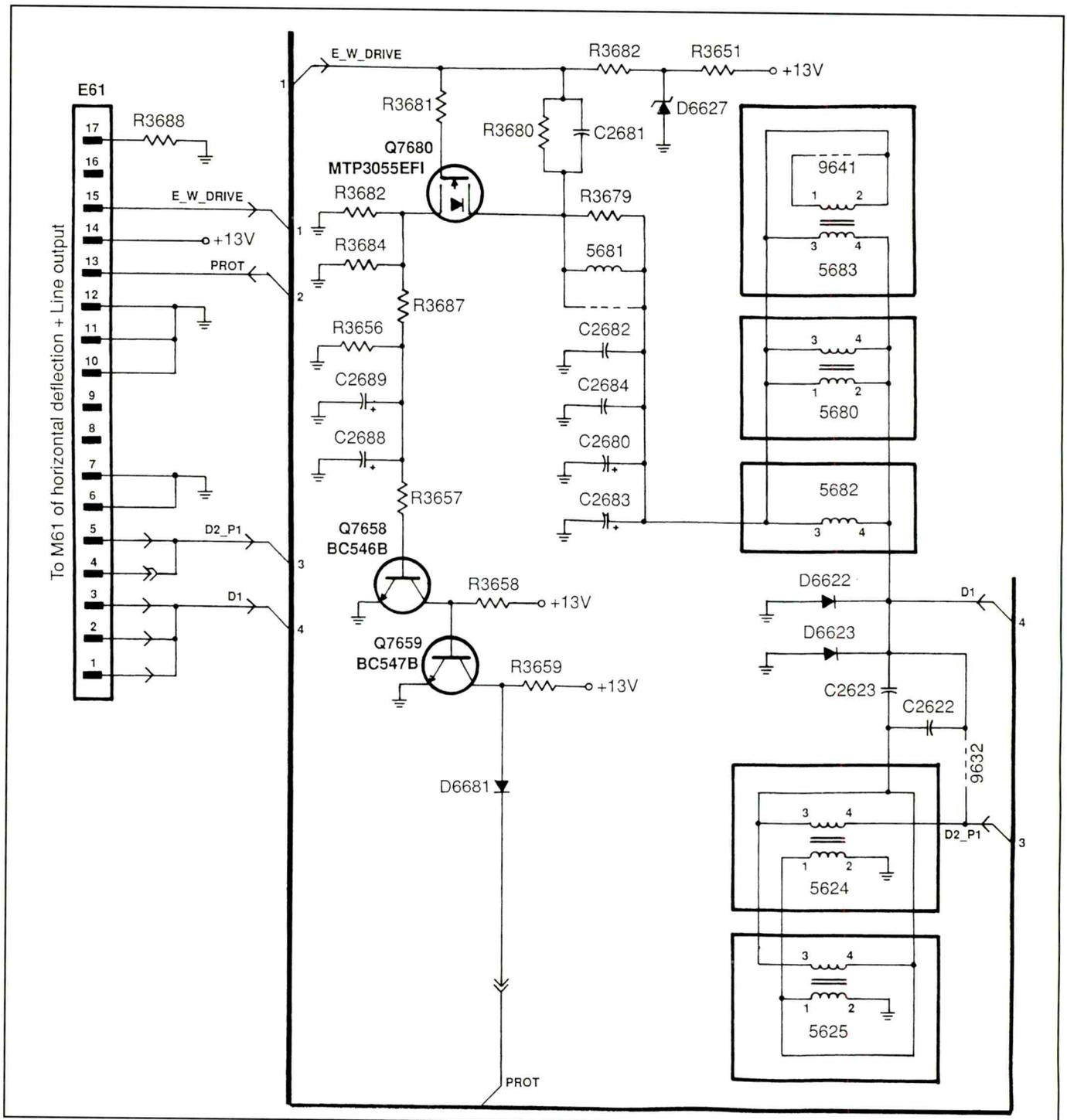
**Figure 5.** Transistor 7680 on the E-W panel monitors horizontal drive. If horizontal drive fails, 7680 turns on permitting transistor 7658 to turn on, which causes transistor 7659 to turn off. Resistor 3959 then applies a dc voltage to the protection line that turns on transistor 7041(Figure 4) which pulls pin 11 of the microprocessor low, and shuts down the set.
