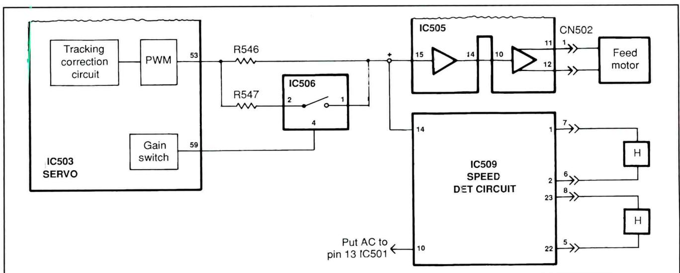
**Figure 4.** Feed motor drive from the tracking correction circuit inside IC503 is routed to a PWM (pulse width modulator) and sent out of pin 53 on its way to pin 15 of IC505, the feed motor drive IC. If you are watching a DVD, the drive goes through R546 before it reaches IC505. If the disk needs to be speeded up, the gain switch inside IC503 turns on IC508 switching R547 in parallel with R546 to increase the gain of the signal.
