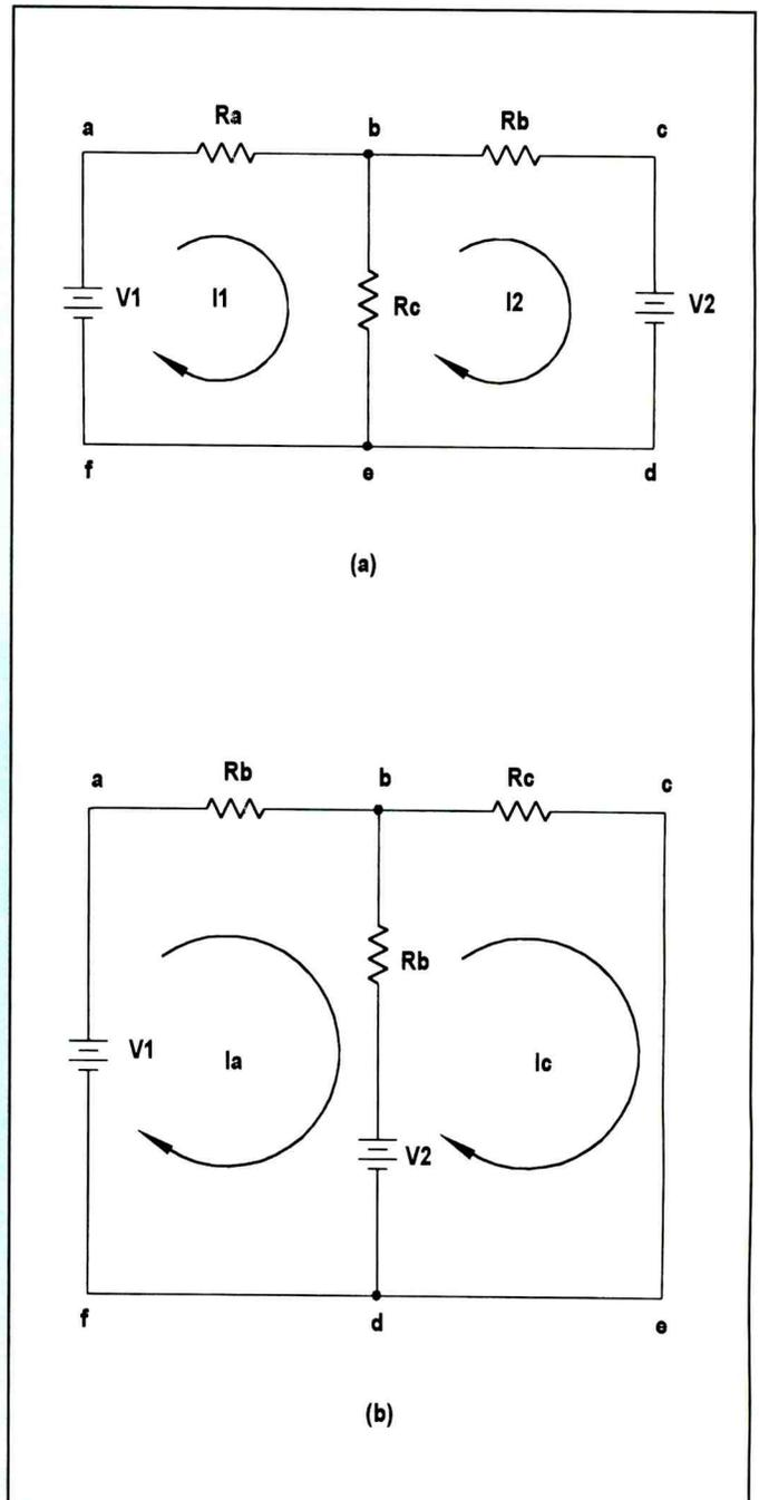
**Figure 1.** If you are going to use Maxwell's loop equations in Figure 1(a) to solve for the current through  $R_C$ , you must first solve for  $I_1$  and  $I_2$ . Then you must subtract those currents to get the value of  $I_C$ . However, if you move branch b to the outside, as shown in Figure 1(b), you only need to solve for one current ( $I_C$ ) to get the current ( $I_C$ ) through  $R_C$ .
