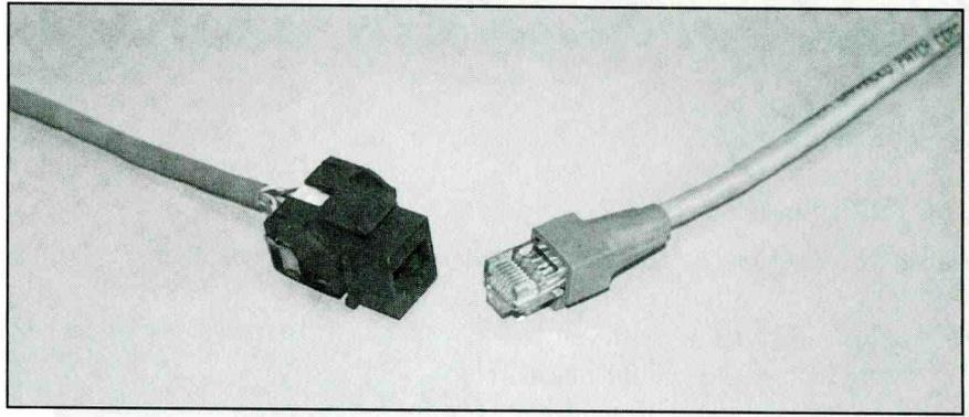
**Figure 2.** RJ45 is the popular name of the modular 8 pin connector used with UTP cable in structured cabling systems.
