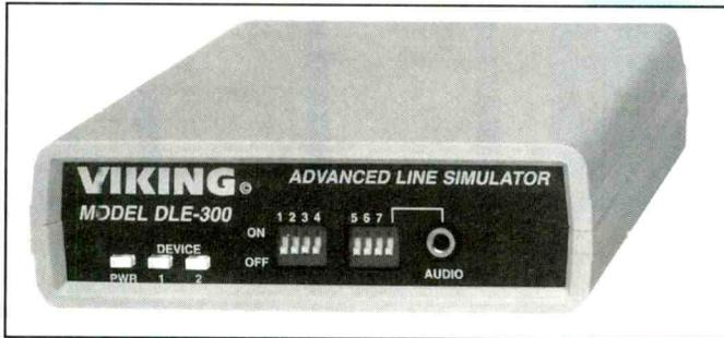
The simulator also provides instant point-to-point communication with ring-down notification. As soon as one connected phone goes off-hook, it immediately rings the other phone.
