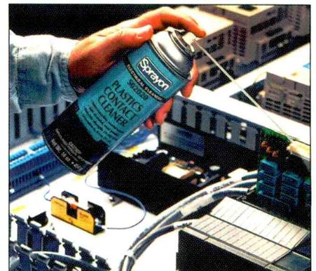
tronic contacts. It is a non-flammable, non-corrosive, non-staining cleaner that is safe on virtually all plastics. Its non-ozone-depleting formulation is an alternative to TFI13. The cleaner removes light contaminants without leaving a residue and without causing temperature control problems. According to the manufacturer, it can be applied while equipment is operating because it instantly evaporates.
