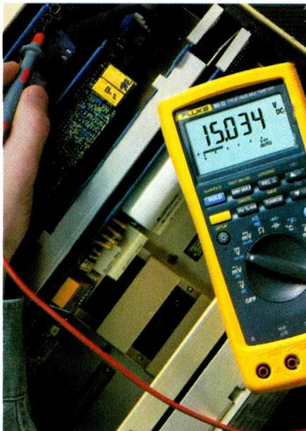
time stamping features with a real-time clock. Expanded capacitance ranges to 50mF provide a wide range of measurement reading for technicians and engineers working on power supplies and other equipment.
