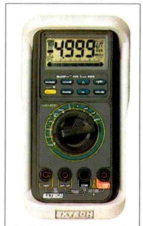
allow the user to collect, display, plot, save, or export data or graphs. Measurements are displayed on a backlit 5000 count LCD with high resolution: 0.01mV, 0.1µA, 0.10ohms, 0.01nF, 0.001Hz. Features also include a wide (voltage bandwidth of 40Hz to 20kHz, smart Auto Power Off which is disabled if
