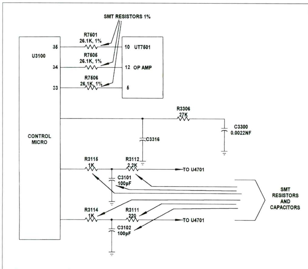
Figure 1. These are some of the critical SMT resistor chips found in the system control circuits.
