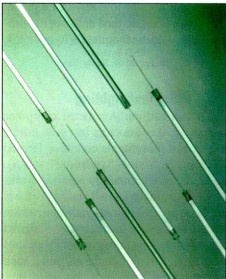
The bright white lamps incorporate special phosphors which enhance visible illumination to 26,000 cd/m<sup>2</sup> levels and the UV lamps have a spectral distribution ranging from 300 nm to 400 nm with a peak wavelength of 350 nm.
