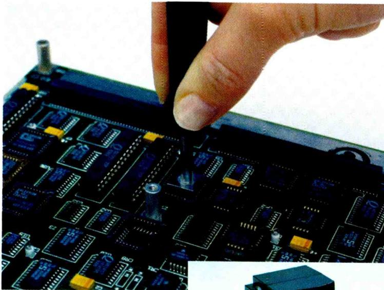
but are incapable of high precision direction. Because there is no direct contact between tool and joint, heat direction is not "self-locating." But, non-contact means the risk of pad damage is minimal. The need to set air flow rates and temperature (and not just temperature) makes optimizing the tool in operation more difficult. High air flow rates can cause solder balls to be blown across the PCB. Reflow of adjacent components must be guarded against.
