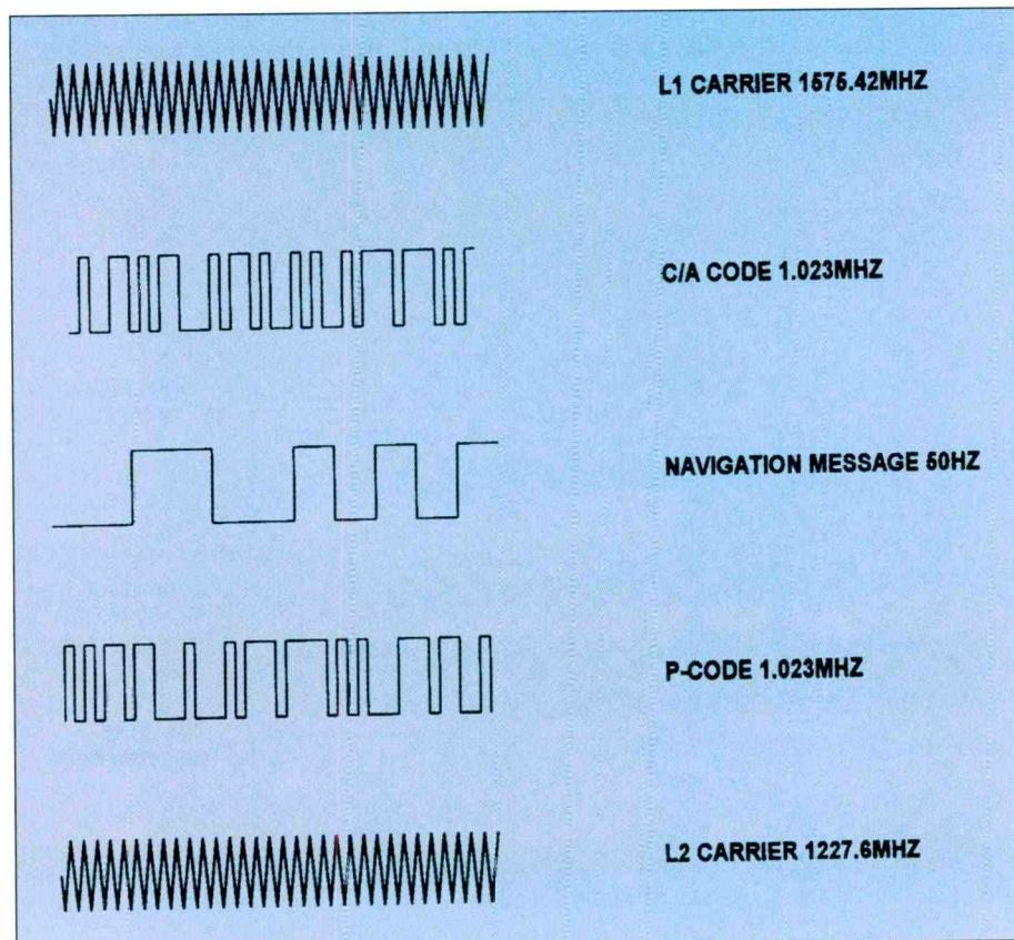
Figure 1. The satellites transmit two microwave carrier signals called L1 and L2. While the 1575.42 MHz L1 signal carries the navigation message and the SPS code signals, the 1227.60 MHz L2 frequency measures ionospheric delay.
