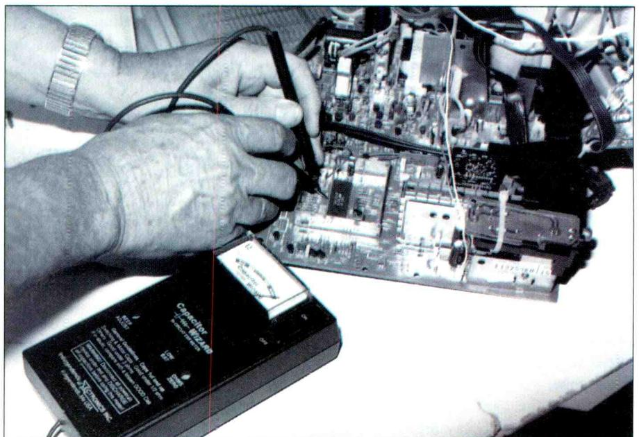
**Figure 7.** Check each pin terminal of IC or microprocessor with the ESR meter to insure a good soldered connection.
