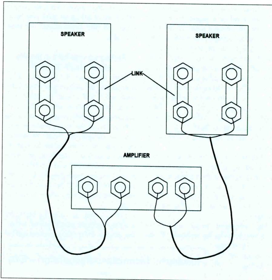
Figure 5. Speakers designed so that they can be connected in a bi-wire arrangement come from the factory with a connecting link between the terminals so they can be wired normally, as shown here.
