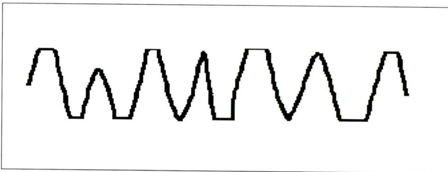
Figure 2. If we take the same music as that represented in Figure 1 and try to reproduce it at a level greater than the amplifier is capable of (clipping), we get something like this waveform, which looks more like a group of square waves than a sinusoid. Square waves contain large amounts of high frequency information, which can destroy tweeters.
