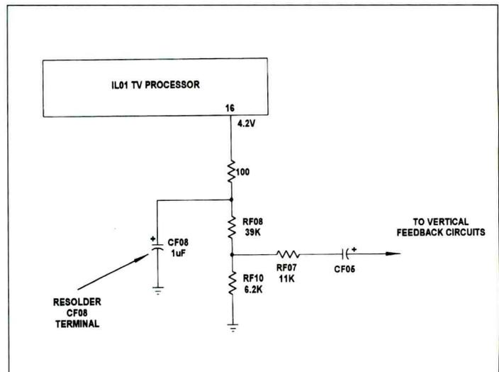
Figure 9. A faulty soldered terminal of CF08 produced insufficient vertical sweep symptom in the RCA TX82 chassis.
