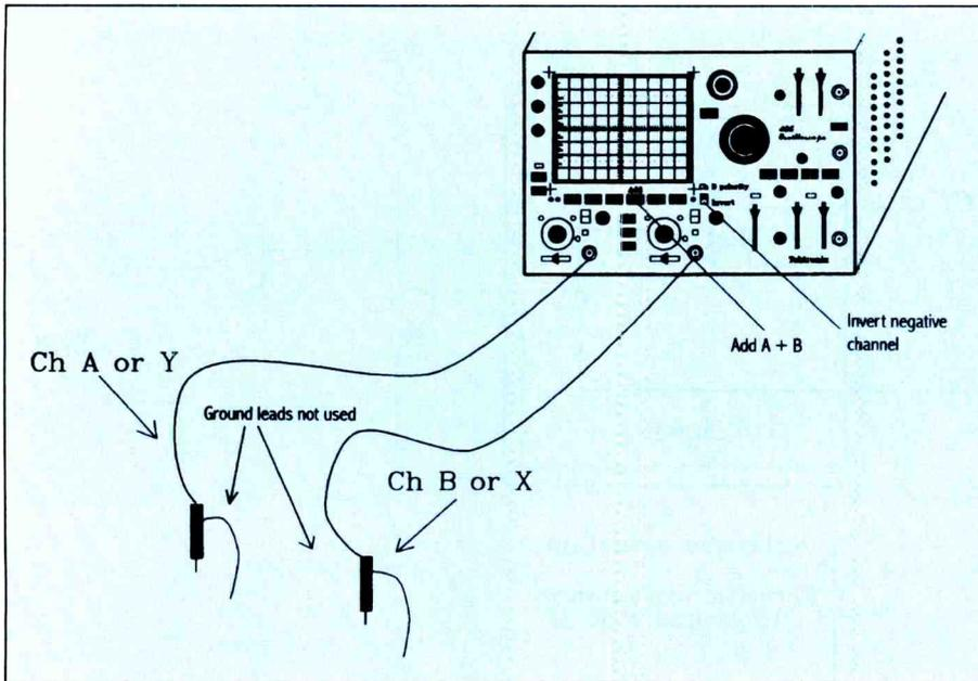
Figure 7. Quasi-differential mode and setup.
