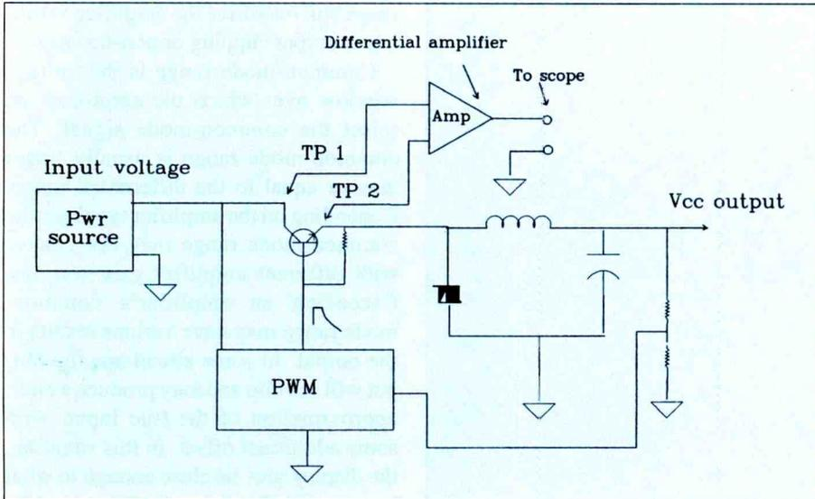
Figure 3. Switching supply connected to a differential amplifier.
