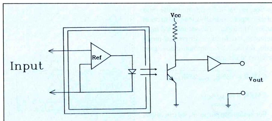
Figure 6. Diagram of isolation probe.
