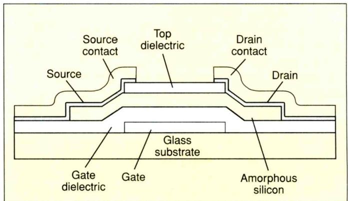
Figure 27. Inverted gate, amorphous silicon TFT.
