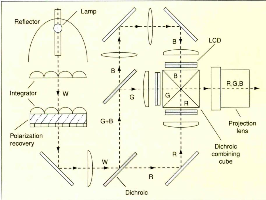
Figure 28. Transmissive LCD projector.
