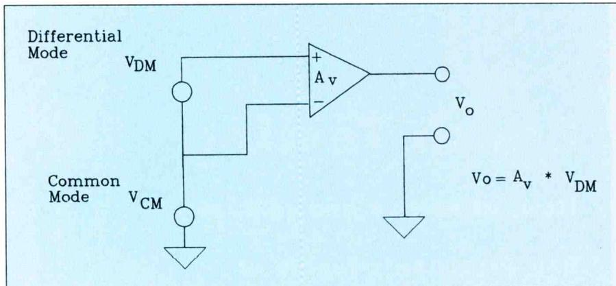
Figure 1. Diagram of differential amplifier with input signals.
