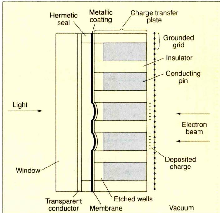
Figure 32. Membrane light modulator.
