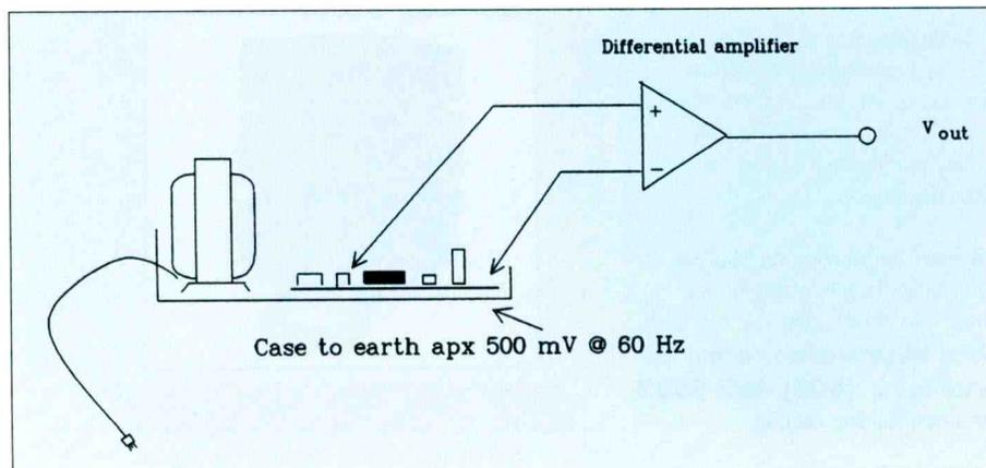
Figure 2. Differential amplifier measuring on a floating ground.
