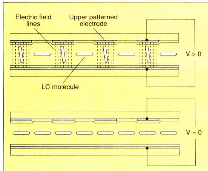
Figure 30. Diffraction grating LCD (one pixel).
