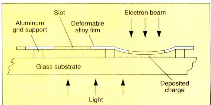
Figure 31. Metal membrane target.
