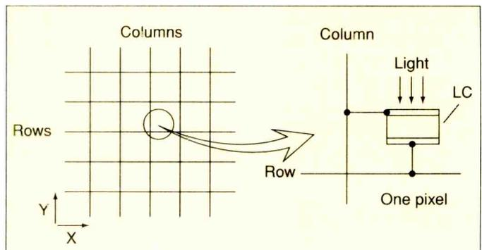
Figure 25. Passive-matrix address method.
