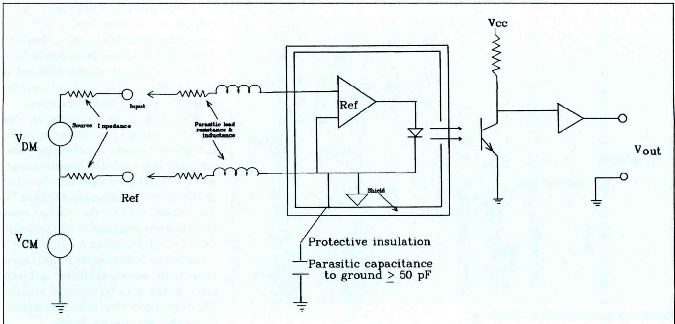
Figure 9. Isolation amp with unequal input capacitance.
