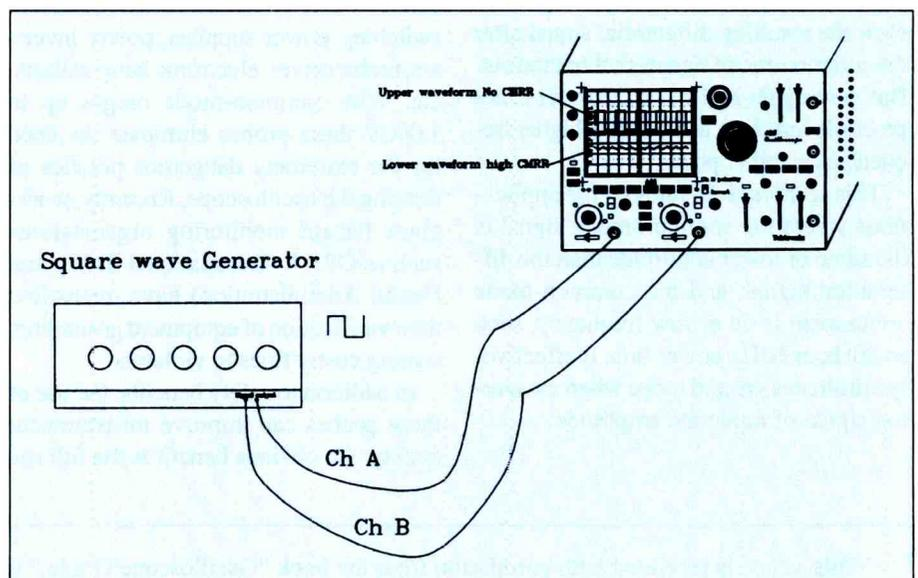
Figure 8. Oscilloscope inputs to square wave generator maximizes CMRR in both input channels for quasi-differential mode.
