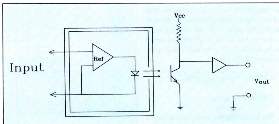
Figure 6. Diagram of isolation probe.
