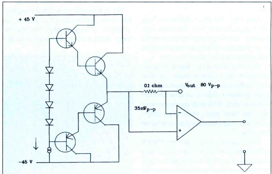
Figure 4. Common-mode error from a differential amp with 100,000 CMRR.
