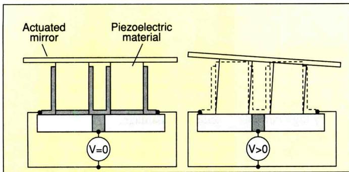
**Figure 34.** Actuated Mirror Array concept (bulk approach).
