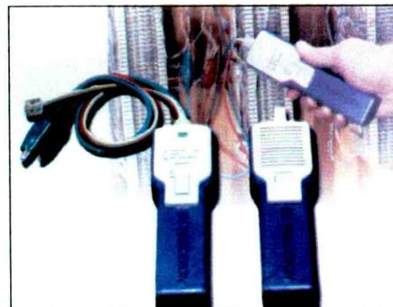
The Model 261 Cable Tracer is hand-held inductive tracer that will help to identify wires without piercing the insulation. It features a Hi-gain, Hi-impedance amplifier and is capable of identifying tones from a distance of up to 12 inches. It can trace Tone Generator signals through dry wall, wood and many other non-metal surfaces (under ideal conditions) and features a rugged, moisture resistant Mylar cone speaker.
