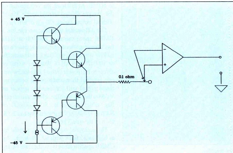
Figure 5. Empirical test for adequate common-mode rejection.
