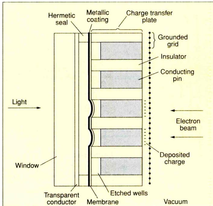
Figure 32. Membrane light modulator.
