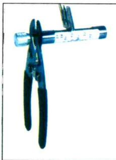
an easy to use dial mechanism, which will move the blade along post to vary shiner (strip-off) length.
