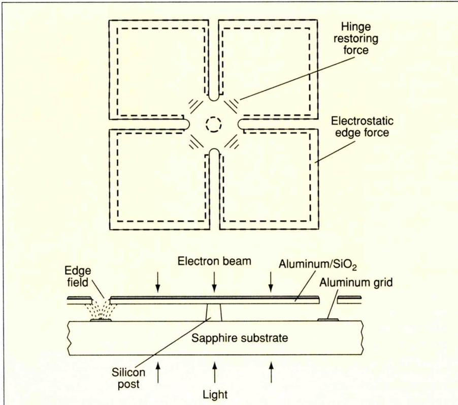
Figure 33. Target of Mirror Matrix Tube (one pixel).
