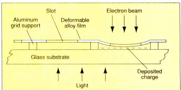
Figure 31. Metal membrane target.
