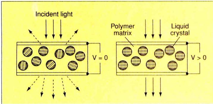
Figure 29. Polymer-dispersed liquid crystal.
