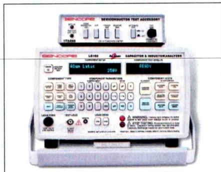
itor's performance at the component's working voltage. The system measures capacitors for value and equivalent series resistance both in and out of circuit eliminating the need for removing the component from the circuit to make the test.
