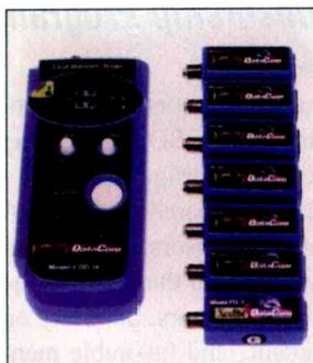
handset. The lead from the tester is simply plugged into a phone jack and if the jack tests OK, the user knows that the problems is in the handset, so a service call to the phone company is unnecessary. Helpful to homeowners but also useful to installers, contractors or electricians working in a home or small business where a number of phone lines are being tested.
