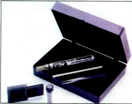
and re-establish the solder spheres on the ball grid array. Therefore, you are able to reuse your components. Each kit contains the Reballer fixture, 10,000 solder spheres of the correct size, flux, tweezers, and a tool to seat the solder spheres. The Reballer Kits are also available for chop scale and flash memory devices.
